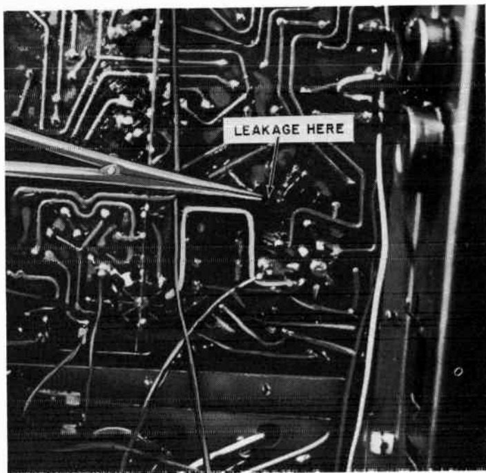
Fig. 410. Leakage paths are not easy to find. Look for accumulation of solder flux, dust and discolored phenolic. Overheated or burned phenolic is carbon. This must be scraped or cut away to eliminate leakage path.
