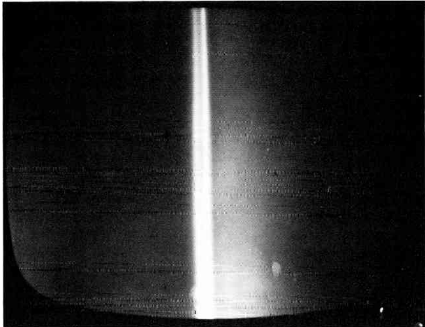
Fig. 606. Overdrive appears as a vertical white line in the raster. It can be used to help set the drive control.
