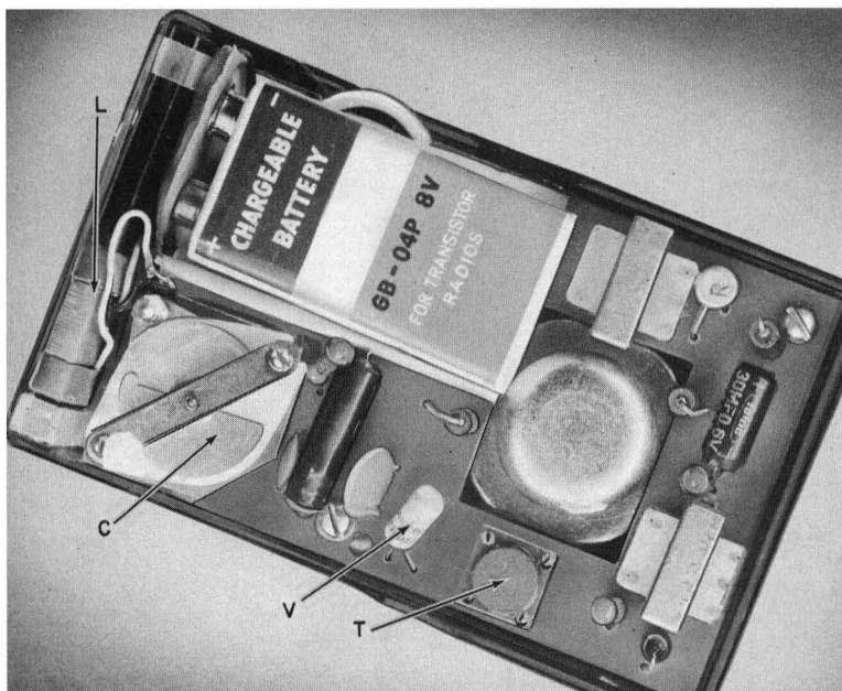
Fig. 424. The printed-circuit board of a two transistor reflex receiver is not very crowded.
