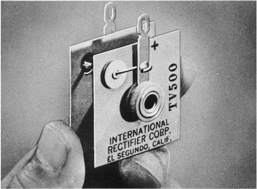
Fig. 114. Silicon rectifier designed to replace 500-ma selenium rectifier stack. Fins help to dissipate heat. (International Rectifier Corp.)
