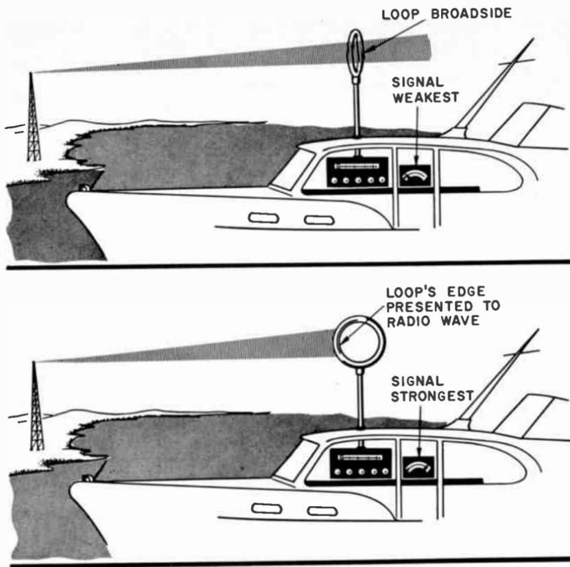
Fig. 705. The received signal is strongest when the edge of the loop points toward the station.
