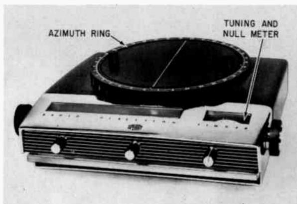
Fig. 708. All-transistorized small RDF designed for three-band reception. Separate ferrite antenna windings are used for long wave beacon, standard broadcast and marine bands. A sensitivity control adjusts for weak or strong signals from beacons or stations and aids in obtaining the best null when rotating the loop antenna for a bearing. (Sperry Piedmont Co.)
