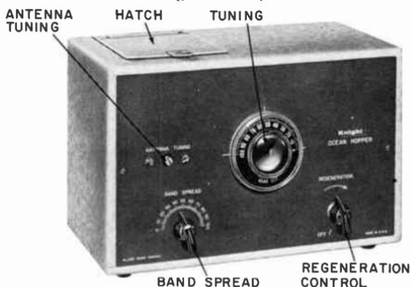
Fig. 204. This is a "build-it-yourself" three-tube radio, available in kit form. It will receive marine frequencies. (Allied Radio Corp.)
