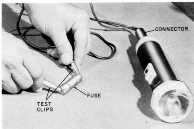
Fig. 415. A continuity checker is a special flashlight equipped with two wire leads. If the fuse being tested is good, the light will glow. (Ray-O-Vac Co.)
