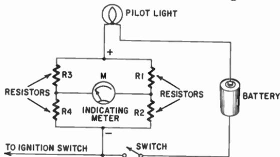
Fig. 512. Circuit diagram of a fuel-vapor detector.
