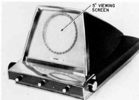
*Fig. 712. Radar unit has cursor and azimuth rings, enabling the pilot to obtain relative bearings of other vessels and objects within range of the radar. This photo shows the indicator only. The antenna unit mounts above deck and contains the radar transmitter and receiver. (Sperry Piedmont Co.)*
