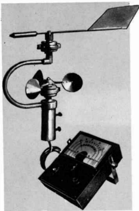
Fig. 508. *Wind velocity and direction indicator gives direction and velocity on one dial, indicating from 0 to 100 miles per hour. (Lafayette Radio)*
