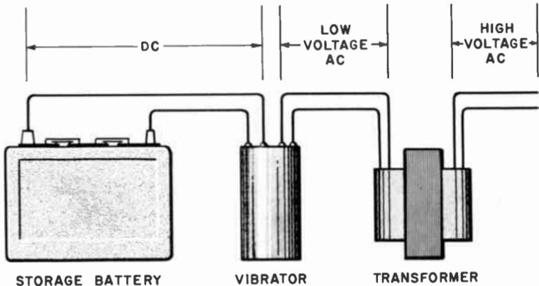
Fig. 402. A vibrator changes dc to ac. The transformer steps up low-voltage ac to higher-voltage ac.
