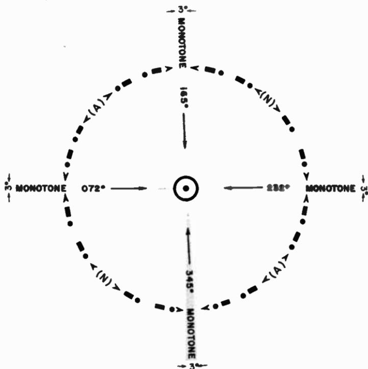
Fig. 703. An aeronautical beacon sends out a beam in four directions. The beam sounds a steady tone in the receiver. Between the beams the Morse letter A or N is heard.
