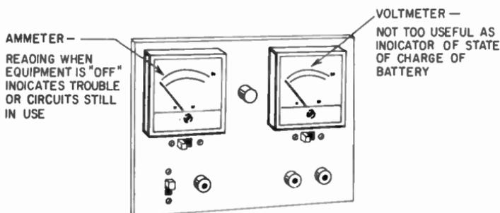
*Fig. 411. The correct voltage of a battery can only be measured when the battery is "under load" — that is, when it is delivering current to equipment. The position of the ammeter needle is an indication of whether the battery is charging or discharging.*
