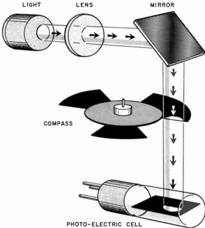
Fig. 506. The heart of the automatic pilot is a unit consisting of a magnetic compass and an electric eye to watch it.
