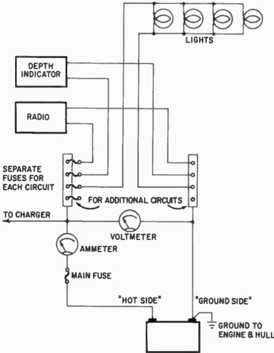
Fig. 410. Typical wiring diagram for lights and accessories on a small boat. Wires to each device would actually be twisted together instead of parallel as shown.
