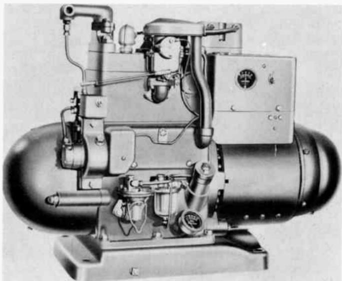
*Fig. 407. If you expect to bring all of your electric appliances along when you go boating, you may need a power plant like this. Gasoline-driven and water-cooled, this outfit supplies 3,000 watts of power at 110 volts ac. Some machines also supply dc for keeping a battery charged. (D. W. Onan & Sons, Inc.)*
