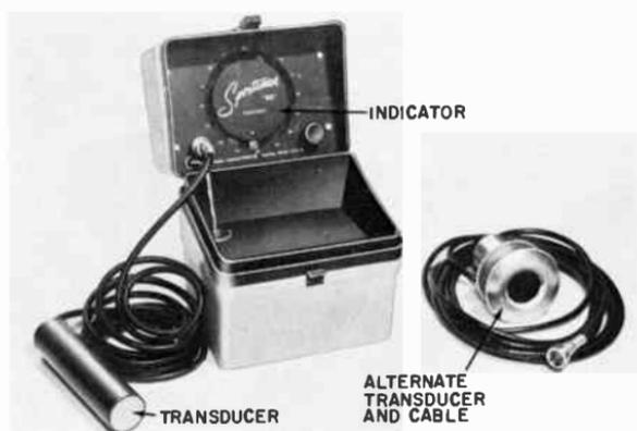
*Fig. 607. A completely self-contained depth indicator. The case and indicator can be set up anywhere on board the vessel, and the transducer placed over the side, below the water line.*
