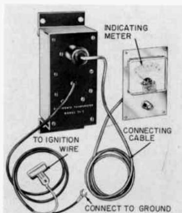
Fig. 513. An electronic tachometer. It registers the engine speed in revolutions per minute. (Heath Co.)
