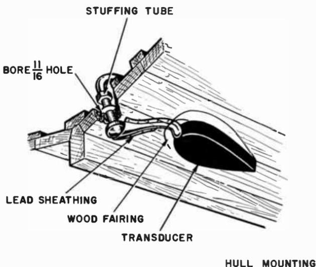
Fig. 603. The transducer for a depth indicator may require a streamlined block or "fairing" to mount it to the hull. (Bendix)
