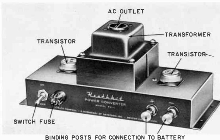
*Fig. 409. Up to 200 watts of 110-volt ac power can be obtained from your storage battery by means of a converter like this. It uses two transistors to change the battery power from dc to ac, and a transformer to step the voltage up to 110. (Heath Co.)*
