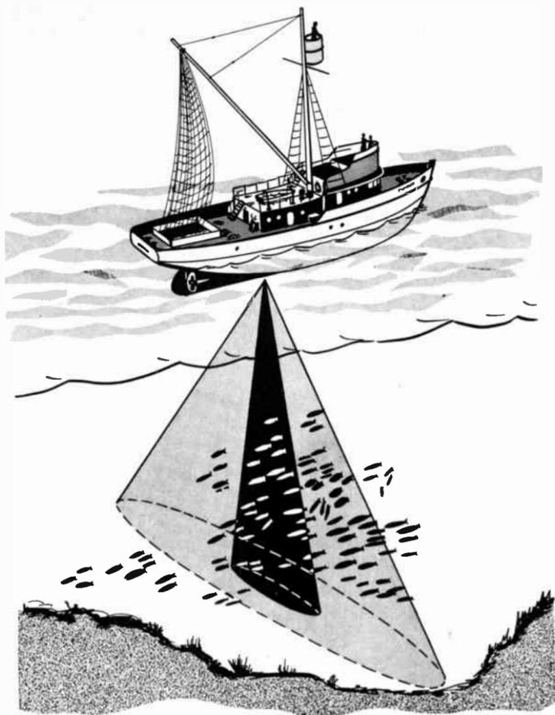
*Fig. 609. A dual sweep beam on a depth recorder permits the use of a narrow beam for navigation and a wider one for finding schools of fish.*
