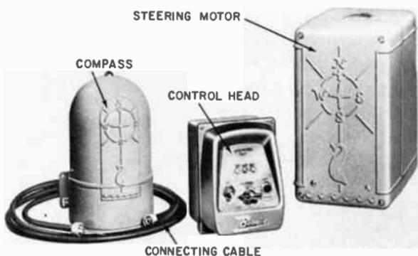
Fig. 507. The three essential units of the automatic pilot are the compass, the control head and the steering motor. (Bendix)
