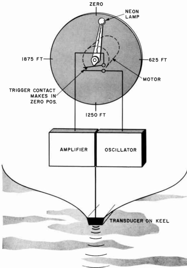
Fig. 602. Diagram of a depth indicator. The indicating portion (top) consists of a motor-driven arm which carries a neon lamp around a dial.
