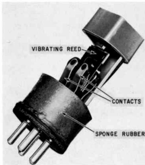
Fig. 403. Inside view of a vibrator.
