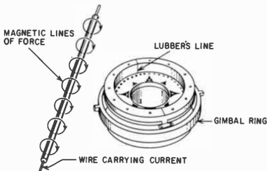
Fig. 502. The magnetic fields around wires carrying electrical currents will affect a magnetic compass if close enough to it.
