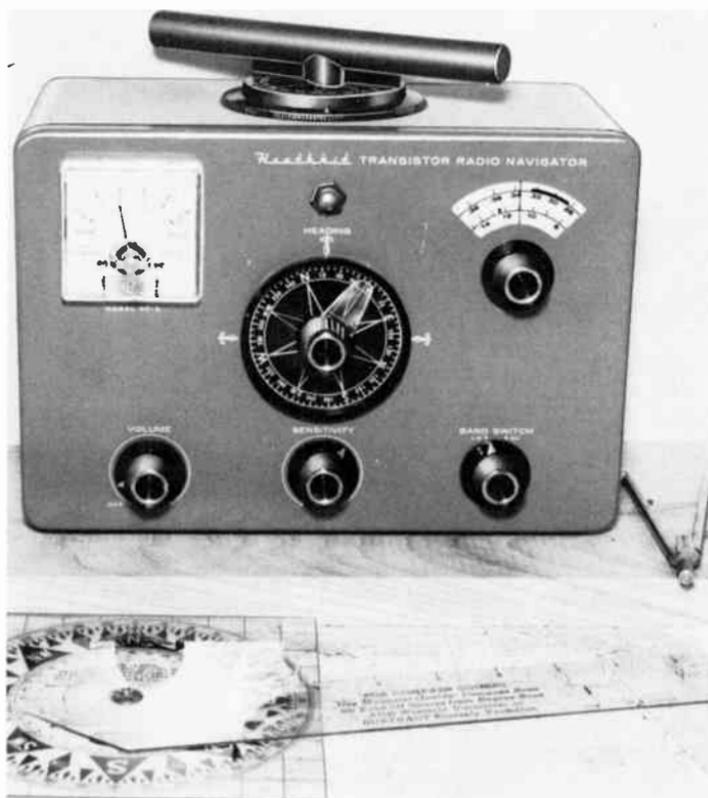
Fig. 709. Setup for navigation: a direction finder, chart and course protractor. (Heath Co.)
