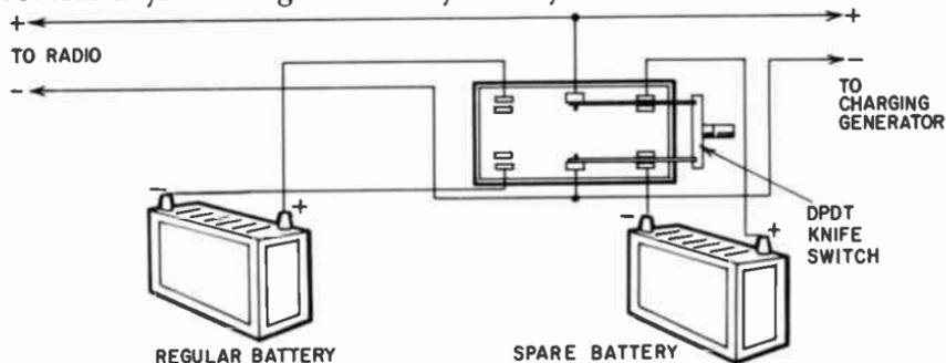
Fig. 406. A fully charged spare battery is nice to have along. If the regular battery runs down, the spare can be connected in its place. A double-pole double-throw knife switch is needed, connected as shown. Note that the charging generator (driven by the boat engine) is connected across the battery in use. The generator cannot normally take care of both batteries. When back to shore, the dead battery can be recharged.
