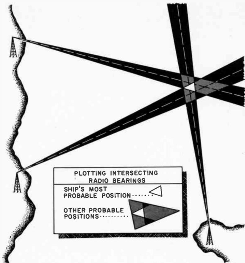
Fig. 710. *Direction finding by means of three shore stations.* (US Navy Hydrographic Office Publication No. 205)
