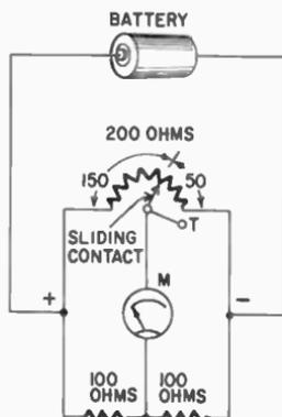
carbon offers more resistance to electric current than does copper. Thus, in the drawing shown, the zig-zag lines are resistors made of carbon, while the straight lines are wires made of copper.
