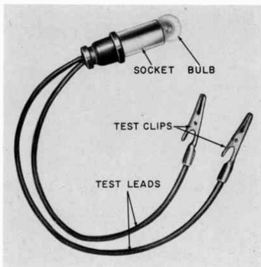
Fig. 413. A "trouble lamp" consists of a lamp, a socket and two wires equipped with clips.
