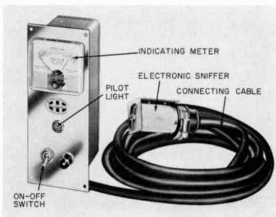
*Fig. 511. A fuel-vapor detector. It consists of an electronic sniffer on one end of a cable, and an indicating instrument on the other.*
