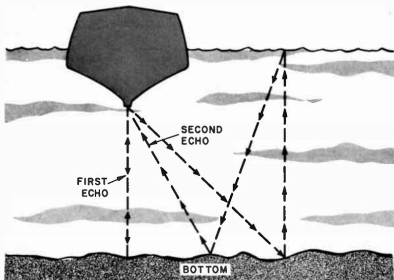
Fig. 605. Multiple reflections cause second echoes which give false indications of depth.
