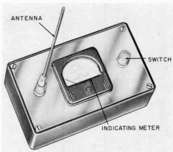
*Fig. 311. An instrument for measuring the power radiated from a radio antenna. When held near a ship's antenna, the meter will give an indication when the transmitter is turned on. (Heath Co.)*
