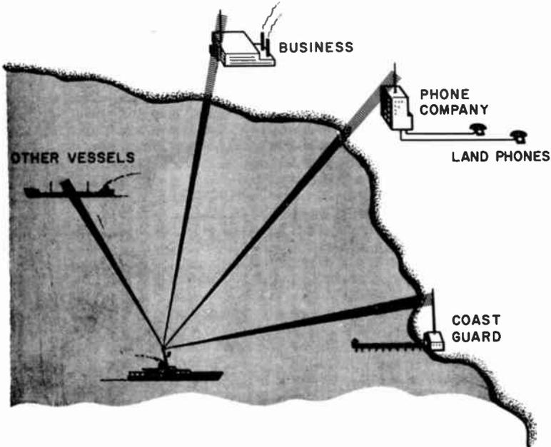
Fig. 104. Marine radio can be used to enable the boat owner to talk to other vessels, a business establishment, the telephone company and to land phones, or to the nearest Coast Guard station.
