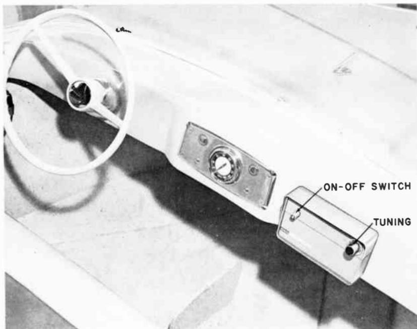
Fig. 202. This is a portable radio receiver which can be fastened in a boat or removed for use on shore.
