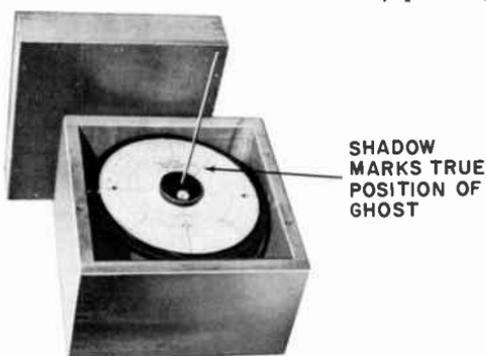
Fig. 504. *The DARRA compass corrector uses the shadow of a vertical wire on a circular card to mark the position of the boat while directions are being checked. (Darrach Co.)*
