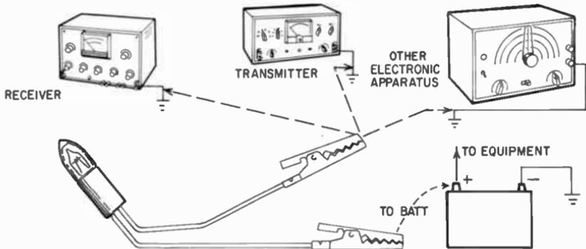
Fig. 414. Method for checking the ground connections of all electronic apparatus.
