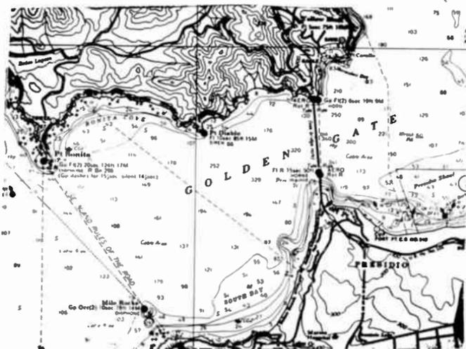
Fig. 701. A mariner's chart showing the entrance to San Francisco Bay. The depths of the water and various aids to navigation are also shown.
