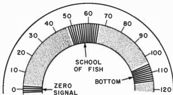
Fig. 606. The flashes of light, represented here by the radial lines, show the zero signal, a school of fish and the bottom reflections.
