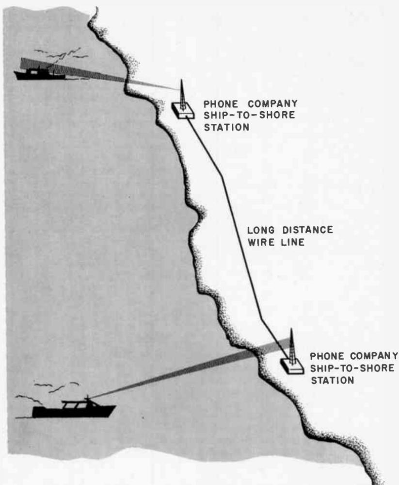
*Fig. 304. Ships that are too far apart to communicate directly may hold a conversation by means of telephone-company shore stations and connecting land lines.*
