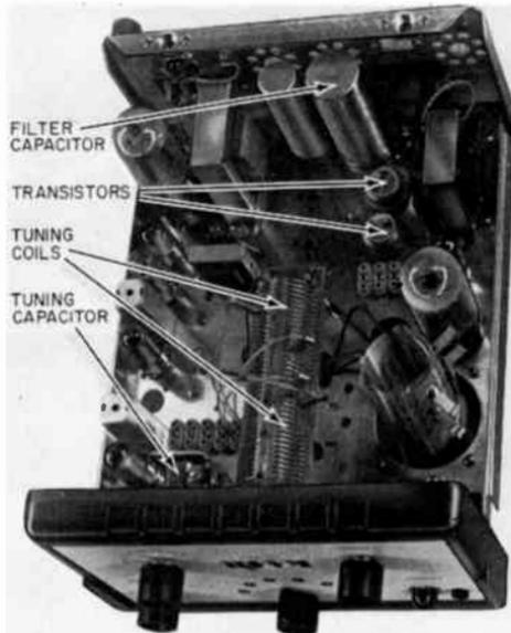
Fig. 312. The inside of a marine radio transmitter looks just about like any other radio set. However, any repairs, even changing the tubes, requires that the repairman hold an FCC second class radiotelephone operator's license. (Kaar Engineering Corp.)
