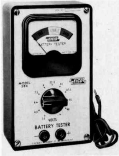
Fig. 412. A battery tester is a handy unit for getting a quick indication of the condition of a battery. Courtesy Eico.
