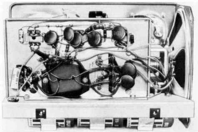
*Fig. 707. Inside view of portable receiver for broadcast- and radio-beacon frequencies.*
