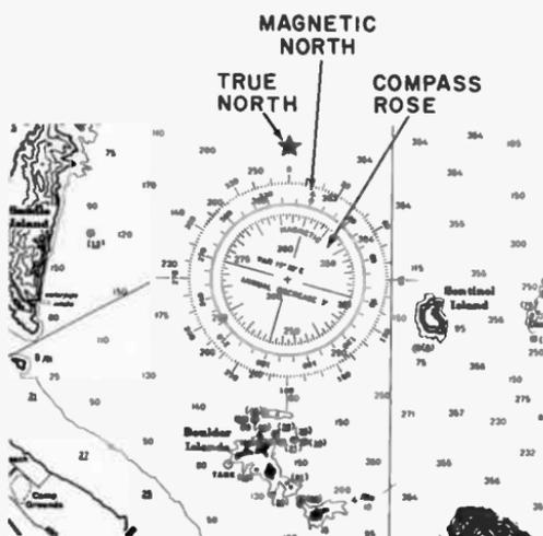
Fig. 501. A portion of a US Coast and Geodetic Survey map of Lake Mead, showing the compass rose. This shows the magnetic North to be  $15^{\circ} 30'$  east of the true North.
