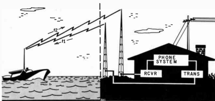
Fig. 303. Duplex operation is more like normal conversation. Both parties can talk at the same time.
