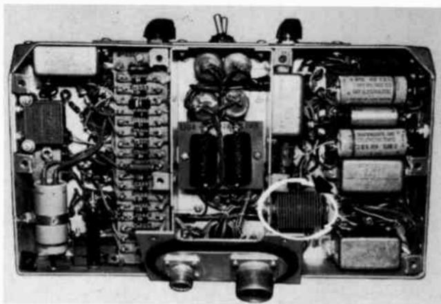
Fig. 404. The rectifiers used in receivers and transmitters are either vacuum tubes, selenium or silicon units, or synchronous vibrators.
