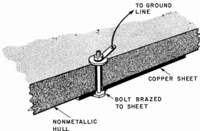
Fig. 309. Method of setting up a good ground.
