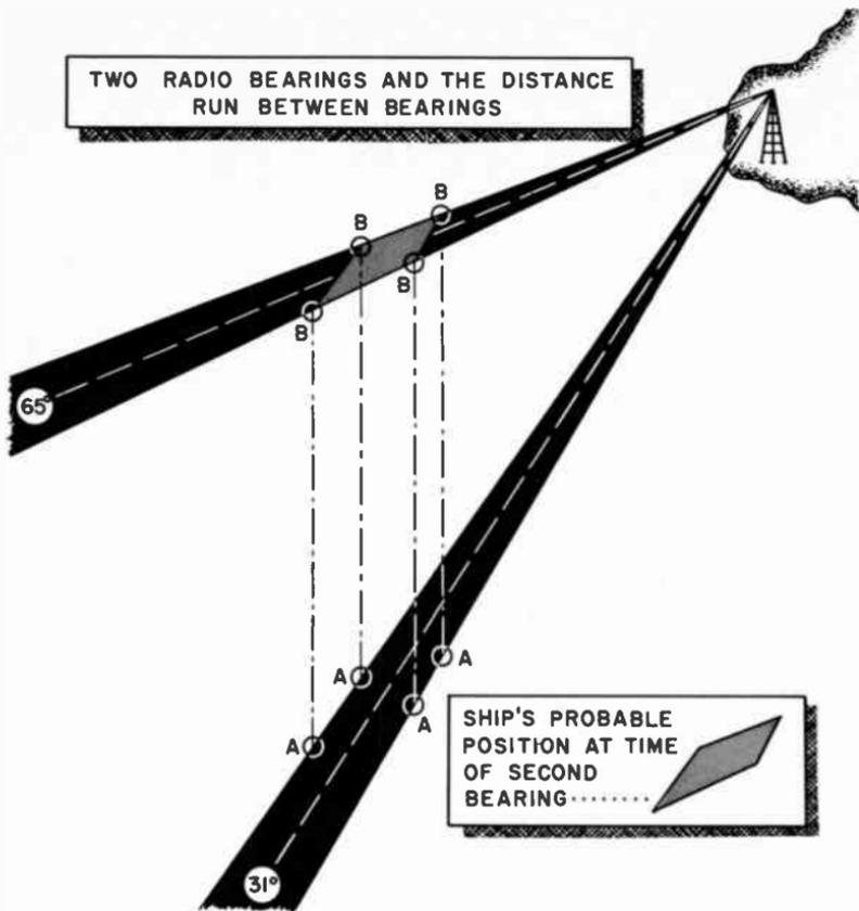
Fig. 711. Direction finding by means of one shore station. (US Navy Hydrographic Publication No. 205)
