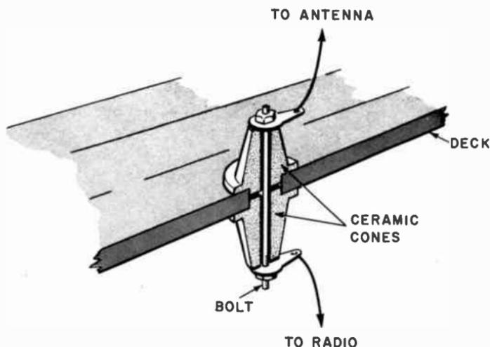
Fig. 308. A feedthrough insulator is used when the lead wire must go through the deck.
