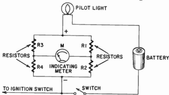
Fig. 512. Circuit diagram of a fuel-vapor detector.
