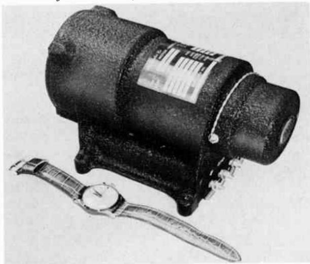
*Fig. 405. The input to a dynamotor is low voltage dc, usually 12 volts. The output is also dc, generally several hundred volts.*
