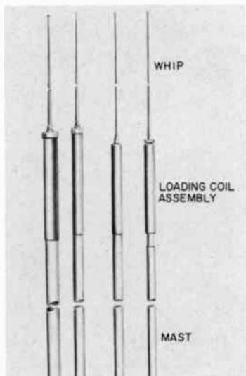
*Fig. 307. Marine radio antennas consist of a mast, a loading coil and a whip. The loading coil, contained in the large cylinder in the center of the assembly, has the electrical effect of lengthening the antenna. (Webster Manufacturing Co.)*
