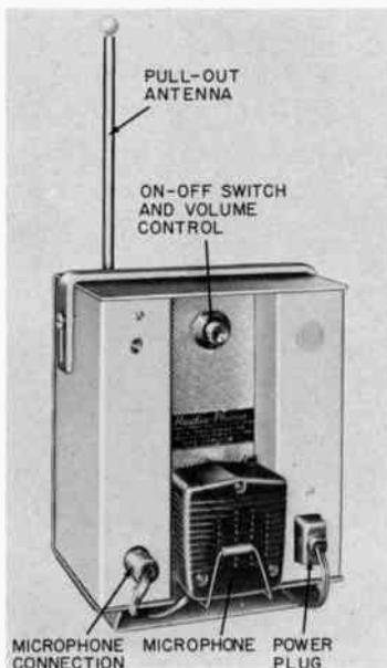
*Fig. 105. A Citizens' radio for use in the 27-mc band. It can be used in marine or land service. (RCA)*
