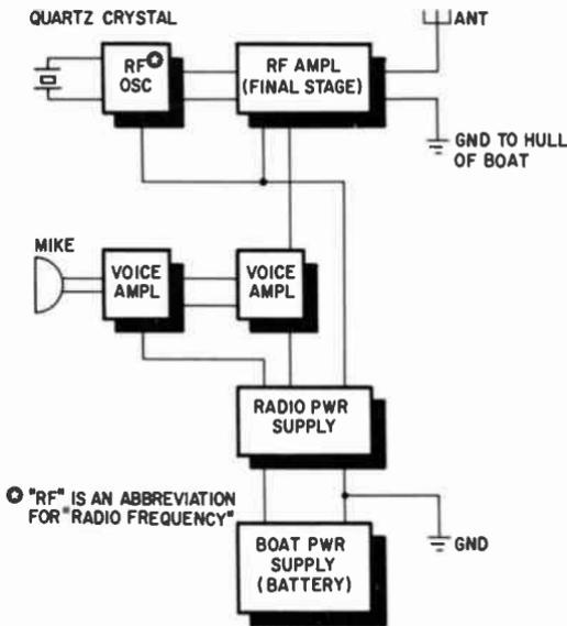
Fig. 301. Block diagram showing the principal parts of a marine transmitter. The amplifiers shown consist of vacuum tubes and associated wiring.
