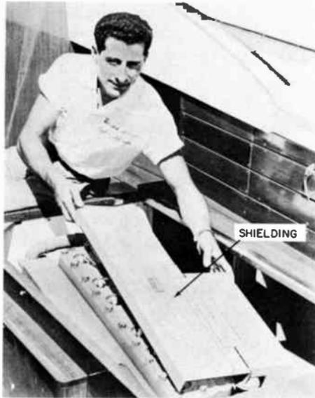
*Fig. 416. A marine engine may require a shield to eliminate noise in the radio. This one is called a Tiffany Spark-shield. (Pearce Simpson, Inc.)*
