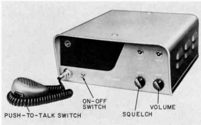
Fig. 310. This transmitter-receiver covers a band of frequencies from 450 to 470 megacycles.
