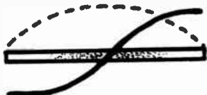
In a half-wave antenna, the voltage (continuous line) is maximum at the ends: current (dotted line) is minimum. The voltage is zero at the center where the current is maximum. However, the voltage has its maximum rate of change at the center. The lead-in comes from the center where the current is maximum.
