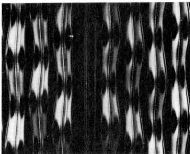
Fig. 506. Microphotographs of grooves in 45/45 stereo records. (Westrex Corp.)
