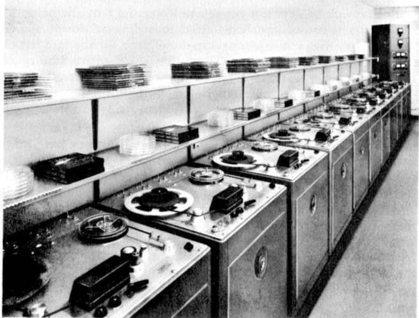
Fig. 405. Duplication of tapes for commercial release is cumbersome and time-consuming, resulting in high retail prices. The master unit at the far right feeds a maximum of ten "slave" recorders, running at 60 ips, and takes four minutes to duplicate a standard 1200-foot reel of tape. (Ampex)
