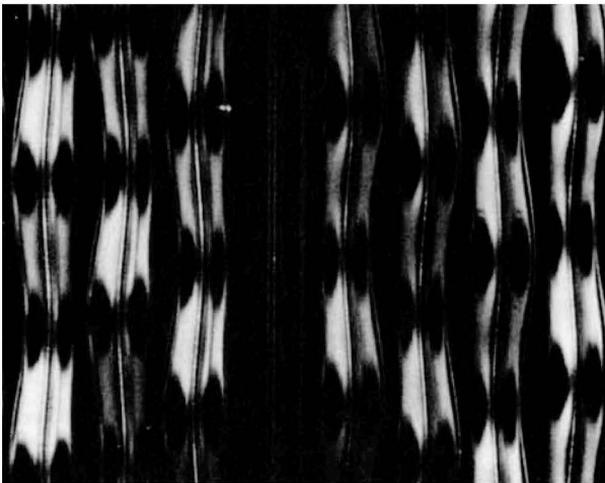
Fig. 506. *Microphotographs of grooves in 45/45 stereo records. (Westrex Corp.)*
