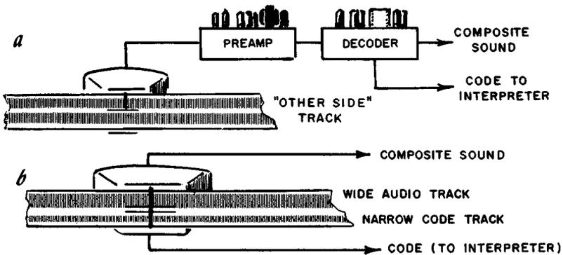
Fig. 403. Coded stereo can be reproduced by using a single coded track (a) or a wide audio track and an accompanying narrow code track (b).
