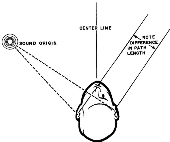
Fig. 103. Origin of path-length differences due to sound source off median line.
