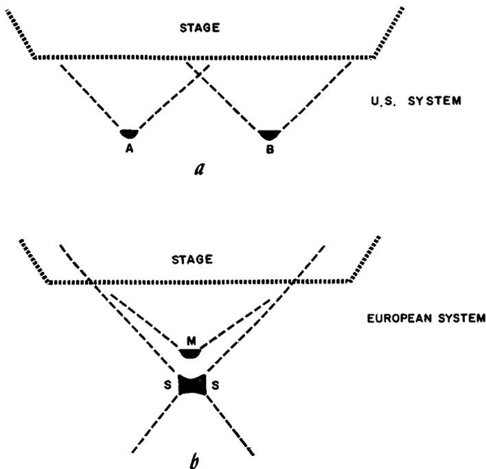
Fig. 701. Domestic and foreign methods of microphone placement.
