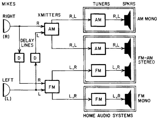
**Fig. 619.** Similar to the Bell simulcasting system, the Becker method also utilizes time delay circuitry and can be used in several combinations of transmitting media, including FM multiplex.
