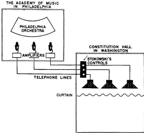
Fig. 211. *Simplified diagram of the Bell Telephone Laboratories three-channel "broadcast".*
