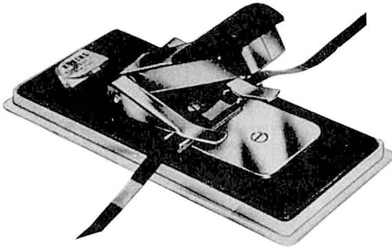
*Fig. 408. A popular tape splicer which cuts slightly into finished splice for a "wasp-waist" effect. The splice made this way will pass smoothly and quietly over the tape heads. (Robins Industries, Inc.)*
