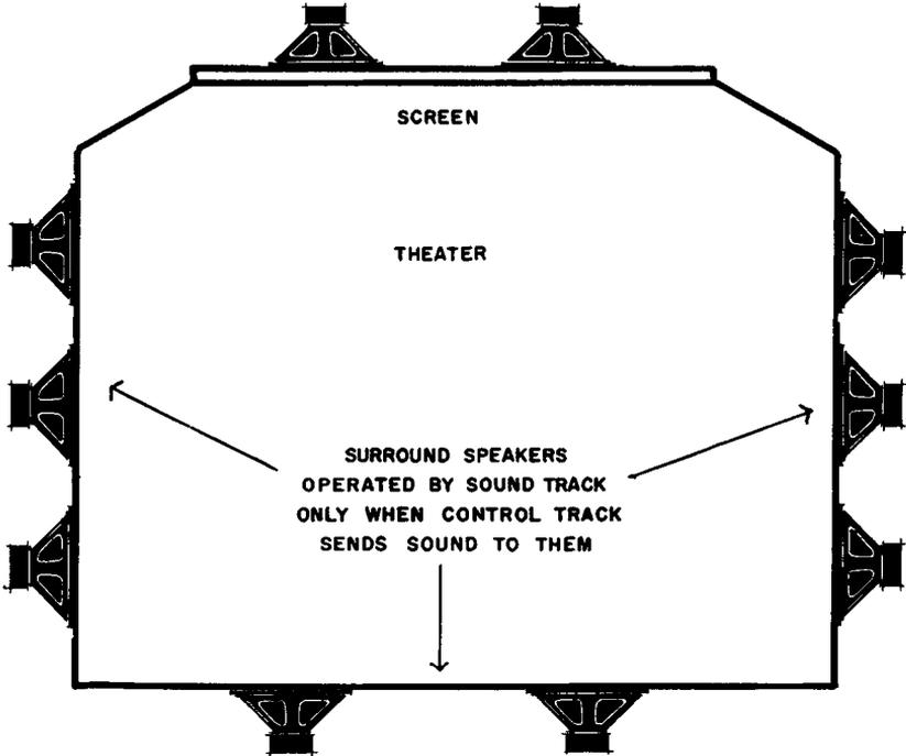
Fig. 305. The "Vitasound" system developed by Warner Brothers.
