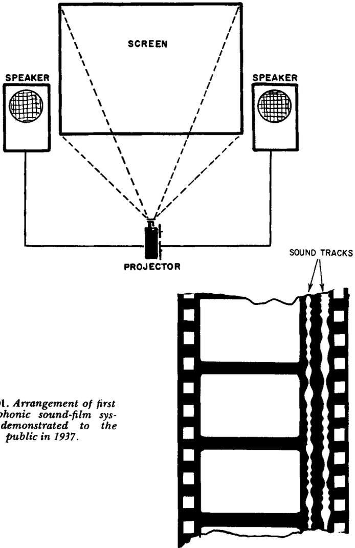
*Fig. 301. Arrangement of first stereophonic sound-film system, demonstrated to the public in 1937.*
