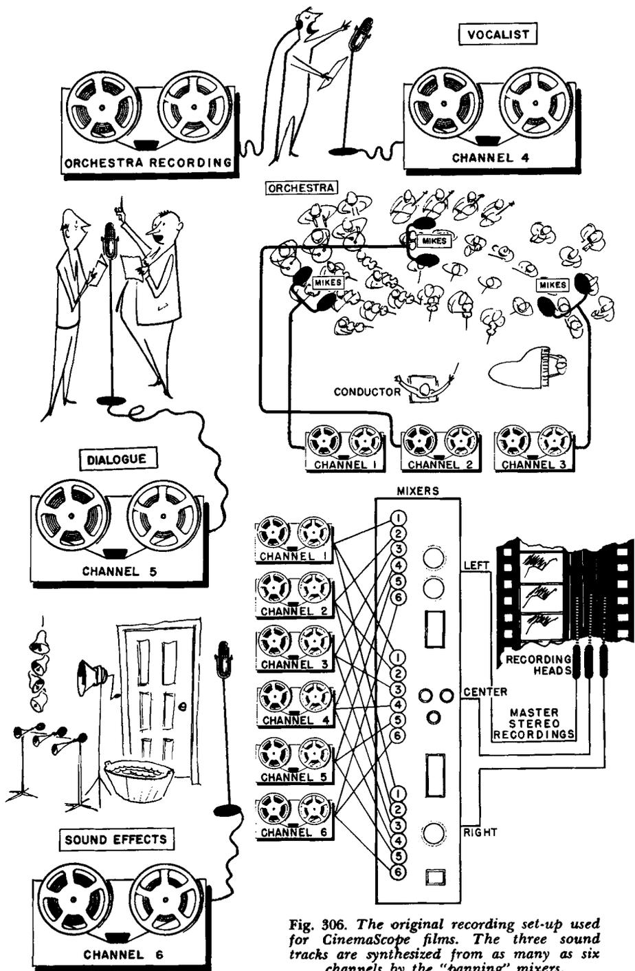
Fig. 306. The original recording set-up used for CinemaScope films. The three sound tracks are synthesized from as many as six channels by the "panning" mixers.
