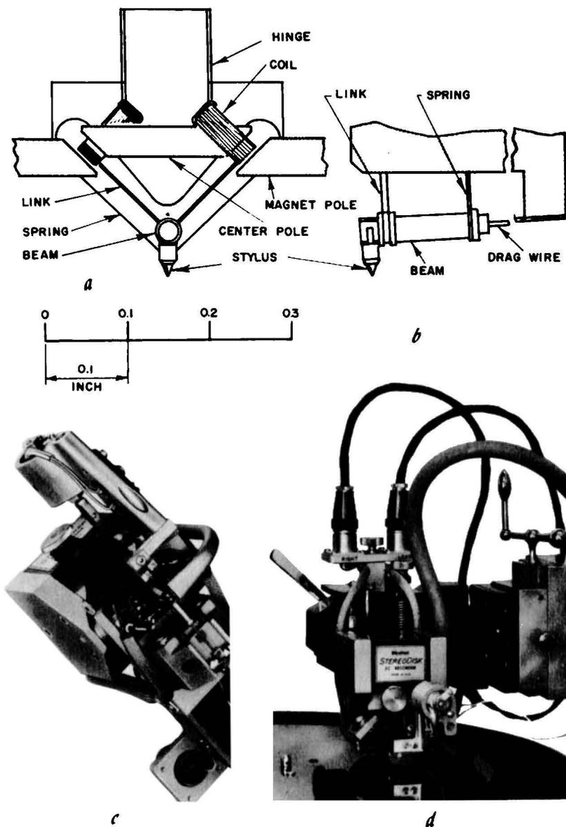
Fig. 504. (a) Cross-sectional view of the 45/45 cutting head. (b) Detail of the stylus mounting assembly. (c) Bottom view of the 3C cutter with automatic depth control. (d) 3C cutter mounted on a Scully lathe. (Westrex Corp.)
