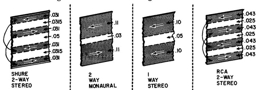
Fig. 410. Diagrammatic comparison of monophonic and two-track stereo tapes with the four-track system which was not adopted by the industry, and the RCA system, which was.
