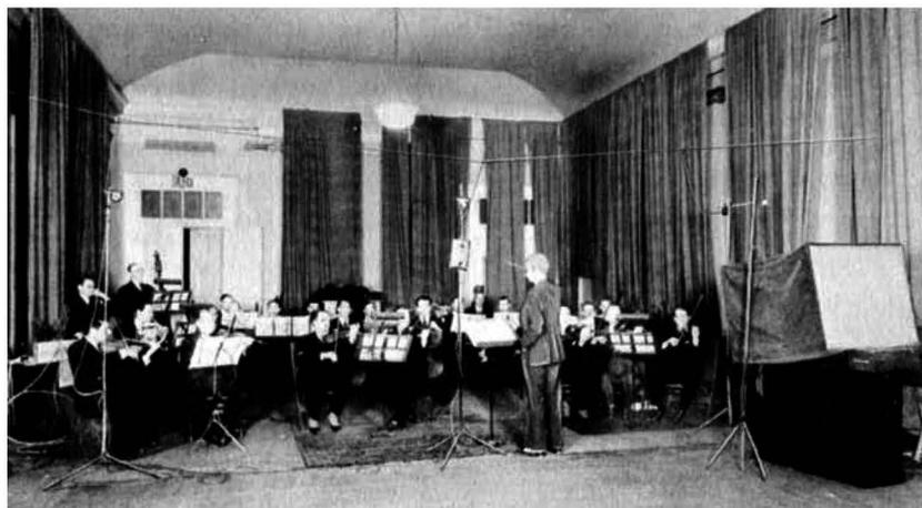
*Fig. 210. Early Bell Telephone Laboratories stereo experiments (1933) included this demonstration where the orchestra was in a room two floors above the auditorium. Three microphones were spaced across the room in line with the conductor.*
