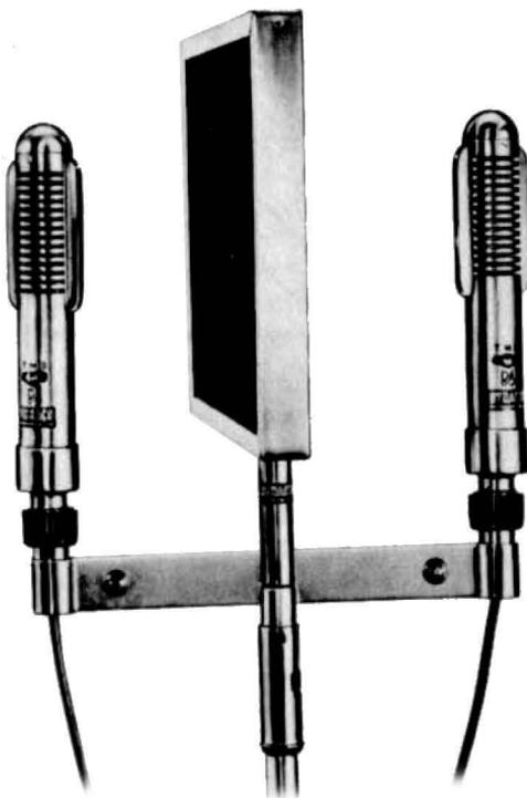
*Fig. 208. This arrangement of microphones is still sometimes used today, with a baffle to simulate the acoustic effect of the human head. However, the figure-eight pickup pattern of these special microphones results in an apparent separation of as much as 10 feet.*
