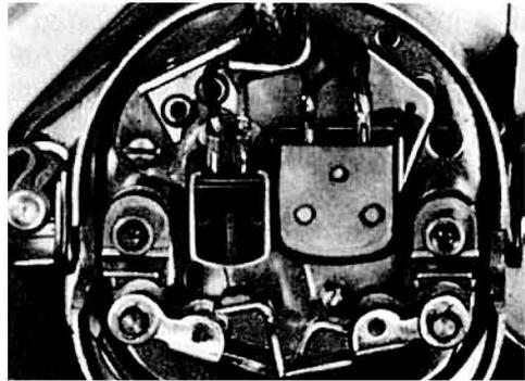
(Below) In this conversion, the original heads are retained while the stereo heads are added on the right. Precise positioning of heads is accomplished by a knob that raises and lowers them for shifting from 2-track to 4-track operation.
