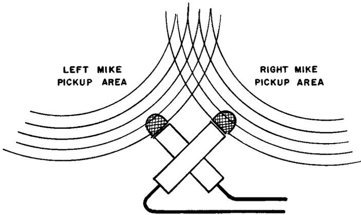
Fig. 206. Arrangement of the microphones in Blunlein's stereophonic recording system.
