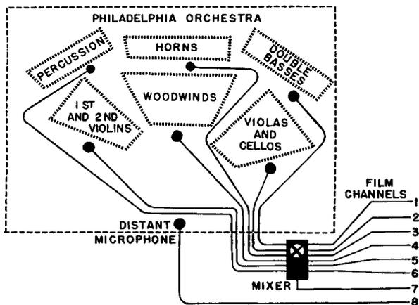
Fig. 304. The stereophonic recording arrangement used for "Fantasia".
