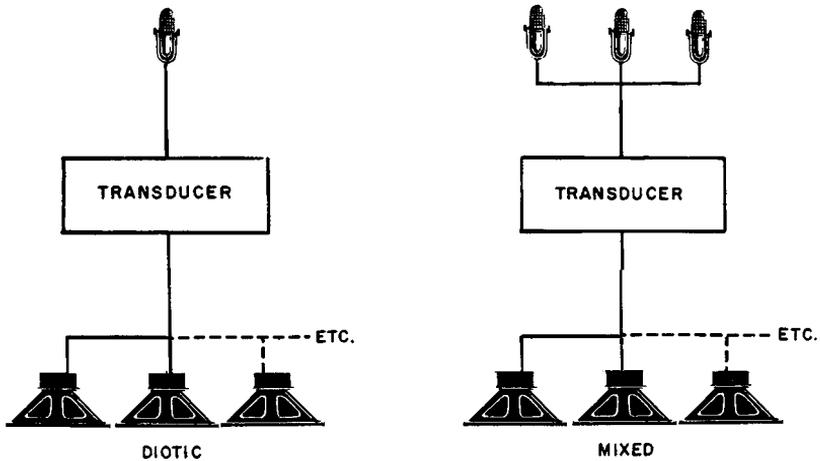
Fig. 209. Representation of diotic and mixed sound transmission.
