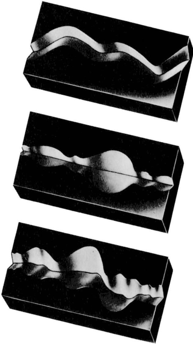
**Fig. 505. Record groove modulation; (a) lateral cut, (b) vertical cut and (c) vertical-lateral combined in a stereo disc.**
