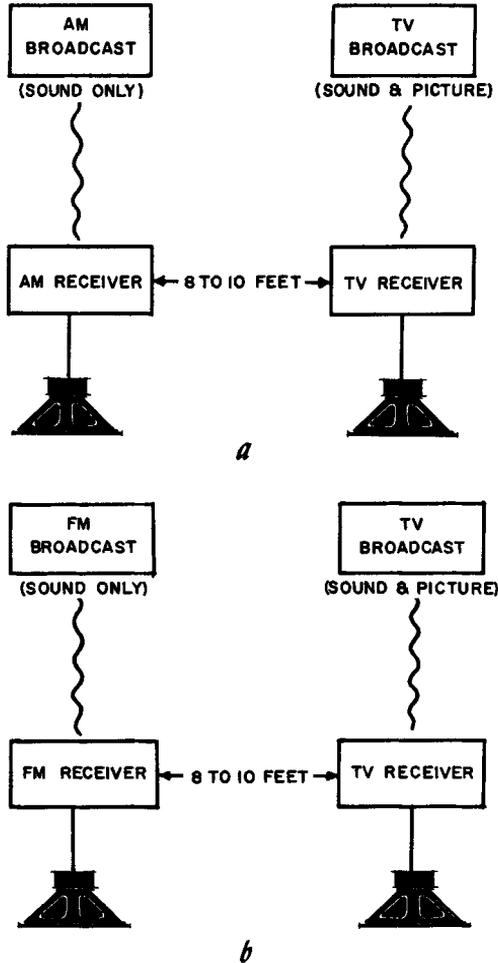
Fig. 605. Other methods of simulcasting use a television-station sound system for the right channel while an AM or FM station broadcasts the left.
