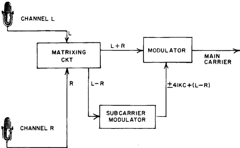
Fig. 615. Block diagram of Crosby method of modulation.
