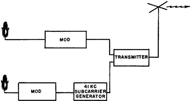
Fig. 609. Schematic diagram of the multiplex method used in musiccasting. The subcarrier signal is added at the transmitter.
