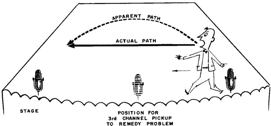
Fig. 112. The problem of the recession of the middle of the sound image, caused by the two microphones being too far apart. A middle microphone would bring the center into proper position.
