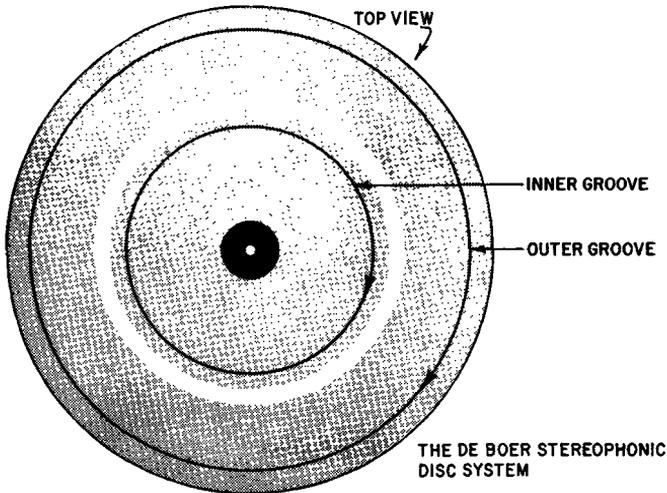
Fig. 213. Early system of stereophonic disc recording.
