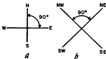
Fig. 503. Comparison of stylus motion in the "VL" (vertical-lateral) system (a) with stylus motion in the 45/45 system (b).
