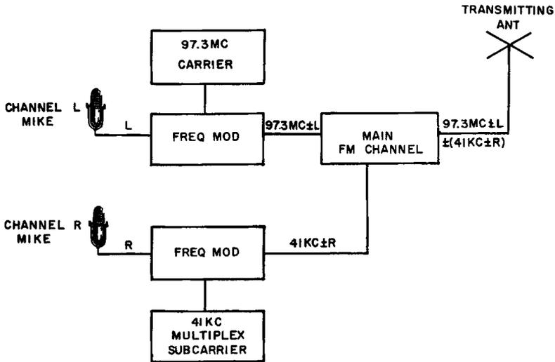
Fig. 608. In FM multiplexing, a principal channel is carried conventionally by the carrier, while a second channel modulates a subcarrier of 41 kc. The modulated subcarrier in turn modulates the main rf carrier.
