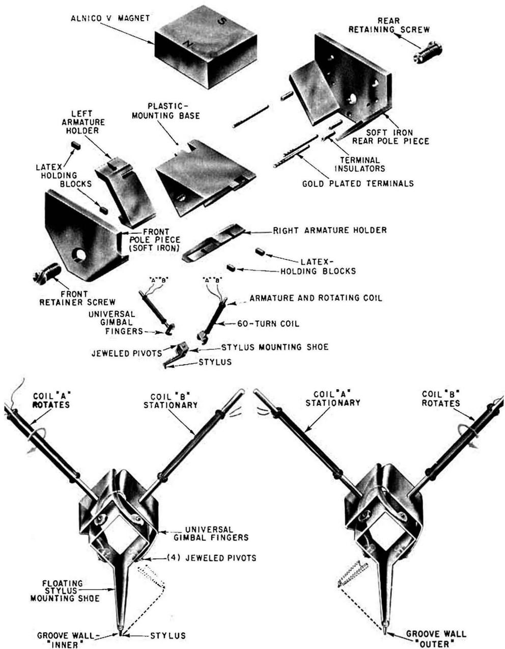
Fig. 509. (Top) Exploded view of magnetic stereo cartridge shows how the two independent rotating coils move in the field of a single Alnico magnet. Lower drawings show magnified detail of the stylus mounting and coil assemblies. Gimbal fingers allow maximum rotation in all directions resulting in high compliance.
