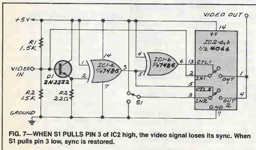
**FIG. 7—WHEN S1 PULLS PIN 3** of IC2 high, the video signal loses its sync. When S1 pulls pin 3 low, sync is restored.
