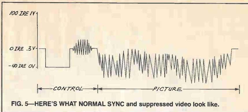
reference for color is the colorburst signal that follows horizontal sync. The colorburst signal lasts only a bit longer than 2 microseconds, but it's used as a reference for the whole video line, which is about 63 microseconds long. As far as color correction is concerned, that means there's no real reference signal available for more than 95% of the line! The color phase for the rest of the line is based on the stand-alone 3.58-MHz generator that's a normal part of the TV set.
