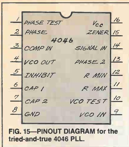
quency to some multiple of the input frequency, we can have the counter/divider chop the VCO frequency down to the input frequency and keep the VCO in sync with the input, even though the frequencies aren't the same. So, PLLs let us easily multiply frequencies, build filters, and—more to our point—keep signals in sync.
