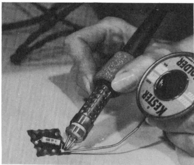
Fig. 739. With resistance soldering the tip remains relatively cool. Heat is generated only when the iron is applied to the work.
