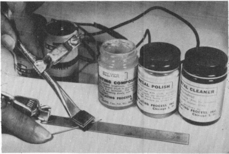
Fig. 744. Silver plating will increase the Q of inductors by reducing their dc resistance.
