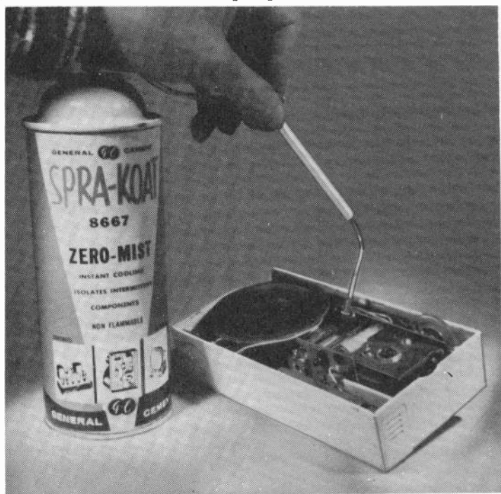
Fig. 716. Freon aerosol dispenser helps pinpoint temperature-sensitive components.
