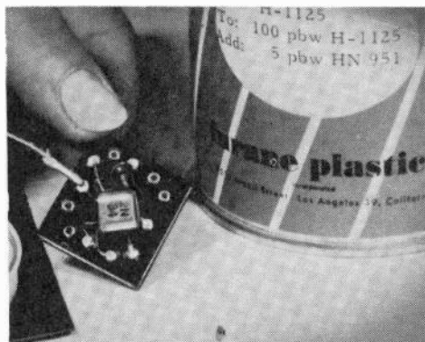
Fig. 418. Conductive epoxy cements can also be used to secure component leads and riser wires for a permanent assembly.
