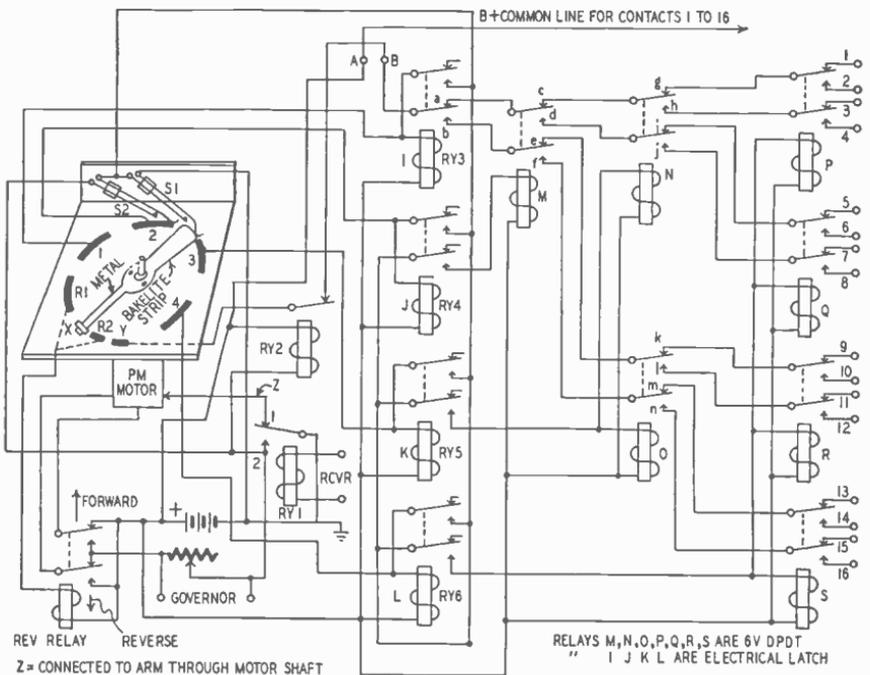
Fig. 1031—The decoder routs power through points A and B. Speed of rotation of the decoder arm can be controlled by a governor.
