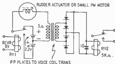
Fig. 1027—Pulse-rate decoder.
