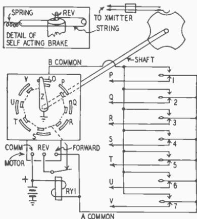
Fig. 1029--Coder for model car.
