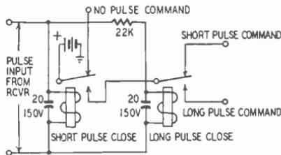
Fig. 504—Delay-open relay and delay-close relay in shunt.
