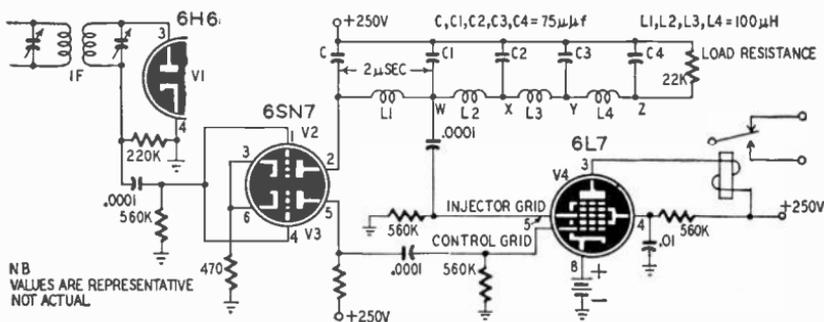
Fig. 520—Representative delay line circuit used as a decoder. Action of the decoder depends upon pulse timing.
