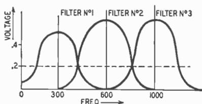
Fig. 513—The voltage across *either* C or L is maximum at resonance.
