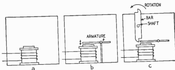
Fig. 1001—Steps in building a simple escapement.
