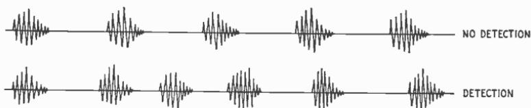
Fig. 402—Superregenerative r.f. output with and without signal. Spacing of r.f. depends upon signal strength.
