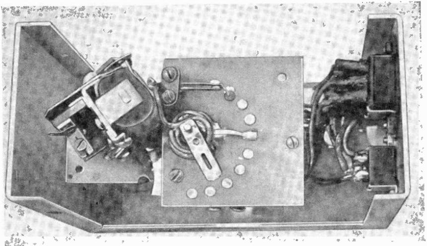
Fig. 1023—Top view of numerical-sequence decoder, showing contact arm assembly.
