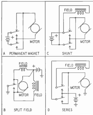
Fig. 603—Reversing relays can control motor rotation.
