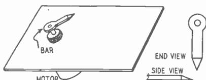
Fig. 1016—Catch bar mounted on gear shaft.
