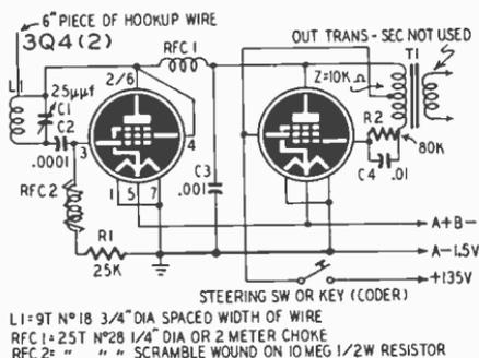
Fig. 1105—The transmitter is modulated by a single tone.
