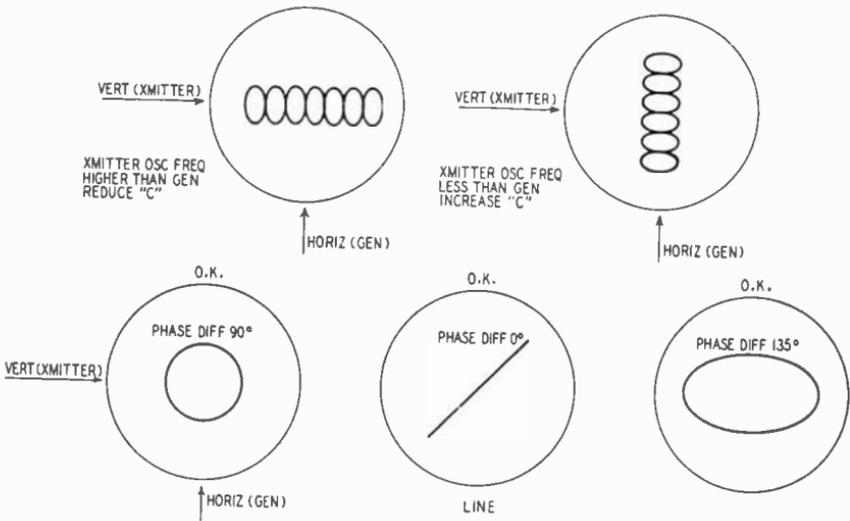
Fig. 906—Lissajous figures obtained in checking frequency of tone modulators.
