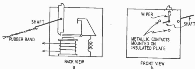
Fig. 508—Back view (a) and front view (b) of a four-contact stepper, controlled by an escapement.
