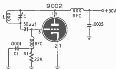
Fig. 401—Superregenerative receiver.
