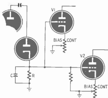
Fig. 521—Counting circuit decoder.
