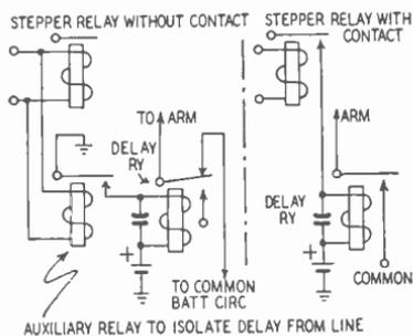
Fig. 510—Stepper relay with and without contacts.
