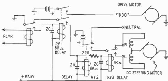
Fig. 1014—Decoder for use with pulse-variation coder.
