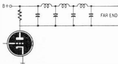
Fig. 518—Fundamental delay line.
