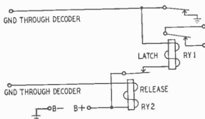
Fig. 602—Electrical latching relay.
