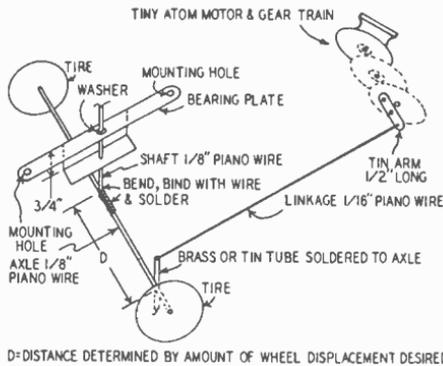
D=DISTANCE DETERMINED BY AMOUNT OF WHEEL DISPLACEMENT DESIRED
