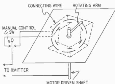
Fig. 202—Motor-driven coder.
