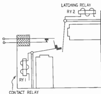
*Fig. 601—Mechanical latching relay.*
