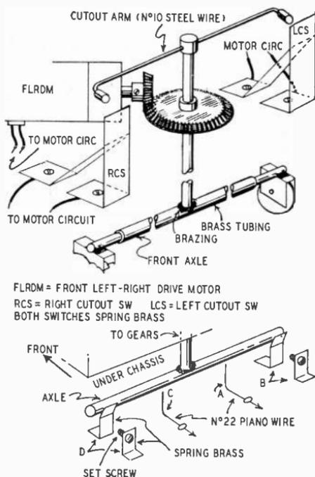
Fig. 1110—Details for building steering mechanism.
