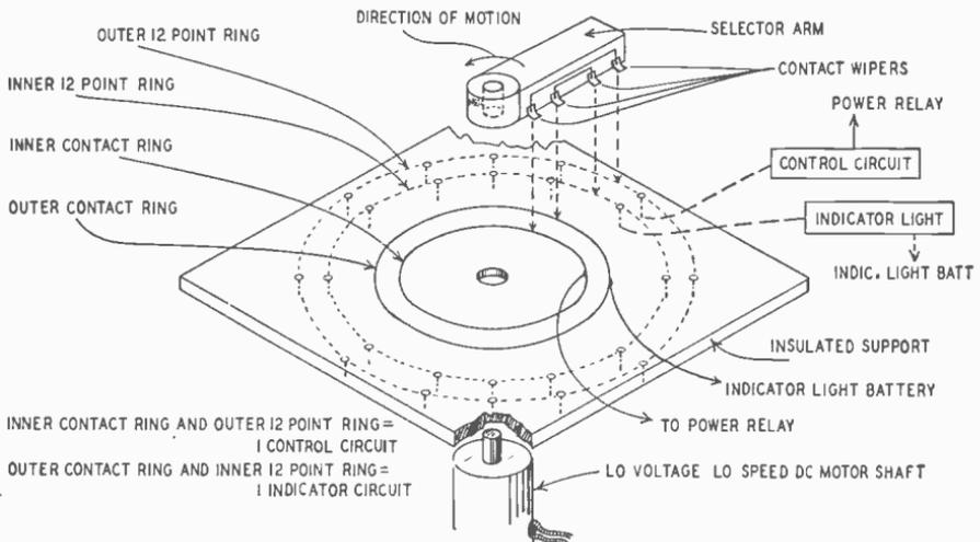
Fig. 1107—Construction details for motor-driven, two-circuit, 12-point selector switch.
