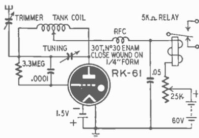
Fig. 801—The Aerotrol one-tube receiver.
