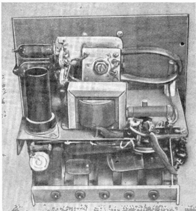
*Fig. 905—Parts layout for the tone-modulated transmitter using push-pull 6C4's.*
