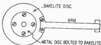
Fig. 1019—Details for the construction of the stepper arm. The T strip is spring metal.
