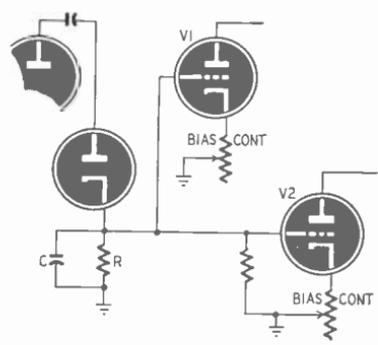
Fig. 521—Counting circuit decoder.
