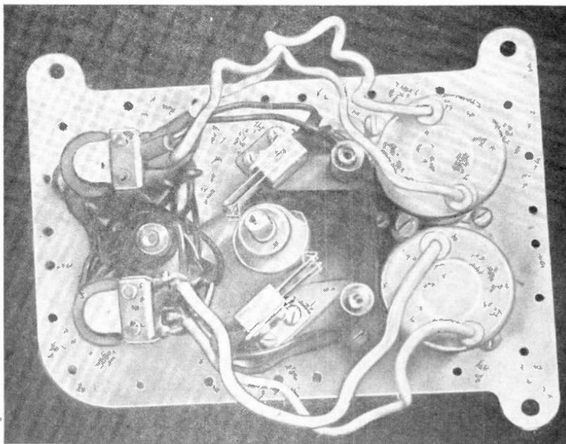
*Fig. 704—Cam-type limit switches and neutralizing relays. The relays are shown at the left; servomotors at the right.*
