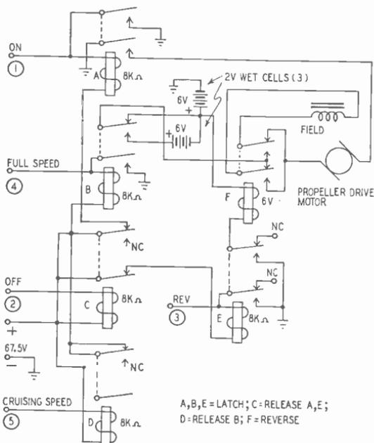
Fig. 1024—Motor control circuit for model boat.
