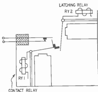
*Fig. 601—Mechanical latching relay.*
