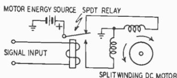
Fig. 501—Forward and reverse motor rotation.
