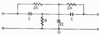
Fig. 514—Twin-T band-rejection filter.
