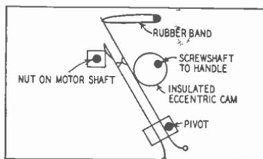
the coder controls pulses of long duration and short spacing or short duration and long spacing, varying gradually from one to the other. The coder is simply a motor, geared down so that it turns an output shaft at about 15 revolutions per minute. On the shaft is placed a small four-point metal contact; this can be a large square nut.
