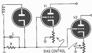
Fig. 522—Pulse amplitude decoder.
