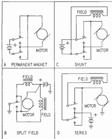
Fig. 603—Reversing relays can control motor rotation.
