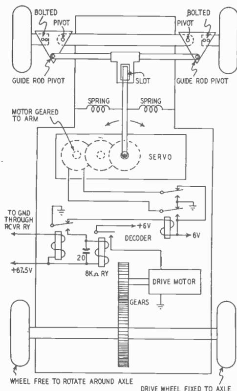
Fig. 1012—Delay decoder used in model car.
