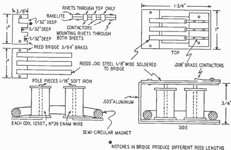
Fig. 1026—Details for construction of resonant-reed decoder.
