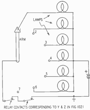
*Fig. 1022—Test unit for numerical-sequence coder.*
