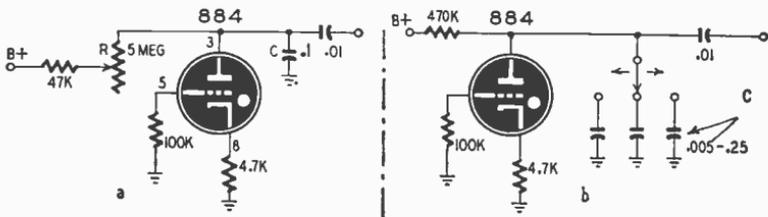
Fig. 207—Gas tube used in coder circuit. Firing of gas tube controlled by varying  $R$  (circuit a) or by varying  $C$  (circuit b).
