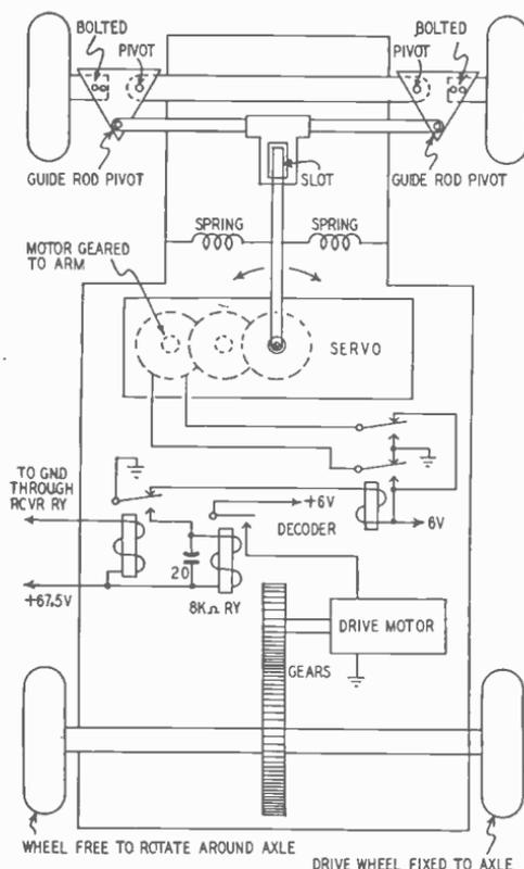
Fig. 1012—Delay decoder used in model car.
