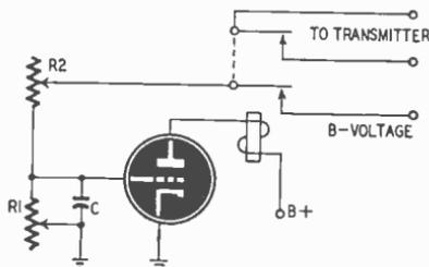
Fig. 206—Coder for variation in pulse width or spacing.
