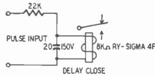
Fig. 503—Delay in closing relay.
