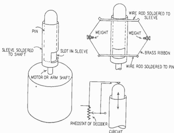
Fig. 1032—This governor is connected to the rheostat of the decoder shown in Fig. 1031.
