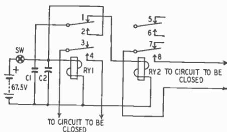
Fig. 505—Relay chain using two relays.
