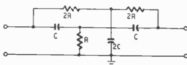
Fig. 514—Twin-T band-rejection filter.
