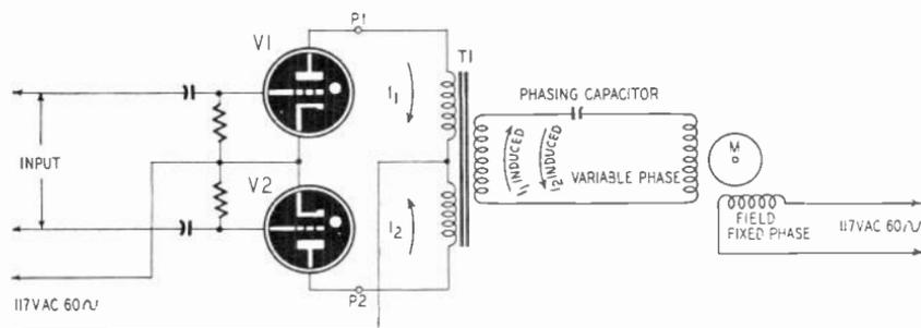
Fig. 605—Bidirectional and speed control of a motor using push-pull thyratrons.
