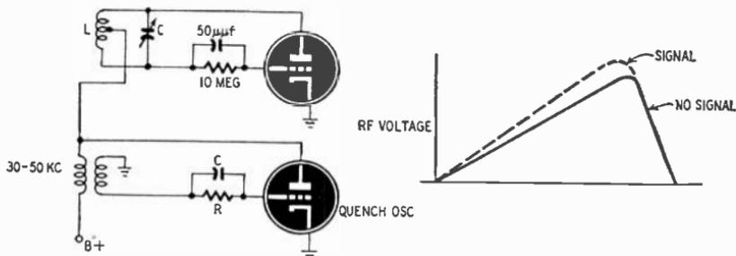
Fig. 403—Superregenerative receiver using a separate quench oscillator. The r.f. voltage increases with signal.
