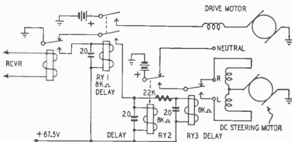
Fig. 1014—Decoder for use with pulse-variation coder.
