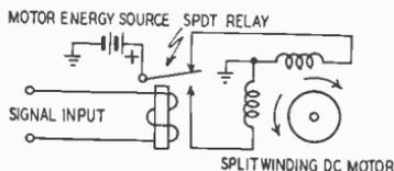
Fig. 501—Forward and reverse motor rotation.
