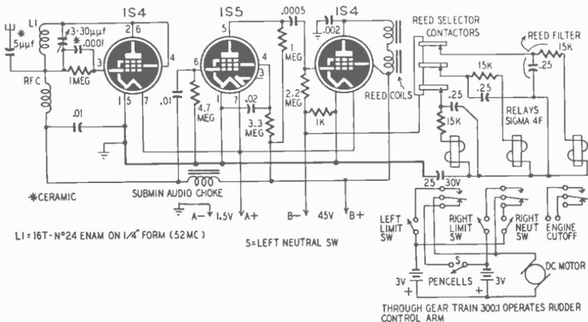
Fig. 810—Receiver using three vibrating reeds as decoders. The reed coil forms the plate load for the 1S4.
