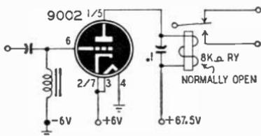
Fig. 404—The relay is the plate load.
