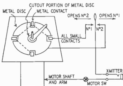
Fig. 1013—Mechanical pulse-variation coder.
