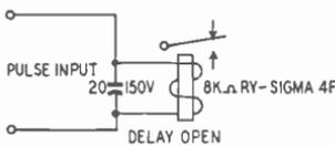
Fig. 502—Delay in opening relay.
