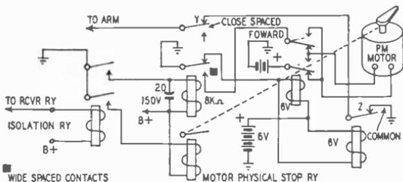
Fig. 1021—Relay system for numerical-sequence decoder.
