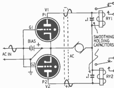
Fig. 604—Power control using gas tubes.
