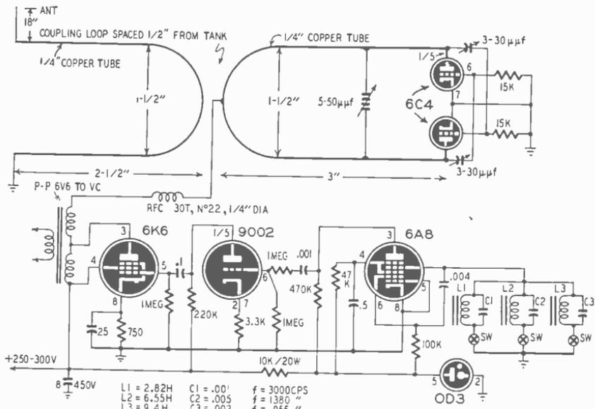
Fig. 904—Tone-modulated transmitter using 6C4's in push-pull. The modulator is a transistron oscillator.
