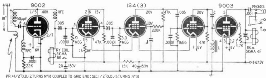
Fig. 807—Tone-operated receiver using band-pass filter in grid circuit of relay tube.
