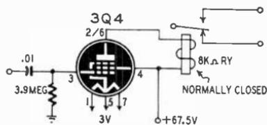
Fig. 405—Normally closed plate relay.
