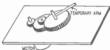
Fig. 1015—Small motor mounted on plate.
