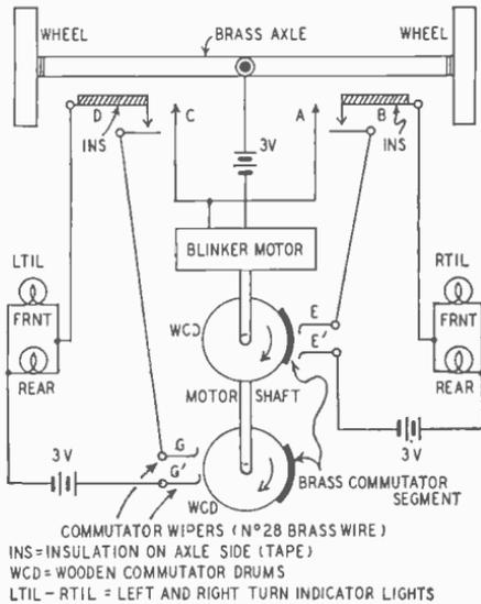
Fig. 1111—Wiring of the turn-indicator circuit.
