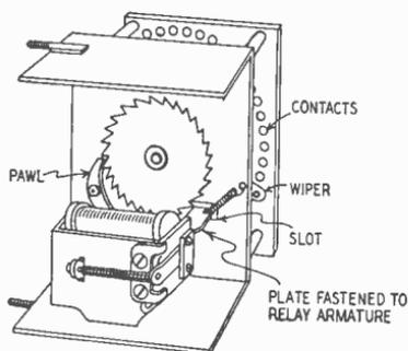
Fig. 509—Relay-driven stepper.
