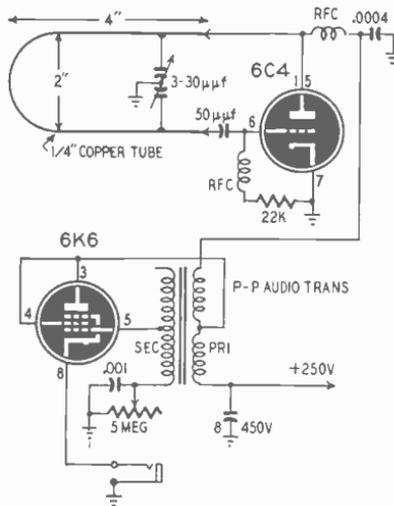
Fig. 902—Transmitter including a tone modulator.
