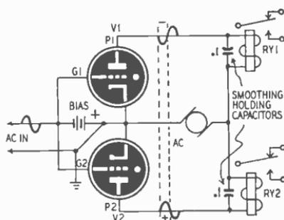
Fig. 604—Power control using gas tubes.
