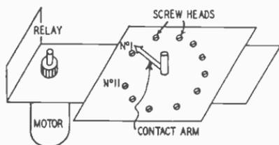
Fig. 1018—Stepper plate and contact arm.
