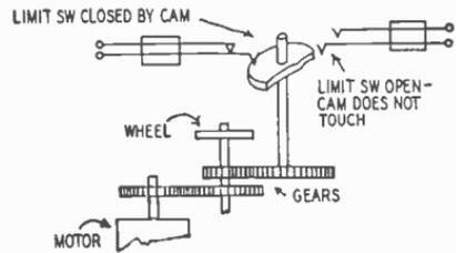
Fig. 702—Limit switch closed by rotating cam.
