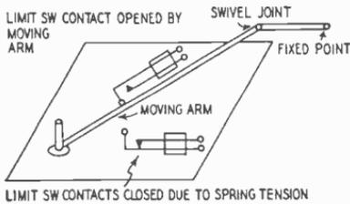
Fig. 701—Limit switches operated through use of a moving arm.
