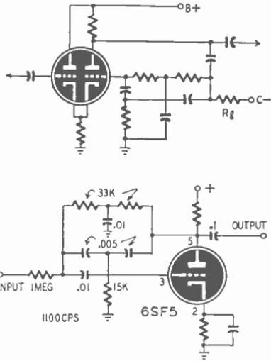
Fig. 515—Twin-T in grid circuit of second half of duo-triode. Fig. 516—Typical Twin-T used in input stage. Drawings courtesy of McGraw-Hill.
