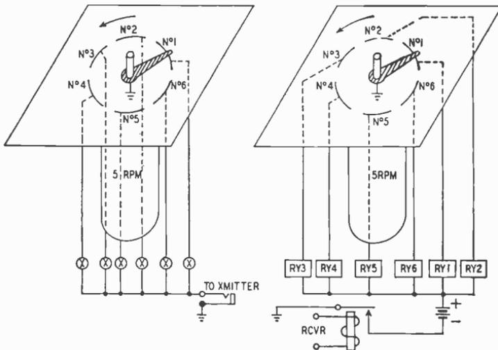
Fig. 511—Motor-driven commutator-type coder and decoder.
