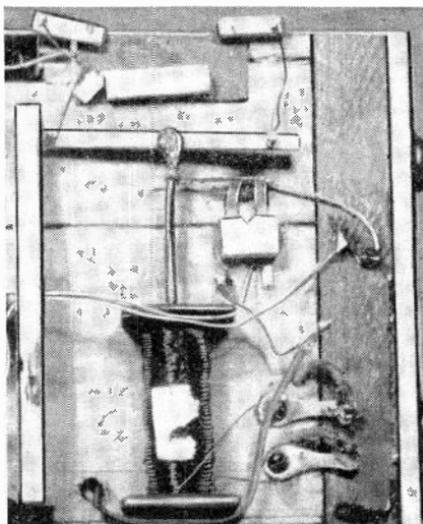
*Fig. 1109—Mechanism for opening the door.*
