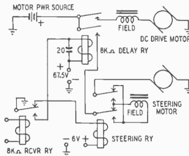
Fig. 1011—Decoder using a delay relay.
