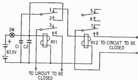
Fig. 505—Relay chain using two relays.
