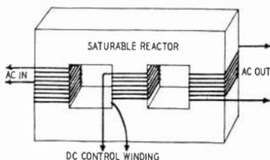
Fig. 606—Saturable reactor type transformer.
