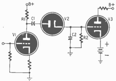
Fig. 525—Integrator circuit used with diode.
