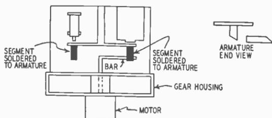
Fig. 1017—Relay and gear box assembly.
