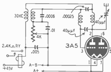
Fig. 802—The Goode one-tube receiver.
