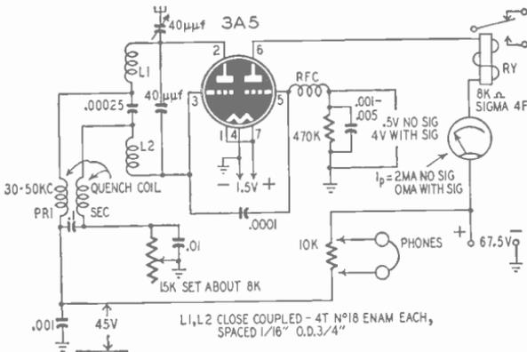
Fig. 803—Modified Goode receiver using Sigma 4F relay.
