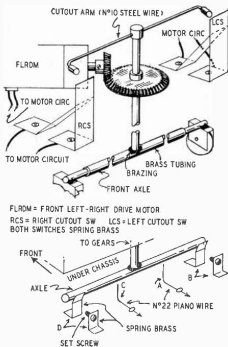
Fig. 1110—Details for building steering mechanism.
