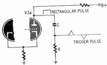
Fig. 526—Differentiator used with vacuum tube. The tube is part of a multivibrator circuit. The differentiator is shorted when the tube conducts. The tube produces a rectangular pulse which is differentiated into a triangular trigger pulse.
