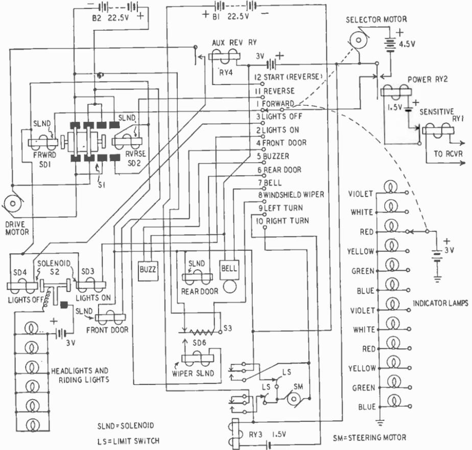
Fig. 1108—Master control diagram. Solenoids and relays in this circuit are controlled by the receiver output.
