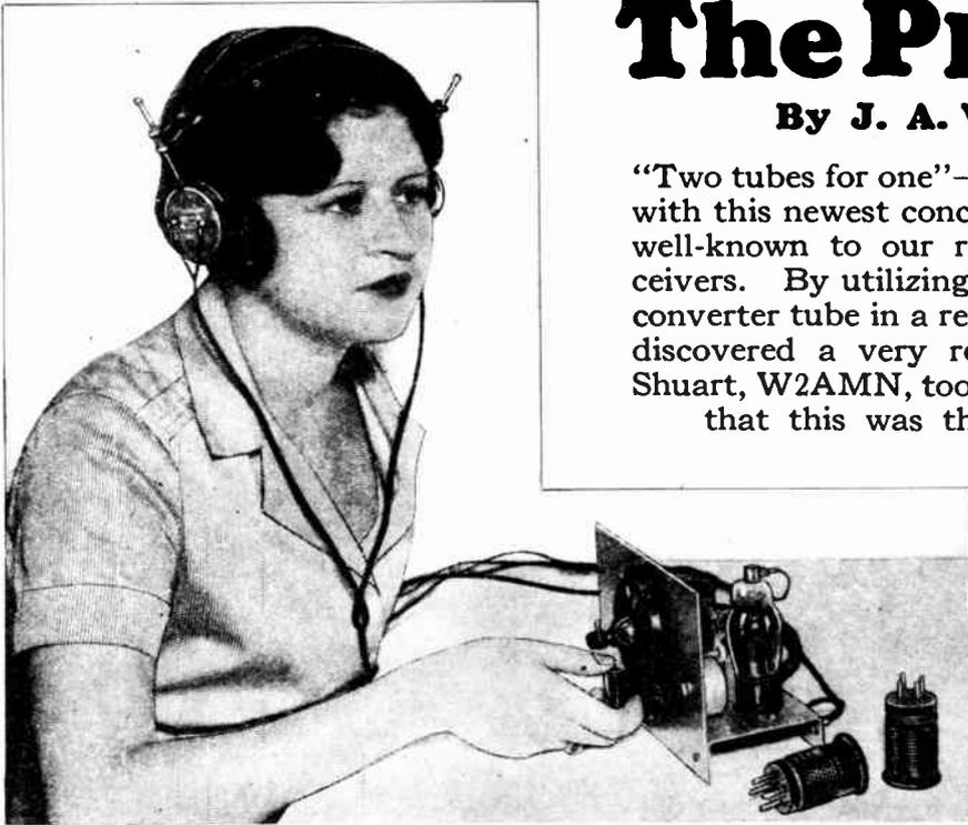
Regeneration is controlled in the usual manner by varying the screen grid voltage with a 50,000 ohm potentiometer.
