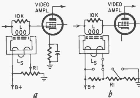
Fig. 504. The inductance of the series correcting coil  $L$  is varied by putting the core in the field of an electromagnet.
