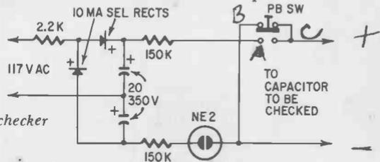
Fig. 705. Simple capacitor checker tests for leakage.
