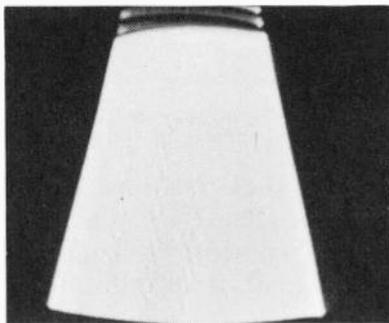
Fig. 914. Horizontal keystone caused by shorting of capacitor C1 in Fig. 913.
