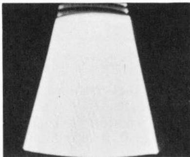
Fig. 914. *Horizontal keystoneing caused by shorting of capacitor C1 in Fig. 913.*
