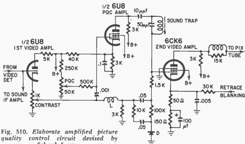
Fig. 510. Elaborate amplified picture quality control circuit devised by Schaub-Lorenz.
