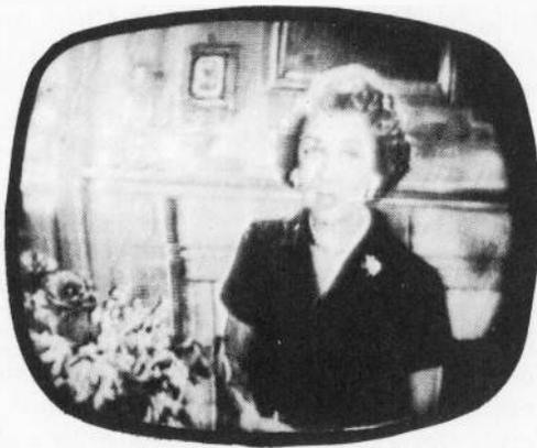
Fig. 1226. *Excessive brightness can be due to insufficient bias on the picture tube.*
