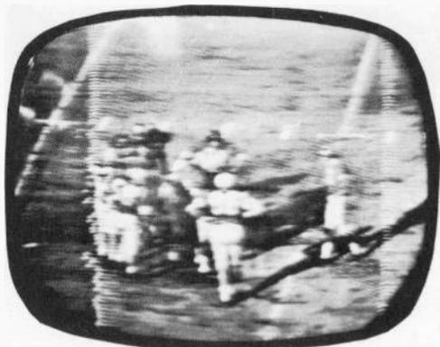
*Fig. 1212. Parasitic oscillation as evidenced by jagged white vertical bars on both sides of the screen. The trouble is often caused by a defective horizontal output tube. Try tube substitution or insert parasitic suppressors in series with tube leads. Adjust all controls in the horizontal sweep circuit.*
