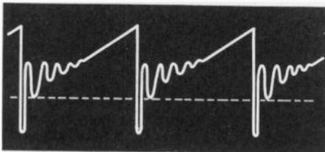
Fig. 804. Natural shape of the waveform in the yoke and flyback without a damper tube.
