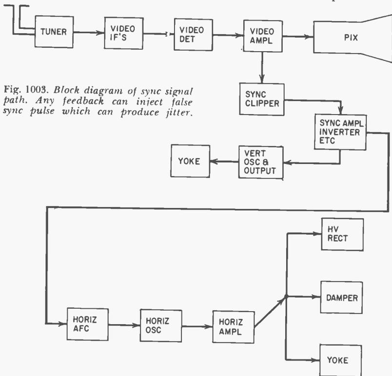
Fig. 1003. Block diagram of sync signal path. Any feedback can inject false sync pulse which can produce jitter.
