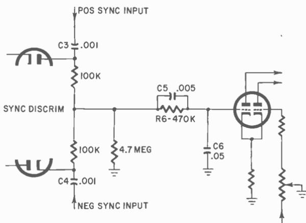
Fig. 604. The coupling network between the sync discriminator and the horizontal oscillator frequency can cause a jump in oscillator frequency.
