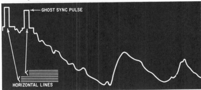
Fig. 1002. Relation between spurious sync pulses and displacement of sections of horizontal lines.
