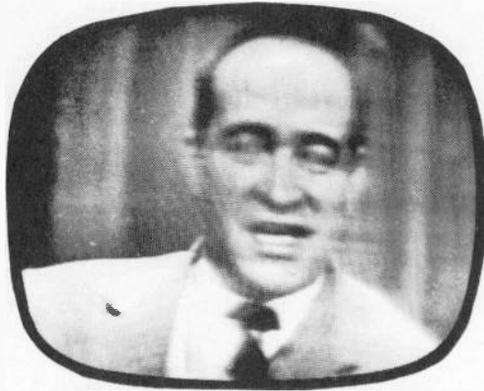
*Fig. 1205. Smearing is usually accompanied by poor definition and focus.*
