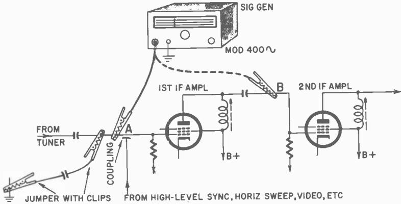
Fig. 1006. Grounded-grid signal injection technique for localizing entry point of the spurious signal.
