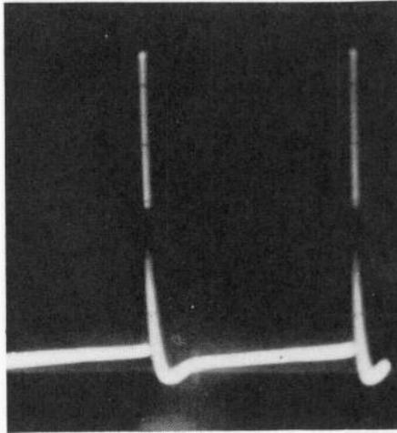
Fig. 902. *Waveform of the blanking pulse applied to the picture tube.*
