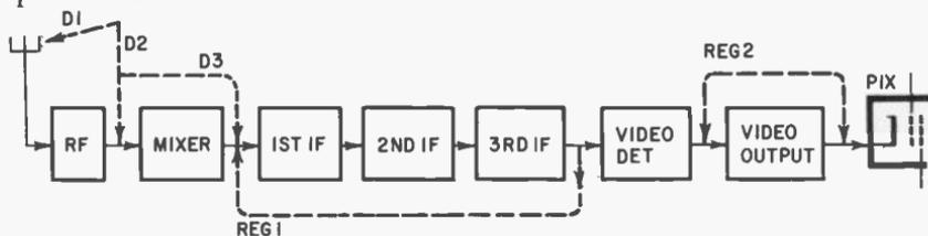
Fig. 203. This block diagram shows pickup and regeneration paths. Direct pickup at D1 and D2 causes leading ghosts. Regeneration paths — REG 1 and REG 2 — produce trailing ghosts.
