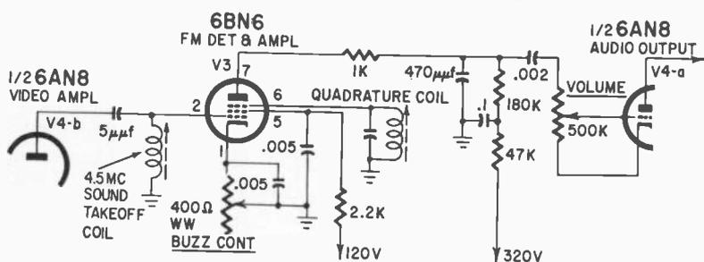
Fig. 1301. The 6BN6 gated-beam discriminator. The 1,000-ohm resistor in the plate circuit suppresses parasitic oscillation.
