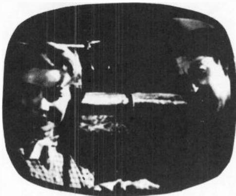
*Fig. 1208. Insufficient brightness. Can be caused by insufficient high voltage, sometimes accompanied by blooming. Condition can be produced by a gassy picture tube. The brightness control may be defective.*
