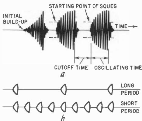
Fig. 301. Squegs are built up in groups or packets that can recur regularly. Typical case of build-up (a) and (b) long and short dead times of the oscillator.
