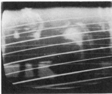
Fig. 903. *Formation of retrace lines as seen on the screen of the picture tube.*
