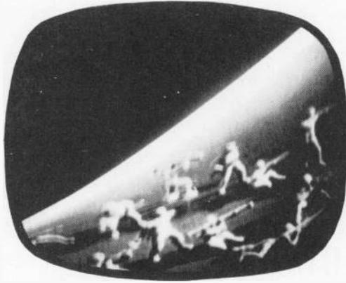
Fig. 1202. This photo shows the effect when one of the vertical deflection coils is shorted.
