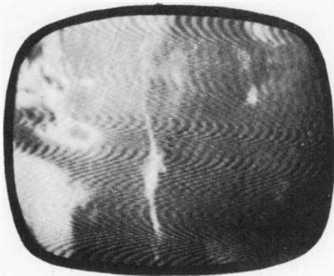
Fig. 1225. *Herringbone pattern produced by interference.*
