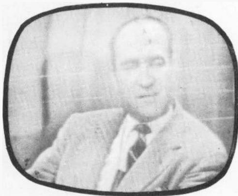
Fig. 1203. Insufficient contrast accompanied by appearance of retrace lines.
