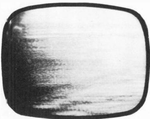
**Symptoms:** Tearing of the picture or raster (Fig. 1214).
