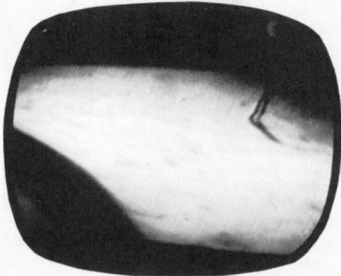
Fig. 1229. *Excessive contrast resulting in an exceptionally dark picture.*
