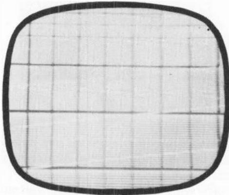
Fig. 909. *Nonlinearity caused by reduced value of resistance in sawtooth network of vertical-multivibrator-vertical-output circuit.*
