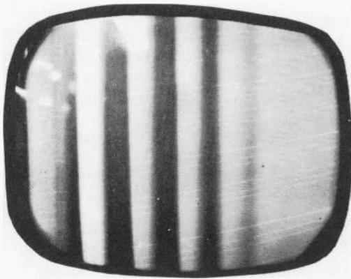
Fig. 1220. *Black vertical bars from center to left side of raster.*
