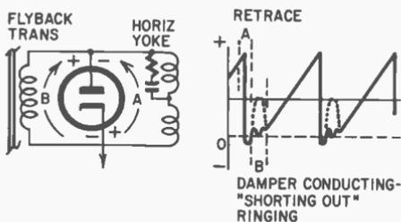
Fig. 805. Polarity of flyback pulse during retrace makes damper cathode positive so damper does not conduct. When ringing voltage starts, the damper cathode is negative and the tube conducts heavily, shorting the ringing.
