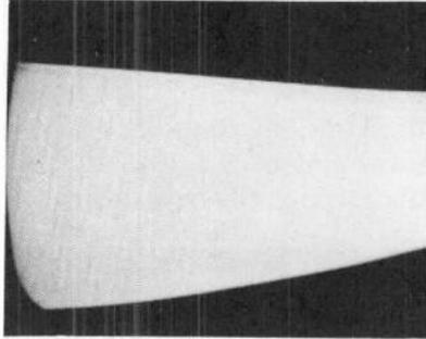
Fig. 912. Keystoning caused by shorted vertical winding in the yoke.
