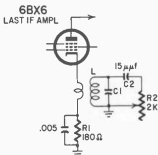
Fig. 506. Modification of the intermediate-frequency response is obtained using this definition-corrector circuit.
