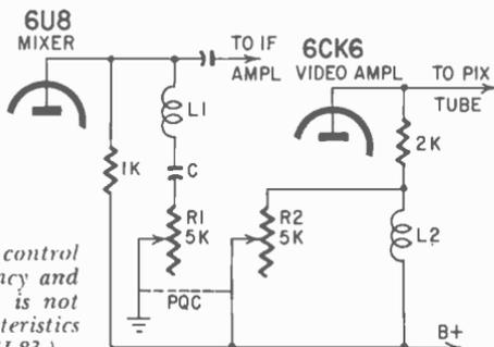
Fig. 508. Combined picture quality control circuits in the intermediate frequency and video amplifier stages. (The 6CK6 is not a readily available tube. Its characteristics are similar to those of the EL83.)
