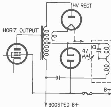
Fig. 913. The capacitor ( $C1$ ) across the top half of the horizontal yoke coils has a damping action.
