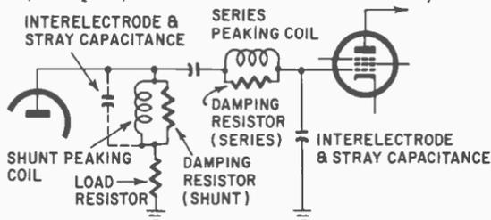
Fig. 204. Video amplifier using shunt- and series-peaking coils. The  $Q$  of the coils is lowered by the resistors shunting the coils, but ringing can occur.
