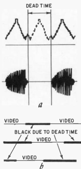
Fig. 302. Dead time (a) correlated with video information. The dead time can cover part of a synchronizing period, either horizontal (as shown here) or vertical. Dead-time symptoms (b) indicate squegging. Successive periods are black. Some can occur during blanking and appear at the finish and start of an active trace.
