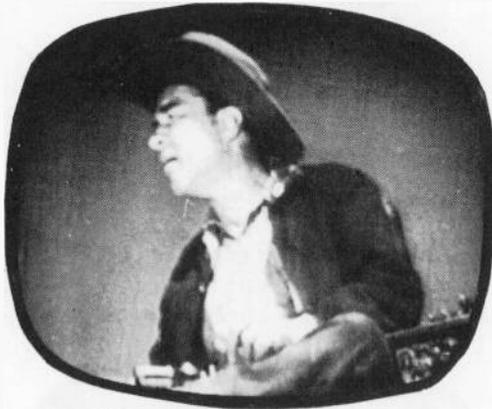
*Fig. 1209. Blooming is caused by trouble in the high voltage supply or by a defective picture tube. Check the high-voltage rectifier, horizontal output and damper tubes by substitution. Blooming is sometimes produced by a gassy picture tube or an internal short in the tube. Check the filament resistor of the high-voltage rectifier.*
