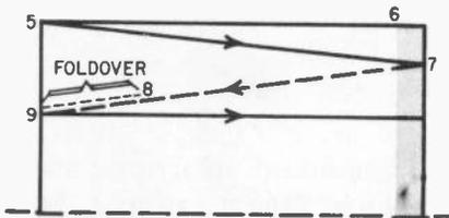
Fig. 1103. Foldover caused by too long a retrace time. The numbers refer to Fig. 1101.
