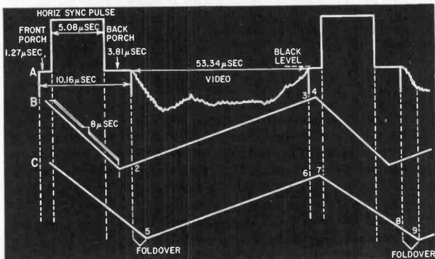
Fig. 1101. Scanning and retrace vs. video information. Line A is a line of video between two sync pulses. Line B is the normal horizontal scanning waveform. Line C is the horizontal scanning with excessive retrace time, causing foldover.
