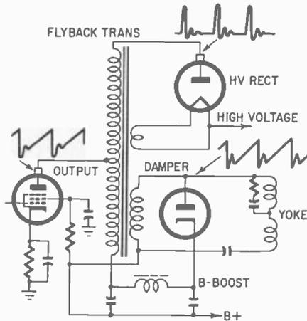
Fig. 803. Horizontal output circuit. Autotransformer action puts a high voltage pulse on the plate of the high voltage rectifier tube.
