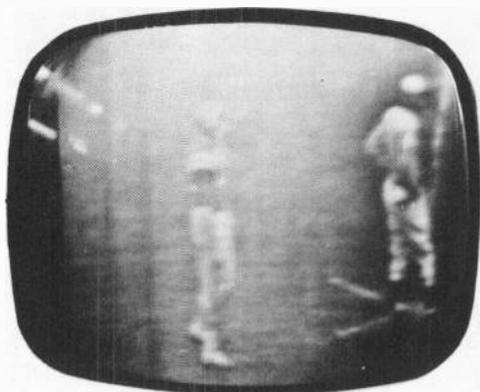
*Fig. 1216. Trouble caused by parasitic oscillation in the vertical sweep circuit.*
