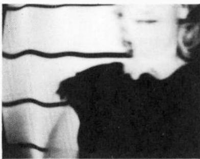
*Fig. 911. Ripples caused by open resistors across the vertical winding in the yoke.*
