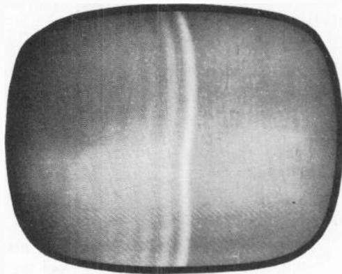
Fig. 1105. Halos caused by the porch level appearing during retrace.
