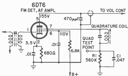
Fig. 1302. Gated-beam discriminator using a 6DT6. Excessive buzz can be caused by using a cathode resistor of the wrong value.
