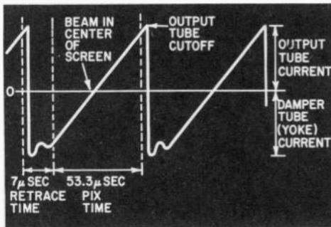
Fig. 802. Sawtooth current through the yoke developed by the trapezoidal voltage.
