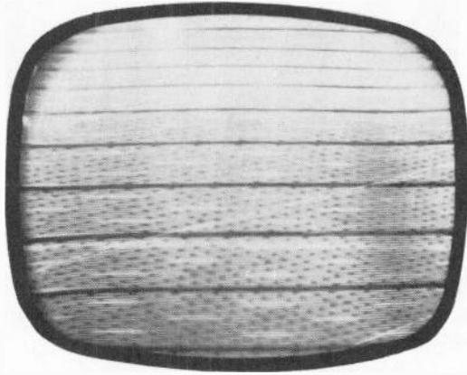
Fig. 1219. Receiver out of horizontal sync. Bar spacing indicates vertical non-linearity.
