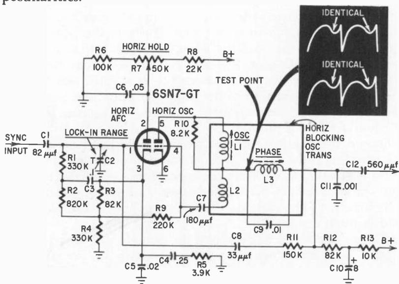
Fig. 701. Basic Synchroguide circuit. Either waveform is correct. See Fig. 703.
