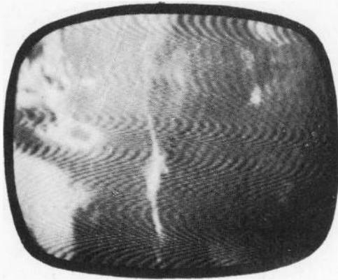
Fig. 1225. *Herringbone pattern produced by interference.*
