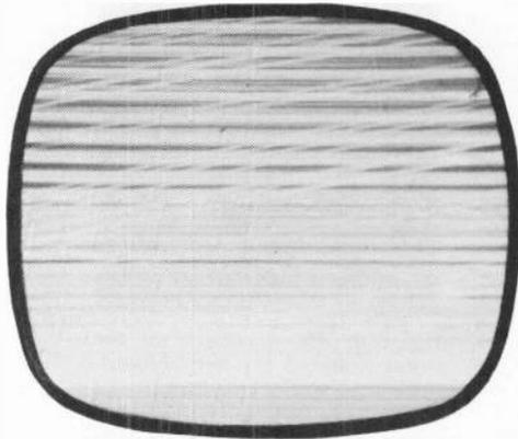
Fig. 908. *Vertical-sweep distortion produced by sawtooth capacitor in vertical-multivibrator-vertical-output circuit.*
