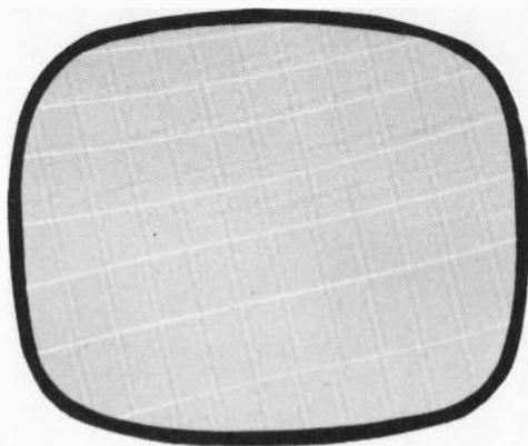
Fig. 906. *Normal number of retrace lines.*
