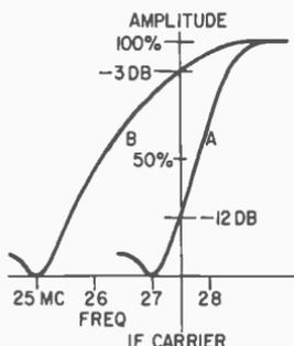
Fig. 507. Effect of the circuit of Fig. 506 on low video frequencies.
