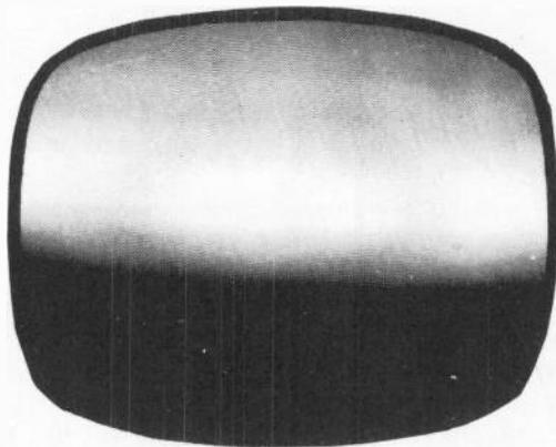
*Fig 1211. Example of 60-cycle hum. Hum pickup can exist in any stage from front end to video amplifier.*
