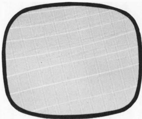
Fig. 906. *Normal number of retrace lines.*
