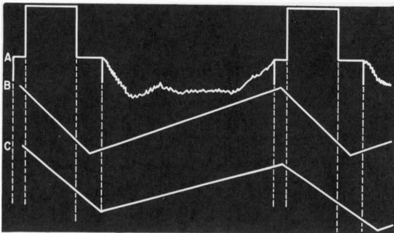
Fig. 1104. Scanning as in C causes halos on the TV screen.
