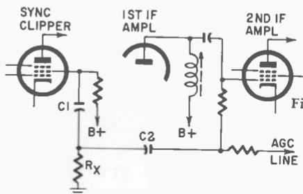
Fig. 1005. *Partial schematic shows what bad solder joint did.*
