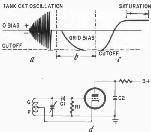
Fig. 303. Oscillatory buildup (a) in tank circuit. Corresponding grid bias developed (b). Characteristic curve (c) showing cutoff and saturation and (d) Hartley oscillator circuit for illustration.
