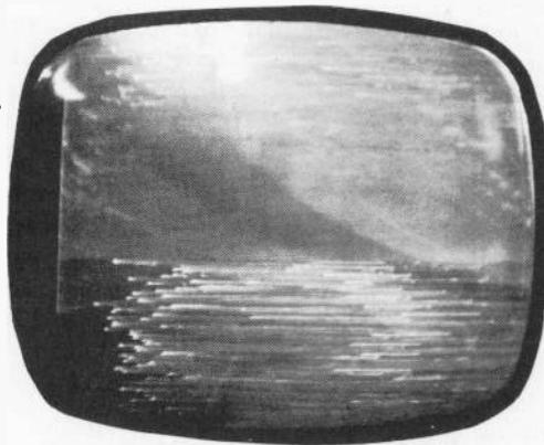
Fig. 1221. *Tearing and jitter caused by intermittent.*
