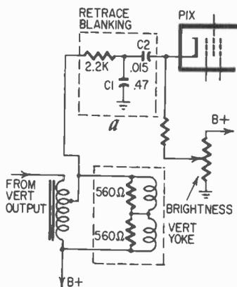
Fig. 901. Retrace-blanking network found in vertical output stages. The vertical yoke coils are shunted by a pair of damping resistors.
