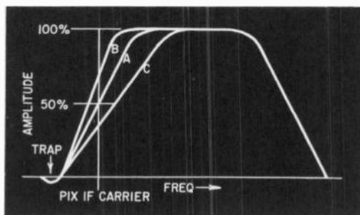
Fig. 505. Effect of modifying the intermediate-frequency response curve.
