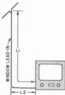
A tunable ghost may be due to other faults, but the direct-pickup type is readily localized. Movement of the body near the TV set (particularly the tuner) will change the ghost's intensity, but will not affect the main signal (unless an indoor antenna is used).
