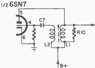
Fig. 702. Basic circuit of the blocking oscillator found in the Synchroguide.
