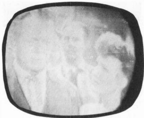
*Fig. 1230. Black area along picture edges. Make sure yoke is as far forward on the neck of the picture tube as possible.*
