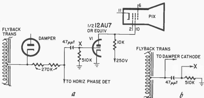
Fig. 1106. Blanking circuit that eliminates halos and retrace lines. For use in phase detector type horizontal circuits (a) and for use in sets with Synchronoscope horizontal circuit (b).
