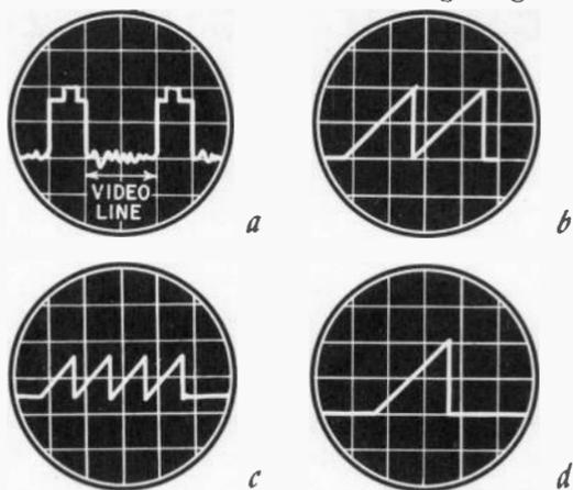
Fig. 601. Composite video and horizontal oscillator waveforms. Two lines of video (a) with sync and blanking pulses. The drawing (b) shows the oscillator on frequency. The remaining illustrations (c and d) show a fast oscillator and a slow one.
