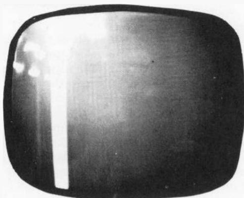
*Fig. 1215. Single thick white bar (brighter than the rest of the screen) appearing at the left side can be due to horizontal foldover.*
