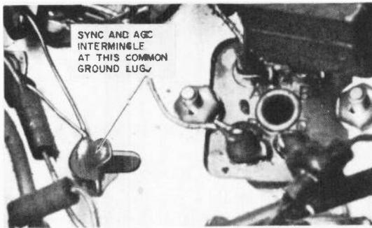
Fig. 1004. Poorly soldered joint on common ground of a sync and an agc capacitor resulted in jitter. Sync fed into agc and if grids.
