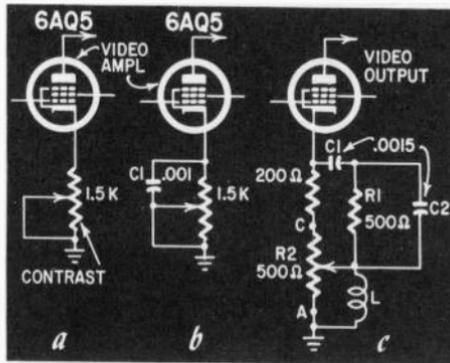
Fig. 502. Modification of a contrast control circuit for picture quality control.
