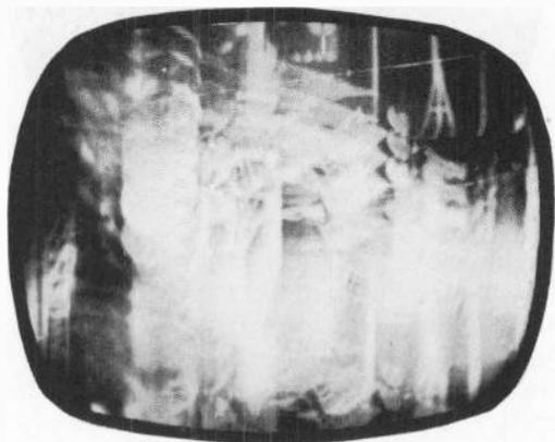
Fig. 1227. *Rolling caused by trouble in the vertical sweep.*
