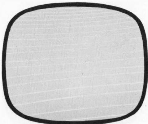
Fig. 907. *Condition due to a shorted resistor in the sawtooth forming network of a vertical blocking oscillator. The number of retrace lines has doubled.*
