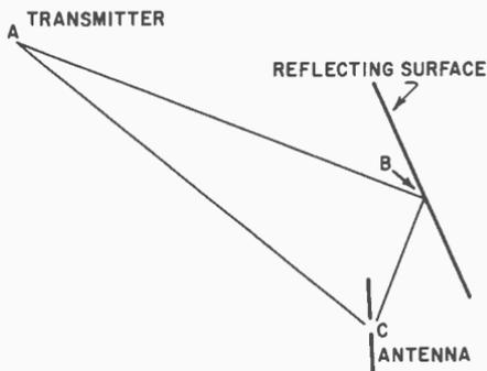
Fig. 201. Direct- and reflected-signal paths result in a trailing, external ghost. The photo shows a trailing ghost caused by a reflected signal.
