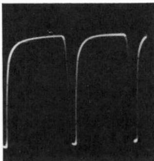
*Fig. 910. The waveform at the input plate of the vertical-multivibrator-vertical-output circuit becomes a fairly sharp square wave when the sawtooth capacitor opens.*
