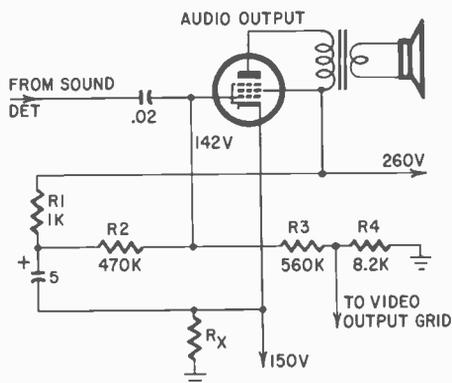
Fig. 915. Schematic shows the basic circuit in a typical stacked-B system.
