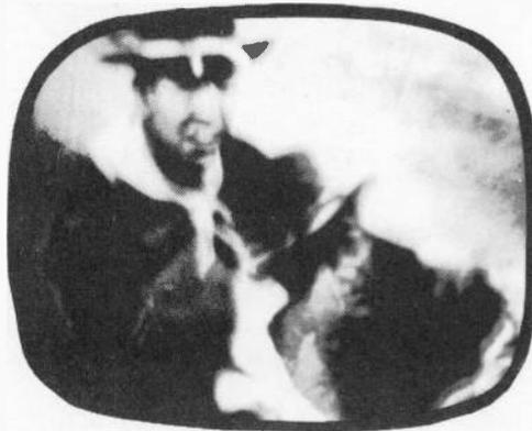
*Fig. 1206. Out-of-focus picture. If the picture goes out of focus when the brightness control is advanced, the trouble is in the high-voltage supply.*
