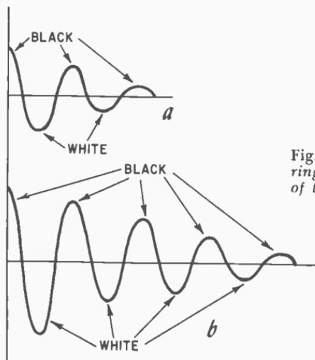
Fig. 205. Normal ringing (a). Excessive ringing (b) takes place when the values of the shunting resistors (across the peaking coils) increase.
