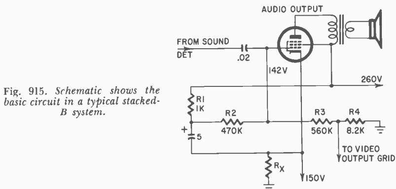
Fig. 915. Schematic shows the basic circuit in a typical stacked-B system.
