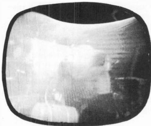
*Fig. 1207. Pincushion effect can be caused by impedance mismatch between horizontal-output transformer and yoke.*
