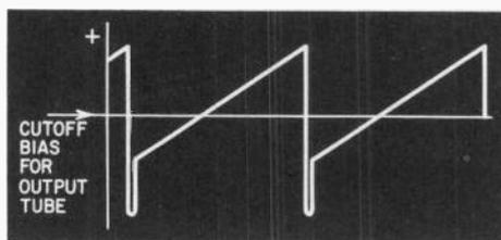
Fig. 801. *Trapezoidal voltage on the control grid of the horizontal output tube.*
