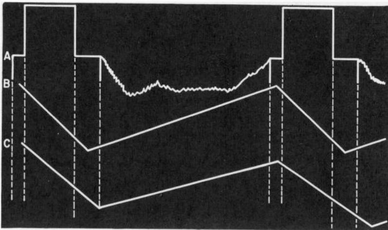
Fig. 1104. Scanning as in C causes halos on the TV screen.
