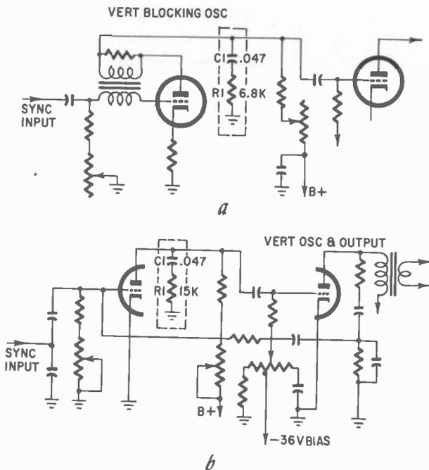
Fig. 904. Sawtooth capacitor in a vertical blocking oscillator (a) and in a vertical multivibrator-vertical output circuit (b).
