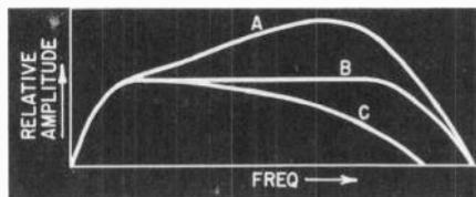
Fig. 503. Effect of the circuit of Fig. 502 on the video-frequency response.
