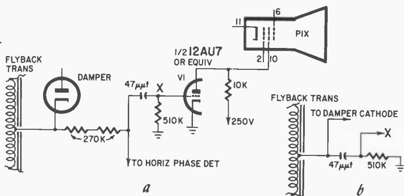
Fig. 1106. Blanking circuit that eliminates halos and retrace lines. For use in phase detector type horizontal circuits (a) and for use in sets with Synchronoscope horizontal circuit (b).
