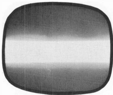
Fig. 905. Condition produced by open sawtooth capacitor in vertical blocking oscillator.
