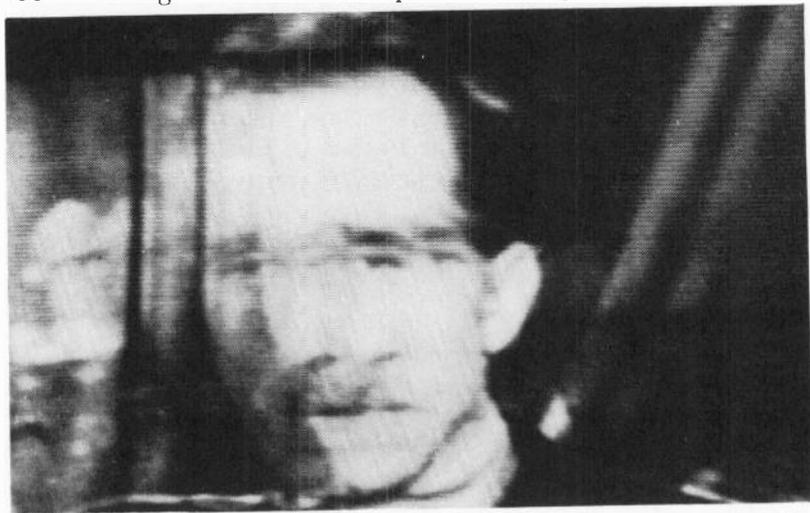
Fig. 1001. *Jitter with long flutter rate. Displacement to right persists for several consecutive fields.*
