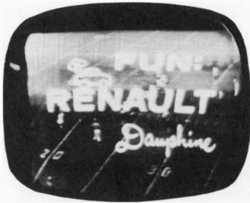
Fig. 1217. *Wiggling vertical lines can be caused by excessive signal.*
