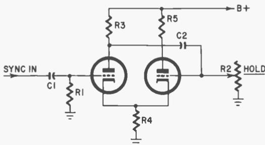
Fig. 305. Typical cathode-coupled multivibrator circuit to illustrate true and apparent squegs in this type of oscillator.
