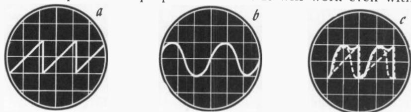
Fig. 704. These drawings show in more detail how the waveforms of Fig. 703 are developed. The oscillator produces a sawtooth (a). The ringing coil adds a sine wave (b). The combination of the sine wave and sawtooth (c) is the waveform illustrated in Fig. 703.
