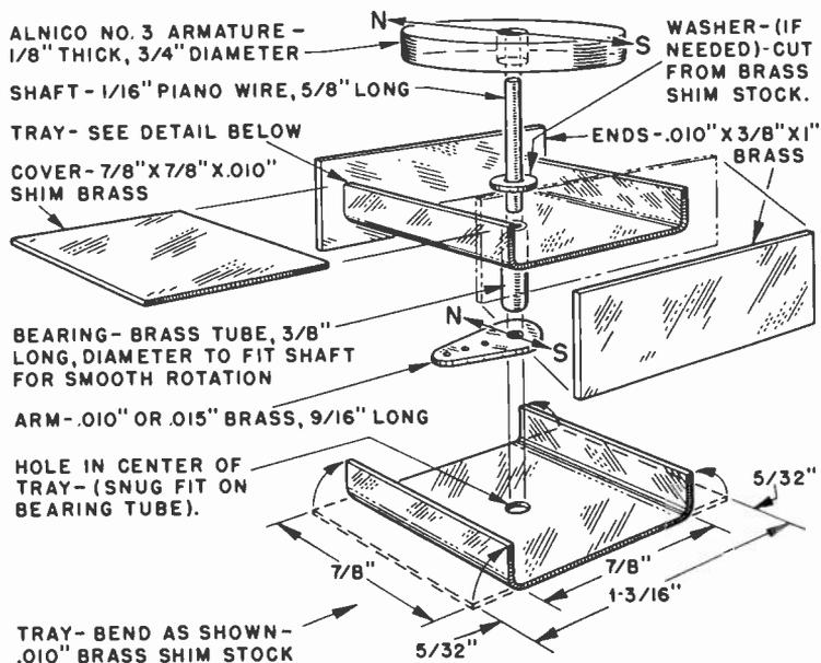
Fig. 210. Simplified style of disc-magnet actuator. This unit has no iron, except in the magnet and in the shaft.
