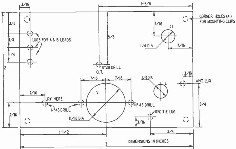
Fig. 410. Suggested layout for the base of the hard-tube receiver.
