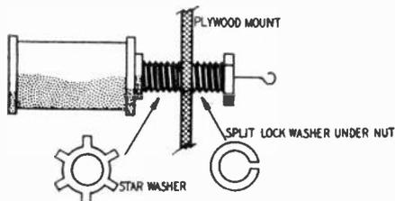
Fig. 904. Single-hole mount escapement must not turn.
