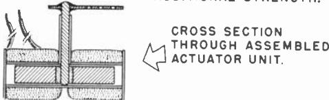
Fig. 212. Construction details of the actuator coil.
