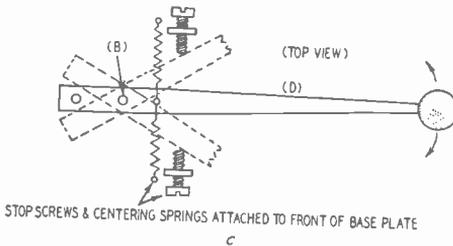
Fig. 809-a. Complete mechanism (a), side view (b), and top view (c) of the control lever. The stops for the lever should be set so that the total movement of the control knob is approximately three inches, or less.
