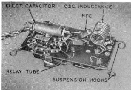
Fig. 505. Receiver parts are mounted on a bakelite base.
