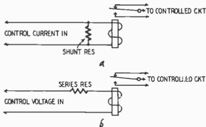
*Fig. 1226-a. -b. The shunt resistor (in the illustration at the top) reduces sensitivity and adapts a low-current relay to a high-current control circuit. The series resistor (bottom illustration) reduces the sensitivity and prevents voltage breakdown in the coil of the relay.*
