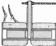
CROSS SECTION THROUGH ASSEMBLED ACTUATOR UNIT.
