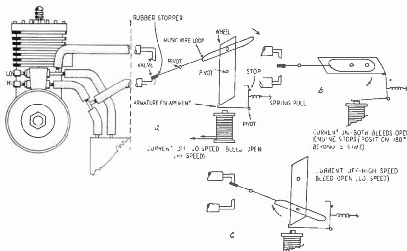
Fig. 302. (left) and Fig. 303 (right). The illustration to the left of the dashed lines shows the "plumbing" for dual needle valves. The drawings, a, b, and c, indicate the steps in motor-control escapement operation.
