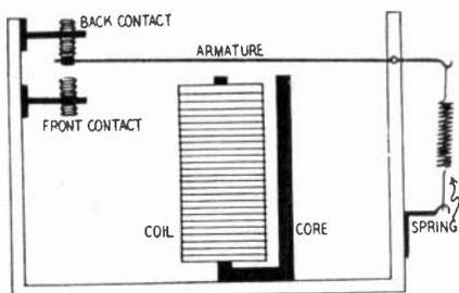
*Fig. 1225. This drawing shows the construction of a typical double-throw type of relay. A single armature may carry several independent moving contacts.*
