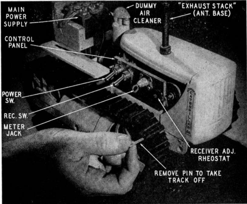
Fig. 1215. Photo of a tractor operated by radio control. A dummy exhaust stack is fitted to the top of the tractor and serves as the base for a vertical antenna. Commercial receiver and transmitter kits are used in this radio-control job.
