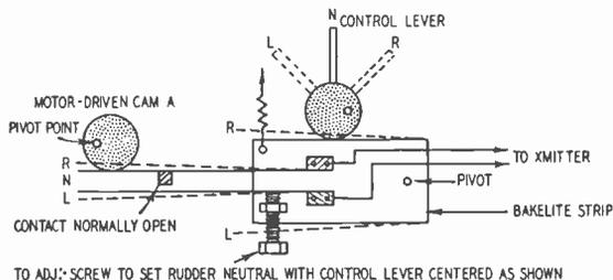
Fig. 203. This arrangement allows variation of proportion of on-to-off signals.
