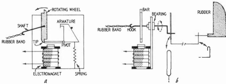
Fig. 103-a, -b. Illustration above shows a front view (left) and a side view (right) of the two-arm escapement.
