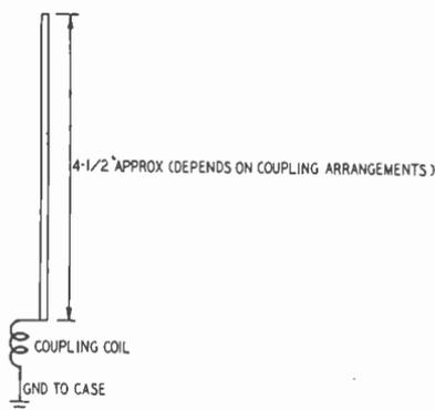
*Fig. 704. Simple 6-meter band antenna is only four and one-half feet in length.*
