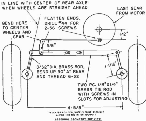
Fig. 1210-b. Top view of the steering-wheel mechanism. With the steering gear in the center position, the wheels are set for the car to move straight ahead.
