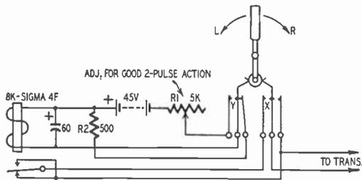
Fig. 807. Relay pulse sender for the compound escapement. Adjust the potentiometer, R1, until you get the desired pulse action. Lever to L, gives one pulse and hold for left turn; lever to R, gives two pulses and hold for right turn; lever to R, then to L, gives three pulses for motor escapement actuation. Points X should close before points Y in the R position.
