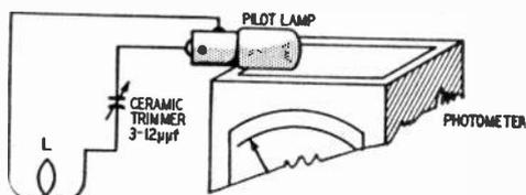
*Fig. 1111. Simple transmitter-output tester. The coil, L, is wound flat, so that it can be slipped between turns of the transmitter plate coil. L consists of 4-3/4 turns of no. 24 insulated wire, 1" in diameter, air wound. In use, a cover is put over the bulb and the top of the meter to keep out stray light.*
