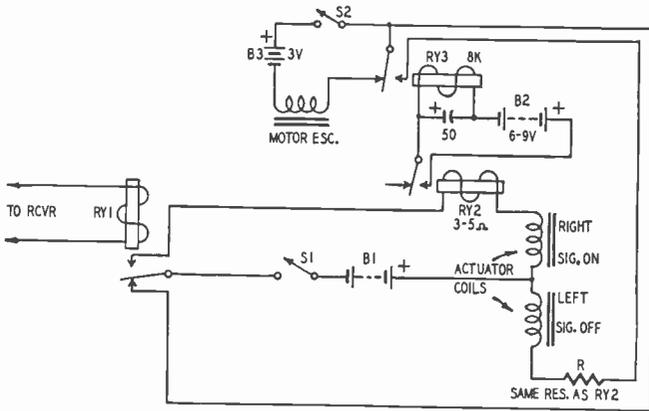
Fig. 314. Close S1 to operate rudder. After pulsing has started, close S2. Secondary relay, RY3, opens when pulses cease. All relays are shown in the signal-off position.
