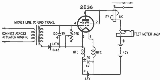
Fig. 313. The addition of a tube gives more reliable pulse-rate change operation.
