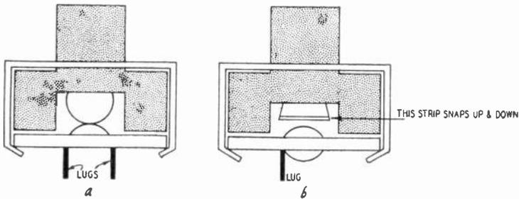
Fig. 908. Cross-sectional views of ball and snap switches. Avoid these. In the illustration at the left (a) the contacts are in the center of the slide and are hemispherical, ball bearing type. Snap switch (b) also has small contact surface area.
