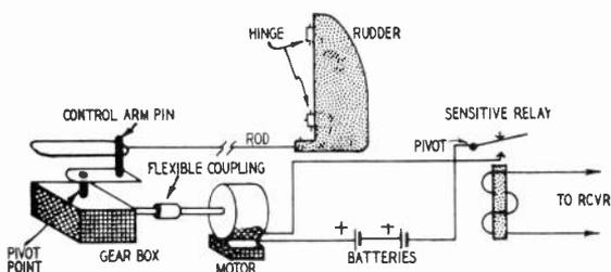
Fig. 102. *The geared-down motor gives lots of power, but relatively slow rudder movement.*
