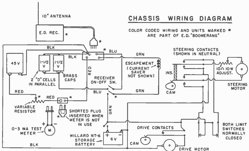
Fig. 1213. Wiring diagram of the chassis. You can control the speed of steering by experimenting with the setting of the slide on the 10-ohm resistor.
