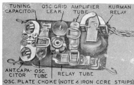
Fig. 504. Receiver occupies minimum amount of space.
