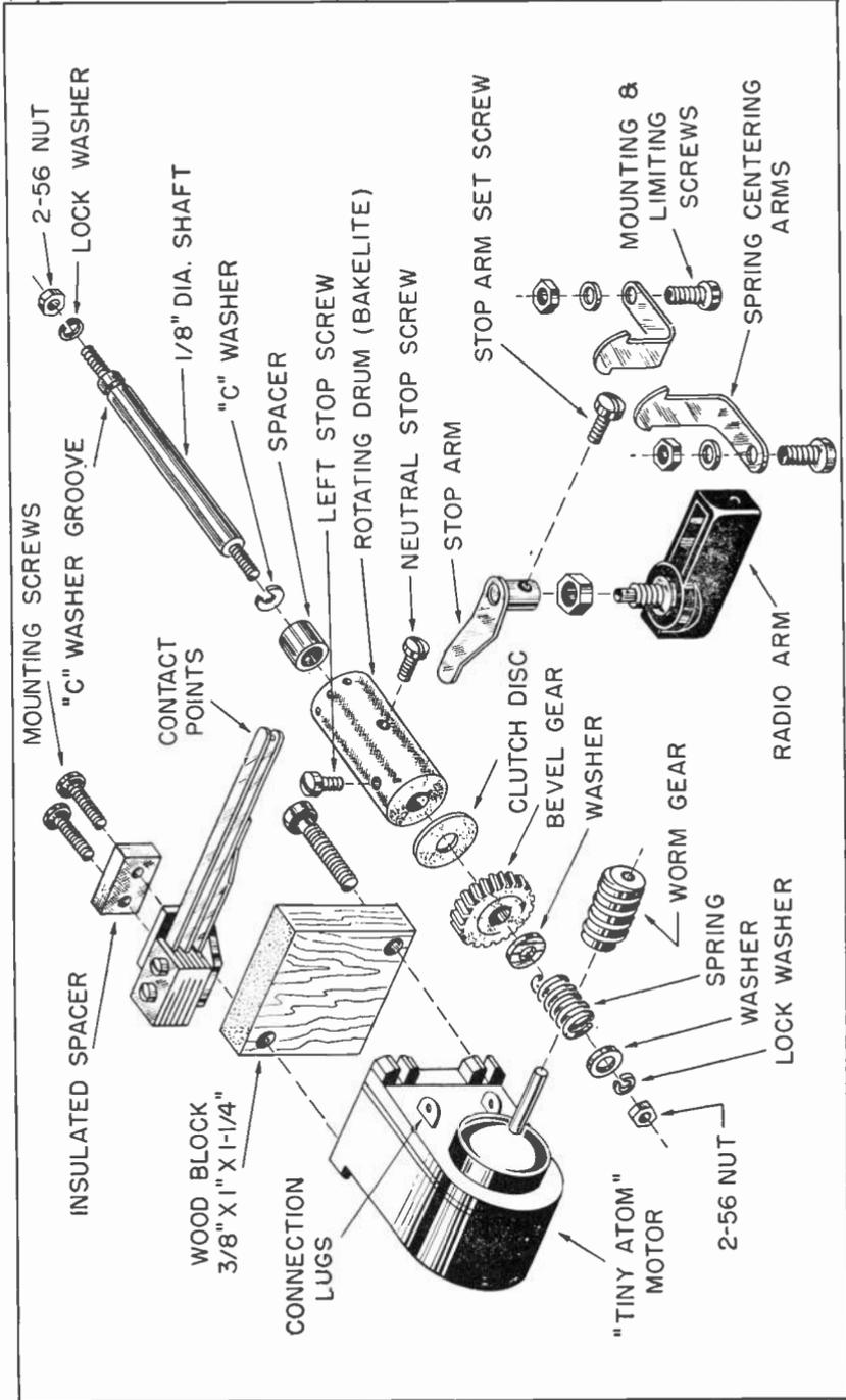
Fig. 803. Exploded view showing parts and assembly of beehive. The drum is operated by a motor through a worm gear.
