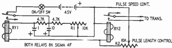
Fig. 811. The twin-relay pulser is more satisfactory for some uses.
