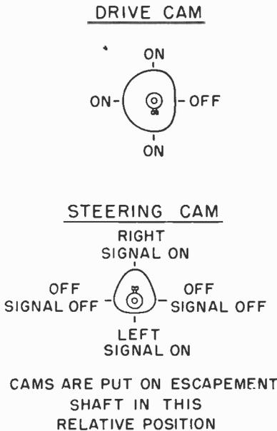
*Fig. 1212. Drive cam and steering cam details. Note how the cams are positioned on the escapement shaft.*
