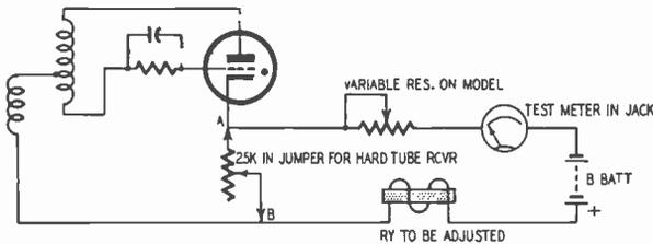
Fig. 1002. The B battery and variable resistor mounted in the plane make a good test circuit if the resistor is of high enough value. Most hard-tube receivers do not use this resistor. Put it in the connection from A to B.
