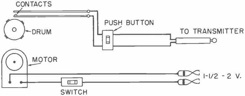
Fig. 805. Top view shows how stop screws on drum push contact points. Lower view illustrates how motor is connected to low-voltage source through a switch.
