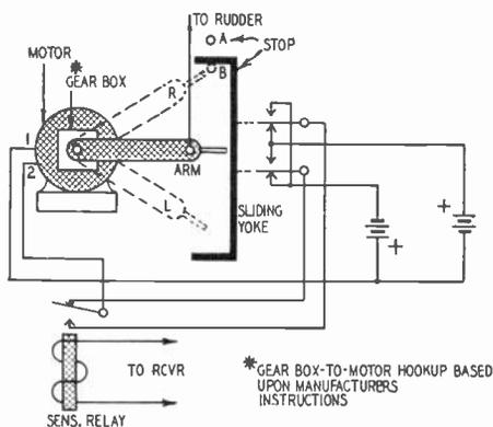
Fig. 213. Safety reverse system goes into action if radio equipment fails.
