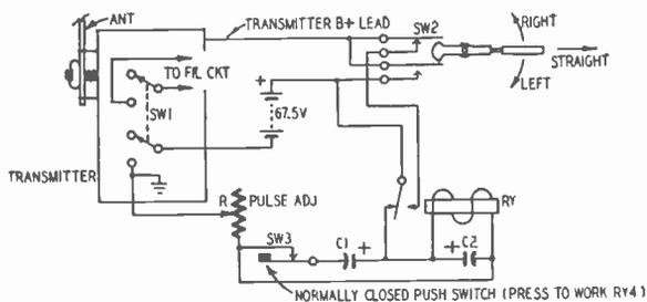
Fig. 1222. Pulsing control unit used for the radio-controlled tractor. Details of the transmitter circuit are not shown since this is supplied with the kit.
