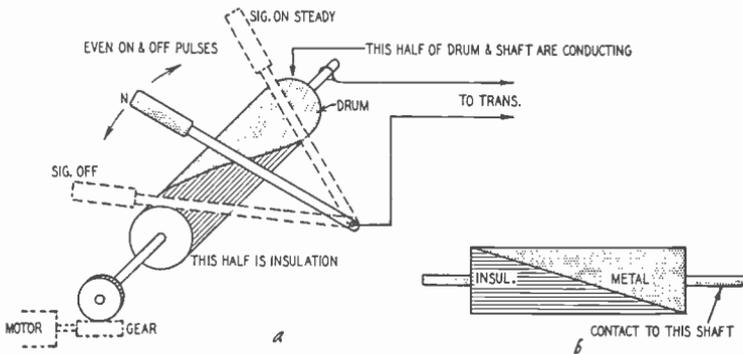
Fig. 814. *The Knipple pulser. Essentially the pulser is a drum, half of which is conductive, the other half insulated.*
