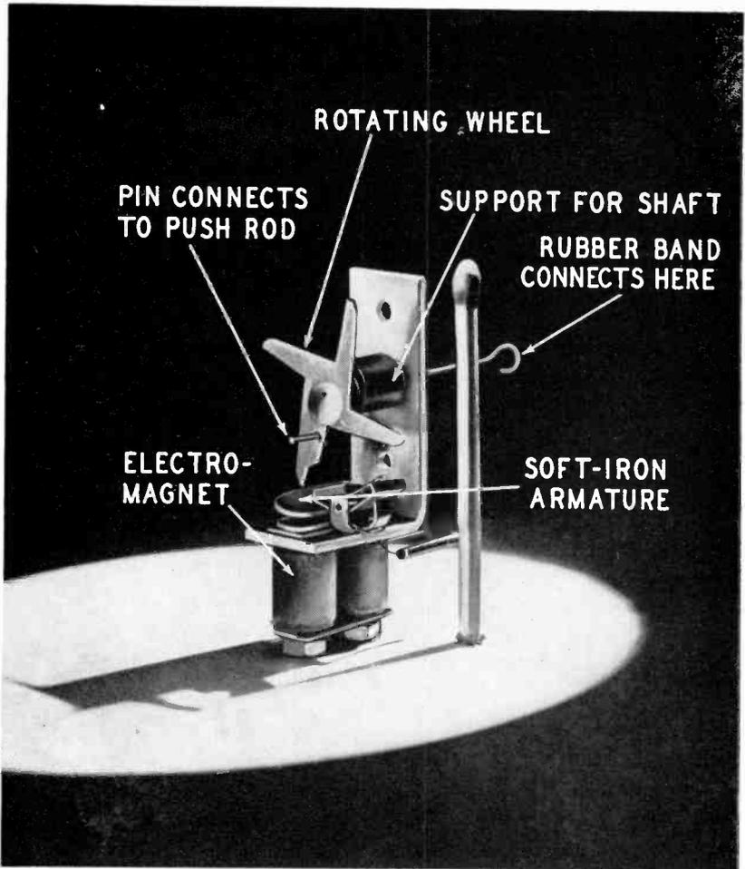
*Fig. 107. Photo of a four-arm escapement. When current flows through the coils of the electromagnet, the soft-iron armature pulls down, releasing the rotating wheel for a 45° turn. The escapement is turned by a rubber band.*
