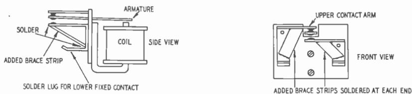
Fig. 506. Side view and front view of Kurnan relay with braces applied to the contact arms.
