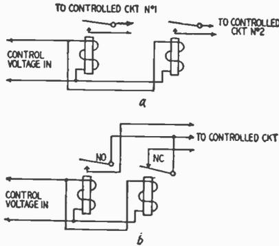
Fig. 123-a, -b. In the top illustration we have a common method of adapting two s.p.s.t. relays for d.p.s.t. use. In the figure at the bottom we have two s.p.s.t. relays (one normally closed) in a s.p.d.t. application. (NO-normally open; NC-normally closed).
