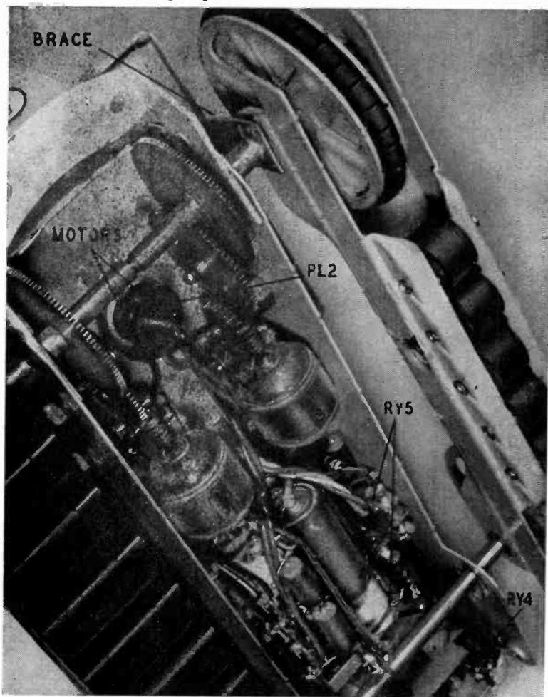
*Fig. 1216. Details of the drive system. Each rear wheel of the tractor is operated by a separate motor. The front wheels are free turning. The motors are geared way down, so there is more than enough driving power.*
