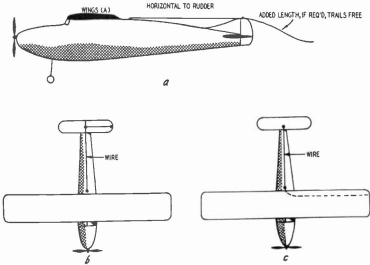
Fig. 910. The antenna can be a single length of wire with a trailing length (a) or it can form an L (b and c). In the illustration at the lower left (b) the wire runs to the top of the rudder, then out to the stabilizer tip. In the picture at the lower right (c) the wire goes to the rudder. Another wire is cemented to the trailing edge or is placed inside the wing, as shown by the dashed lines.
