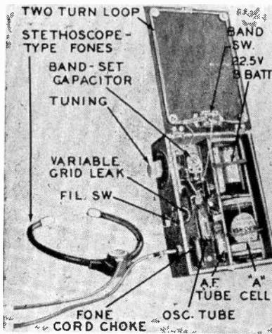
Fig. 1107. Direction finder with cover in operating position.
