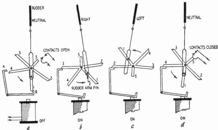
Fig. 108. Steps in the operation of a compound escapement. For the sake of clarity, the text refers to arm 5; however the compound escapement does not really have a fifth arm, the contacts being closed by a lug punched up on the ratchet wheel.
