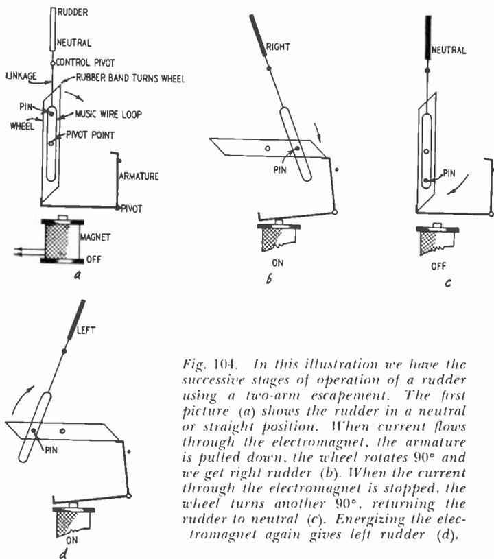
Fig. 104. In this illustration we have the successive stages of operation of a rudder using a two-arm escapement. The first picture (a) shows the rudder in a neutral or straight position. When current flows through the electromagnet, the armature is pulled down, the wheel rotates 90° and we get right rudder (b). When the current through the electromagnet is stopped, the wheel turns another 90°, returning the rudder to neutral (c). Energizing the electromagnet again gives left rudder (d).
