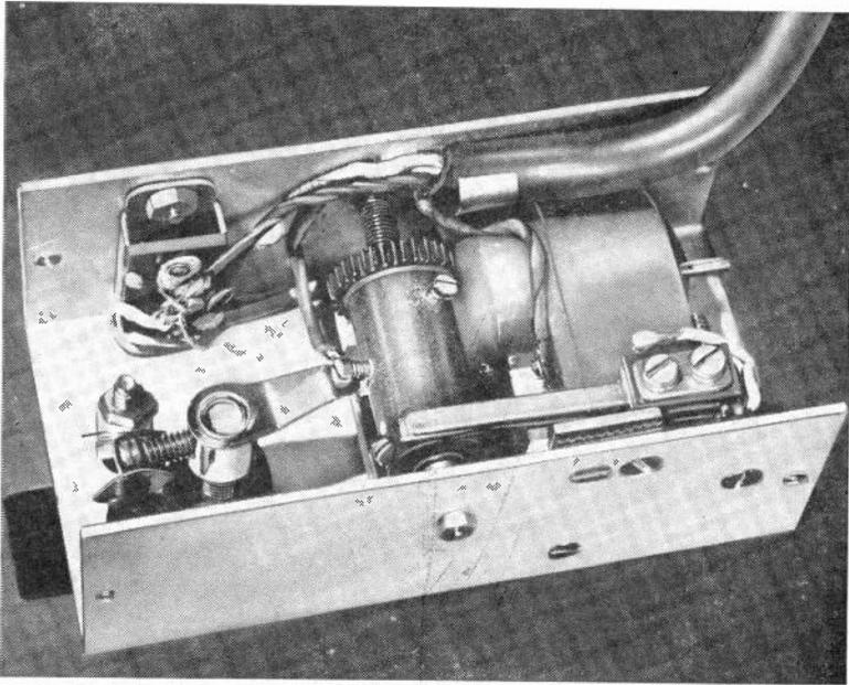
*Fig. 802. This beep box utilizes a small motor geared to a drum having stop pins.*
