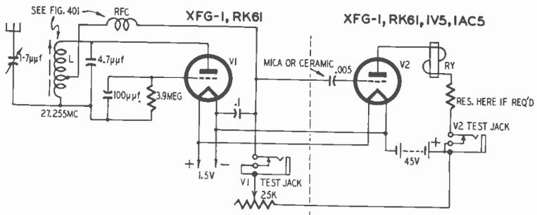
Fig. 501. The two-tube receiver can use either gas or hard tube in second position.
