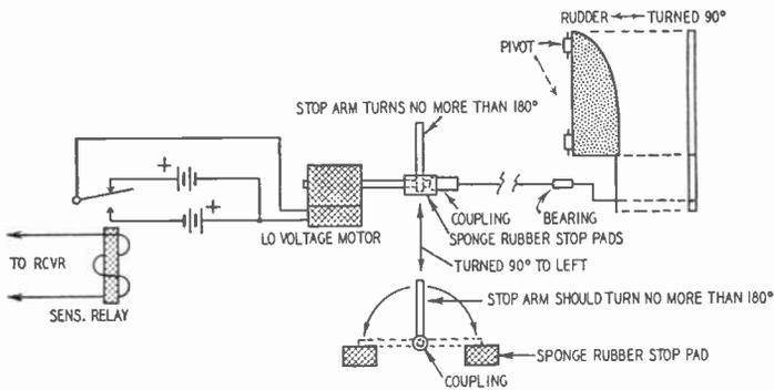
Fig. 205. A low-voltage motor can be used to move a rudder or elevator.
