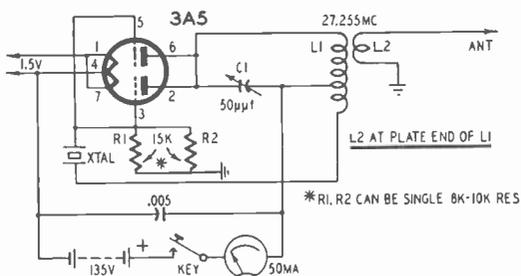
Fig. 608. Transmitter circuit after modification for 27.255 mc. L1, 12 turns #16 enamelled wire, on form 1-1/8" long, 5/8" i.d. Tap at second turn. L2, 4 turns #16 enamelled wire close-wound on form 5/8" i.d.
