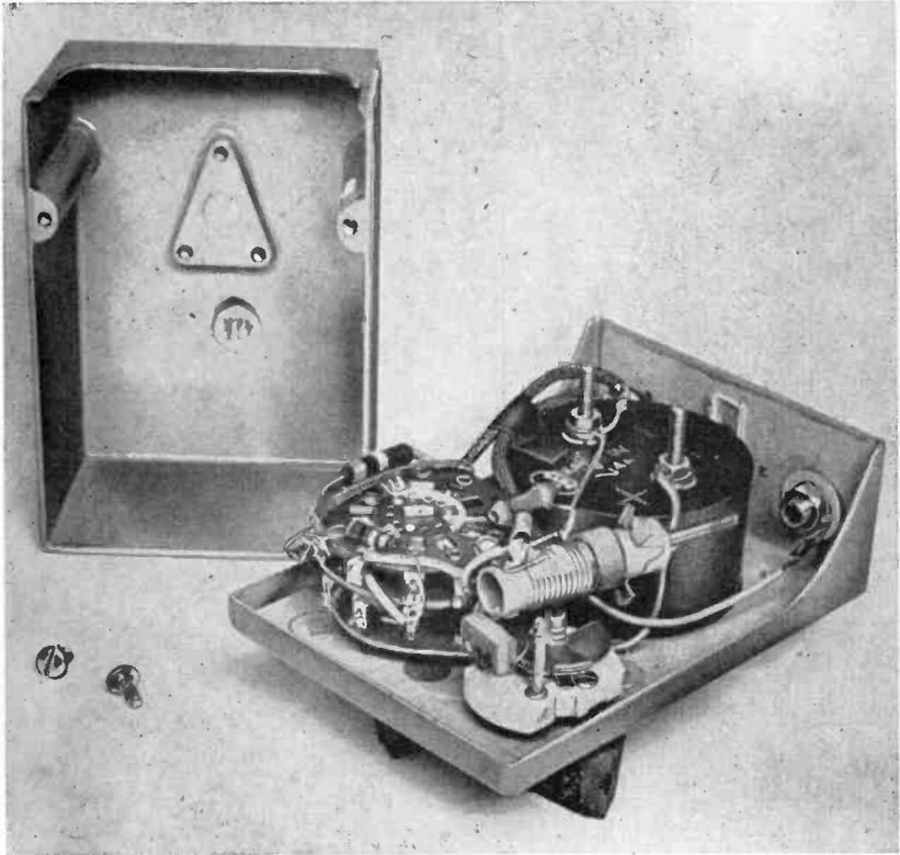
Fig. 1103. Inside view of the combination test meter. All the parts are mounted on the cover.
