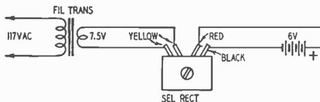
Fig. 1214. This very simple circuit will help you keep the storage battery fully charged.
