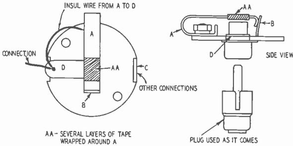
Fig. 1005. Popular phono jack can be converted into closed-circuit type.
