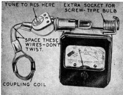
Fig. 1113. Photograph of the completed tester. The cardboard cover for the bulb is not shown.
