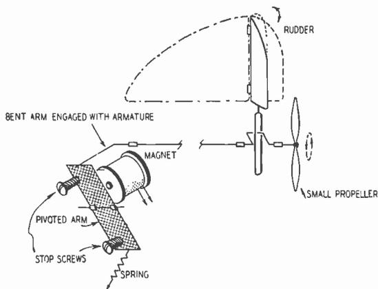
*Fig. 118. In the illustration at the left we have a simple rudder control system for light-weight model planes. When the magnet is energized, the armature engages the linkage going to the rudder. The motion of the propeller (during flight) moves the rudder back and forth until the electromagnet becomes energized.*
