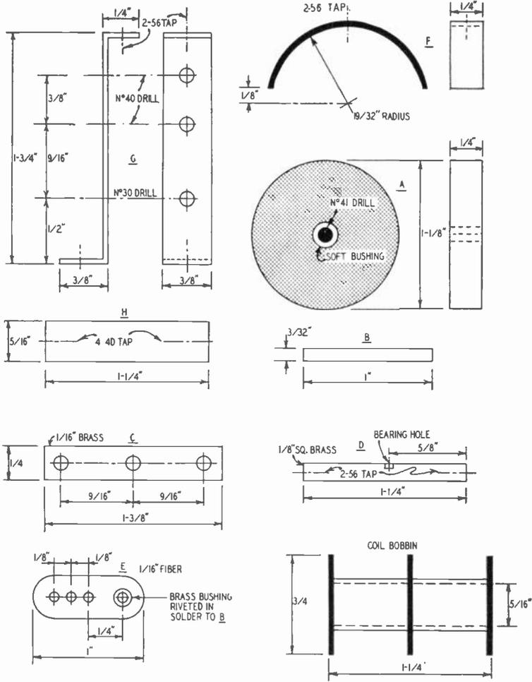
Fig. 208. Dimensions of the parts needed for the actuator illustrated in Fig. 206.
