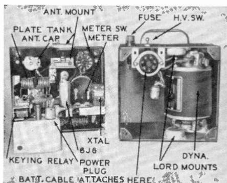
Fig. 706. Inside view of high-power transmitter.
