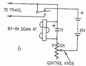
Fig. 810-a, -b. Here we have a simple relay proportional pulser. In the illustration (a) a three-position lever switch is used while knob control is used in the schematic at the right (b).
