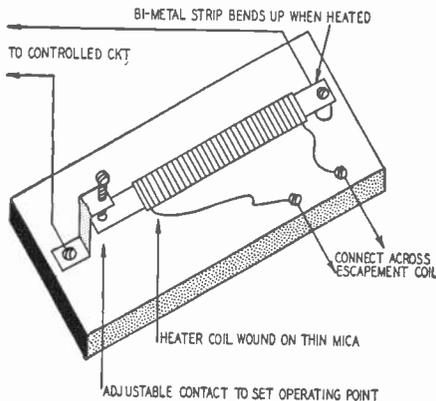
Fig. 309. Thermal release device uses bimetal strip.
