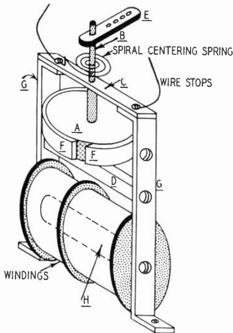
Fig. 206. Disc-magnet type rudder actuator. The letters on each part correspond to similar letters in the detail drawing of Fig. 208.
