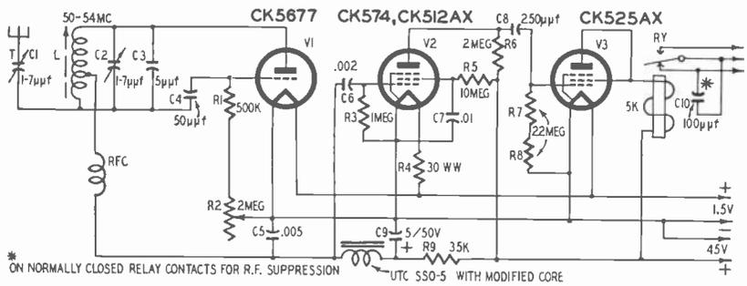
Fig. 503. Three-tube receiver. For the 50-mc band, coil L consists of 11 turns of #16 wire, center tapped, wound on a form 7/16" i.d., 1-1/4" long. The sockets are Cinch, subminiature 5 prong. The choke (RFC) is on a form 3/16" diameter and 5/8" long, wound full of #36 enamelled wire.
