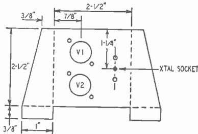
Fig. 712-c. Tube and crystal socket shelf. Bend up on all dotted lines. Cut holes to suit sockets used.
