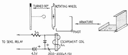
Fig. 116. Delay circuit for the escapement coil is simple, uses only a resistor and capacitor.
