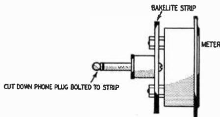
Fig. 1004. Keep receiver test-meter leads short. Mount the meter right on the plug.
