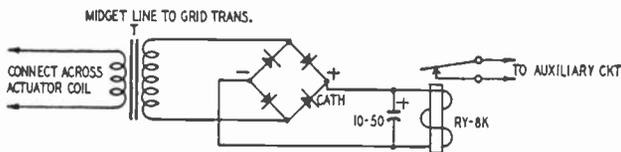
Fig. 312. Circuit for utilizing pulse-rate change.
