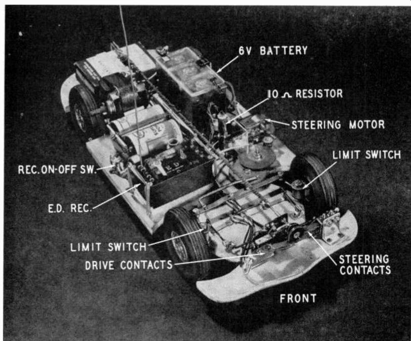
*Fig. 1209. This is a photo of the chassis taken from the front. The drive motor is used to operate one of the rear wheels. Running this car will require some practice. The 10-ohm resistor is used to slow down the speed of the steering motor.*
