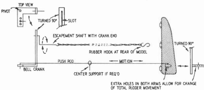
Fig. 901. There are two techniques for getting rudder motion—push rod and torque rod. Illustration above shows push-rod method.
