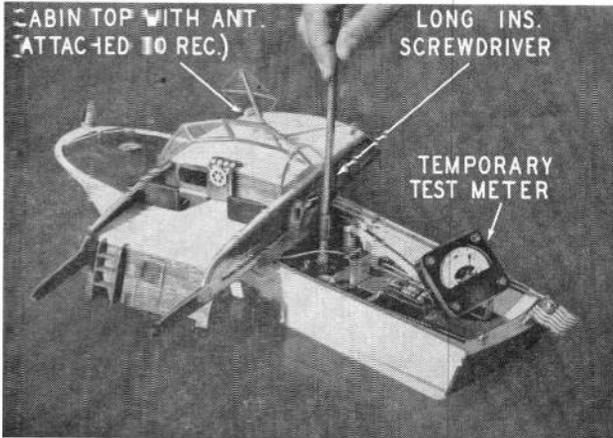
Fig. 1204. This photo shows the boat in the water and the receiver in process of adjustment. The cabin is placed across the hull, and the test meter is plugged into the closed-circuit jack. The boat should always be on the water when the receiver is tuned.
