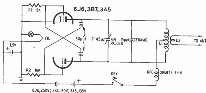
Fig. 702. Circuit of push-pull radio-control transmitter for use on 11-meter band. This unit can only be operated by licensed amateurs. For a 6J6, heater battery should be 6.3 volts. Do not use this transmitter on the 27.255-mc spot. See Fig. 701 for coil values.
