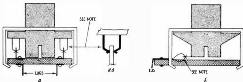
Fig. 907. Cross-sectional views (a and b) of reliable slide switches. Note: Detail (aa) shows how double sliding contact is obtained by using both sides of a fixed contact. The same sort of double contacts are used in the illustration at the right (b) but they are stationary in this type.
