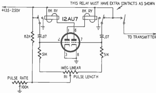
Fig. 812. Multivibrator-type pulser. Control knob or lever can be used to operate R1.
