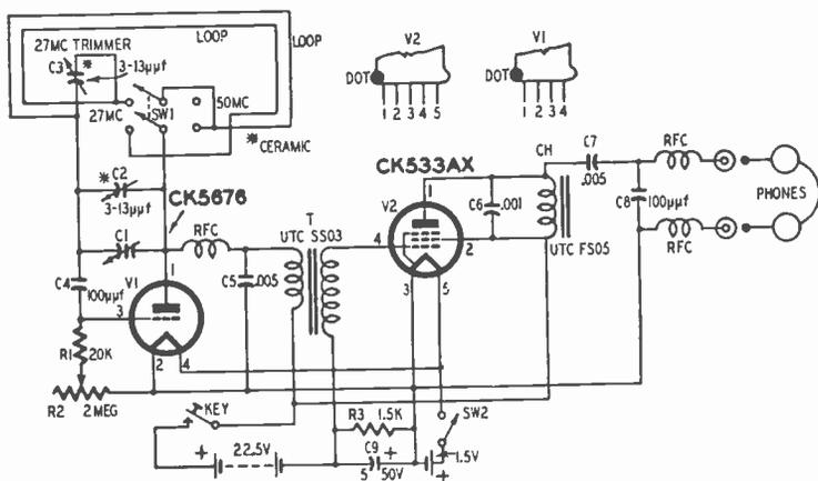
Fig. 1108. Circuit diagram of the direction finder. The radio-frequency chokes are made of 135 turns of no. 34 enamelled wire wound on a form, 1/4" in diameter and 1" long. The antenna is a double loop (3-1/2" x 5") of no. 22 double-cotton covered wire. The outer turn is used for 50 mc, both turns in series for the 27.255-mc spot.
