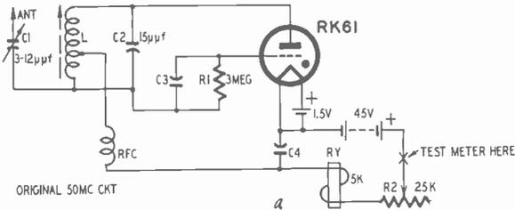
Fig. 412-a. Circuit of gas-tube receiver prior to conversion.
