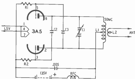
Fig. 607. Conventional 3A5 push-pull 50mc transmitter. This circuit is a self-excited oscillator, but it can be converted to a crystal-controlled transmitter for work on the 27.255-mc spot, as shown in Fig. 608.
