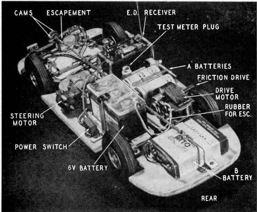
Fig. 1208. Photo of the inside of the Porsche car. All the works are below window level, adding to scale effect. The antenna is an elongated whip. The rubber band for the escapement runs practically the complete length of the car.
