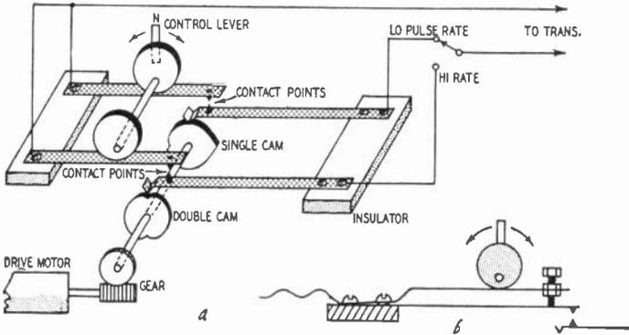
Fig. 813. Mechanical system for producing independent pulse rates. The use of two cams allows instant selection of two pulse rates (a). A fine adjustment for neutral can be added to the left-hand contacts as shown in lower right (b).
