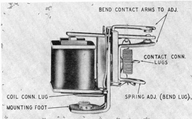
*Fig. 1224. Picture of a sensitive relay. A spring, one end of which is connected to the armature, controls the sensitivity of the relay. The greater the spring tension, the less the sensitivity will be. In some relays the spring is connected to an adjustment screw. If there is no such adjustment, it will be necessary to stretch the spring to increase sensitivity. Do this carefully; avoid overstretching.*
