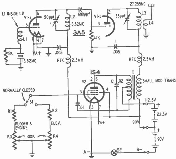
Fig. 714. This transmitter is for use with a reed receiver. The unit modulates with two different tones, depending upon the position of S1. A third audio tone can be easily added. The tones can be varied by adjusting the setting of potentiometers R3 and R4. L1, 20 turns of #22 enamelled wire on form 3/8" o.d.; L2, 24 turns, L3, 10 turns, L4, 4 turns, #22 enamelled wire on 1/2" dia. form. For L2, L3, and L4 you can use B & W Miniductors, #3004. All variable capacitors receiving type.
