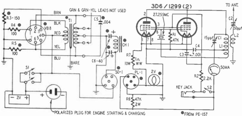
Fig. 710. Circuit diagram of the transmitter, popularly known as the Mac II. L1, 10 turns #14 wire. Tap at second turn. L2, 8' turns #20 insulated wire. See also Fig. 711-C. All variable capacitors receiving type.
