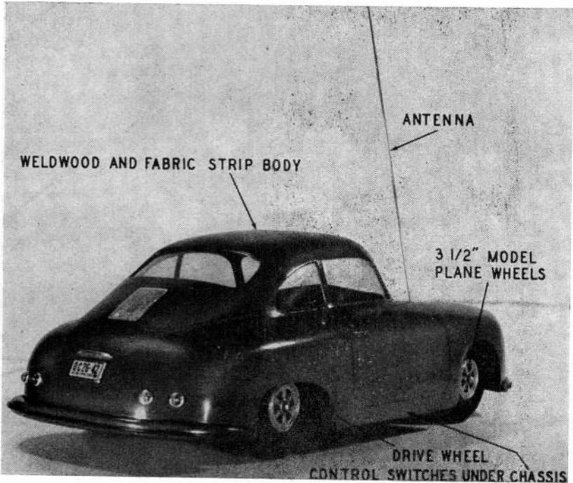
Fig. 1207. This is a close scale copy of a real Porsche Sports car. Standard  $3\frac{1}{2}$ -inch diameter model-plane wheels are used. Careful sanding will produce a fine finish on the car.
