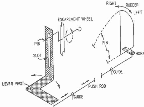
Fig. 112. The push-rod linkage is fine if carefully made and adjusted.
