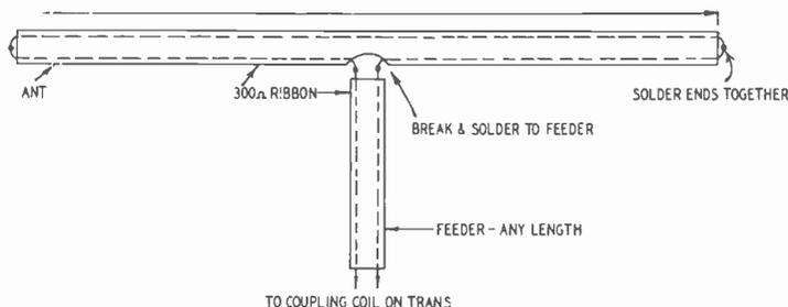
Fig. 609. Half-wave horizontal antenna for use on 27.255 mc. The total length of the antenna, as indicated by the solid arrow, should be 16 feet, 11 inches.
