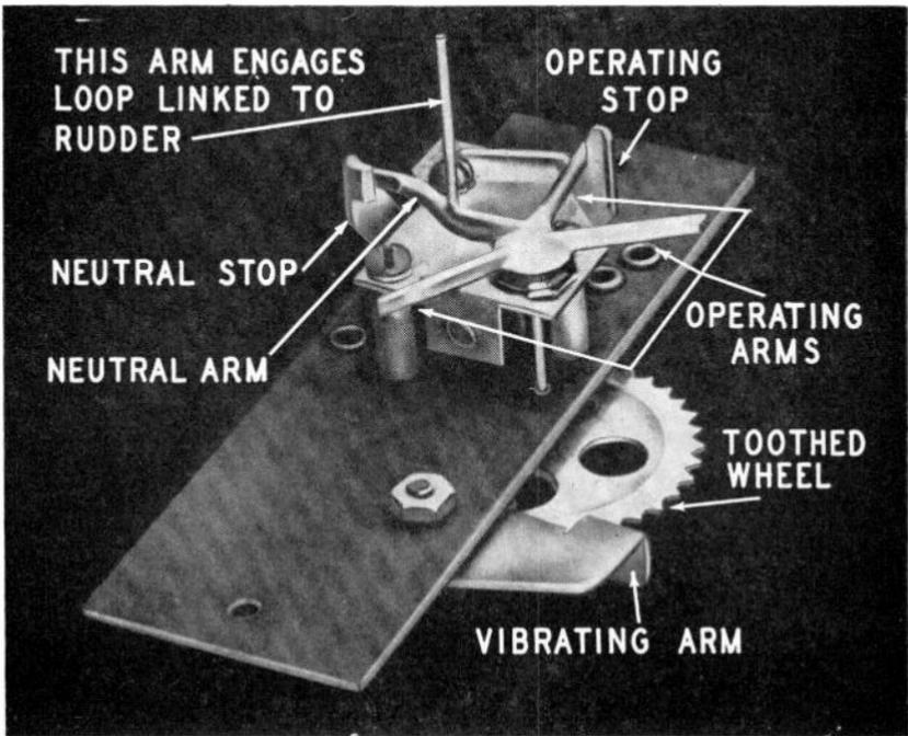
Fig. 109. Photo of a compound escapement. Note the toothed-wheel governor to slow rotor movement.
