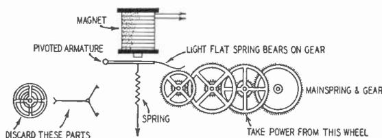
Fig. 115. Very little power is required to control this clockwork escapement which has no set stop positions.
