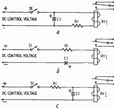
Fig. 1229-a, -b, -c. In the illustration at the top, RY1 remains closed for a short interval after the opening of S1. In the center illustration (b), the relay closes when S1 is closed. It then opens automatically after a timed interval when capacitor C1 is charged. In the illustration at the bottom, the operation of RY1 is delayed on opening or closing control switch S1.
