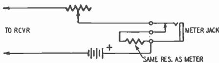
Fig. 1101. *Iron vane meters require compensating resistor across meter test jack.*
