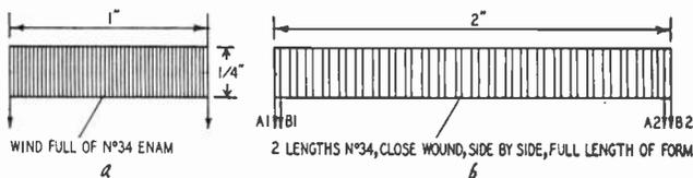
Fig. 817. To keep r.f. out of the pulser you can use individual chokes of the type shown at the left (a) or you can wind two chokes on one form as shown at the right (b).
