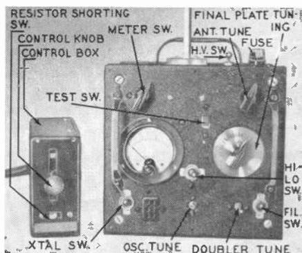
Fig. 705. Front view of high-power transmitter.
