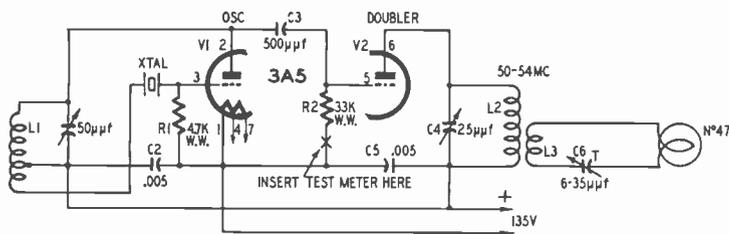
Fig. 703. Transmitter for operation on the 50 to 54-mc band. The fundamental frequency of the crystal should be between 25 and 27 mc. L1, 17 turns #18 enamelled wire on form 1/2" i.d., 1-3/8" long; L2, 9 turns #16 enamelled wire on form 1/2" i.d., 3/4" long; L3, 3-1/2 turns #16 enamelled wire on form having 3/4" i.d.
