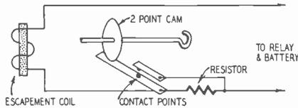
Fig. 113. Escapement gets full power to move armature. Reduced power will hold it operated.
