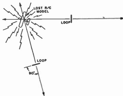
*Fig. 1110. A double "fix" is needed for proper operation of the direction finder. With only a single "fix" the model could be in either direction. A second "fix" (from a different point) makes direction certain.*
