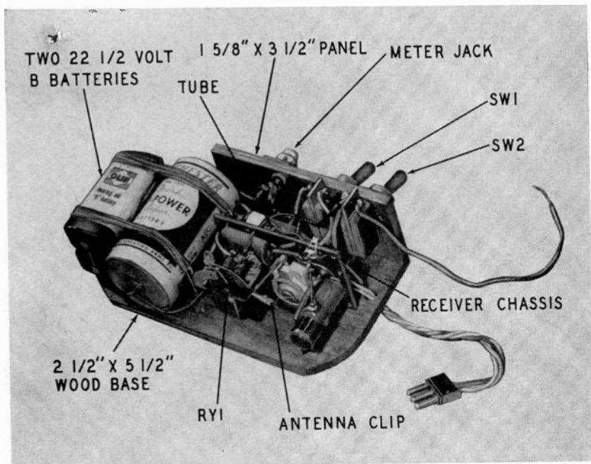
Fig. 1217. Photo of the receiver chassis with the batteries attached. The A and B batteries for the receiver are mounted on the wooden base. The receiver is mounted on edge so that the tuning controls can be reached from the side of the tractor hood.
