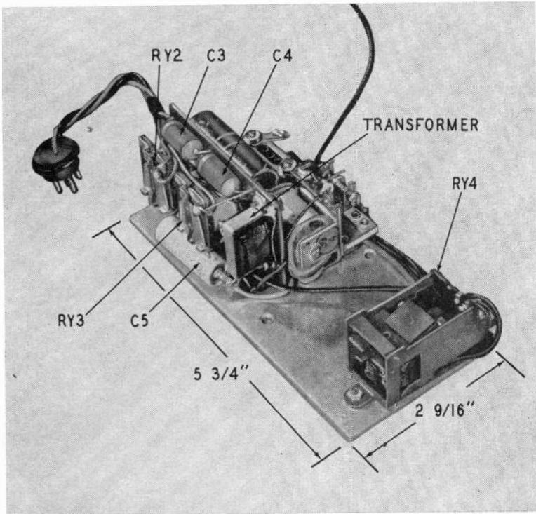
Fig. 1218. Photo of the control chassis. Note RY4 at the lower right. The control chassis, made of aluminum, is held to the underside of the tractor by three screws, two of which are wood screws and run into the receiver base.
