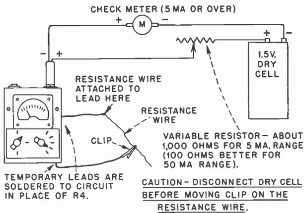
Fig. 1106. Circuit to be used when making your own meter shunts.
