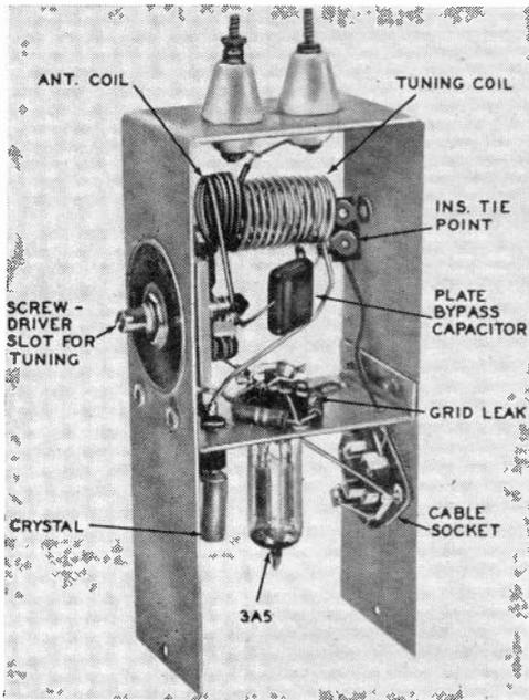
Fig. 611. Another view of the modified transmitter. The unit is connected to the power supply by means of a cable.
