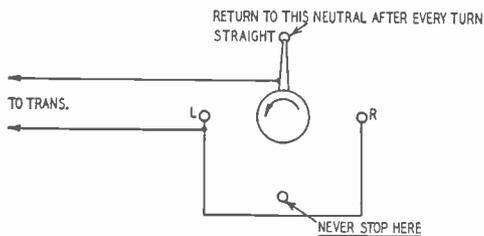
Fig. 801. Rotary switch helps keep escapement pulses in order. Rotate only in direction of arrow on knob.
