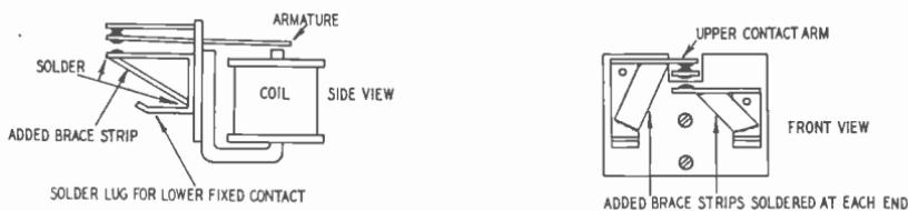
Fig. 506. Side view and front view of Kurman relay with braces applied to the contact arms.
