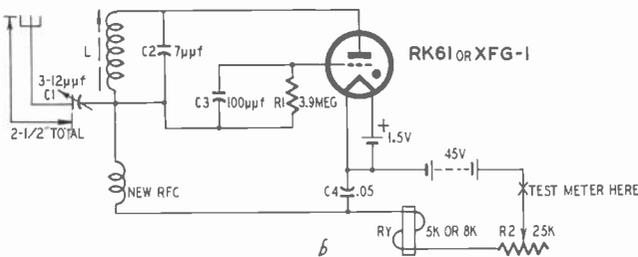
Fig. 412-b. Gas-tube receiver modified for 27.255-mc operation. RFC: ¼" x 1" bakelite form wound full of #34 enamelled wire; L: CTC L53 coil form with red painted slug. Remove brass ring that is threaded on the stem next to the iron slug. Use 20 turns of #24 enamelled wire, centered on the form, and close wound.
