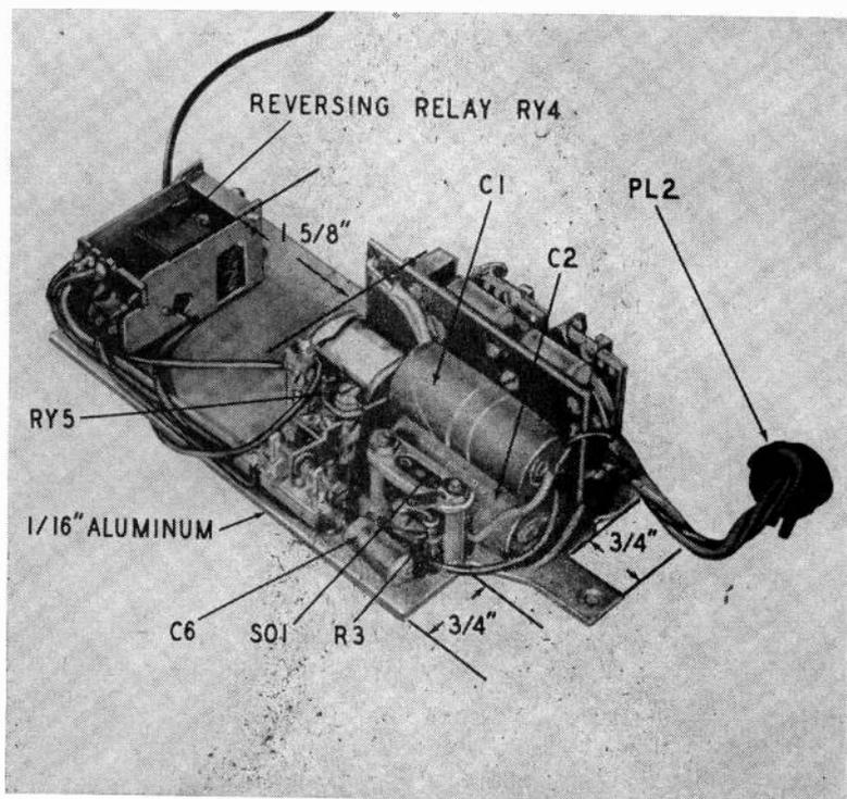
Fig. 1219. Another view of the control chassis. The reversing unit RY4 is mounted as far as possible from RY5, since its heavy magnetic field leads to erratic operation of the sensitive relay, if mounted too close to the latter.
