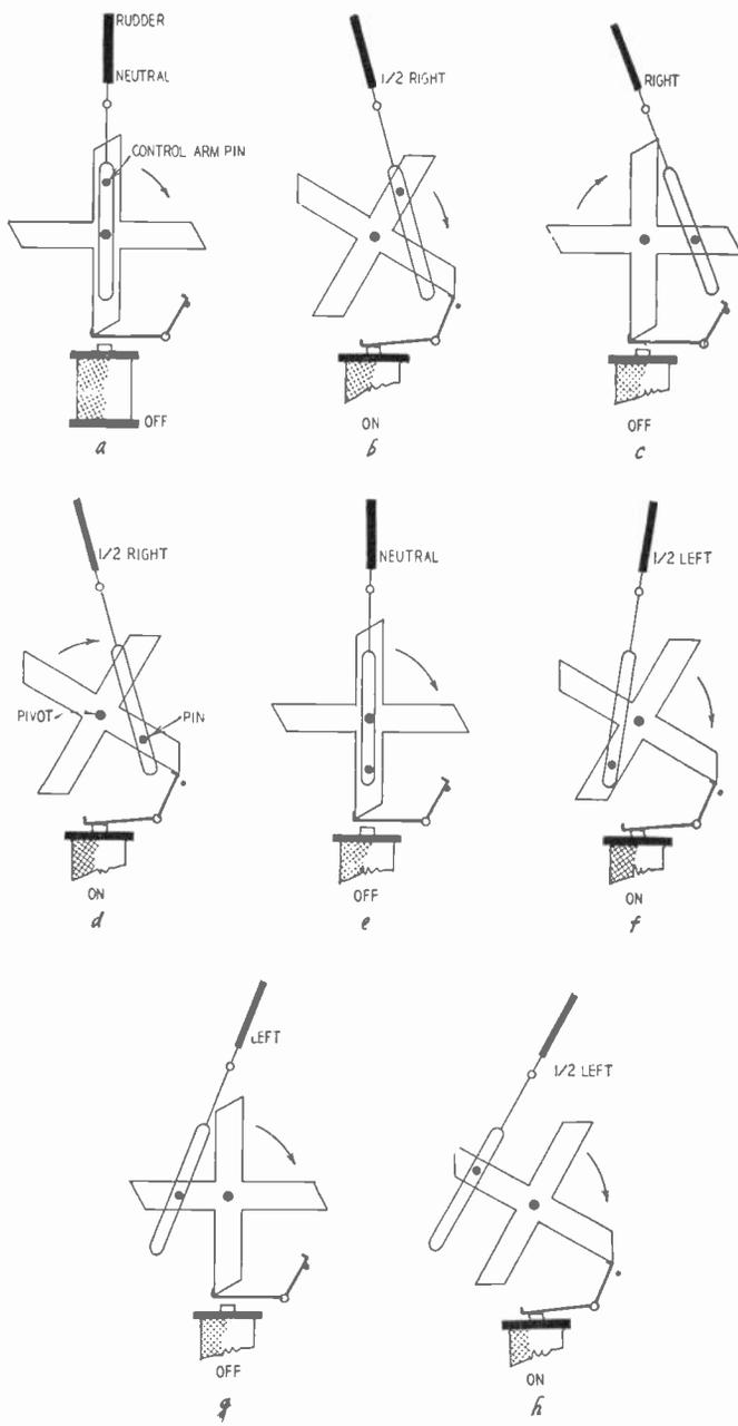
Fig. 106. The four-arm escapement shown above will hold continuous turns without current drain. Like the three-arm escapement, it can supply  $\frac{1}{2}$  right and  $\frac{1}{2}$  left rudder for making shallow turns.
