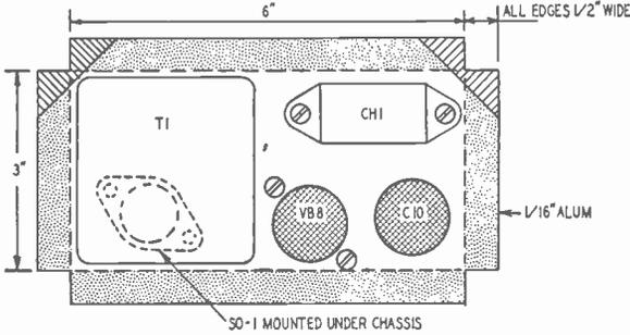
Fig. 712-b. Recommended chassis layout for the vibrator power supply. Bend edges down on dotted lines. Cut off shaded corners. Power supply mounted with 3-3/4" between upper surface and top of case.
