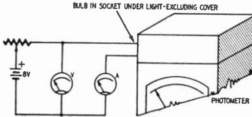
Fig. 1112. Circuit diagram for calibrating the test unit.
