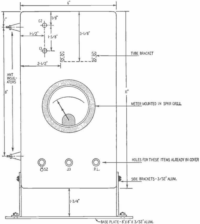
Fig. 712-a. Suggested front-cover layout for the transmitter whose circuit is shown in Fig. 710. In order to carry the unit around, mount a handle on top of the transmitter.
