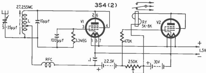
Fig. 502. This two-tube receiver uses a direct-coupled amplifier. For 27.255-mc operation coil L consists of 15 turns of #28 enamelled wire wound on a CTC LS3 coil form. (see Fig. 406). Use a core identified with a white tip. The choke is a 3/4" x 1/4" form wound full of #34 enamelled wire.
