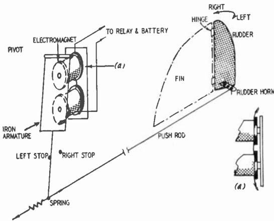
Fig. 101. Simplest possible system to move the rudder. A side view of the electromagnet is illustrated in (a) at the lower right. Note the three holes in the rudder horn.
