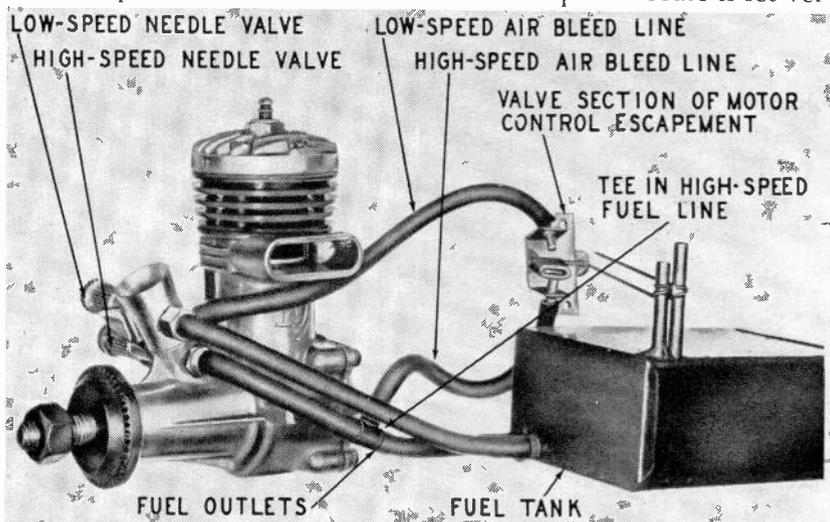
Fig. 304. Two-speed engine fitted with dual needle valves. Engine stops when both valves are opened. Wire loop on valve engages escapement rotor pin.
