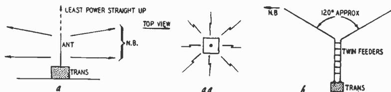
Fig. 911. Quarter-wave vertical antenna (a). N.B. Power is concentrated toward the horizon, and 360 degrees around the antenna (aa). The horizontal half-wave doublet is shown at the right (b). N.B. Least signal is off ends, maximum signal broadside to antenna. Halves of antenna are often inclined upward to give more uniform output signal pattern.
