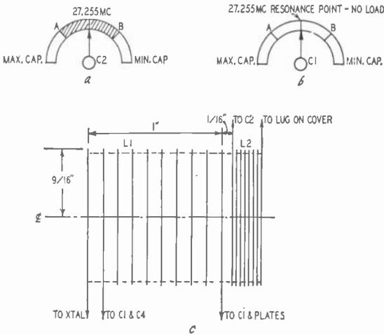
Fig. 711. Tuning procedure (a and b) and coil data (c). Proper loading may be had with C2 near either A or B; C1 will resonate near corresponding A or B.
