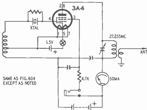
Fig. 605. This circuit gives about 30% more power than that illustrated in Fig. 604. Coils same as Fig. 604.
