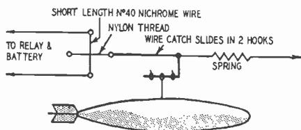
Fig. 311. This gadget will drop a bomb or a parachute.
