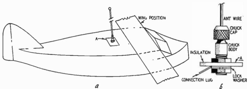
Fig. 909. The chuck from a radio test prod makes a good mount for the antenna (a). A small square of insulation can be set into the fuselage top as shown at A. Illustration at the right (b) shows mounting details.
