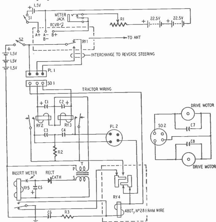
Fig. 1220. Wiring diagram of the entire control system of the tractor. Power for the entire unit (except the receiver) is obtained from three 1.5-volt storage cells. Storage cells can be recharged, but are much heavier than other types.
