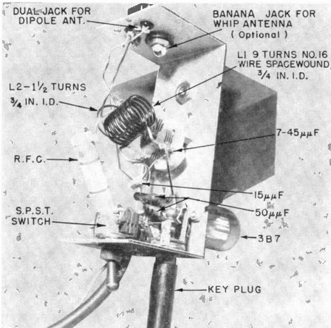
Fig. 701. Photograph shows under-chassis view of push-pull transmitter.
