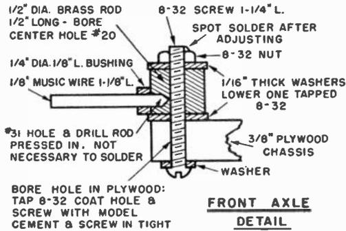
Fig. 1210-a. This illustration shows the detail of the front axle.
