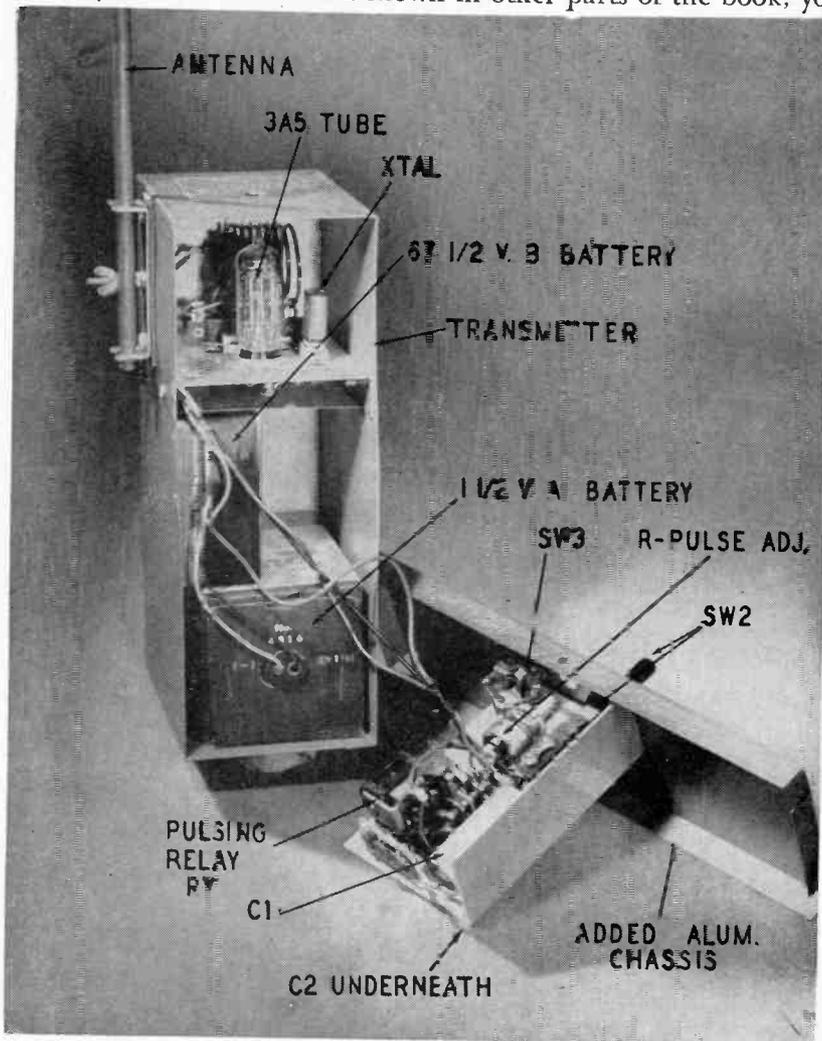
Fig. 1223. Photo of the transmitter and its associated control unit. When assembled, the control unit fits the space immediately above the 1½-volt cell shown at the bottom of the transmitter case. The transmitting antenna at the upper left of the transmitter case, is held in place with a single wing nut. The pulsing relay, RY, is mounted on a piece of insulating material.
