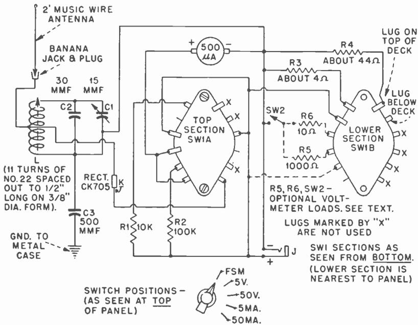
Fig. 1104. Circuit diagram of the combination test meter. The switch connections are tricky, so follow the diagram closely.
