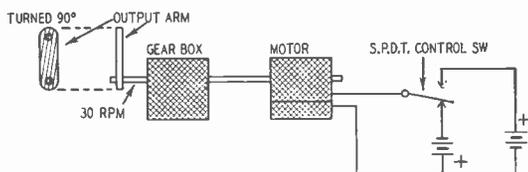
Fig. 201. Simple arrangement for demonstrating semi-proportional control.
