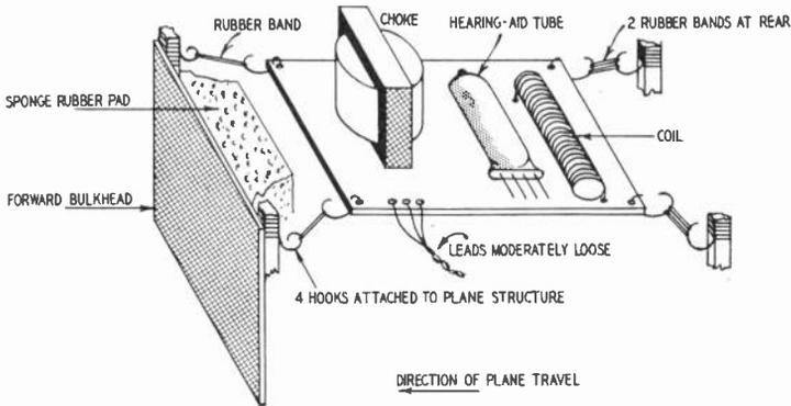
Fig. 906. Technique for mounting the receiver and protecting it.
