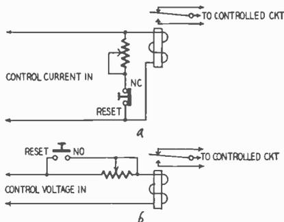
Fig. 1227-a, -b. Two types of self-latching relays. In the upper illustration, the circuit is controlled by a change in current. In the lower illustration, the circuit is controlled by a variation in the applied voltage. (NO-normally open; NC-normally closed)
