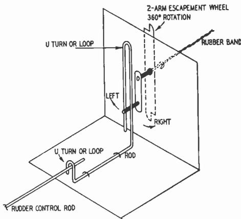
Fig. 111. Simple linkage controlled by a two-arm escapement wheel.
