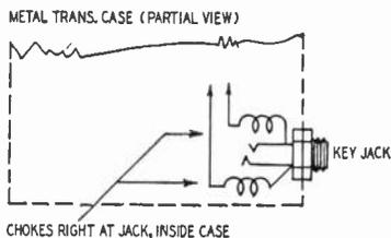
Fig. 816. The use of radio-frequency chokes as shown in the illustration at the left will keep the signal inside the metal case, minimizing the possibility of throwing the transmitter out of oscillation.
