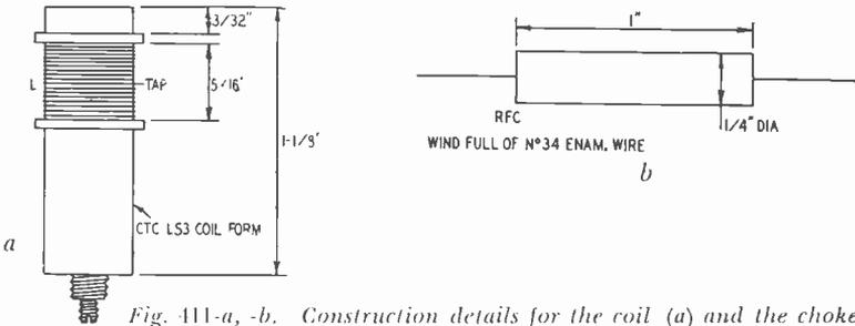
Fig. 411-a, -b. Construction details for the coil (a) and the choke (b).
