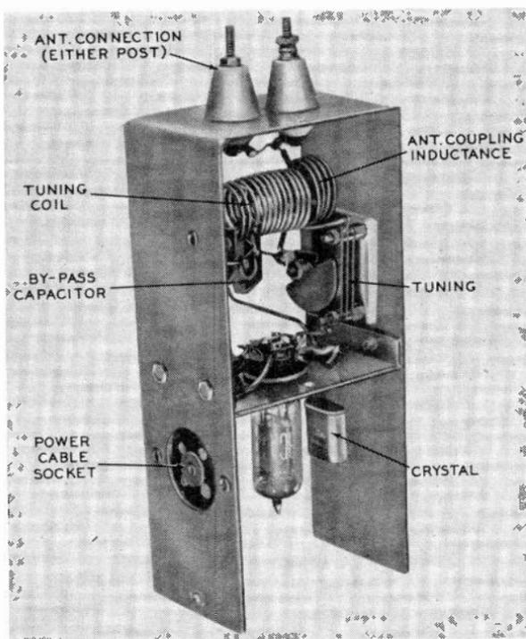
*Fig. 610. Photograph of the rebuilt transmitter. Upside down mounting of the tube permits use of shorter leads, makes for more compact equipment.*
