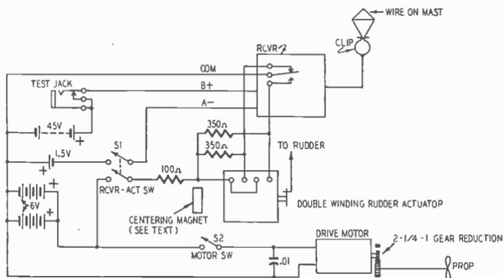
Fig. 1203. Complete electrical diagram of the boat installation. Note that the drive-motor batteries are connected in parallel. Make sure these are of equal strength. Never parallel a good battery with a weak one. The tuning meter should be a 0.3 ma d.c. milliammeter. Keep the receiver plate-current drain below 2 ma.
