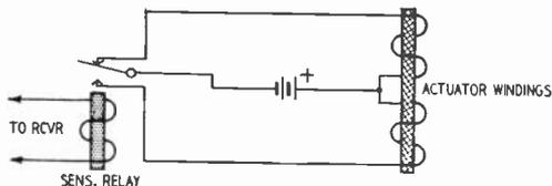
Fig. 207. Preferred actuator hookup uses only one battery.
