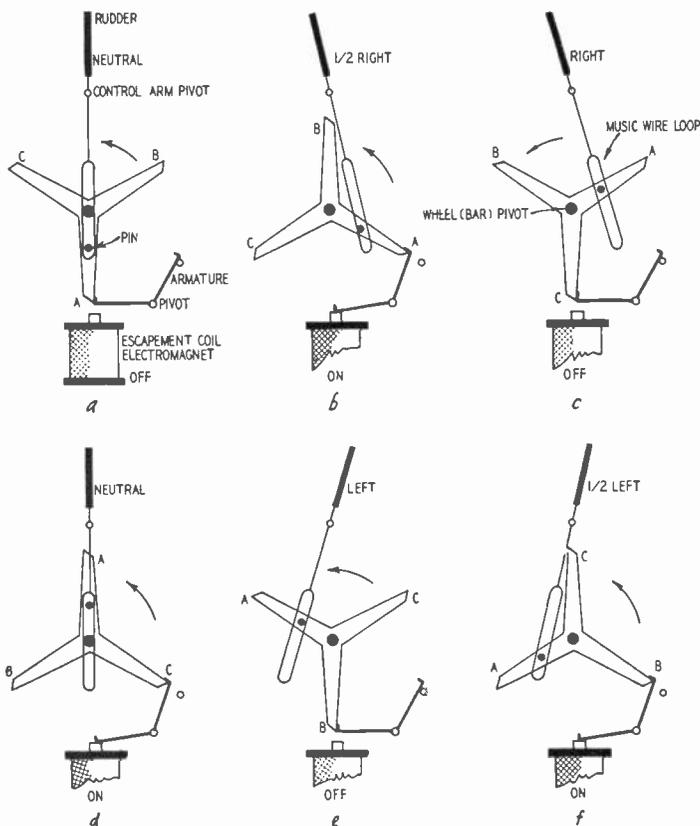
Fig. 105. Positions taken by a three-arm escapement. Such escapements are not very widely used.
