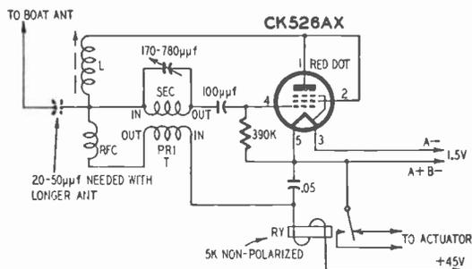
Fig. 1202. Circuit diagram of the single, hard-tube receiver. Special parts needed are: L, CTC type LSM form with red core. Wind 25 turns of no. 34 enamelled wire; RFC, form 5/32" dia. x 3/4" long, wound full of no. 38 enamelled wire (or commercial 10- $\mu$ h unit); T, ESSCO subminiature quench transformer; trimmer capacitor, Arco #469; RY, E. D. 5,000-ohm non polarized; tube is Raytheon CK526AX; base plate, linen bakelite 1-1/2" x 2-1/8" x 1/16"; socket, Cinch subminiature 5 prong.
