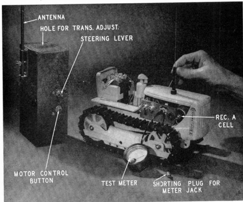
Fig. 1221. Photo of the tractor with receiver in process of adjustment. The transmitter is contained in the box at the left.
