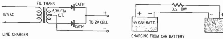
Fig. 713. Techniques for charging the 2-volt cell. The power supply at the left uses a magnesium-copper sulphide full-wave rectifier that was removed from a PE-157 unit.
