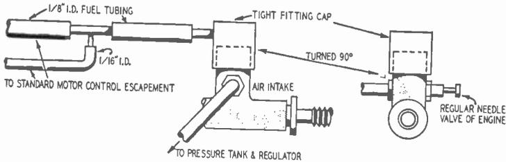
Fig. 308. This arrangement is good for small engines only, unless a special escapement with extra-large valves is used. Low speed, 1/16" line open; medium speed, 1/8" line open; high speed, both lines open; or, low speed, 1/16" line open, high speed 1/8" line open; motor cut, both lines open.
