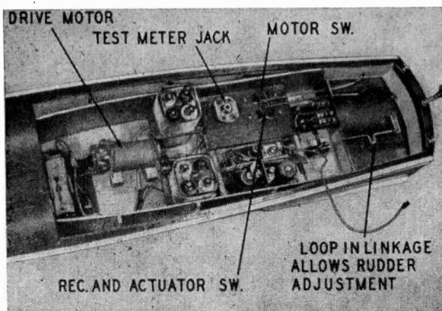
*Fig. 1206. Another interior photo of the boat. The motor is held on two wood blocks by rubber bands, has small gear on shaft. Note the details of the rudder linkage. The A and B batteries of the receiver are located in front of the drive motor.*
