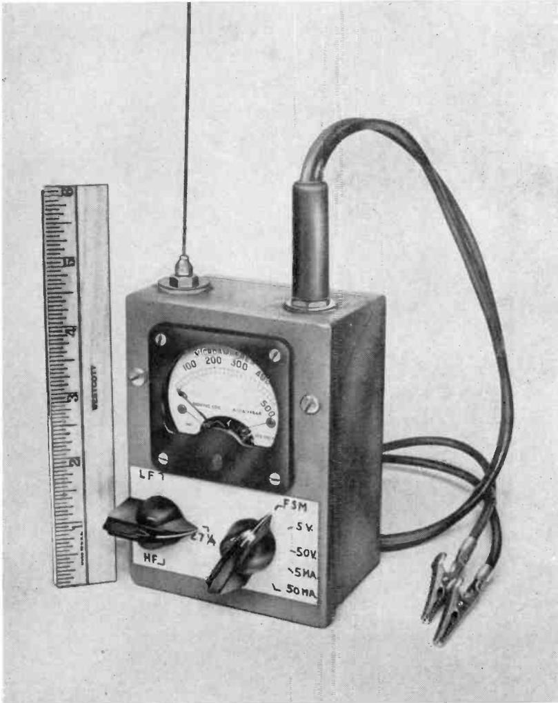
Fig. 1102. Combination test meter can be used for checking transmitter, receiver, or batteries. It can also be used for testing the field strength of the transmitted signal.
