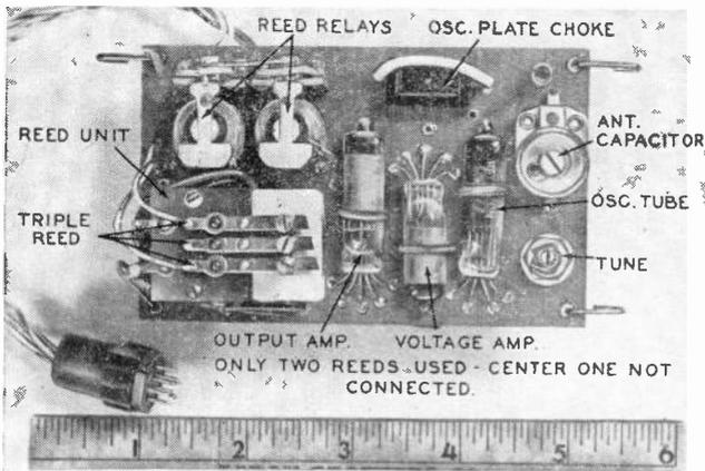
Fig. 507. Audio-tone receiver fitted with triple reed unit. Only two reeds are used in this particular set.
