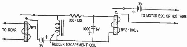
Fig. 310. This arrangement will permit you to work auxiliary circuits.
