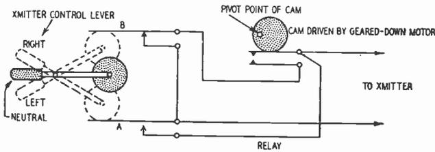
Fig. 202. *Semiproportional mechanical pulser. The transmitter control lever is shown at the left.*
