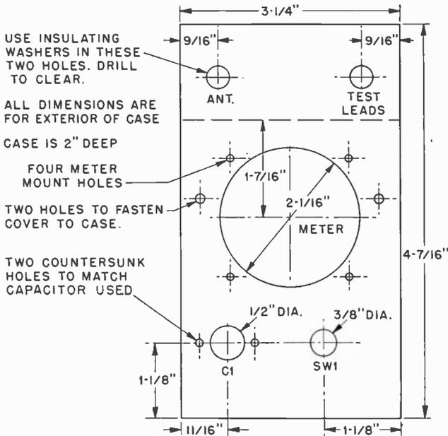
Fig. 1105. Dimensions of the front panel of the combination test meter.
