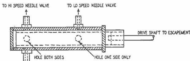
Fig. 315. Rotary-type fuel valve is made of brass tubing. Solder fuel tube fittings on before drilling holes through brass valve body. The valve is shown in the cutoff position—engine escapement energized.
