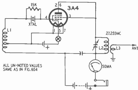
Fig. 606. This transmitter circuit gives still more power, but is trickier than that shown in Fig. 605. L1, 22 turns #22 enamelled wire close wound on 3/8" diameter rod, tap at third turn. L2, 8 turns #14 enamelled wire, wound on form 3/4" i.d., 3/4" long. L3 same as in Fig. 604.
