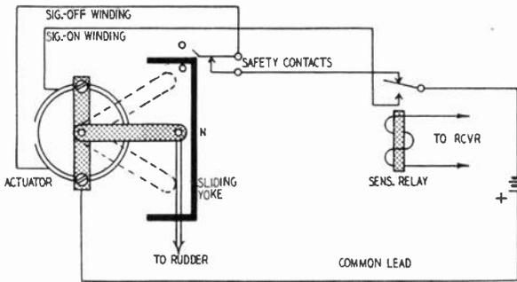
Fig. 214 Safety system that can be used with a magnetic actuator.
