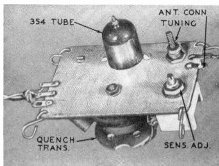
Fig. 407. Photograph of the hard-tube receiver.
