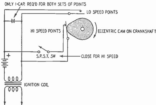
Fig. 301. Many users of spark ignition stick to this so-called old-fashioned form of ignition because it offers such a simple way to change engine speed.
