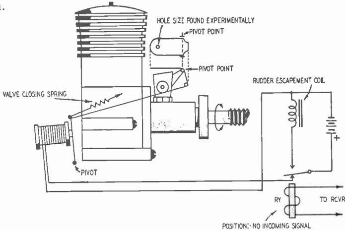
Fig. 305. A flap valve on the air intake cuts engine speed. A small hole in the flap valve permits the engine to run at slow speed.
