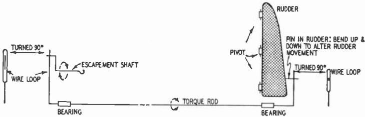
Fig. 902. The torque-rod method for getting rudder motion.
