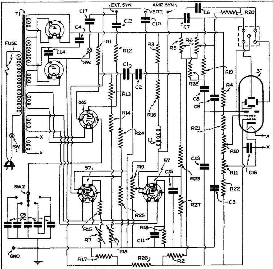
Fig. 50. Schematic of Model 154 Dumont 3" Oscilloscope.
