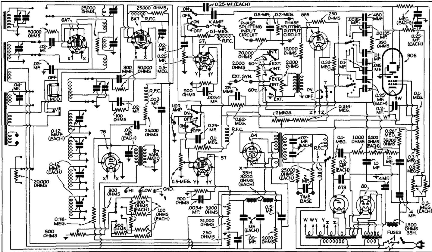
Fig. 12. Diagram of Model 555 Supreme Diagnoscope.
