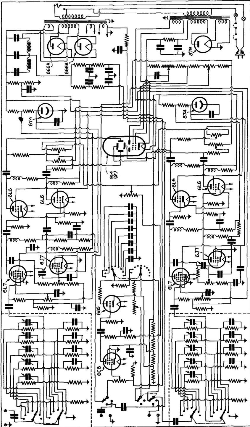
Fig. 32. Schematic of RCA 9" Oscilloscope TMV 168A.
