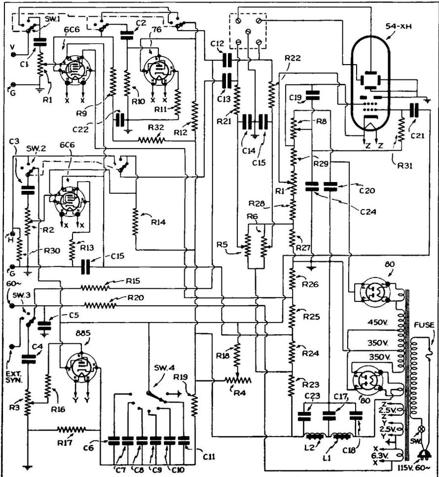
Fig. 51A. Schematic of Model 168 Dumont 5" Oscillograph
