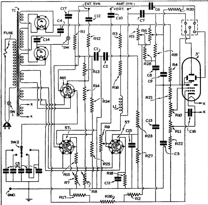
Fig. 50. Schematic of Model 154 Dumont 3" Oscillograph.
