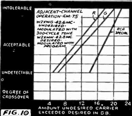
"F.M. 40" system having a total band width of 100 kc. occurs at about 43 db. Since this provides a very good signal/noise ratio and the required band width is only 100 kc., F.M. 40 is believed by many to have more overall merit than F.M. 75 when the comparative gains and limited space in the allocation spectrum are considered.
