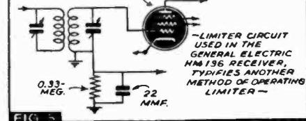
FIG 5 ~ LIMITER CIRCUIT USED IN THE GENERAL ELECTRIC HM 136 RECEIVER, TYPICAL OF ANOTHER METHOD OF OPERATING LIMITER ~
