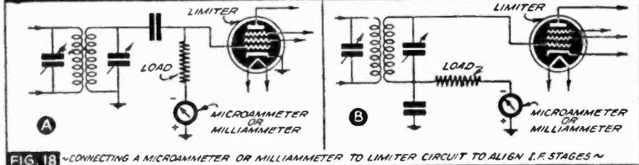
FIG. 18 ~CONNECTING A MICROAMMETER OR MILLIAMMETER TO LIMITER CIRCUIT TO ALIGN I.F. STAGES~
