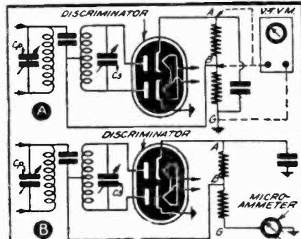
FIG. 20 ~METHOD OF CONNECTING INDICATOR FOR DISCRIMINATOR ALIGNMENT~
