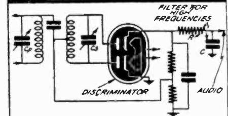
FIG. 21 ~POSITION OF HIGH-FREQUENCY ATTENUATING FILTER IN DISCRIMINATOR-AUDIO CIRCUIT. REDUCTION IN R OR C VALUES WILL INCREASE HIGH-FREQUENCY RESPONSE~
