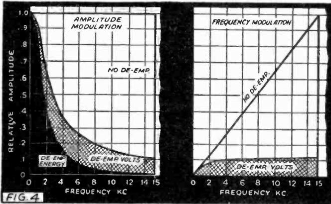
◀ Fig. 4. High-frequency pre-emphasis is used in the transmitter and de-emphasis is used in the receiver to improve the signal/noise ratio. The importance of this characteristic in ultra-H.F. broadcasting and its greater effectiveness in F.M. are illustrated at left. Comparison is on the same scale of relative amplitude.
