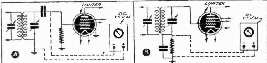
FIG. 17 ~CONNECTING A VTVM TO EITHER TYPE LIMITER CIRCUIT TO ALIGN I.F. STAGES~
