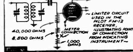
FIG 6 ~ LIMITER CIRCUIT USED IN THE PILOT FM-12 RECEIVER, ILLUSTRATING POINT OF CONNECTION FROM INDICATING INSTRUMENT ~
