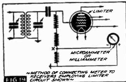
**FIG. 19** ~METHOD OF CONNECTING METER TO RECEIVERS EMPLOYING LIMITER CIRCUIT SHOWN~
