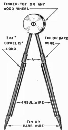
Device for shunting condensers across units under test.
