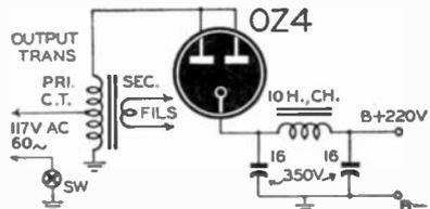
Center-tapped output transformer for power supply.
