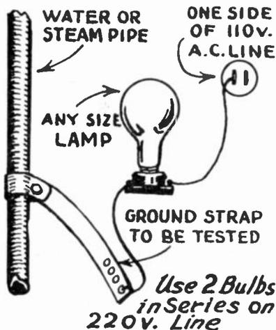
Simple ground test, using light bulb.
