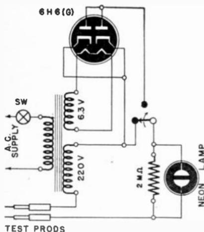
Condensers, including electrolytics, may be tested on a.c. or d.c. with this rig.
