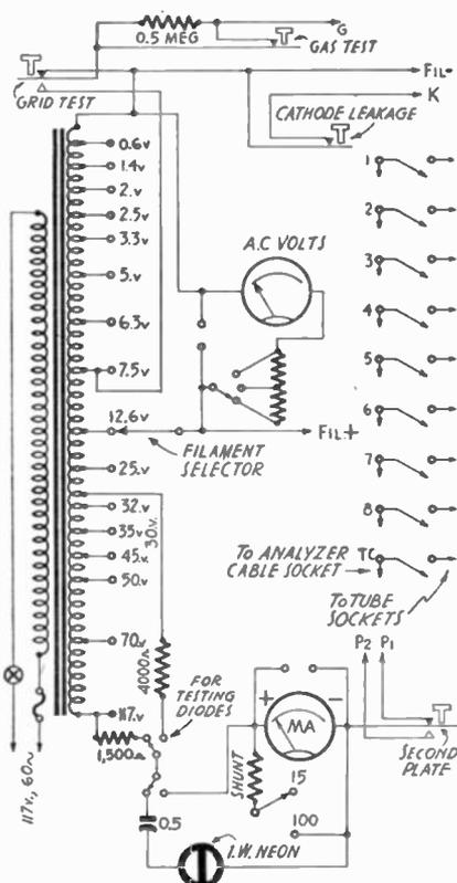
Handy tube tester with special transformer built from a power transformer. Tests all tubes. Uses neon "short" indicator.
