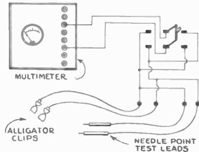
Quick reverser-switch for condenser tests.
