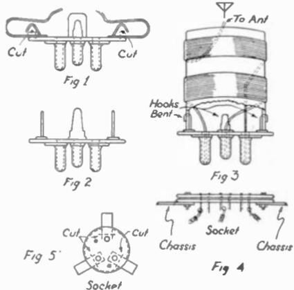
Plug-in coil from battery plug and socket.
