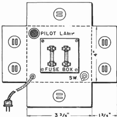
Pilot lamp and fuse for "test" outlets.
