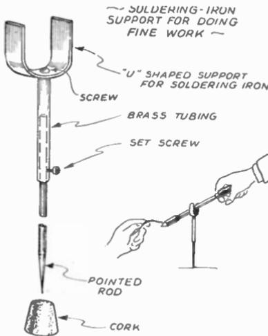
Soldering iron support for fine work.
