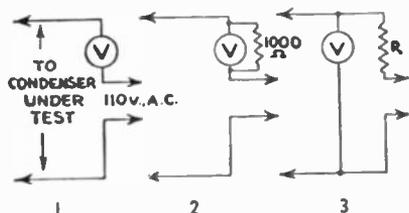
Determining condenser capacity with a.c. voltmeter.
