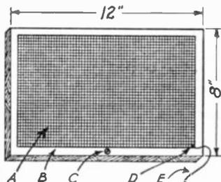
Portable antenna — A, copper screening. B, plywood strips. C, mounting screws. D, solder. E, lead to Ant. post.
