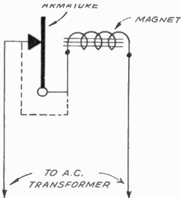
Doorbell noise eliminated by converting to a.c.
