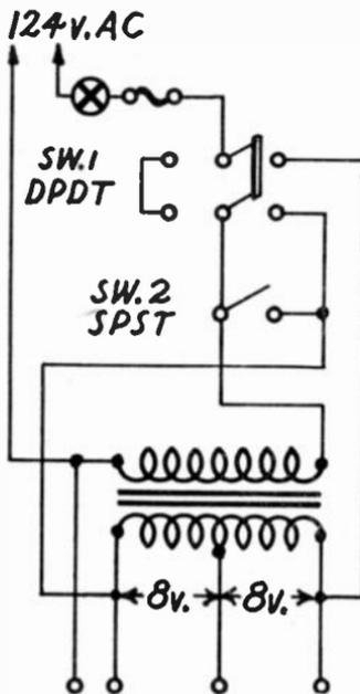
Auto-transformer hook-up to control line voltage.
