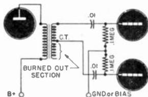
Transformer burn-out bridged by shifting connections.
