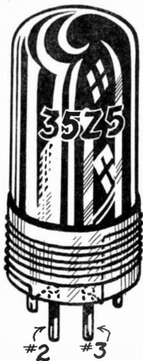
Repairing 35Z5 with open filament tap by winding resistance wire on base.
