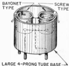
Pilot lamp tester from 4-prong tube base.
