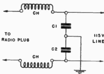
Simple line filter to eliminate noise.
