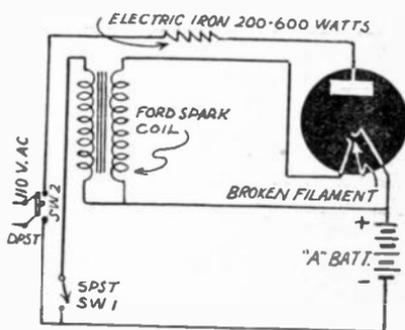
Charger from ignition coil and Tungar tube.
