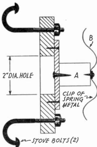
Simple jig for winding coils.
