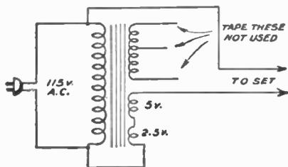
Using filament windings as line voltage booster.
