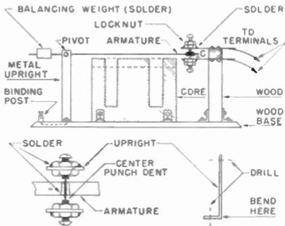
Audio transformer converted into sensitive relay.
