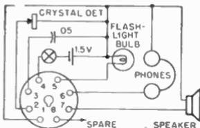
Tube socket and test lead, with phone tip, provide flexible test set.
