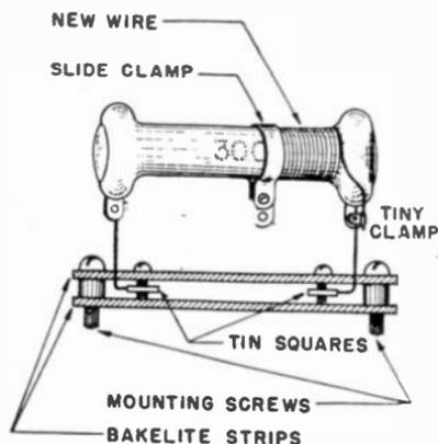
Odd-sized resistors from old insulated units.
