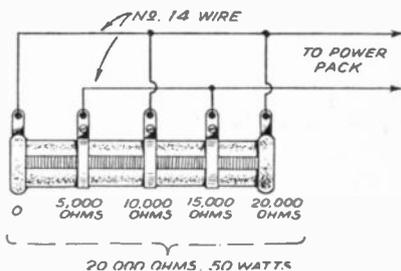
Increasing wattage capacity of resistor.
