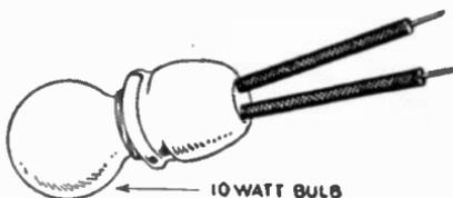
Lamp substituted for tube locates "opens".
