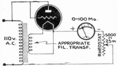
Filament emission tester of simple design.
