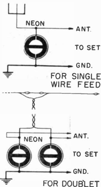
Neon lamps connected as lightning arrestors.
