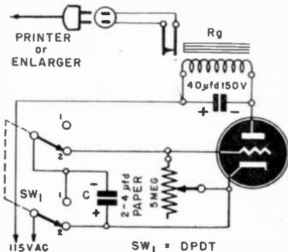
Adjustable time-interval circuit controller.
