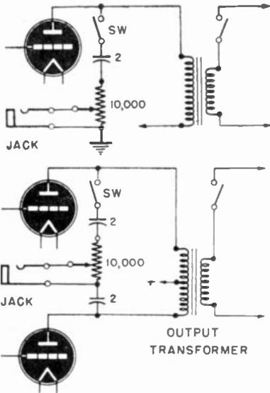
Top—adding phone jack to single tube output; Bottom—push-pull hook-up.
