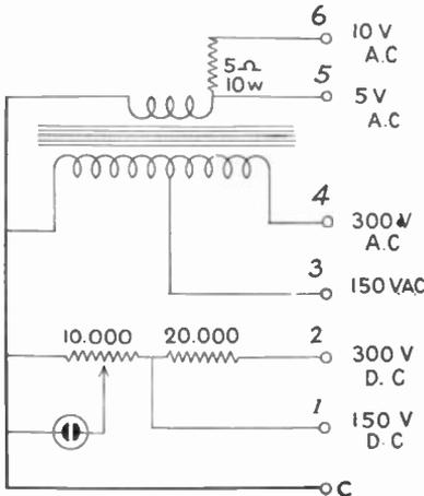
A.c. and d.c. voltage tests are quickly made with this neon tube and transformer set-up.
