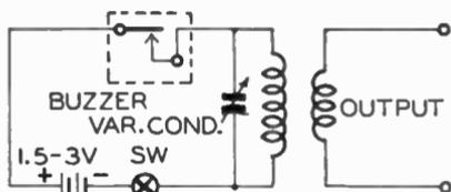
H.f. buzzer, plus b.c. coil=test oscillator.
