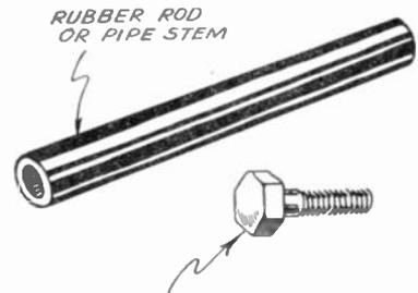
CLAMP IN VISE AND HEAT BEFORE FORCING INTO HOLE WHICH IS SLIGHTLY SMALLER THAN HEAD
