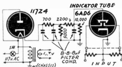
Comparison tester for resistors and condensers.
