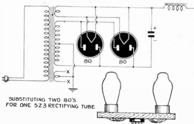
Using two 80's as a substitute for a 5Z3 rectifier.
