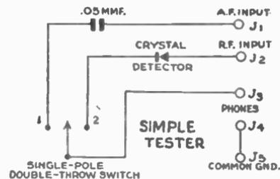
Flexible set tester for use with voltmeter.
