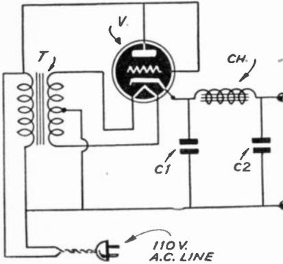
Simple power supply for test bench.
