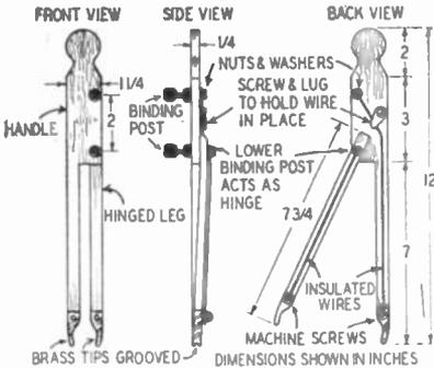
Compass legs make contact with hard-to-reach parts of circuit; test instrument connects to terminal posts.
