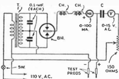
Capacity and leakage tester for condenser.
