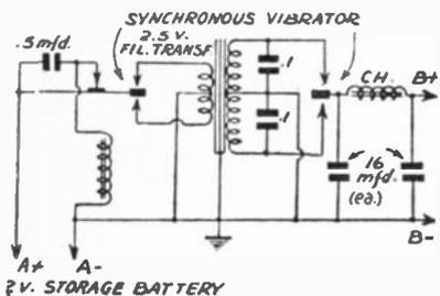
Power pack from vibrator and filament transformer.
