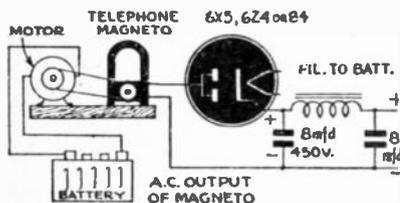
Rectifier and filter for magneto power supply.
