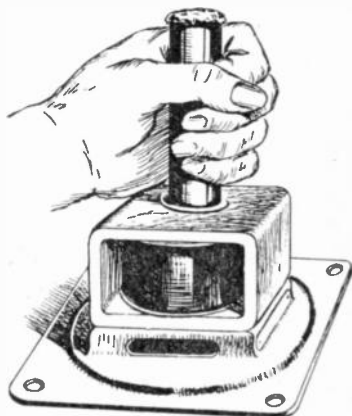
Fig. 26—How to remove some speaker fields.
