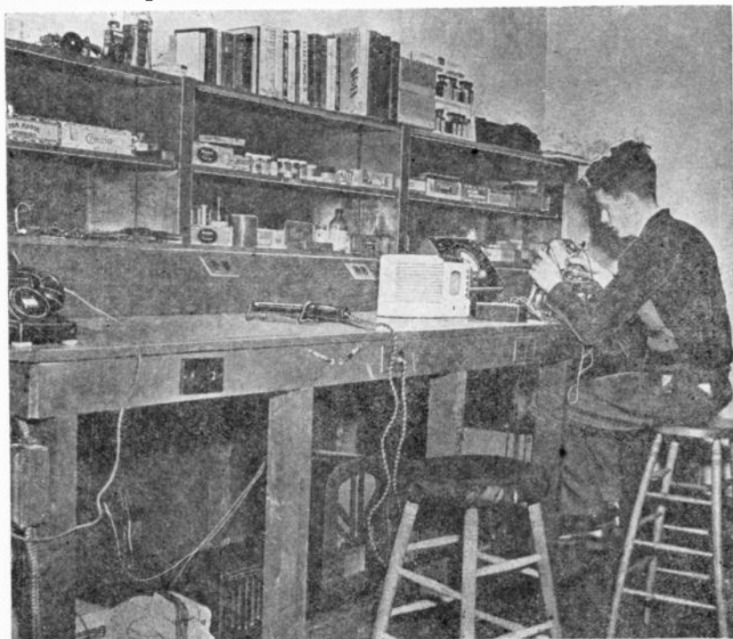
Fig. 4—Another systematic service bench arrangement which will save time and speed up work. A telephone on the bench saves time in answering customers' calls.
