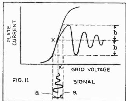
If a three-element tube is operated on the straight section of its characteristic curve, it will faithfully reproduce any alternating current impressed on its grid. The amplitude of the plate current variations represents amplification of the signal.
