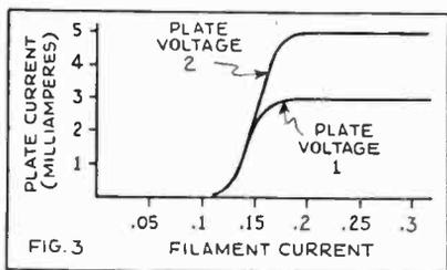
FIG. 3. The plate current stops increasing with increasing filament current at a point determined by the space-charge effect. The latter can be overcome only by raising the plate voltage. In this curve also the flat upper section represents the condition of saturation.
