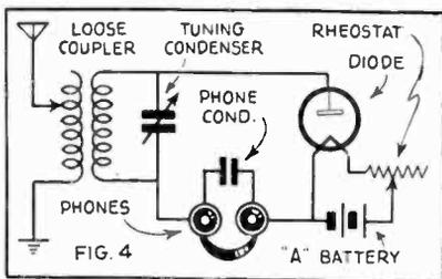
FIG. 4. The two-element tube, when used in the circuit above, makes an effective detector or rectifier of radio-frequency currents. This elementary circuit was used at one time for the reception of "spark" signals from old-fashioned transmitters.
