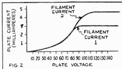
FIG. 2 This curve illustrates the increase in plate current obtained by raising the temperature of the filament. Saturation is reached at the point where the curve flattens out at the top. The values indicated are purely relative and do not apply to any particular tube.
