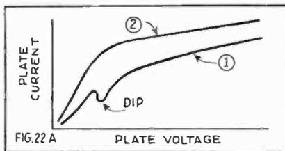
The dip in the plate-voltage, plate current curve of screen-grid tubes is due to the secondary emission effect of the plate. This dip is eliminated in the "pentode" by the third grid element.
