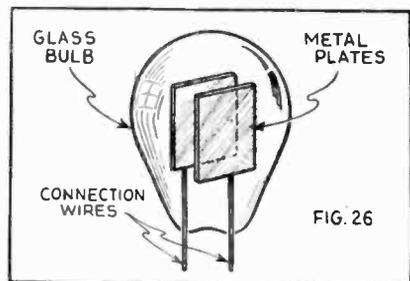
The neon tube used for television reception consists merely of two flat metal plates, separated a short distance in a bulb filled with neon gas.
