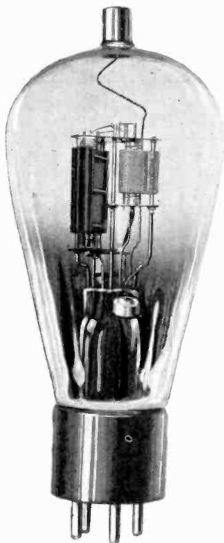
The Triple-Twin tube resembles an overgrown '45-type. Notice how the two sections are mounted on a common stem.
