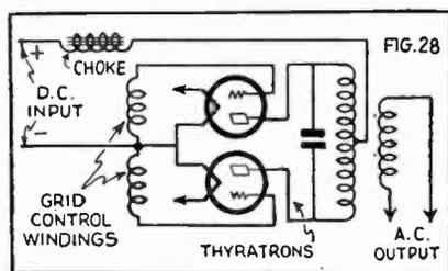
This odd circuit shows how thyratron tubes are used to convert direct current into alternating current.
