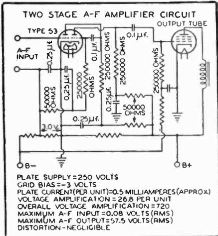
Application of the 53 tube as a class A driver. It may be also employed as a class B power stage. See chart for specifications.
