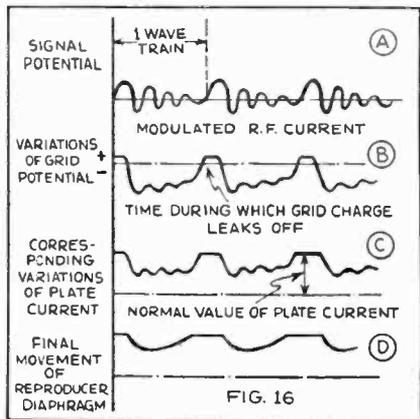
These curves show how the grid-condenser detector changes modulated radio-frequency signals into audio currents that are capable of operating earphones or other reproducers.
