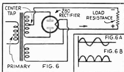
In the full-wave rectifier, both halves of the alternating current wave are used, and the output current, as shown graphically in Fig. 6B, is much smoother than the output of a half-wave rectifier.
