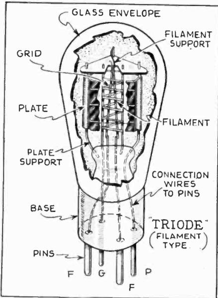
The triode or three-element tube is radio's "jack of all trades": amplifier, detector and oscillator. In this class are the 112A, 120, 171A, 201A, 226, 230, 245, etc.
