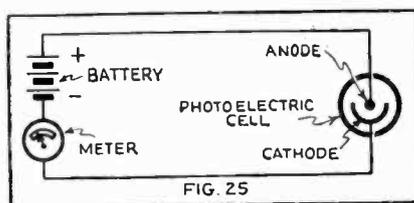
The circuit of the photo-electric cell is very similar to that of the two-element rectifier. The anode is made positive to accelerate and attract the electrons from the cathode.
