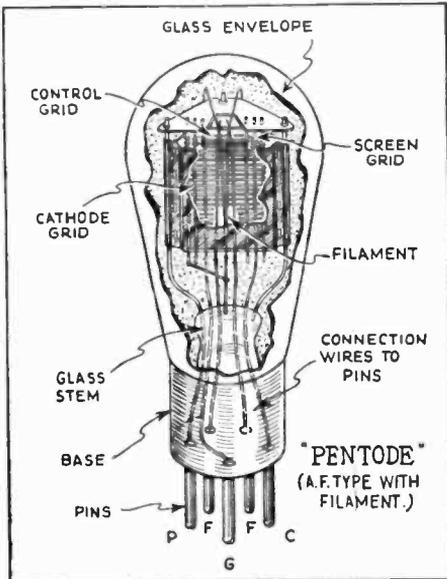
The pentode or five-element tube has three grids. The cathode or suppressor grid, located between the screen grid and the plate, is connected internally to the center of the filament.
