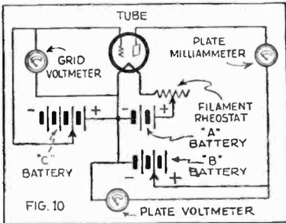
The curves of Fig. 9 may be obtained quite easily with this circuit. Only three small meters are required, in addition to the usual filament, grid and plate batteries.
