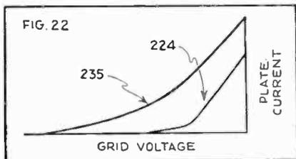
These curves show the difference in characteristics between the regular 224 screen-grid tube and the special 235 variable-mu type. Note the gradual slope and wider grid voltage range of latter.
