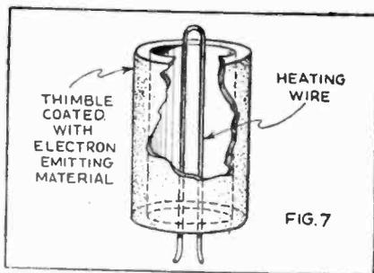
This exaggerated view shows the construction of the heated cathode used in the majority of present-day A.C. tubes. The filament in this case is merely a heater.
