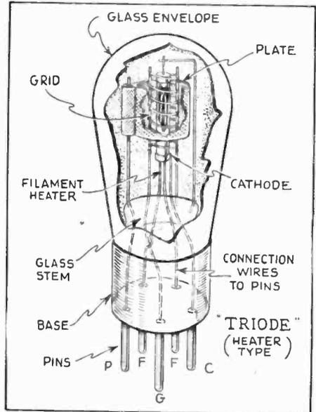
The triode with a heated cathode is the well-known 227. For purposes of heat radiation the plate in some makes is close mesh instead of sheet metal. Notice the filament inside the cathode.
