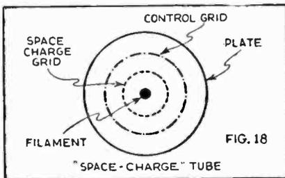
In the space-charge tetrode, the second grid is located between the filament and the regular control grid.
