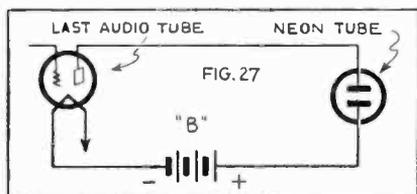
The neon tube is connected in the plate circuit of the last amplifier tube just like a loud speaker. It is illuminated by the normal plate current of the tube, to which it must be matched carefully for proper operation.
