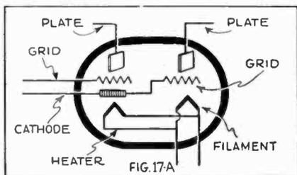
In the Triple-Twin tube, the cathode of the first section is connected internally to the grid of the second section.
