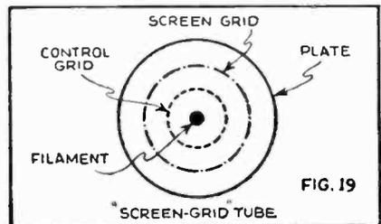
In the screen-grid tetrode, the second grid is situated between the control grid and the plate.
