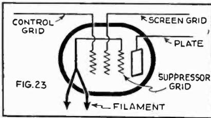
Arrangement of the electrodes in the pentode. The third grid, known as the "suppressor grid," is connected internally to the center of the filament, and has no external terminal.
