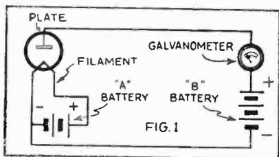
This simple circuit illustrates the Edison Effect. When the filament is lighted and the plate made positive, the galvanometer will indicate a flow of current in the series circuit.
