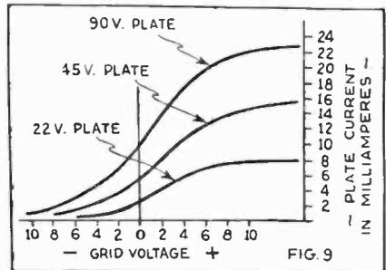
These typical curves show how the plate current of a three-element tube varies with different grid and plate voltages. Notice how sharply the plate current rises when the grid is made positive.
