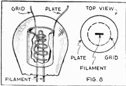
The three-element tube or "triode" has a grid encircling the filament. This element thus can control the electron stream from the filament to the plate.
