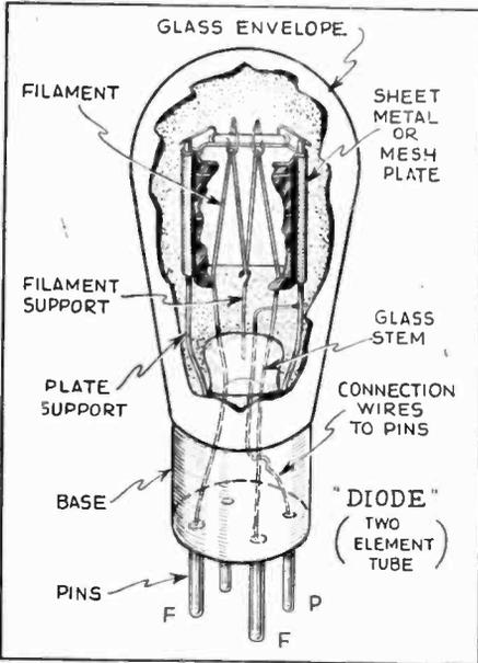
The commonest form of the diode or two-element tube is the 281 half-wave rectifier. Other diodes, built on a smaller scale, are used for detecting purposes.
