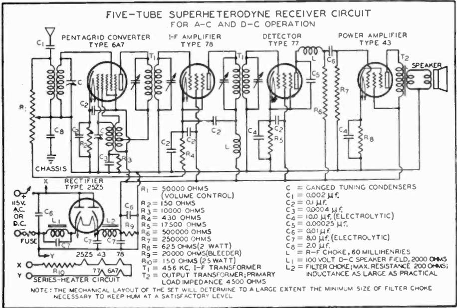
Illustrating the application of the 6.3-volt type tubes, in a typical midget receiver of the a.c.-d.c. variety. The 43 and 25Z5 are 25-volt tubes whose filament consumption is the same as that of the 6.3 volt types.
