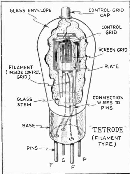
The tetrode or four-element (screen-grid) tube has two grids in addition to the filament and plate. Note that the screen-grid completely encircles the plate. The 222 and 232 are in this class.
