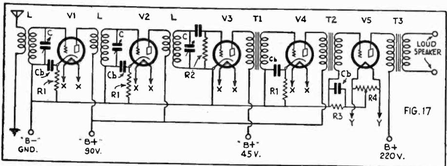
This typical tuned radio-frequency receiver shows the uses of three-element tubes as radio-frequency amplifiers, detector, and audio frequency amplifiers. The various "B" posts are intended for connection to a "B" power pack. Filament leads "X" and "Y" run to a filament light transformer. (Note: this circuit is shown only for purposes of illustration; we do not have constructional data on it.)
