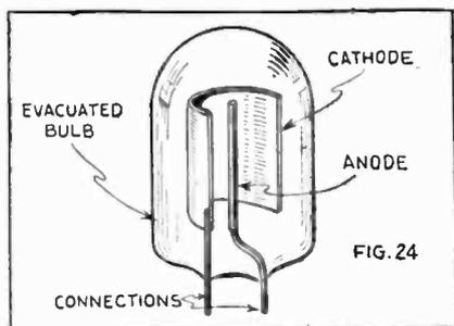
The photo-electric cell is a very simple device, consisting merely of a cathode coated with a light-sensitive material, and an anode to attract the liberated electrons. In some types, the cathode is a metallic deposit on the inside of the glass bulb.
