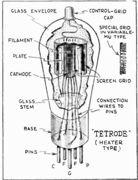
The tetrode with a heated cathode is the popular 224 screen-grid tube. An identical construction is used in the 236. In the 235 variable-mu type the control grid has uneven pitch, as shown.
