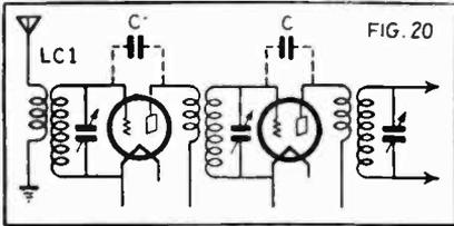
The fixed condensers C represent the grid-to-plate capacity of ordinary three-element tubes. This capacity effect becomes very serious as the frequency of the radio signals goes up (as the wavelength goes down).
