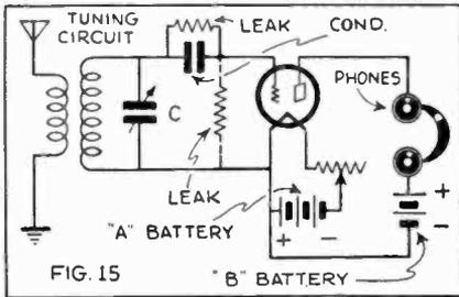
In the familiar grid-condenser system of detection, a small fixed condenser is connected in the grid lead of the tube, with a resistance of high value added in either of the two positions shown.
