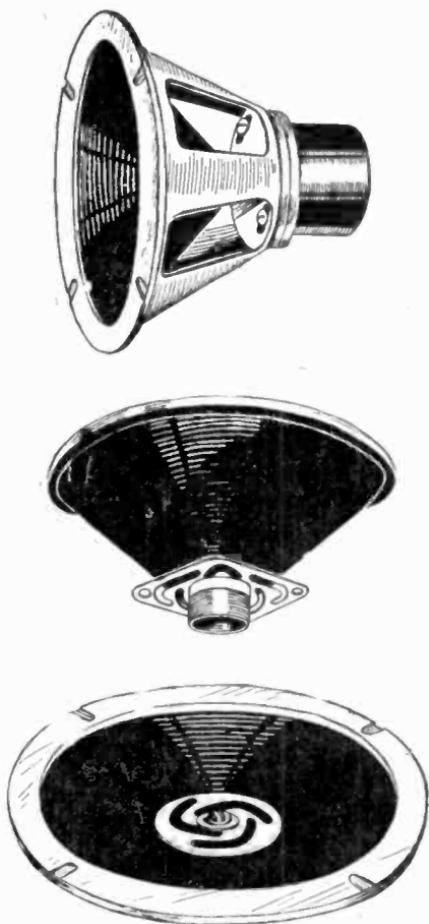
Fig. 23—The cone may be centered by: top—an adjustable frame; middle—an external spider or; bottom—a spider centered on the magnet core.
