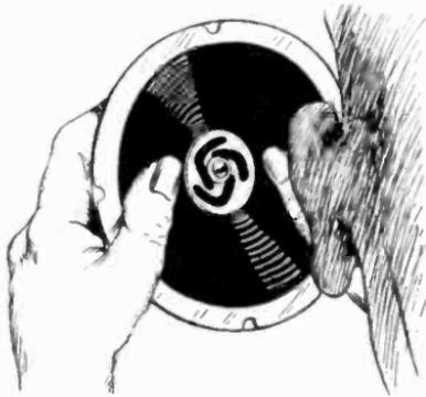
Fig. 24—How to find scraping voice coil.
