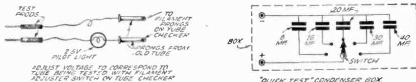
Fig. 14—left—Tube filament checker. Fig. 15—right—Simple condenser substitution box.
