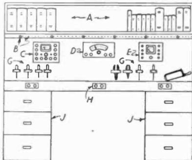
Fig. 1—Well arranged service bench. A—Books and manuals. B—Antenna jacks. C—Tube tester. D—Signal generator. E—Multitester. G—Loops for tools. H—Electric outlets. J—Drawers.
