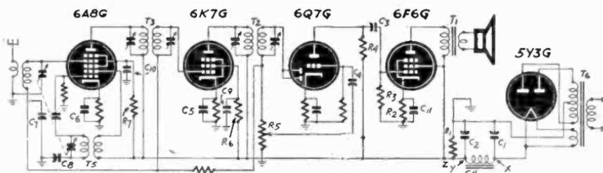
Fig. 28—Typical a.c. superhet used as illustration of trouble-shooting technique.
