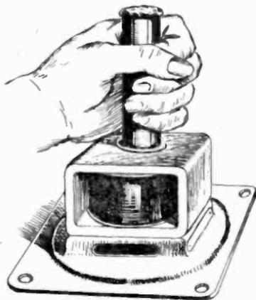
Fig. 26—How to remove some speaker fields.
