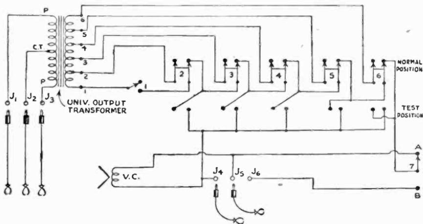
Fig. 29—A flexible loudspeaker tester which permits connecting the speaker to any type output circuit. It also enables the operator to quickly test the speaker or output of a set without removing it.
