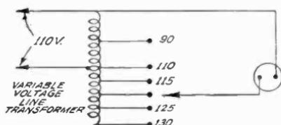
Fig. 17—A variable voltage line transformer is useful when checking for intermitents.
