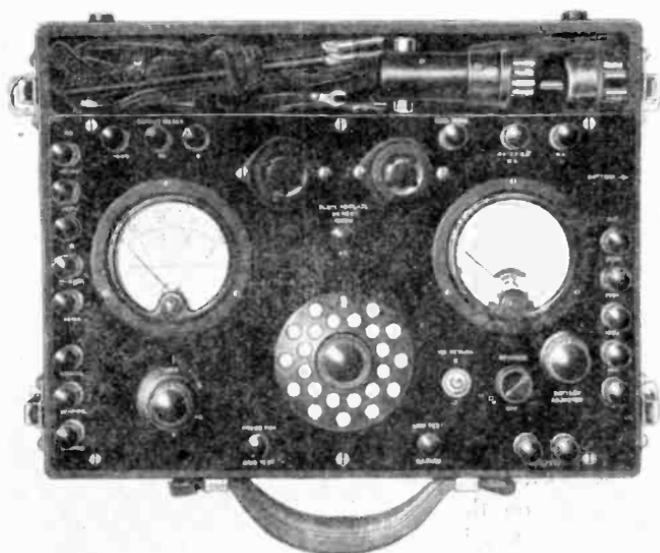
Fig. 5—A radio set analyzer of a type widely used a few years ago. (Photo courtesy Weston Electrical Instrument Co.)
