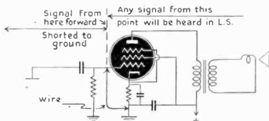
Fig. 9—Effect of squelching in any given stage. Noise in a certain stage may be quickly located.
