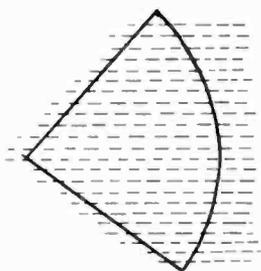
Fig. 519. A variation of plain-slicing uses quartered logs. Called quarter-slicing, this method results in grain patterns composed of narrow straight stripes.
