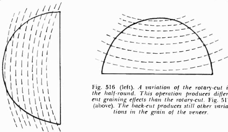
Fig. 516 (left). A variation of the rotary-cut is the half-round. This operation produces different graining effects than the rotary-cut. Fig. 517 (above). The back-cut produces still other variations in the grain of the veneer.
