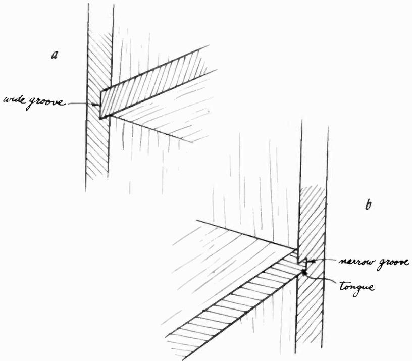
Fig. 617. Two ways of inserting a fixed partition in a cabinet: a) full dado; b) partial dado or tongue and groove.
