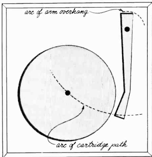
Fig. 108. Because the pivot point of the tone arm is several inches from its end, allow room so that the arc of the overhang does not hit the cabinet side before the cartridge arc can traverse the playing area of a record.
