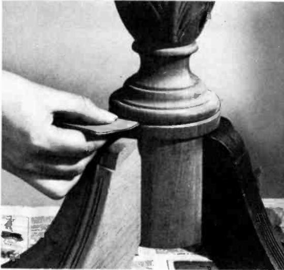
*Fig. 703. Curved and carved portions of the cabinet must be finished by hand. Do not use a sanding block.*
