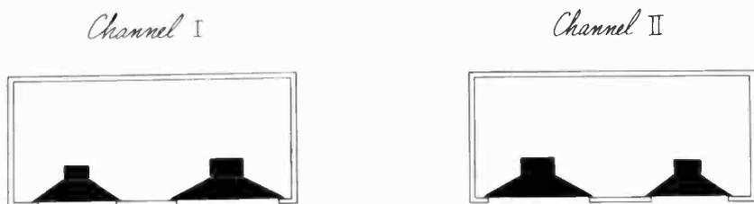
Fig. 120. *Identical speaker systems in identical enclosures.*
