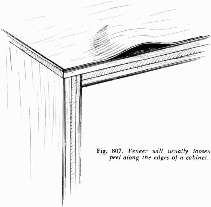
Fig. 807. Veneer will usually loosen or peel along the edges of a cabinet.
