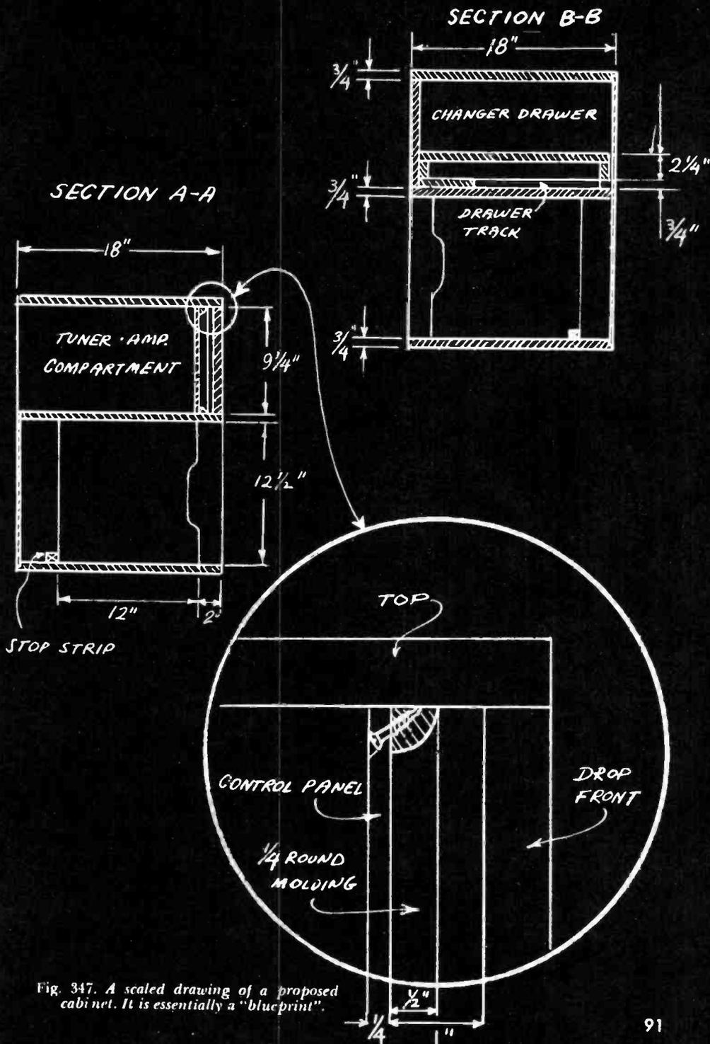
Fig. 347. A scaled drawing of a proposed cabinet. It is essentially a "blueprint".
