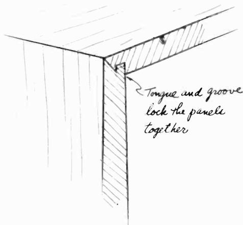
Fig. 614. The lock mitre is the strongest of the variations, but a shaper is essential if this joint is to be prepared properly.
