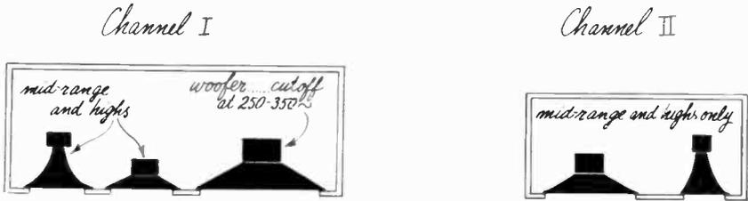
Fig. 121. Stereo setup using different speaker systems.
