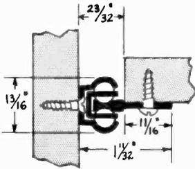
Make sure that the drawer slide will be able to carry the weight of the equipment. The drawings at the left show ball-bearing catches—a few of the many different types that could be used.
