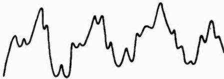
Fig. 303. *Noise is characterized by its random irregularity.*
