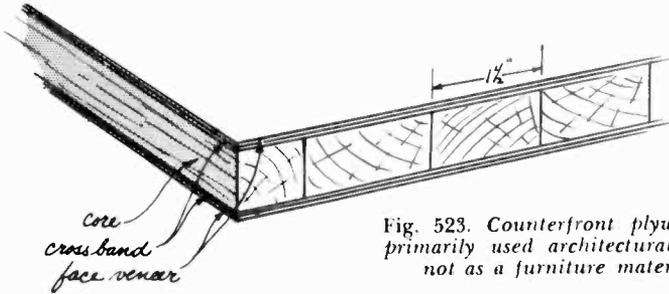
Fig. 523. Counterfront plywood is primarily used architecturally and not as a furniture material.
