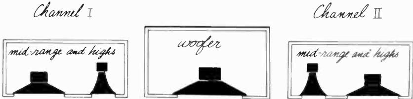
Fig. 122. Putting the woofer in the center gets rid of the apparent dead spot in the middle.
