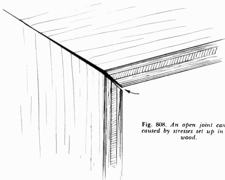
*Fig. 808. An open joint can be caused by stresses set up in the wood.*
