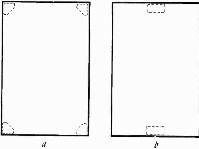
Fig. 201. There is a rule of thumb for speaker placement in rectangular rooms: (a) corner speakers work well in any corners; (b) wall enclosures function best when centered on either short wall.
