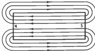
Fig. 301. Flux lines of a bar magnet.
