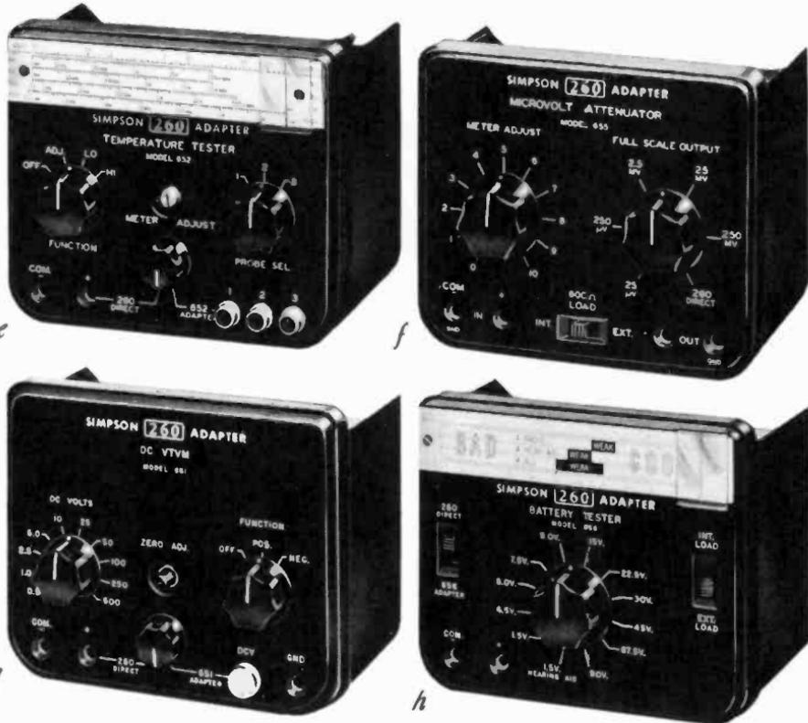
Fig. 1205. (continued). Temperature tester adapter (e) uses thermistors as sensitive elements. The microvolt attenuator (f) supplies calibrated test voltages. The vtvm adapter (g) makes the vomm into a sensitive vtvm with more than 10 megohms input resistance. The battery tester (h) adapter for the vomm makes the latter into an instrument for testing all batteries, important with the increased use of transistors. (Simpson Electric Co.)
