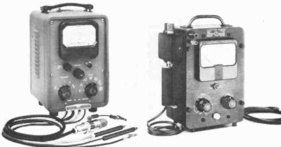
Fig. 1210. Laboratory vtvms (a) performs all the familiar functions with greater accuracy while the unit at (b) only indicates voltage. (Hewlett-Packard Co. and General Radio Co.)
