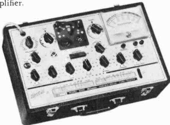
Fig. 1208. A transconductance type tube tester is essential for preventive maintenance.
