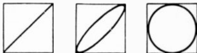
Fig. 703. Scope patterns indicate phase relationship between generator and audio-amplifier output. Straight line indicates zero or 180-degree shift.
