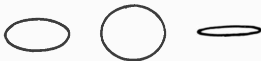
Fig. 1303. Trace seen on scope can be circle or ellipse in absence of 120-cycle hum.
