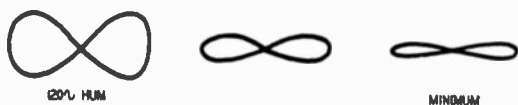
Fig. 1301. Forms of 120-cycle hum as seen on the face of a scope. This is the frequency of power-supply ripple in the output of a full-wave rectifier.
