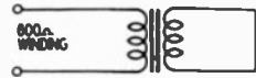
Fig. 603. An inductive dummy load can be made by using an old transformer and shorting the secondary winding.
