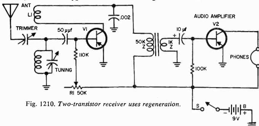
Fig. 1210. Two-transistor receiver uses regeneration.
