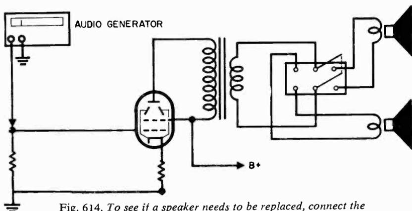
Fig. 614. To see if a speaker needs to be replaced, connect the old speaker and a new one to a double-pole double-throw switch. Operate the switch and listen carefully. If you can hear a definite improvement, replace the old speaker.
