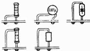
Fig. 1205. Schematics that come with imported receivers include more information than we are used to seeing. Here component polarity is indicated. In compact units component size and height are important. (Sony)
