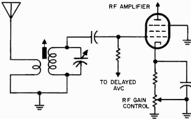
Fig. 919. Rf gain-control circuit.
