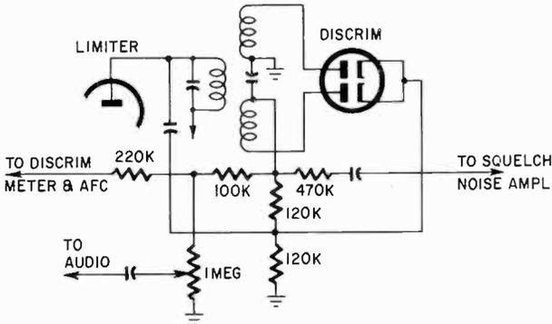
Fig. 1111. Phase detector used in a mobile receiver. There are four types of FM detectors that can be used: the discriminator, the ratio, gated-beam and phase detectors.
