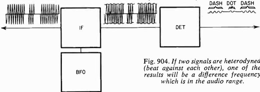
Fig. 904. If two signals are heterodyned (beat against each other), one of the results will be a difference frequency which is in the audio range.
