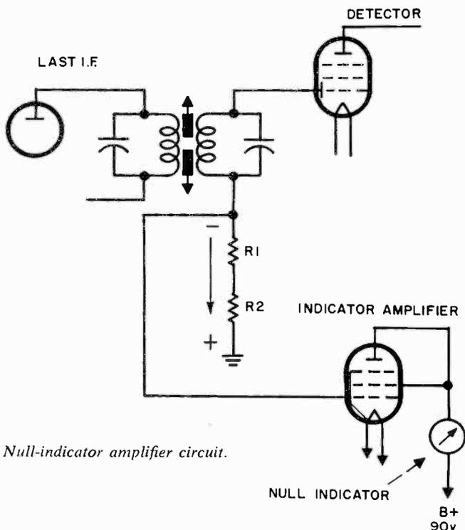
Fig. 1009. Null-indicator amplifier circuit.
