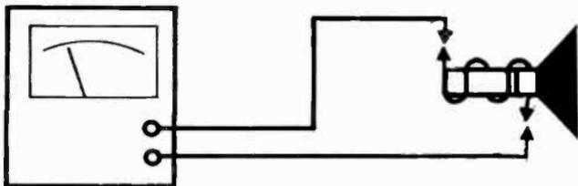
Fig. 613. How to check a voice coil for an open circuit. Disconnect one lead of voice coil from secondary of output transformer. Rub test leads of an ohmmeter against the voice-coil leads. Scratching noise out of speaker indicates speaker is working.
