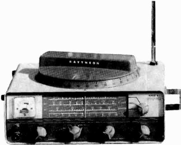
*Fig. 1007. This portable radio direction finder receives signals from long-range Consolan stations and standard broadcast bands as well as regular marine beacons. Sense antenna, right rear, differentiates between correct bearings and reciprocal bearings. Six standard flashlight batteries power the receiver. A dual purpose meter indicates battery strength and provides visual null reading for accurate bearings. (Raytheon Co.)*
