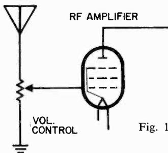
Fig. 1010. Volume control in the rf input.
