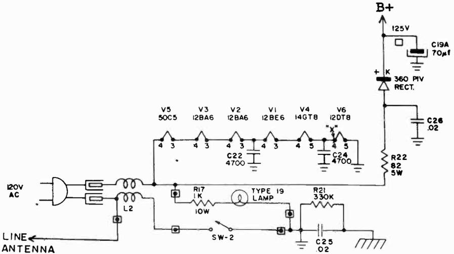
Fig. 702. Transformerless supply. The series filaments are bypassed by two capacitors. Capacitor C26 protects the rectifier from transient surges in the power line. (Arvin Industries, Inc.)
