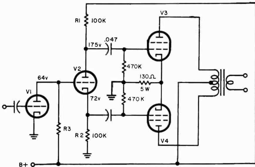
Fig. 712. The phase splitter. Note that the cathode and plate resistors have equal values. The signal voltage is developed across both resistors and is delivered to the push-pull tubes, V3 and V4, by a pair of coupling capacitors.
