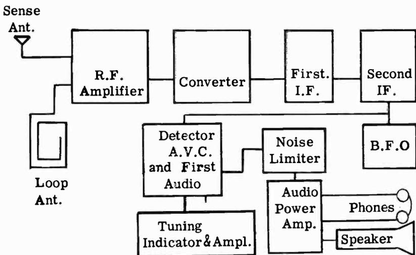
Fig. 1004. Block diagram of a marine radio receiver.
