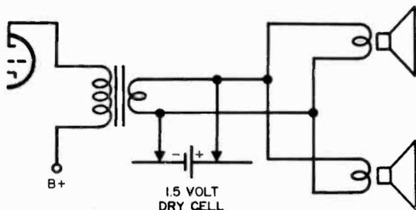
Fig. 616. Method of checking phasing of speakers. Connect the dry cell. Tap one lead from the secondary winding of the transformer against one terminal of the cell while watching the movement of both cones. The cones should move in or out at the same time. Do not make a permanent connection to the dry cell.
