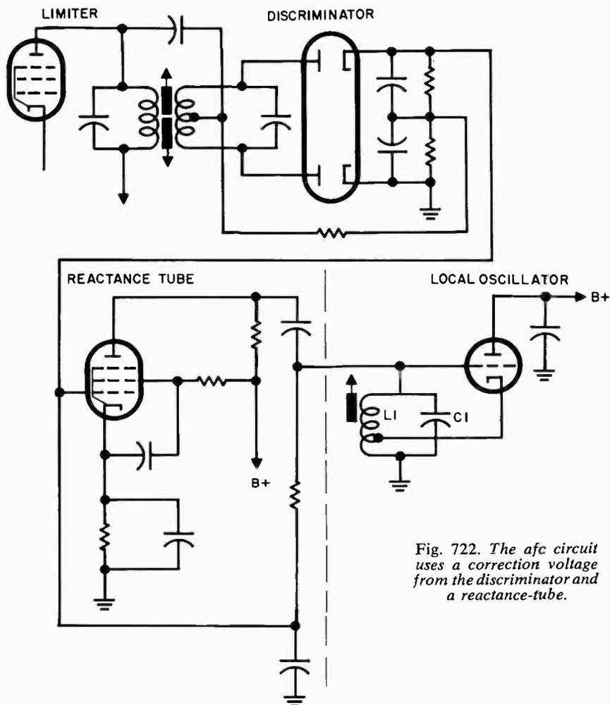
Fig. 722. The afc circuit uses a correction voltage from the discriminator and a reactance-tube.
