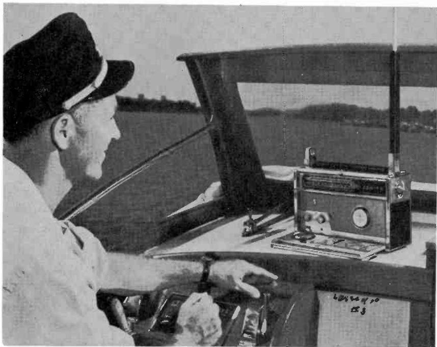
Fig. 1003. Transistor portable covers nine bands and is useful for marine navigation (Zenith Radio Corp.)
