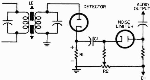
Fig. 918. This noise-limiting circuit has to be adjusted for noise conditions. It is called a manual noise limiter (mnl).
