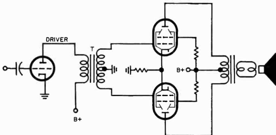
Fig. 711. Push-pull output stage. Interstage push-pull transformer *T* couples the driver of the push-pull tubes. Good interstage transformers are expensive, take up room. Most sets use a tube (or a transistor) as a phase inverter to take the place of the transformer.
