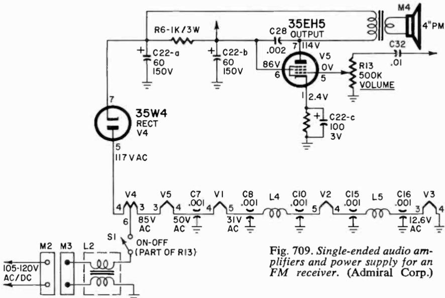
Fig. 709. Single-ended audio amplifiers and power supply for an FM receiver. (Admiral Corp.)
