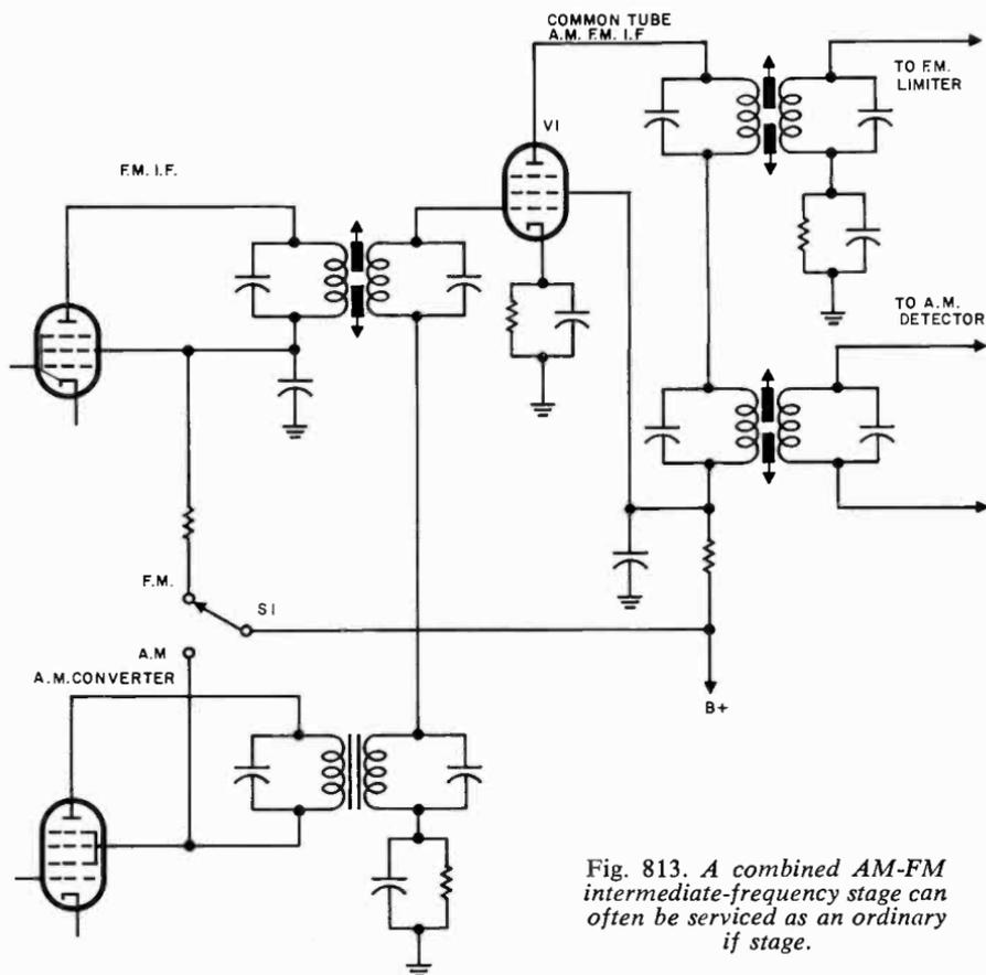
Fig. 813. A combined AM-FM intermediate-frequency stage can often be serviced as an ordinary if stage.
