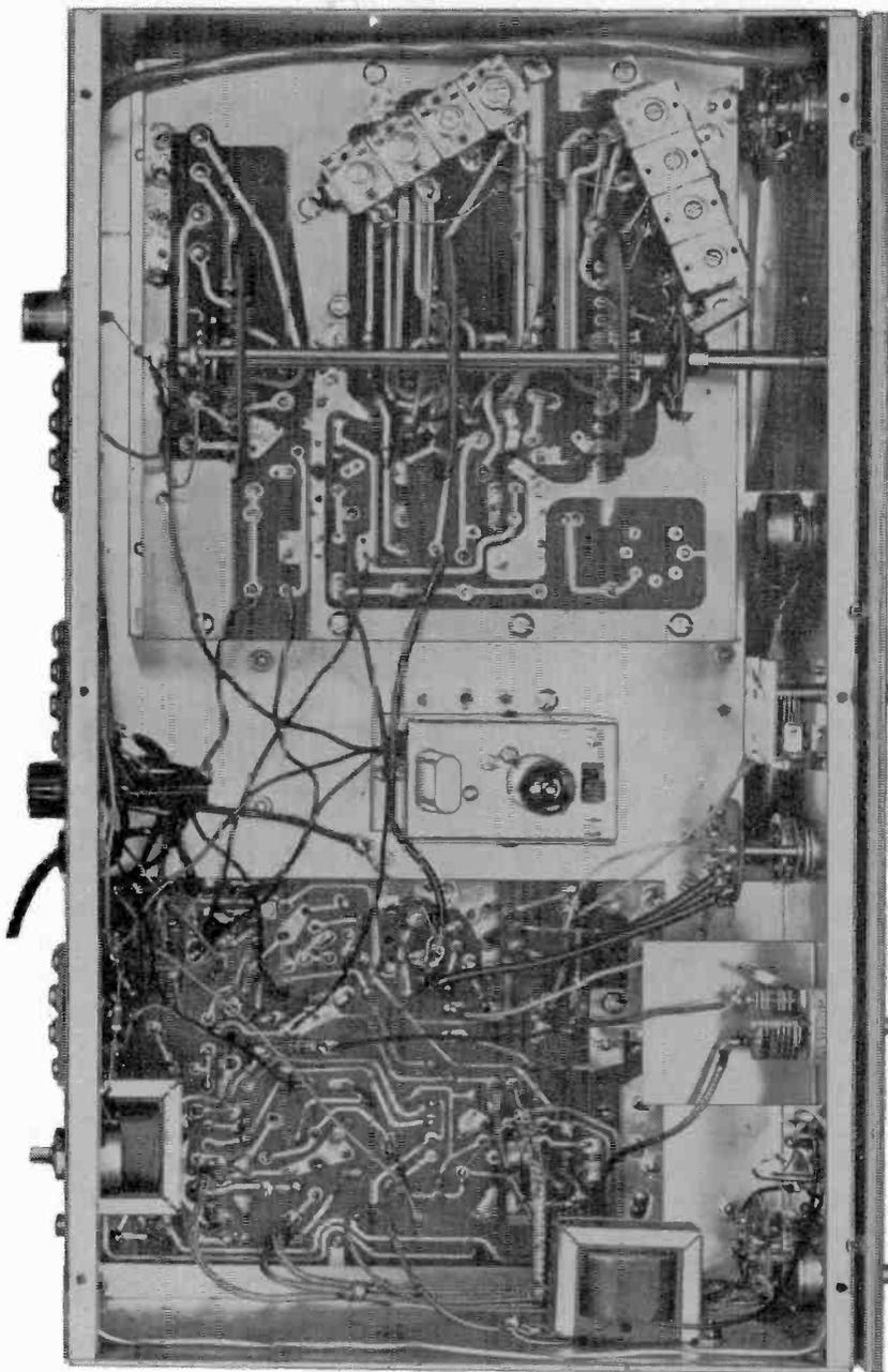
Fig. 912. Communications receivers are often constructed with one or more printed-circuit boards. (Allied Radio Corp.)
