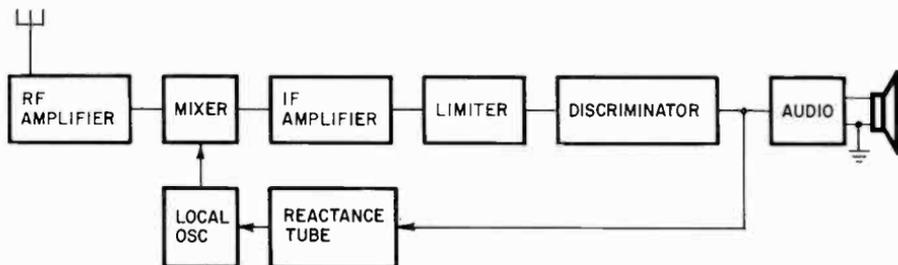
Fig. 721. Block diagram of FM receiver using afc.
