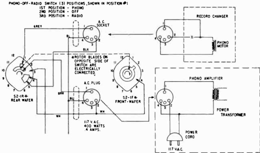
Fig. 707. Wafer switches can be a source of trouble. In this circuit the wafer switch has three positions and serves three functions. (Shown in position 1.) First position is phono; second, off; third, radio. (Zenith Radio Corp.)
