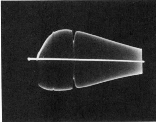
*Fig. 244. The illustration above clearly shows the positioning of the absorption marker at 300 kc on the sweep output waveform.*
