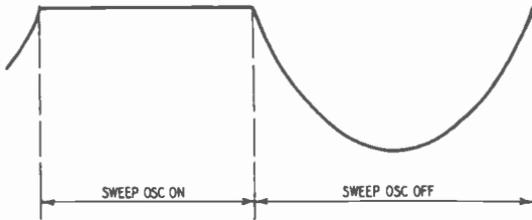
*Fig. 231. Keying waveform of voltage often applied to grid of sweep oscillator to develop a zero-volt reference line. Only the "on" portion of the voltage need be clipped since the oscillator does not respond to changes in grid bias during the time it is cut off.*
