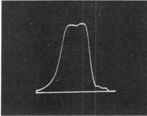
Fig. 402. Typical bandpass response of the chroma amplifier in a color TV receiver.
