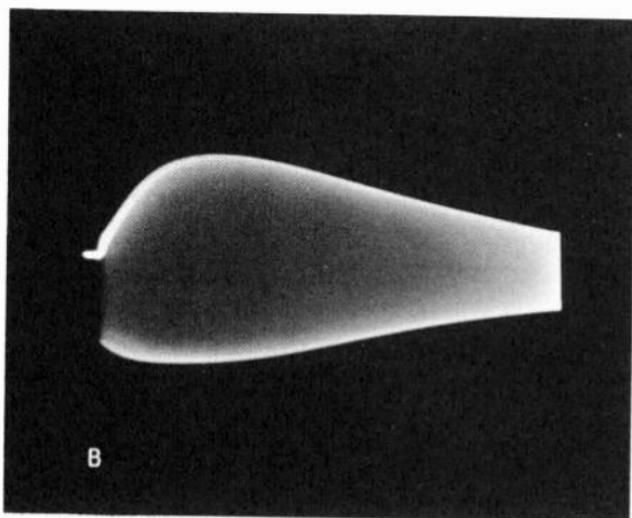
*Fig. 242-a,-b. Dissymmetry caused by waveform error from generator. Display of output (a) of video sweep-generator when zero-volt reference line is used. Display of video-sweep generator output (b) applied directly to input terminals of scope.*
