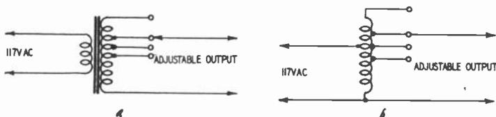
Fig. 905-a,-b. Techniques for increasing or decreasing the line voltage. The transformer type (a) provides line isolation but the autotransformer (b) does not.
