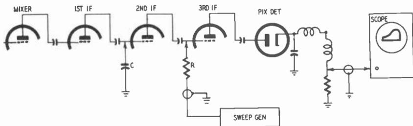
Fig. 1030. Technique for i.f. stage alignment. Capacitor *C* kills operation of all i.f. and r.f. stages preceding the isolation resistor *R* connected to cable of the generator. Values of *C* and *R* are not critical. *C* can be .001  $\mu$ f and *R* can be 1 megohm.
