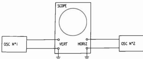
*Fig. 803. For absolute zero beat, the output from one oscillator must be applied to the vertical input of the scope, while the output from the other oscillator is connected to the horizontal input. This arrangement works quite well when audio frequencies are used, but is impractical for i.f. and r.f. testing since vertical and horizontal amplifiers of most scopes do not extend into the i.f. and r.f. range.*
