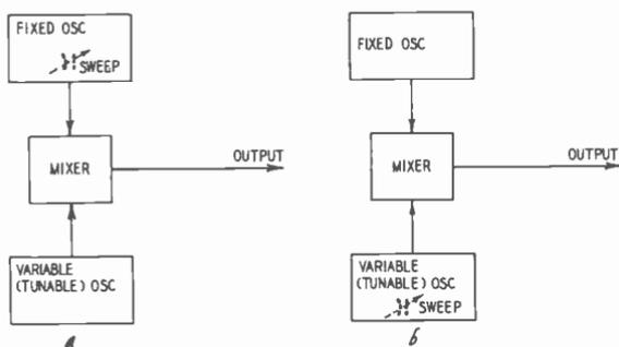
Fig. 215-a,b. Beat-frequency sweep generators may be arranged to sweep the fixed-frequency oscillator (a) or may be designed to sweep the tunable (variable frequency) oscillator (b).
