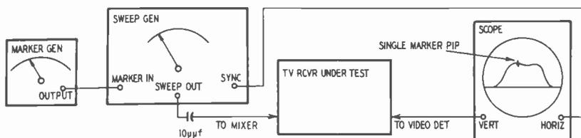
Fig. 1032. Setup for sweep alignment. To get the overall response, connect generator to control grid of mixer or converter. A small mica capacitor (not shown) of about  $10\ \mu\text{f}$  can be connected in series between the sweep cable and the grid. The capacitor acts as a decoupling unit. Do not turn the marker generator on until you get the desired response curve.
