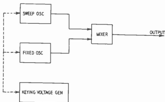
Fig. 236. Here the keying voltage is applied to both the fixed-frequency and sweep oscillators. This ensures zero output from the sweep generator during the zero-volt interval.
