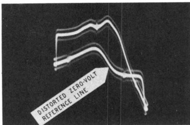
*Fig. 407. Result of testing the output from a sweep generator with a demodulator probe and scope when there is leakage from the sweep oscillator into the fixed oscillator circuit. A zero-volt reference line exhibits curvature under these conditions when the output from the fixed oscillator is not flat.*
