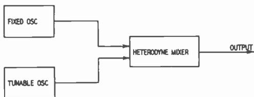
*Fig. 804. Some marker generators use a beat-frequency arrangement to get wide frequency coverage with minimum complications. Circuit-wise this cannot be successfully calibrated against a crystal oscillator because of the excessive number of confusing cross beats which result.*
