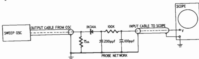
Fig. 208. Circuit of demodulator probe used to connect sweep generator to scope input.
