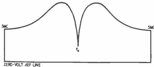
*Fig. 516. When the output from a sweep generator contains strong harmonics and this output is utilized to produce a heterodyned output from a Chromatic probe, the low-frequency region of the sweep signal from the probe develops abnormally high voltage.*
