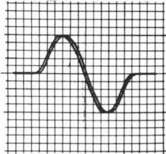
Fig. 1036. Discriminator S curve in TV set is same as in FM receiver, except bandwidth is somewhat less.
