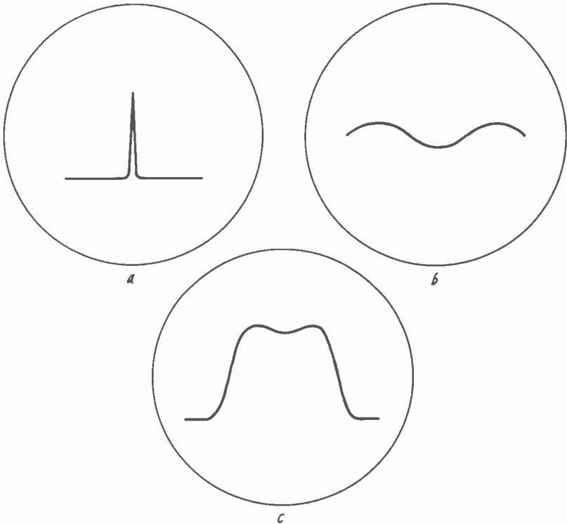
*Fig. 1008-a,-b,-c. FM i.f. response curve appears as narrow pip (a) because sweep width of generator is excessive. Only top of FM curve is seen (b) because sweep width is inadequate. Satisfactory display is seen (c) when generator sweep width is suited to bandwidth of circuits being tested.*
