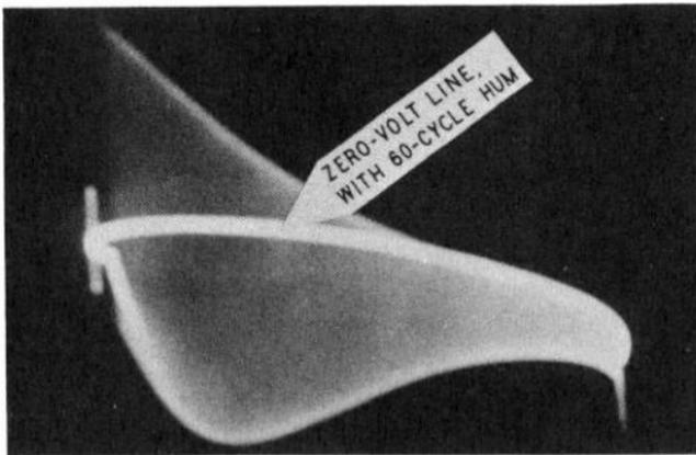
*Fig. 409. Leakage between sweep and fixed oscillators in the beat-frequency generator causes substantial even-harmonic distortion at low frequencies. The curvature of the zero-volt reference line and sweep output is due to the presence of 60-cycle hum voltage in the generator output system.*
