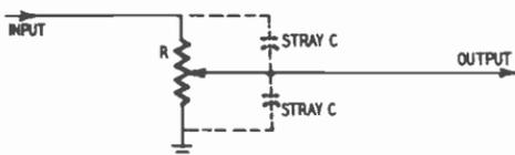
Fig. 303. Stray capacitance,  $C$ , shunts the output potentiometer.
