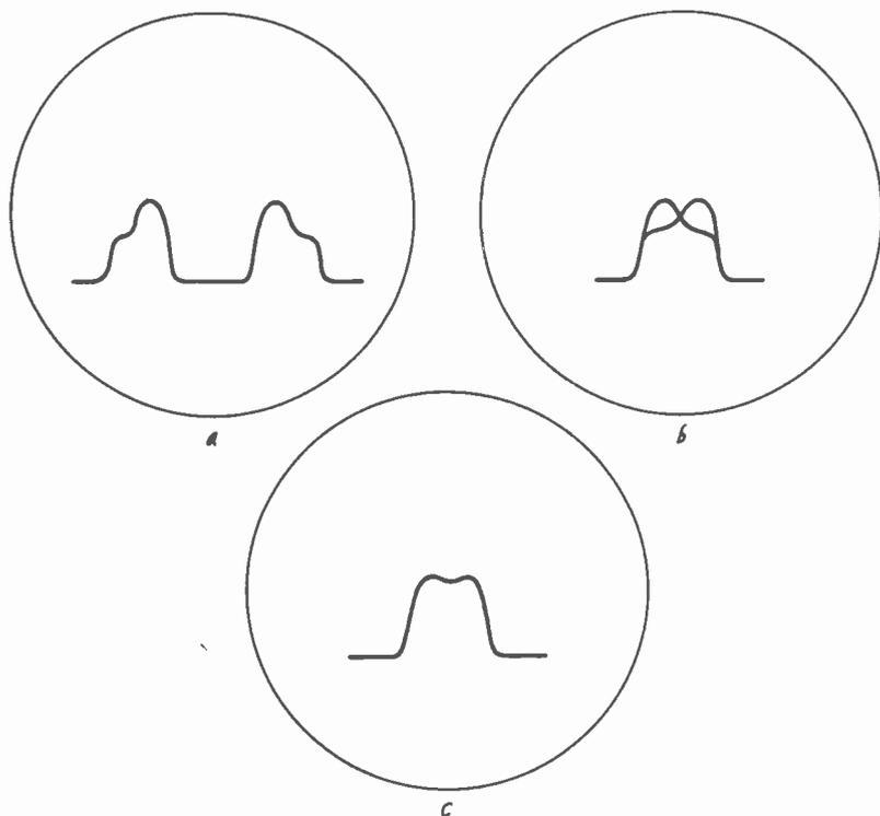
*Fig. 1005-a, b, c. Using 60-cycle sawtooth sweep, the illustration (a) shows the i.f. response curve when the i.f. transformers are misaligned. Increasing the sweep to 120 cycles produces the curve shown at the top right (b). Proper adjustment of the i.f. stages using 120-cycle sweep results in the curve shown in the bottom illustration (c).*
