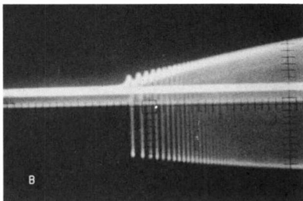
Fig. 240-b. Photograph shows oscillators locked below 100 kc.
