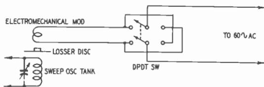
Fig. 511. Electromechanical modulation of oscillator circuit.
