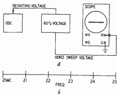
Fig. 202-a,-b. When a 60-cycle sine-wave voltage (a) is used to drive the vibrator in the sweep-oscillator circuit and the same sine-wave voltage deflects the scope beam horizontally, a linear frequency sweep is obtained. (if properly designed) equal horizontal intervals correspond to equal frequency increments. (b)
