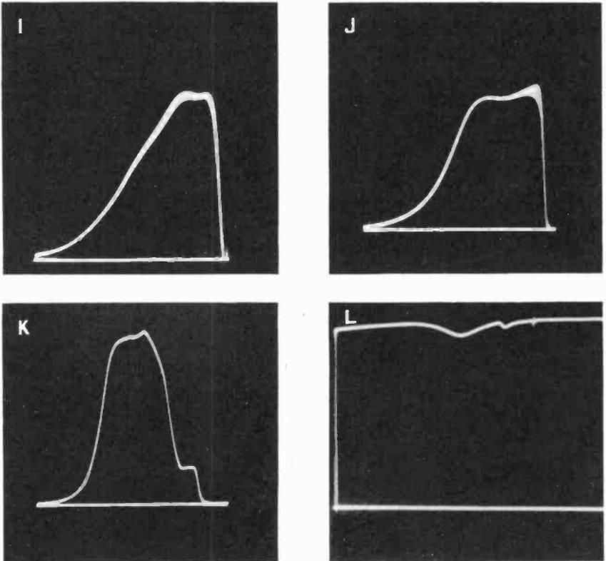
*Fig. 109-i,j,k,l. In (i) we have a Q demodulator response curve; sweep width of 3 mc is adequate; (j) frequency response of 1 video amplifier, sweep width, 6 mc; (k) frequency response of a chroma amplifier; sweep width of 5 or 6 mc is sufficient and (l) impedance check of an antenna and lead-in; maximum sweep width should be used. 12 to 15 mc is satisfactory.*
