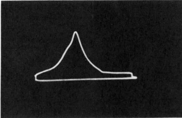
Fig. 228. Bandwidth of circuit is too great to permit full display.
