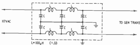
Fig. 412. Leakage of sweep voltage into the line cord is prevented by use of a lowpass line filter. It is often advantageous to shield the filter.
