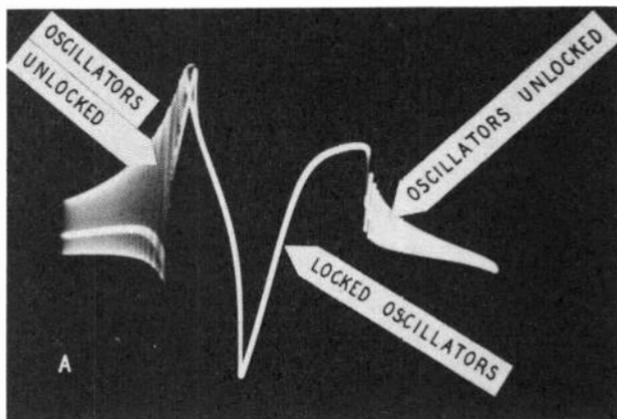
Fig. 240-a. The low-frequency notch may define the low-frequency limitation of the beat-frequency sweep generator or the low-frequency limitation of the demodulator probe utilized in the test, whichever is the greater. To check the generator output with certainty, apply the output of the generator directly to the vertical-input terminals of the scope. The illustration above shows the oscillators locked below 1 mc.
