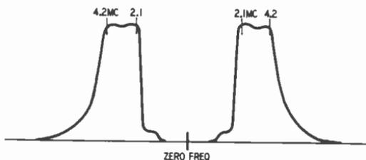
*Fig. 403. In this illustration, the sweep generator is tuned to a center frequency of approximately zero. To locate the zero-frequency point accurately, hold the generator output and scope input cables together. Residual leakage is often sufficient to place a marker on the base line at the zero-frequency point.*
