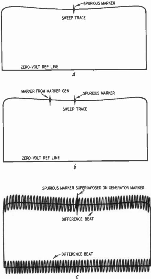
Fig. 501-a,b,c. Effect of interaction between spurious marker and signal output of the marker generator.
