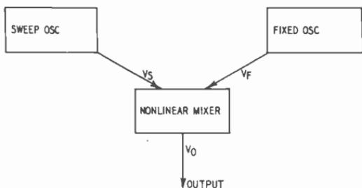
*Fig. 220. When the output voltage  $V_s$  from the sweep oscillator is much larger than the output voltage  $V_f$  from the fixed oscillator, the beat frequency output  $V_o$  is flattest (has least amplitude variation). But if  $V_f$  is larger than  $V_s$ , changes in  $V_s$  will appear in output. By making  $V_s$  very large and  $V_f$  very small the variation in output voltage can actually be made much less than that present in  $V_s$ .*
