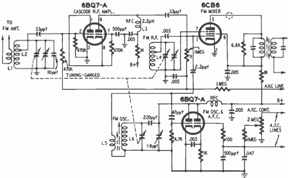
Fig. 1019. Front end of a representative FM receiver. The use of a separate local oscillator improves frequency stability.
