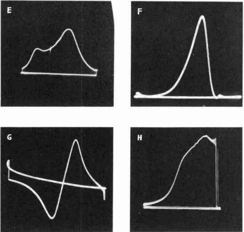
Fig. 109-e,f,g,h. In (e) above, we have the front-end response for channel 6. (f) an i.f. response curve; a sweep width of 8 mc is adequate; (g) ratio-detector response curve; sweep width of 1 or 2 mc; (h) green video-amplifier response curve in color TV receiver; sweep width is 6 mc.
