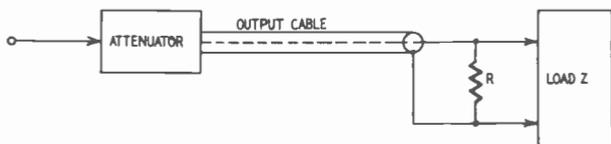
Fig. 311. Low values of  $Z$  can result in reflections of sweep voltage back to the attenuator.
