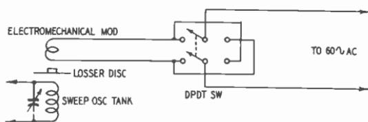
Fig. 511. Electromechanical modulation of oscillator circuit.
