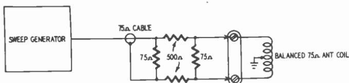
Fig. 1025. Termination pad helps convert single-ended generator output to double ended.
