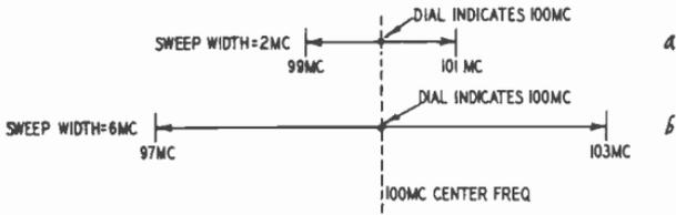
Fig. 107-a,b. When the sweep-generator dial indicates center frequency, the sweep-width control does not change the dial indication because equal frequency excursions occur above and below center frequency.
