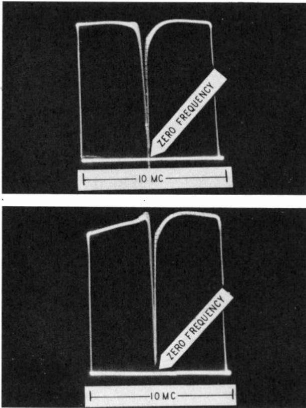
*Fig. 105. Sweep-flatness test of video-frequency range of sweep generator. The output of the generator contains a low-pass filter which eliminates all but the difference frequency from the output. The attenuator is not distortionless; above, attenuator at maximum setting; below, attenuator near minimum setting, scope gain advanced. Zero frequency appears in center of pattern. Sweep width is 10 mc or  $\pm 5$  mc either side of zero frequency.*
