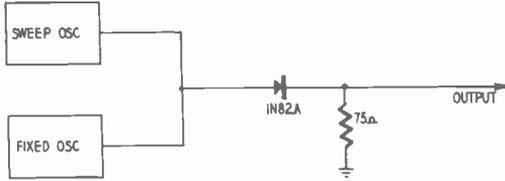
Fig. 212. Principle of a beat-frequency oscillator. Nonlinear mixing takes place in the crystal diode. Sum and difference frequencies appear across the 75-ohm load resistor.
