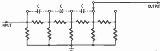
Fig. 308. One of the causes for leakage from a sweep generator. There is a certain small value of capacitance from one switch contact to the next (and from one lead to the next) providing a path for flow of high-frequency currents.
