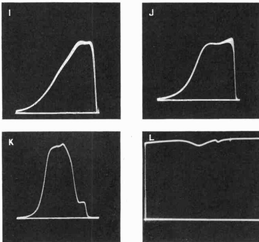
*Fig. 109-i,j,k,l. In (i) we have a Q demodulator response curve; sweep width of 3 mc is adequate; (j) frequency response of 1 video amplifier, sweep width, 6 mc; (k) frequency response of a chroma amplifier; sweep width of 5 or 6 mc is sufficient and (l) impedance check of an antenna and lead-in; maximum sweep width should be used. 12 to 15 mc is satisfactory.*
