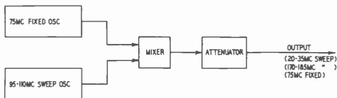
Fig. 237. Unfiltered output results in large numbers of undesired frequencies in the output.
