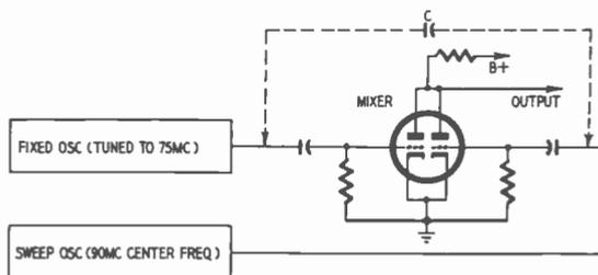
Fig. 408. When leakage occurs via stray capacitance  $C$ , the FM modulator not only varies the sweep oscillator, but also the fixed oscillator to some degree. The sweep output is not flat and if the sweep oscillator is keyed, the resulting zero-volt reference line exhibits kinking.
