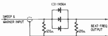
*Fig. 214. Practical arrangement for using the beat-frequency principle. Circuit has three crystal diodes to match the low impedance of the sweep output system.*
