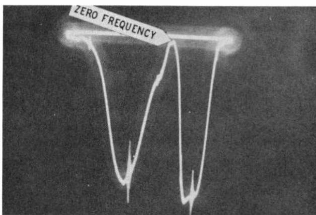
*Fig. 508. Low-frequency flatness test of a poor beat-frequency sweep generator. Zero frequency is located approximately in the center of the display. A severe fall-off of output starts at 2 mc (marker points) and proceeds progressively within the low-frequency region of the sweep. Another dropoff starts at 2 mc and proceeds progressively to 4 mc. The dropoff at frequencies below 2 mc is caused by use of too small a value of blocking capacitor in the mixer output circuit.*
