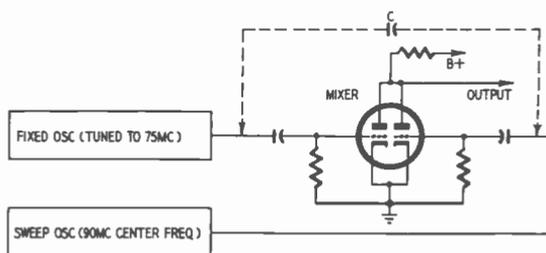
*Fig. 408. When leakage occurs via stray capacitance C, the FM modulator not only varies the sweep oscillator, but also the fixed oscillator to some degree. The sweep output is not flat and if the sweep oscillator is keyed, the resulting zero-volt reference line exhibits kinking.*
