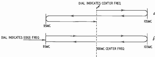
*Fig. 106-a,b. Distinction between center-frequency and edge-frequency indications.*
