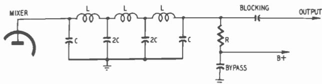
Fig. 314. When the mixer is followed by a low-pass filter, only the difference frequency is passed to the output.
