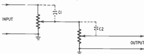
Fig. 515. Stray capacitances appear across the dual potentiometer.
