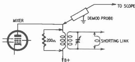
is then checked for zero beat at 98.7 mc ( $88 \text{ mc} + 10.7 \text{ mc}$ ). If zero beat occurs at this frequency the low-end tracking is accurate. But if you do not get zero beat then the tracking is off accordingly. It may be possible to bend the plates of the local oscillator tuning capacitor to improve the low-end tracking. Some receivers provide a low-frequency tracking adjustment. Consult the receiver manufacturer's service notes to determine the recommended procedure.
