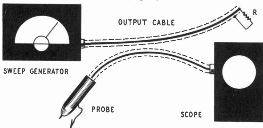
Fig. 401. The output cable from the sweep generator is terminated by the resistor  $R$ . In case deflection is obtained on the scope screen when the scope cable (with crystal probe) is brought near the output cable, it shows that the termination has not been properly.
