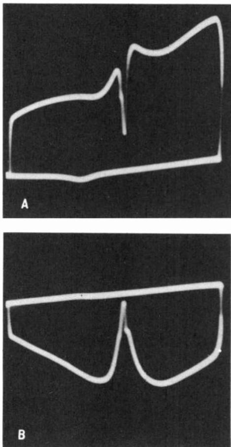
*Fig. 410-a,b. When the crystal diode is reversed in a demodulator probe, waveform error in the form of even-harmonic distortion will cause the sweep trace to change.*
