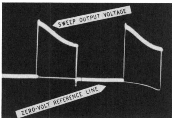
Fig. 104. Typical result of test depicted in Fig. 103, using 30-cycle sawtooth sweep for horizontal deflection of the scope beam.
