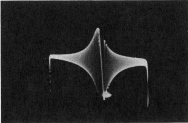
*Fig. 504. Demodulated waveform obtained by passing FM sweep waveform and marker generator voltage through a germanium crystal used as a nonlinear mixer. It can readily be seen that the sweep voltage is not uniform over the sweep range.*
