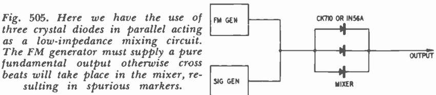
can be used. The outputs from an FM generator and from a signal generator are heterodyned in a suitable low-impedance triple-diode mixer arrangement to develop a low-frequency *difference* output. An arrangement of this type is capable of providing very-low-frequency sweeps, because of the extensive decoupling which is afforded. The two generators are isolated in separate cases, and the two outputs are also isolated by the output networks of the two instruments.
