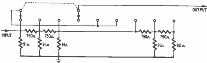
Fig. 306. Typical step-type attenuator. The network is a ladder construction, provides reasonably constant impedance at each step.
