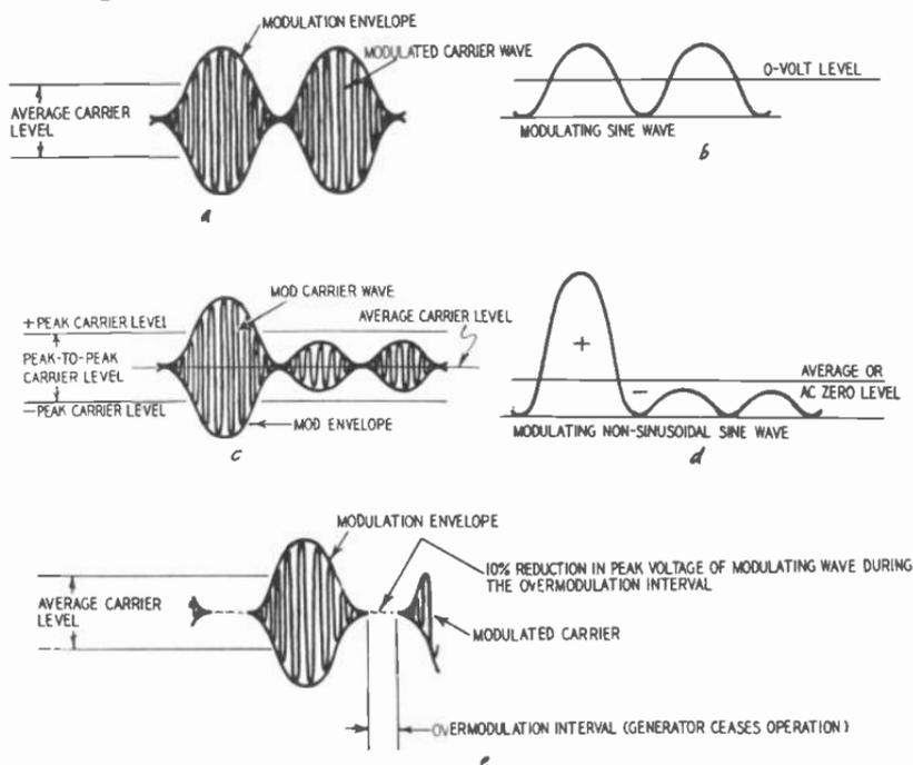
Fig. 606 (a to e). An illustration of 100% modulation (a) of an r.f. carrier. The modulating sine wave (b) represents an ideal condition. An illustration of 100% downward modulation but 300% upward modulation (c) of an r.f. carrier wave by a nonsinusoidal audio-frequency wave. The modulating waveform (d) is characteristic of some signal generators. Overmodulation (e) of an r.f. carrier wave.
