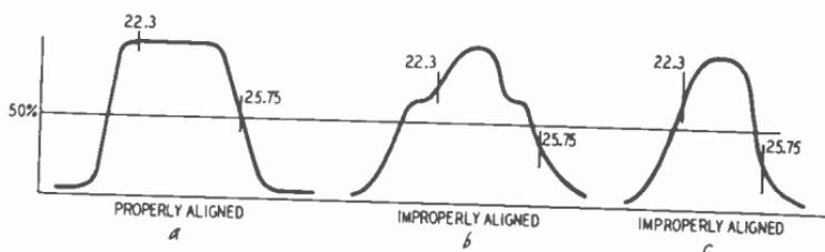
Fig. 1033-a,b,c. A properly aligned curve (a) shows that the ideal curve is essentially flat-topped. Undesirable peaking is seen in (b) and inadequate bandwidth is illustrated in (c).
