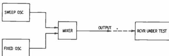
*Fig. 301. The first problem in application of the sweep signal to the circuit under test is to provide an output-cable arrangement which will transport the signal without distortion and essentially without loss.*
