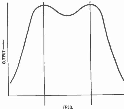
Fig. 908. Double-humped response of the i.f. section of an FM receiver. A limiter stage or ratio detector following the i.f. will flatten the top of the curve.
