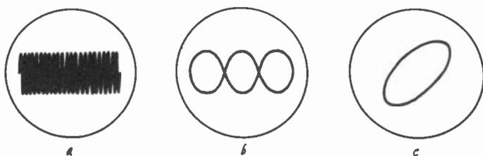
*Fig. 802-a,b,c. Screen pattern obtained on scope (a) when generator is far off zero beat. The Lissajous figure (b) when the generator is near zero beat and (c) generator zero-beat with horizontal sweep of scope; frequency coincident within 60 cycles. This zero-beat pattern may vary from a straight line through an ellipse to a circle, depending upon the phase relations of the beating voltages.*
