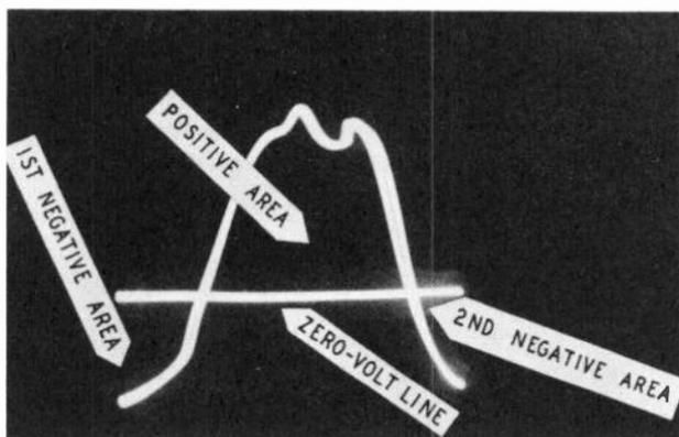
*Fig. 234. When a waveform is developed by use of 60-cycle sine-wave sweep, the spot moves fast over the center, but slowly at the ends of the pattern. The spot takes longer to traverse the negative excursion of the waveform, hence the time axis is compressed at the ends. Because the spot travels faster in the central region, the positive area of the pattern is larger than the sum of the negative areas.*
