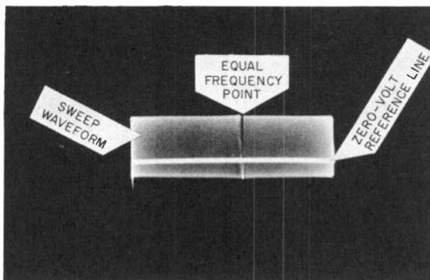
*Fig. 601. When the outputs from FM and CW generators are heterodyned, demodulated, and displayed on the screen of a wide-band scope, the display is marked by a small gap at the zero-beat point. At this point the frequencies of the two generators are instantaneously equal.*
