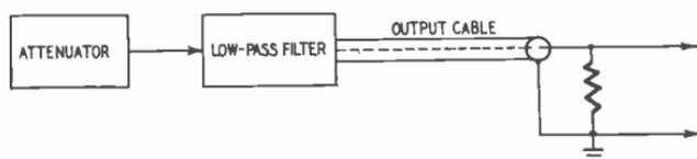
*Fig. 224. Location of the low-pass filter in the sweep-generator output system. The filter may be "built in" or constructed as a plug-in form. In some cases the filter can be switched in or out by means of a switch on the generator.*
