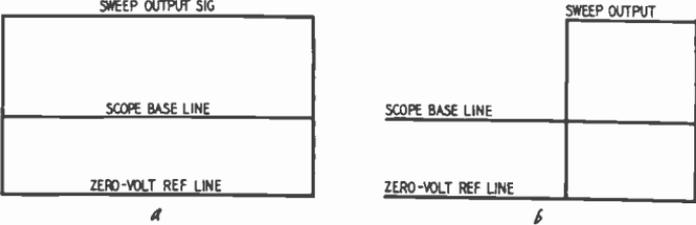
Fig. 232-a,b. The sweep signal and zero-volt reference line (a) are unequally spaced above and below the scope base line (resting position of the scope beam) when the sweep time is less than the zero-volt reference time. This is caused by inequality of keying periods. When the keyed output from the sweep generator is displayed on sawtooth sweep (b) the relative on-and-off times are readily apparent.
