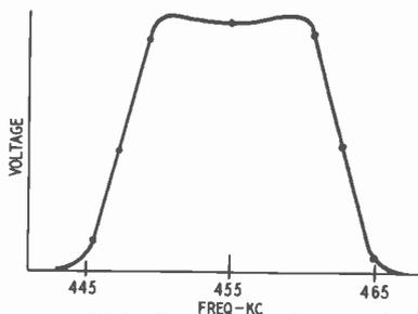
*Fig. 1001. You can make a point-by-point plot of a response curve by using an AM generator. This method is tedious and time consuming. It is a far easier and certainly a much better technique to use a sweep generator for this purpose.*
