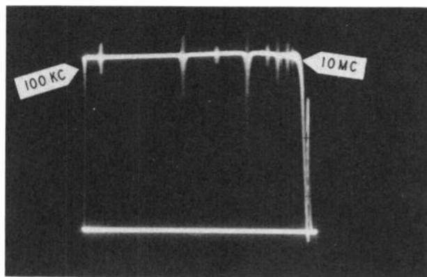
*Fig. 245. The advantage of an absorption marker is that it results in fewer spurious pips on the sweep waveform. Note the large number of pips produced by beat markers.*
