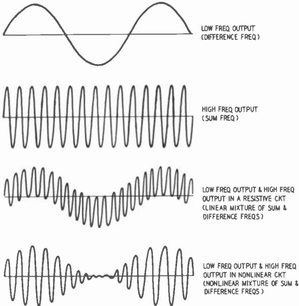
*Fig. 217. Some fundamental types of signal voltages which may be present simultaneously in the output of elementary types of beat-frequency sweep generators.*
