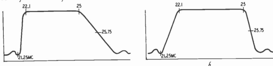
Fig. 204-a,b. Typical response curve (a) displayed on scope screen when sweep-frequency output from generator has good horizontal linearity. Nonlinear sweep-frequency (horizontal nonlinearity) expands curve (b) on left-hand side, compresses curve on right-hand side. Note that markers appear at the same level on both curves.
