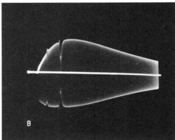
*Fig. 243-a,-b. Marker at 100 kc (a) and at 200 kc (b). Marker disturbances are caused by spurious outputs from the generator. For example, the intended absorption marker is illustrated above in the photo (b) at 200 kc. An undesired harmonic causes a smaller spurious marker to appear at the left in the sweep waveform at the 100 kc point.*
