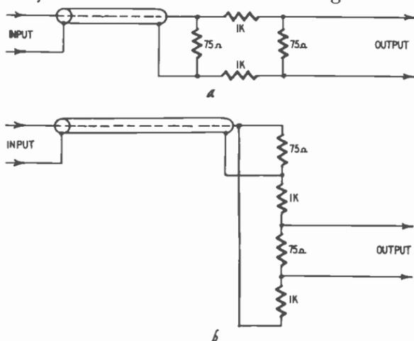
Fig. 319-a,-b. The use of the resistive H pad (a) also provides conversion of single-ended to double-ended output at the expense of voltage attenuation. This principle is clearer from the redrawn circuit (b). Note that both sides of the output are now above ground and although an attenuation of approximately 30 times is incurred, an effectively balanced output is provided.
