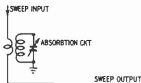
*Fig. 707. Typical circuit used for producing an absorption type marker in the sweep output waveform. The name "absorption circuit" is somewhat misleading since the circuit does not absorb energy, but reflects a high impedance into the sweep output circuit at the resonant frequency of the absorption circuit.*
