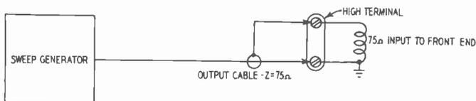
Fig. 1022. This method of connecting the sweep generator to the receiver input is also incorrect.
