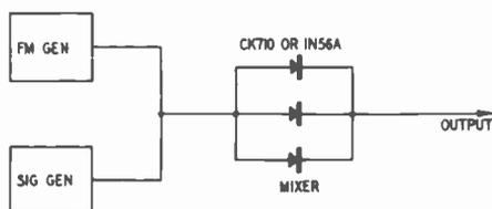
can be used. The outputs from an FM generator and from a signal generator are heterodyned in a suitable low-impedance triple-diode mixer arrangement to develop a low-frequency *difference* output. An arrangement of this type is capable of providing very-low-frequency sweeps, because of the extensive decoupling which is afforded. The two generators are isolated in separate cases, and the two outputs are also isolated by the output networks of the two instruments.
