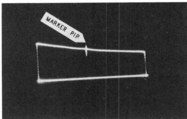
*Fig. 602. When the output from an FM generator is mixed with the output from a CW generator, demodulated, and displayed on the screen of a narrow-band scope, the display is marked by a pip at the zero-beat point. The pip has the same bandwidth as the scope.*
