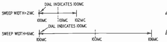
Fig. 108-a-b. When the sweep-generator dial indicates edge frequency, the sweep-width control causes a shift of center frequency when reset, because the deviation is not a plus-and-minus excursion about center frequency.
