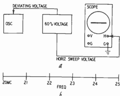
Fig. 202-a,-b. When a 60-cycle sine-wave voltage (a) is used to drive the vibrator in the sweep-oscillator circuit and the same sine-wave voltage deflects the scope beam horizontally, a linear frequency sweep is obtained. (if properly designed) equal horizontal intervals correspond to equal frequency increments. (b)
