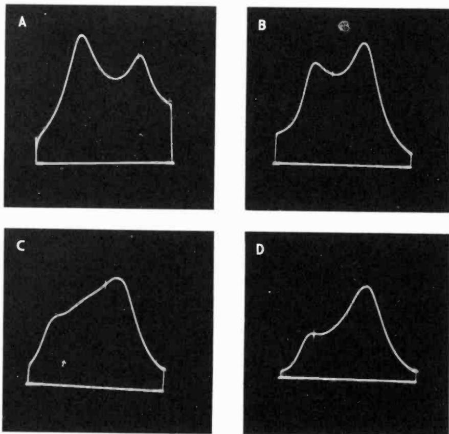
*Fig. 109-a, b, c, d. Front-end response curves for v.h.f. television bands, displayed on a sweep width of 12 megacycles. (a) channel 2; (b) channel 3; (c) channel 4; (d) channel 5. These curves depart considerably from the receiver manufacturer's specifications and require attention.*
