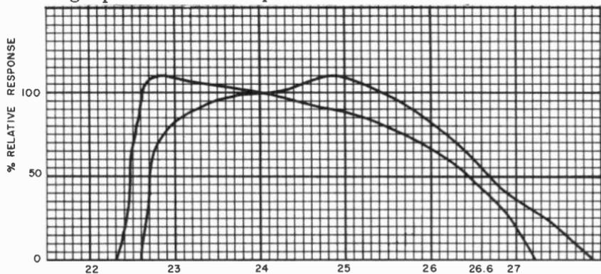
Fig. 1035. Typical tolerable variation in shape of i.f. response curve obtained in step (d) of Fig. 1034. Note that an ideal response curve is usually unobtainable.
