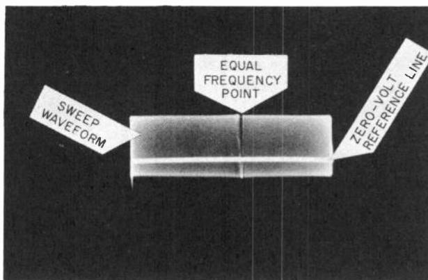
*Fig. 601. When the outputs from FM and CW generators are heterodyned, demodulated, and displayed on the screen of a wide-band scope, the display is marked by a small gap at the zero-beat point. At this point the frequencies of the two generators are instantaneously equal.*
