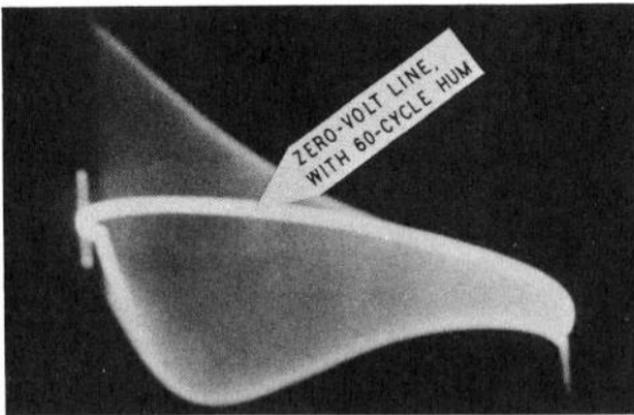
*Fig. 409. Leakage between sweep and fixed oscillators in the beat-frequency generator causes substantial even-harmonic distortion at low frequencies. The curvature of the zero-volt reference line and sweep output is due to the presence of 60-cycle hum voltage in the generator output system.*
