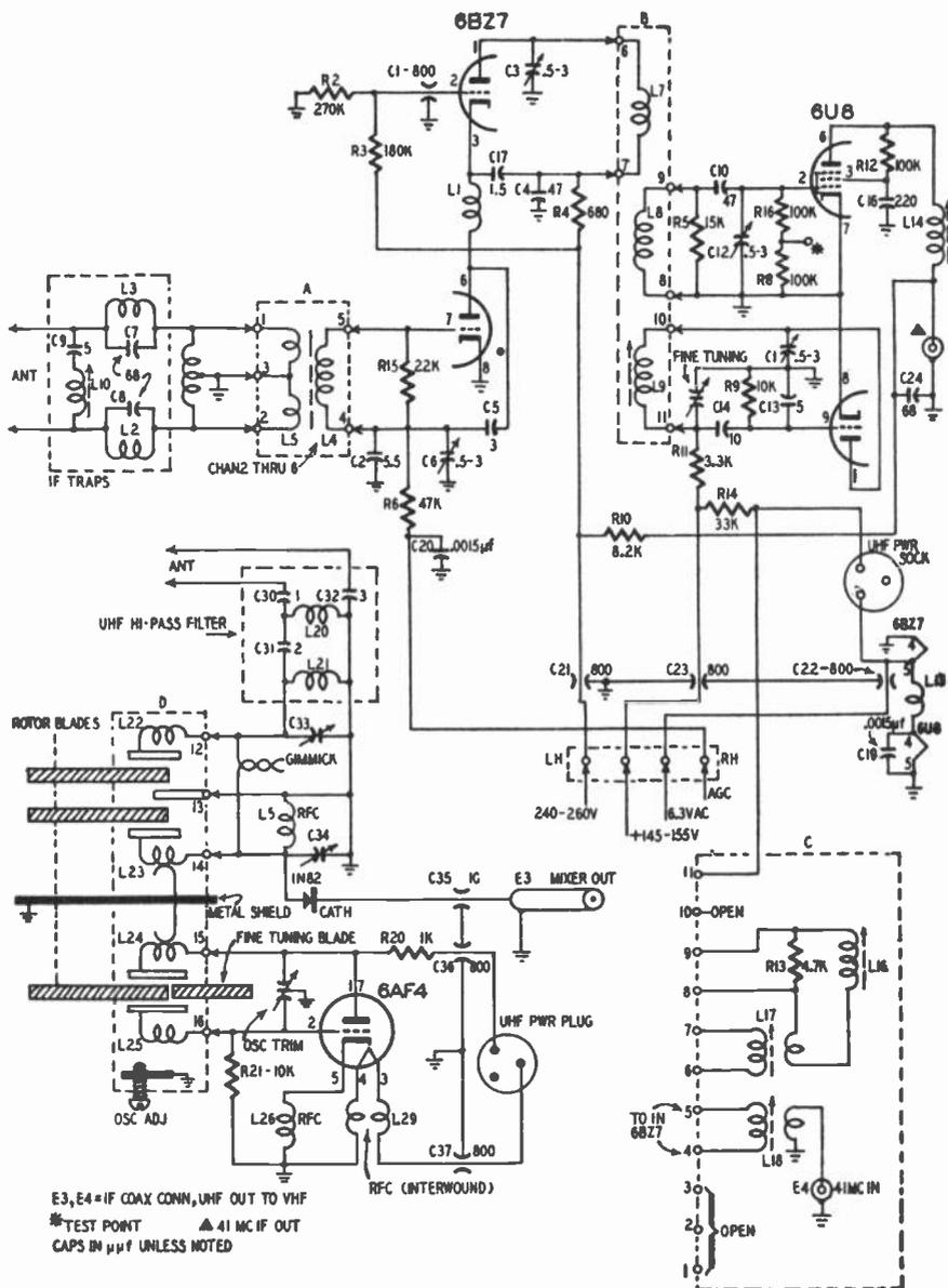
Fig. 1040. Schematic diagram of all-channel turret-type television tuner.
