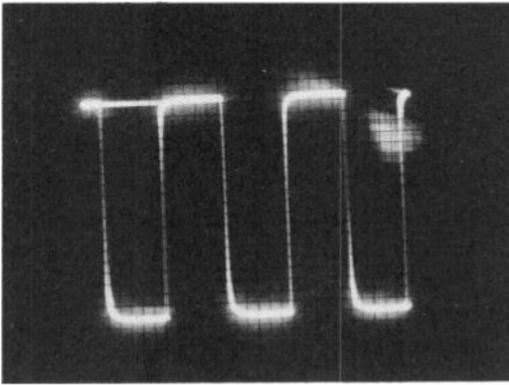
*Fig. 230. A 60-cycle square-wave voltage which can be utilized for keying the control grid of the sweep oscillator to develop a zero-volt reference line.*
