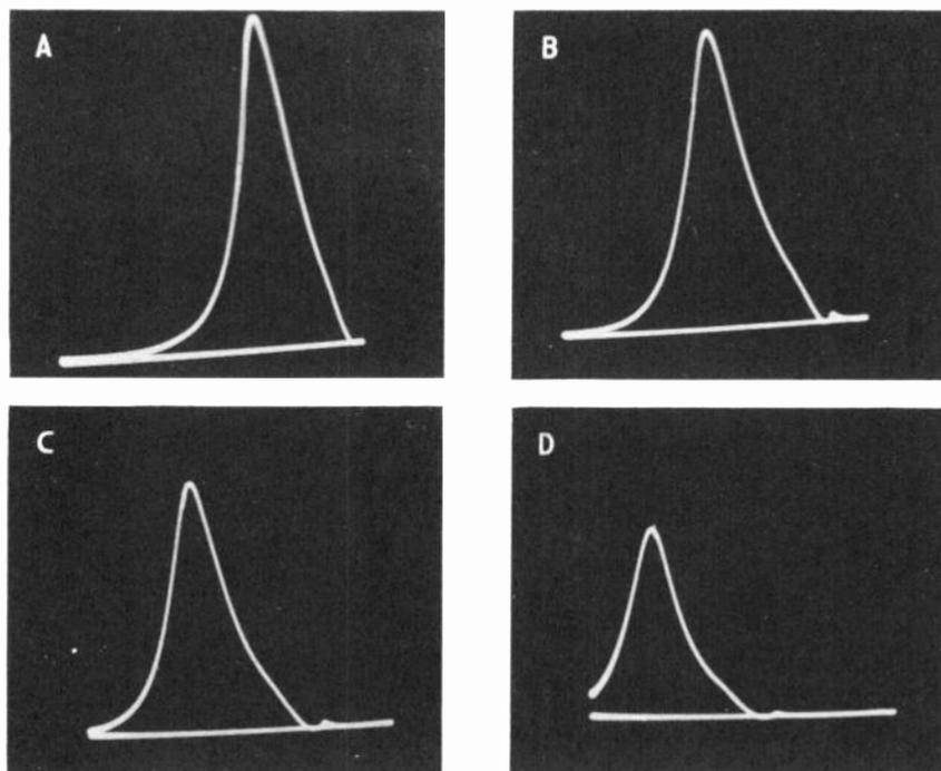
*Fig. 221. Illustrations of the variations in height of an i.f. response curve as the tuning control of the sweeper is varied from one end of the base line to the other. This is caused by change of the L-to-C ratio in the fixed oscillator tank as the tuning capacitor is rotated. A flatness check with a demodulator probe will show that the output is flat over the swept band.*
