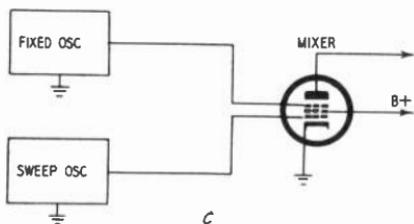
Fig. 239-c. The fixed and sweep oscillators are still less extensively coupled due to still smaller effective capacitance between the suppressor output and control grids. Still more extended low-frequency response can be obtained.
