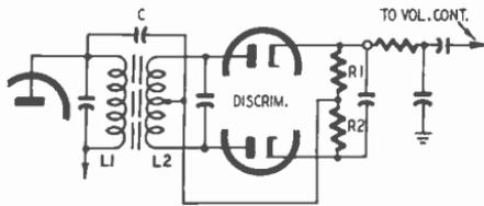
*Fig. 910. Typical discriminator arrangement. The test meter is connected across  $R_1$  and  $L_1$  is adjusted for maximum output. The meter is then placed across the total diode load ( $R_1$  and  $R_2$ ) and  $L_2$  is adjusted to null at the i.f. center frequency.*
