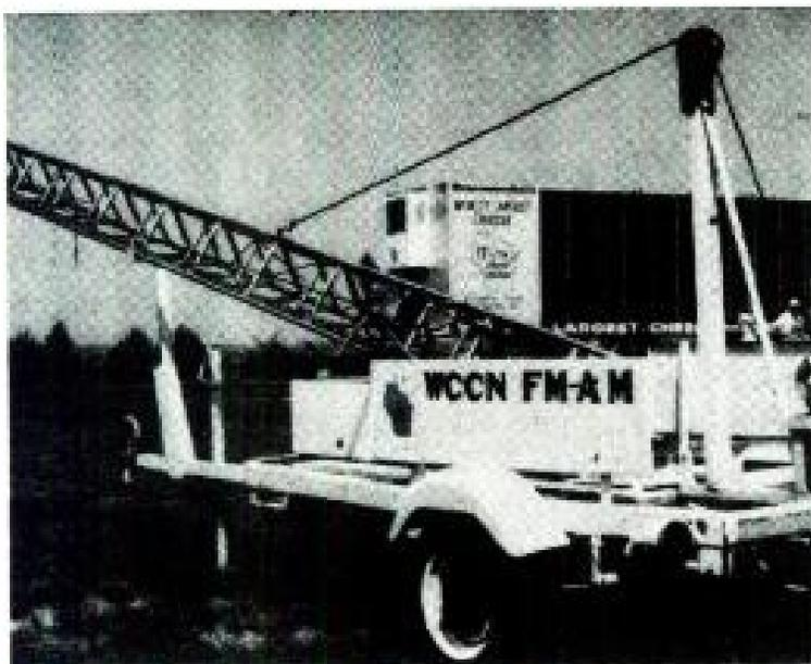
Trailer-mounted crank-up antenna facilitates remote operation. Last 20-ft section isn't extended till distance from antenna exceeds 25 miles.
