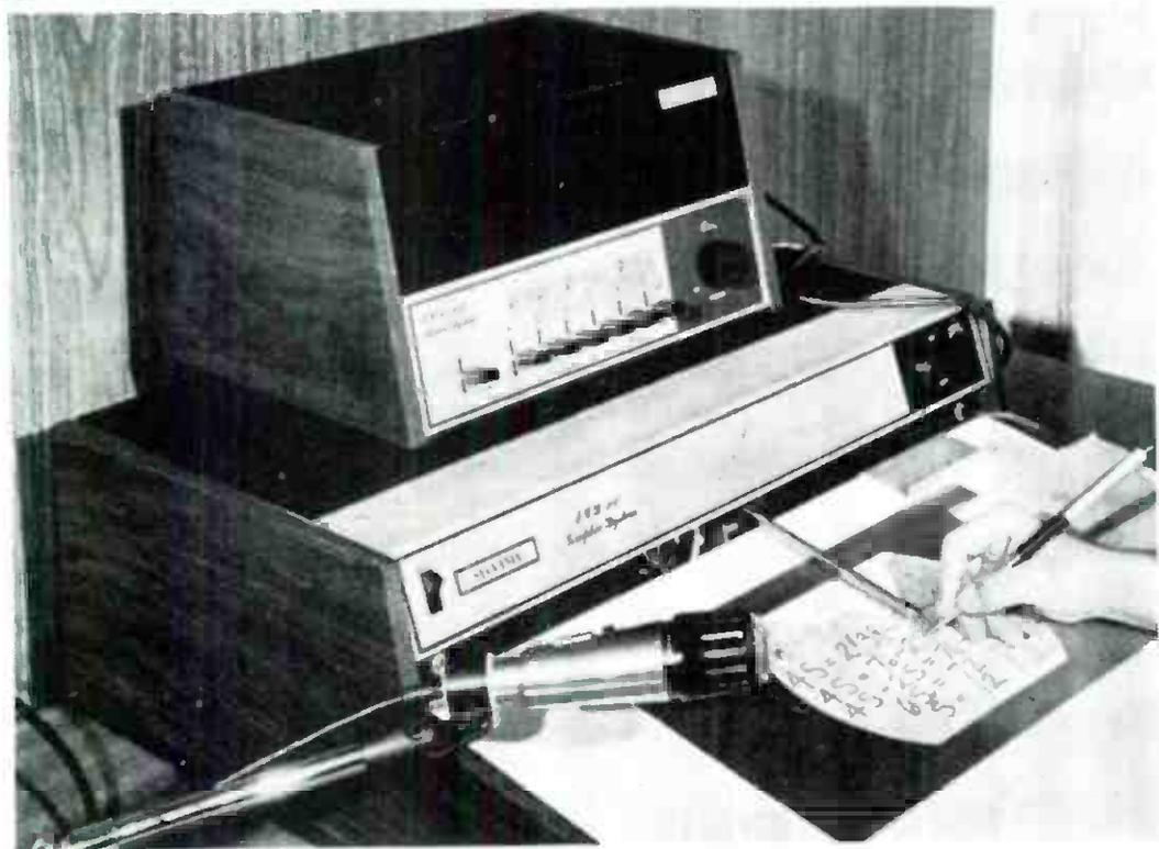
Hardware for transmission of visual material via SCA or telephone lines. The Victor Electrowriter Remote Blackboard (VERB) shown above transmits handwritten notations. Sylvania's ECS-100 blackboard-by-wire system (below) has the additional capability of storing visual material for up to one hour.
