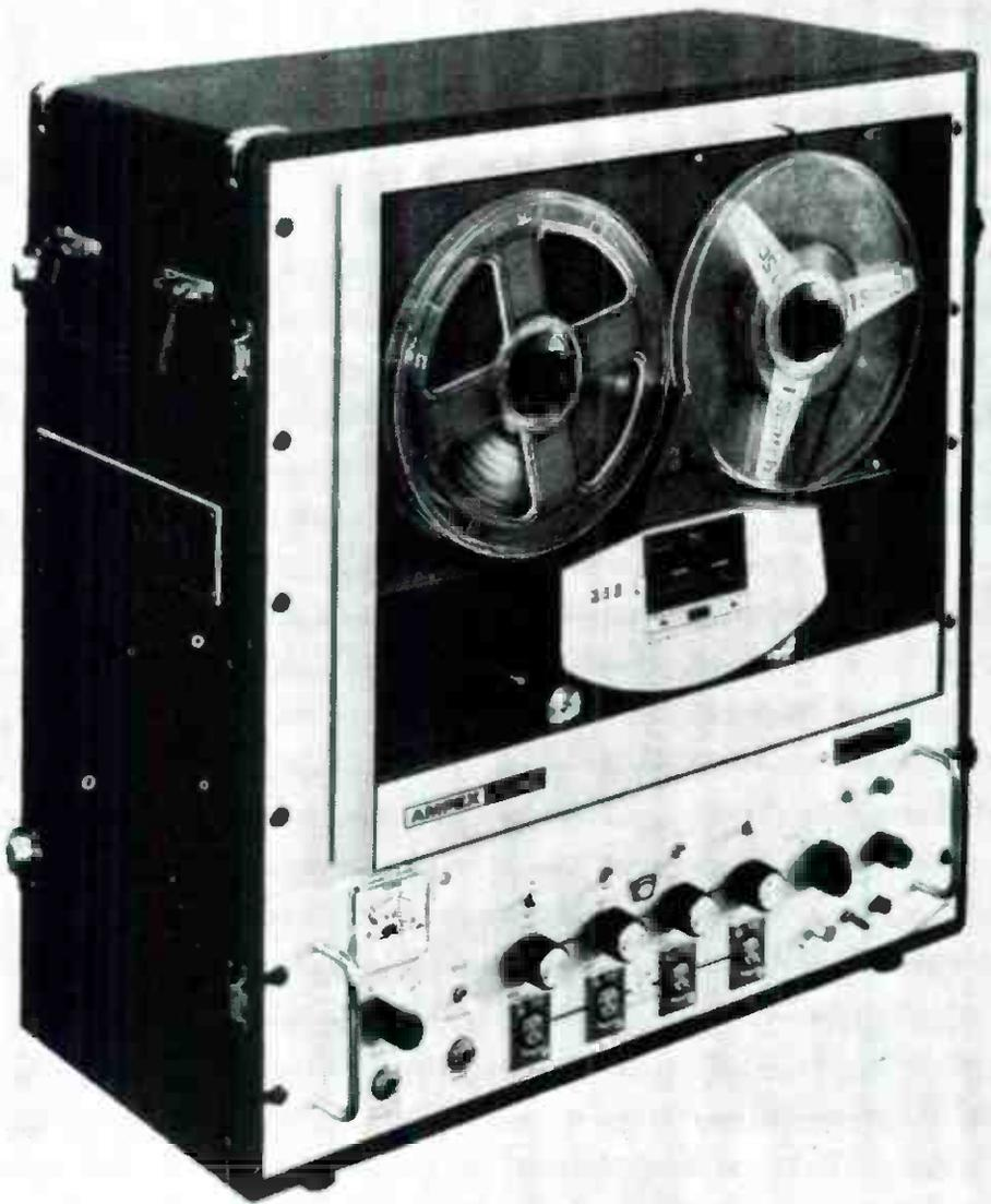
Modified Ampex recorder plays back four tracks simultaneously for the four concurrent programs going out on SCA channels.
