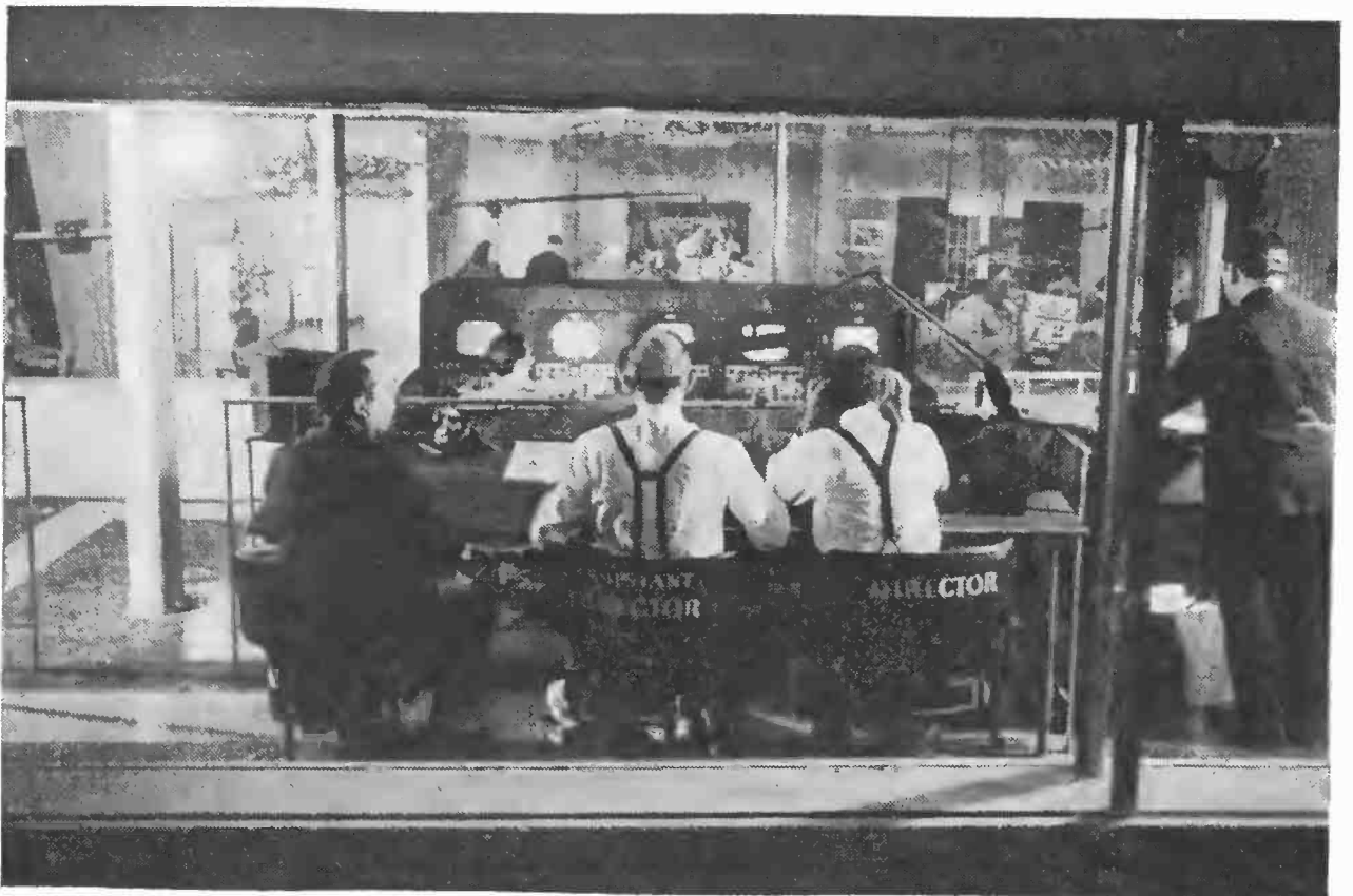
The new Du Mont Wanamaker studios from the rear of the control room. The five-screen viewing system is seen in the center of the picture with three studio sets in the background.
