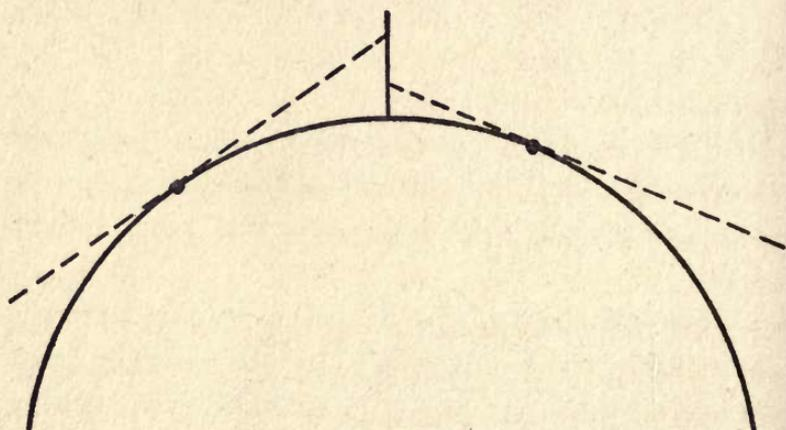
Signals broadcast from a high television antenna can be received at a greater distance than from a low one, since the beams travel in a *straight* line and cannot follow the curvature of the earth.
