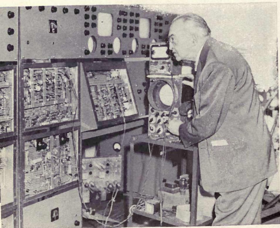
*Here the author uses an oscilloscope for testing a circuit. The "lazy Joe" patterns which appear indicate to television experts where in the "bird's nest" the trouble is.*
