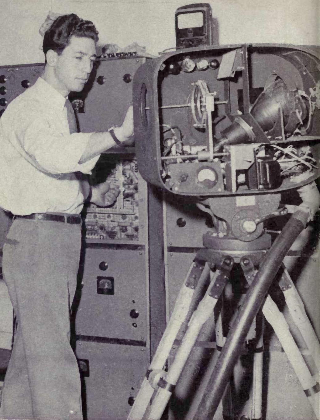
*We see here a television camera with the side removed so that we can learn a little about the maze of wires and strange tubes and lenses which make up its working parts. The large conduit leading from the front of the camera is a coaxial cable.*
