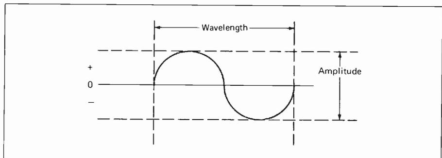
**Figure 9-3.** Wavelength and Amplitude. Amplitude—strength of a radio wave—is indicated by the distance from the top of the positive phase to the bottom of the negative phase. The stronger the radio wave, the greater the amplitude. The distance one radio wave travels through space before another is radiated is called the wavelength. Wavelength is indicated on a sine wave as the distance from the beginning of the positive phase to the end of the negative phase.
