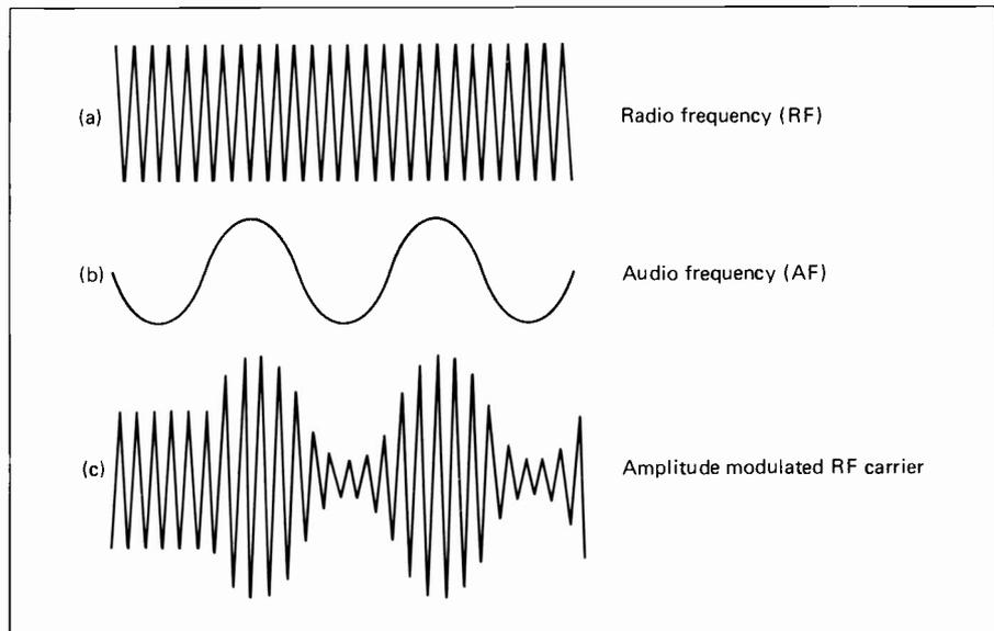
**Figure 10-11.** Amplitude Modulation. (a) Radio frequency (RF), that is, unmodulated carrier. (b) Audio frequency (AF). (c) Amplitude modulated RF carrier.
