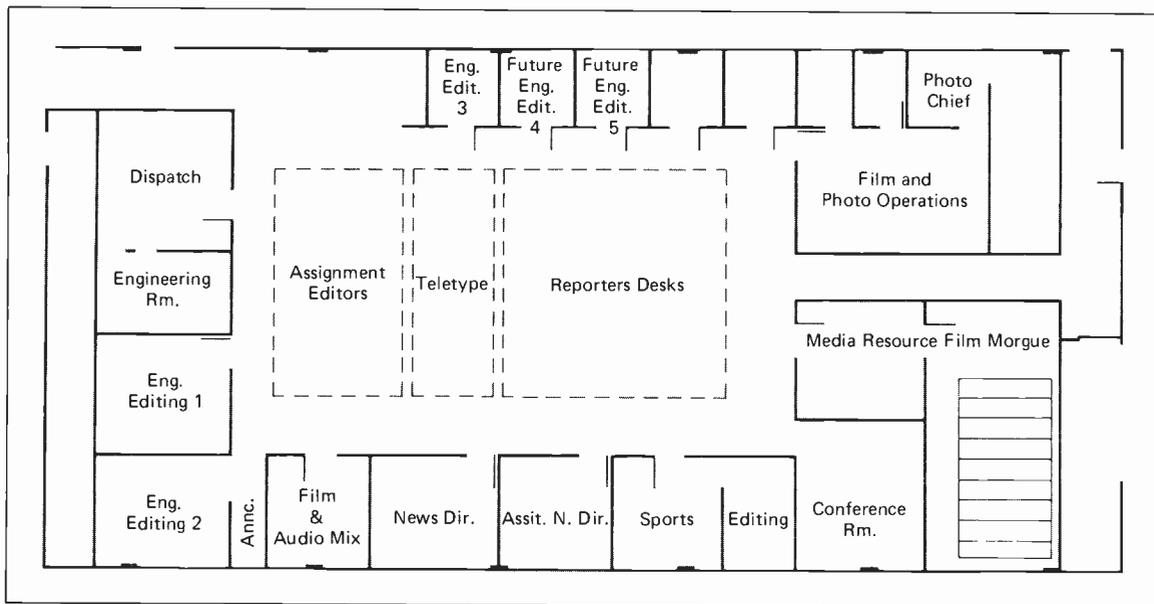
**Figure 18-3.** Floor Plan of Television Newsroom. KSTP-TV, channel 5, the ABC affiliate for Minneapolis-St. Paul, designed its newsroom for optimum efficiency.
