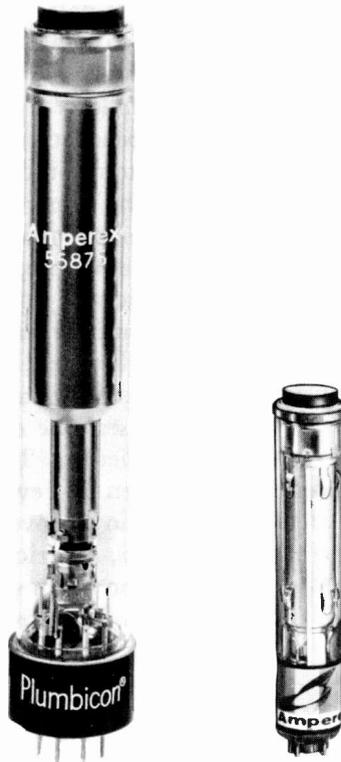
**Figure 11-2.** Plumbicon Camera Tubes. Tube at left (a) is used in studio color television cameras; that at right (b), in portable, hand-held color cameras.
