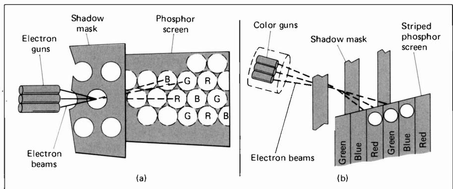
**Figure 11-11.** Two Types of Color Television Tubes. (a) Most American-manufactured tubes: beams converge through hole in shadow mask to hit triad. (b) Trinitron: beams converge through aperture grill to hit phosphors in stripes.
