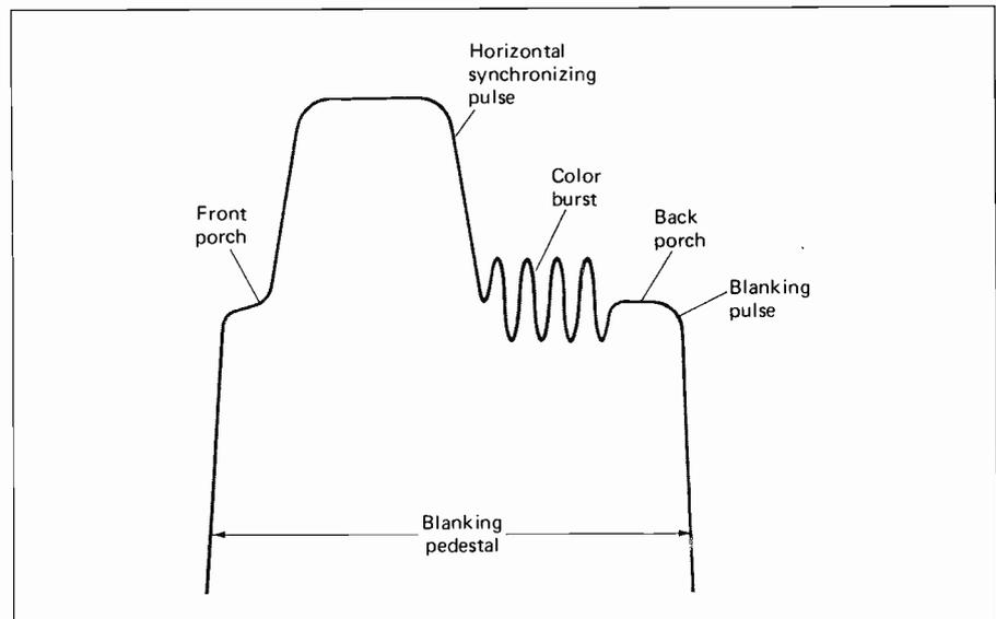
**Figure 11-7.** Accessory Signals: Color Burst, Sync, and Blanking.
