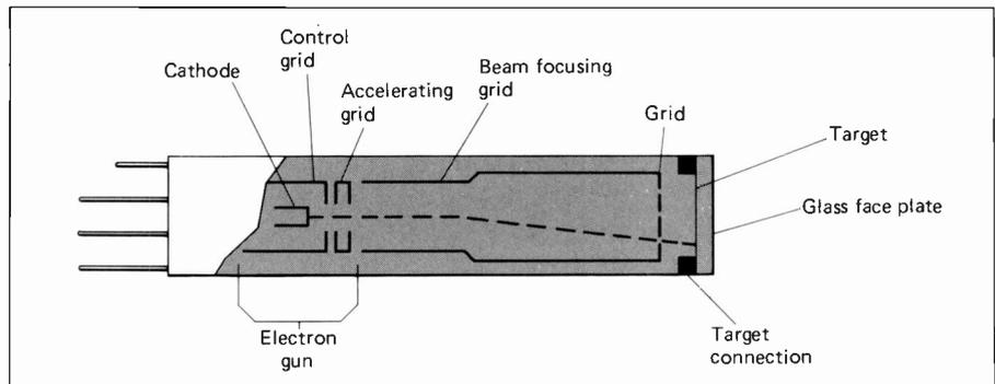
**Figure 11-3.** Structure of Vidicon Camera Tube. The dashed line shows the path of the electron beam. The video signal is conducted from the tube via the metal collector ring.
