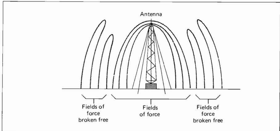
**Figure 9-2.** Lines of Force Radiating from Antenna. Alternating current in the antenna sets up fields of force (electric fields and magnetic fields) around the antenna. If the current frequency is high enough, these fields break free and continue to travel through space as electromagnetic waves.
