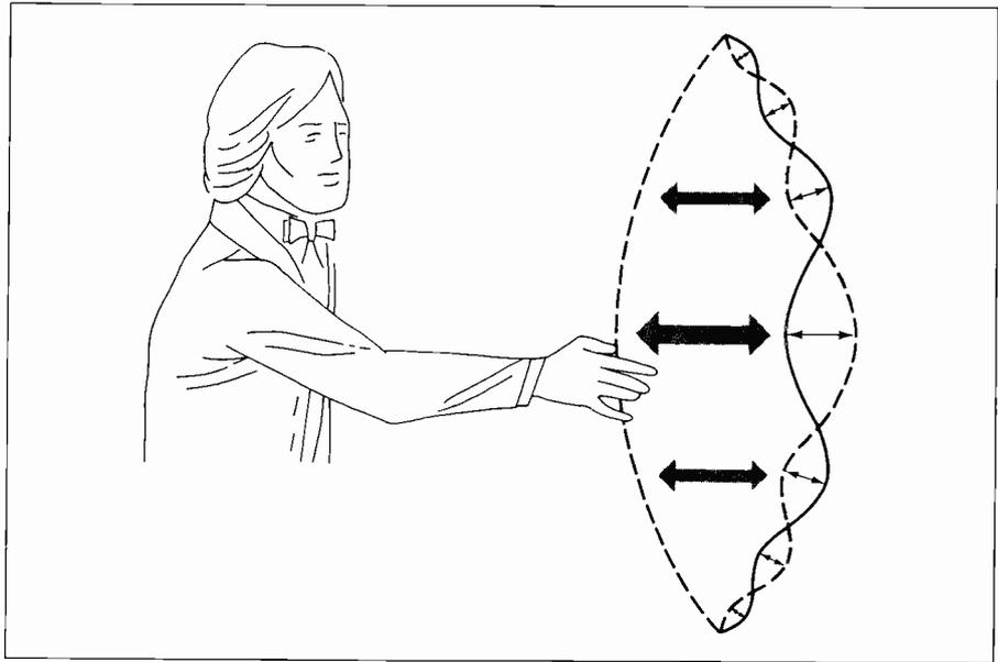
**Figure 10-8.** Creation of Overtones. Again, the example is our harp string. Not only does the whole string move back and forth, but individual segments of the string also move back and forth. The string's gross movement creates the fundamental tone, the note that you hear. Its segmental movements create overtones.
