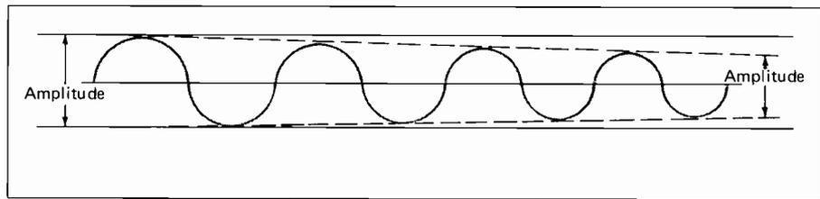
**Figure 9-4.** Attenuation. As radio waves travel, amplitude decreases.
