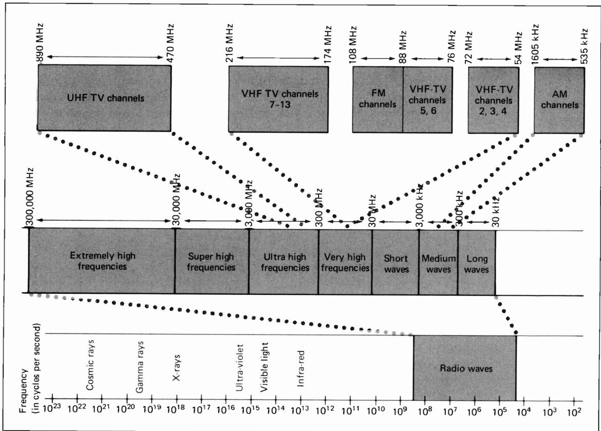
**Figure 9-6.** Electromagnetic Spectrum.
