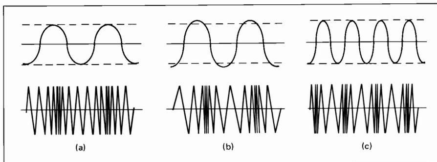
**Figure 10-15.** Frequency Modulation of Frequency and Amplitude. (a) The AF signal (top) modulates the frequency of the carrier (bottom). (b) Increased amplitude in the AF signal (top) intensifies the frequency groupings in the RF signal (bottom). (c) Increased frequency in the AF signal (top) produces a greater number of frequency groupings in the RF signal (bottom).
