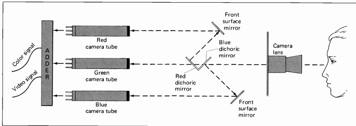
Figure 11-1. Block Diagram of a Color Television Camera.
