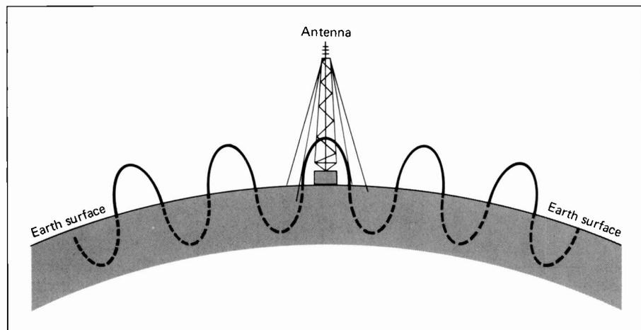
**Figure 9-7.** Ground Wave Propagation.
