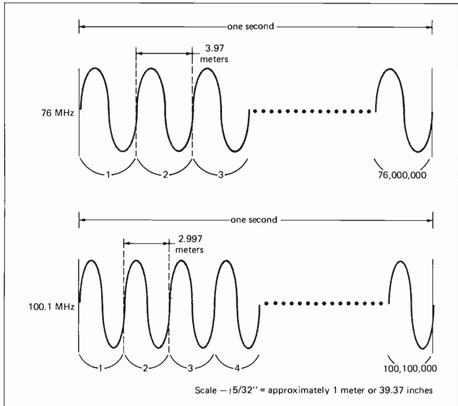
**Figure 9-5.** Frequency and Wavelength. Since velocity is constant, the only way to increase frequency (say, from 76 MHz to 100.1 MHz) is to decrease wavelength (here, from 3.97 meters to 2.997 meters).
