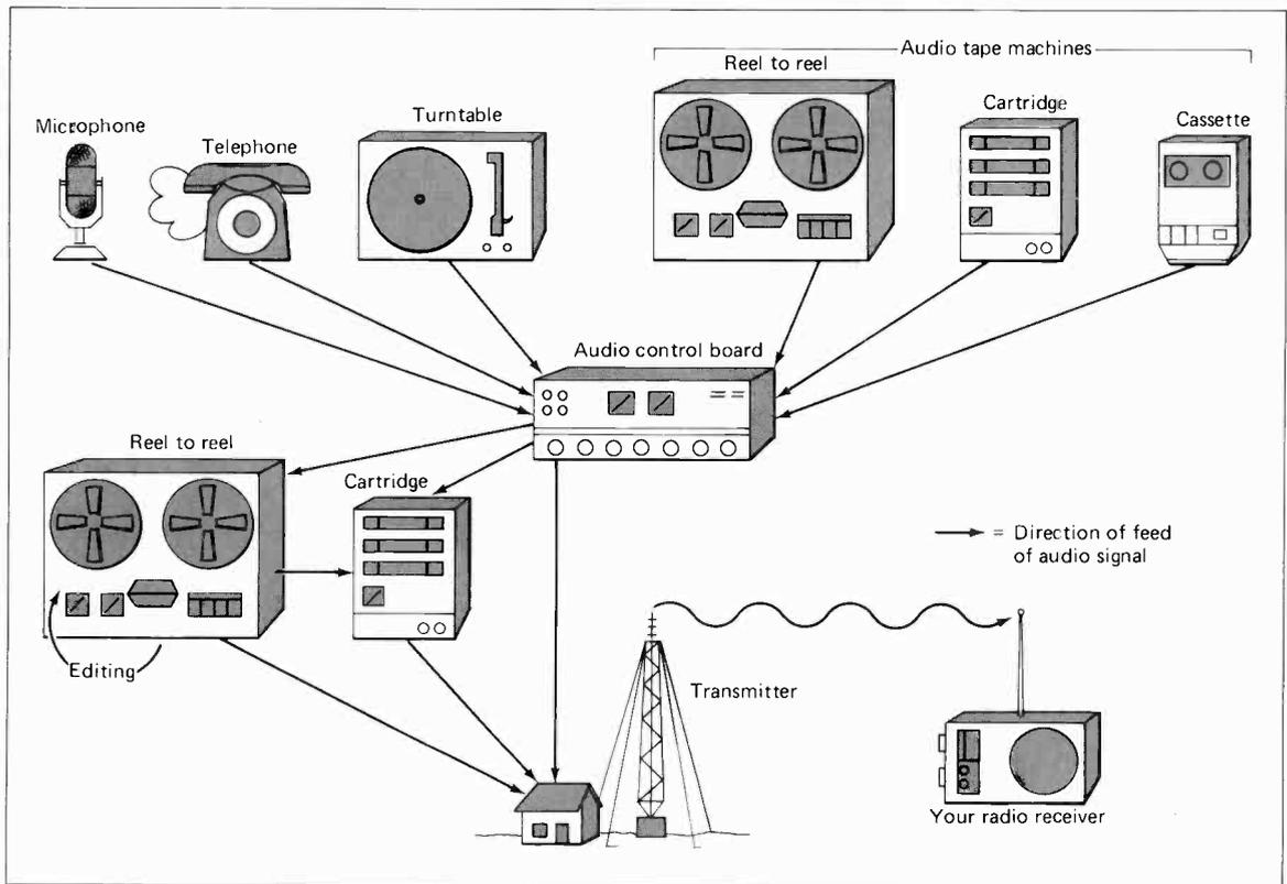
Figure 5-2. Radio Production Process.
