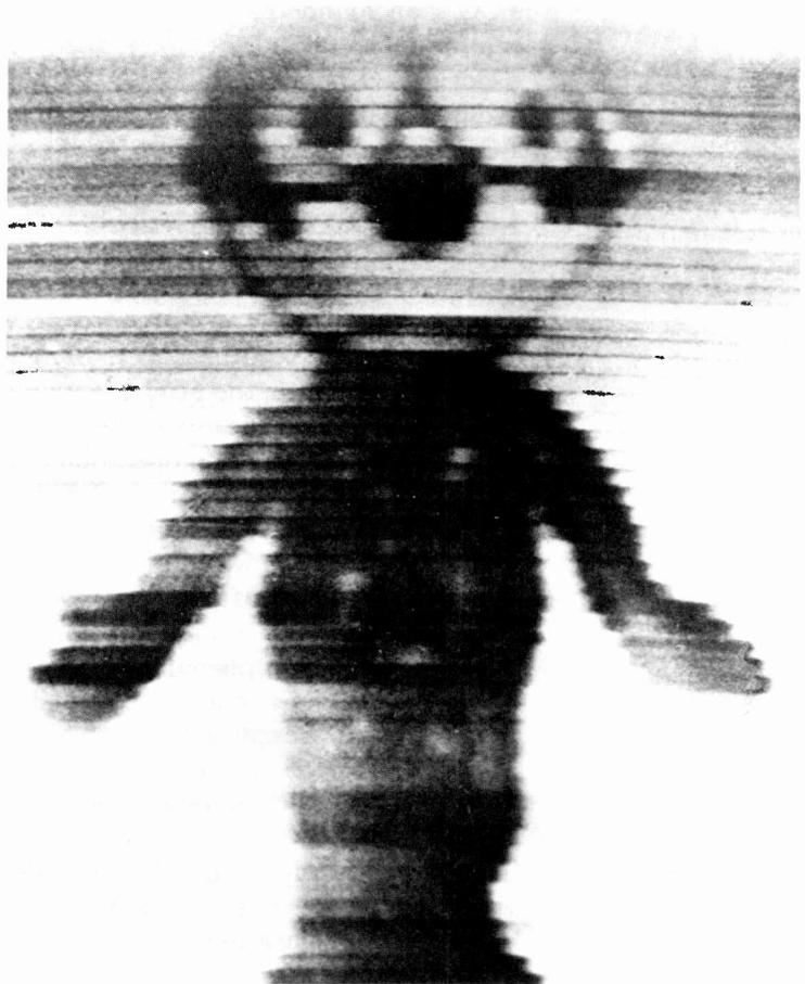
**Figure 4-3.** 1928 Television Picture. In 1928, RCA-NBC cameras ran experimental transmissions in mid-Manhattan, including this 60-line version of Felix the Cat.
