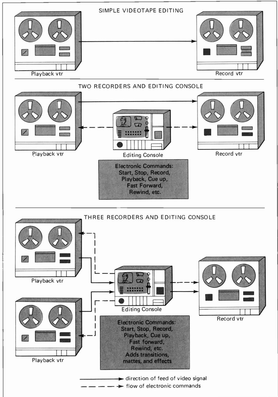
Figure 5-10. Videotape Editing Process: Three Methods.
