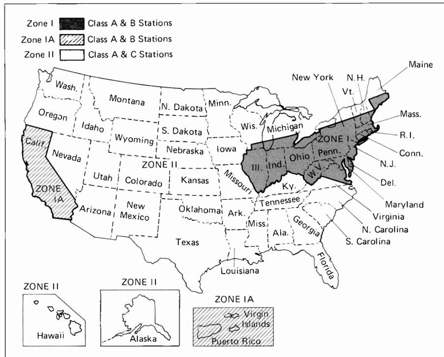
**Figure 10-4.** FCC's FM Zones and Types of Stations Operating in Each Zone.
