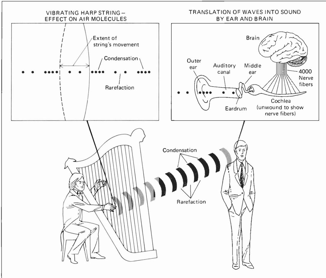
**Figure 10-6.** Origination, Transmission, and Reception of Sound. The condensation-rarefaction patterns (in the air molecules) radiate outward in all directions from the sound source. For clarity, the illustration shows the waves going only to the listener's ears, and the inserts show only one line of air molecules.
