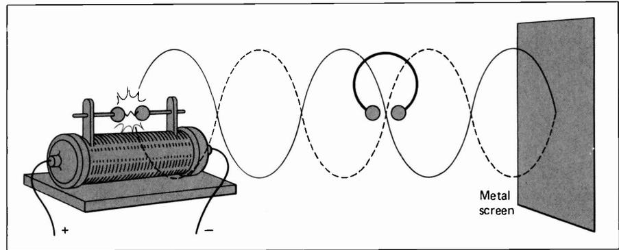
**Figure 2-1.** Hertz's Device. The wires led to a power source. The power source caused electrical sparks to oscillate between the two metal balls. These sparks sent out waves of high frequency alternating current. The waves hit a metal screen which reflected them. When properly positioned between the spark gap and the metal screen, an open copper wire loop would spark in resonance with the metal balls.
