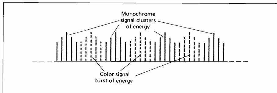
**Figure 11-6.** Interleaving of Color Information. The clusters of energy carrying color information are placed in gaps between those carrying video (monochrome) information.
