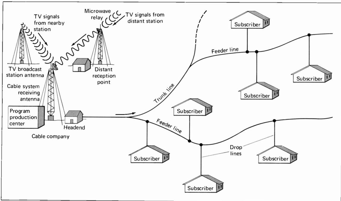
**Figure 21-1.** Typical Cable System. This system uses a combination of direct off-air reception and microwave relay (i.e., the signals of stations too distant for direct off-air reception are picked up nearer their transmitters, then relayed to the cable company's headend via microwave transmission).
