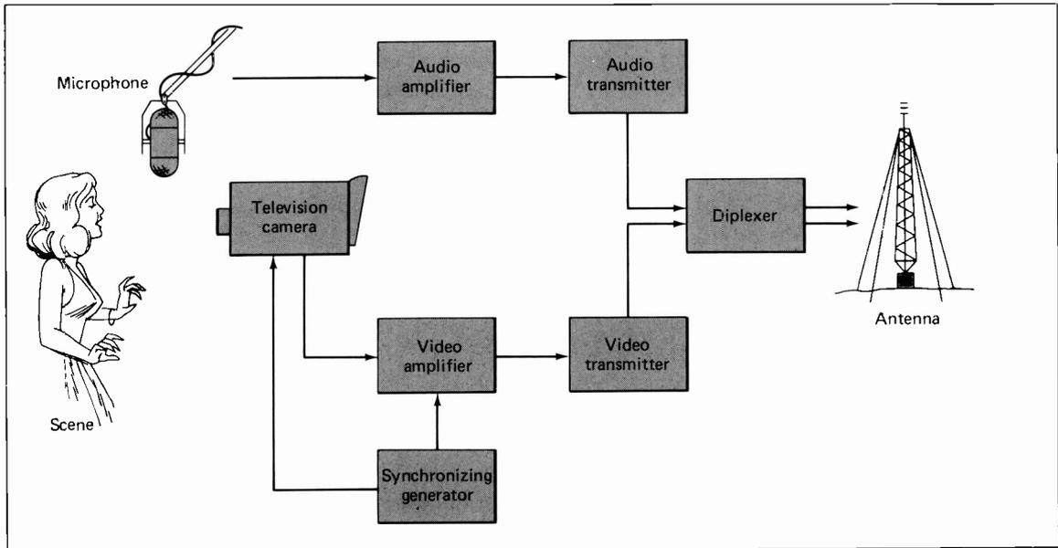
**Figure 11-9.** Block Diagram of Television Station and Transmitter.
