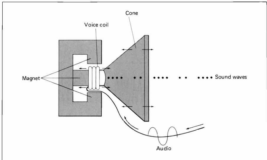
**Figure 10-14.** Speaker: Conversion of Audio into Sound. Note the similarity in construction and operation to the dynamic microphone (Figure 10.9).
