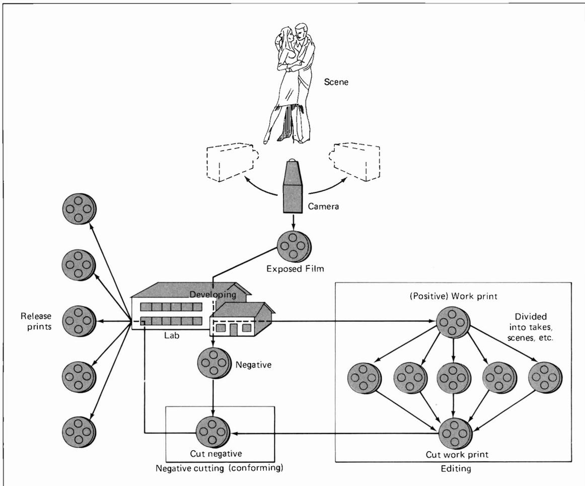
**Figure 5-13.** Film Production Process. Audio, design, costuming, opticals, and many other steps have been omitted for the sake of clarity.
