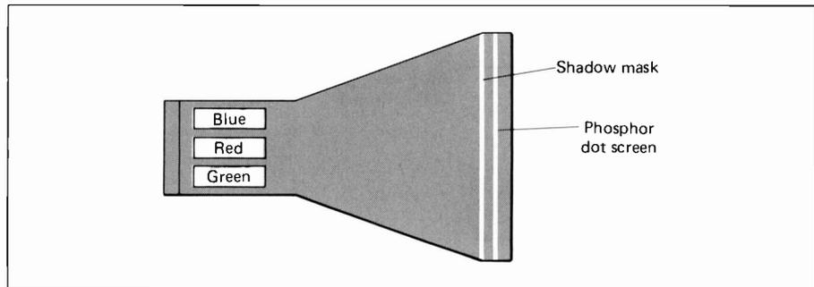
**Figure 11-10.** Color Receiver Picture Tube.
