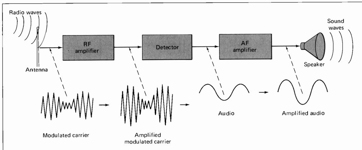
**Figure 10-13.** Block Diagram of an AM Receiver. The radio waves induce a weak reproduction of the modulated carrier frequency in the antenna. A tuner (not pictured) blocks all frequencies except those in the channel to which you have tuned. An RF amplifier boosts the modulated RF carrier frequency. A detector recovers the audio signal and grounds out the RF. An AF amplifier boosts the audio signal and feeds it to the speaker.
