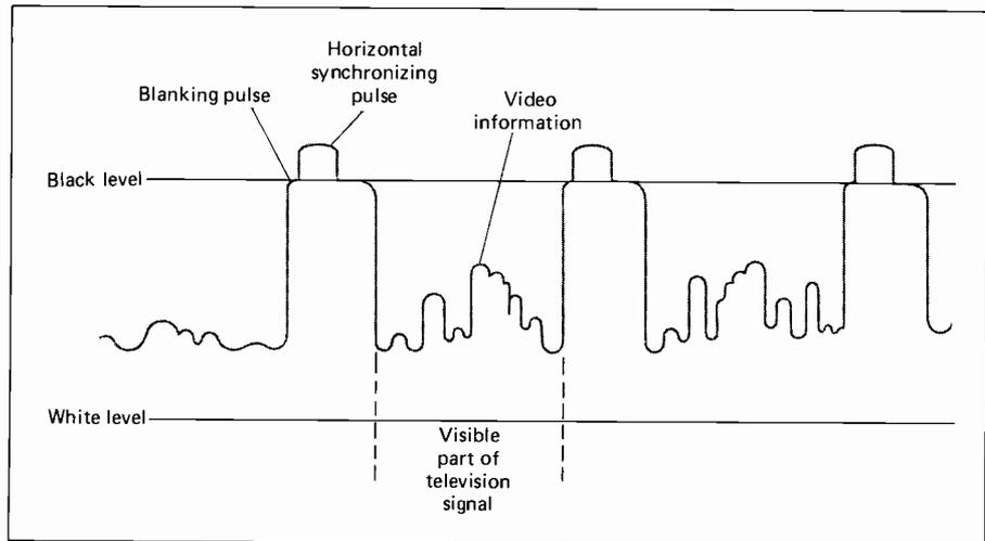
**Figure 11-8.** Video Signal and Accessory Signals. This diagram shows three horizontal lines of video signal with accessory signals.
