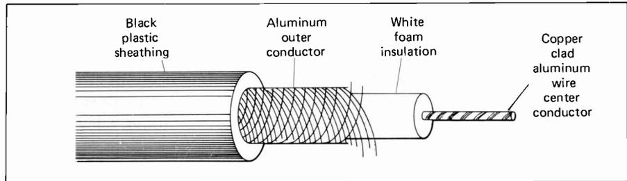
**Figure 21-4.** Coaxial Cable.
