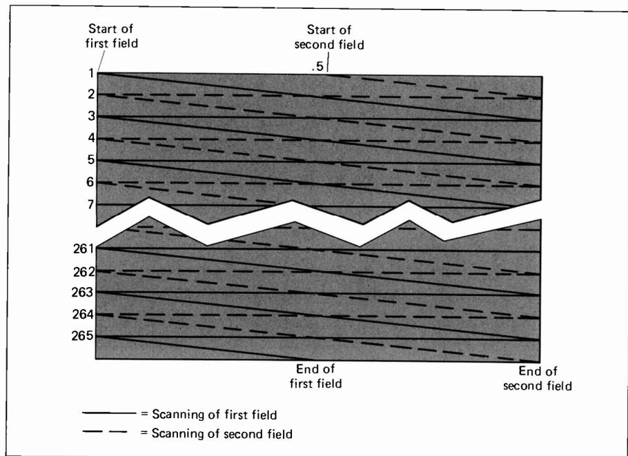
**Figure 11-4.** Interlaced Scanning Pattern.
