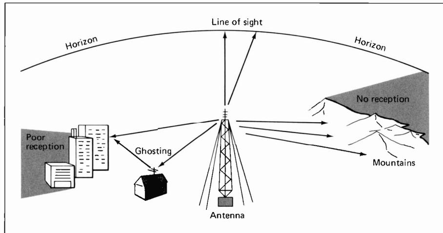
**Figure 9-9.** Direct Wave Propagation.
