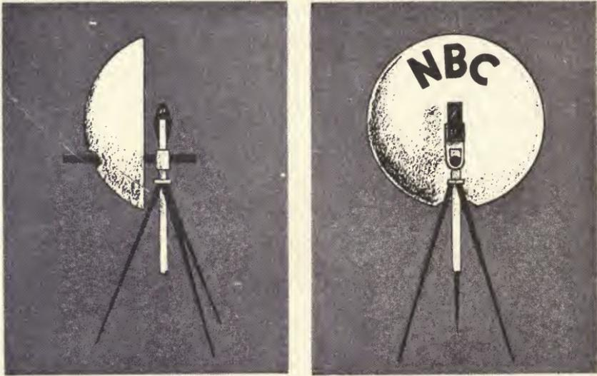
*Figure 36.* Microphone with parabolic reflector.
