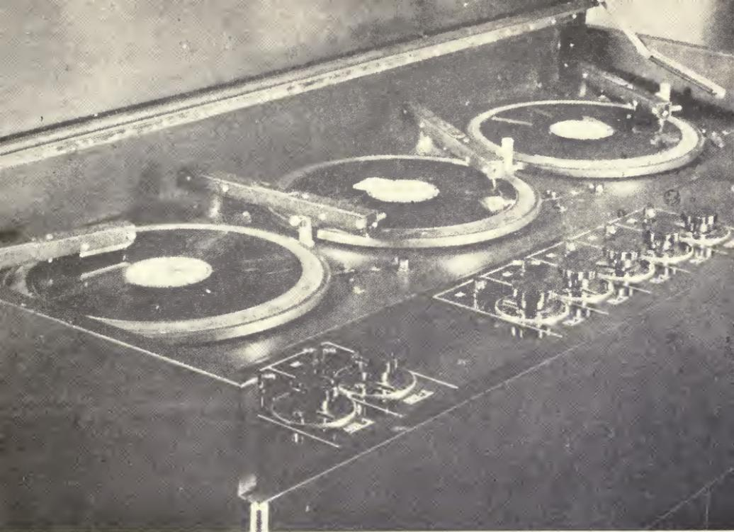
Figure 46. Turntable-speaker combination (*bottom*). Close-up of turntables (*top*).
