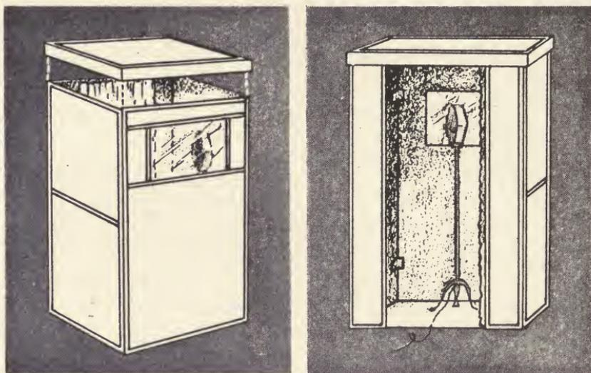
Figure 26. Booth constructed with acoustic screens.
