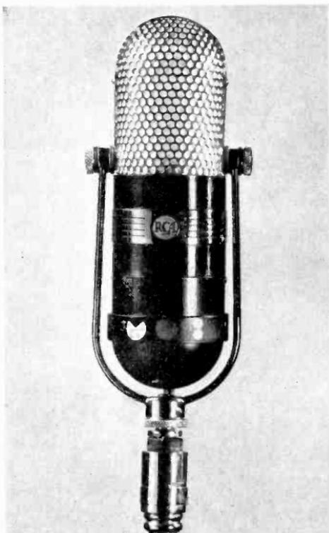
RCA all-purpose microphone Type 77-C. By turning the switch to line up the pickup pattern desired, it may be used for bi-directional, uni-directional, or non-directional purposes. (Courtesy of RCA.)
