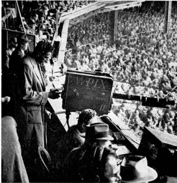
Photo shows a Zoomar lens in use at a baseball game. This lens is operated either manually or electrically and permits a rapid move from an extreme long shot to a close-up, remaining in focus throughout the entire move. (Photo courtesy of WPIX television.)
