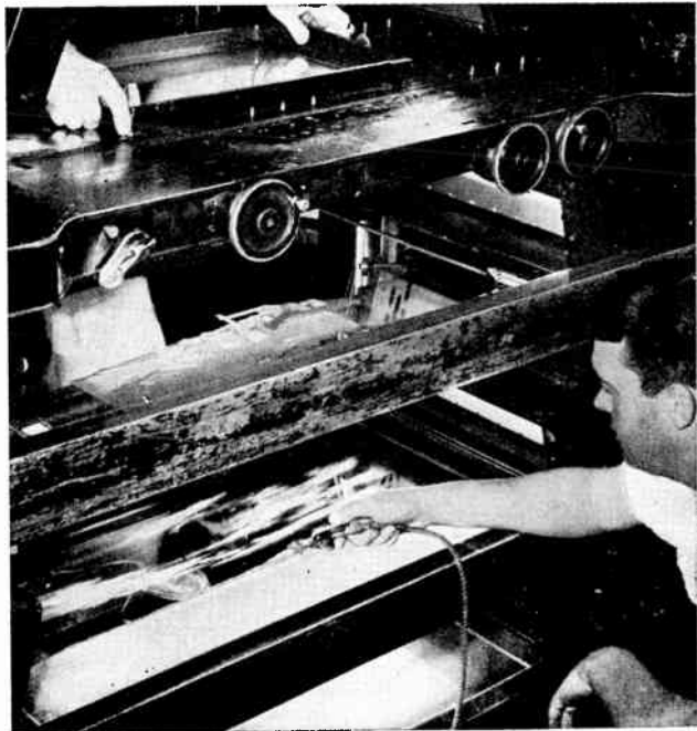
The Disney multiplane camera stand. Mr. Disney is shown discussing a scene with one of the operators. The camera and stand are virtually automatic in operation, being pre-set to cue sheets. This equipment makes possible the extraordinary three-dimensional effects in Disney films. Second picture is a close-up of part of the machine, showing the glass levels or backgrounds through which the camera photographs downward. A technician cleans a cel by use of compressed air. (Photos copyright Walt Disney Productions.)
