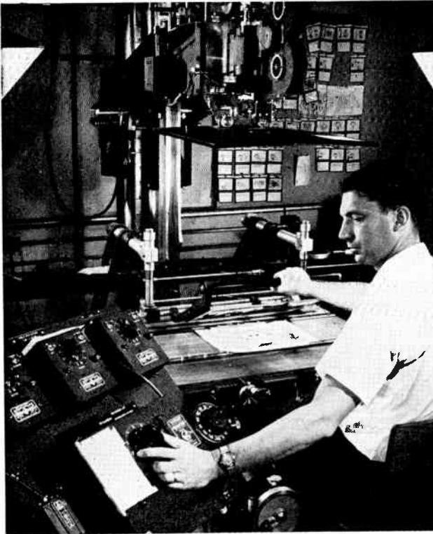
Another type of animation camera stand in use at Transfilm, Inc. This equipment weighs 3,000 pounds, costs more than $30,000. Operated electrically, it enables cameraman Norman Witlen to shoot special animation effects in a fraction of the time required by conventional methods. More important, its fine calibrations enable the production of flawless animation films. (Photo courtesy of Transfilm, Inc.)
