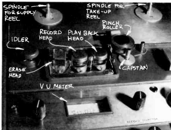
7-30 Head Assembly of the Reel-to-Reel Tape Recorder.
