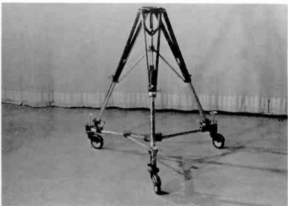
4-2 Tripod Dolly Collapsed and Assembled.
