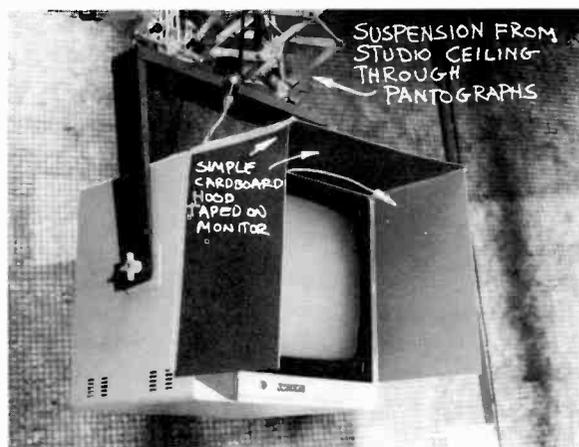
**8-3 Studio Monitor:** In case of excessive light spill in the studio, you can build a simple cardboard hood for the monitor that will shield the screen from the light and make the picture more visible.
