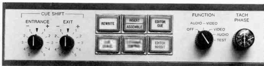
sound deterioration, however momentary, at the points of transition. The electronic editor permits the simultaneous editing of video and audio, or of either track (video or audio) separately, without affecting the other. (See 10.28 and 10.29.)
