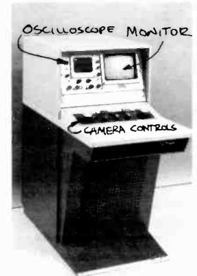
**2-4 Camera Chain:** The camera chain consists of (1) the camera head, which is what we ordinarily call the television camera; (2) the camera control unit, or the CCU; (3) the sync generator; and (4) the power supply. The color camera has an additional part, (5) the encoder.
