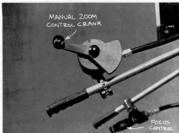
**3-25 Zoom Control:** With most zoom controls, you turn the handle clockwise to zoom in and counter-clockwise to zoom out. The faster you turn the handle, the faster the zoom will be.
