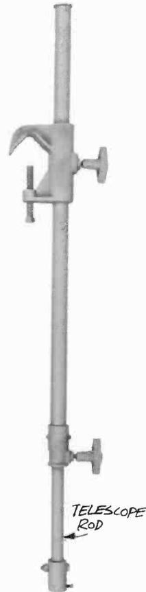
**5-38 Telescope Hanger:** The *telescope hanger* is similar to the sliding rod, except that the rod telescopes into itself when the hanger is pushed up. Thus the telescope hanger needs little clearance between grid and ceiling.
