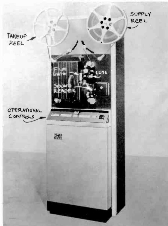
**9-29 RCA TP-66 Film Projector:** The professional television film projector adjusts the 24-frames-per-second 16mm sound speed to the 30-frames-per-second electronic scanning of television. It can be remotely started and stopped, backed up in reverse, and stopped for still-frame projection without burning up the film. The largest reels can accommodate almost two hours of continuous film programming.
