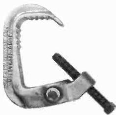
**5-34 C-Clamp:** With the C-clamp, you can securely attach even the heaviest lighting instrument to the mounting pipe. A bolt at the bottom of the C-clamp enables you to swivel the instrument into the desired position. For increased safety, secure each instrument directly to the grid by a small chain or cable.
