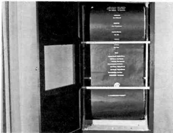
**12-29** The crawl is a strip of paper on which the long list of credits is lettered. As you rotate the drum in a direction away from the camera, the credit
