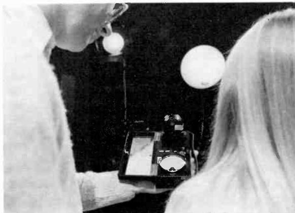
**a Incident Light Reading:** Light meter is pointed into the lights.
