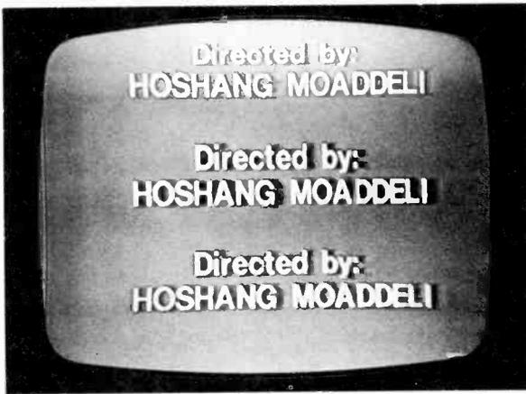
**12:30 Character Generator:** A character generator produces a variety of letters electronically. They can be stored and recalled at any time for a key or matte key. The lines can be moved right or left on the screen, rolled up or down, or crawled sideways.
