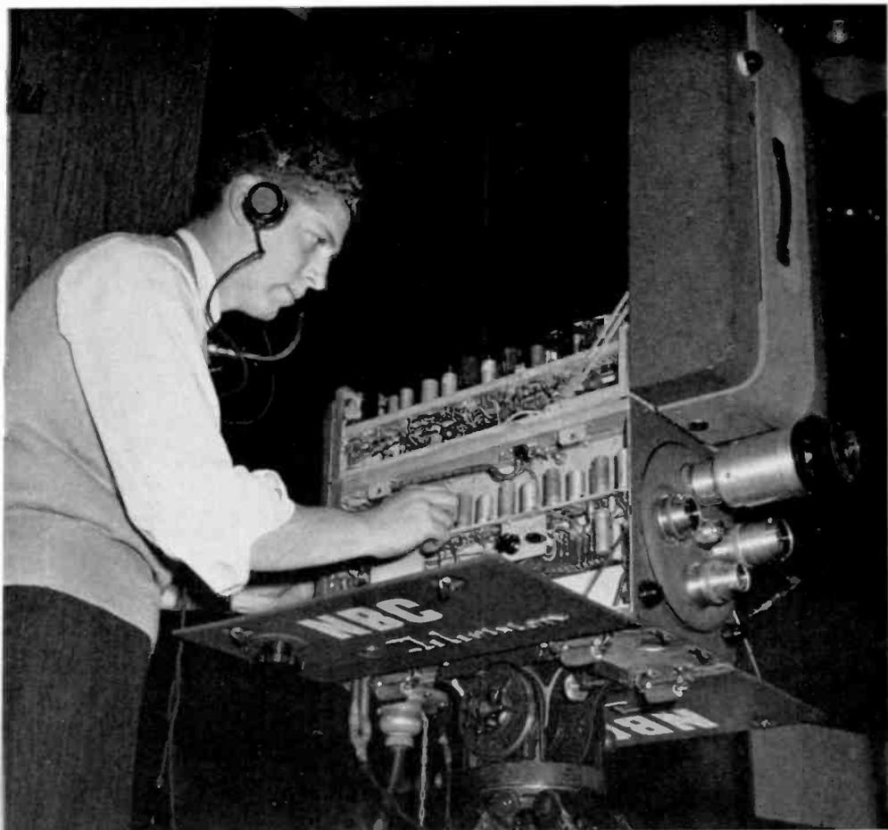
Here is a perfect view of the inside of a television camera. In appearance it differs little from that of a modern radio set. The radio set, however, functions under the impact of sound waves, while the TV camera reacts to light waves.
