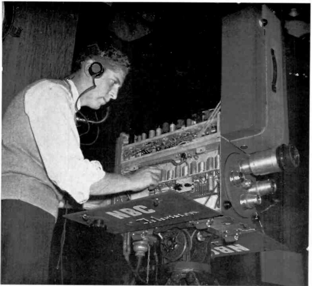
Here is a perfect view of the inside of a television camera. In appearance it differs little from that of a modern radio set. The radio set, however, functions under the impact of sound waves, while the TV camera reacts to light waves.
