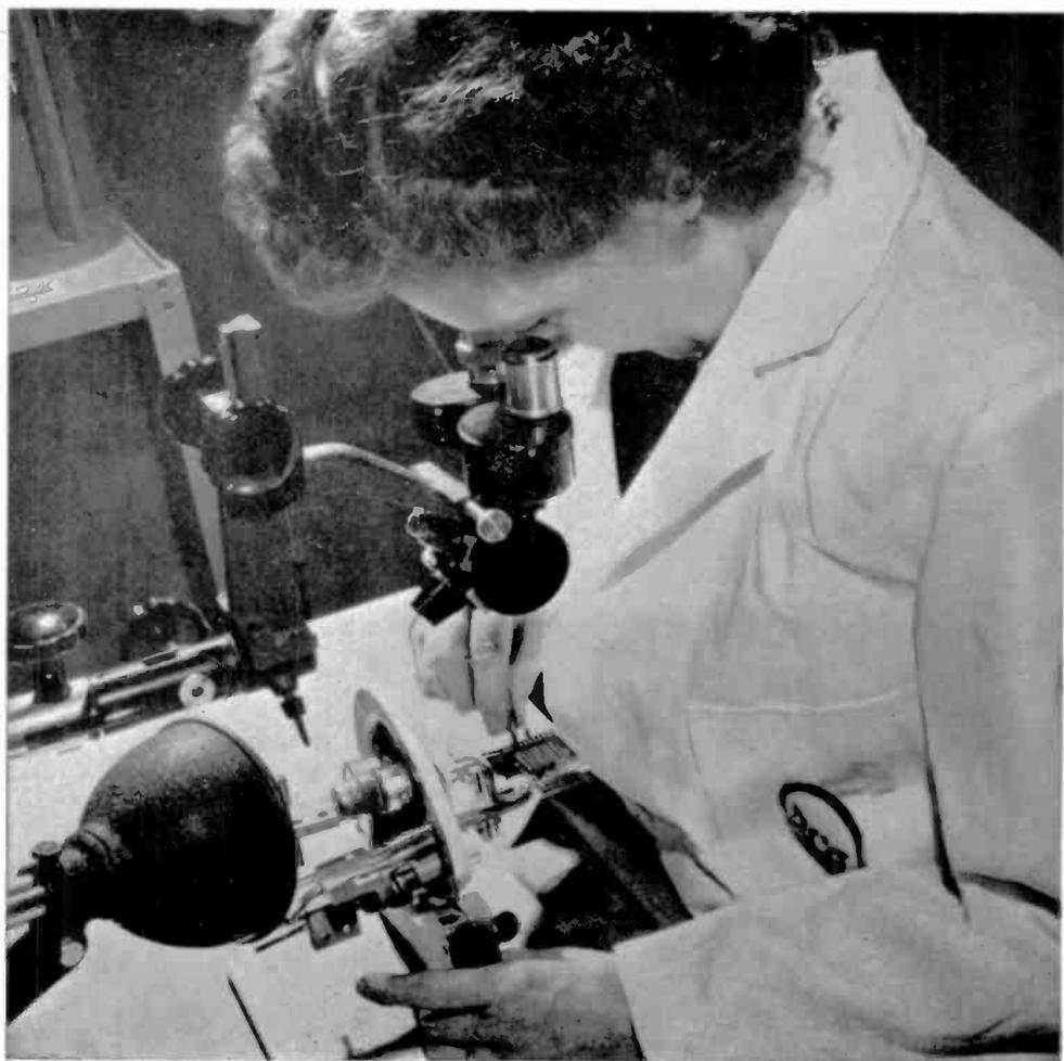
The human eye, no matter how good, is not sharp enough to fit certain parts that go into the assembly of, say, an image orthicon. Here the microscope is a must.
