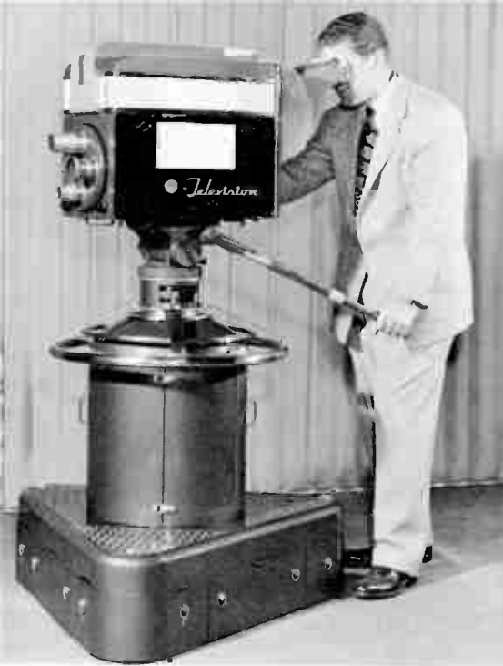
Figure 17. Camera Pedestal, RCA Image Orthicon Camera Mounted on Houston Fearless Pedestal, PD-3.
