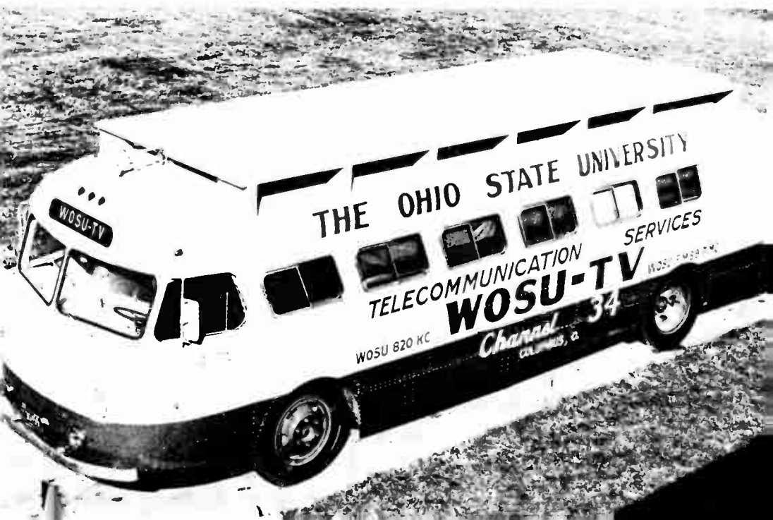
Figure 5. TV Mobile Unit, WOSU-TV, Columbus (Ohio). The platform on top of this Ohio State University bus is for mounting of cameras and microwave equipment.
