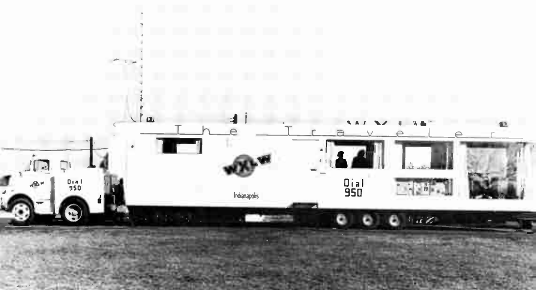
Figure 4. Radio Mobile Unit, WXLW, Indianapolis (Indiana). Completely self-contained with studio, relay unit, and living facilities.
