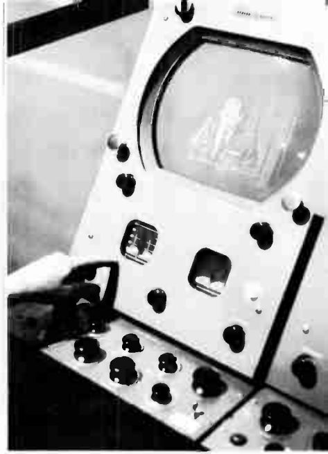
Figure 29. Monitor Pedestal and Wave Form, General Electric. Director points to scope showing wave form for horizontal pattern. Vertical pattern at right.
