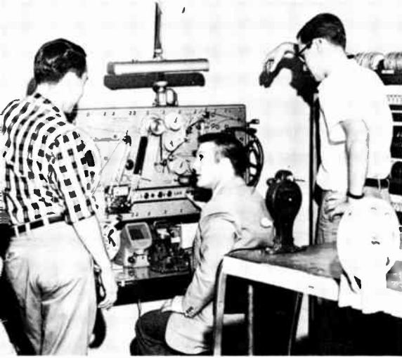
Figure 55. Film Editor, Inspect-O-Film, Harwald. Apparatus measures footage, counts splices, and detects flaws.
