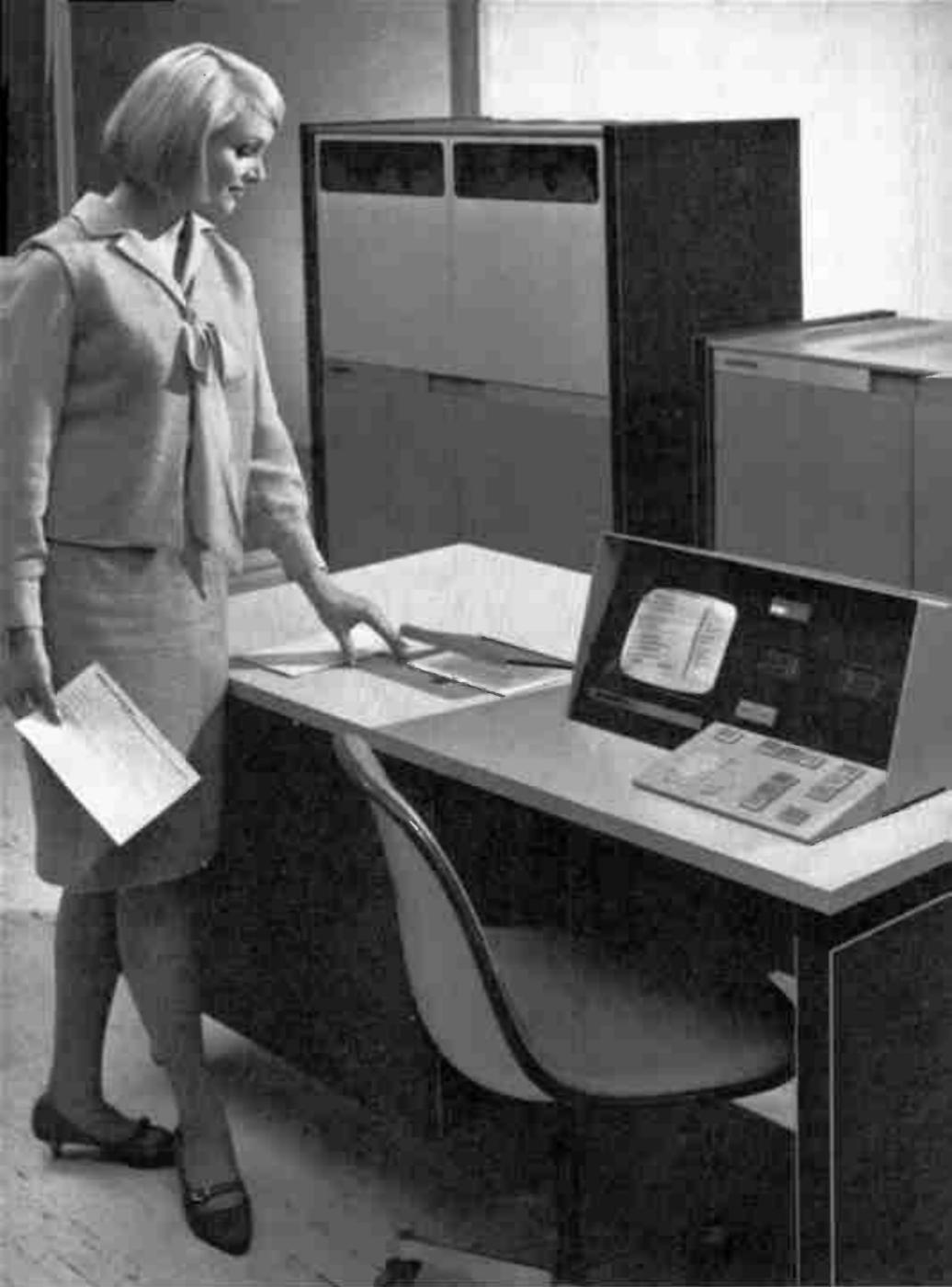
*Ampex's Videofile handles document filing and retrieval, replacing file folders with television recordings that may be updated electronically.*
