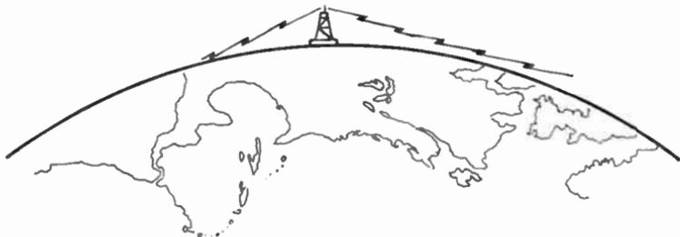
*A signal from a TV tower can travel only 20 or 30 miles before it strikes the earth or is lost in space.*
