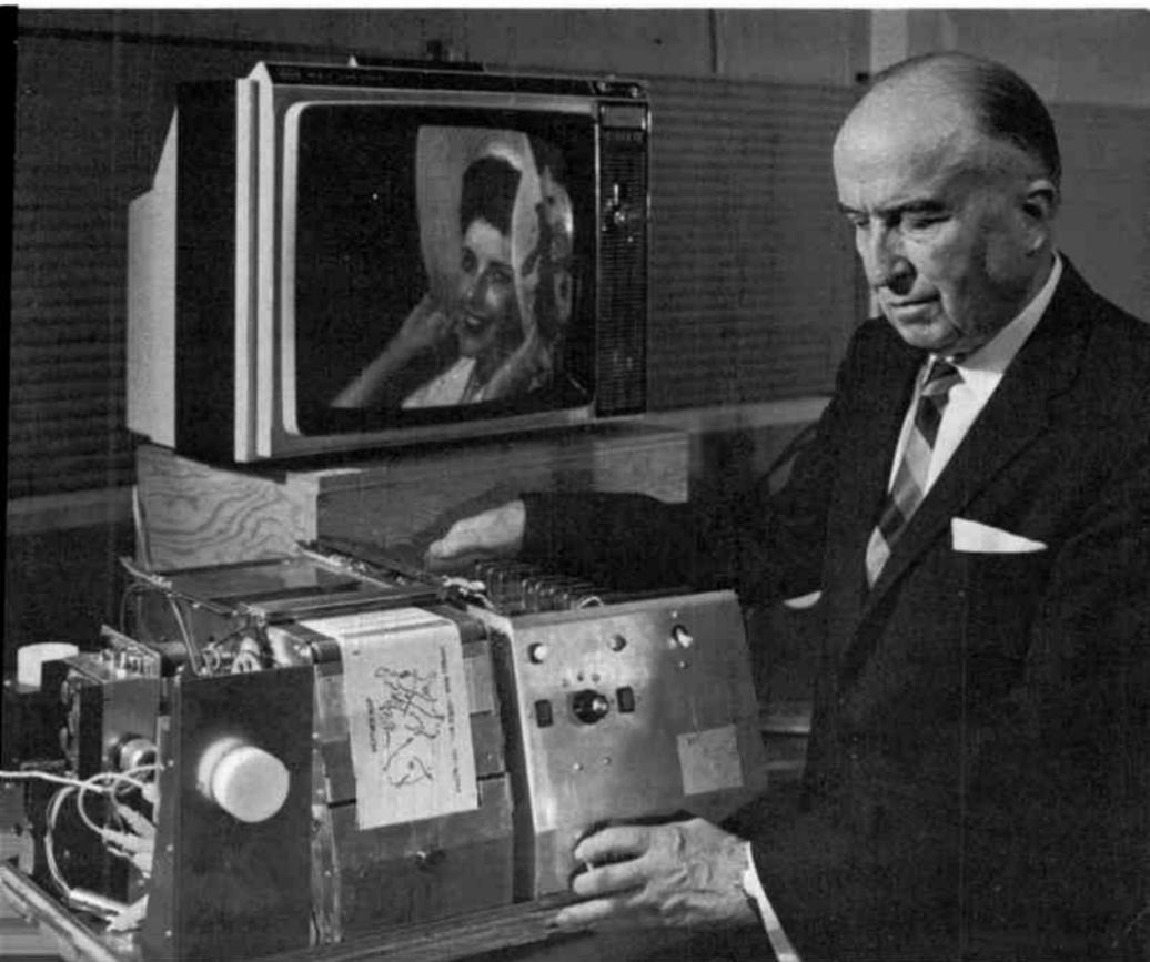
*RCA's facsimile television system is used to transmit printed material.*
