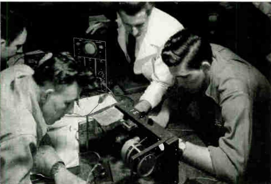
The picture above shows students building and checking Photo-electric Cell phase shifter circuits. Coyne training is practical through and through. Every job that you do is designed to give you practical knowledge and experience on an important phase of Electrical work out in the field. That is why you make rapid progress at Coyne.
