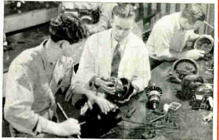
Here you see students getting training and practice in proper procedure in eliminating bearing trouble. The student with the Instructor is using a Line Reamer to align bearings on a Fractional Horsepower Motor. The service man in the field will find this training a mighty valuable feature of this Department.
