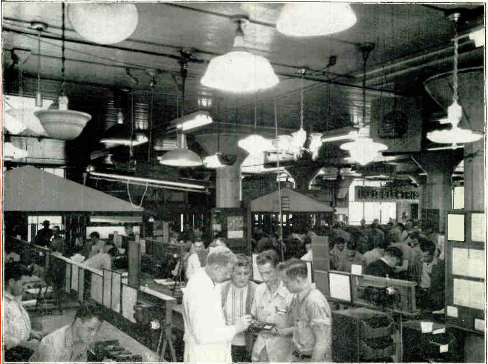
Here you see a picture of the illumination section, and some of the different kinds of light fixtures you work with. The instructor is showing students how to test the amount of light from each fixture with a "foot-candle meter." You are taught which type of fixture is best for home, office or factory use. Note the fluorescent lighting units mounted on the ceiling which furnish general lighting. Our entire building is equipped with this modern type of lighting units.
