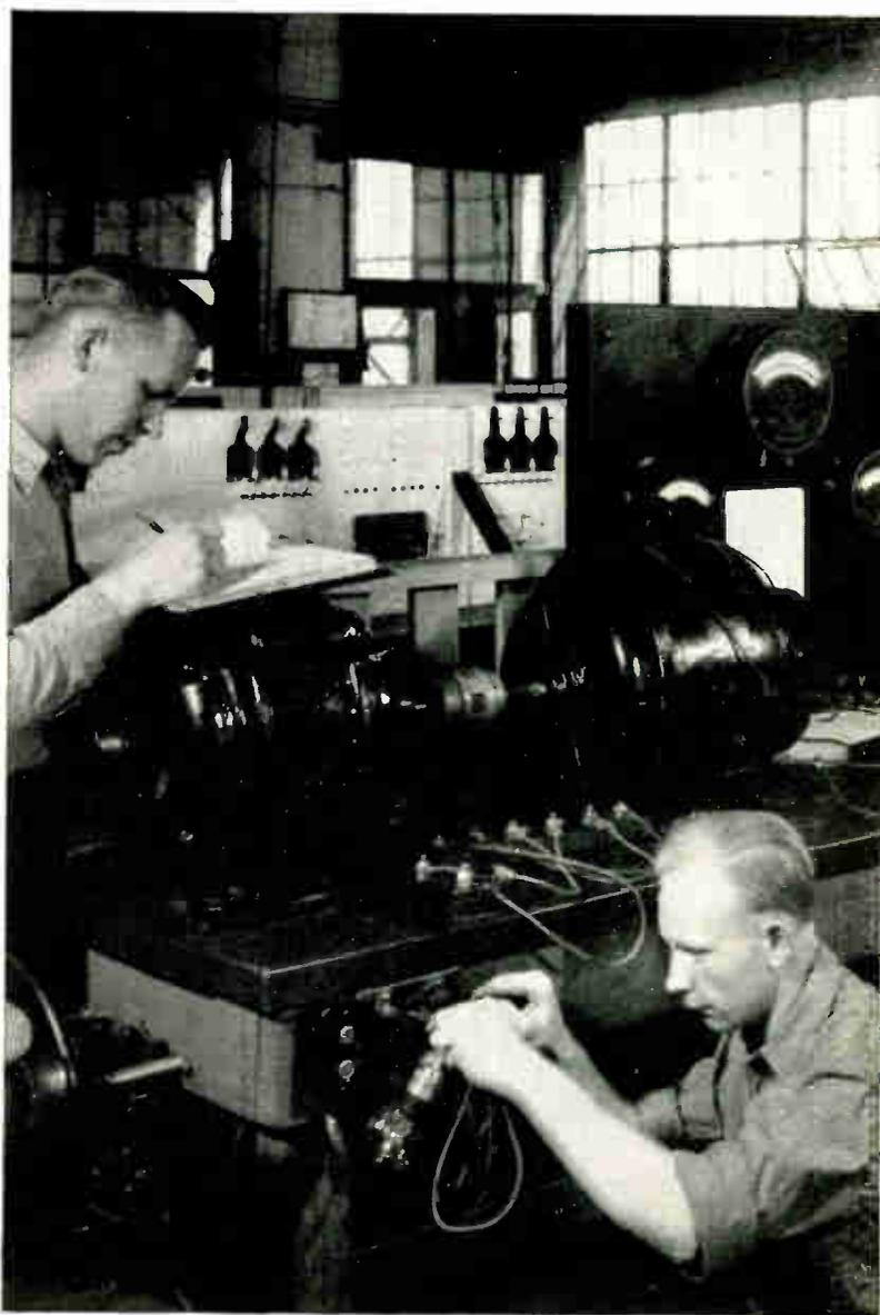
These students are testing the horsepower, efficiency, and power factor of induction motors. This is very important training for the practical maintenance man.
