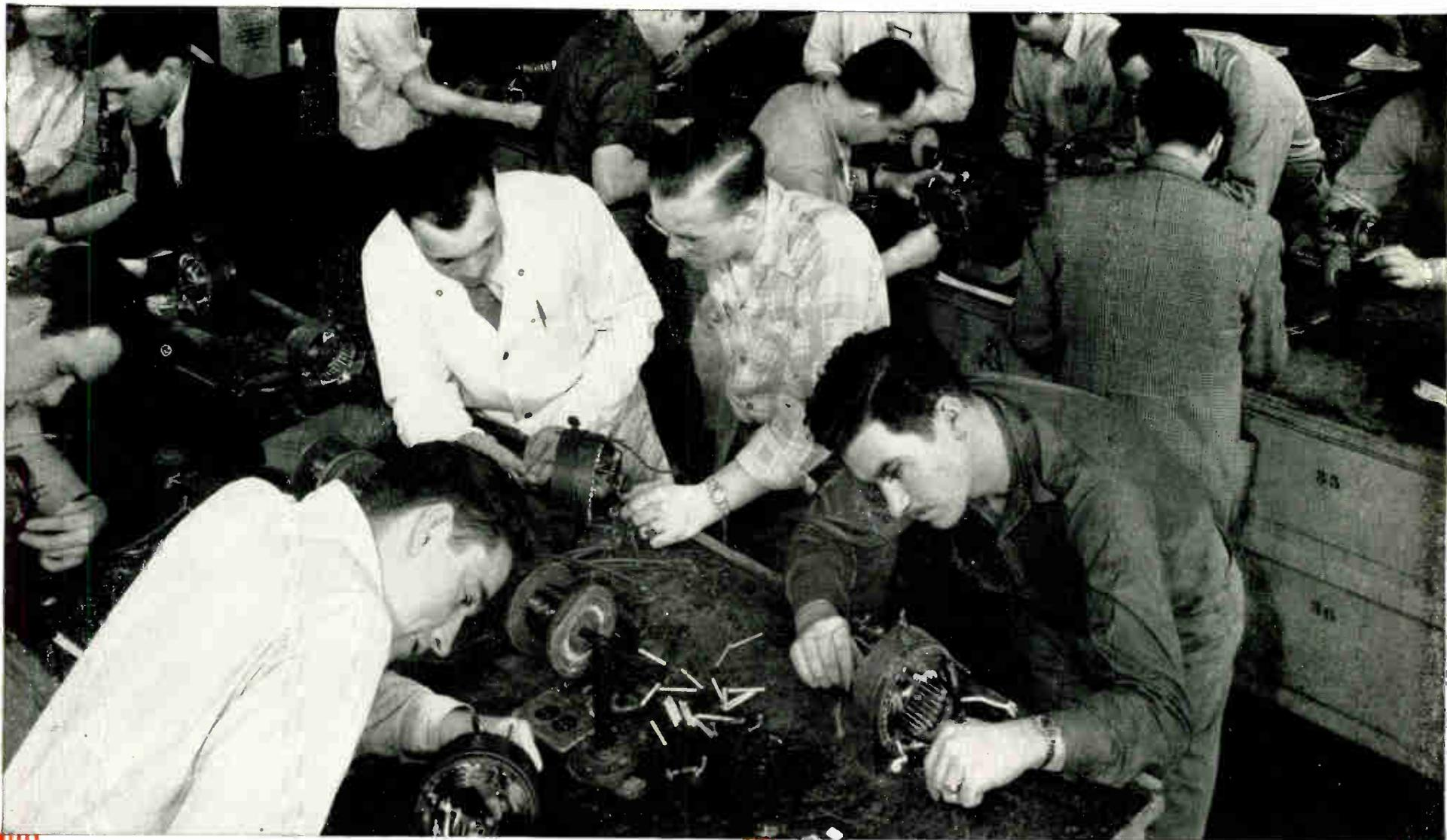
Here you see a view of the Stator Winding section. Notice that real wire is used in winding these stators. Actual winding and testing of Alternating Current motors gives you the practical training you need in this work. Motor repair work of this kind is often necessary in Electrical maintenance jobs in Power Plants, factories, stores, office buildings and, in fact, wherever Alternating Current motors are used.
