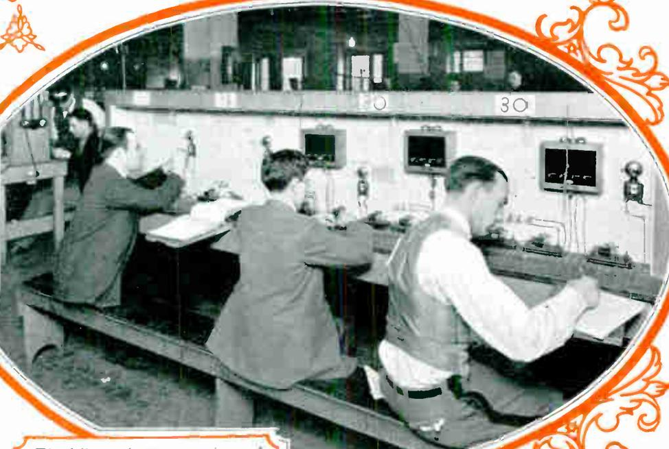
The fellows above are getting real experience on circuit tracing and testing on advanced alarm and signal systems. And they keep a copy of the diagram for each job and their notes of the things they test and prove out in writing it.
