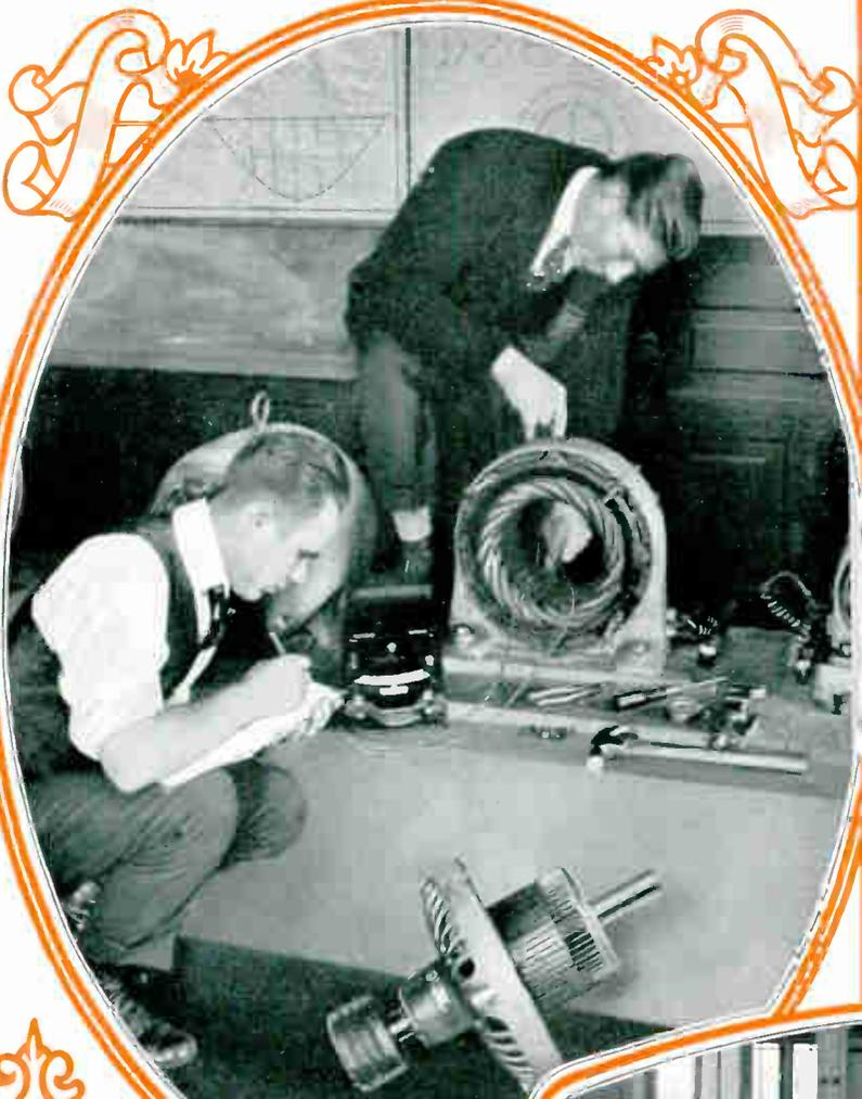
Real practical work overhauling and repairing on A. C. induction motor. This is the kind of work that makes you sure of yourself when you get out on the job, for when you thoroughly understand all the working parts of a machine you have confidence in yourself
