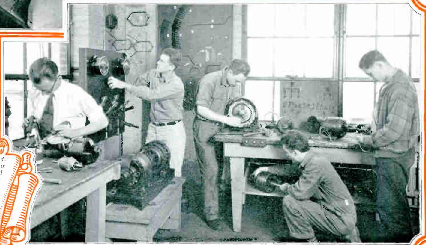
These fellows are testing finished windings of armatures and stators. This is the way they find their mistakes and learn to make their windings correct, so they can become perfect in their work. Testing armatures and stators and locating faults in the windings, is very valuable to any maintenance man whether he follows armature winding or not.
