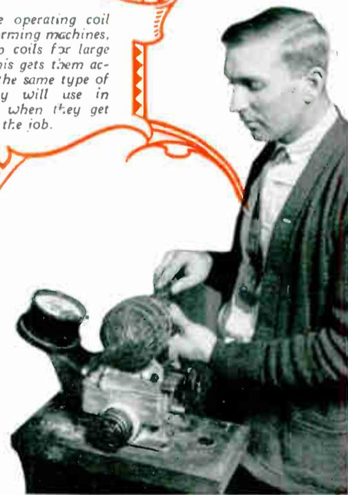
This man is testing an armature on the growler, a machine for quickly locating trouble and faults in windings. This kind of instruction enables my graduates to get right at the cause of armature troubles without waste of time.
