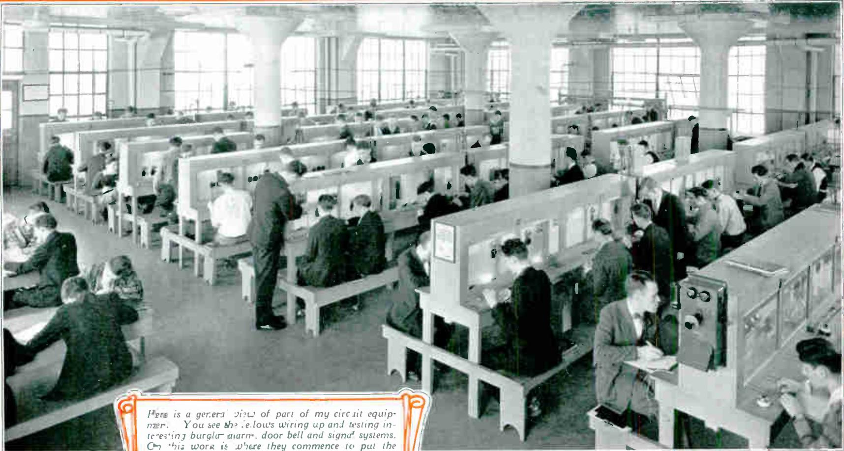
Here is a general view of part of my circuit equipment. You see the fellows wiring up and testing interesting burglar alarm, door bell and signal systems. On this work is where they commence to put the current to work, and apply many of the things learned in their elementary instruction.
