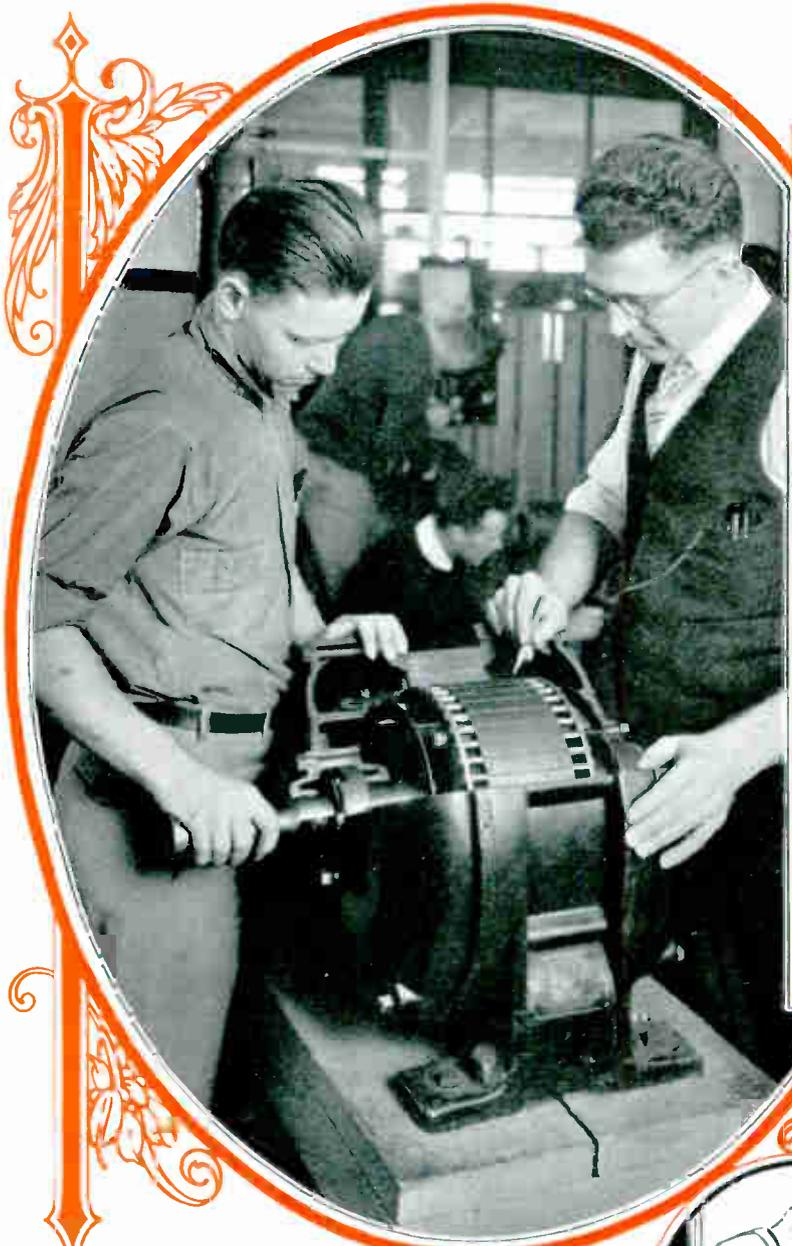
Here an instructor is explaining important principles of an induction motor on a machine specially cut away, so you can observe these points both while it is idle and when it is running. This is an example of how some of our specially prepared equipment will save your time, and quickly and easily make these things clear to you.
