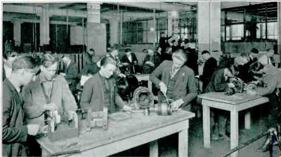
And these fellows are doing general trouble shooting and repair on A. C. motors, and building a complete test transformer for high voltage testing of insulation.
