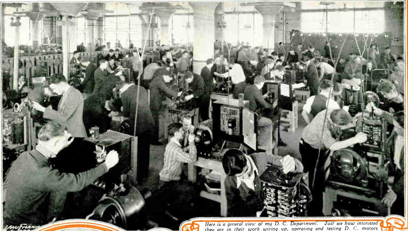
Here is a general view of my D. C. Department. Just see how interested they are in their work wiring up, operating and testing D. C. motors and controllers of all common types. Notice the wires coming down from overhead, to supply current for running tests on every machine, no dead machinery or toy models, all actual running machinery.
