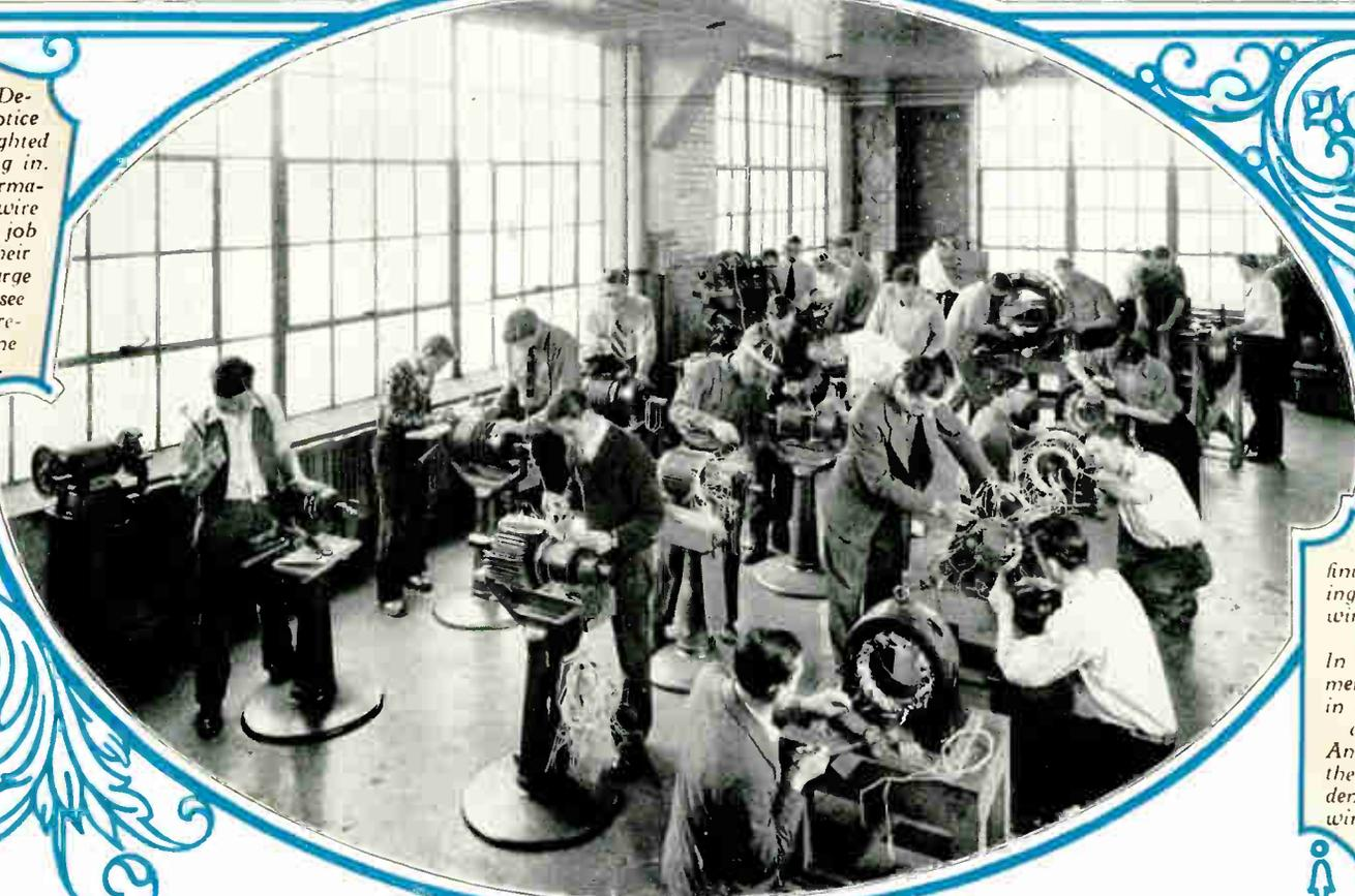
These fellows have finished their first small winding and here you can see them winding and testing large armatures and stators. In the background you will see men trueing up a commutator in a lathe and others winding a 200 h. p. A. C. stator. And in the foreground one of the instructors showing a student how to test his finished winding, before connecting up the leads.
