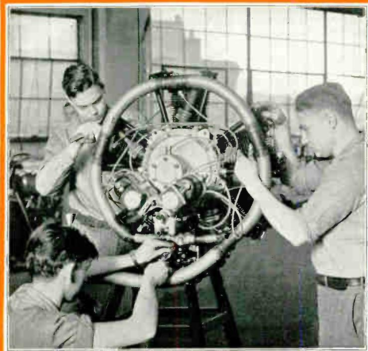
Here is where you learn the use of the twin magnetos and spark plugs for double ignition on airplane engines. And these men are also learning carburetor and valve adjustment, which of course, are necessary for the proper "tuning" of the motor. There is a great and growing demand for expert ground men to work at the hangars and landing fields, and keep these motors in "tune".
