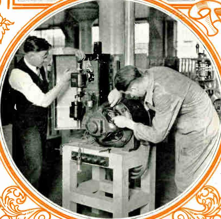
These fellows are learning the operation of an automatic controller and compound motor, and learning to make the same tests and repairs they will have to do out on the job.
