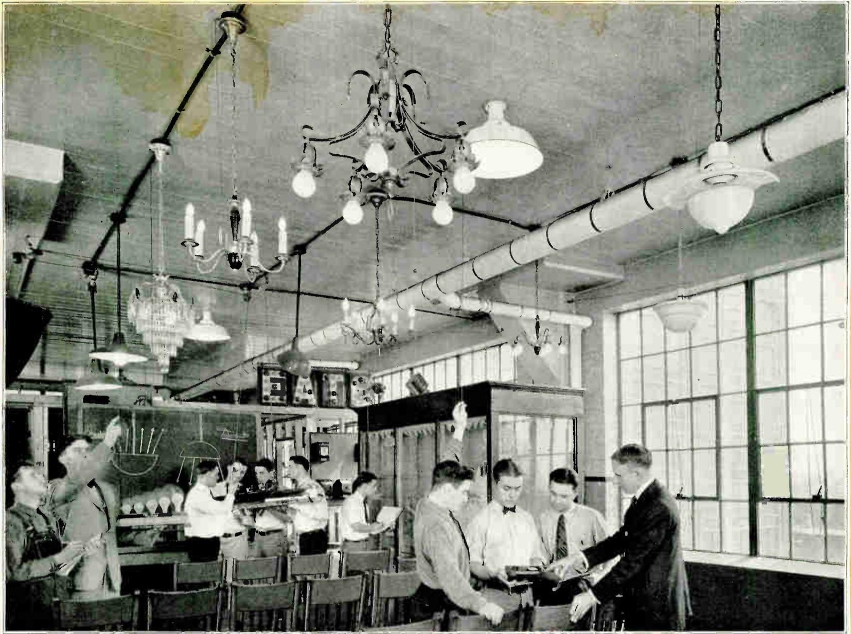
Here you see part of the illumination section, and some of the different kinds of light fixtures you work with. The instructor in the right foreground is showing students how to test the amount of light from each fixture with a "foot candle meter." You learn which type of fixture is best for home, office, or factory use.
