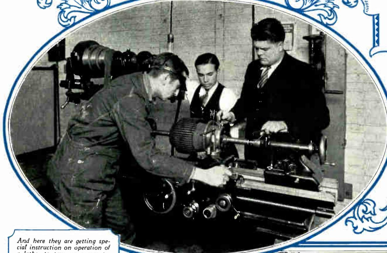
And here they are getting special instruction on operation of a lathe, to true up commutators on armatures. The instructor shows them how to grind and set the cutting tool, and how to make a nice smooth cut on the copper.
