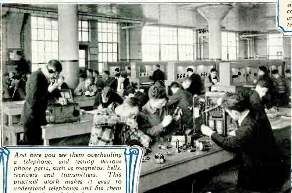
And here you see them overhauling a telephone, and testing various phone parts, such as magnetos, bells, receivers and transmitters. This practical work makes it easy to understand telephones and fits them for the real jobs later on.
