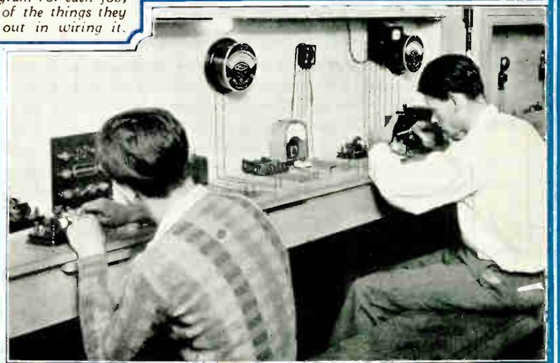
Wiring and testing special equipment for proving Ohms law and effects of electricity with meters and instruments. These students you see are experimenting with spark coils, neon tubes, transformers and carbon arcs.
