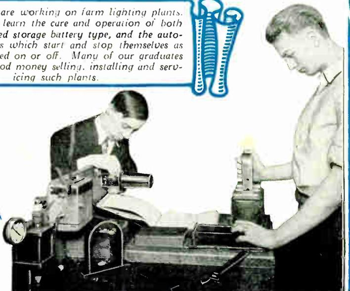
These men are testing motor driven auto horns, and recharging field magnets of magnetos. You will also note the glass spark plug test chamber at the left of this bench.
