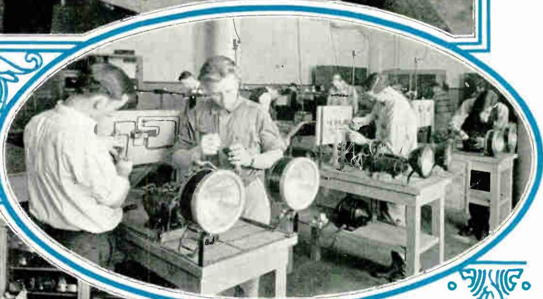
Here you see them wiring and testing complete electrical systems of different types of cars, with all the parts and wiring laid out on a bench for convenient and practical work on trouble shooting, and checking of firing orders and timing. This work enables them to quickly locate by systematic tests, the troubles such as "open circuits", "grounds", shorts, etc., that cause many car troubles.
