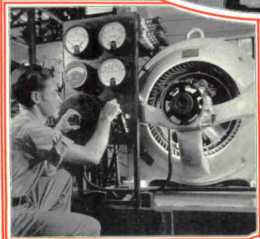
A student preparing to test a large synchronous motor which is used for correcting power factor and saving money on power bills. Every trained electrical maintenance man should be familiar with this type of work.
