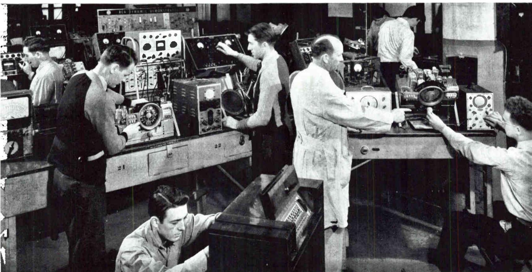
This photo shows students working with modern radio receivers and test instruments to locate faults and troubles. Note the Cathode Ray Oscilloscopes and other up-to-date test equipment which the students are learning to use with the help of the instructor.
