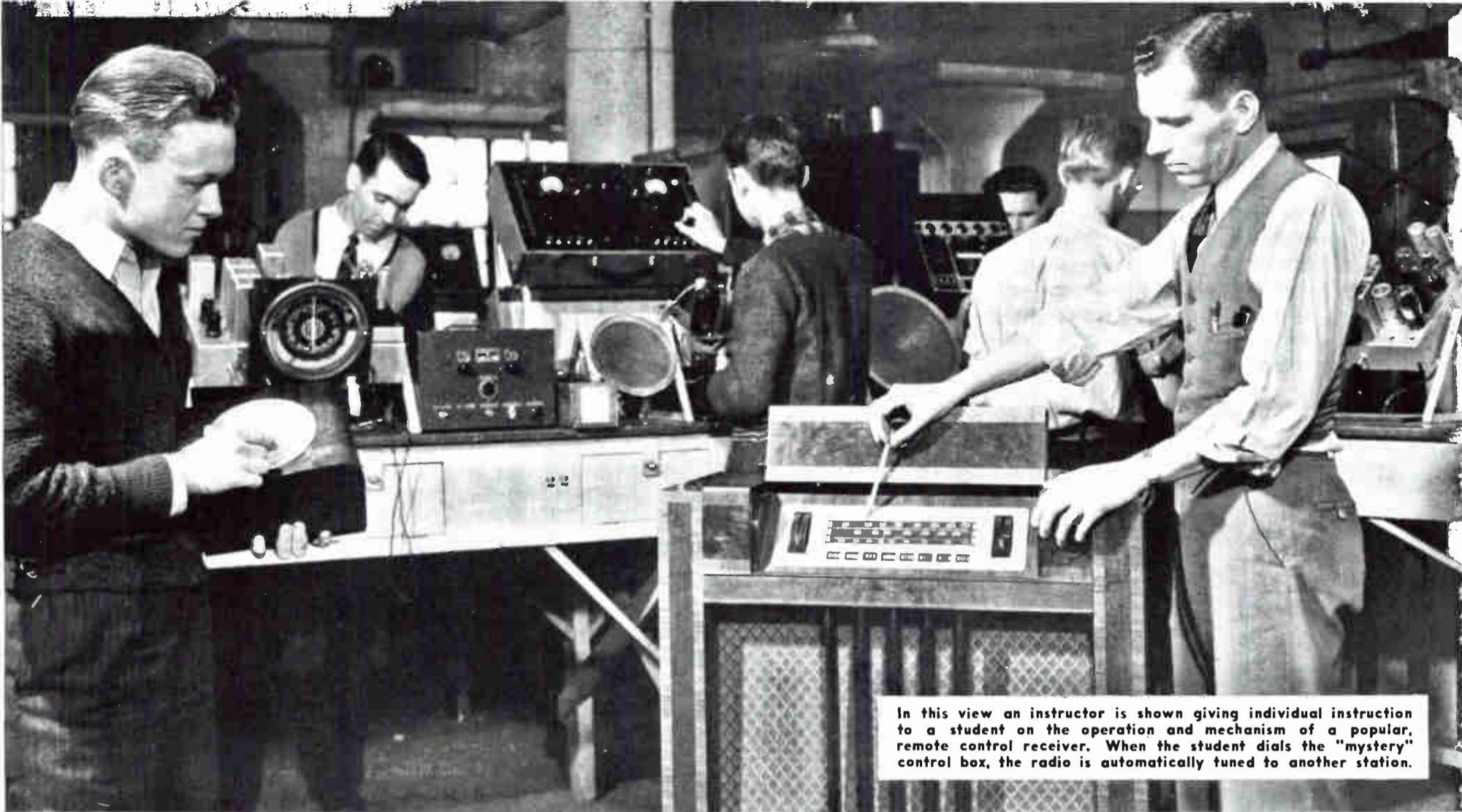
In this view an instructor is shown giving individual instruction to a student on the operation and mechanism of a popular, remote control receiver. When the student dials the "mystery" control box, the radio is automatically tuned to another station.
