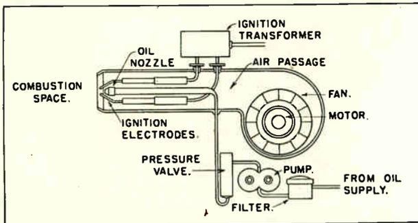
Fig. 9. Principal parts of gun type oil burner.
