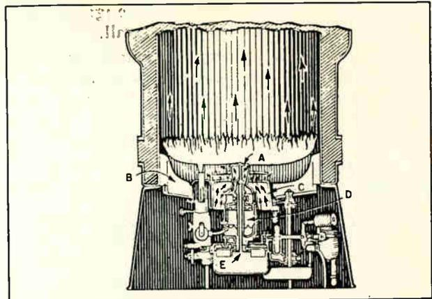
Fig. 10. Rotary centrifugal atomizing oil burner with vertical shaft: A. Atomizer. B. Chamber lined with refractory material. C. Air space. D. Electric motor. E. Hollow shaft.
