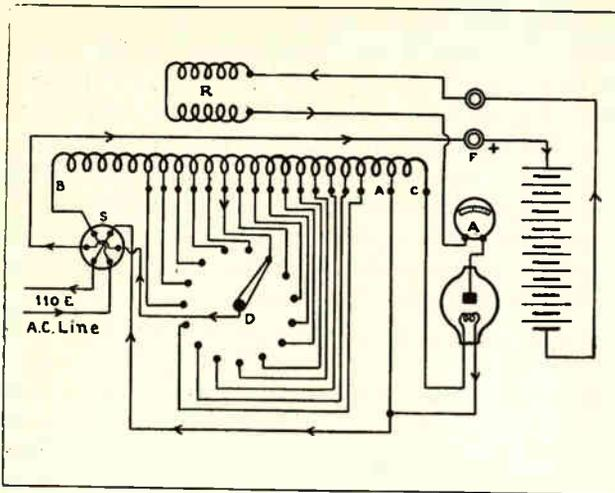
Fig. 230. Wiring diagram of a Tungar type bulb rectifier showing the taps on the auto transformer winding for varying the charging voltage.
