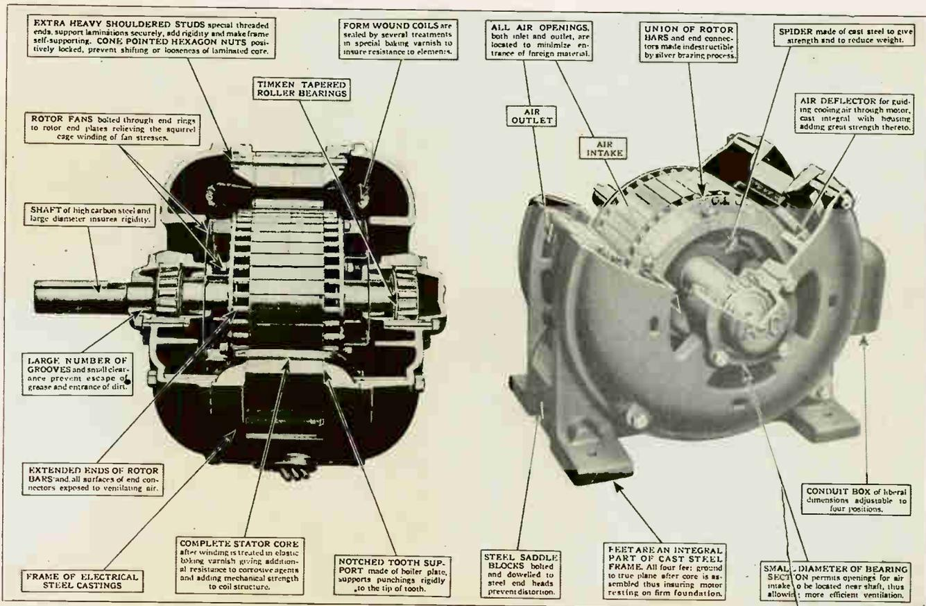
Fig. 176. The above photo shows two cut-away views of a polyphase squirrel-cage induction motor. The important parts of the motor are clearly shown in these two views and you should carefully note the descriptions given for each part. A careful study of this figure will show a number of very important features of induction motor construction. (Photo courtesy Allis-Chalmers Mfg. Co.)
