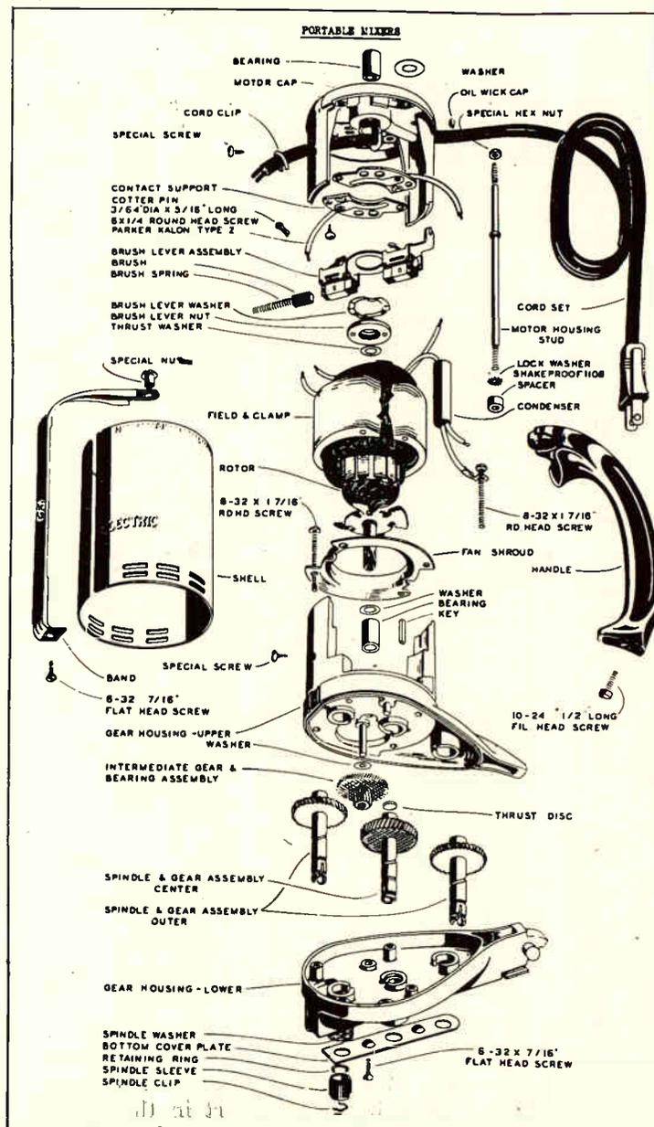
Fig. 1. The Parts of an Electric Food Mixer (General Electric).
