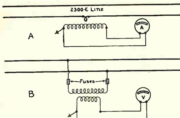
Fig. 144. A shows the connections for a current transformer which is used to operate A. C. ammeters, wattmeters, and current relays. B. Connections for potential transformer used to operate voltmeters, potential elements of wattmeters, potential relays, etc.
