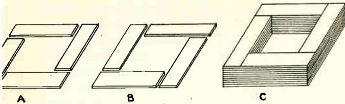
Fig. 153-B. A core type transformer core may be constructed with alternate layers of laminations as shown above.
