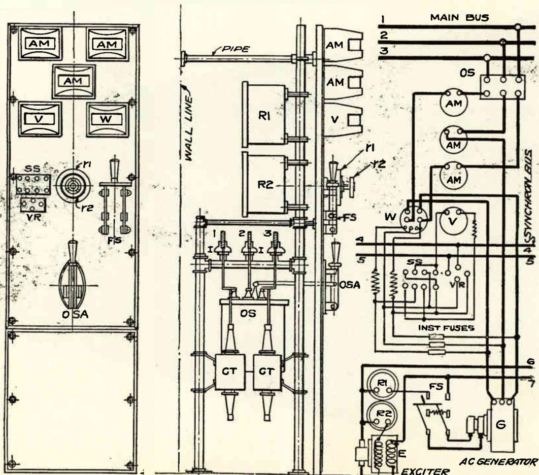
Fig. 416. These diagrams from left to right show respectively a front view, side view, and the wiring of a single panel in an A. C. plant.
