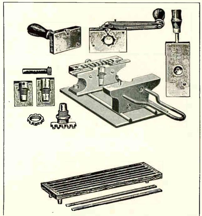
Fig. 45. Above is shown a combination mold used for casting threaded type posts and nuts, while below is a simple mold used for casting plain lead bars to be used in filling lugs when burning on connections.
