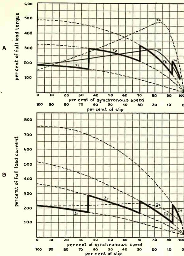
Fig. 185. A shows the torque curves of a slip-ring induction motor as the resistance is cut out of the rotor circuit and the motor comes up to speed. B shows the current curves of the same motor and corresponding to the various steps of the torque curves. Study these curves very carefully with the accompanying explanation.
