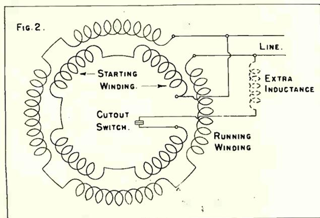
Fig. 2. Connections in a Split-phase Motor.
