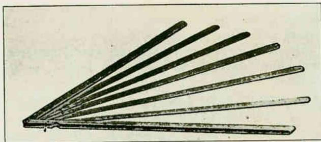
Fig. 459. Common motor air gap gauge, for measuring clearance between the armature or rotor and the field poles or stator. Note the several different "feelers" or blades which are of different thicknesses.
