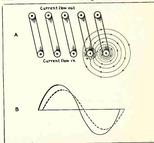
Fig. 16. The above diagram illustrates the manner in which the counter-voltage of self-induction is built up in an inductance coil.
