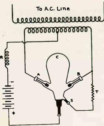
Fig. 238. Circuit diagram of a bulb type mercury arc rectifier used for battery charging purposes. Trace this circuit carefully with the accompanying explanation.
