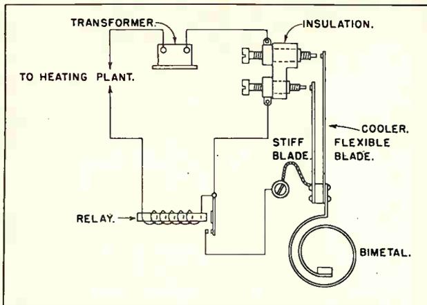
Fig. 5. Holding relay used with double-blade thermostat.
