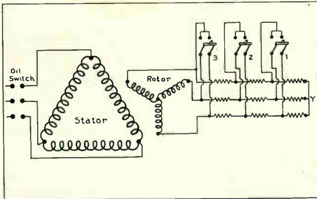
Fig. 184. Connection diagram of slip-ring induction motor with knife switches used to cut out the starting or speed control resistance step by step.
