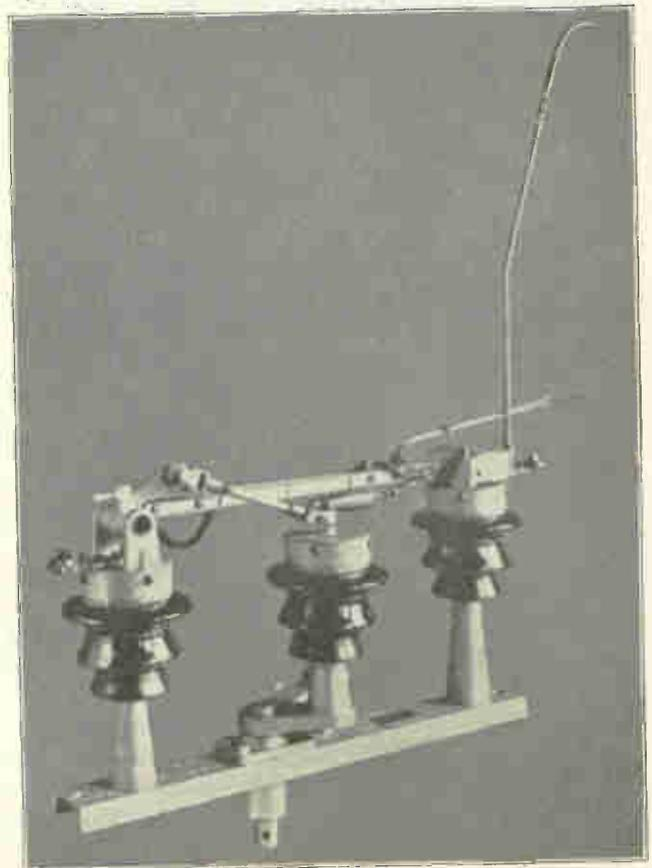
Fig. 430. High-voltage air break switch for pole top mounting or use in substation structures. Note the arcing horns used to prevent pitting and damage to the switch contacts. (Courtesy of Hi-Voltage Equipment Company.)
