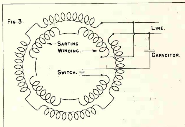
Fig. 3. Connections in a Capacitor-start Motor.
