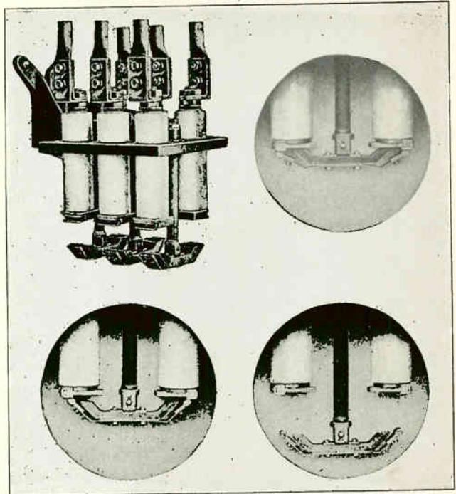
Fig. 424. At the upper left is shown the mechanism of a different type oil switch, and in the three other views are shown the steps or movement of the contacts during the opening of a switch of this type.
