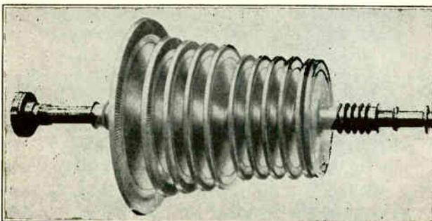
Fig. 313. Complete rotor of a modern steam turbine, showing several sets of moving blades through which the steam passes in succession. (Courtesy of Elliott Company.)
