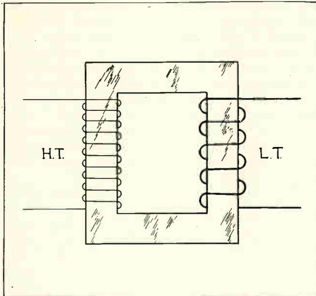
Fig. 99. This sketch shows the core and windings of a simple transformer. The winding on the left with the greater number of turns is the high tension winding, and the one on the right the low tension winding.
