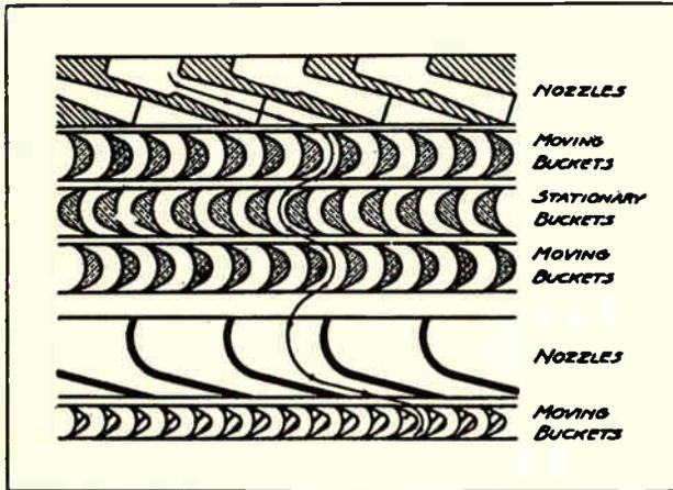
Fig. 312. This sketch illustrates the operating principles of a steam turbine. Note the nozzles and stationary and moving blades or buckets. (Courtesy of Elliott Company.)
