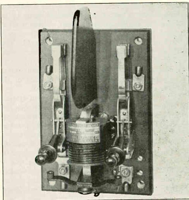
Fig. 420. Small air circuit-breaker for use on circuits of 600-volts and loads up to 400 amperes. Note the flash barrier placed between the two poles of the breaker. (Courtesy of G. E. Company.)
