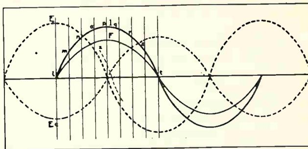
Fig. 19. Curves for a single-phase circuit in which the current and voltage are approximately 90° out of phase with each other, due to inductance in the circuit.
