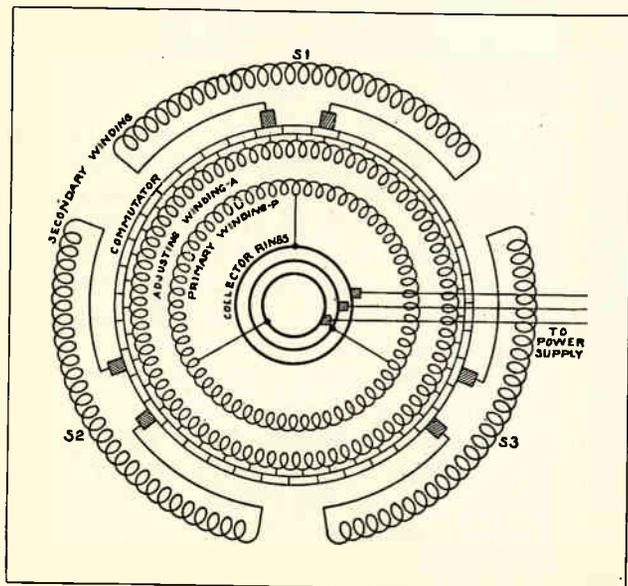
Fig. 202. This diagram shows the connections of the armature and stator windings of a BTA variable speed A. C. motor. Examine the diagram carefully while reading the accompanying explanation.
