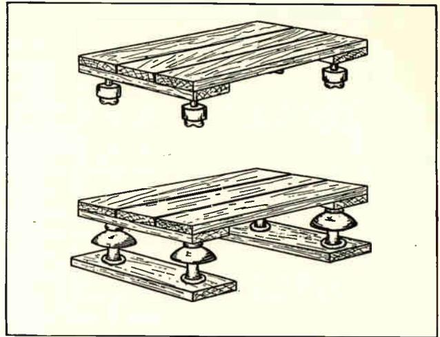
Fig. 449. The above sketch shows two types of insulated stools or platforms for safety in working around live wires. These are very simple and inexpensive to make.
