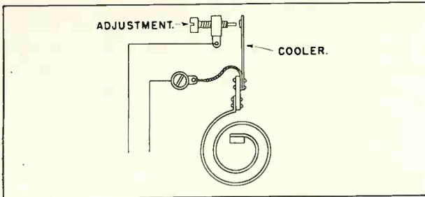
Fig. 3. Insulated spiral bimetallic element.
