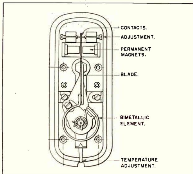
Fig. 1. The working parts of a room thermostat.
