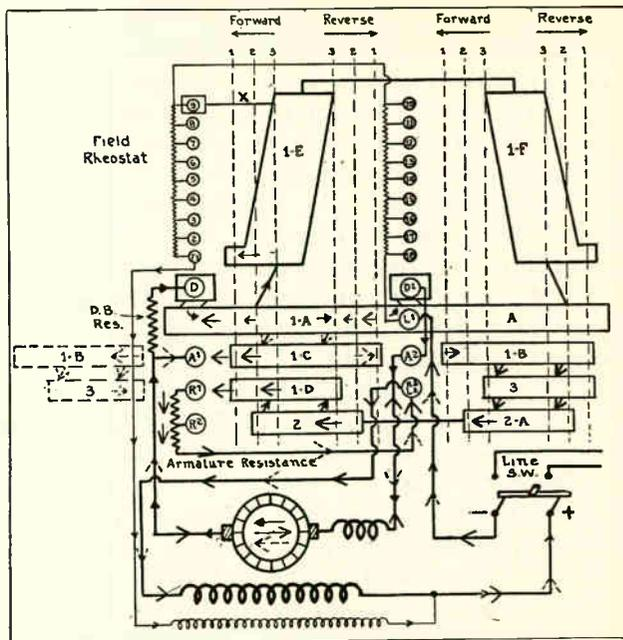
Fig. 140. This diagram shows the wiring for a drum controller used for starting, reversing, and varying the speed of a compound motor.
