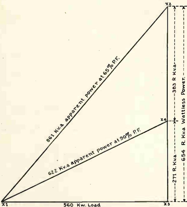
Fig. 221. This diagram also shows the reduction obtained in the apparent power and wattless power by improving the power factor of a system. By carefully measuring the top section of the vertical line in the diagram we can find the size of the condenser required to correct the power factor.
