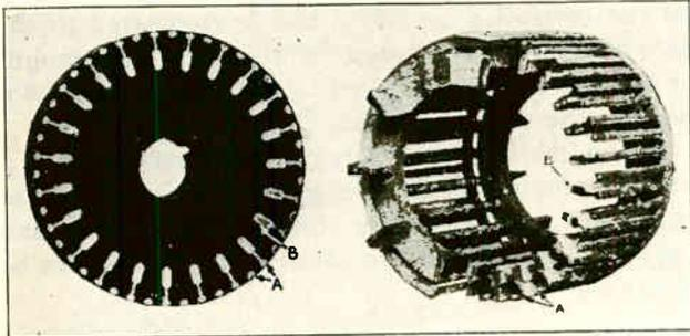
Fig. 199. This figure shows two views of a double squirrel-cage rotor. On the left is a sectional view and on the right the core iron has been eaten out by acid, clearly showing the construction and shape of the double squirrel-cage. (Photo courtesy General Electric Co.)
