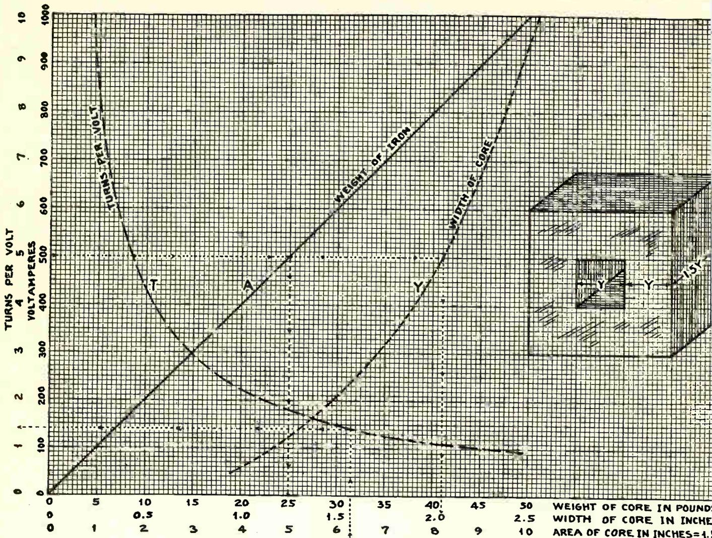
Fig. 153-A. Transformer design chart.
