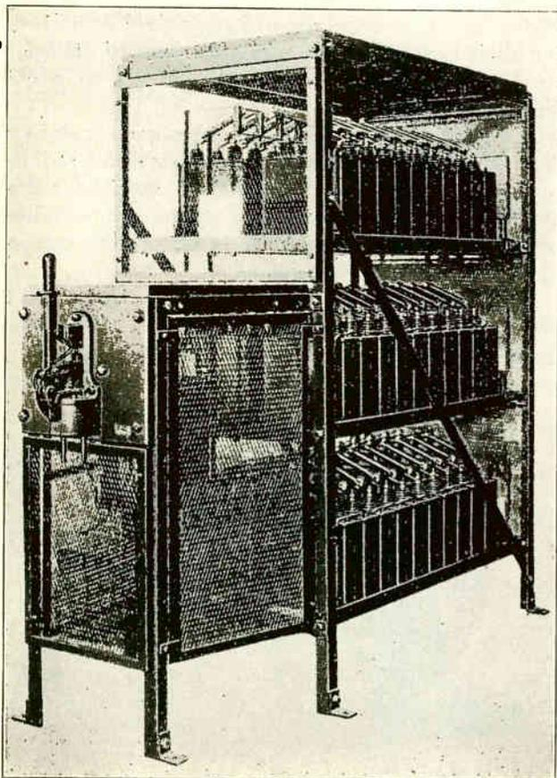
Fig. 213. 300-kv-a., three-phase, 2500-volt, capacitor or static condenser, used for improving power factor. (Courtesy General Electric Co.)
