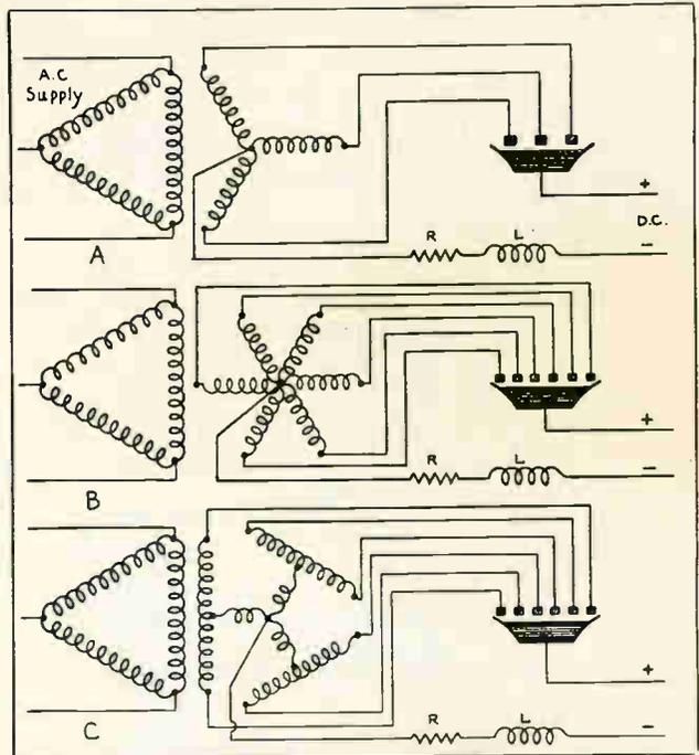
Fig. 245. The above diagrams show three different types of transformer connections which are commonly used with three-phase and six-phase mercury arc rectifiers.
