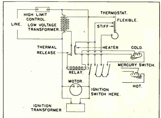
Fig. 14. Control system with safety features.
