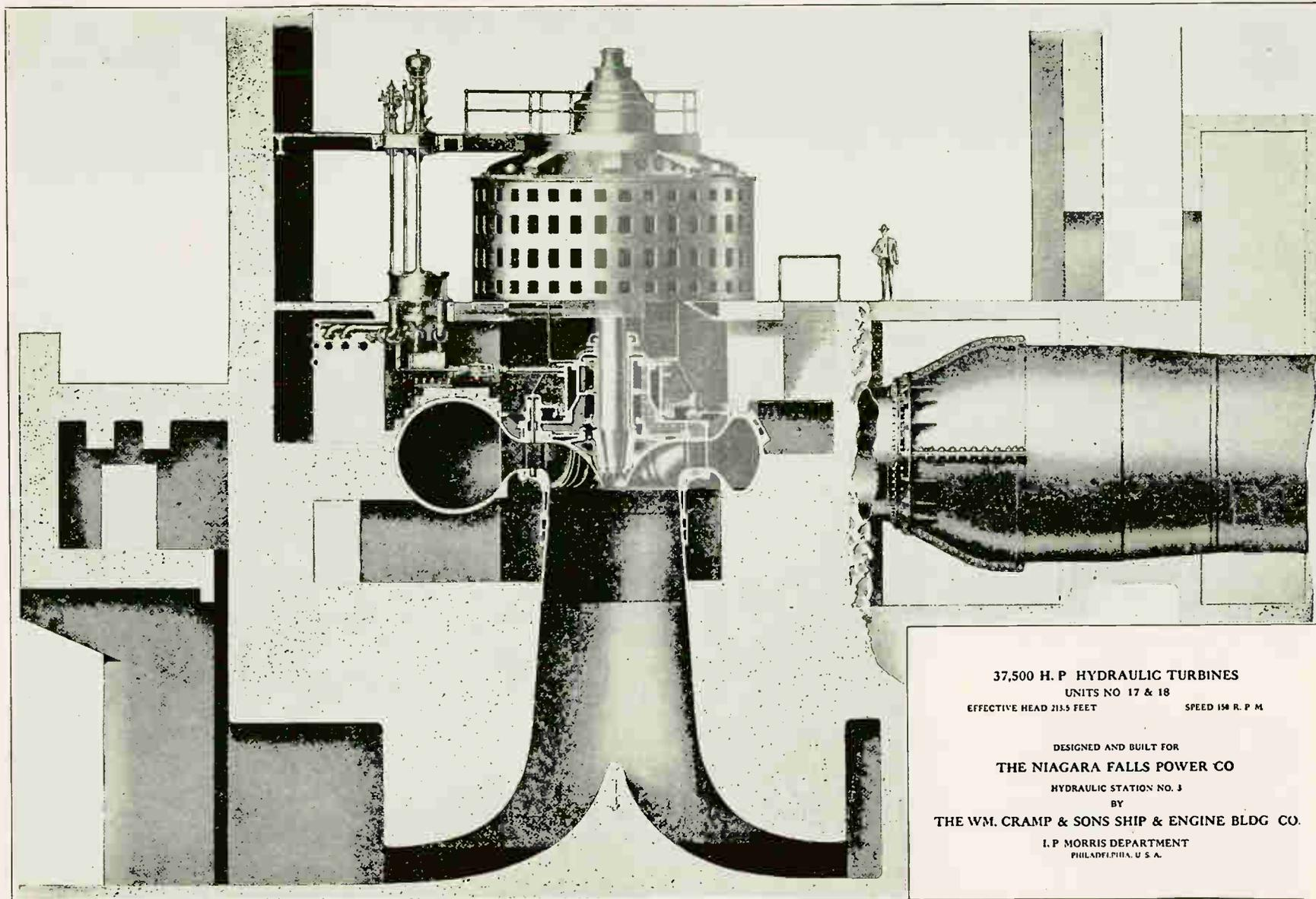
Fig. 98-A. This photo shows a large water-wheel driven alternator and also an excellent sectional view of the hydraulic turbine which drives the alternator. Note the size of the generator compared with the man in the picture. Hundreds of machines of this type are in use in hydro-electric power plants throughout the country.
