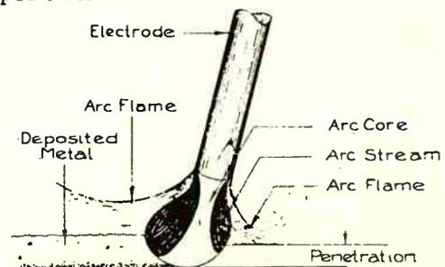
Fig. 1. Diagram of the welding arc.
