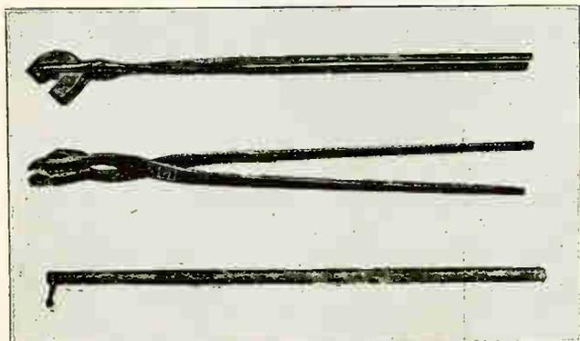
Fig. 436-C. At the top are shown two wood handled fuse tongs for removing and replacing high-voltage fuses, and below is shown a wood handled switch stick or pole for operating disconnect switches. (Courtesy of Schweitzer & Conrad, Inc.)
