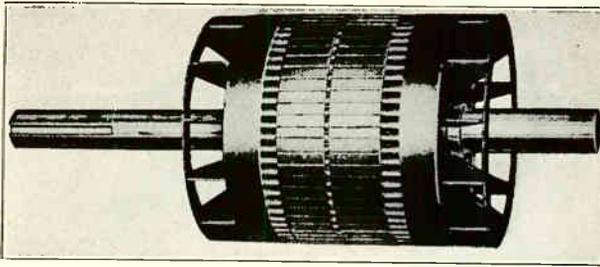
Fig. 160. Squirrel-cage rotor from an A. C. induction motor. Note the manner in which the bars are imbedded in the core slots and also note the ventilating fans at the ends of the rotor.
