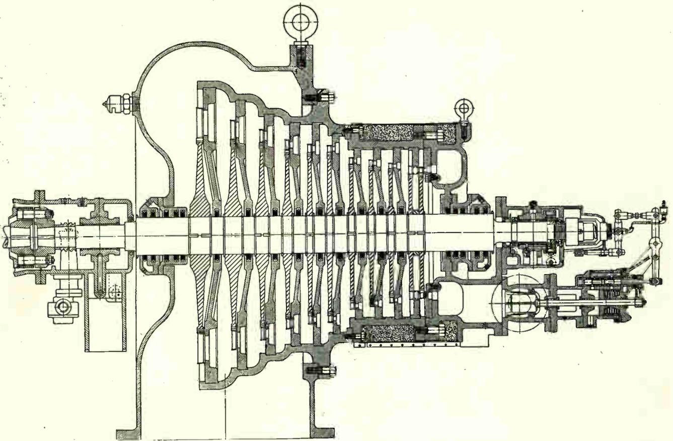
Fig. 315. An excellent sectional view of a modern steam turbine showing how the steam enters the high pressure end at the right and passes through one set of blades after another as it expands toward the exhaust end on the left. The stationary blades redirect the steam to apply its force against each successive ring of movable blades. (Courtesy of Elliott Company.)
