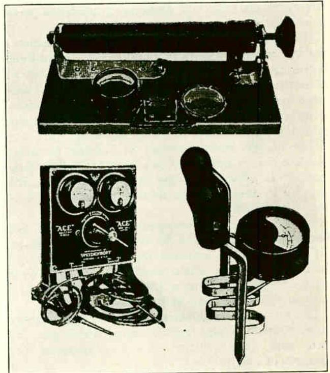
Fig. 22. Several styles of hy-rate discharge test sets. The one above is for either portable or bench use. The one at the lower left for bench use, and the one at lower right for portable use for testing individual cells.
