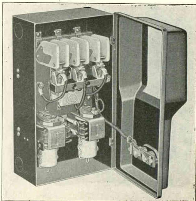
Fig. 268. In this view are shown the overload-relays located beneath the magnetic contactors of an across-the-line starter. (Courtesy Allen Bradley Co.).
