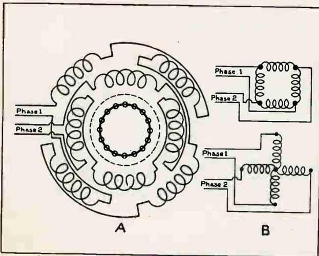
Fig. 175. A. This diagram shows the connections of the stator windings of a two-phase induction motor. At B are shown two schematic diagrams illustrating different methods of connecting two phase windings.
