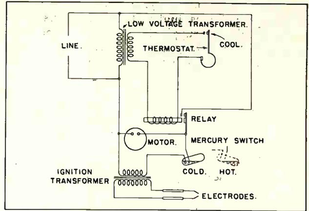
Fig. 13. Control system for an oil burner.
