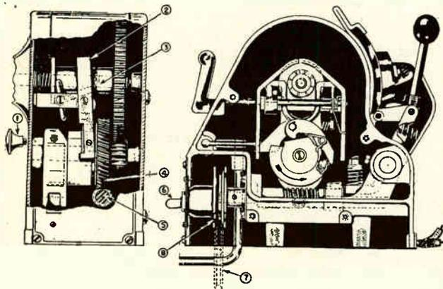
Fig. 11. Drive Mechanism for an Ironer (Kelvinator). 1. Shifter knob. 2. Shifter. 3. Jaw clutch. 4. Worm gear. 5. Worm. 6. Switch. 7. Motor belt. 8. Belt pulley.
