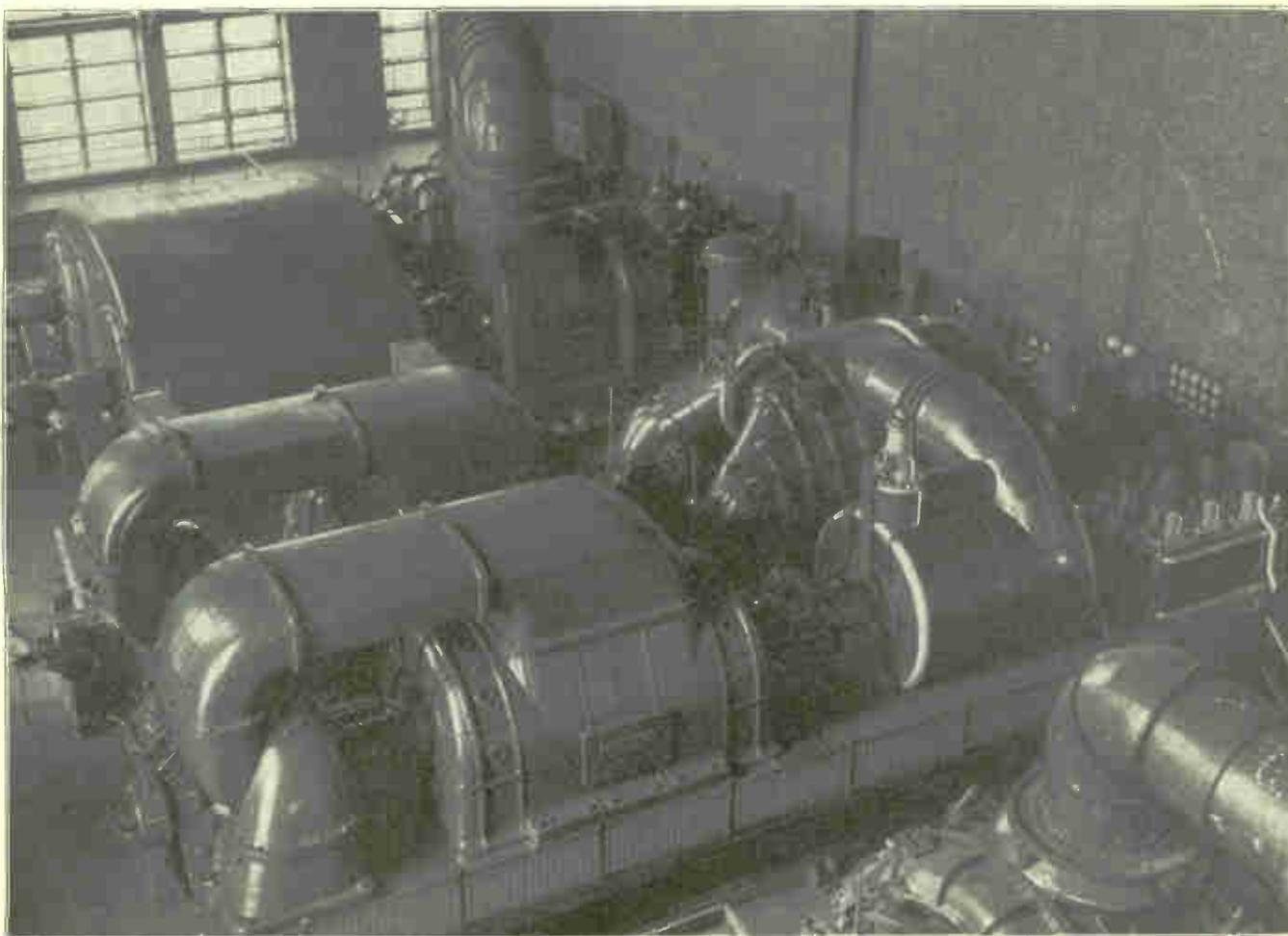
Fig. 3. Modern steam generators of the above type produce many millions of h. p. of electrical energy, for use in lighting and the operation of power machinery. The generator shown in this photo is of 165,000 kw. capacity and is driven by steam turbines. (Photo courtesy of American Brown Boveri Co.)
