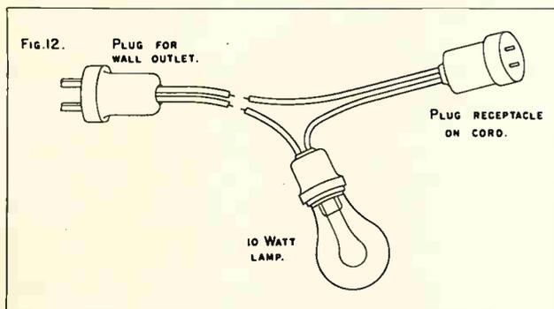
Fig. 12. Test Lamp and Plug Connectors.
