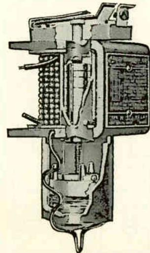
Fig. 280. Sectional view of a magnetic overload-relay and dash pot. When the core is lifted the rod above it forces open the spring contacts which break the circuit to the holding magnet. (Courtesy Allen Bradley Co.).
