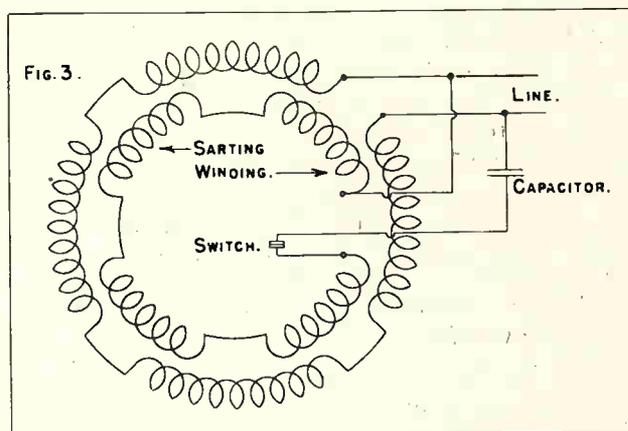
Fig. 3. Connections in a Capacitor-start Motor.
