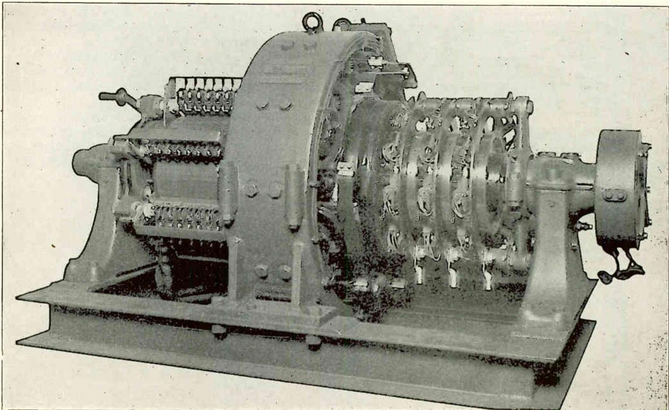
Fig. 251. The above photo shows an excellent view of a modern synchronous converter used for changing A. C. to D. C. The commutator and D. C. brushes are shown on the left and the slip rings and A. C. brushes on the right. Also note the armature, and the shunt and series windings on the field poles. The device on the right-hand end of the shaft is an overspeed safety switch. (Photo courtesy General Electric Co.).
