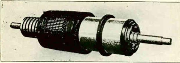
Fig. 254. Photo of converter armature clearly showing the armature winding, slip rings and commutator. A. C. enters at the slip rings and D. C. is taken off from the commutator when this armature is revolved at synchronous speed in the flux of D. C. field poles. Courtesy Allis-Chalmers Mfg. Co.).
