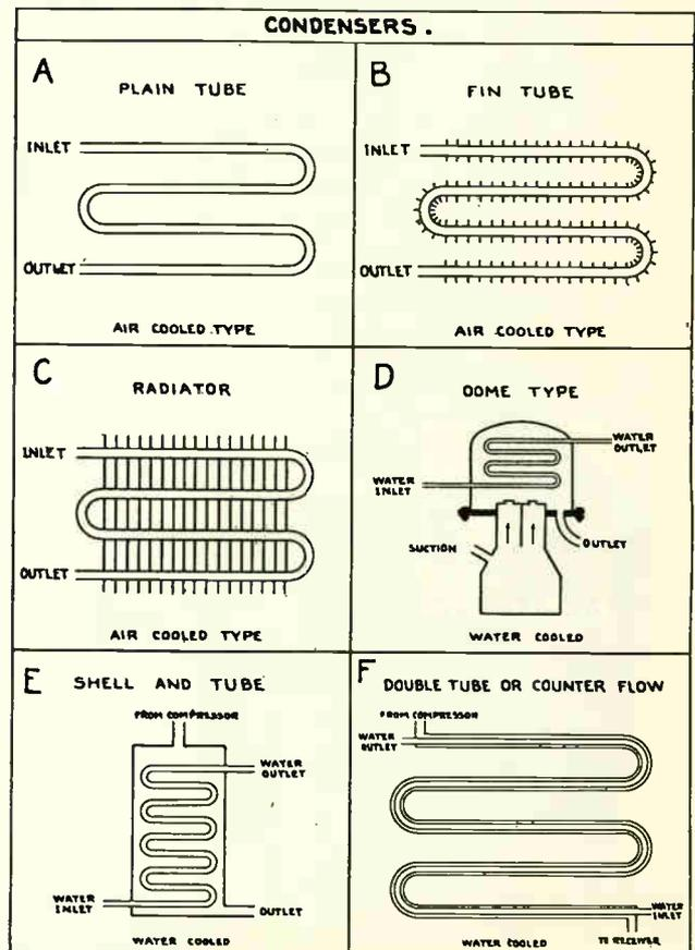
Fig. 45. The above diagram show the construction of several different types of air-cooled and water-cooled condensers such as used in electric refrigerators.
