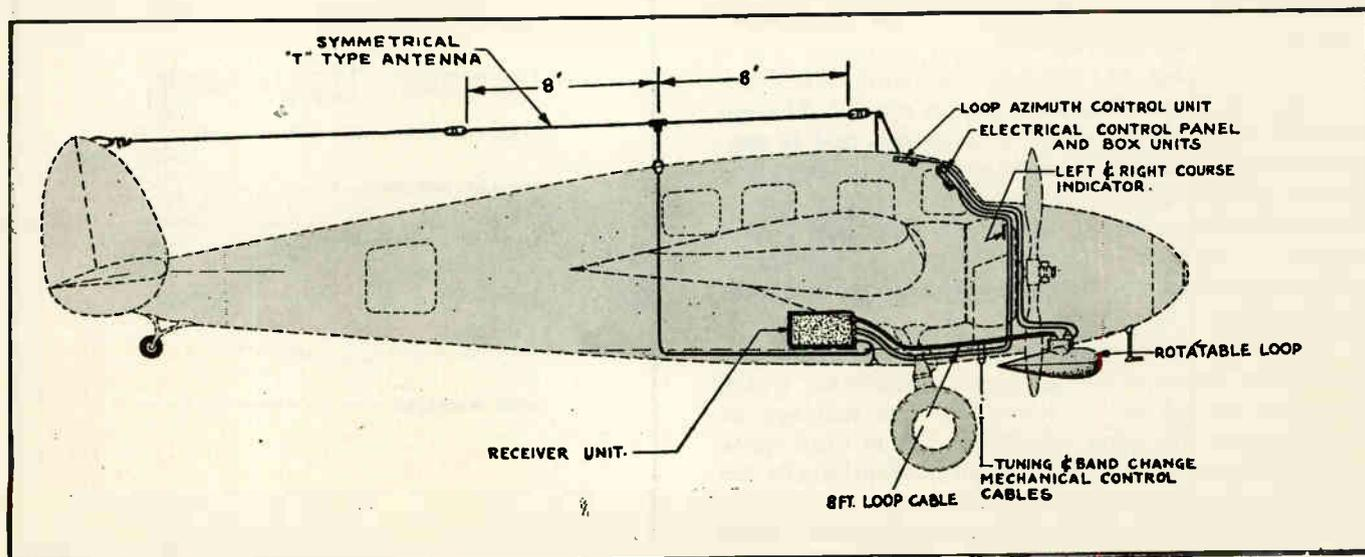
How a rotatable loop and T-type antennae is installed on a biplane.
