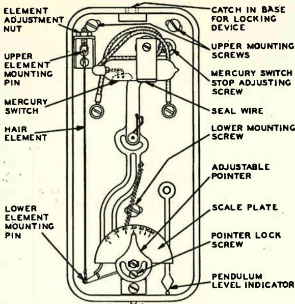
Fig. 155. Diagram of a humidistat such as used for controlling humidity in air-conditioning installations. An electric switch is operated by expansion and contraction of strands of human hair. Courtesy Minneapolis Honeywell Corp.
