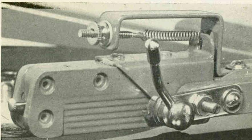
Crystal cutter with special mounting for adjusting cutting depths.
