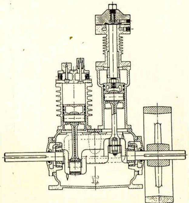
Fig. 80. Sectional view of a 2 stage air compressor used for supplying starting air for Diesel engines.
