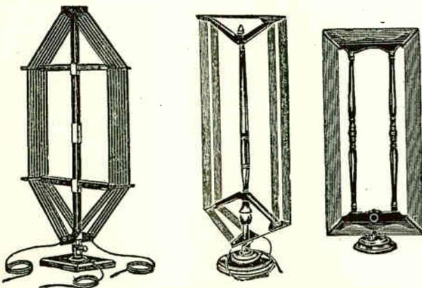
Fig. 31. Several different types of early loop antennas for use with radio receivers. By rotating these loops directional reception can be accomplished. Modern loop antennas will be covered in the Aviation Radio Section.
