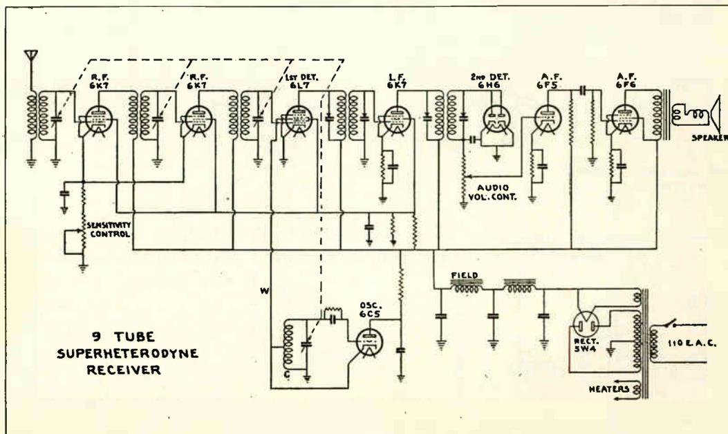
audio stage using the 6F5 tube, and one resistance coupled audio stage using a 6F6 tube.
