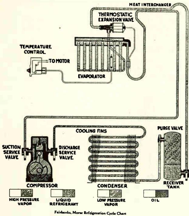
Fig. 26. Cycle diagram of a Fairbanks-Morse refrigerator. Note the different shadings used to represent the refrigerant vapor and liquid and the lubricating oil, and then carefully trace this refrigeration cycle until you thoroughly understand its operation. Also note the similarity between this unit and the one shown in Fig. 25. Courtesy Fairbanks-Morse Co.
