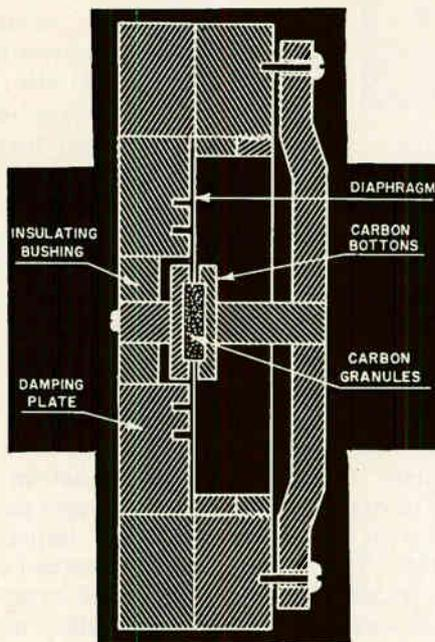
Cross-section of carbon microphone used in inexpensive recorder attachments.
