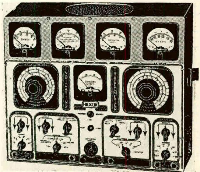
Fig. 211. Above: Dynamic tester for locating circuit troubles in auto radios. Left: An Oscilloscope for checking vibrator performance.
