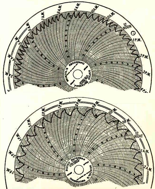
Fig. 131. Note the difference in these two recording thermometer charts taken before and after adjusting the controls on a refrigerator.
