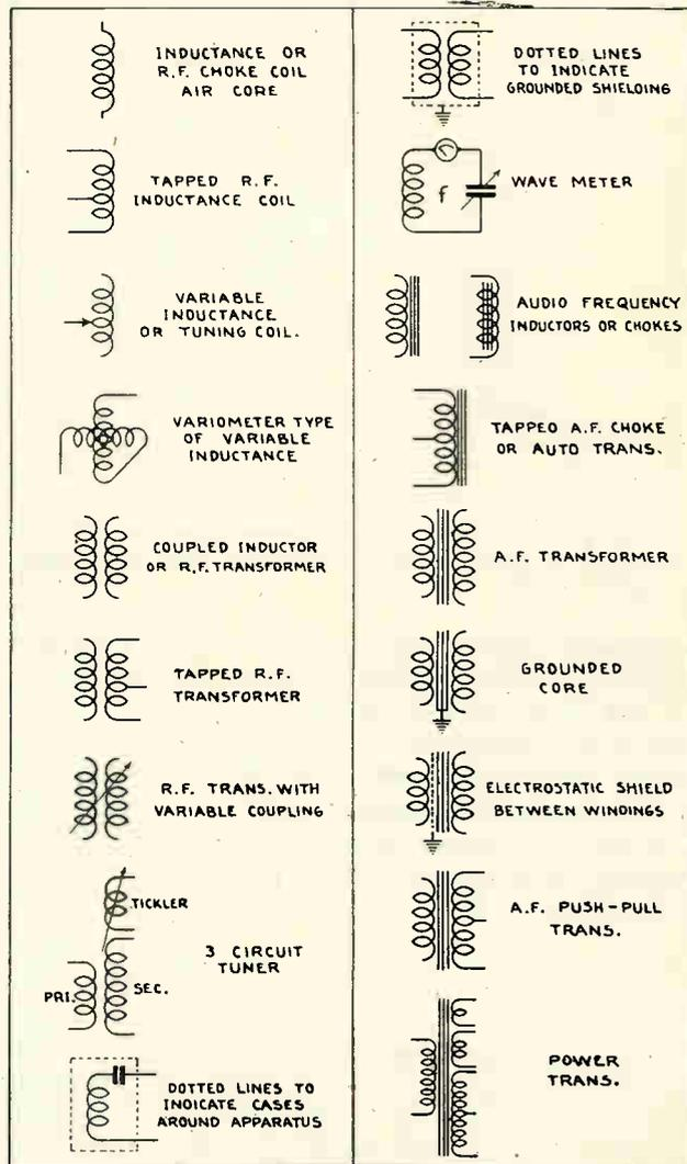
Fig. 48. Radio coil and transformer symbols.
