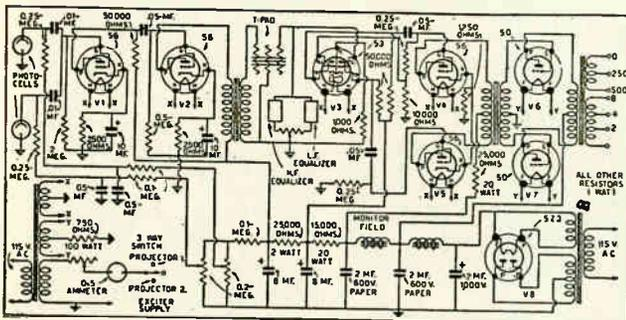
Fig. 238. Circuit diagram of an amplifier such as used with sound picture installations. Note the photo-cell pick-ups and the "T" pad type of volume control. Also note the power supply unit and the push-pull stages of power amplification to the output. Courtesy RadioCraft Magazine.
