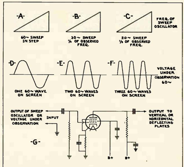
Fig. 250. The sketches at D, E and F in this figure show the type of curves which will be produced by an oscilloscope with the sweep oscillator adjusted to different frequencies with respect to the frequency of the alternating voltage being observed. The diagram at G shows the circuit of a resistance coupled amplifier used to increase the voltages applied to the deflecting plates, in case the receiver circuit voltages are too low to produce normal deflection without amplification.
