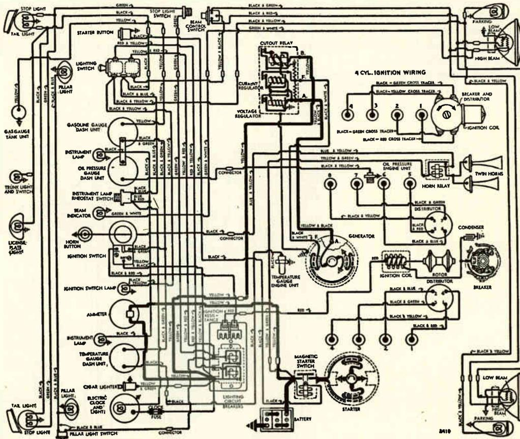
Fig. 94. Complete wiring diagram of V-Eight Ford car. This diagram shows the wiring for the starter, generator, ignition and lights. Trace out each part of the wiring until you thoroughly understand the entire system. Courtesy National Automotive Service.
