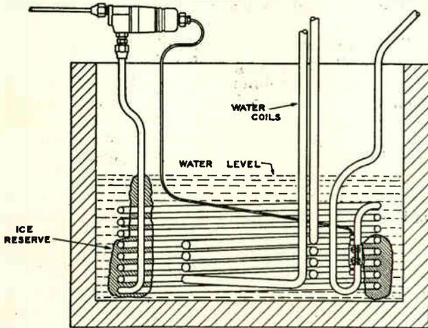
Fig. 132. Refrigerator evaporator coil used in a drinking water cooler.
