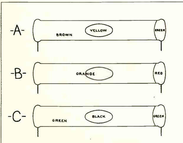
Fig. 152. Sketch showing color code markings used to indicate the resistance values of various resistors. Examine each one carefully while reading the instruction material which explains this color code.
