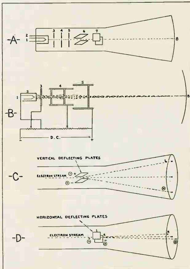
Fig. 248. The above diagrams show several views of cathode ray tubes and illustrates the principle of operation of the electron beam which traces the image of voltage or current waves on the fluorescent screen. Carefully note the various important parts of the tube which are numbered and explained in the instruction material on these pages.
