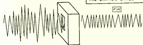
THIS FIGURE SHOWS IN PICTORIAL FORM HOW THE LIMITER FUNCTIONS TO SMOOTH OUT THE AMPLITUDE VARIATIONS IN THE FREQUENCY-MODULATED SIGNAL.
