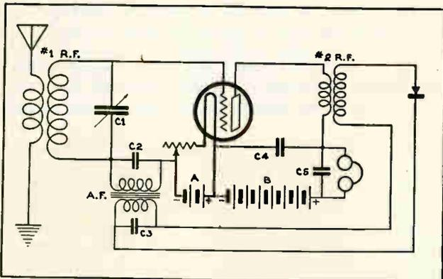
Fig. 106. Circuit diagram of a reflex receiver, in which the one vacuum tube is made to serve both as an R. F. and A. F. amplifier, and a crystal is used as the detector.
