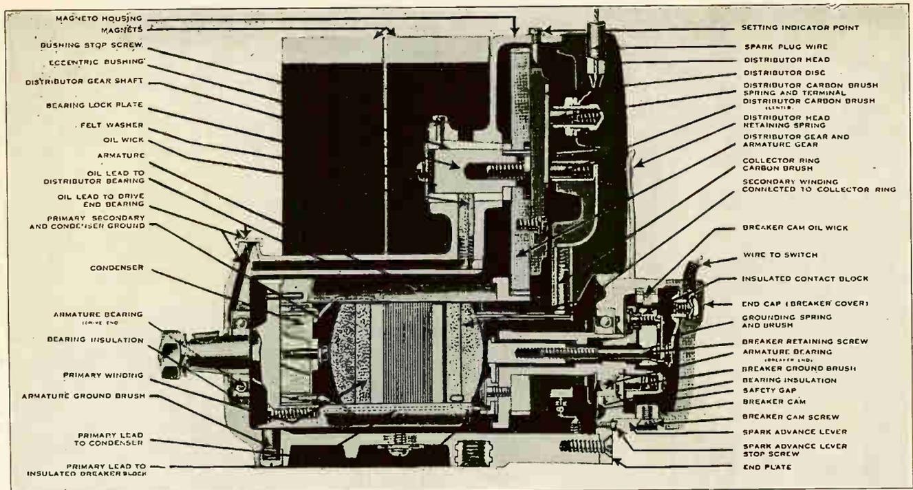
Fig. 58. This excellent sectional view of a magneto shows the arrangement and names of all the important parts. Examine each part very carefully and compare with instructions describing various magneto parts. Courtesy Eisemann Magneto Corp.
