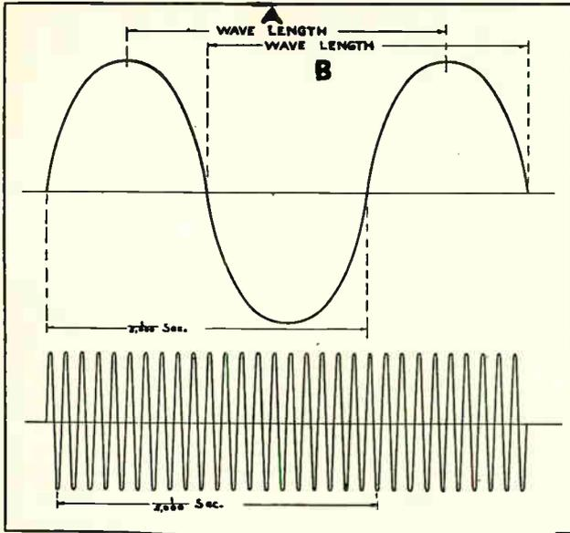
Fig. 9. The above two sets of curves roughly illustrate the difference between the frequency of sound waves and that of radio waves. The contrast between ordinary 60 cycle alternating current and the radio waves would be still greater.
