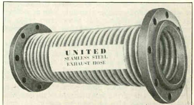
Fig. 99. Short section of flexible exhaust tubing, such as frequently connected in exhaust pipe lines to reduce vibration and to allow for expansion and contraction. (Courtesy United Steel Tubing Company.)
