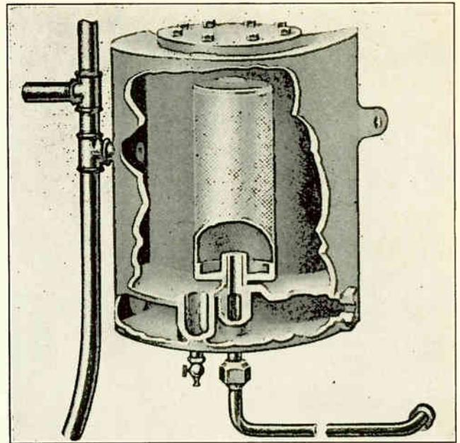
Fig. 50. Cut-away view of auxiliary fuel oil tank, showing filter screen, water pump and valve, and hot water chamber for pre-heating heavy fuel oils. (Courtesy Ven-Severin Co.)
