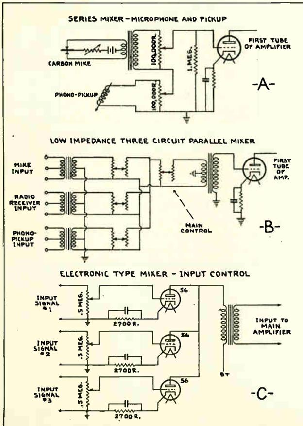
Fig. 235. The above diagram shows several different types of constant impedance volume and mixer controls for use with public address amplifiers.
