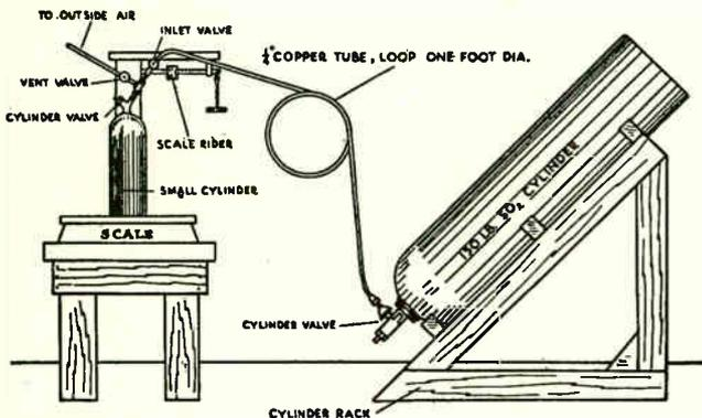
Fig. 64. The above diagram illustrates the method of transferring SO<sub>2</sub> refrigerant from a large shipping cylinder to a small service cylinder. Note the air-vent for purging the transfer tube of air, also the scales for weighing the amount of refrigerant placed in the small cylinder. The large cylinder is inverted so that any vapor in this cylinder will rise above the liquid and force liquid refrigerant to flow through the tube.
