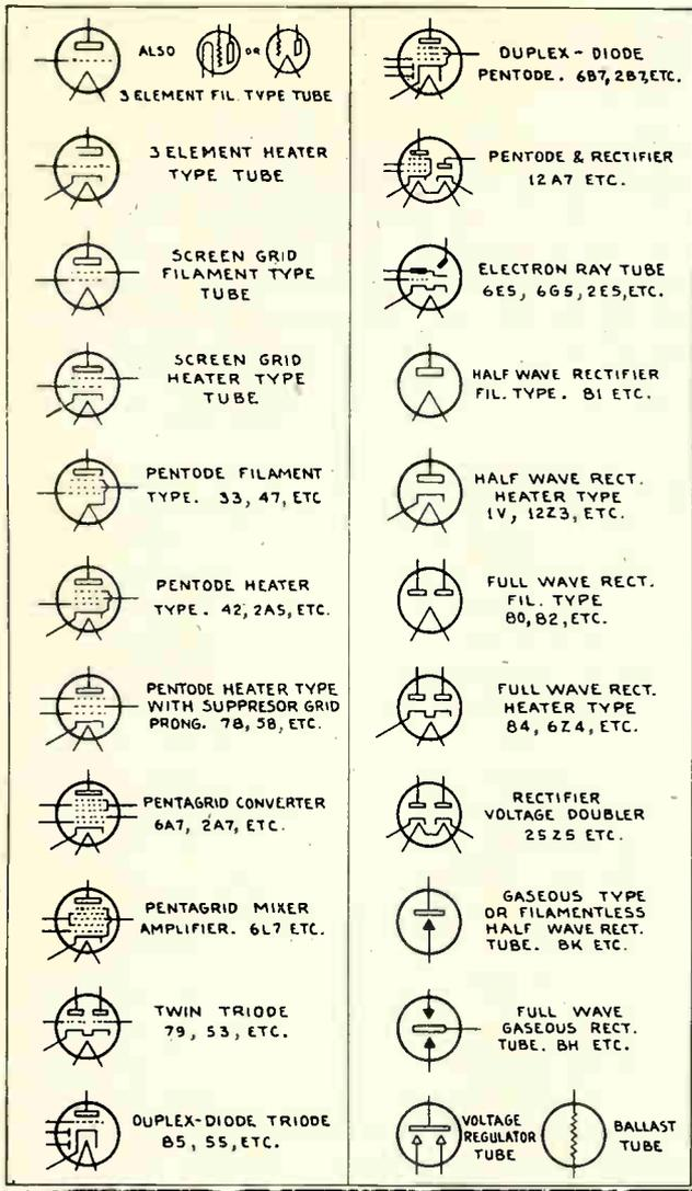
Fig. 49. Radio vacuum tube symbols.
