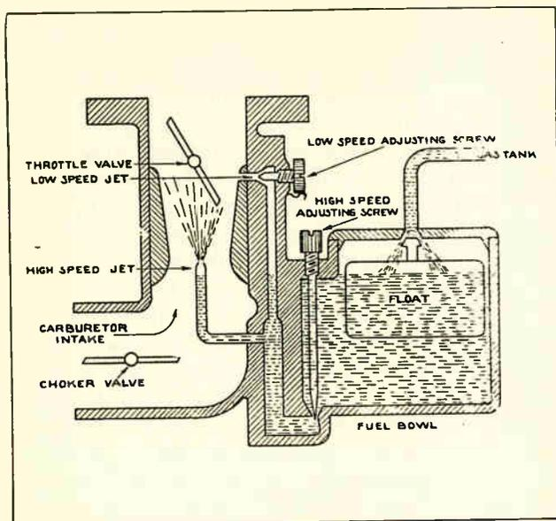
Fig. 6. Diagram showing a sectional view and the operating principles of a simple carburetor used for supplying the proper mixture of gasoline and air fuel to the engine.
