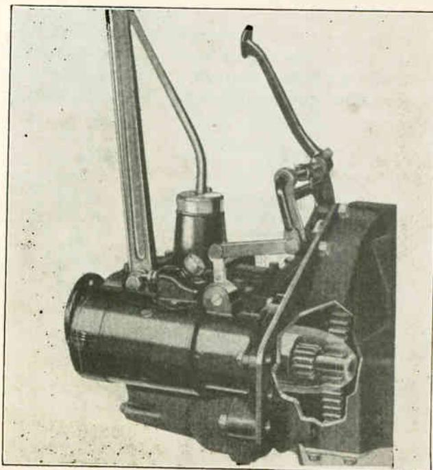
Fig. 67. This view shows method of making the starter pinion with the flywheel gear by means of the starter pedal which operates both the gear and starter switch.
