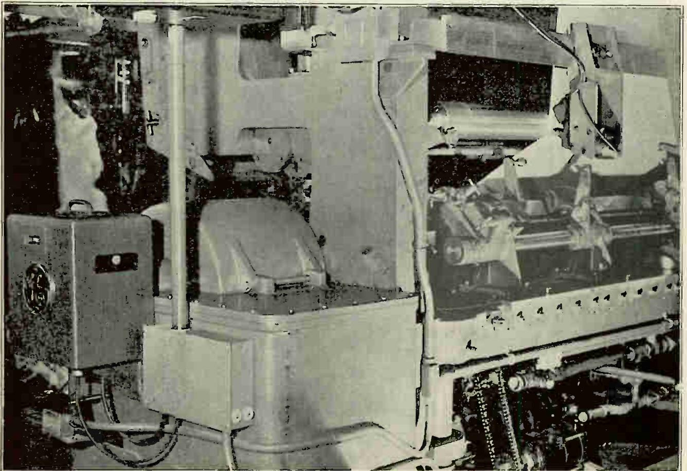
Photo Electro color register control for Multi-color gravure press. View shows mixing panel at top, web scanner at right, disc scanner at left and fractional gear motor for cylinder correction at bottom.
