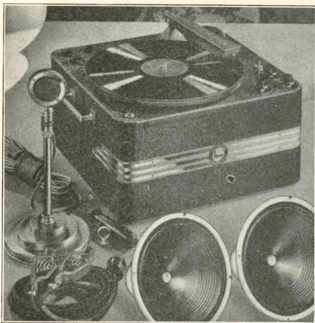
Fig. 229. Phonograph or record turn table and pick-up head with amplifier enclosed in the same compact cabinet. Note the microphone and dynamic speakers which are used with this unit. Courtesy Montgomery-Ward.
