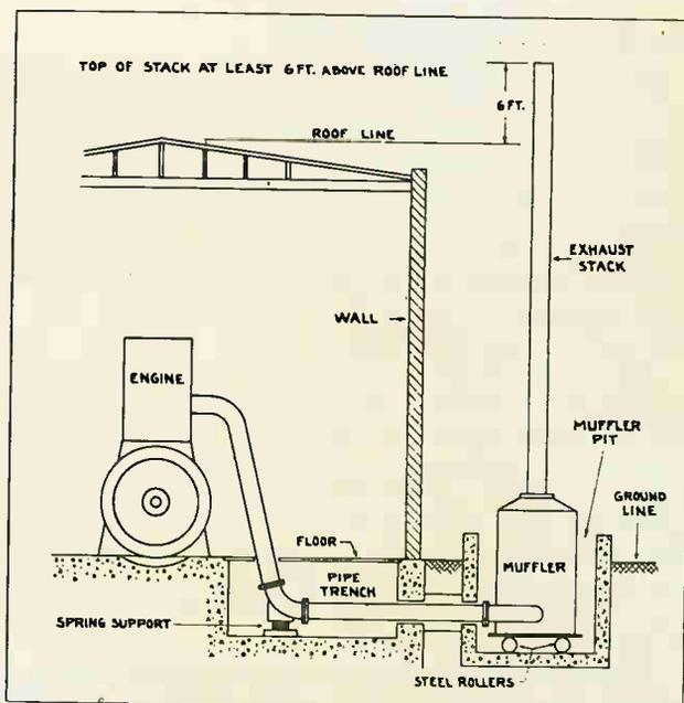
Fig. 93. Diagram showing layout of exhaust system in Diesel engine plant. Note the exhaust pipe, muffler and stack, and the provision for movement due to expansion.
