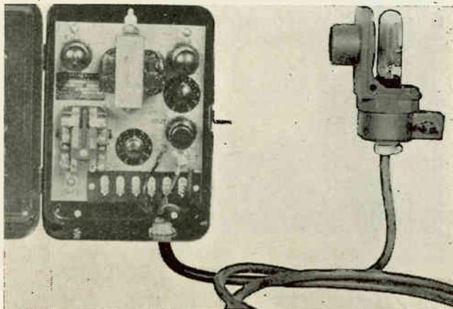
G-E photoelectric relay equipment. The two-unit assembly consists of the phototube holder and associated relay box.
