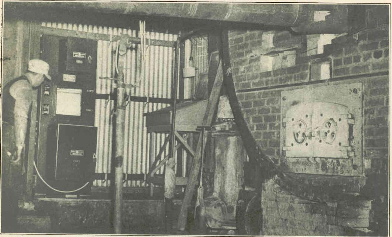
G. E. photo Electric Pyrometer Panel with double chart recorder amplifying equipment and speed-control for temperature control of electrical cement kiln; photo tube holder and optical system on standard in rear center.
