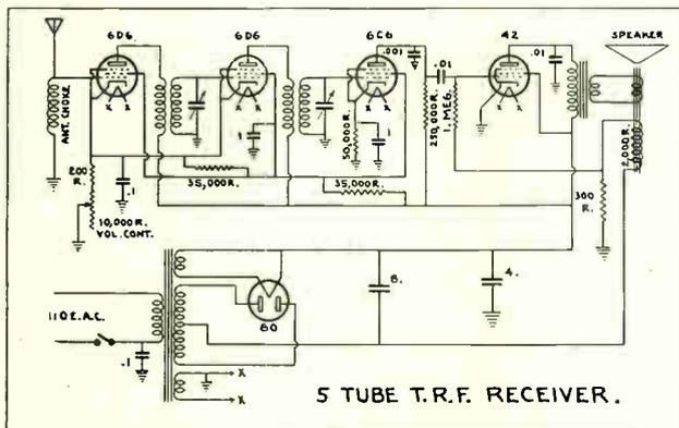
Fig. 148. Circuit diagram of a popular type 5 tube A. C. midget receiver. Note the pentode tubes used for two R. F. amplifiers, detector and one A. F. amplifier. Carefully trace the receiver and power pack circuits, and note the ground connections to the chassis, which completes various circuits.
