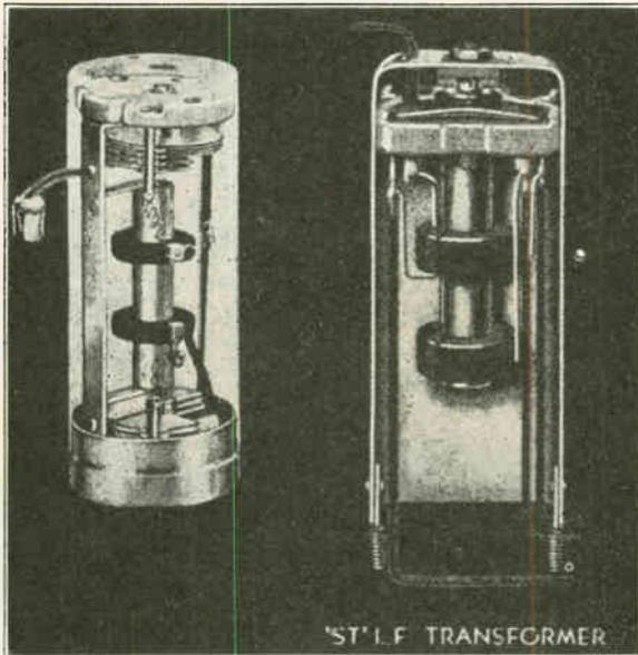
Fig. 165. Two types of I. F. transformers. The one on the left has an air type, variable trimmer condenser, while the one on the right has a mica type, screw-adjusted trimmer condenser in the top section.
