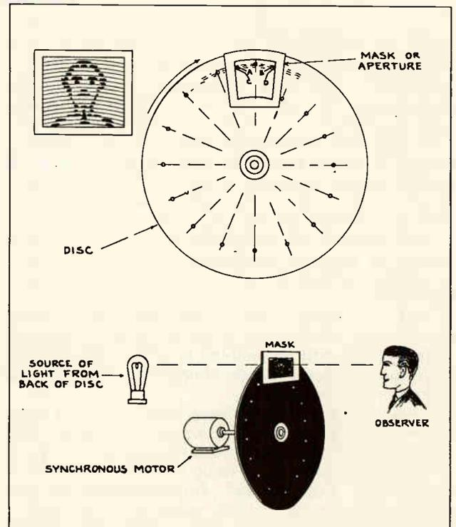
Fig. 259. The above sketch illustrates the mechanical method of scanning a television image. Note the motor driven scanning disc, the mask or aperture, and the light source. Observe this sketch carefully while reading the accompanying explanation on these pages.
