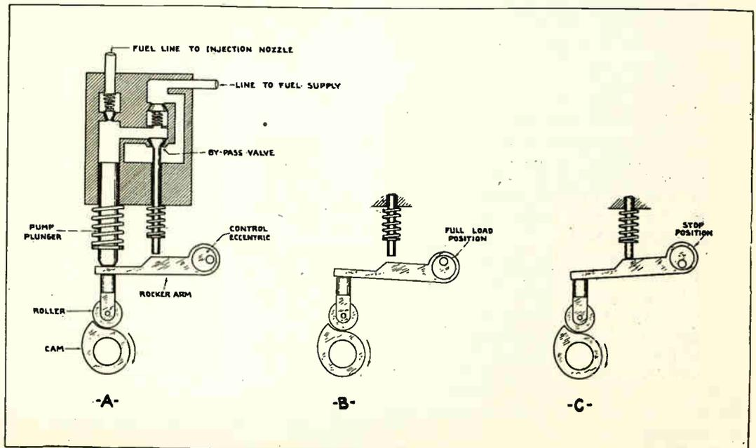
Fig. 34. The figure on the right illustrate the operation of a Diesel fuel injection pump using the by-pass valve method of fuel control. Note how the time of opening of the by-pass valve, and the amount of fuel charge is governed by the position of the control eccentric.
