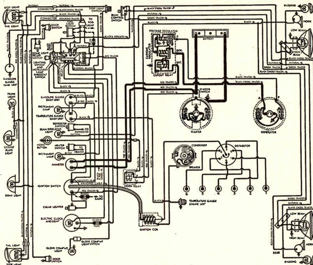
Fig. 90. Wiring diagram of 1941 Oldsmobile car. Note the current-voltage regulator used for controlling generator output, and also the lighting switch and instrument lamp rheostat. Courtesy National Automotive Service.
