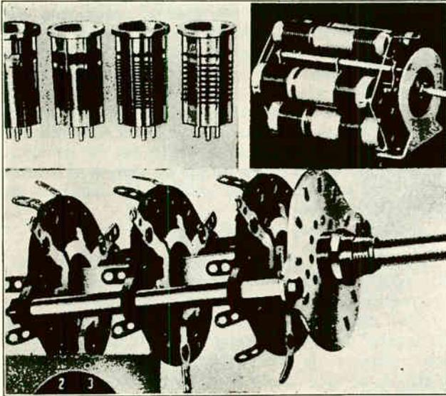
Fig. 179. At the upper left are shown several plug-in type coils, and at the upper right a set of coils and selector switch assembly for quickly changing wave lengths on all wave sets. In the lower view is shown a 3-gang, multi-point selector switch such as used for changing the coil connections on all wave receivers. Courtesy Montgomery-Ward & Company.
