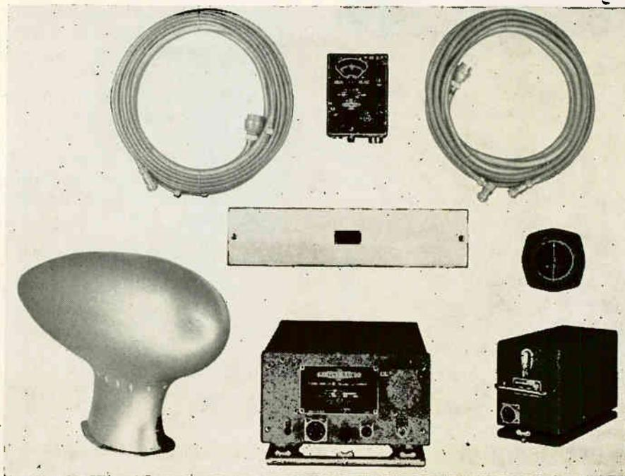
Modern shielded loop antenna is streamlined to present little resistance to wind.
