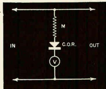
Correct way to connect a copper-oxide rectifier type output meter.
