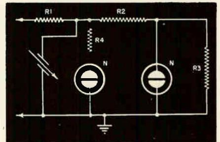
Two neon lamps show volume peaks in this circuit.
