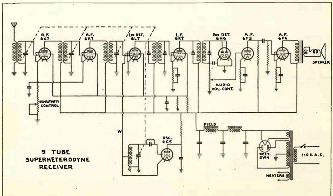
audio stage using the 6F5 tube, and one resistance coupled audio stage using a 6F6 tube.
