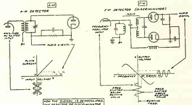
HOW THE SIGNAL IS DEMODULATED. THE DETECTOR OR DISCRIMINATOR. THE AMPLITUDE-MODULATION DETECTOR CONVERTS THE VARIATIONS IN AMPLITUDE OF THE MODULATED WAVE INTO THE ORIGINAL AUDIO SIGNAL. THE FREQUENCY-MODULATION DETECTOR CONVERTS THE VARIATIONS IN FREQUENCY OF THE F.M. WAVE INTO THE ORIGINAL AUDIO SIGNAL. THE CHARACTERISTIC OF THE DISCRIMINATOR CIRCUIT WHICH ACCOMPLISHES THIS IS SHOWN ABOVE.
