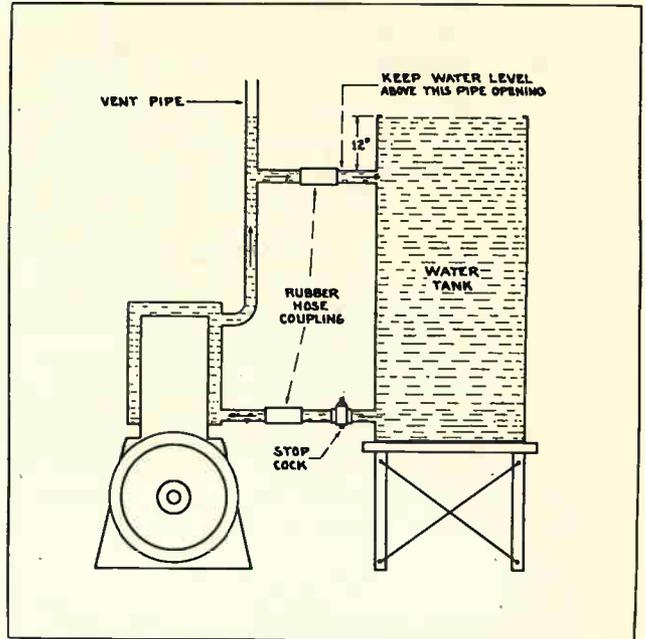
Fig. 109. Diagram showing the tank and pipe arrangement for a thermo-syphon cooling system for a stationary Diesel engine.
