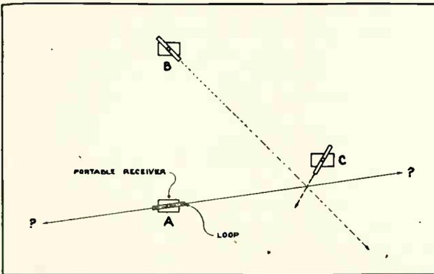
Fig. 270. This sketch illustrates the method of locating a source of radio interference with a portable receiver and a loop aerial.
