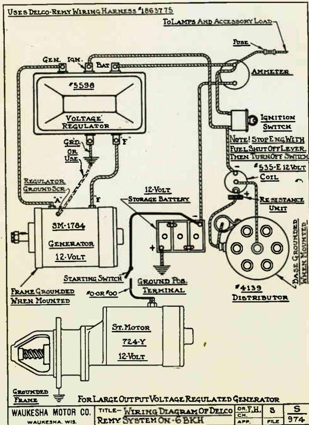
Fig. 91. Circuit diagram of the electric starting motor, battery, generator and ignition equipment of a Waukesha engine, which uses spark plug ignition. Note the instructions for stopping this type of engine. (Courtesy Waukesha Motor Co.)
