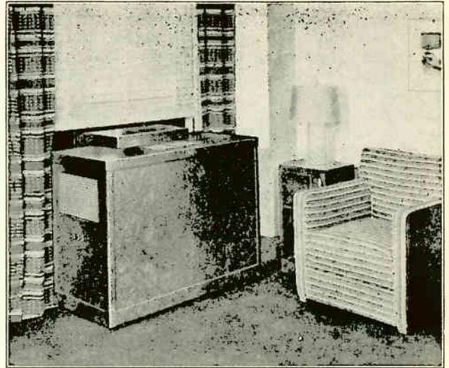
Fig. 144. Photo showing convenient portable room cooling unit located in a living room. This electrical cooling unit draws air from the window for cooling and ventilating the room, and also for cooling its own refrigerator condensing unit. Courtesy Pacific Mfg. Corp.
