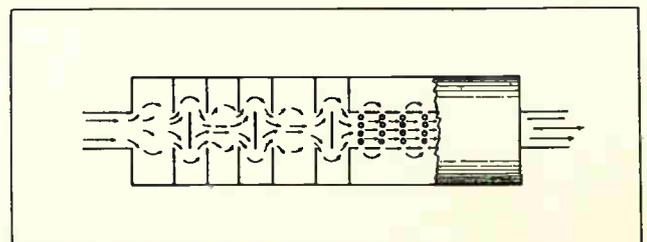
Fig. 96. This sketch shows how the exhaust gases pass through a muffler of the baffle type.
