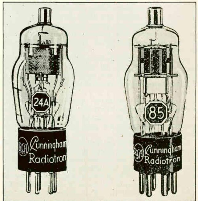
Fig. 53. The 24A tube shown above is a R. F. amplifier tube and the 85 is a duplex tube.
