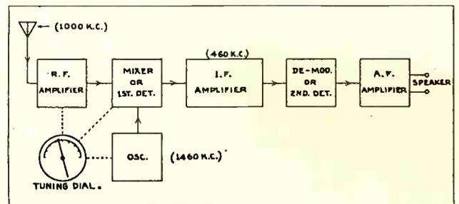
Fig. 157. Simple block diagram showing the important parts or sections of a superheterodyne receiver, and the order in which signals must pass through this type of set.
