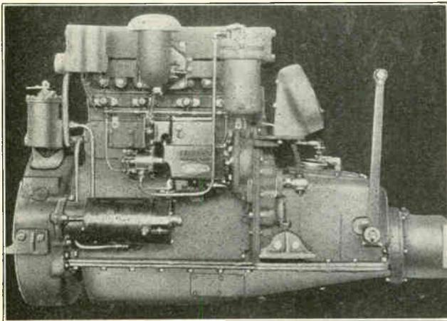
Fig. 73. Above photograph shows a Diesel engine equipped with an electric starting motor similar to those used for starting automobile engines. Diesel engines used on trucks and busses are commonly equipped with this type of electric starter. Courtesy Buda Engine Company.
