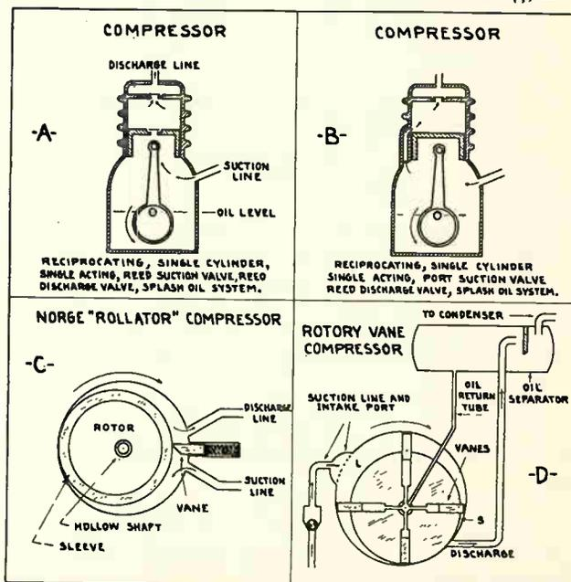
Fig. 35. The above diagrams show several types of reciprocating and rotary refrigerator compressors. Examine and check every operation carefully while reading the lesson material.
