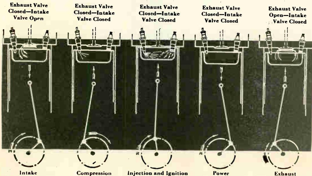
Fig. 62. The above views show the shape of the piston head, the angle of fuel injection and the combustion cycle of a Waukesha Hesselman engine. This engine is one of the lower compression types using spark plug ignition. The shape of the depression in the piston head mixes the fuel spray with the air and also directs the mixture against the spark plug. (Courtesy Waukesha Engine Co.)
