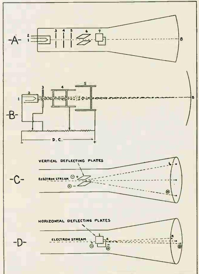
Fig. 248. The above diagrams show several views of cathode ray tubes and illustrates the principle of operation of the electron beam which traces the image of voltage or current waves on the fluorescent screen. Carefully note the various important parts of the tube which are numbered and explained in the instruction material on these pages.
