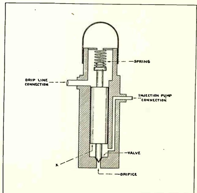
Fig. 43. Sectional view showing the construction of a closed type injector nozzle. Note the spring loaded valve which keeps the nozzle orifice closed until the oil pressure underneath the piston overcomes the spring pressure.
