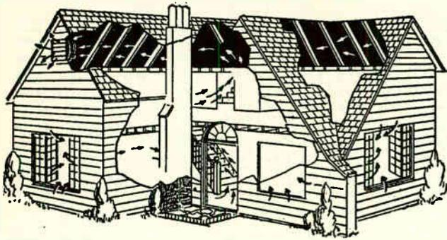
Breez-Air Fan mounted in box which stands on attic floor.
