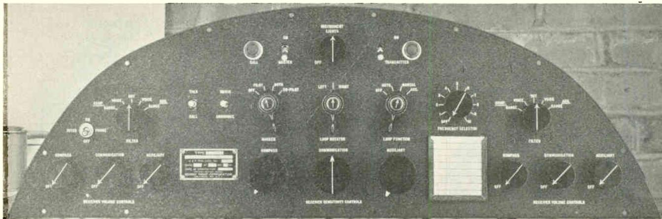
Modern aircraft instrument control panel. Duplicate controls are provided for each pilot.
