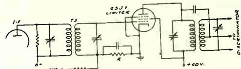
THE LIMITER STAGE IS USED IN F.M. RECEIVERS TO REMOVE VARIATIONS IN AMPLITUDE OF THE FREQUENCY-MODULATED WAVE. LOW PLATE AND SCREEN VOLTAGES ARE EMPLOYED SO THAT THE LIMITER AND SCREEN VOLTAGES ARE KEPT NEARLY CONSTANT REGARDLESS OF OVERLOADS. WHEN THE INPUT SIGNAL IS WEAK, THE OUTPUT FROM THE DISCRIMINATOR IS THEREBY MAINTAINED CONSTANT DUE TO NOISE OF VARIATIONS IN THE STRENGTH OF THE INCOMING SIGNAL. IN A.M. RECEIVERS, OF COURSE, THE LIMITER IS NOT USED.
