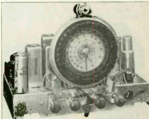
Fig. 175. A good view of the push button dial of the manual automatic tuning system used on another modern type of radio. Courtesy Wells-Gardner Company.
