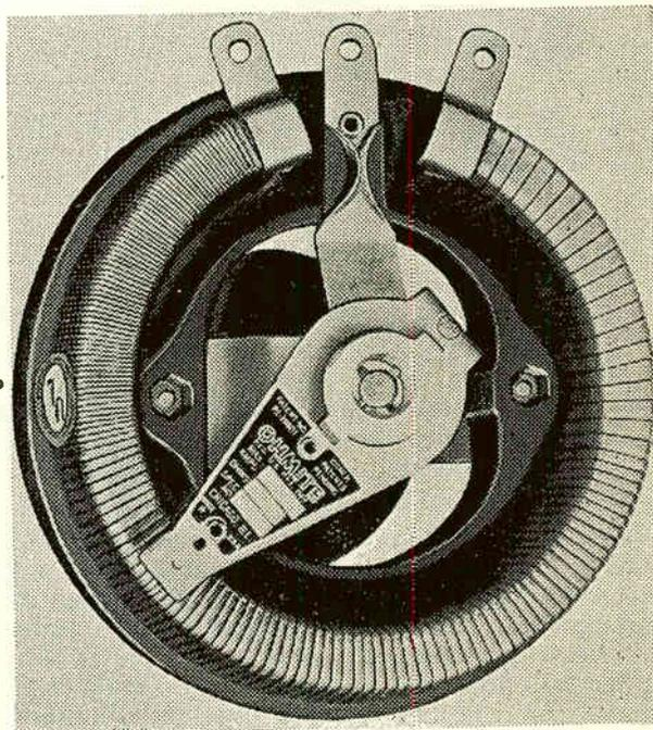
Fig. 187. Heavy duty rheostat. Wire size varies to produce a "taper." Some rheostats are 12 inches in diameter.
