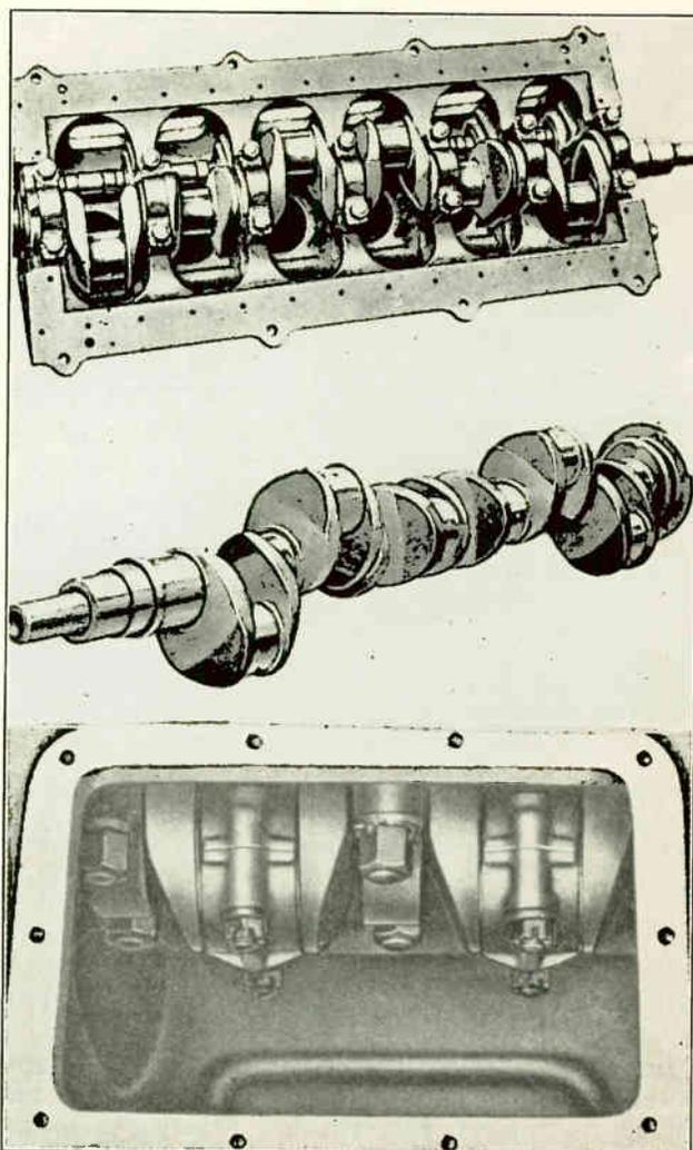
Fig. 145. At the top is shown a crank shaft mounted in the bearings and crank case while in the center view it is shown removed. Below one of the side plates is shown removed to permit accessibility to the crank shaft bearings for easy adjustment.
