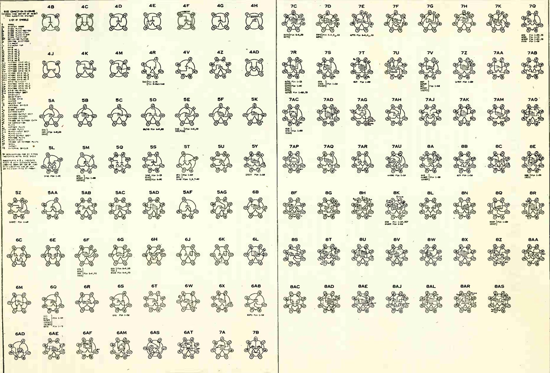
Fig. 100A. Tube base chart. (Courtesy Ratheon Mfg. Co.)
