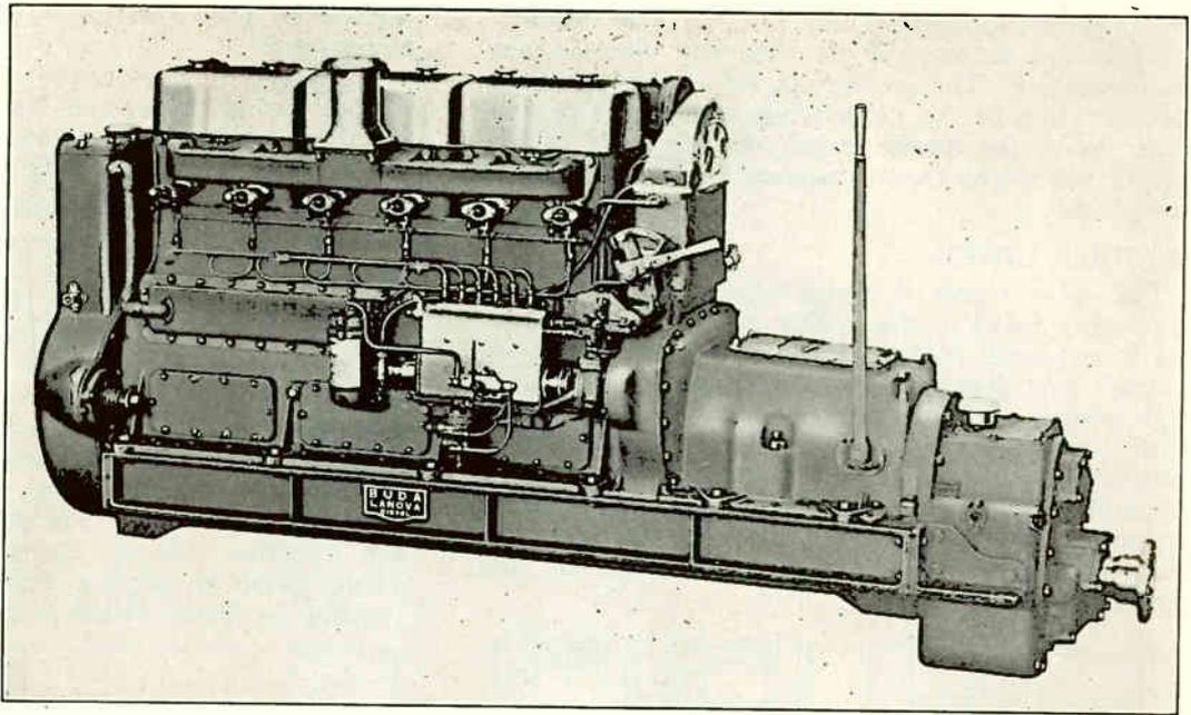
Fig. 42. This photograph shows the mounting and arrangement of the fuel injection pump, filter, fuel lines, injector nozzles, and throttle control on six cylinder marine type Diesel engine. (Courtesy Buda Manufacturing Co.)
