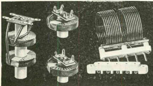
Fig. 103. On the left are various types of tuning coils. The large space-wound unit is for low-power transmitters. On the right are the parts needed to assemble a permeability tuner coil.
