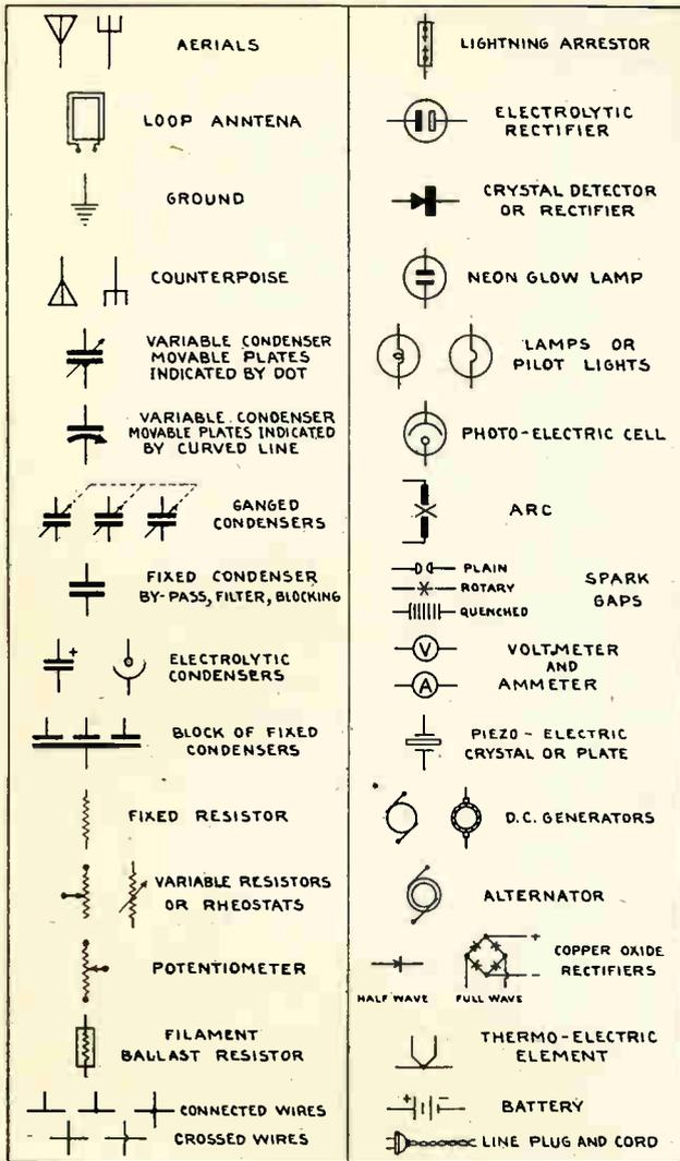
Fig. 47. Radio wiring symbols.
