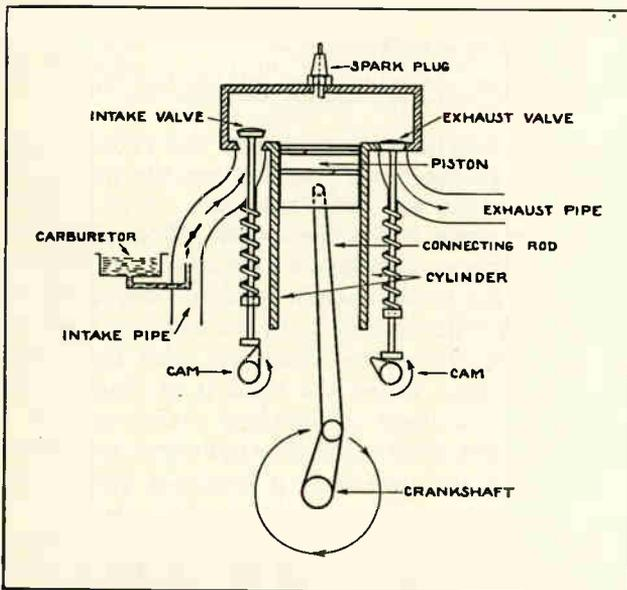
Fig. 1. This diagram illustrates the operating principle of a simple one-cylinder internal combustion engine. Study the diagram carefully while reading the explanation.
