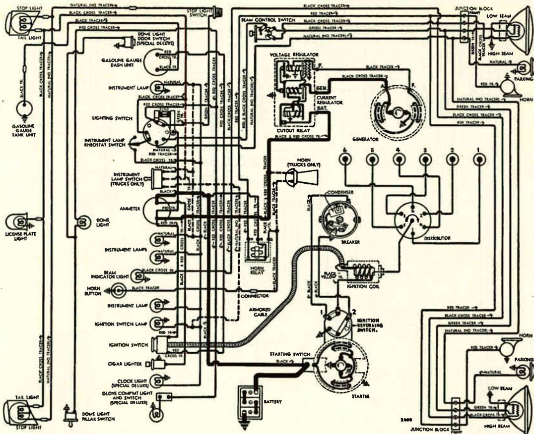
Fig. 89. Complete wiring diagram of 1941 Chevrolet. Note carefully the location and arrangement of all of the electrical devices. Trace the circuits one at a time to become thoroughly familiar with the common types of automobile wiring systems. Courtesy National Automotive Service.
