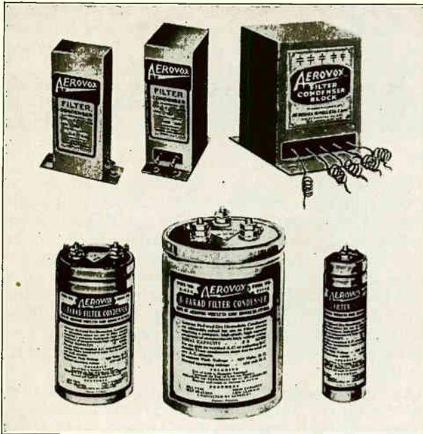
Fig. 146. Photo showing several types of fixed condensers used for filter condensers in power supply units. The condensers in the top row are paper and mica types, while those below are electrolytic types. (Photo courtesy of Aerovox Wireless Corp.)
