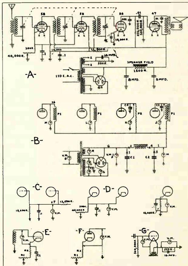
Fig. 208. Carefully refer to the above partial circuit diagrams of this receiver while reading the instructions on radio service tests as illustrated in these sketches.
