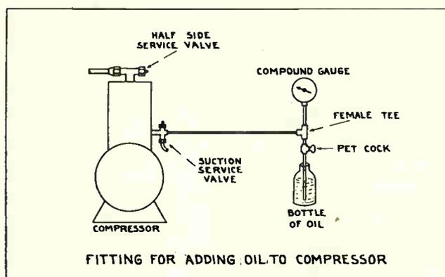
Fig. 110. A very convenient device for adding oil to refrigerator compressors can be made with short lengths of tubing, compound gauge, and pet cock as shown above.
