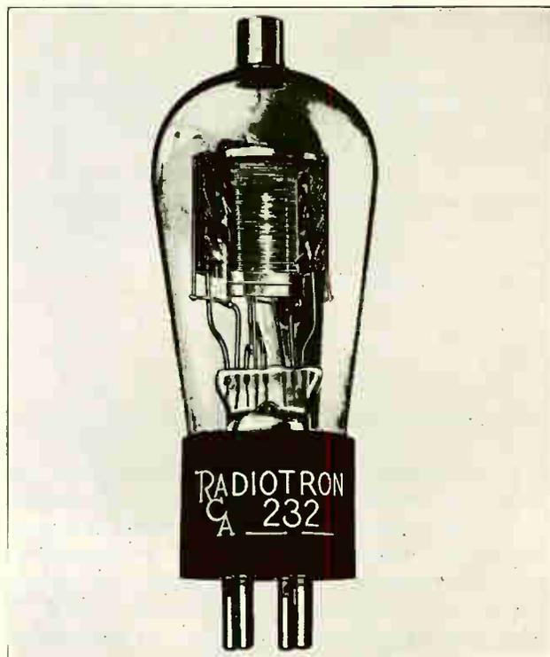
Fig. 77. This excellent photograph shows a vacuum tube with part of the outer screen grid and part of the plate removed, to clearly show the inner screen grid in its position between the control grid and plate. (Photo courtesy of R. C. A. Radiotron Co., Inc.)
