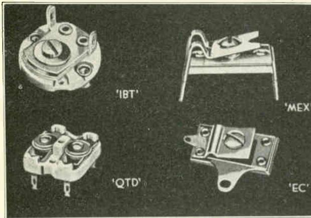
Fig. 167. Several types of trimmer condensers such as used on I. F. and R. F. transformers for aligning or balancing their circuits. The moveable plate or strip is moved closer to, or farther from, the stationary plate by turning the adjusting screws.
