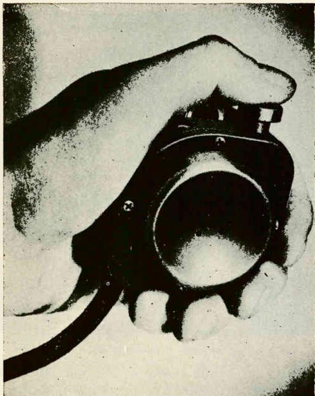
Aircraft microphone for close-talking—operator has to be very close to it to exclude all outside noise.
