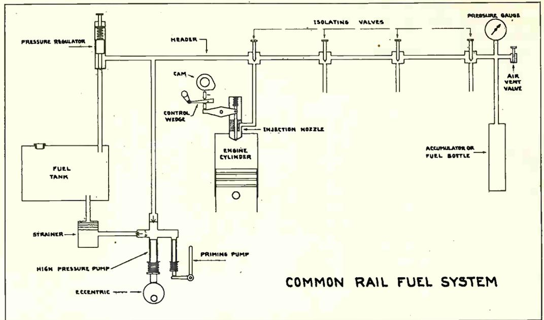
Fig. 47. Diagram showing the essential parts of the common rail fuel system for a Diesel engine. Carefully note the arrangement and purpose of each part while studying the accompanying explanation.
