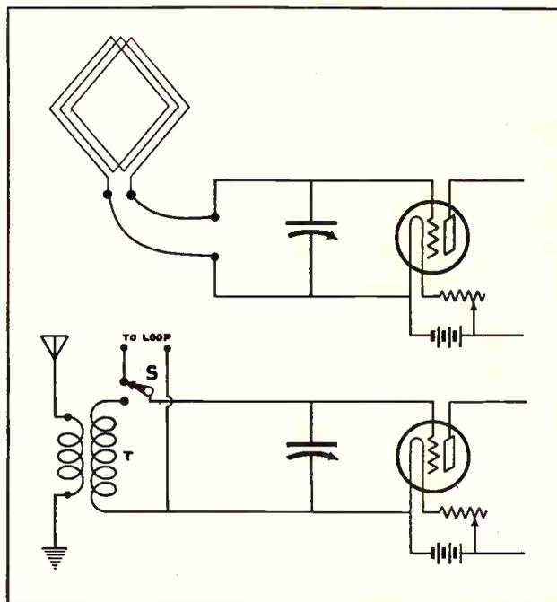
Fig. 30. The top sketch shows a loop aerial connected directly to the grid circuit of a vacuum-tube receiver. The lower sketch shows how a receiver can be adapted for use with either a loop or an aerial and ground.
