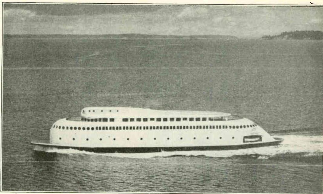
Fig. 2. Photo of a modern streamlined Diesel powered ferry boat. Diesel engines are extensively used on boats, dredges and tugs. Many of these units are also Diesel-Electric combinations, and require trained men with electrical and Diesel knowledge to operate and maintain them.
