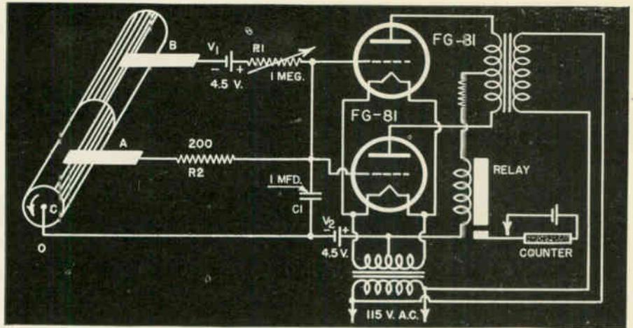
A modern hydraulic flow indicator circuit.
