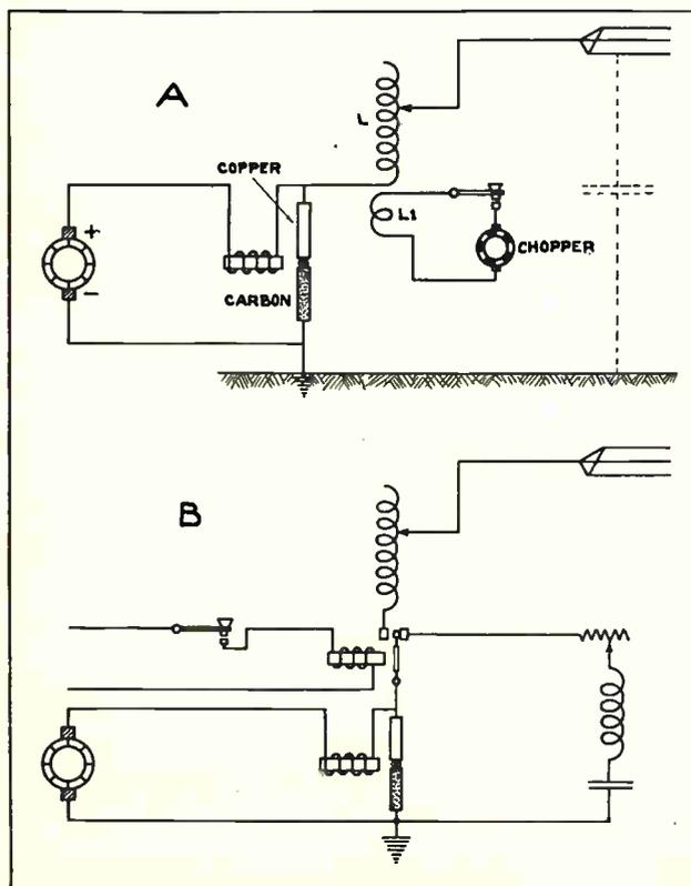
Fig. 17. Two simple sketches of arc radio transmitters, using different methods of controlling the antenna current for code signalling.
