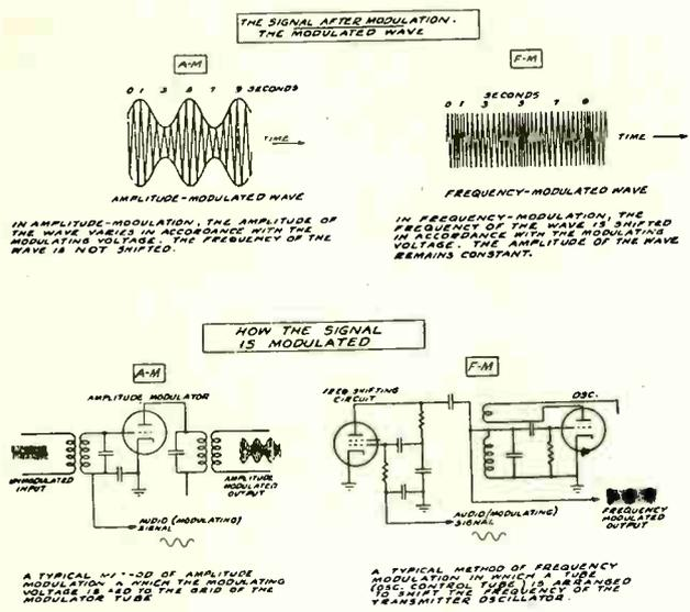
Fig. 191A. This diagram illustrates the difference between A. M. and F.M. modulated waves above, and modulating circuits below.
