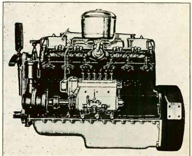
Fig. 54. Photo of Hercules automotive type Diesel engine showing vacuum type generator unit attached to left end of fuel pump, and connected by tubing to the intake manifold.
