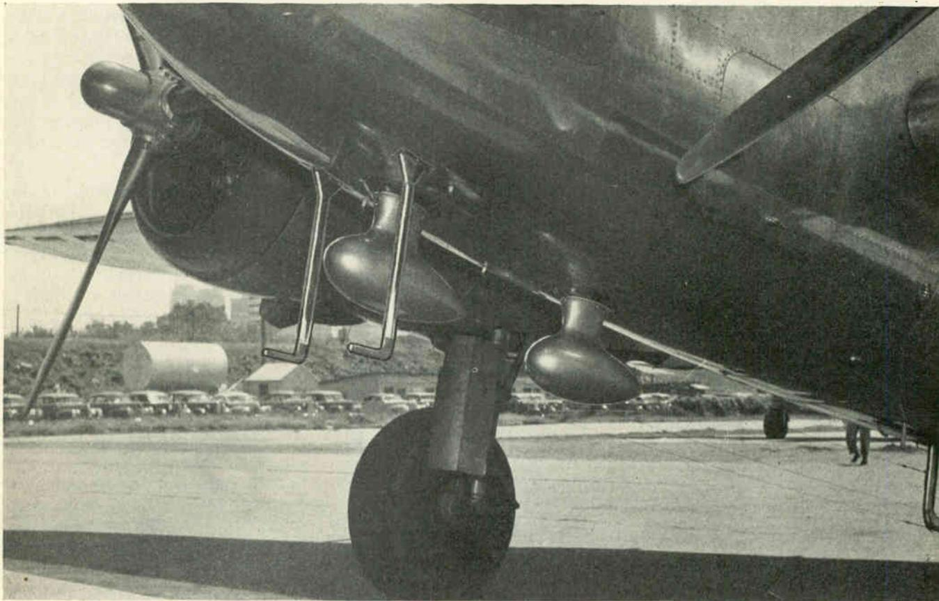
The loop antennas under the "belly" of this huge transport plane guide the ship safely over its air route.
