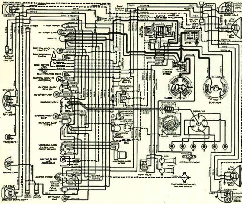
Fig. 91. Wiring diagram of a 1941, eight cylinder Chrysler auto. Trace out the primary and secondary ignition circuits, the starting motor and generator circuits and the various light circuits. Note the color code of the various wires. This is a great help in electrical trouble shooting on the car.
