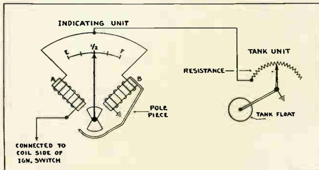
Fig. 46. Diagram of a resistance type gasoline gauge.
