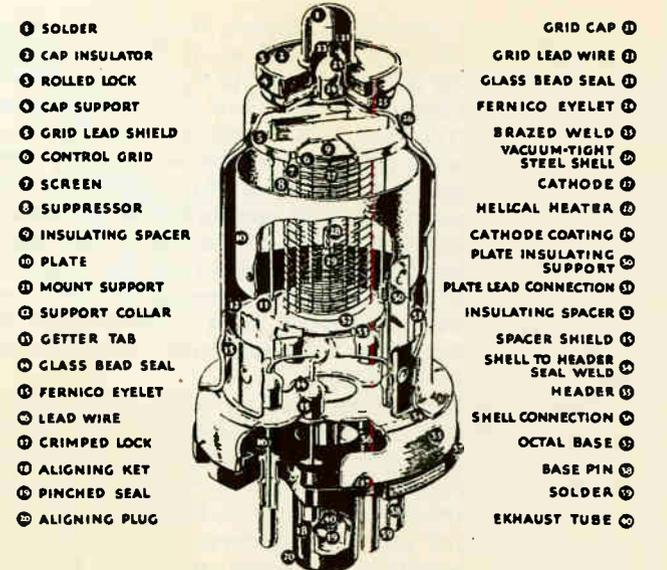
Fig. 57. This figure shows the structure of an all-metal tube.
