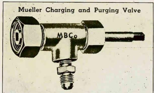
Fig. 101. Charging and purging valve such as used in connection with the regular shut-off valve for charging or purging rotary type compressors which are not equipped with regular low side and high side service valves. Courtesy Mueller Brass Company.
