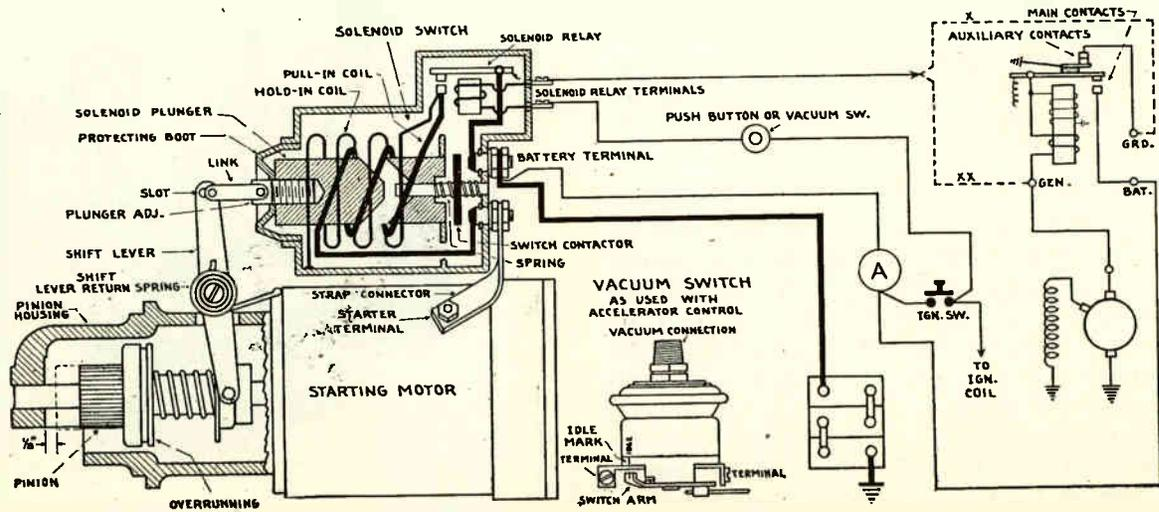
Fig. 68. Wiring diagram for a common tune automatic starter switch.
