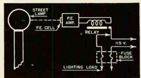
Photocell and relay operate when street light is turned off.
