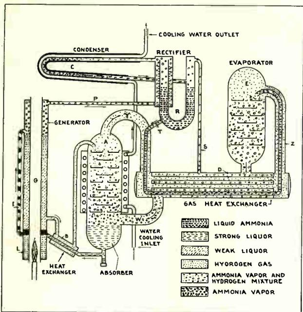
Fig. 66. This diagram clearly illustrates the operating principles of the Electroflux absorption type refrigerator. Carefully study and check each part of the cycle as explained in the accompanying instructions.
