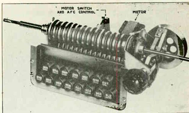
Fig. 174. This excellent photo shows the automatic tuning mechanism of a modern radio. Note the push buttons which energize the motor, which in turn rotates the gang condenser shaft until the proper disk or cam allows its catch to drop in the slot. Courtesy Stewart-Warner Company.
