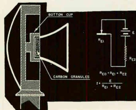
Construction view of carbon telephone transmitter. Now is obsolete by crystals.
