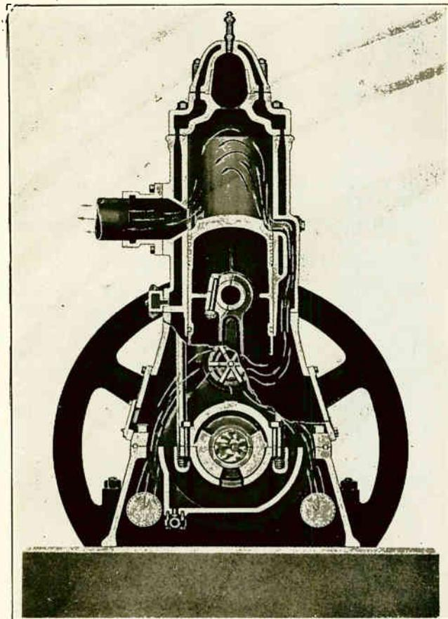
Fig. 21. Sectional view of a two stroke, two port Diesel engine clearly showing the path of the air and exhaust gases. (Courtesy of the Ven-Severin Company.)
