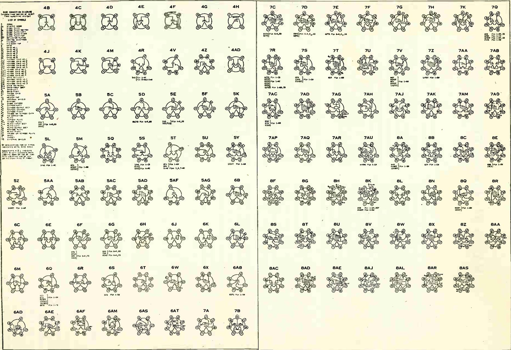
Fig. 100A. Tube base chart. (Courtesy Raytheon Mfg. Co.)
