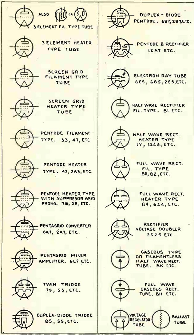
Fig. 49. Radio vacuum tube symbols.
