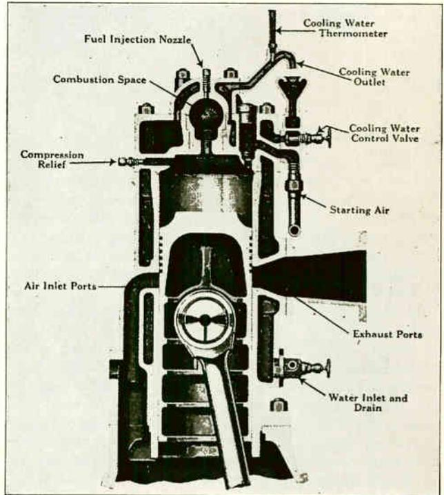
Fig. 130. Sectional view of a Diesel engine showing the piston on its down stroke and the connecting rod at an angle. Note how this would cause the piston to be forced against the left hand side of the cylinder, increasing wear at this point during the power stroke. Courtesy Fairbanks Morse Co.
