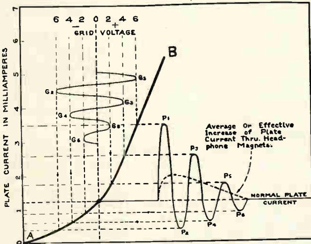
Fig. 64. Curves showing the manner in which the signal voltage of a damped wave train is applied to the grid of a tube, and is both amplified and rectified in the resulting plate current impulses. Study this action carefully in the accompanying paragraphs.
