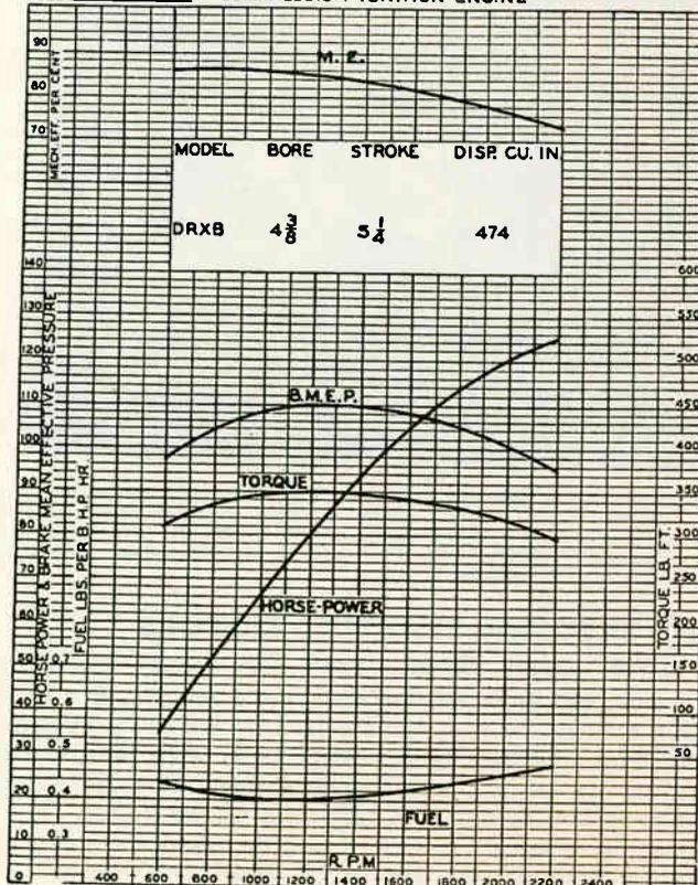
Fig. 72. Curves showing h.p., torque, efficiency, and fuel consumption, per h.p. hour, for a 6 cylinder Hercules engine. Note that the h.p. increases with the speed, and also that the fuel consumption per h.p. hour is less at speeds between 1000 and 1200 R.P.M.
