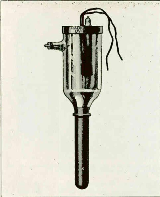
Fig. 52. A 10 Kw. water cooled transmitter tube.
