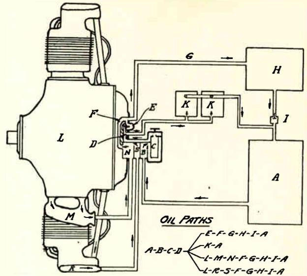
Fig. 156. The above diagram shows the lubricating oil system and units used with the Guiberson radial Diesel engine.
