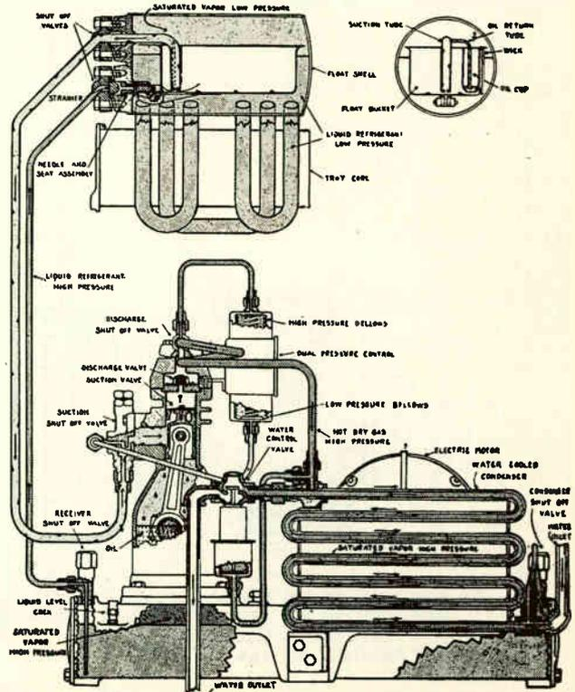
Fig. 28. Cycle diagram of a Servel unit using a flooded evaporator, low side float valve, and water-cooled condenser with a water flow control valve. Courtesy Servel Corp.
