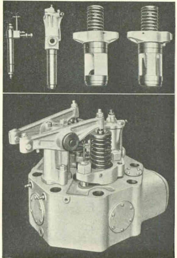
Fig. 139. In the lower view is shown a removable cylinder head which is equipped with removable valve cages and assemblies. In the upper view are shown in order from left to right, the fuel valve, starting air valve, intake and exhaust valves as they appear when removed from the cylinder head shown below.
