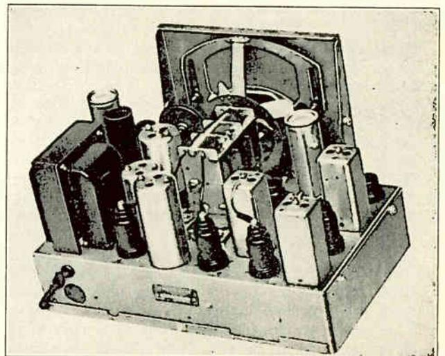
Fig. 194. This view shows the chassis of a radio receiver and illustrates how the serviceman can easily get at the tubes, R. F. and I. F. transformers, tuning condenser and tuning mechanism, and the power transformer. To reach the resistors, condensers and circuit connections on the under side of this set, the chassis must be removed from the cabinet and turned on its side or up side down.
