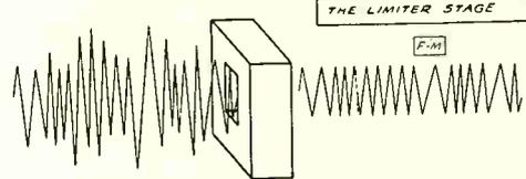
THIS FIGURE SHOWS IN PICTORIAL FORM HOW THE LIMITER FUNCTIONS TO SMOOTH OUT THE AMPLITUDE VARIATIONS IN THE FREQUENCY MODULATED SIGNAL.
