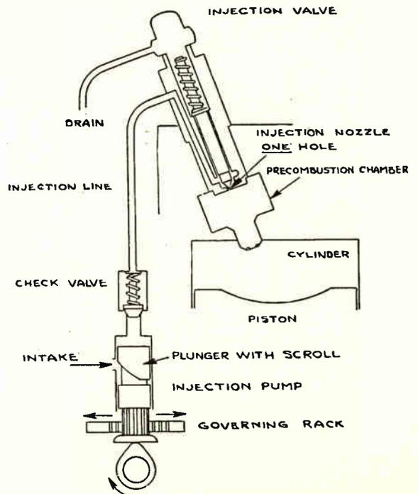
Fig. 32. This sketch shows a simple cylinder Bosch constant stroke, variable discharge fuel pump, with check valve, injection nozzle, pre-combustion chamber, and drain line. Refer to this figure often while reading the accompanying explanation. (Courtesy United American Bosch Corp.)
