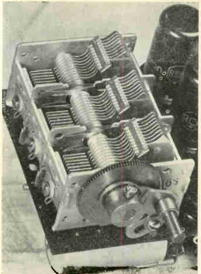
Fig. 35. Modern tuning condenser of three-gang variety. Gears on shaft permit finer tuning and prevent slipping.
