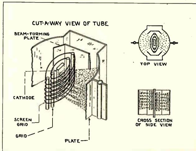
Fig. 87. Diagrams showing several views of a beam power tube in which electron streams are concentrated in beams to obtain high efficiency and high power output with low secondary emission.
