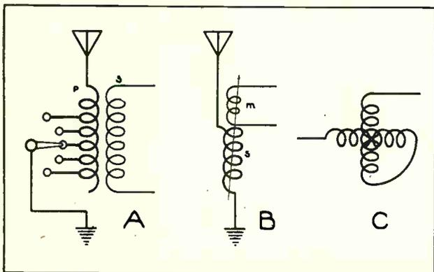
Fig. 37. The above three sketches show different methods of tuning radio circuits with various inductances.
