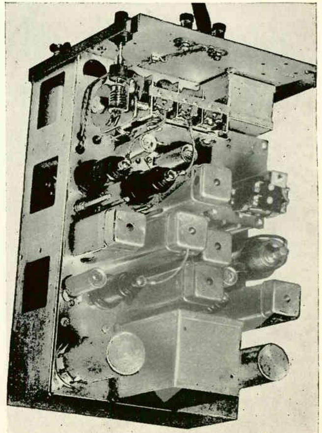
Fig. 101. The modern receiver chassis is built to last for many years. All coils are enclosed in metal shield cans to isolate them from stray fields that are set up by other parts and circuits.
