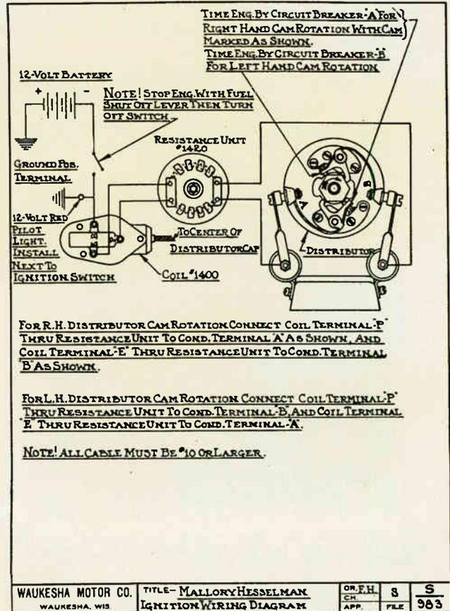
Fig. 92. Ignition wiring diagram for Waukesha Hesselman fuel oil engine. Note the printed instructions for timing and stopping this engine. (Courtesy Waukesha Motor Co.)
