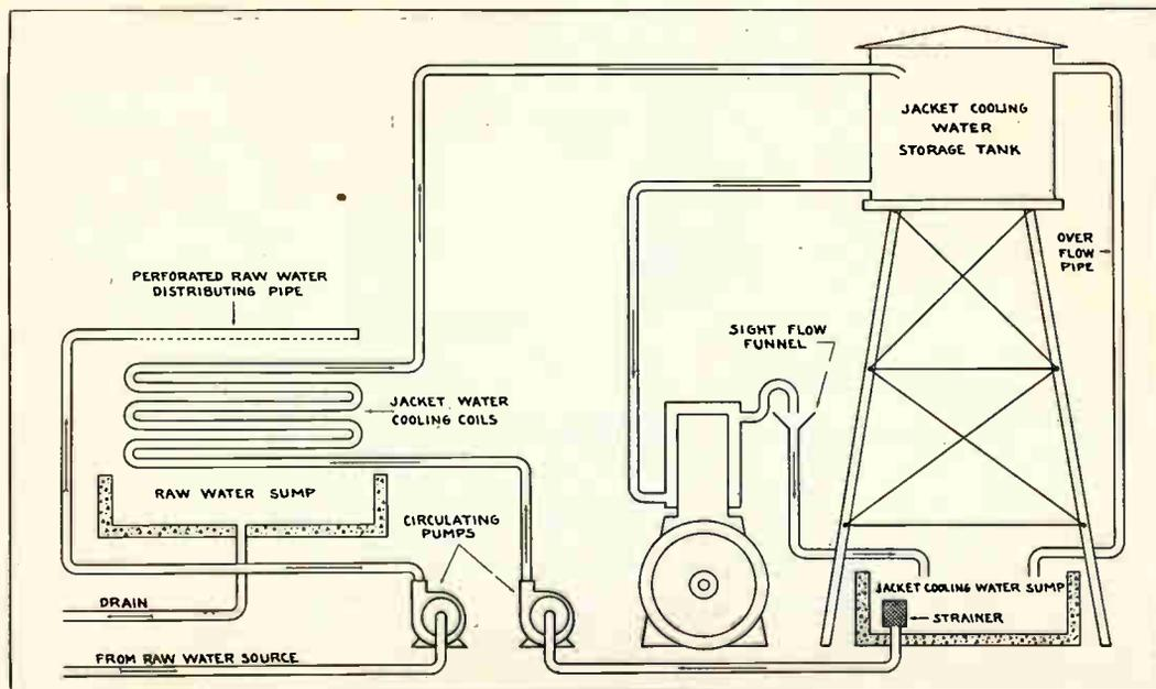
Fig. 112. Diagram showing the water tank, piping, pumps, and arrangement of a double flow, closed type cooling system for a Diesel power plant.
