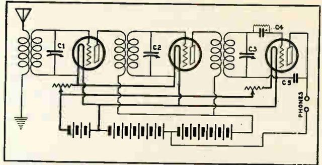
Fig. 107. Circuit diagram of a three tube receiver using two stages of R. F. (radio frequency) amplification and a detector.
