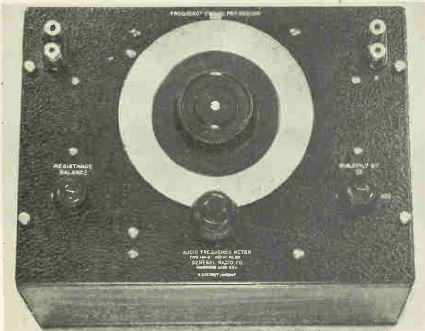
Portable laboratory frequency meter—20 to 20,000 cycles.
