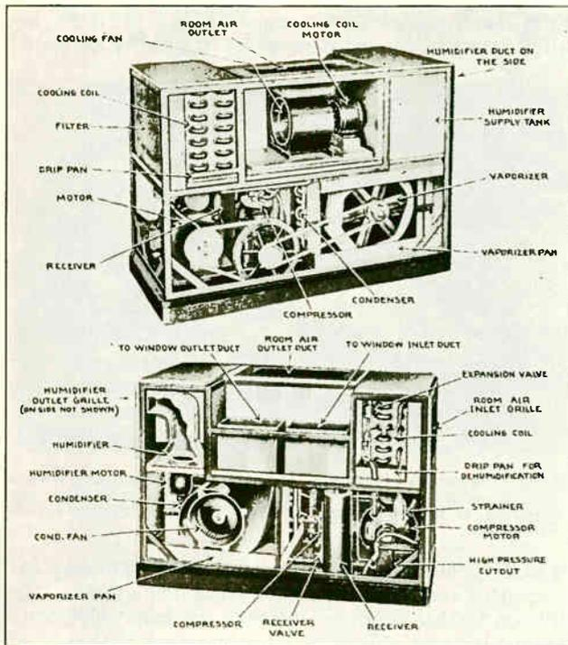
Fig. 145. Two excellent views of a room cooler unit with cover removed to show all working parts. Note the location and names of all the parts as marked on the photos. Courtesy Pacific Mfg. Corp.
