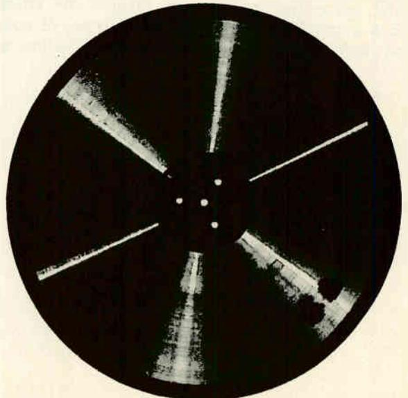
Shiny disc is properly cut. Dark sections are the results of "skipping", or low spots.
