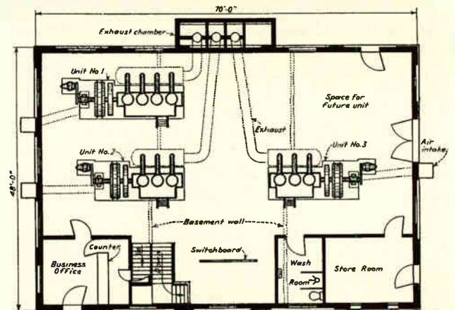
Fig. 95. This diagram shows the layout of a Diesel-Electric power plant with 3 engines driving electric generators. Note the arrangement of the exhaust and air intake pipes. (Courtesy Diesel Power Magazine.)
