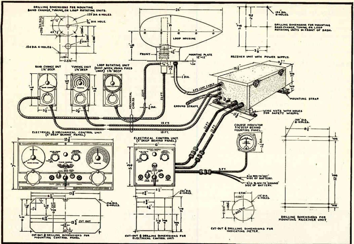
Here is the complete installation of a modern radio compass. The use of cables prevents interference to receiver.
