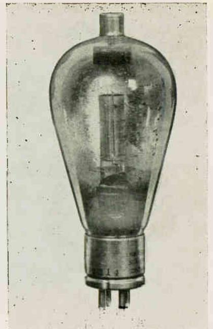
G-E Phanotron tube, type FG-32.
