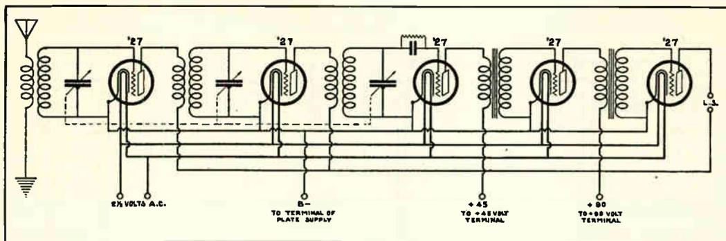
Fig. 140. Circuit diagram of a five tube A. C. receiver, using A. C. heater-element tubes. The "27" type tubes as shown above are used in both the R.F. and A.F. amplifiers and in the detector stage. Note the connections of the cathodes of the heater-element tubes to the B— terminal.
