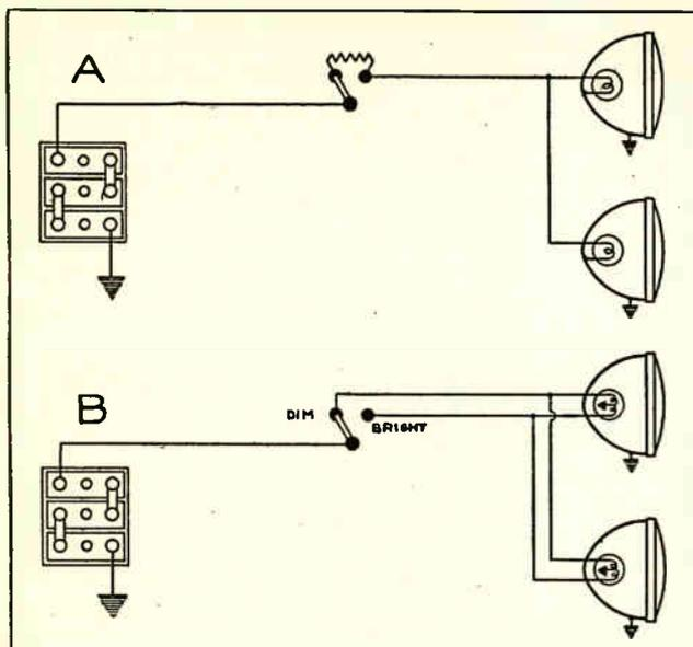
Fig. 84. A. Diagram showing resistance method of headlight dimming; B. Double filament method of a dimming or "dropping" headlight beams.
