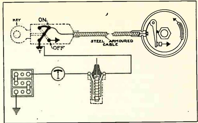
Fig. 43. The above sketch shows the primary ignition circuit through a special ignition lock switch and cable. Study the principles of this circuit carefully while reading the accompanying explanation.
