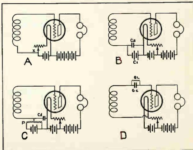
Fig. 65. The above sketches show four common methods of biasing the grid of a vacuum tube with a low negative potential.
