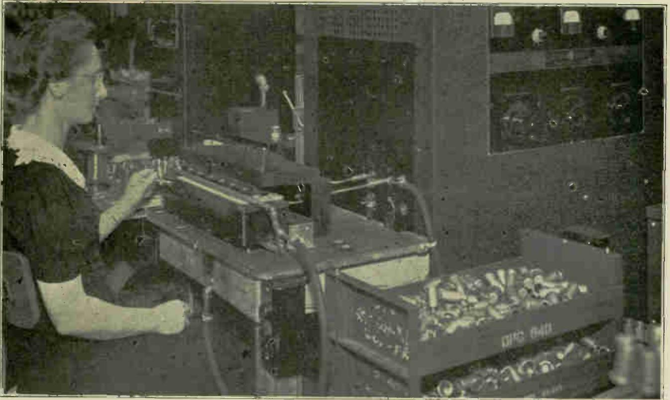
5-KW Power Oscillator, with fixture for soldering crystal shells in closed position, operator ready to throw "wipe" lever.
