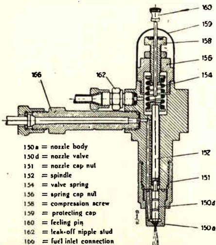
Fig. 45. Sectional view of Bosch fuel injection nozzle, nozzle holder and valve, showing pintle valve in open position. Refer to this figure and the numbered parts while studying the explanation in the lesson. (Courtesy United States American Bosch Corporation.)
