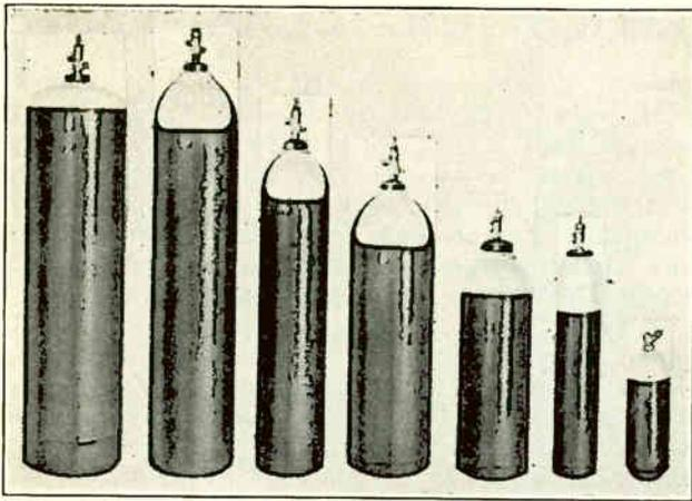
Fig. 59. Several types and sizes of metal cylinders or drums which are used for shipping and handling refrigerant chemicals.
