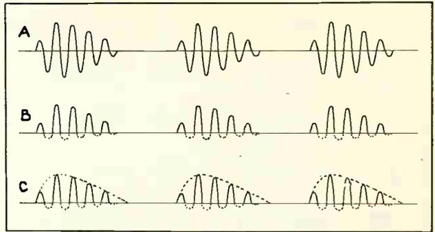
Fig. 45. The curve at A represents the alternating current induced by damped wave-trains striking an aerial. At B is shown the curve for this energy after it has been rectified into pulsating D. C. by the crystal. At C the large dotted curves illustrate how each group of pulsations supply one current impulse to the headphones.
