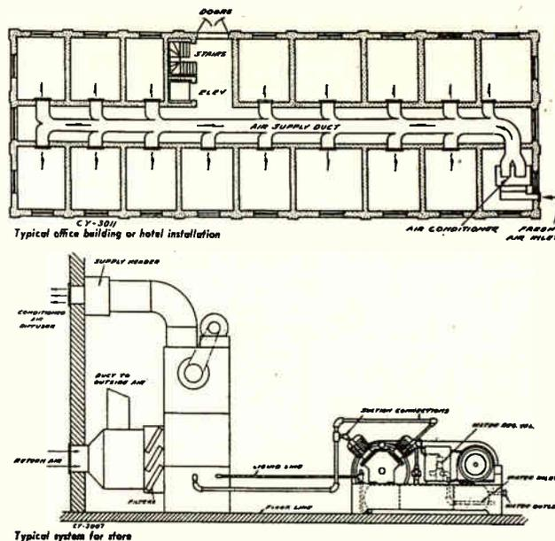
Fig. 168. Top diagram shows duct layout for distributing conditioned air to a group of small offices. Lower diagram shows the air-conditioned unit and refrigerating compressor and condenser for a store or office. Courtesy Carbondale Machine Corp.
