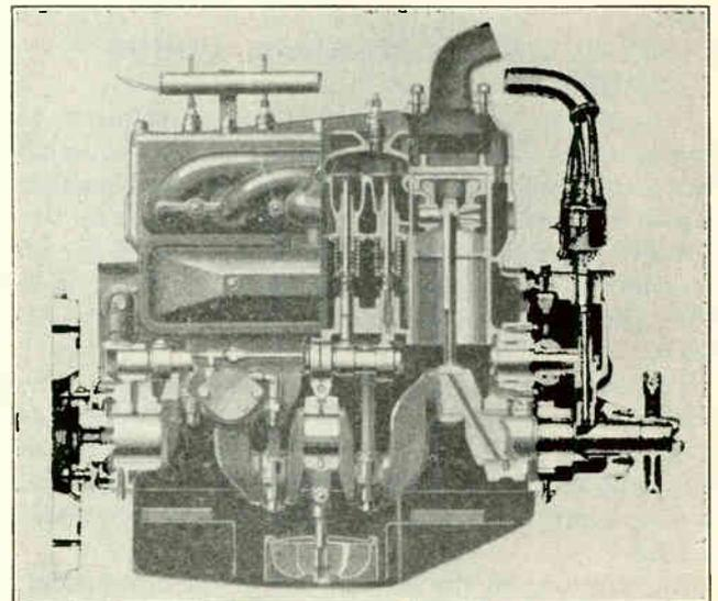
Fig. 12-A. Side sectional view of Chrysler Plymouth four-cylinder engine showing the shape of the crank shaft and arrangement of pistons, valves, etc.
