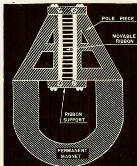
The velocity microphone employs a permanent magnet and ribbon.
