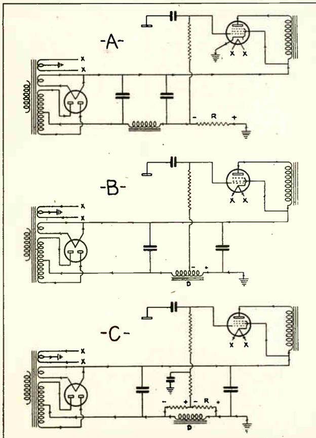
Fig. 74. Circuits showing three additional methods of obtaining grid bias voltage for amplifier tubes.
