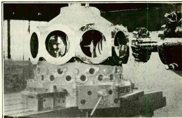
Fig. 152. Complete crankcase in process of machining. Note large openings to which cylinders will be attached and small openings for valve rods and fuel pump barrels.
