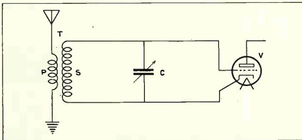
Fig. 36. A simple radio frequency tuning circuit.
