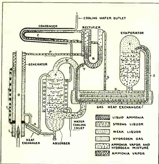
Fig. 66. This diagram clearly illustrates the operating principles of the Electrolux absorption type refrigerator. Carefully study and check each part of the cycle as explained in the accompanying instructions.
