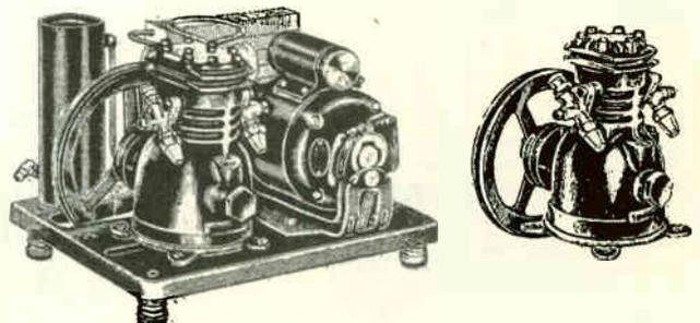
Fig. 85. Separate compressor or complete condensing units such as shown above can be purchased from refrigeration supply houses for use by the serviceman in replacing defective units in domestic refrigerators. This permits the old units to be taken out and serviced in the shop at leisure without tying up the customer's refrigerator.
