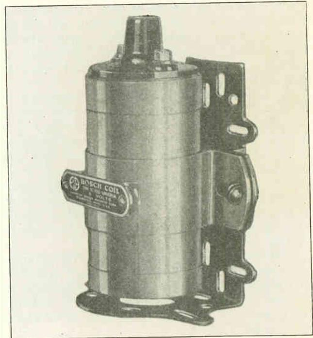
Fig. 22. High-tension ignition coil such as used for supplying high voltage impulses to the spark plugs on the ignition systems of automobiles. The heavy insulated bushing on the top of the coil is where the high voltage lead connects.
