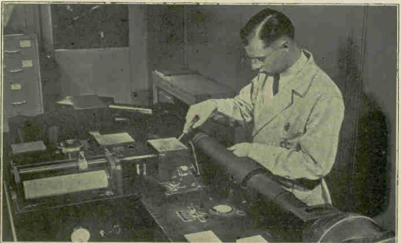
A recording spectrophotometer, a high precision instrument widely used in the paper, textile, chemical and paint industries for analyzing quality and color of product.
