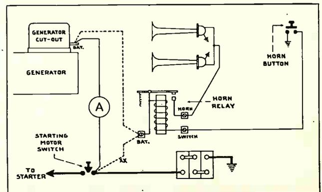
Fig. 88. Diagram of a horn relay circuit.
