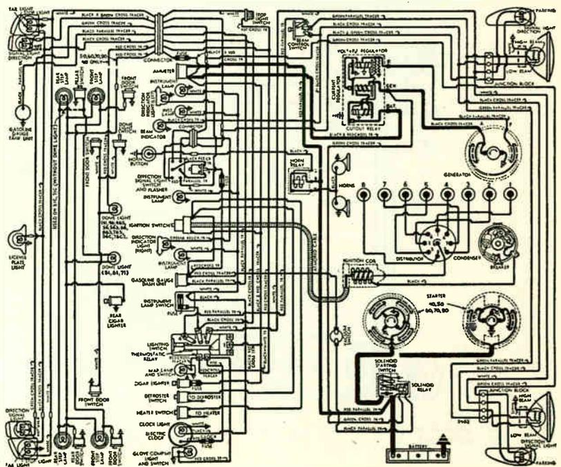
Fig. 92. Wiring diagram of a 1941 Buick car. Examine the light wiring, ignition wiring and the generator, starter and horn circuits.
