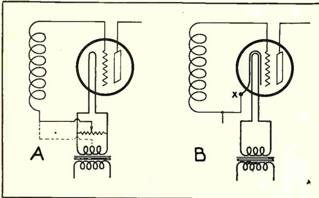
Fig. 78. At A is shown a vacuum tube using A. C. to heat the filament, and having grid return lead connected to the center of a potentiometer. At B is shown an A. C. heater-element type tube using A. C. for the filament and having a separate cathode which is heated by the filament.
