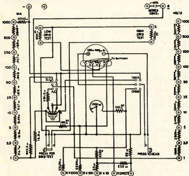
Fig. 207. Circuit diagram of a convenient portable radio analyzer, showing the connections of the meter, rectifier, pin jacks and resistors for checking various voltages, currents, and resistances on a radio receiver. Courtesy Weston Electrical Instrument Company.
