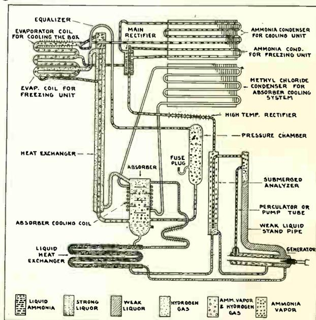
Fig. 67. Cycle diagram of an air-cooled absorption type refrigerator. Note that the absorber in this unit is cooled by methyl-chloride instead of by running water as in the preceding unit.
