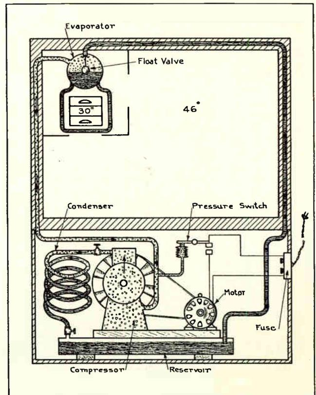
Fig. 21. This diagram shows the circulation of the refrigerating solution throughout the machine, and also illustrates the general principles of the mechanical refrigeration cycle.
