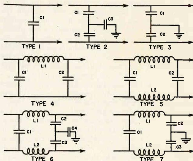
If the appliance to be silenced is a hand held instrument, or if the user is apt to come in contact with grounded metal while touching the appliance frame, it is advisable to employ a filter utilizing a third condenser as shown in the diagram of the Type 2 filter. This third condenser eliminates any possibility of the appliance operator receiving a mild shock, although it slightly reduces the filtering effect of the unit.
