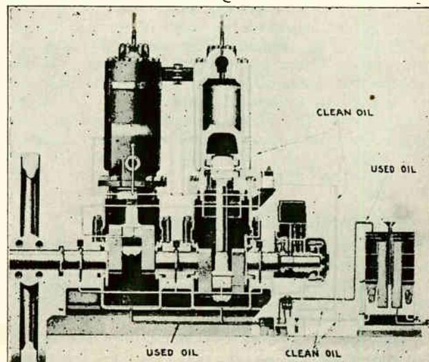
Fig. 124. Sectional view of a heavy duty two cylinder Diesel engine showing the path of the clean oil from the filter, through the oil pump to the engine bearings and also the path of the used oil from the crank case back through one section of the pump, to the filter. (Courtesy Fairbanks Morse Co.)
