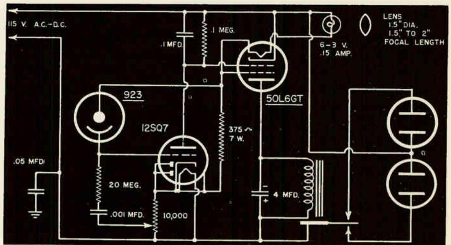
Experimental grid-controlled relay unit.
