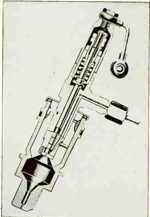
Fig. 59. Injection nozzle and pre-combustion chamber of Caterpillar Tractor Diesel Engine. Note that this pre-combustion chamber is attached right to the end of the injector nozzle, and has a rather small opening which somewhat restricts or slows down the discharge of partly burned fuel to the cylinder.
