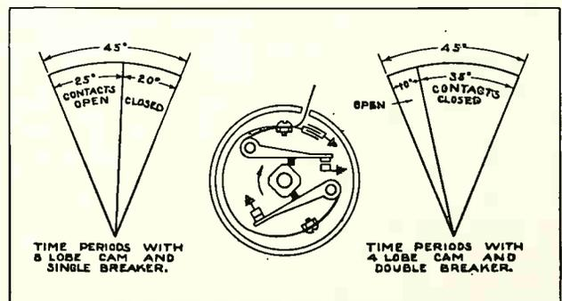
Fig. 41. Diagram showing construction of breaker mechanism for high-speed distributor and also showing periods of time which contacts remain open and closed with both single and double breaker distributors.
