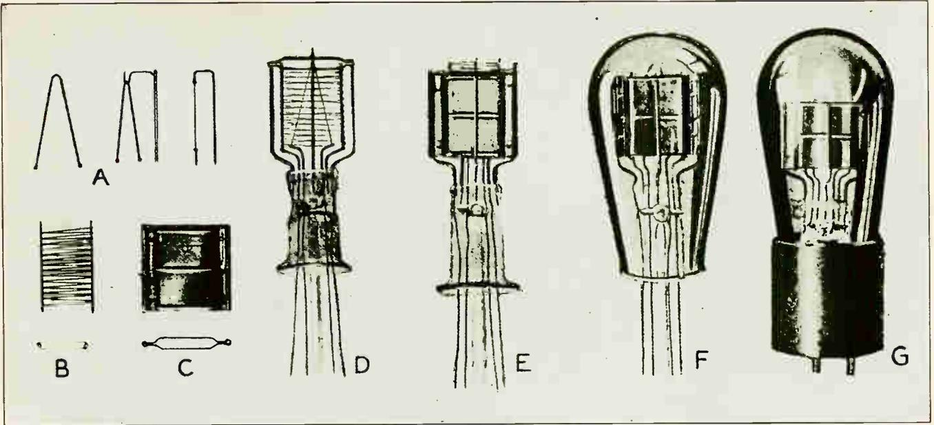
Fig. 54. The above views show the various parts of a vacuum tube and illustrate the manner in which these parts are assembled and mounted in the complete tube. Refer to these views frequently while reading the accompanying paragraphs.
