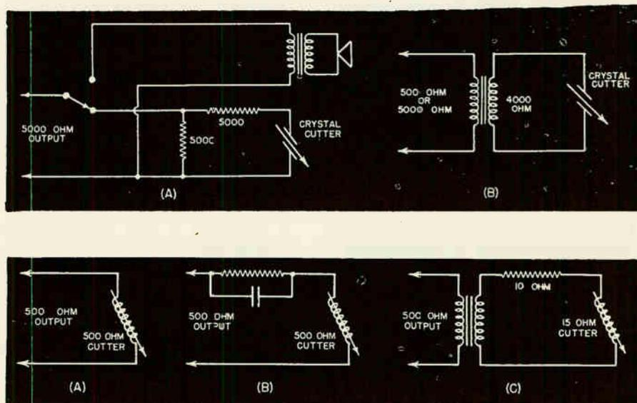
How to connect both crystal and magnetic cutters to amplifier output terminals.
