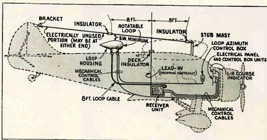
Installation of loop placed on top of planes fuselage.
