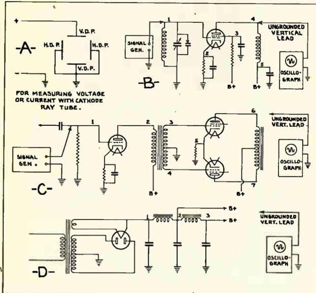
Fig. 255. Above are shown various methods of connecting the deflector leads of an oscilloscope to the different parts of a radio receiver circuit for testing the gain at each stage, for checking tubes and condensers, for locating distortion in the radio receiver, and for checking A.C. ripple in the power supply.
