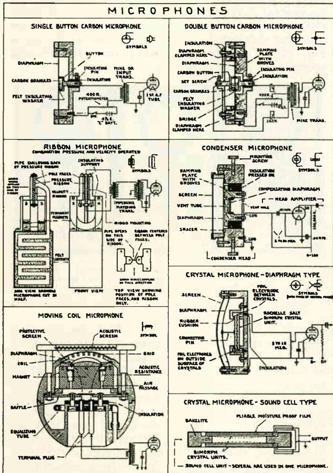
Fig. 243. The above sketches show the construction and connections of carbon, condenser, crystal, and ribbon type microphones. Study each view carefully while reading the accompanying explanations.
