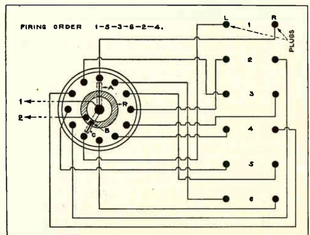
Fig. 39. Diagram showing distributor rotor arms and high voltage leads from the distributor cap to the spark plugs of a six-cylinder engine with a dual ignition.
