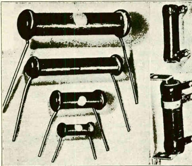
Fig. 151. Several composition type resistors of 2 watt, 1 watt, 1/2 watt, and 1/8 watt sizes on the left; and two wire wound resistors on the right.
