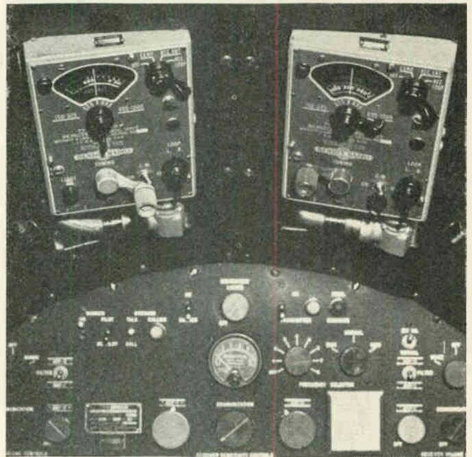
Dual instrument installation in modern airliner of radiocompass.
