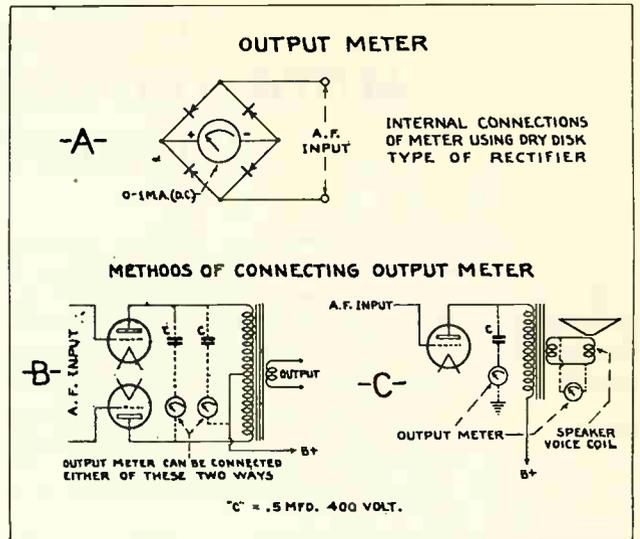
Fig. 171. At "A" are shown the connections of an output meter and its rectifier. At "B" and "C" are shown methods of connecting output meters to receivers when aligning "supers."
