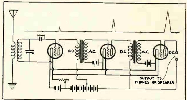
Fig. 70. Circuit diagram of a simple 3 tube receiver with one tube used as a detector and two as amplifiers. Note how the signal strength is increased by each tube.
