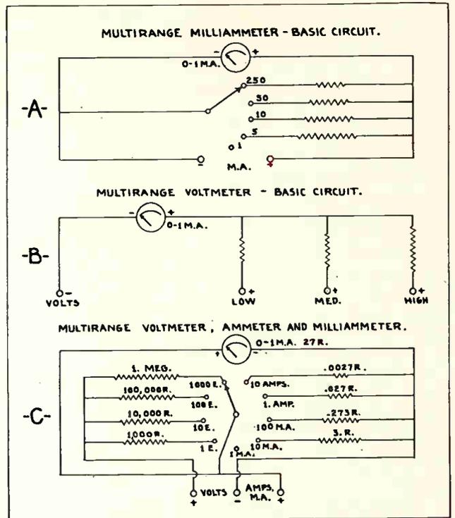
Fig. 203. The above diagram shows the wiring and connections for a multi-range milliammeter, voltmeter and a combination voltmeter, ammeter and milliammeter, such as commonly used for radio service tests.
