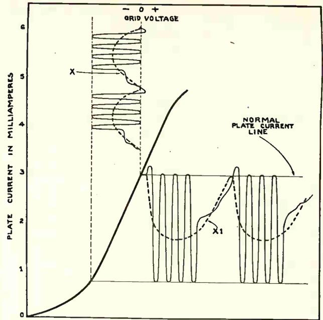
Fig. 67. Curves illustrating detector action of a tube using a grid leak and condenser to obtain maximum rectification with plate current impulses falling below normal plate current.
