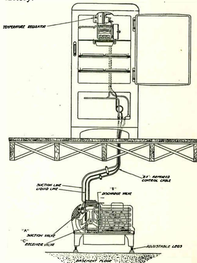
Fig. 70. Diagram showing the method of installation of a refrigerator with a condensing unit located in the basement some distance from the cabinet.
