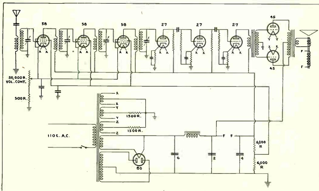
Fig. 149. Circuit diagram of a 9 tube tuned Radio Frequency A.C. receiver, using three stages of T. R. F. amplification, power detector, two stages of resistance coupled A. F. amplification, and one stage of push-pull audio amplification. Trace all of the above circuits carefully.
