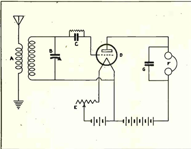
Fig. 102. A simple one tube Radio receiving circuit.
