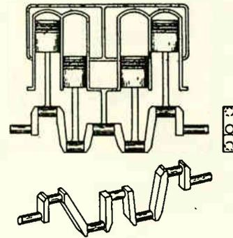
Fig. 12. Sketch showing the design of the crank shaft and arrangement of pistons in a four-cylinder engine.
