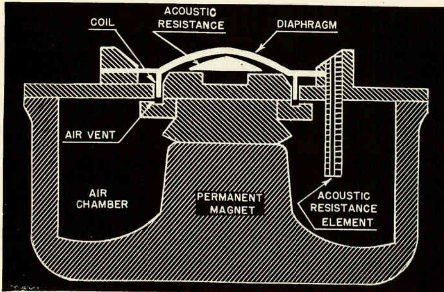
Cross-section of dynamic microphone used in practically all broadcasting stations.
