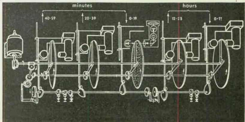
Block diagram of the photoelectric time-telling device.
