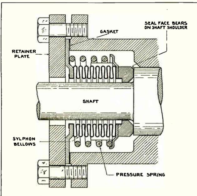
Fig. 39. Carefully examine all details of the slyphon bellows type shaft seal shown in the above diagram. This type of seal is extensively used in domestic type refrigerators.
