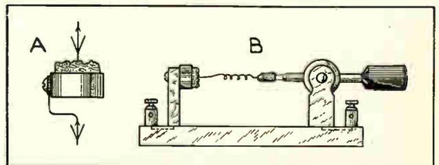
Fig. 43. The sketch at A shows a crystal and illustrates the rectifier effect on the current passing through it. At B is shown a complete crystal mounting with the crystal and cat-whisker in place.
