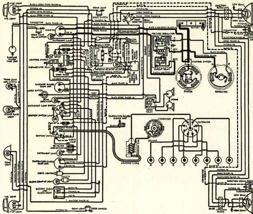
Fig. 93. Wiring diagram of a 1941 Pontiac. Note the code markings and trace each circuit carefully. Checking such circuits and visualizing their operation and possible troubles is a great help on actual trouble shooting jobs.
