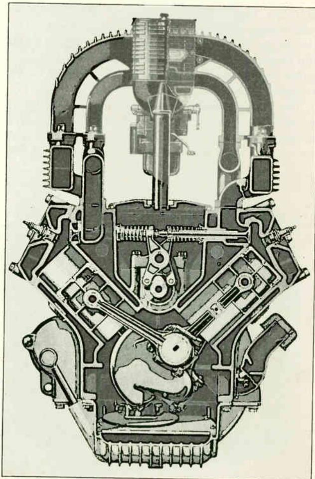
Fig. 20. An excellent end sectional view of a V-type, eight-cylinder engine. Note carefully the arrangement of the pistons, valves, cam shaft, rocker arms, spark plugs, carburetor and intake and exhaust manifolds. Courtesy Oldsmobile Mfg. Co.
