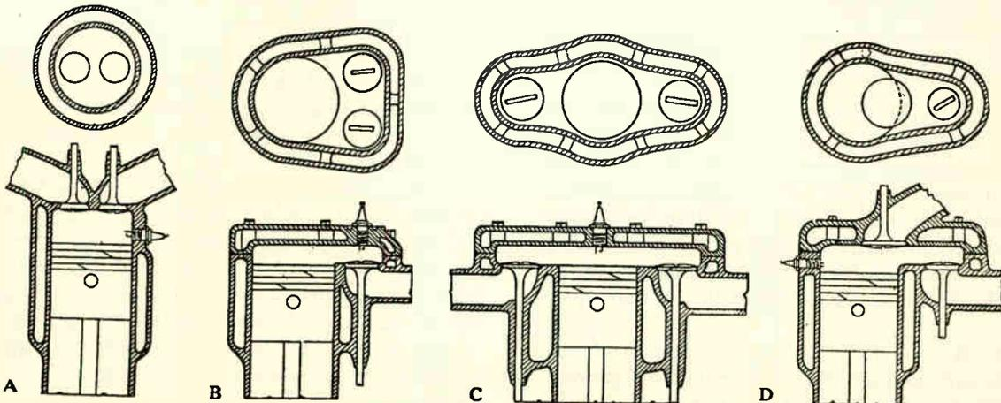
Fig. 8. The above diagrams show the location and arrangement of valves with respect to the cylinder in various types of automobile engines.
