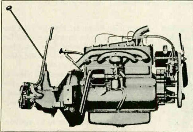
Fig. 11. Side view of a four-cylinder automobile engine used by the Chrysler Plymouth automobile. Note the position of the carburetor, intake and exhaust manifolds and spark plugs.
