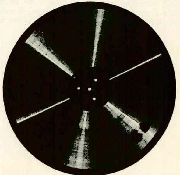
Shiny disc is properly cut. Dark sections are the results of "skipping", or low spots.
