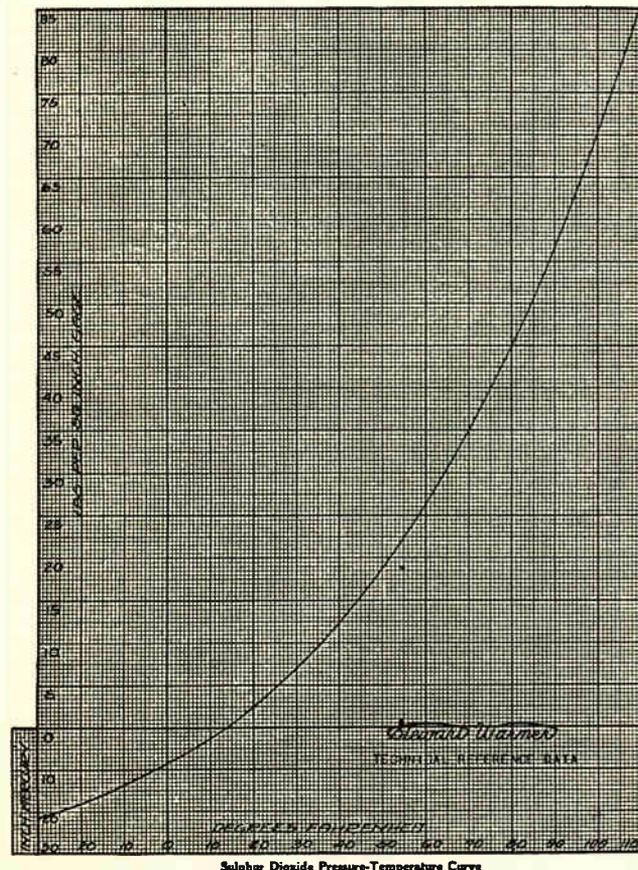
Fig. 15. Chart showing the boiling point of sulphur-dioxide (SO<sub>2</sub>) refrigerant at various pressures and vacuums. Refer to this chart often while studying about pressures and evaporation. Courtesy Stewart-Warner Corporation.
