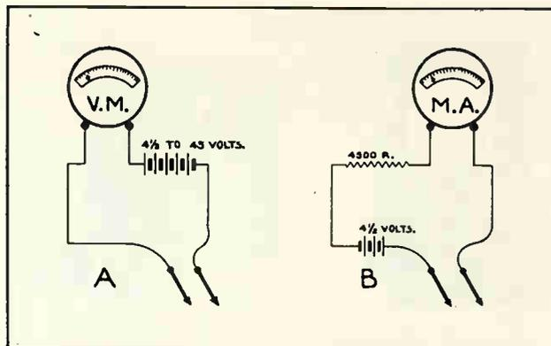
Fig. 196. The sketch at A shows the connections for using a low reading voltmeter for making continuity tests, and the one at B shows the connections for using a milliammeter for this purpose.
