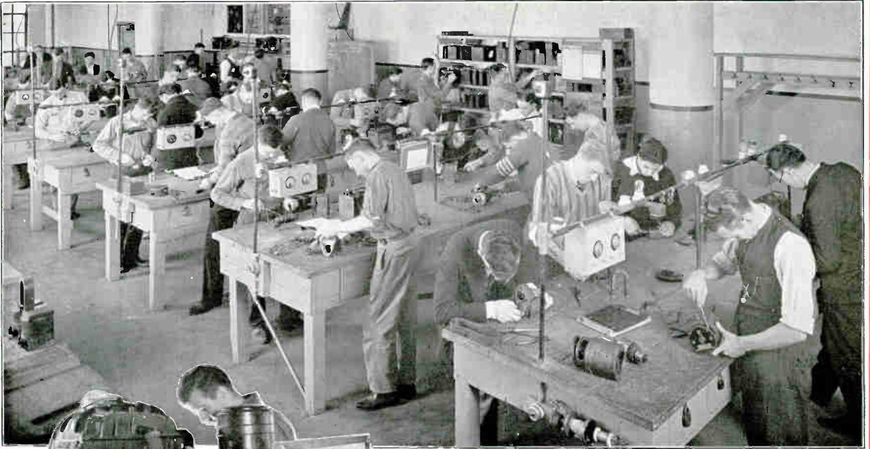
This section of our auto department shows some of the benches where you will overhaul, repair and test many types of generators, starters, ignition coils, magnetos, condensers, etc. You are trained to quickly find and fix their common troubles, and how to use the tools and test meters and devices to simplify this work.
