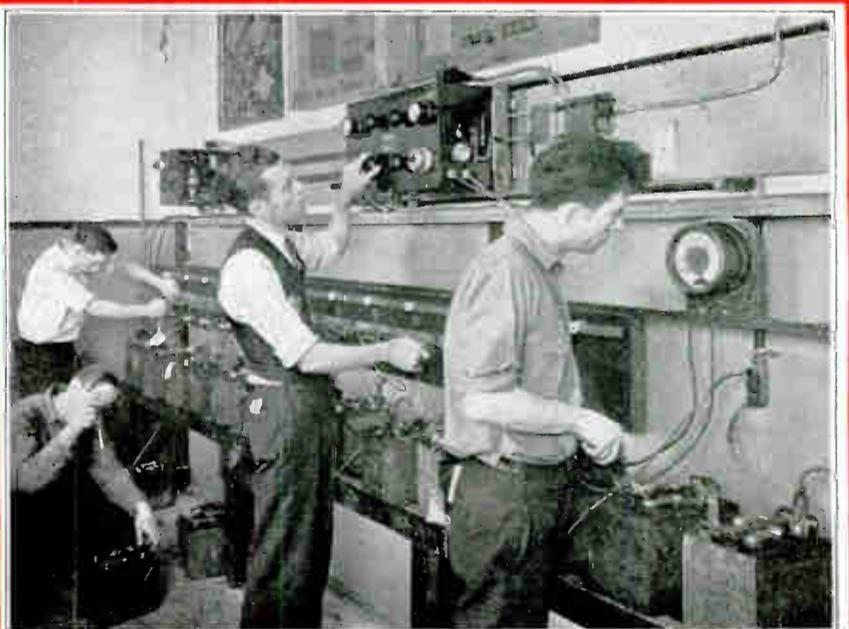
Here they are operating the charging line and equipment of the Tungar type. Both the half wave and later type full wave chargers are used here. And you see these students testing the acid, and the voltage to determine the exact condition of the batteries being charged.
