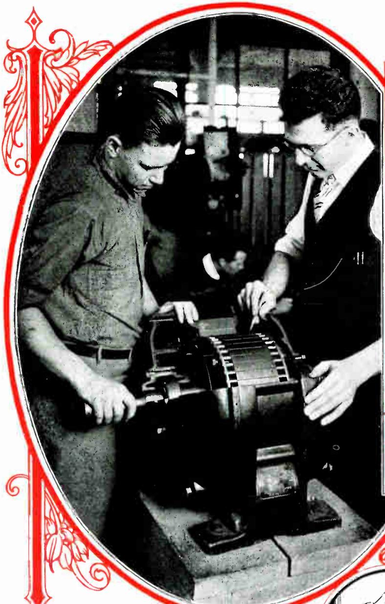
Here an instructor is explaining important principles of an induction motor, on a machine specially cut away, so the student can observe these points both while the motor is idle and when it is running. This is an example of how some of our specially prepared equipment will save your time, and quickly make its operation clear to you.
