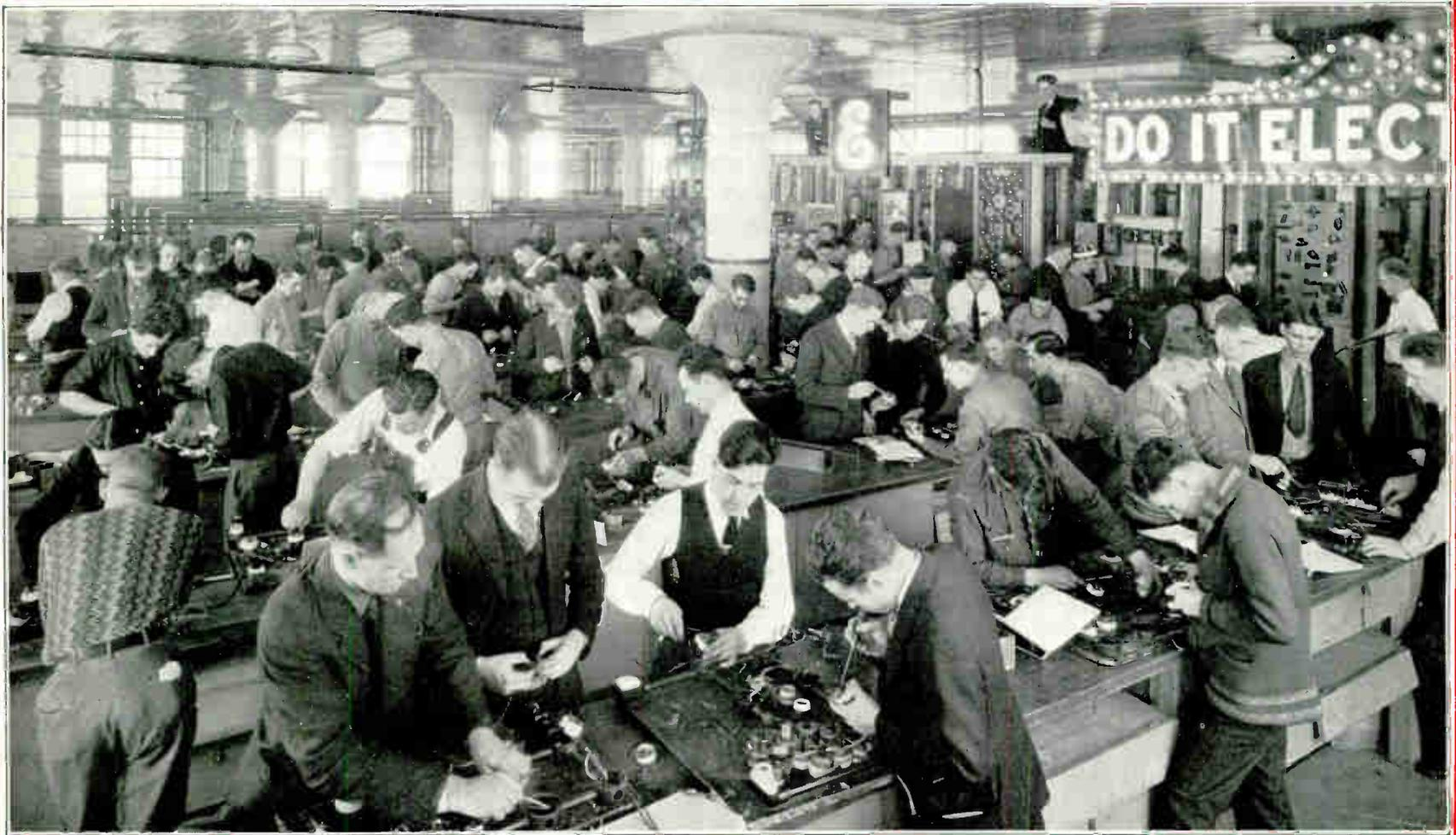
General view of a section of the electrical wiring department. Notice the large and well lighted shop. The men are wiring and testing light control circuits in their first small conduit layout, and getting real practical experience in the handling of tools and different kinds of switches.
