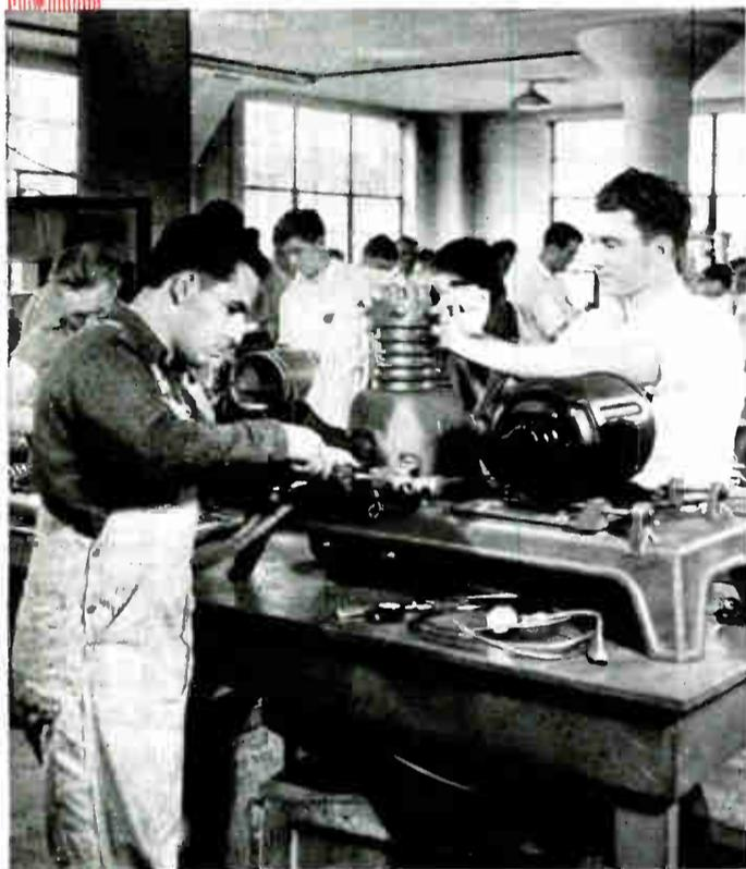
Coyne students assembling and checking a modern commercial refrigeration compressor for an ice cream machine.
