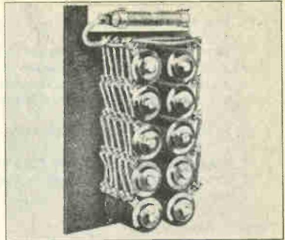
Fig. 11. Copper oxide rectifier consisting of a number of units connected in series and parallel to obtain increased voltage and current capacity.
