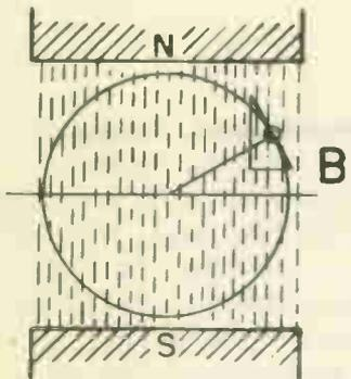
In diagram B, the conductor is moving through the field flux at an angle of  $30^\circ$  electrical and the rate of cutting lines of force has increased. Sketch B1 shows the effect of the changing direction of conductor motion, which has proved through this angle of  $30^\circ$ .
