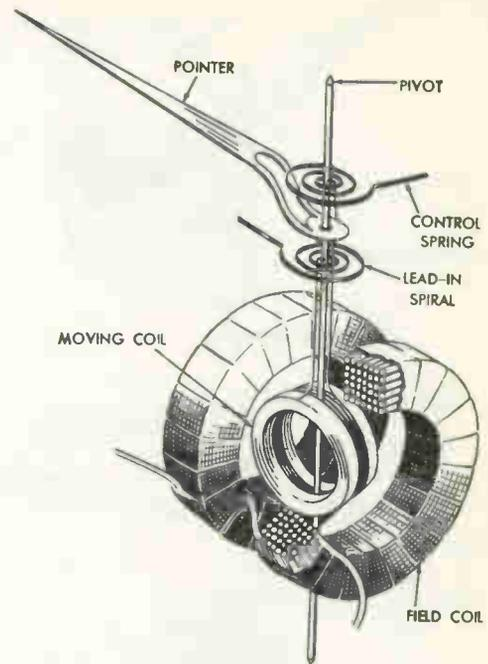
Fig. 9 Diagram of dynamometer mechanism
