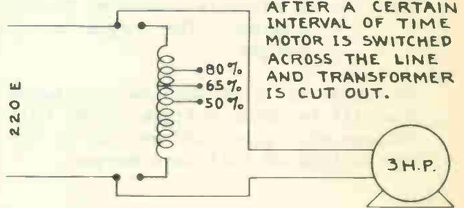
AFTER A CERTAIN INTERVAL OF TIME MOTOR IS SWITCHED ACROSS THE LINE AND TRANSFORMER IS CUT OUT.
