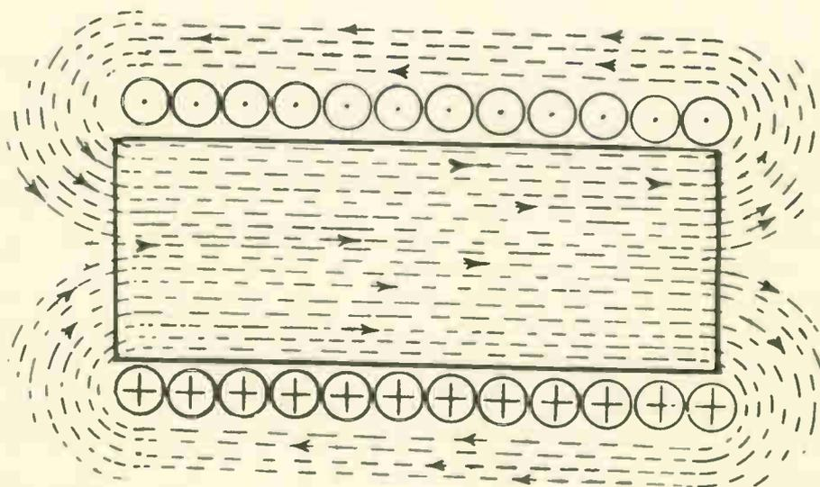
Fig. 6 A cross section of a single layer coil, tightly wound, and showing by diagram what happens as fluxes are added.
