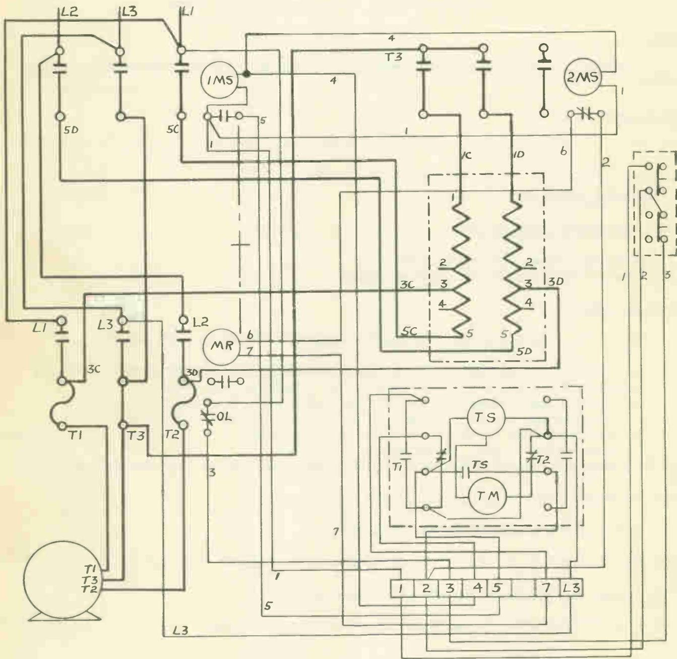
Fig. 1 Reduced voltage squirrel cage induction motor starter (Westinghouse)
