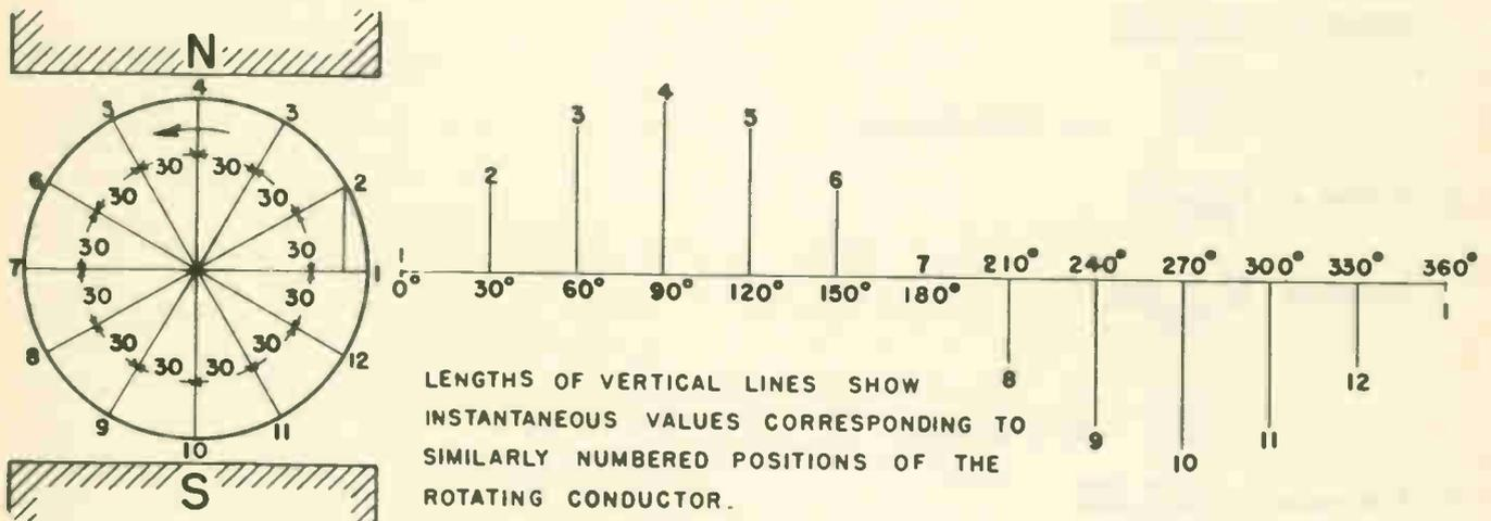
These values are based on the assumption that the conductor moves at constant angular velocity thru a magnetic field of uniform strength.
