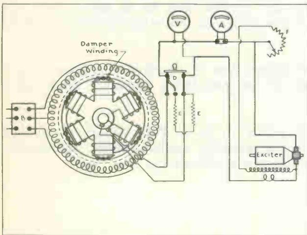
Fig. 5 The above diagram shows the connections for the stator and field of a synchronous motor and also the exciter-generator field discharge switch and instruments.
