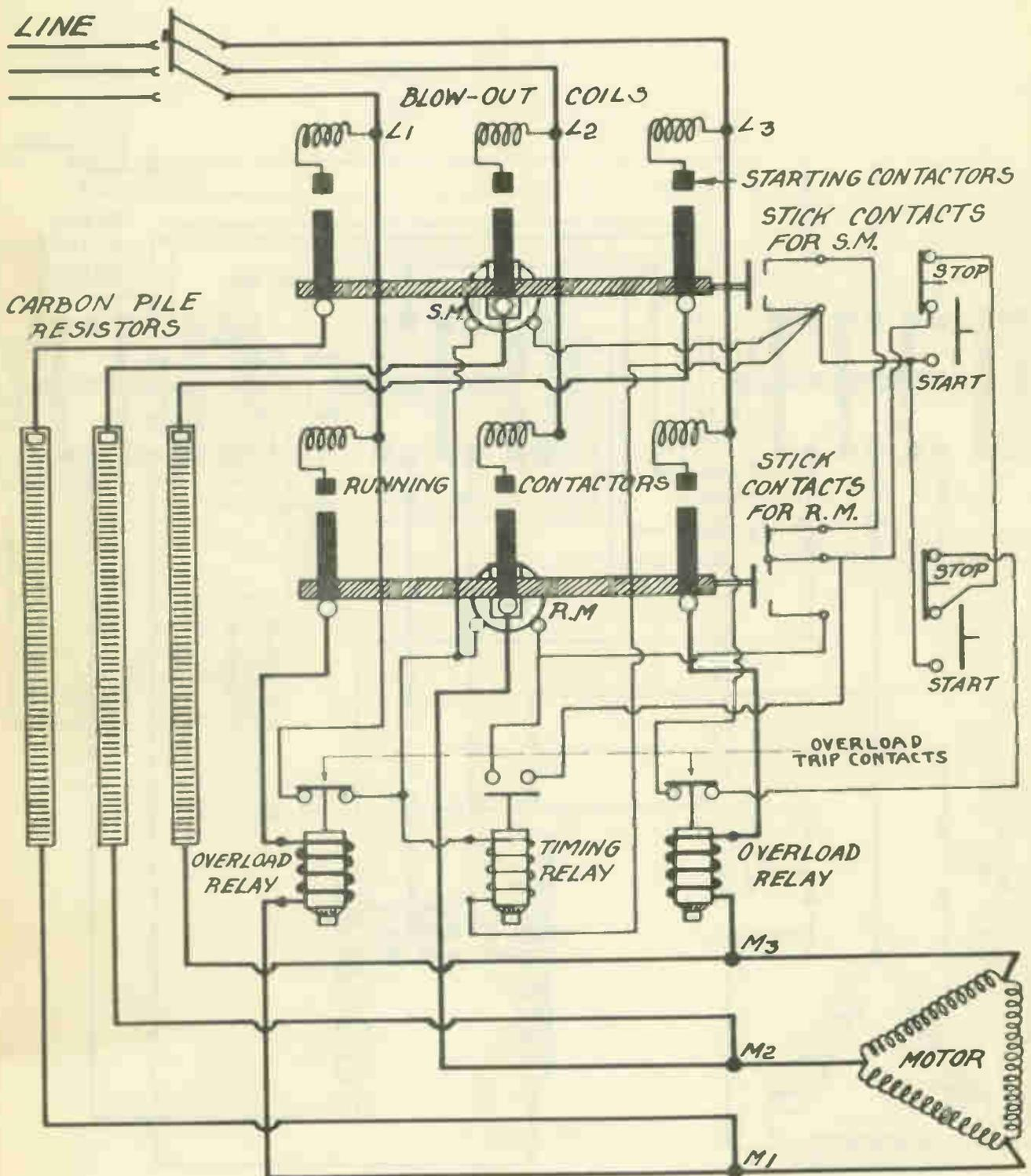
Fig. 3 Automatic resistance 3 phase starter
