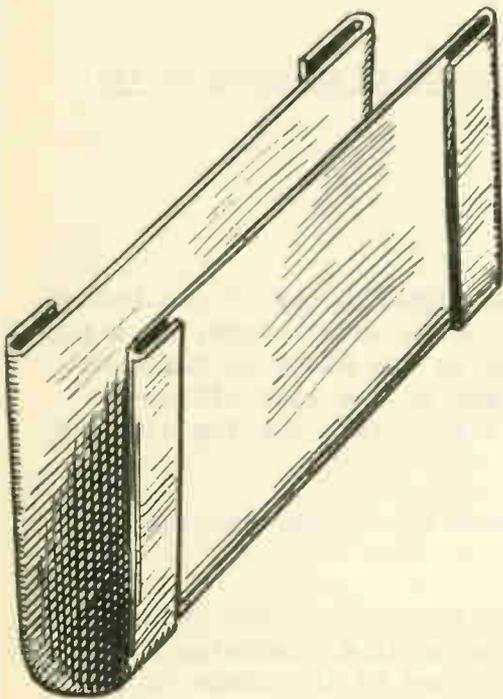
Fig. 2 - Slot insulation with cuffs
