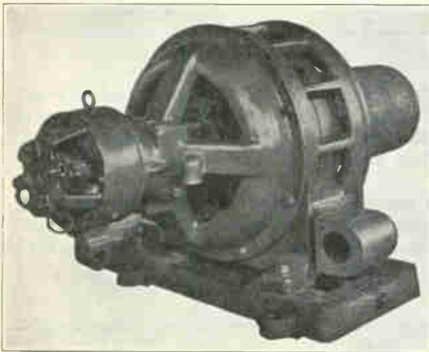
Fig. 1B This photo shows a 75 h. p. synchronous motor of the revolving field type. Note the small exciter-generator which supplies D. C. to the field of the large motor. (Photo courtesy General Electric Co.)
