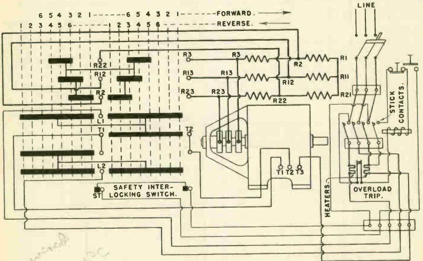
Fig. 2 Six position forward-reverse drum control for slip ring motors.
