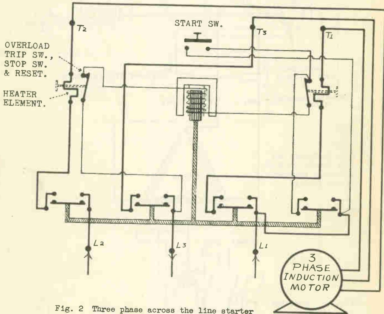
Fig. 2 Three phase across the line starter (Westinghouse)
