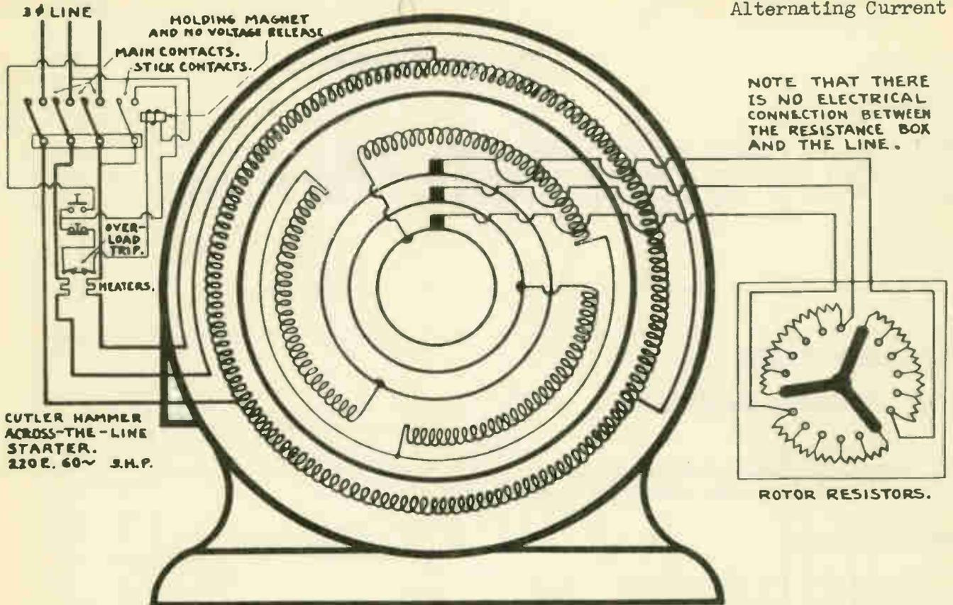
Fig. 1 Slip ring induction motor with Y-box
