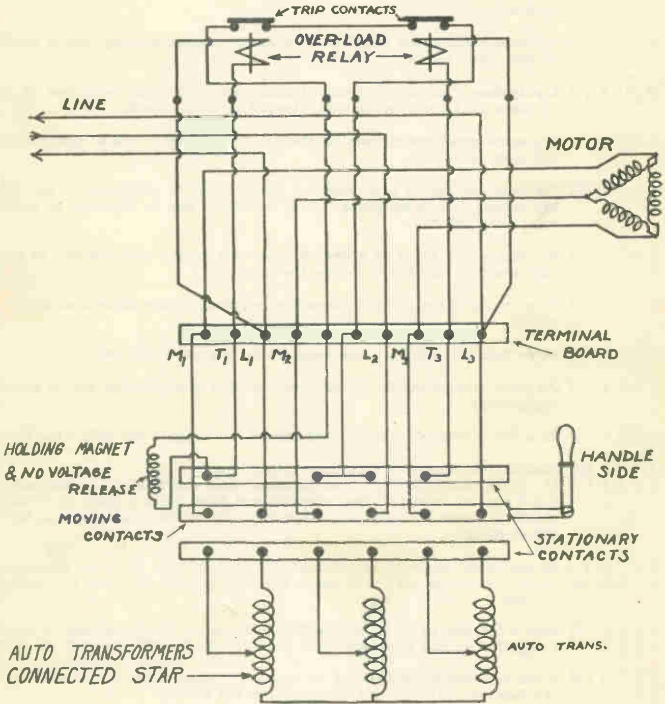
Fig. 2 Reduced voltage manual type starter for 3-phase motor equipment, 5-10 HP. (Western Electric)
