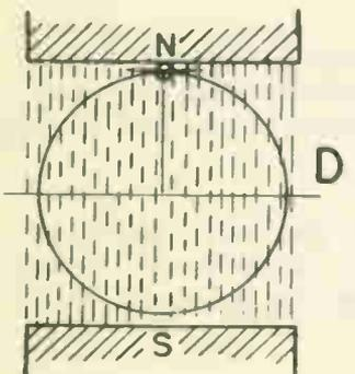
In Figure D, the conductor is moving at right angles to the field flux and is, therefore, cutting lines of force at the maximum rate. The induced voltage at this point in the rotation, therefore, is maximum because it has moved through  $90^\circ$  electrical.
