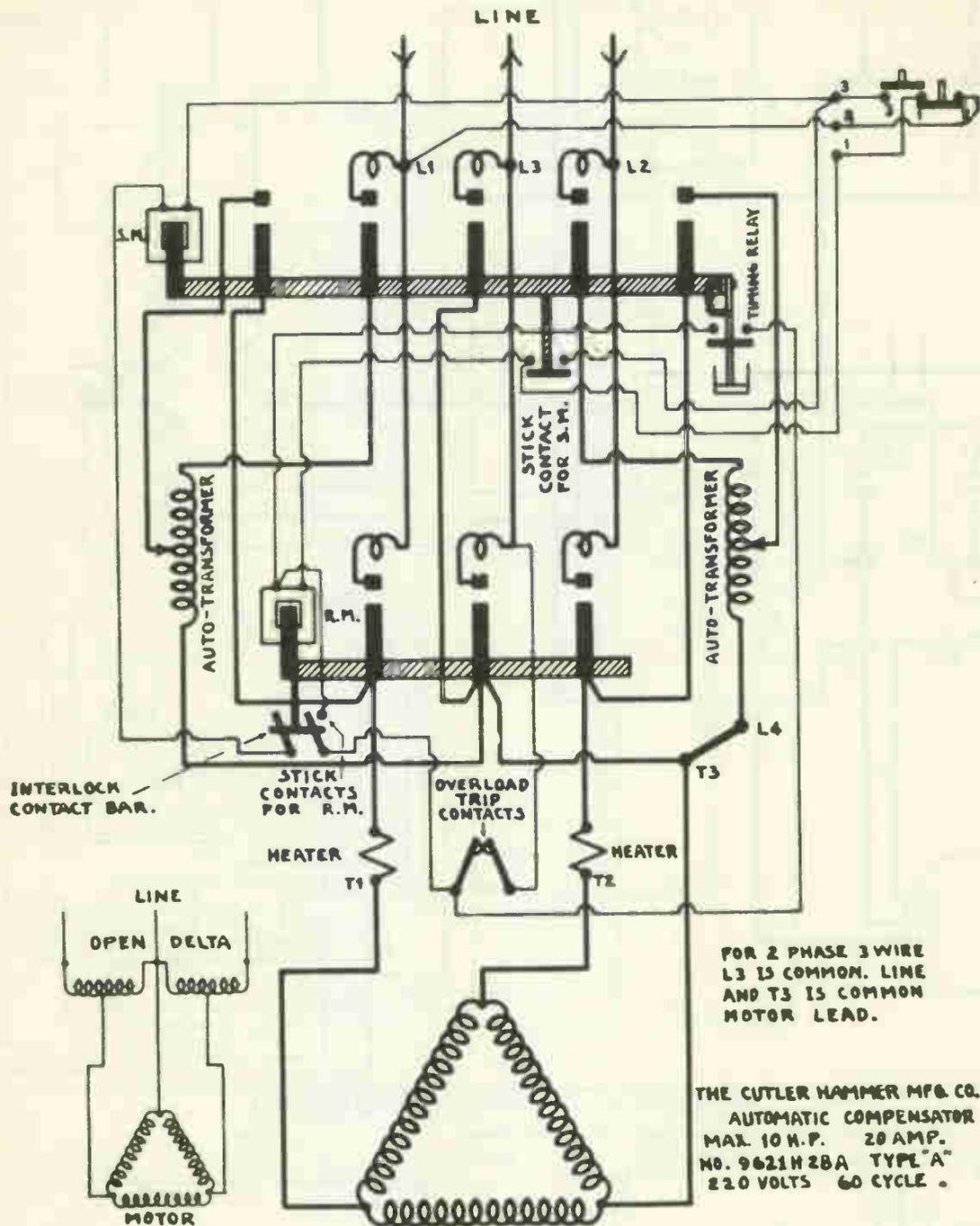
Figure 6. A Cutler Hammer Starter which is used for reduced voltage motor starting. Trace the following circuits:
