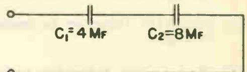
$$C_T = \frac{C_1 \cdot C_2}{C_1 + C_2} = \frac{4 \times 8}{4 + 8} = 2.67 \text{ Mf}$$
