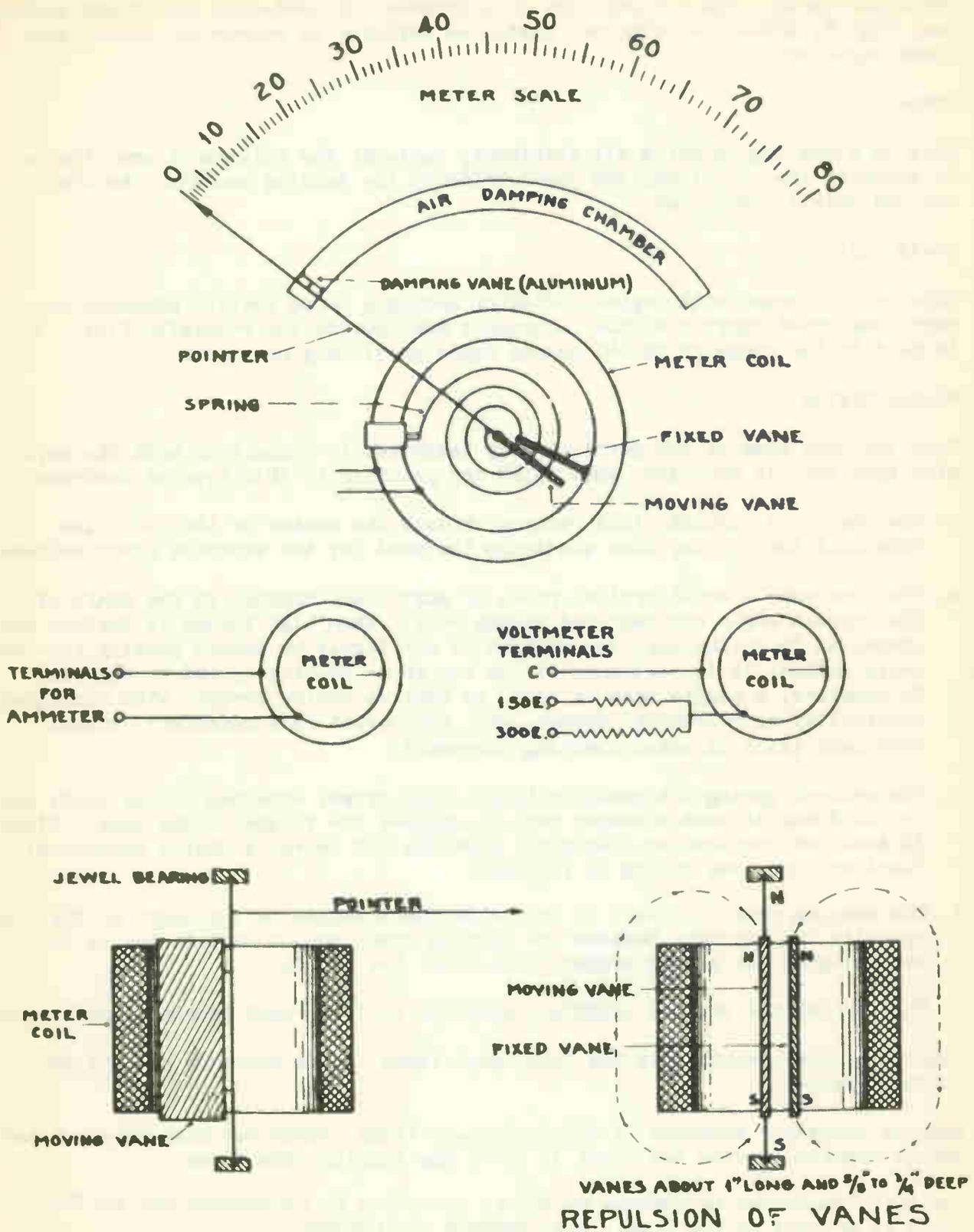
Fig. 1A. Moving iron type ammeter or voltmeter
