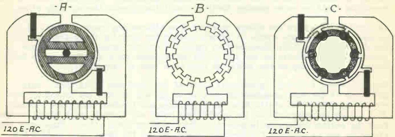
Fig. 1A Small synchronous motors
