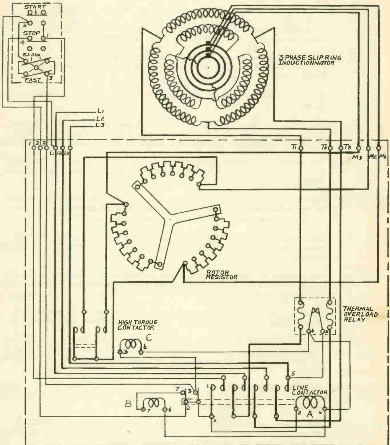
Fig. 3 Hosiery machine controller for 3-phase slip ring induction motor.
