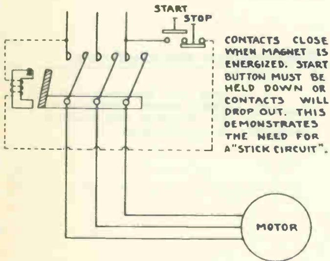
CONTACTS CLOSE WHEN MAGNET IS ENERGIZED. START BUTTON MUST BE HELD DOWN OR CONTACTS WILL DROP OUT. THIS DEMONSTRATES THE NEED FOR A "STICK CIRCUIT".
