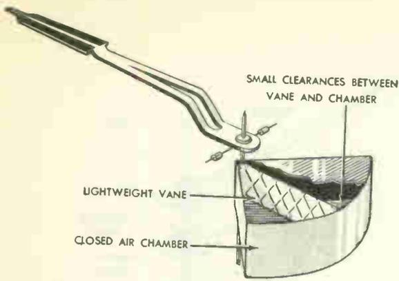
Fig. 5 Air-damping mechanism
