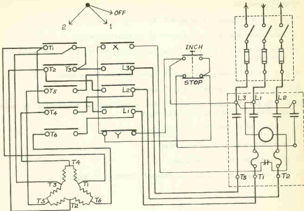
Two speed motor with drum control and inching control.
