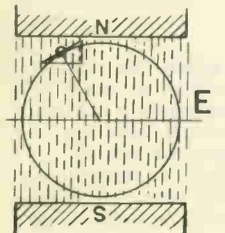
In Figure E, the angle at which the conductor is moving with respect to the lines of force is diminishing. The rate of cutting lines of force is, therefore, reduced, and the generated voltage is less than in Fig. D. The manner in which the voltage varies from point to point is shown in Fig. 1A and 1B. The conductor, which is now at  $120^\circ$ , gives a similar value as at  $60^\circ$  electrical.
