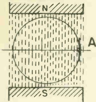
When a conductor moves in a magnetic field, the voltage induced in it depends upon:
