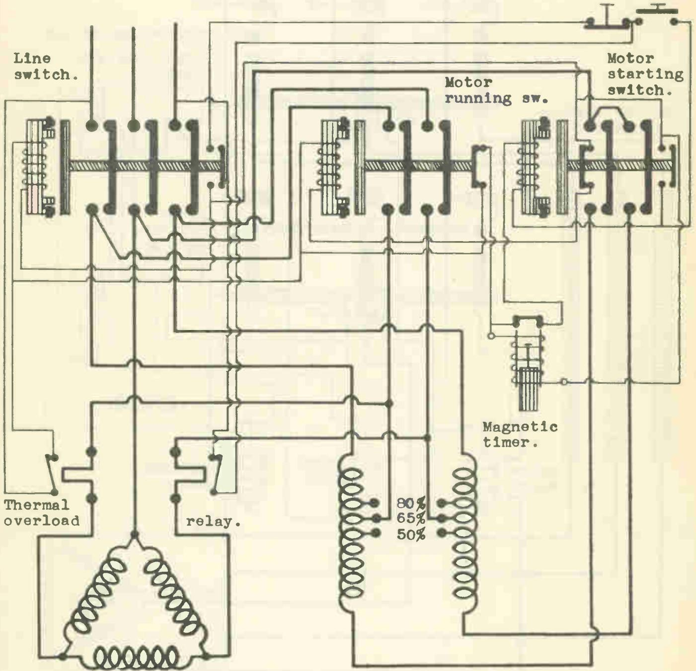
Fig. 2 Auto transformer starter
