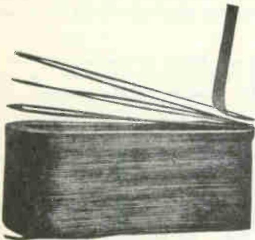
Fig. 11. Field coil which is wound with thin copper strip, making a coil which is very compact and easily wound.
