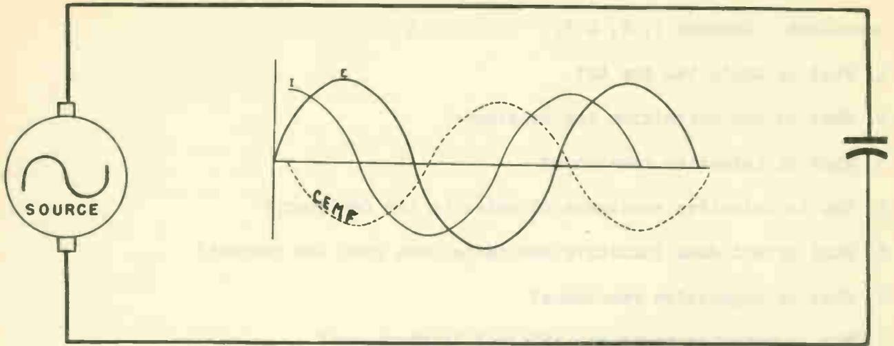
Fig. 4 A capacitor connected to an a-c source.
