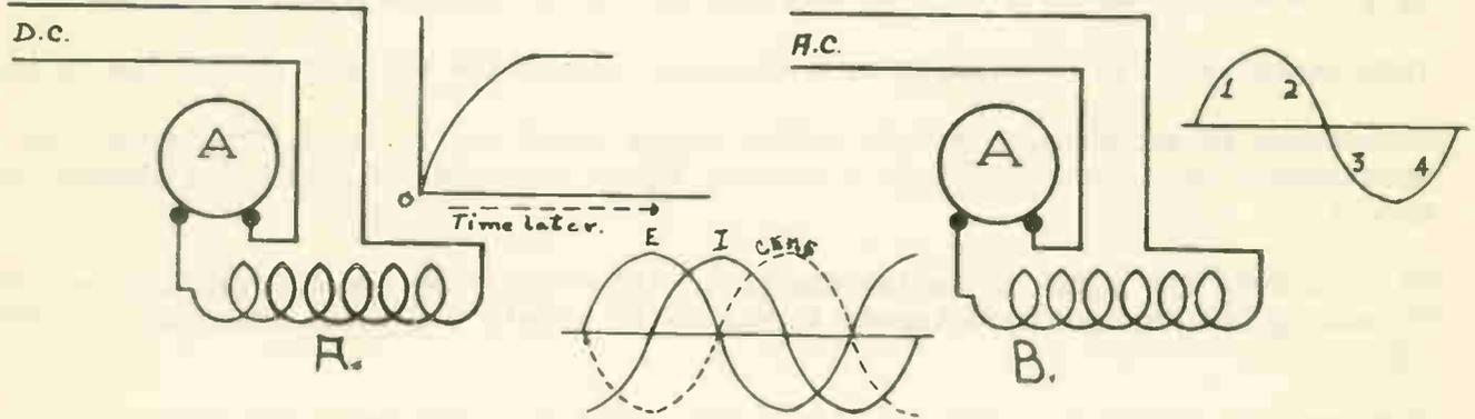
Fig. 7 Figure "A" shows the graphical effect of DC applied to a coil' "B" shows the same coil connected to an AC source. Note the curves showing the angular displacement between the voltages, E, current, I and the counter-electromotive-force (CEMF).
