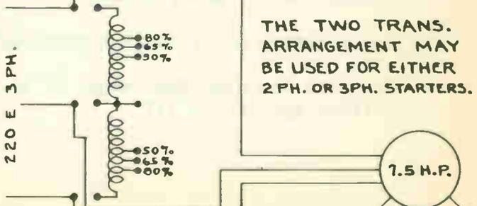
THE TWO TRANS. ARRANGEMENT MAY BE USED FOR EITHER 2 PH. OR 3 PH. STARTERS.
