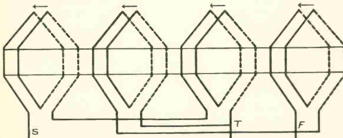
Same connection as shown above. Trace the circuit from the center tap. This places the 2 sections of the phase winding in parallel, reversing the current in  $\frac{1}{2}$  of the coil groups, producing 4 regular & 4 consequent poles. Note that phase rotation is reversed and it will be necessary to reverse 2 leads on this connection to obtain the same rotor rotation.
