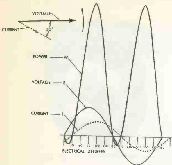
Fig. 8 Current and voltage relations in a-c circuit with 0.866 lagging power factor
