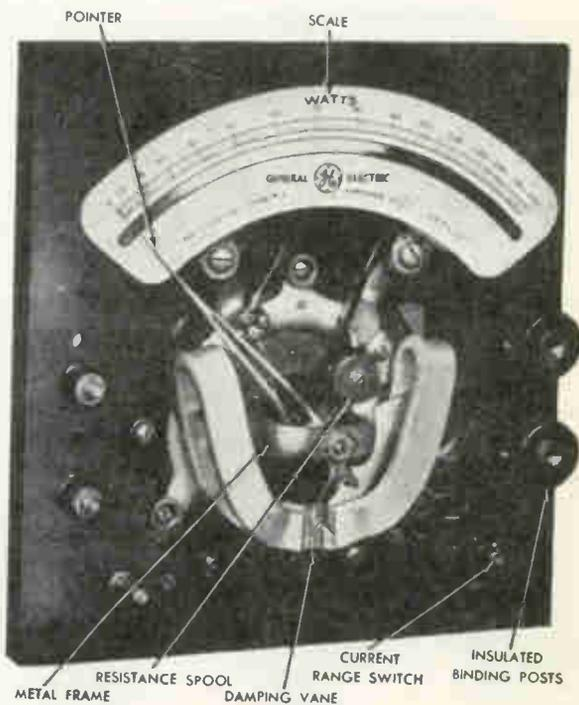
Fig. 12 Portable wattmeter removed from case
