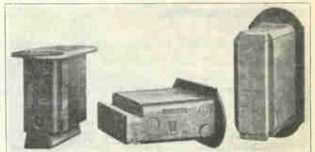
Fig. 9. Several views of laminated field poles such as commonly used in revolving field alternators.
