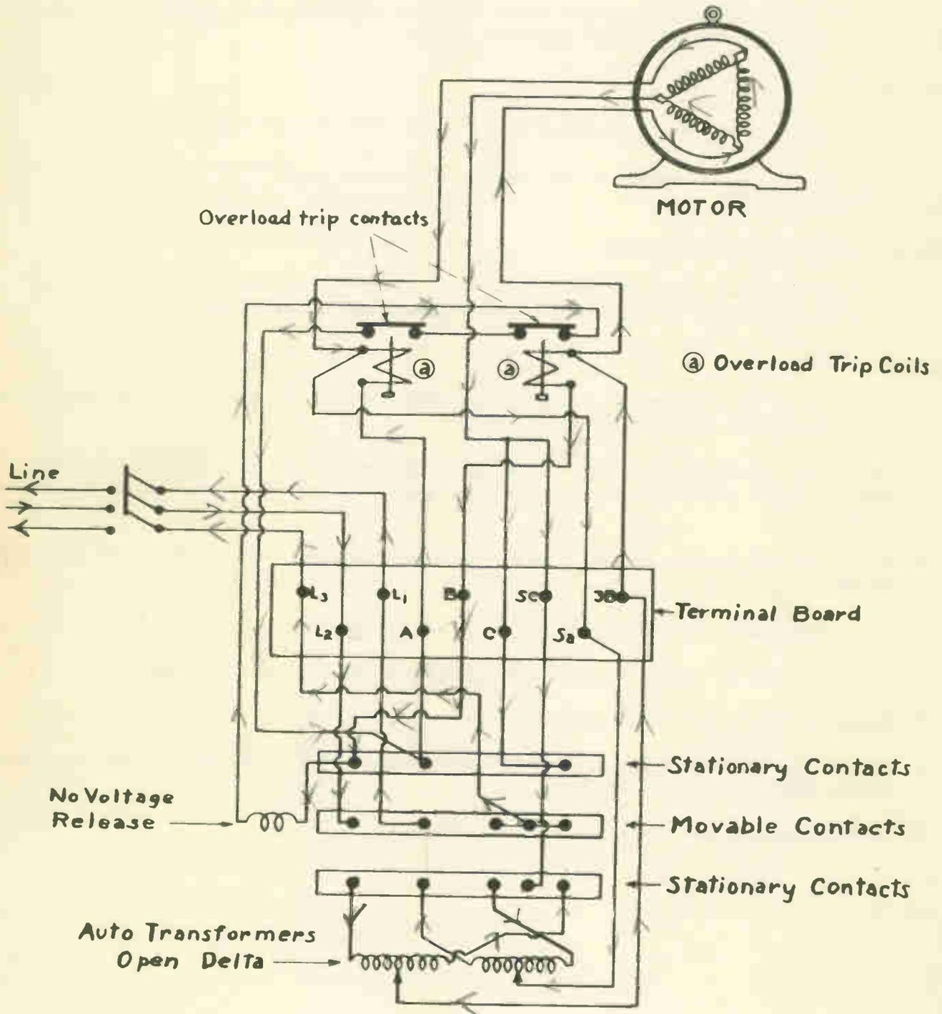
Fig. 1 Reduced voltage manual starter by 3-phase motors, 5-15 HP.
