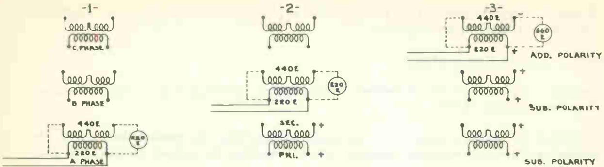
Fig. 2 Polarizing transformers
