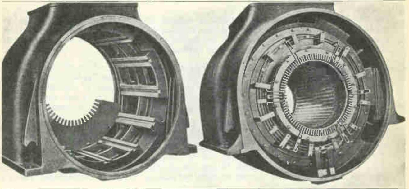
Fig. 7 The above two views show very clearly the method of construction of the stator core and windings of high speed steam-turbine-driven alternators.
