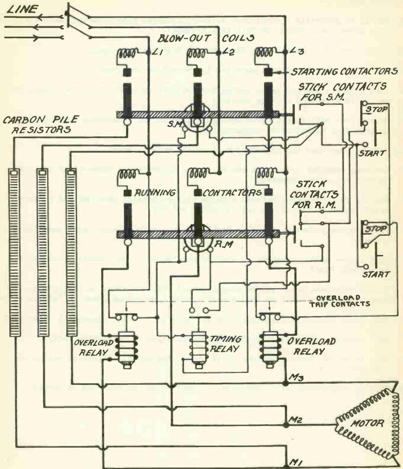
Fig. 7 Automatic resistance starter
