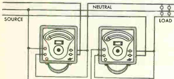
Fig. 14B External connection diagram for two wattmeters in a single-phase, two-wire circuit
