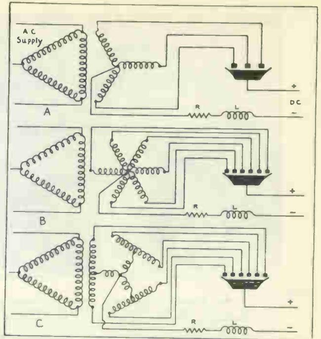
Fig. 7 The above diagrams show three different types of transformer connections which are commonly used with three-phase and six-phase mercury arc rectifiers.
