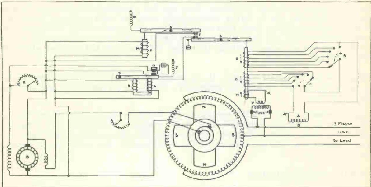
Fig. 10. The above diagram shows the wiring and illustrates the principles of a Tirrill automatic voltage regulator, properly connected to the exciter and line leads of a three-phase alternator.
