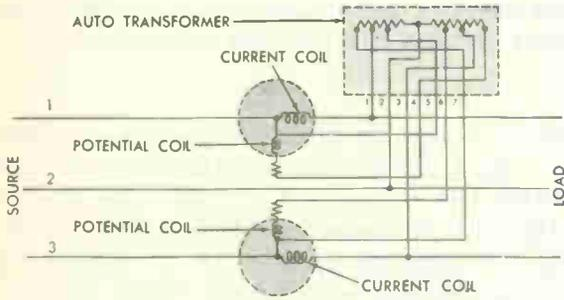
Fig. 17 Connections of dynamometer mechanisms and autotransformer for measuring vars
