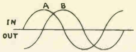
TWO PHASE, LAP WINDING, FULL PITCH, SLOTS = 24
