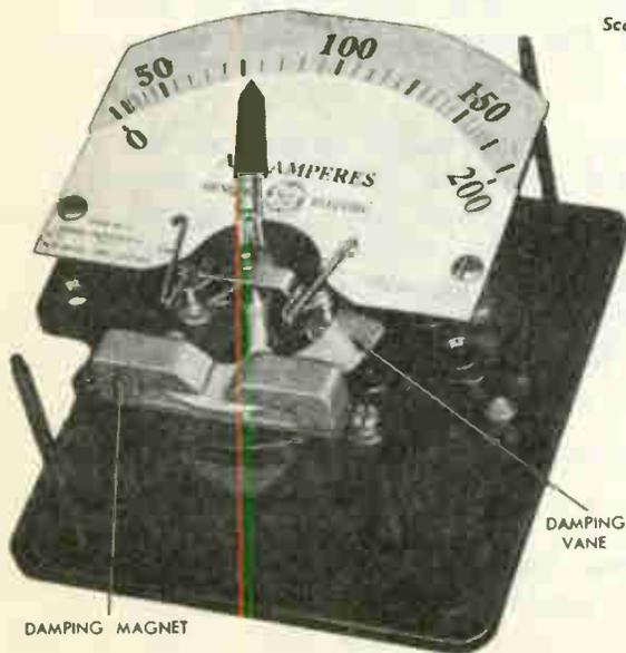
Fig. 4A Rectangular switchboard instrument, with cover removed to show magnetic damping system
