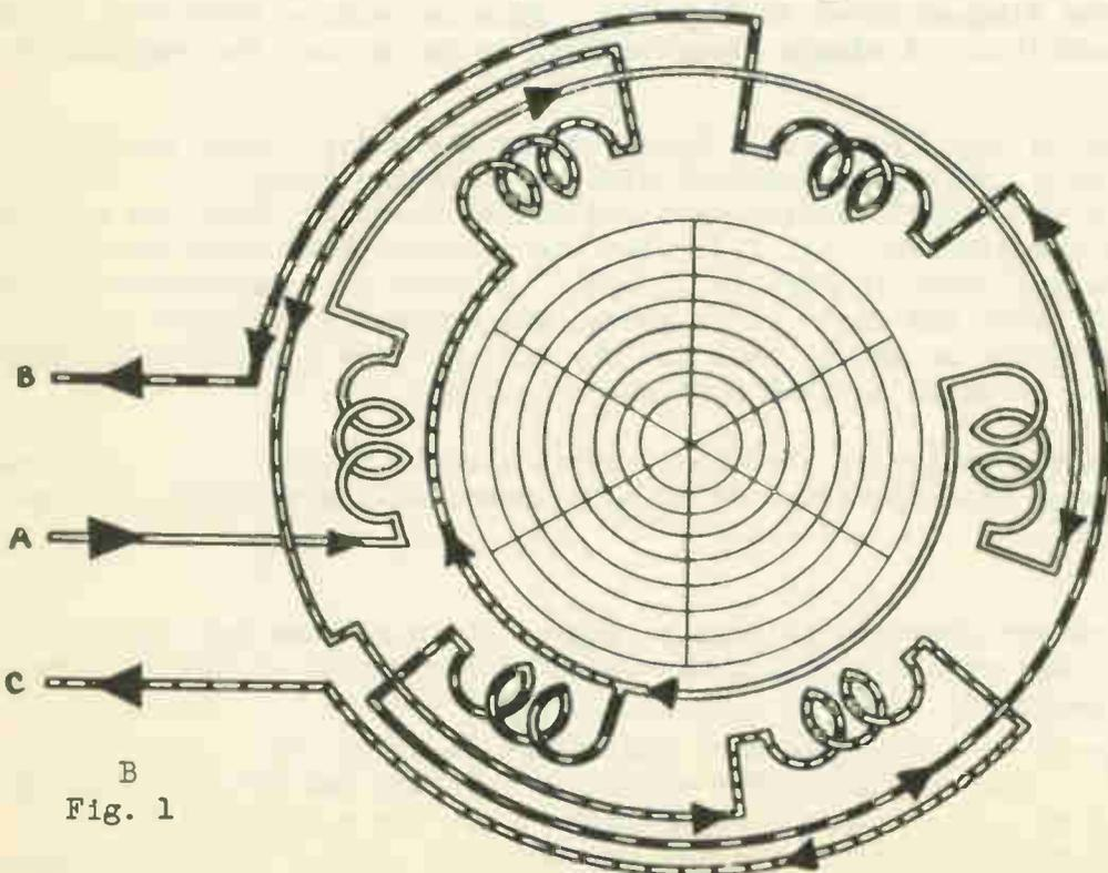
ASSUME CURRENT FLOWING CLOCK-WISE TO SET UP A SOUTH POLE, AND CURRENT FLOWING COUNTER-CLOCKWISE TO SET UP A NORTH POLE
