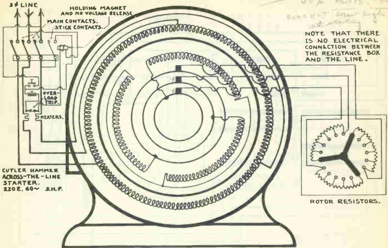
Fig.1 Slip-ring motor with a "Y" box including the electrical interlock connection block
