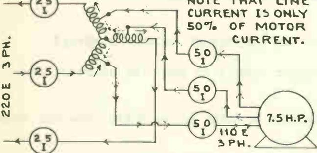
NOTE THAT LINE CURRENT IS ONLY 50% OF MOTOR CURRENT.
