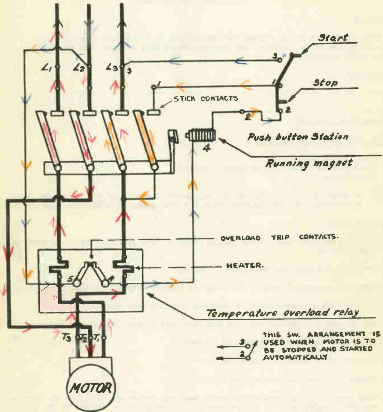
THIS SW. ARRANGEMENT IS USED WHEN MOTOR IS TO BE STOPPED AND STARTED AUTOMATICALLY.
