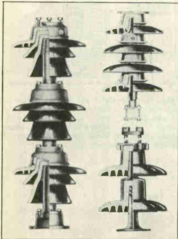
Fig. 4 Three styles of pedestal type insulators which can be built up in rigid pedestal or pillar form to support high-voltage bus bars and switching equipment.
