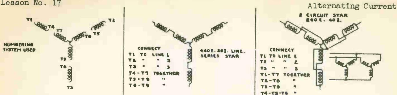
Fig. 3 Nine lead star connections
