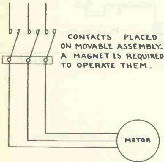
CONTACTS PLACED ON MOVABLE ASSEMBLY. A MAGNET IS REQUIRED TO OPERATE THEM.
