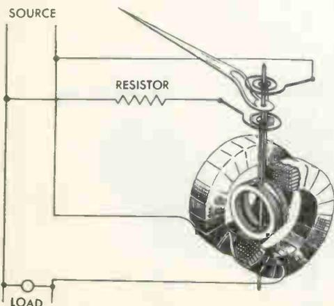
Fig. 11 Dynamometer mechanism used as a wattmeter
