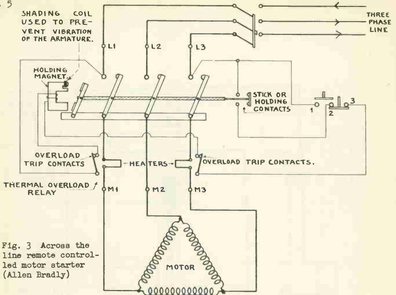
Fig. 3 Across the line remote controlled motor starter (Allen Bradley)
