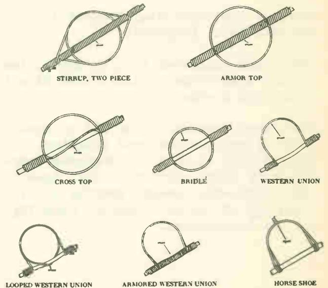
Fig. 6 METHODS OF TYING LINE WIRE TO INSULATORS
