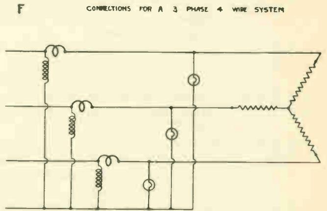
1. A ( ) B ( ) With respect to the line, what is the connection (Series or parallel) made for: (A) the current element (B) the potential element of a wattmeter.
