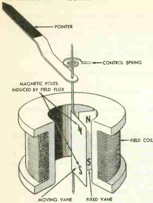
Fig. 1B Essential parts of radial-vane form of repulsion-type mechanism
