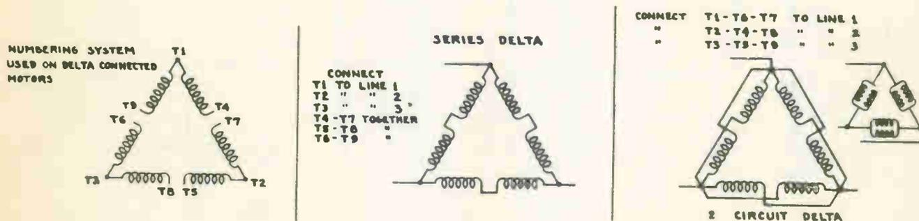
Fig. 4 Nine lead delta connections
