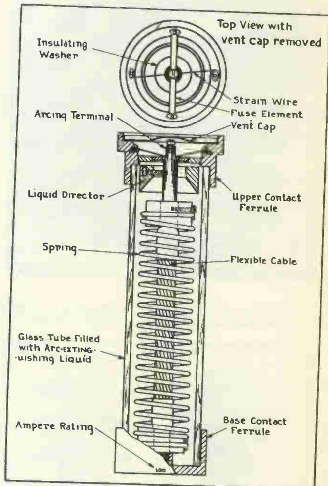
Fig. 8. The above sketch shows the principal parts of a high-voltage fuse of the liquid filled type. Examine each part carefully and compare with the explanations given on these pages. Courtesy of Schweitzer & Conrad, Inc.
