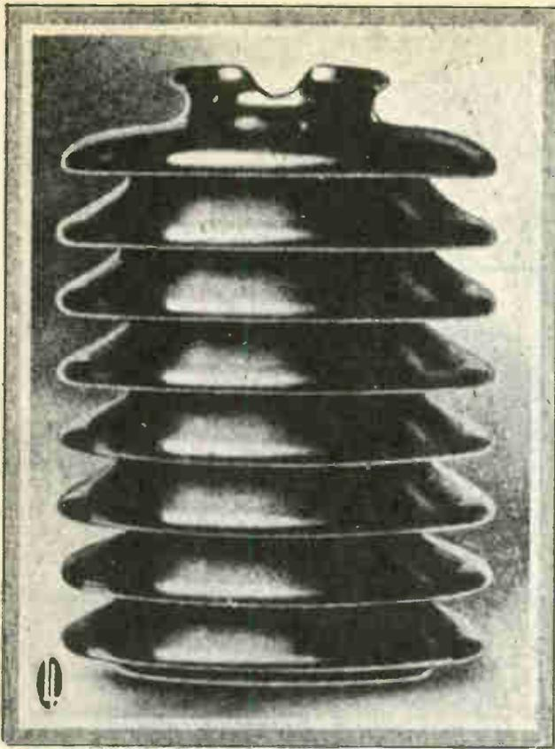
Fig. 3 Large special fog type pin insulator having a number of extra skirts to prevent flashover in districts subject to heavy salt fogs, mist, dirt, etc. Courtesy Lapp Insulator Company, Inc.
