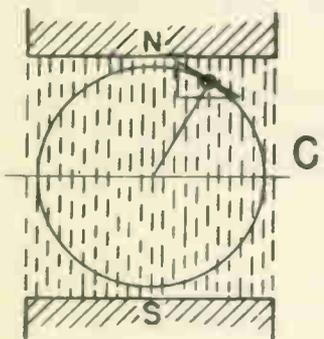
In Figure C, the conductor is moving across the flux at a different angle and, as can be seen readily by referring to Fig. C1. The number of lines of force cut per degree of angular motion has increased, because the degree of cutting has now increased to  $60^\circ$  electrical.
