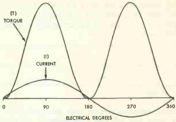
Fig. 2 Relationship of current and torque in moving-iron instrument
