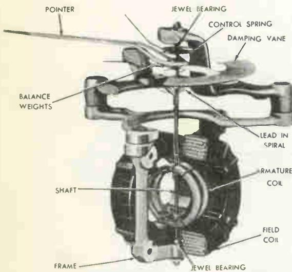
Fig. 10 Cutaway view of dynamometer mechanism
