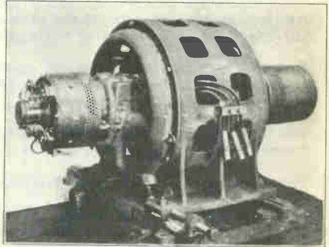
Fig. 2. This photo shows a 125 kv-a. alternator of the horizontal belt-driven type. Note the D. C. exciter-generator which is direct connected to the left end of the shaft.
