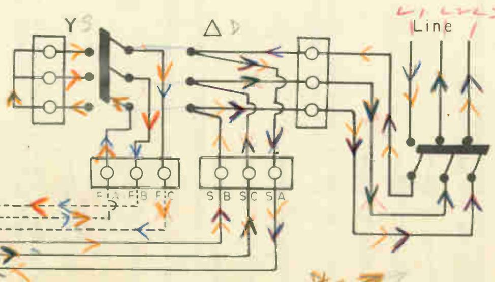
Fig. 7 Emergency 3 phase motor starter
