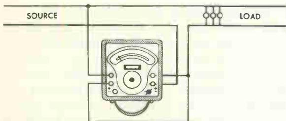
Fig. 14A External connection diagram for wattmeter in a single-phase, two-wire circuit
