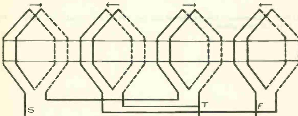
"A" Phase only of 3 phase winding illustrating long jumper method of connection. (Top to Bottom, Bottom to Top) Trace the circuit for 4 poles disregarding the center tap, and mark the polarities in the proper position. Note that the poles are established in the same position as for the common method of connection.
