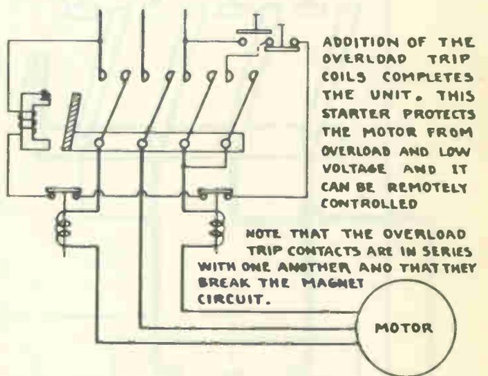
ADDITION OF THE OVERLOAD TRIP COILS COMPLETES THE UNIT. THIS STARTER PROTECTS THE MOTOR FROM OVERLOAD AND LOW VOLTAGE AND IT CAN BE REMOTELY CONTROLLED
