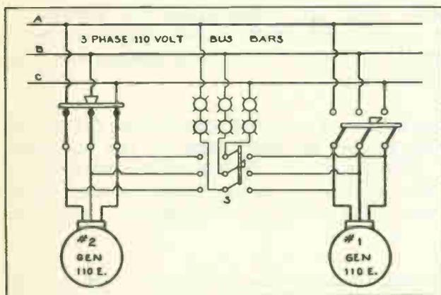
Fig. 2. Connection diagram for synchronizing either of two alternators with the bus bars by means of a lamp bank and double-throw switch.
