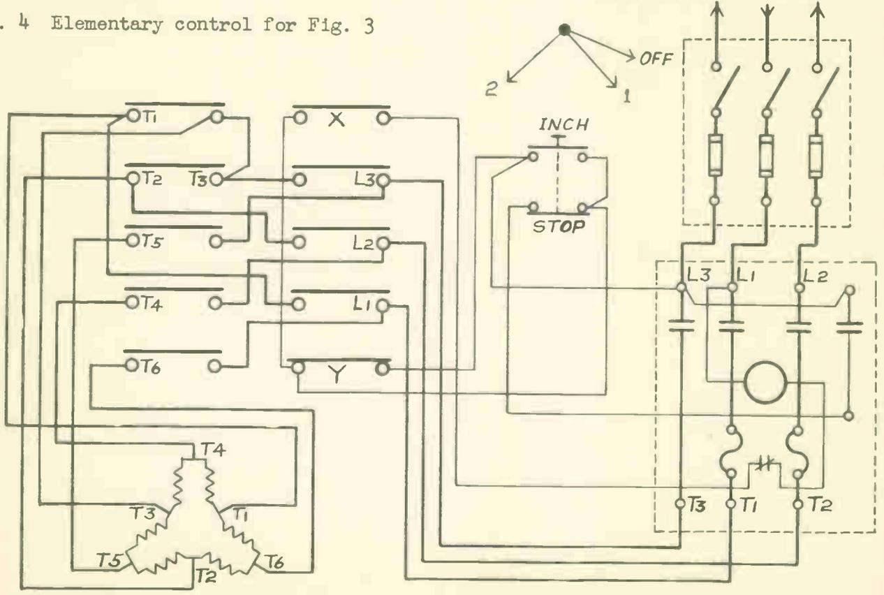
Fig. 5 Two speed motor drum control and inching control
