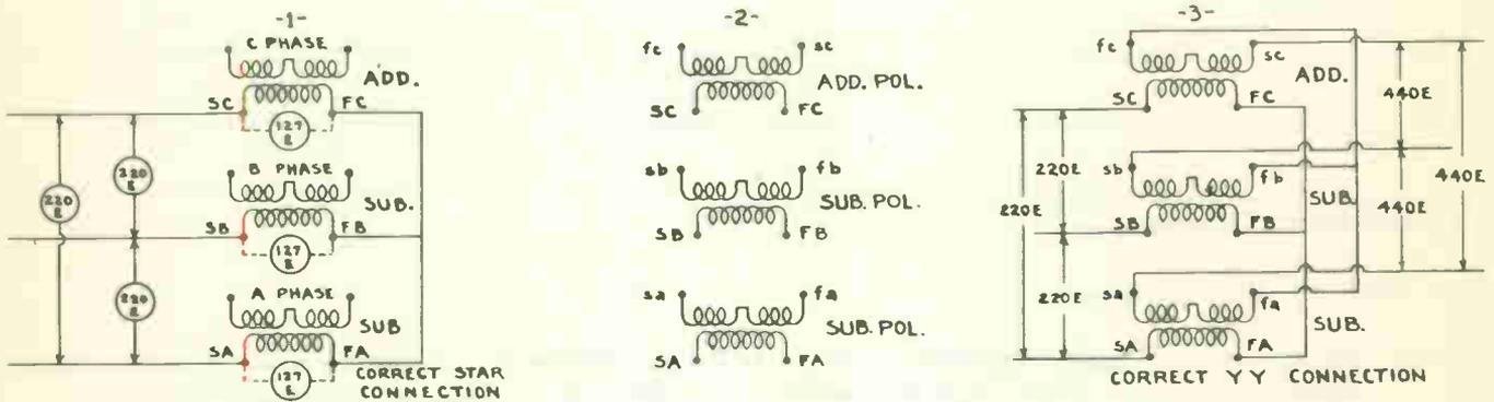
Fig. 3 Phasing out transformers
