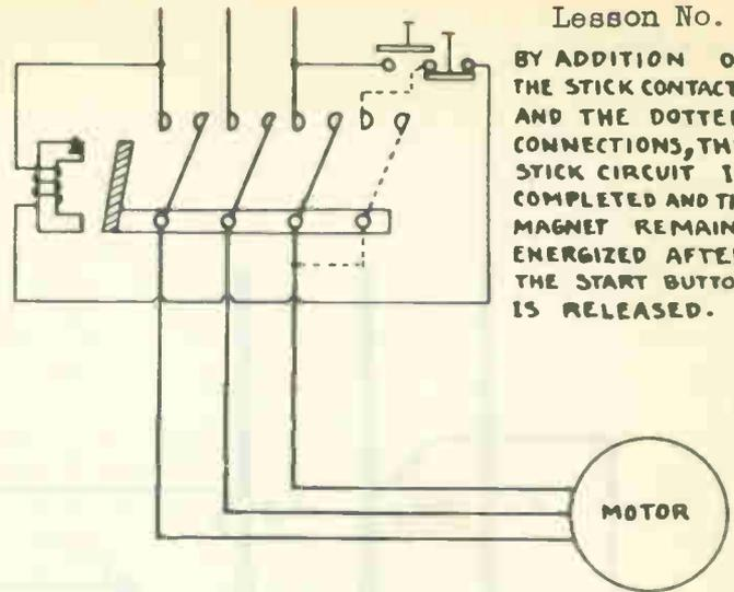
BY ADDITION OF THE STICK CONTACTS AND THE DOTTED CONNECTIONS, THE STICK CIRCUIT IS COMPLETED AND THE MAGNET REMAINS ENERGIZED AFTER THE START BUTTON IS RELEASED.
