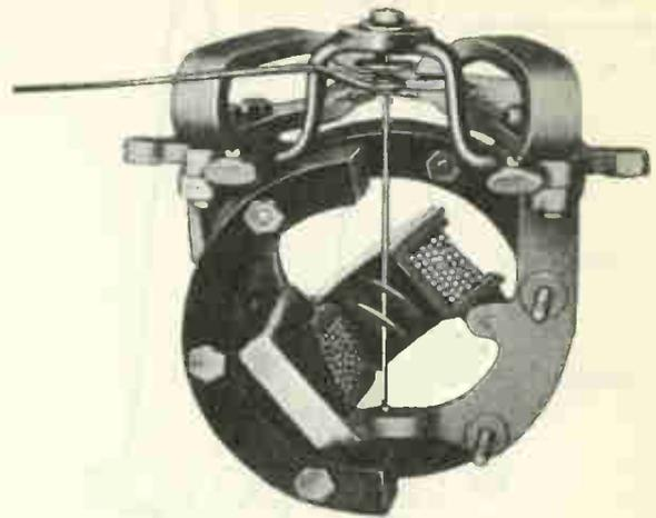
Fig. 6 Cutaway view of inclined-coil attraction-type voltmeter
