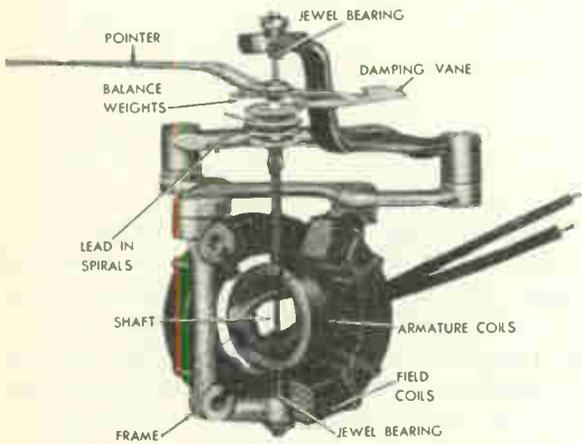
Fig. 18 Cutaway view of mechanism of crossed-coil power-factor meter
