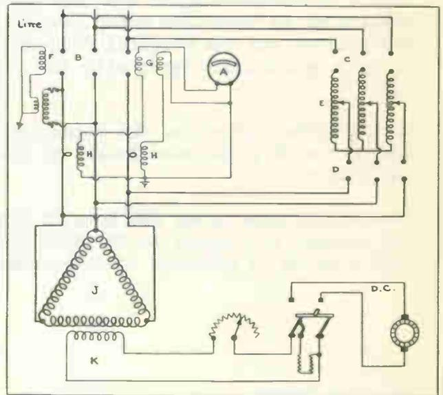
Fig. 6 Diagram of connections for a large synchronous motor with a compensator for starting at reduced voltage. Also note the protective device connected with a circuit-breaker in the line leads.
