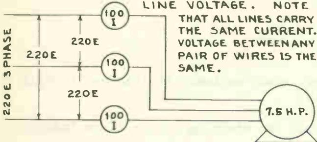
MOTOR STARTING AT FULL LINE VOLTAGE. NOTE THAT ALL LINES CARRY THE SAME CURRENT. VOLTAGE BETWEEN ANY PAIR OF WIRES IS THE SAME.
