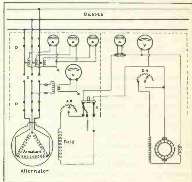
Fig. 3. This diagram shows the wiring and arrangement of a three-phase alternator, and the meters and equipment commonly used on the switchboard panels.
