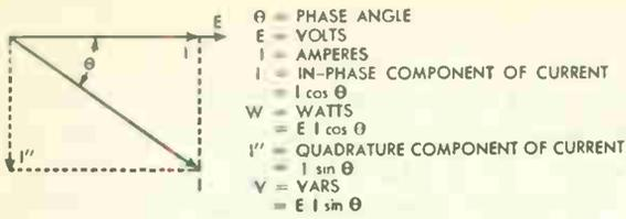
Fig. 15 Vector diagram showing relation of vars to voltage and current in single-phase circuit
