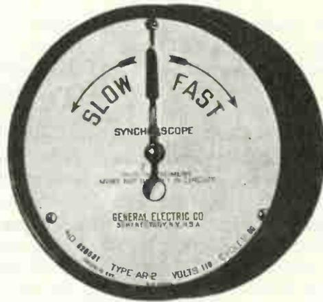
Fig. 21 Typical crossed-coil synchroscope
