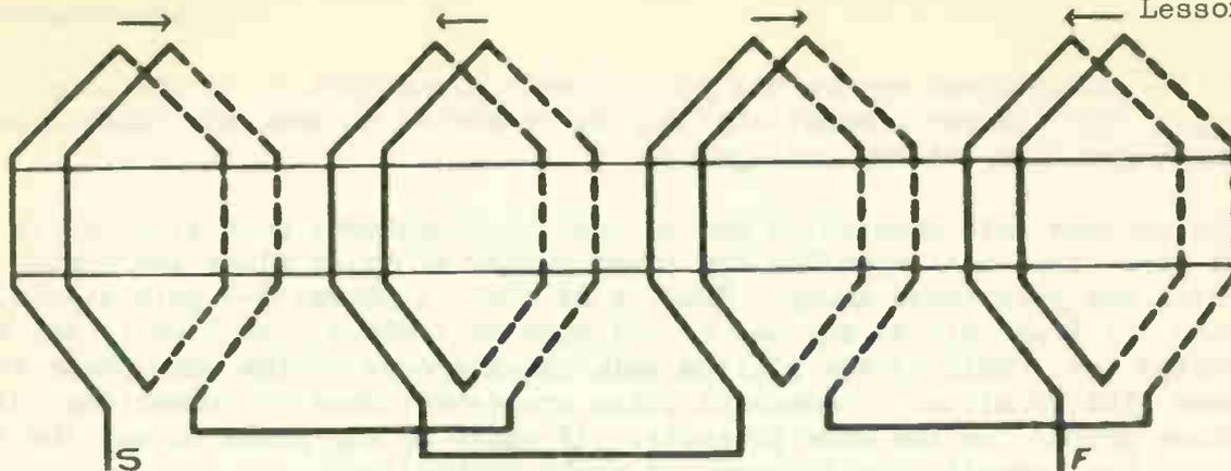
Slots = 24, Poles = 4, Fractional Pitch Coil Span = 1 to 5.
