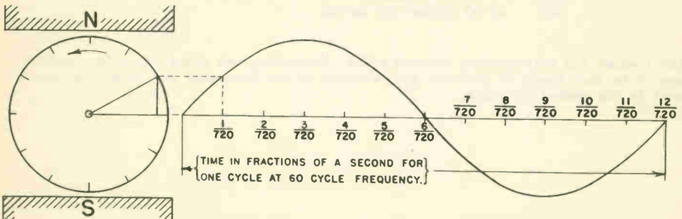
The smooth curve above shows the manner in which the generated voltage varies from instant to instant. The distance of the curve from the base line at any point is a measure of the voltage generated at that instant.
