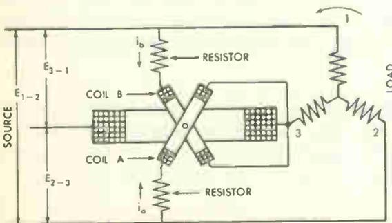
Fig. 19B Diagram of three-wire, three-phase, crossed-coil power-factor meter
