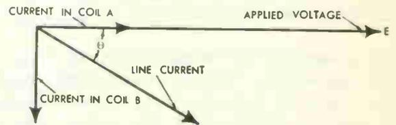
Vector diagram showing relationship of voltage and currents in single-phase, crossed-coil power-factor meter
