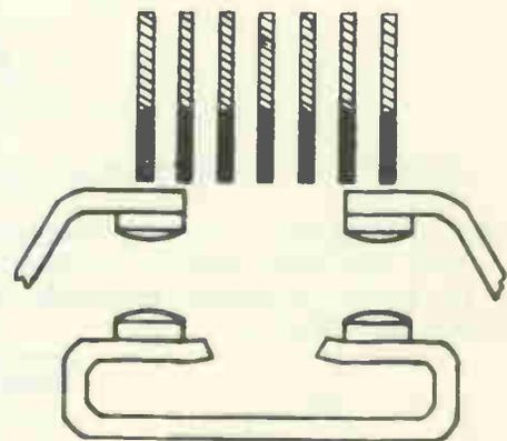
Fig. 6B "DE-ION" ARC QUENCHER.
