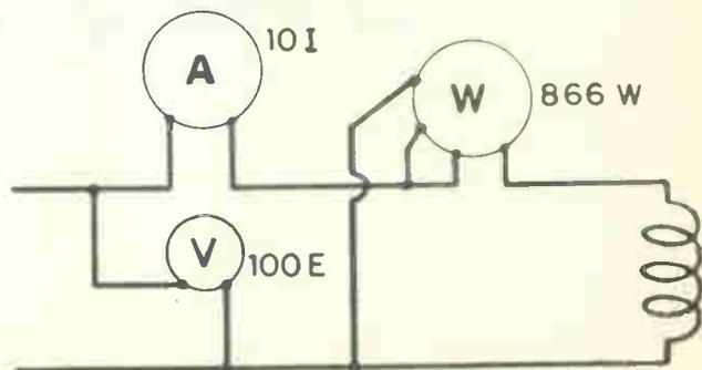
$$\begin{aligned} \text{Active Current} &= \text{Line Current} \times \text{Cos } \theta \\ 8.66 &= 10 \times .866 \end{aligned}$$
