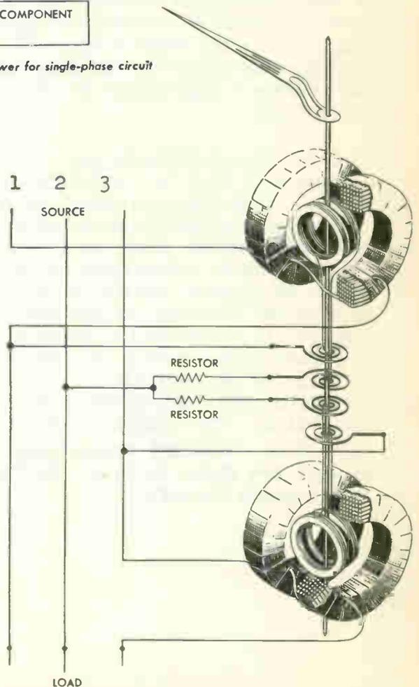
Fig. 14C Diagram of a two-element wattmeter
