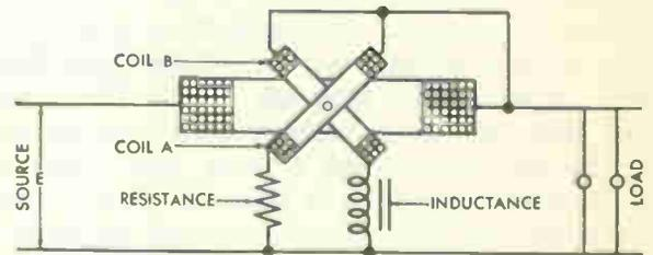
Fig. 19A Diagram of single-phase, crossed-coil power-factor meter
