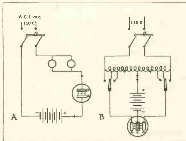
Fig. 13A shows a half-wave, electrolytic rectifier and B shows an electrolytic rectifier of the full-wave type. Current can only pass through these devices in one direction.
