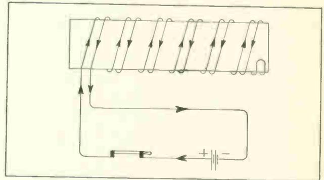
Fig. 13 Non-magnetic winding. One half of the turns oppose the other half, so the core does not become magnetized.
