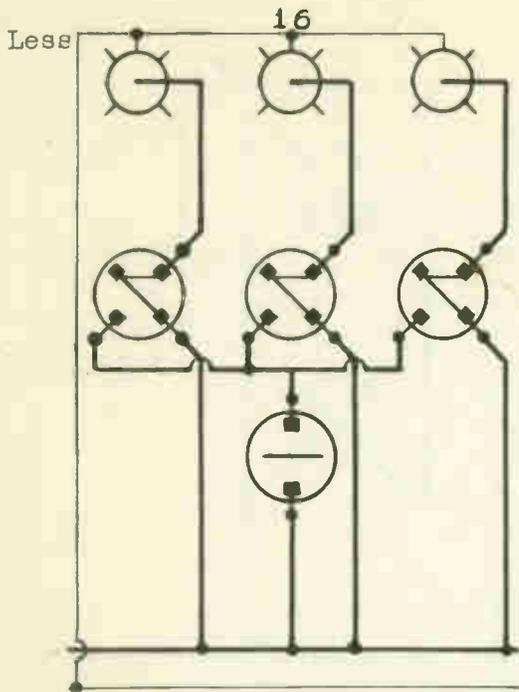
This shows 3 lights, each one individually controlled from one place, using a three-way switch as a single-pole switch. The one single-pole switch is used as a master switch when the master switch is on; the other lights cannot be turned off.
