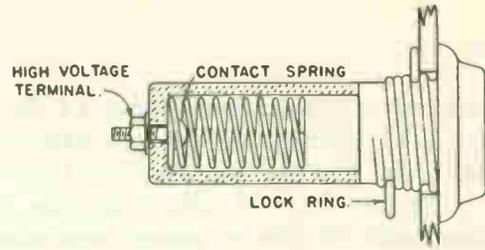
Fig. 8B A Receptacle for Luminous Tubing.
