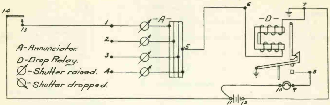
To Find Common Terminal of Annunciator, With Test Leads.
