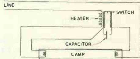
Fig. 8 How the Thermal Starter Is Connected To the Lamp.
