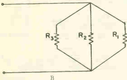
1. R<sub>1</sub> is connected in series with R<sub>2</sub> & R<sub>3</sub>      TRUE      FALSE
