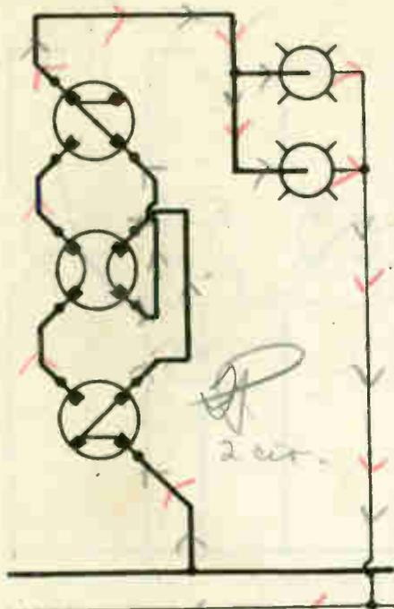
FIG. A Method used to control one or more lights from three places.
