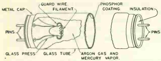
Fig. 1 Construction of a Fluorescent Lamp.
