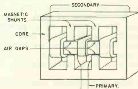
Fig. 13 Sign Transformer Having High Leakage Reactance, Showing the Magnetic Shunts Between Winding Sections.
