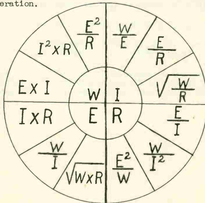
Fig. 5. "WIRE" Wheel. Any of the four values shown in the center-- W, I, R, or E, can be found in three different methods, according to which values are known.
