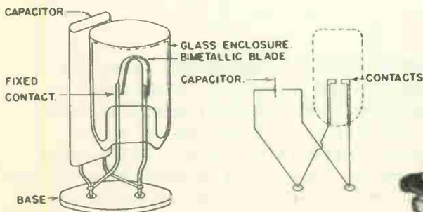
Fig. 4 Construction and Connections of a Glow Switch Starter.
