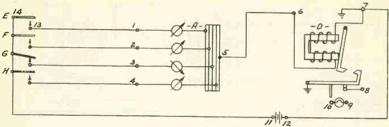
The circuit through battery, relay and annunciator has been completed through the movable contact at signal station G when the annunciator shutter #3 indicating the station falls and relay trips.
