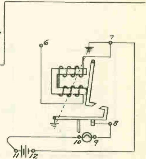
When relay trips the light or bell circuit is completed through the drop terminal #8 and ground, as indicated by the dotted line, and alarm will continue to operate until relay is reset manually.
