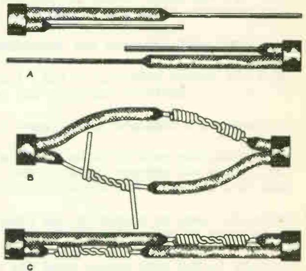
Fig. 4 When making splices in pairs of conductors they should be staggered as shown above so each splice will be close to good insulation on the other wire.
