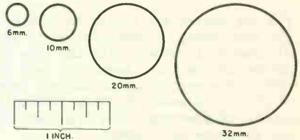
Fig. 11 Relative Sizes of Some Luminous Sign Tubing.
