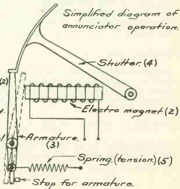
Fig. 1 Gravity drop type annunciator
