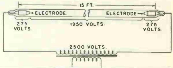
Fig. 12 Voltage Distribution in Sign Tubing.
