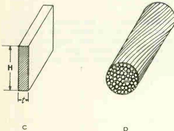
Fig. 2. Electrical conductors are commonly made in the several shapes shown above. Note particularly the comparative areas of round and square conductors as shown at "B".
