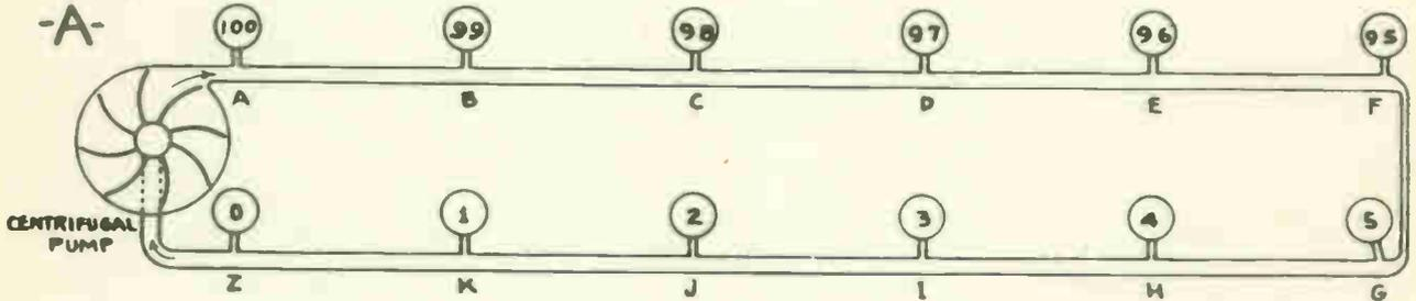
1. Which point is at the higher pressure? A or B, J or I, B or D, K or A. \_\_\_\_\_
