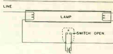
Fig. 5 How the Glow Starter Is Connected To the Lamp.
