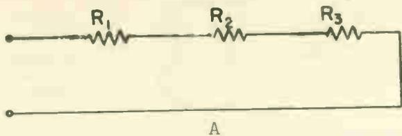
1. R<sub>1</sub> is connected in series with R<sub>2</sub>      TRUE      FALSE
