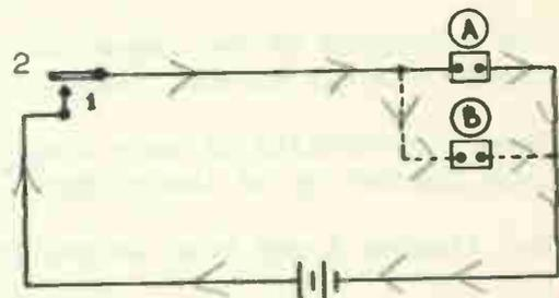
Open circuit switch used to control 2 bells in parallel
