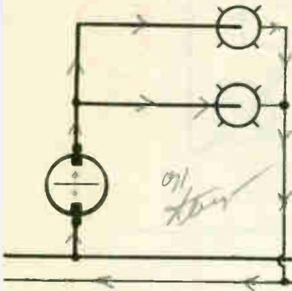
A single-pole switch used to control two lights in parallel.
