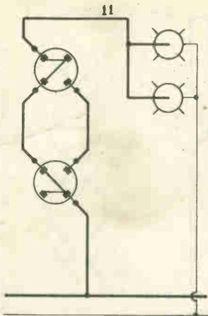
This circuit is the "Standard" method for two-place control using two 3-way switches and is approved by the Code for 110E.
