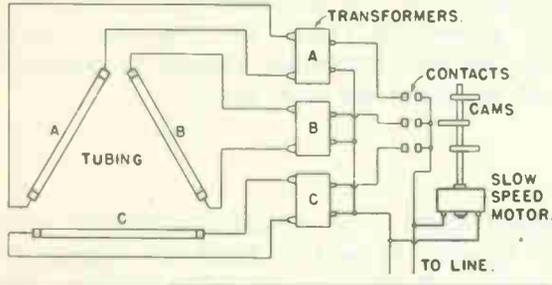
Fig. 8C Sign Flasher on Primary Side of Transformers.
