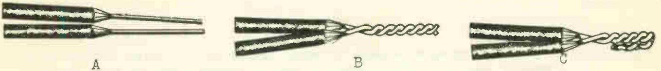
Fig. 1 Steps to be followed in making a pigtail splice.
