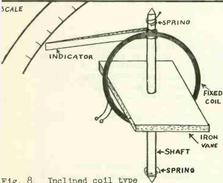
Fig. 8. Inclined coil type
