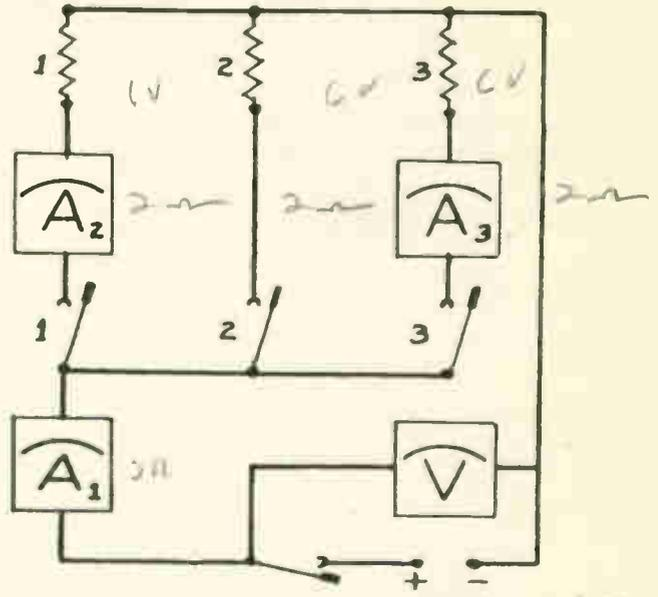
2. The Voltmeter reading with no resistors connected (no load) is 7V.
