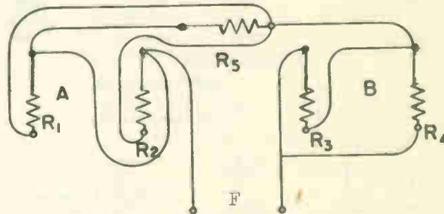
1. R<sub>1</sub> is connected parallel with R<sub>2</sub>      TRUE      FALSE
