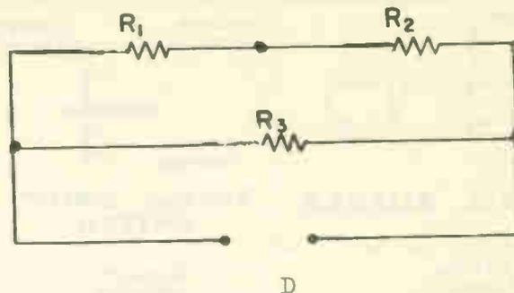
1. R<sub>1</sub> is connected in series with R<sub>2</sub>      TRUE      FALSE
