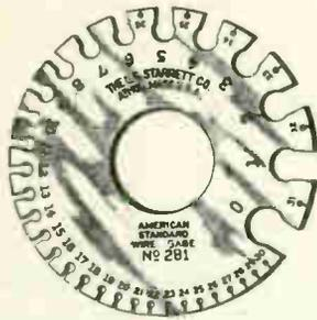
Fig. 1 A wire gauge of this type is commonly used to determine the size of wires for various uses.
