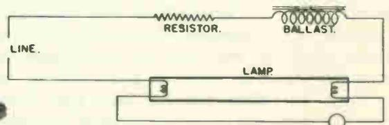
2. Construction and Operation of Ballast - a. A coil having many turns wound on an iron core has high inductance. When current has been flowing in such a coil and suddenly is stopped the magnetic lines of force which have existed around the windings collapse and cut back through the turns. This cutting of the conductor by lines of force induces a voltage which is much higher than that which was sending current through the coil. It is commonly referred to as "inductive kick".
