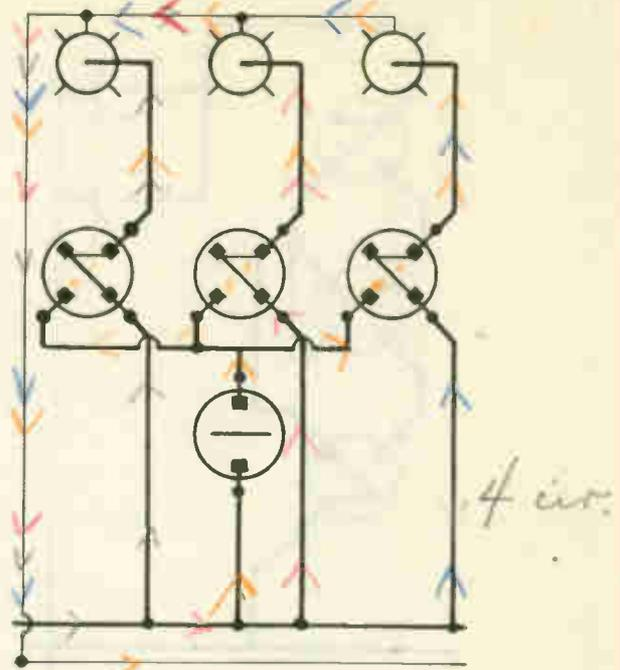
FIG. B This shows 3 lights, each one individually controlled from one place, using a three-way switch as a single-pole switch. The one single-pole switch is used as a master switch. When the master switch is on; the other lights cannot be turned off.
