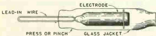
Fig. 10 An Electrode in its Glass Jacket for Attachment to Tubing.
