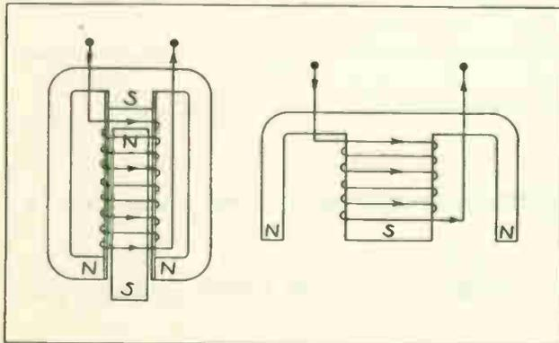
Fig. 10. Plunger type magnet at left. Shell type magnet at right.
