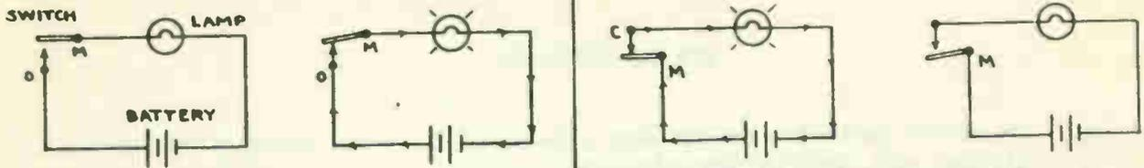
IF THE LAMP LIGHTS WHEN THE BUTTON IS PRESSED, IT IS AN OPEN CIRCUIT SWITCH HAVING OPEN AND MOVING CONTACTS.
