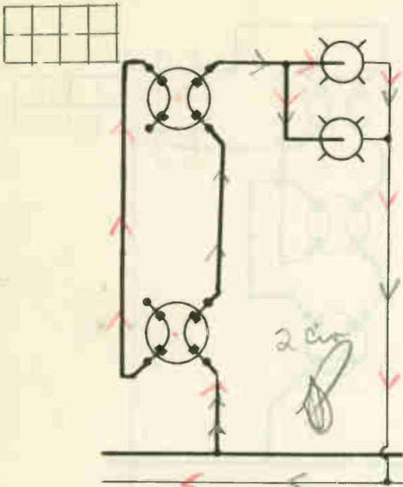
FIG. A Possible circuit used to control two lights in parallel from two places using two 4-way switches.
