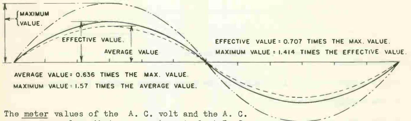
The meter values of the A. C. volt and the A. C. ampere are values that represent equivalent D. C. values. An A. C. current that will produce the same heating effect as a D. C. current of one ampere is said to have an effective value of one A. C. ampere. Note that the curve of effective values is somewhat lower than the curve of maximum values, and slightly higher than the curve of average values.
