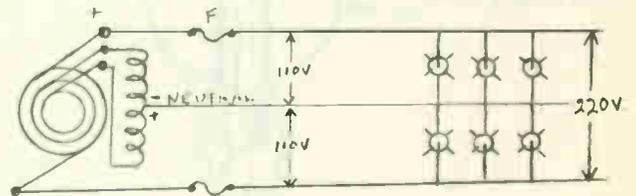
Fig. 2B Six lamps connected to a 3-wire system using a balance coil.
