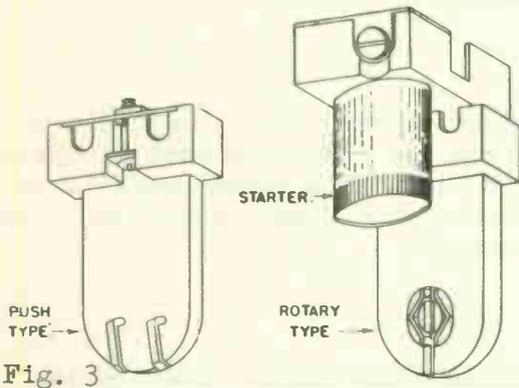
Fig. 3 Lampholders for Supporting the Lamp and Making Contact With the End Pins.
