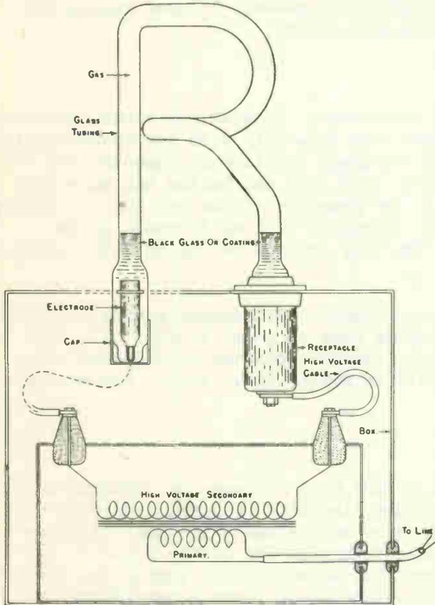
Fig. 9 The Principal Parts of a Neon Sign.
