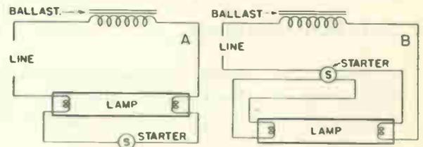
Fig. 9 How the Ballast Is Connected In Circuit With the Lamp and Starter.
