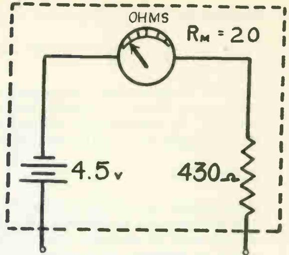
Fig. 4 Basic Ohmmeter Circuits
