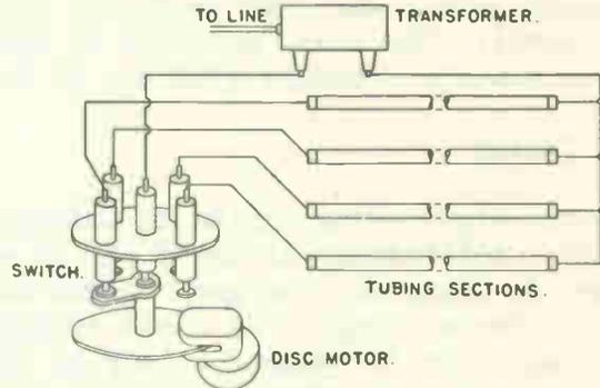
Fig. 8D Sign Flasher Operating in the High Voltage Secondary Circuit of a Single Transformer.
