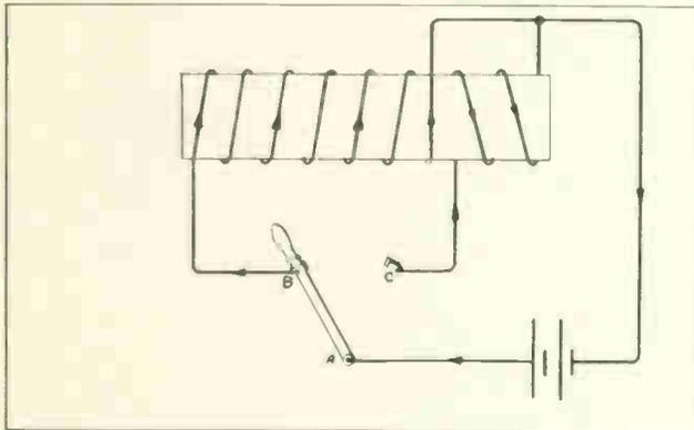
Fig. 12 Electric magnet with demagnetizing coil for destroying residual magnetism.
