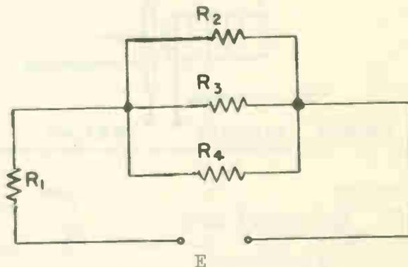
1. R<sub>1</sub> is connected in series with the network      TRUE      FALSE
