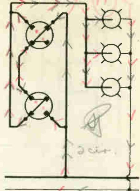
FIG. A This circuit is the "Standard" method for two-place control using two 3-way switches and is approved by the Code for 110v.
