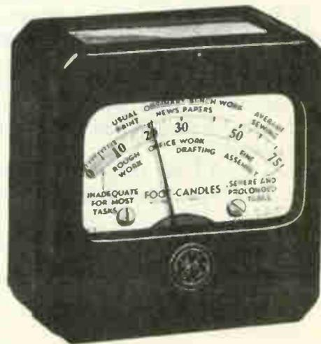
This G-E Light Meter closely resembles a small thin desk clock. It is 2 1/4 inches square and 1 1/8 inches thick and can be carried in the vest pocket. The normal scale range of the meter is from 0 to 75 footcandles but each meter is provided with a multiplying shield so that illumination values up to 750 footcandles can be read.
