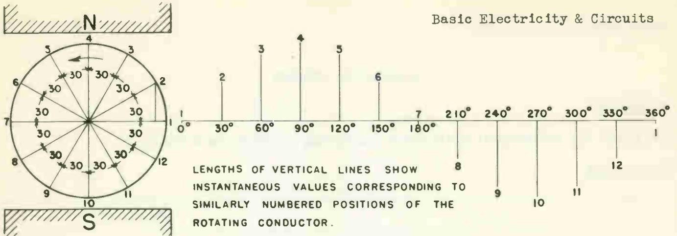
LENGTHS OF VERTICAL LINES SHOW INSTANTANEOUS VALUES CORRESPONDING TO SIMILARLY NUMBERED POSITIONS OF THE ROTATING CONDUCTOR.
