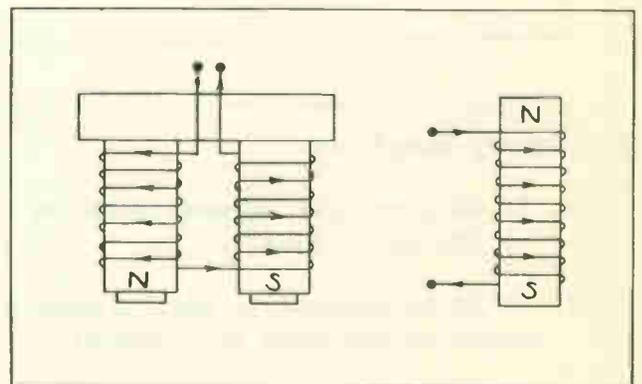
Fig. 11 Double and single electro-magnets.
