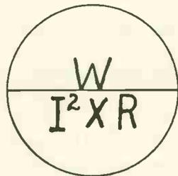
Fig. 3. Simplified formula for use when voltage is unknown.
