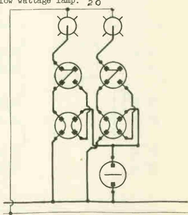
When the single-pole switch is open, each of the 2 lights may be controlled from 2 places. When the single-pole switch is closed, all the lamps will remain lighted, regardless of the position of the other switches.
