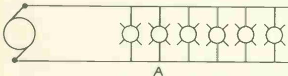
Fig. 2A Six lamps connected to a 2-wire system
