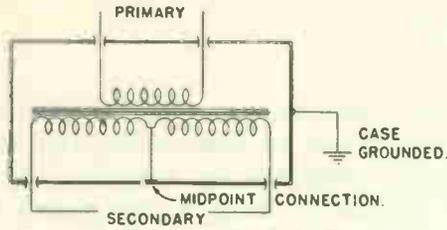
Fig. 8A How the Secondary Midpoint is Grounded.
