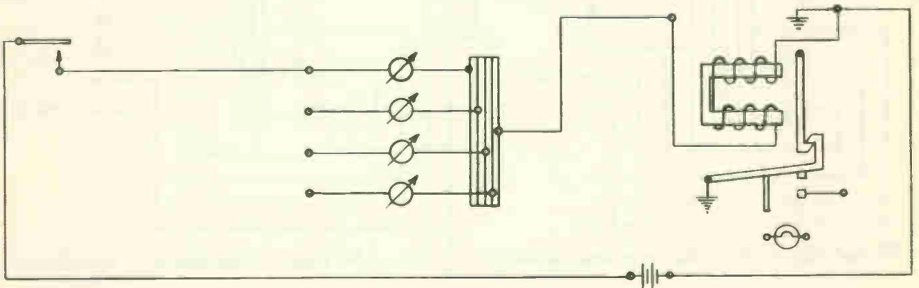
Required wiring connections to battery, annunciator and relay so that station signaling is recorded and relay tripped. For wiring of warning lamp or bell signal equipment see following sheet.
