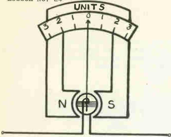
Fig. 1 Moving Coil d'Arsonval Galvanometer
