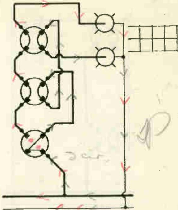
FIG. B This diagram shows how to control each light alternately from three different places.
