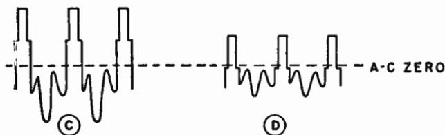
Fig. 113-2.—Picture signals and sync pulses represented as alternating potentials without d-c components.
