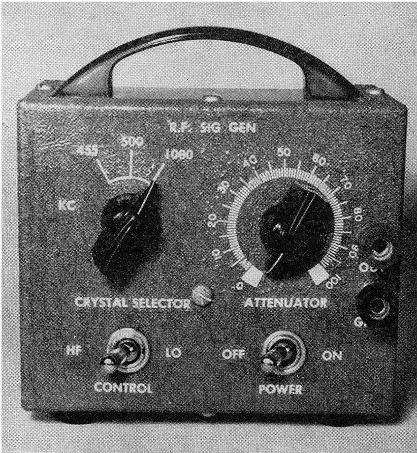
Fig. 9-5.—Author's model of the R.F. Alignment Generator.
