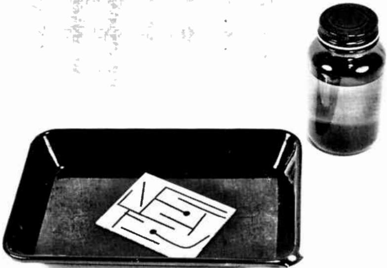
**Fig. 13-4.**—After the desired layout has been transferred to the copper-clad laminate as a pattern of resist, the board is etched in an enamel or plastic tray.
