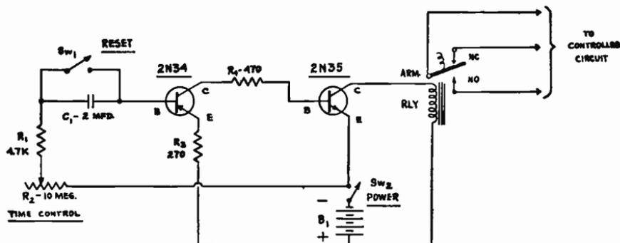
Fig. 10-2.—A "Precision" transistorized Timer circuit—no electrolytic capacitors are used.
