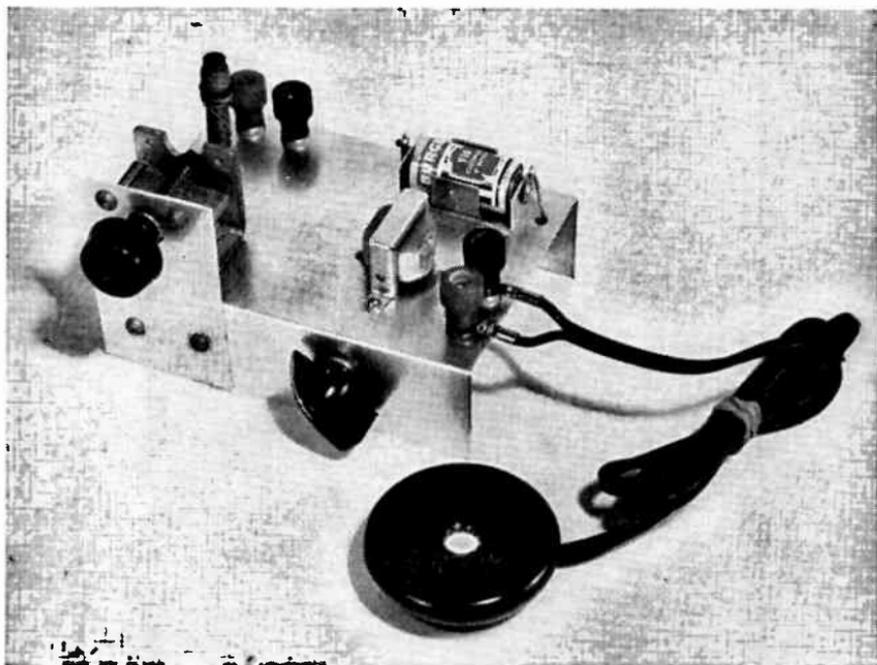
Fig. 8-4.—Author's model of the *Regenerative Receiver*. Transistors are mounted below chassis.
