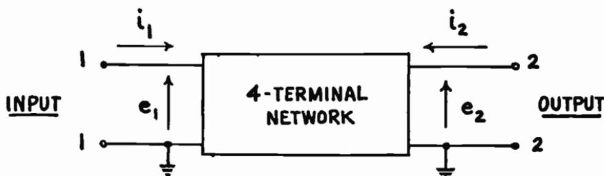
Fig. 12-1.—Basic four-terminal network representation shown as a "black box." Input and output terminals and input and output voltages and currents are identified. Arrows show conventional flow.
