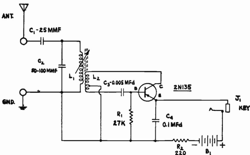
Fig. 8-15.—Circuit for a Wireless Code Practice Oscillator.
