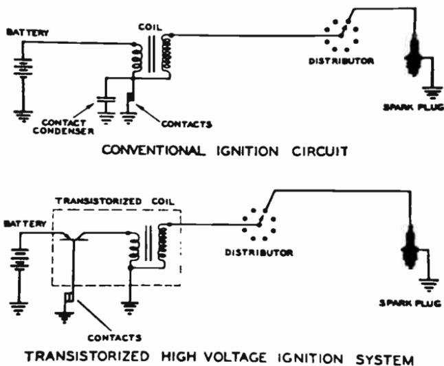
Fig. 14-26: Here, "conventional" and transistorized automobile ignition circuits are compared.
