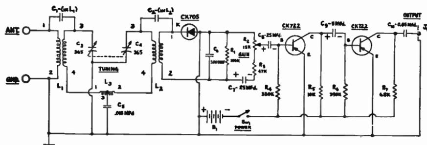
Fig. 8-8.—Diagram of a Hi Fi AM Tuner featuring a transistorized preamplifier.
