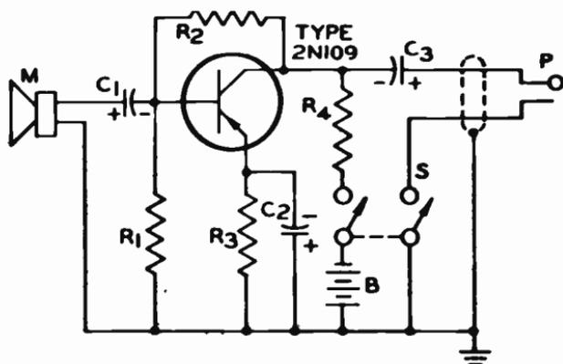
Fig. 14-1.—Single-stage microphone preamplifier — used with a magnetic cartridge or small loudspeaker, this circuit provides an output level comparable to that obtained from a carbon microphone.
