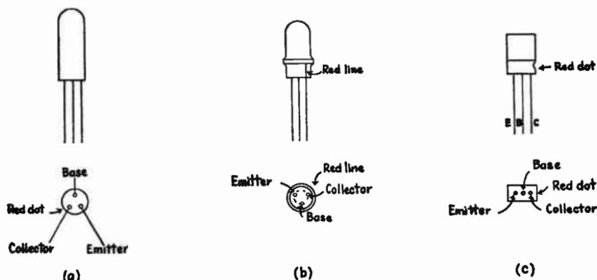
Fig. 2-8.—Special transistor pin connections used by some manufacturers. *TRANSITRON* (a); *PHILCO* (b); *RAYTHEON* (c).
