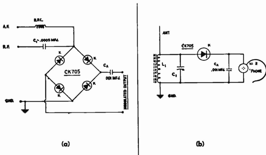
Fig. 10-26.—R.F. Semiconductor Diode applications: (a) Bridge Modulator; (b) Simple Crystal Receiver.
