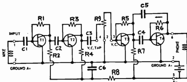
Fig. 14-6.—Typical Hearing Aid amplifier schematic. Component values vary with the exact types of transistors used.
