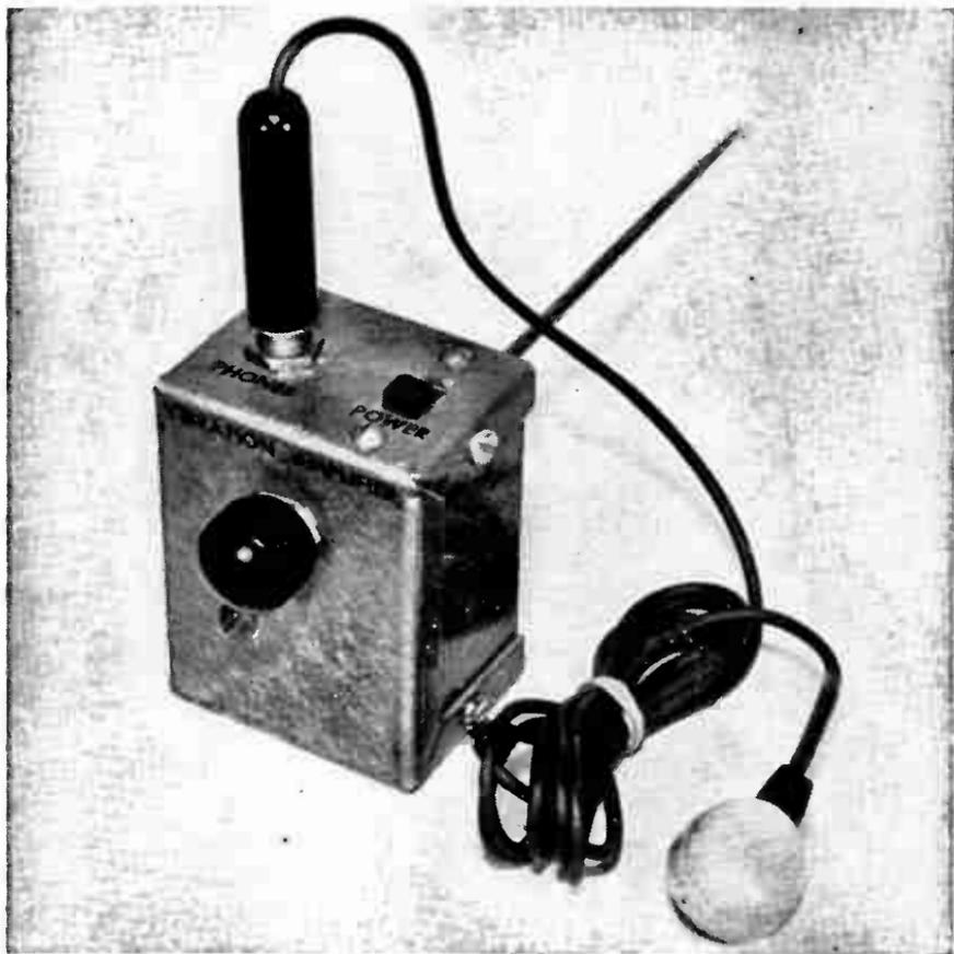
*Fig. 7-6.—Exterior view of the electronic "Stethoscope"*
