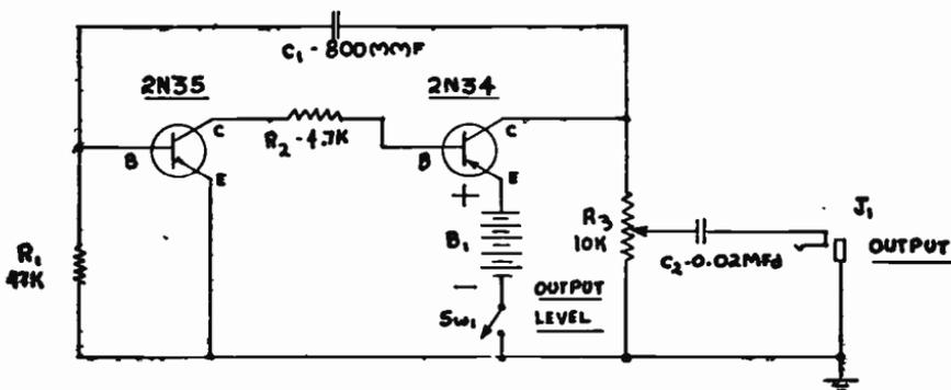
Fig. 9-7.—Circuit for The Signal Squirrelter.
