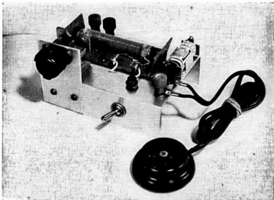
Fig. 8-2.—Overall view of the Simple Receiver.
