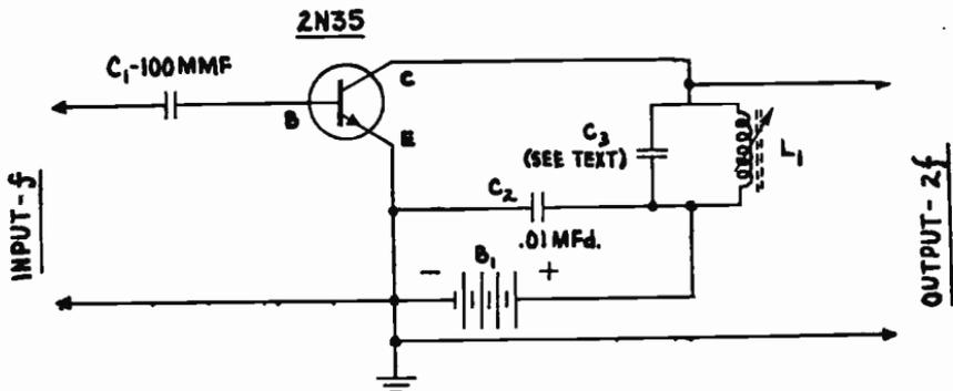
Fig. 8-24.—Diagram of a basic transistorized R.F. Frequency Doubler.
