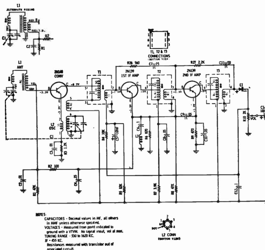
Fig. 14-16.—Circuit diagram of MOTOROLA Models 76T1 and 76T2 (Chassis HS-507). Note that a variety of output connections are used in various production runs of this seven-transistor radio. Manufacturers will frequently make minor circuit changes during production.
