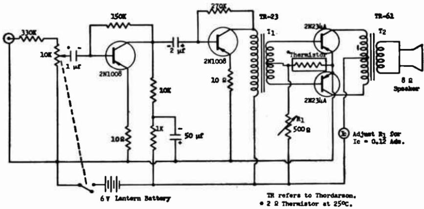
**Fig. 14-4.**—Schematic diagram of a phonograph amplifier. Designed for use with a crystal or ceramic pick-up, this amplifier delivers good room volume, but requires relatively little battery power, insuring long battery life.
