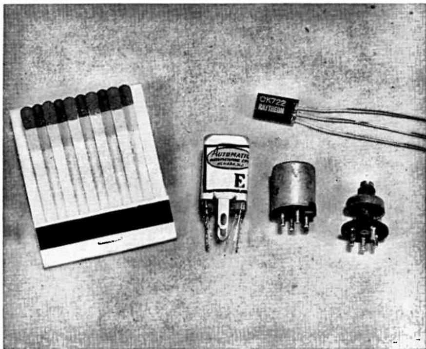
Fig. 3-3.—Subminiature R.F. coils and I.F. transformers.
