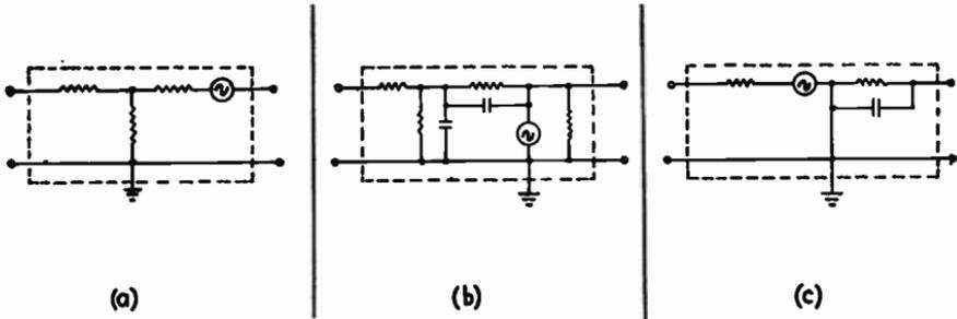
Fig. 12-2.—Three basic equivalent circuits which may be represented as four-terminal networks. (a) *T* Network; (b) *Pi* Network; (c) *H* Network.
