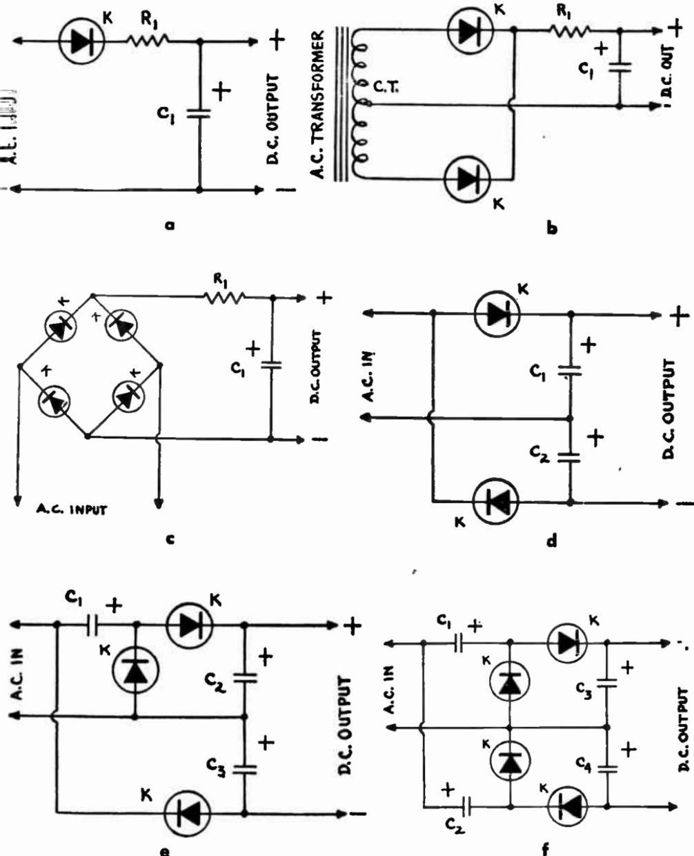
Fig. 10-20.—Basic semiconductor diode Rectifier circuits: (a) Half-Wave; (b) Full-Wave; (c) Full-Wave Bridge; (d) Voltage-Doubler; (e) Voltage-Tripler; (f) Voltage-Quadrupler.
