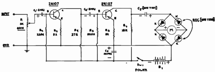
Fig. 9-26.—Schematic of an easily built Audio Level Meter.
