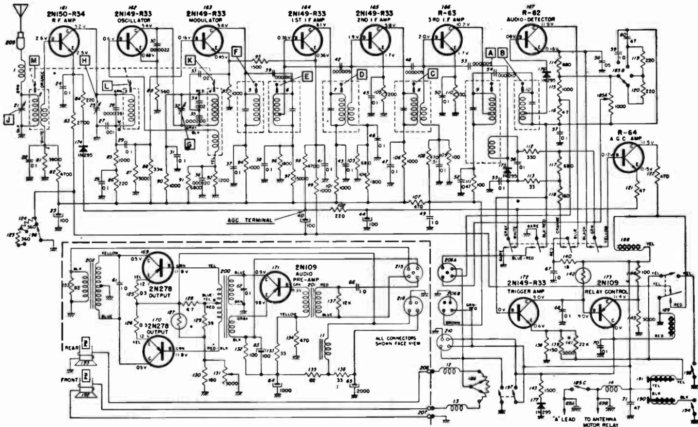
Fig. 14-17.—Schematic wiring diagram of DELCO'S Model 7268085 automobile receiver. Designed for the CADILLAC Brougham, this thirteen-transistor receiver features push-pull output and automatic "search" tuning.
