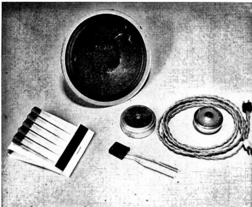
**Fig. 3-5.—Subminiature audio transducers . . . loudspeaker, microphone, and earphone. Bookmatches and transistor give some idea of relative sizes.**
