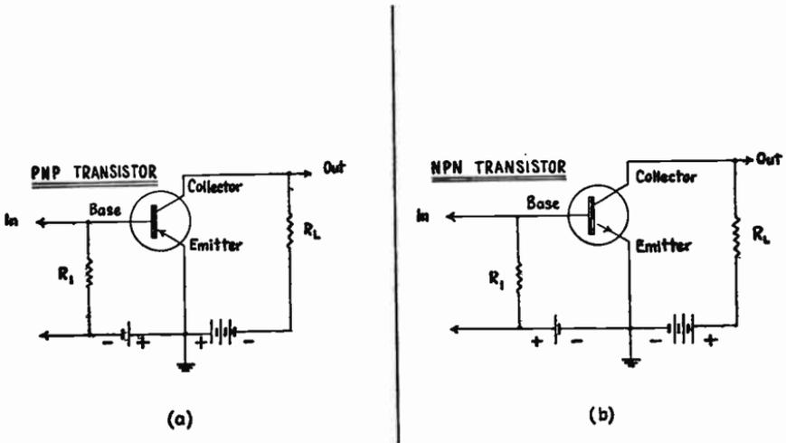
Fig. 1-6.—The schematic symbols and D.C. power supply connections for PNP and NPN transistors are shown here. The only difference in the schematic symbols is in the direction in which the arrowhead points on the line representing the emitter electrode.
