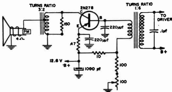
Fig. 14-2.—Typical audio output using a single power transistor. Depending on the transistor used, this type of circuit can deliver from 0.5 to as high as 4.5 watts.
