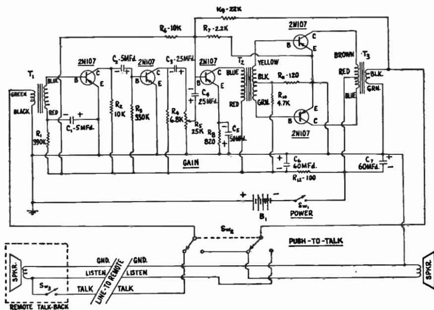
Fig. 7-13.—A transistorized two-station intercom.
