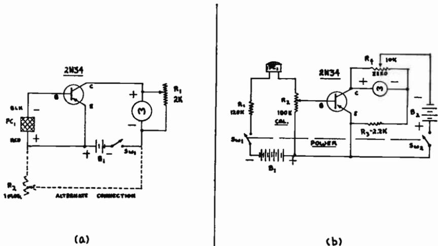
Fig. 9-24.—Two Light Meter circuits—(a) Basic circuit using a selenium photocell and (b) Basic circuit using a Cadmium Sulfide photocell.
