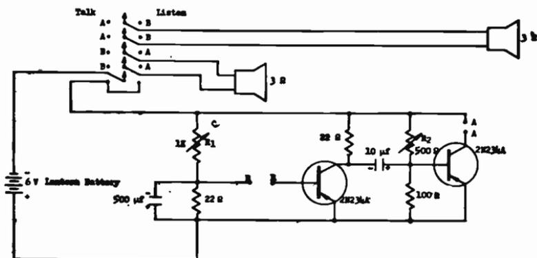
Fig. 14-3.—Circuit of a two-station transformerless intercom. Output level is approximately 1/5 watt.
