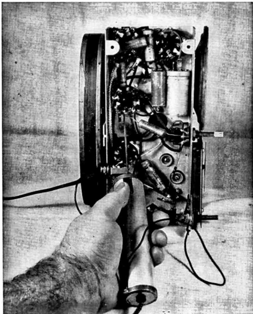
*Fig. 9-29.—Using the Signal Tracer to service a broadcast receiver.*
