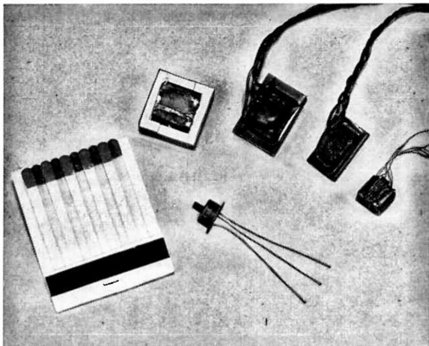
Fig. 3-4.—Subminiature iron-core audio transformers and chokes.
