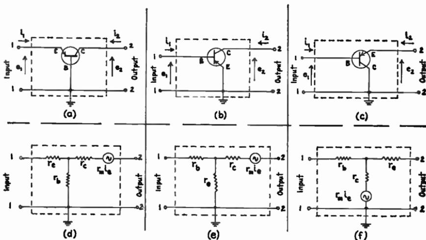
Fig. 12-3.—The three fundamental transistor circuit configurations together with their  $T$  network equivalent circuits. The grounded-base configuration is shown at (a) and (d); the grounded-emitter configuration is shown at (b) and (e); the grounded-collector configuration is shown at (c) and (f).
