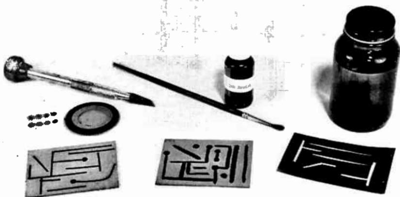
Fig. 13-3.—Three popular techniques used for making up "one-shot" etched circuits in the laboratory. Reading from left to right, the methods shown include tape resist, ink resist, and a photographic negative for a printed circuit layout.
