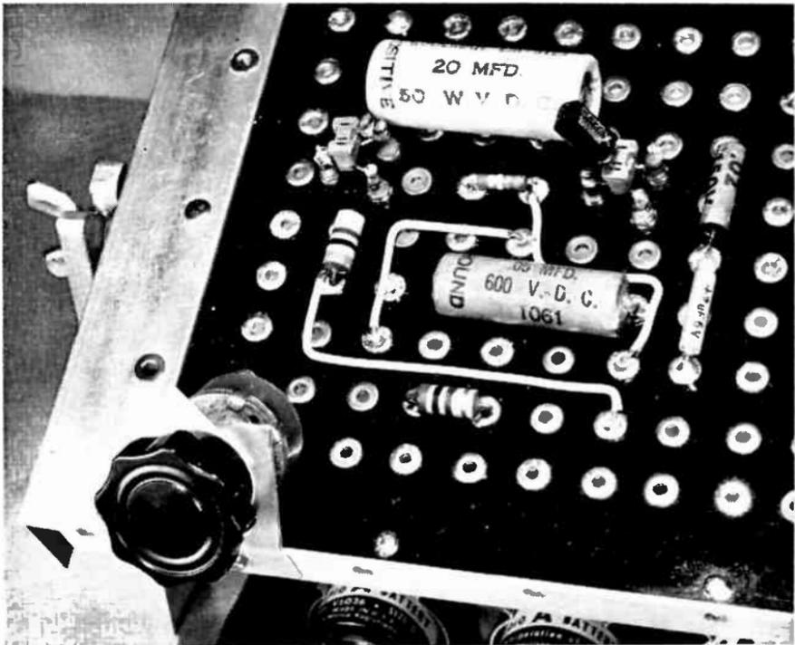
Fig. 13-6.—An experimental transistor circuit wired on a commercial "Breadboard" Chassis. Photo Courtesy The Electratonic Company, Wheaton, Md.
