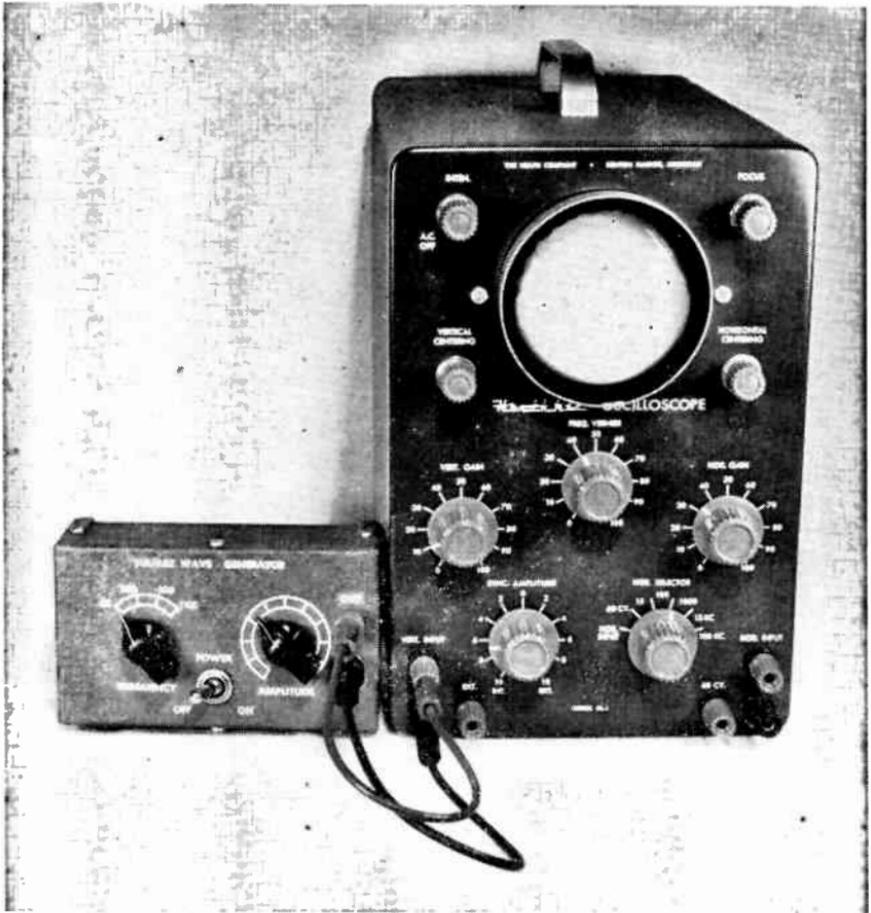
Fig. 9-11.—The Square-Wave Generator connected to an Oscilloscope.
