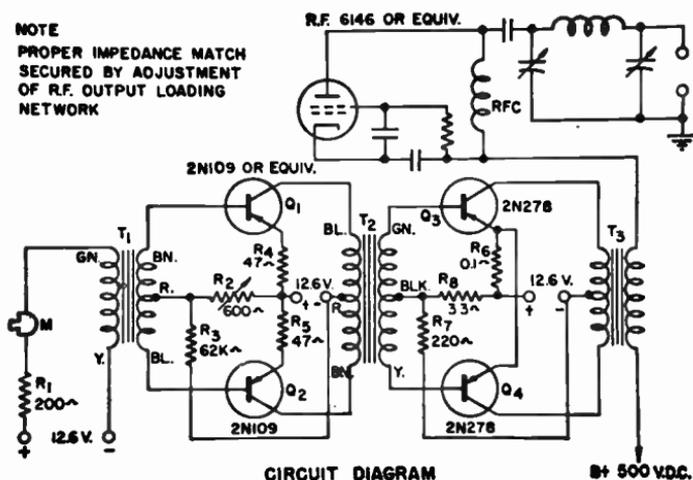
Fig. 14-20.—Wiring diagram of a 25 watt modulator designed for use in a tube-operated Radiotelephone transmitter. As power R.F. transistor become available in quantity, fully transistorized radio transmitters will become feasible.
