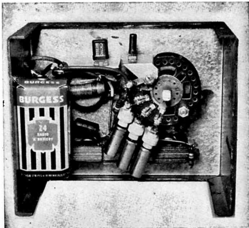
Fig. 9-6.—Interior view of the R.F. Alignment Generator—note crystal mounting.
