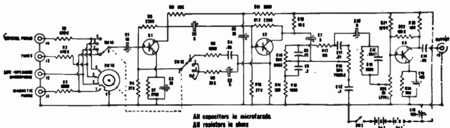
Fig. 14-7.—Schematic diagram of REGENCY'S Model HFT-1 Preamplifier-Equalizer. Designed for use with a High Fidelity power amplifier, this unit has four inputs and provides proper compensation for a variety of phonograph cartridges.
