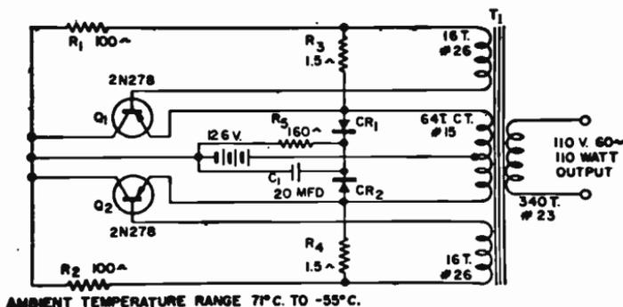
Fig. 14-22.—Schematic of a typical transistorized INVERTER. This type of unit converts D.C., obtained, say, from a storage battery, to A.C. for the operation of line-powered equipment.
