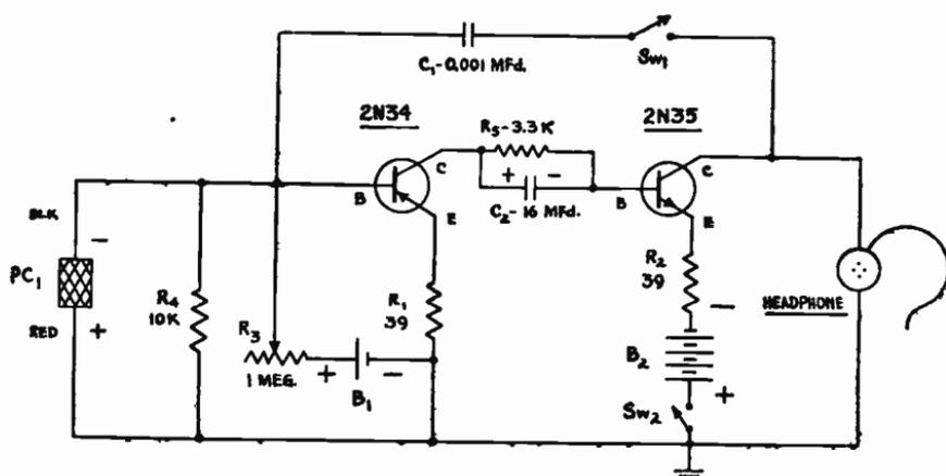
Fig. 10-15.—Circuit for a Light Beam Receiver or Audio Photometer.
