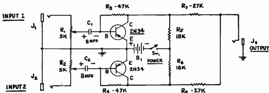
Fig. 7-17.—A transistorized 2-Channel Audio Mixer.
