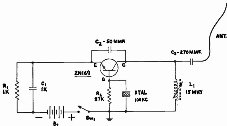
Fig. 8-18.—Diagram of a 100 KC crystal-controlled Calibrator.
