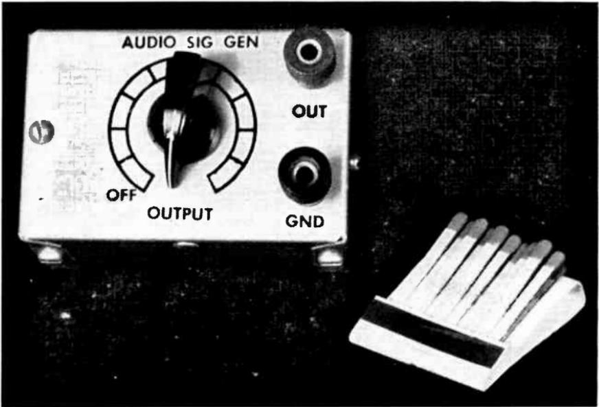
Fig. 9-2.—Exterior view of the Audio Sine Wave Generator—book matches show size.
