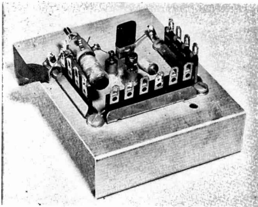
Fig. 8-25.—Breadboarded Frequency Doubler.
