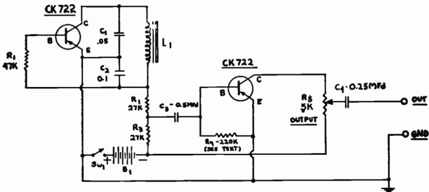
Fig. 9-1.—Circuit for the transistorized Audio Sine Wave Signal Generator.
