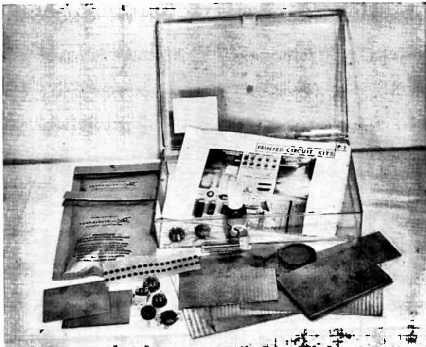
**Fig. 13-2.**—A **TECHNIQUES** Printed Circuit Kit. Designed for small laboratories, this kit includes copper laminate, tube sockets, ink resist, tape resist, a small drill, eyelets, and packets of etching powder, together with full instructions.
