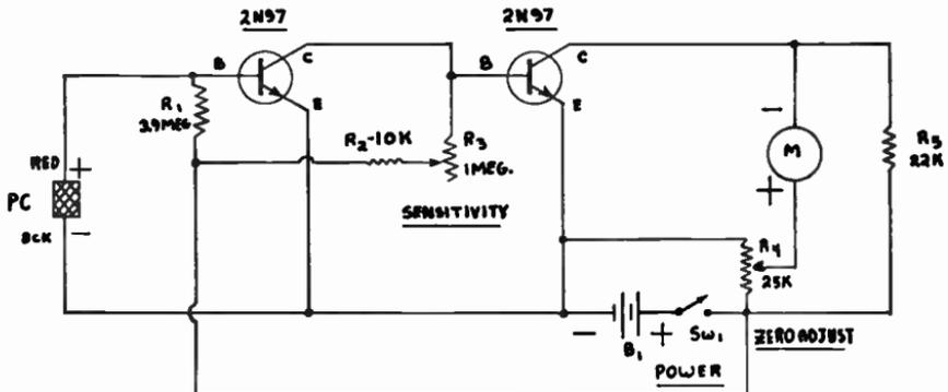
Fig. 9-25.—A very Sensitive Light Meter circuit featuring a cascaded complementary amplifier.
