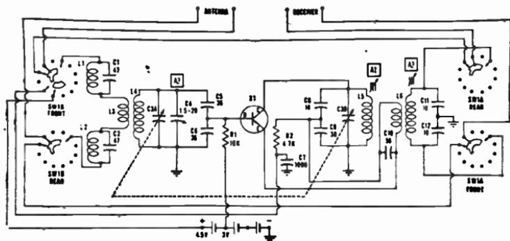
Fig. 14-21.—Circuit of REGENCY'S Model RC-103 FM TeleVerter. This interesting device permits the reception of FM Broadcast Band stations through any standard TV set.
