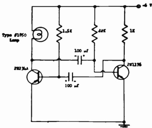
Fig. 14-27.—A transistorized LIGHT FLASHER circuit. Such circuits are used extensively in the manufacture of warning and safety light systems.
