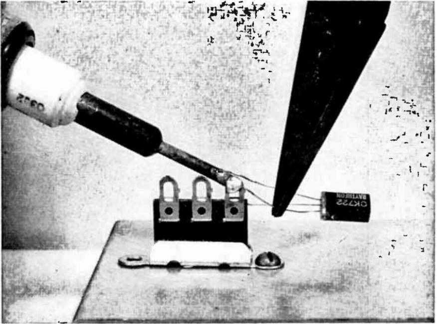
**Fig. 2-9.**—*Proper use of a heat sink in soldering a transistor lead.*
