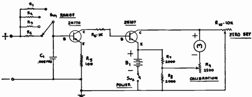
Fig. 9-22.—Schematic of a high impedance transistorized D.C. Voltmeter.
