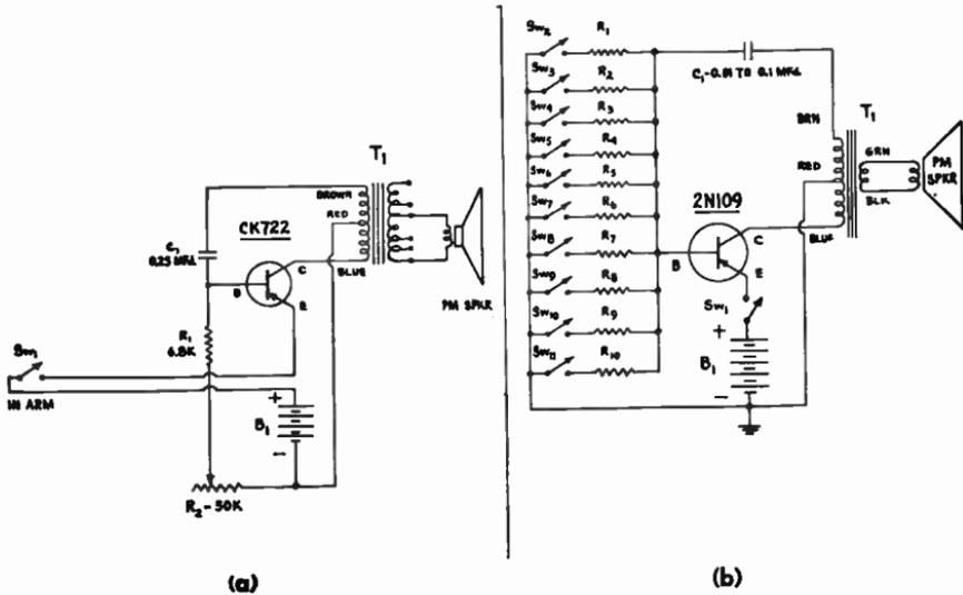
Fig. 10-18.—Two transistorized Musical Toys—(a) an electronic "Banjo"; (b) an electronic "Organ".
