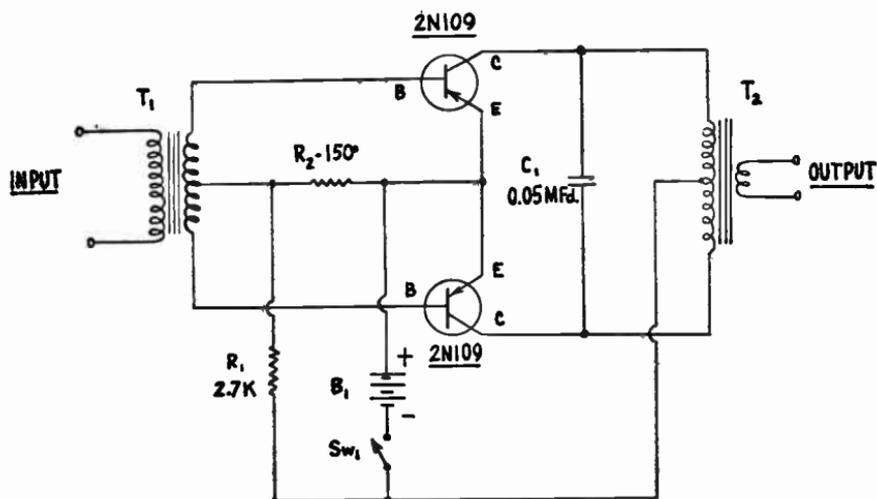
Fig. 7-2.—Basic Push-Pull Power Amplifier.
