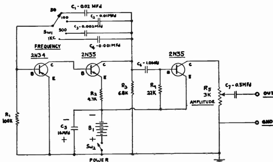
Fig. 9-10.—Schematic of a simple 4-frequency Square-Wave Generator.
