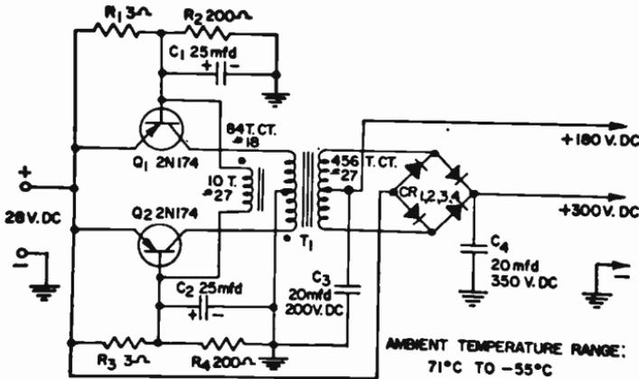
Fig. 14-23.—Wiring diagram of a D.C. to D.C. CONVERTER. Often called a "D.C. Transformer" circuit, this type of equipment converts a relatively low D.C. voltage to a higher voltage; it is often used as a replacement for an electromechanical DYNAMOTOR.
