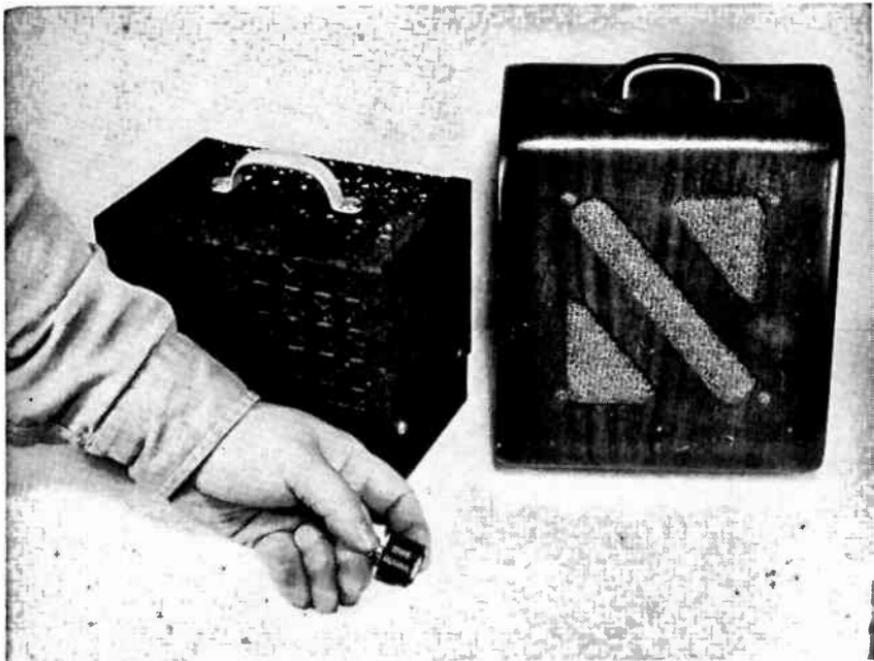
**Fig. 7-20.**—The transistorized P.A. System, less microphone. The loudspeaker is in the floor baffle to the right, the amplifier itself in the case to the left. The type of power transistor used is shown.
