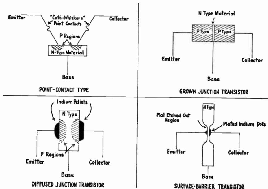
Fig. 1-3.—The four types of transistor construction are shown schematically in this sketch.
