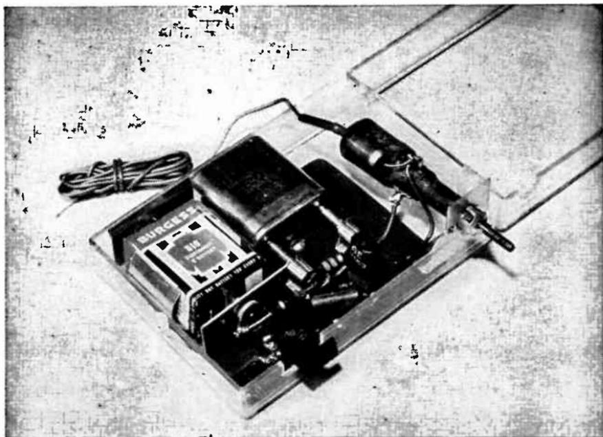
Fig. 8-20.—Interior view of the Crystal Calibrator.
