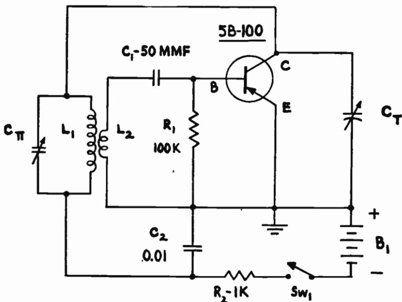
Fig. 8-26.—Schematic of a High Frequency Oscillator featuring a "Surface Barrier" transistor.
