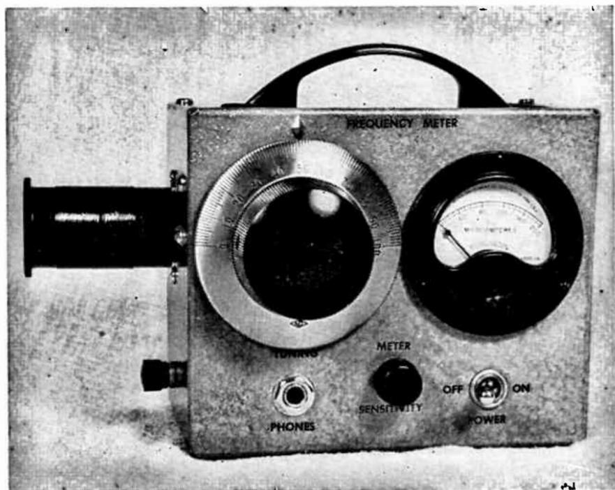
Fig. 8-23.—Exterior view of the R.F. Frequency Meter.
