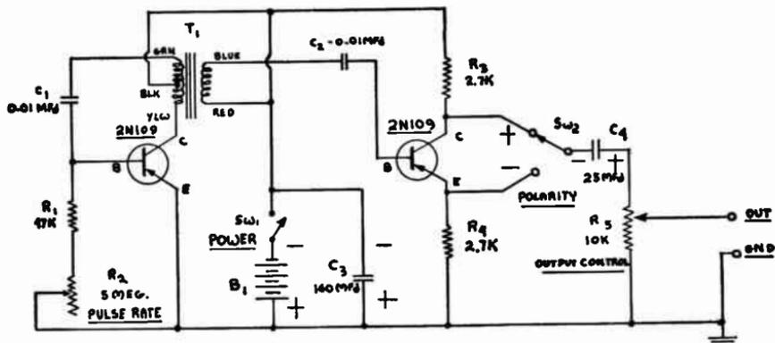
Fig. 9-13.—Circuit of a transistorized Pulse Generator delivering both positive-going and negative-going pulses.
