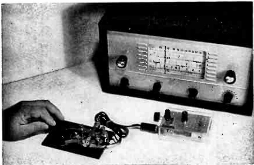
*Fig. 8-16.—Using the Wireless C.P.O.*
