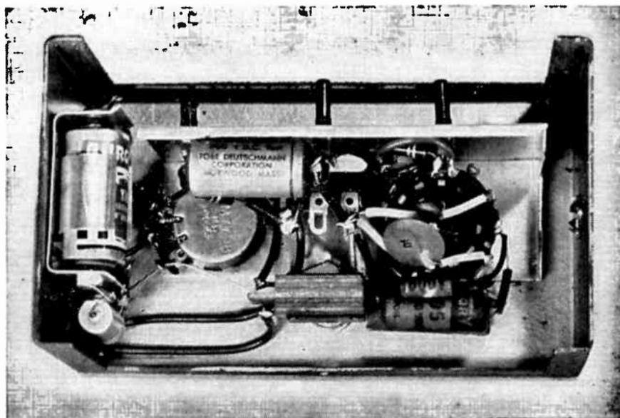
Fig. 9-12.—Interior view of the transistorized Square-Wave Generator.
