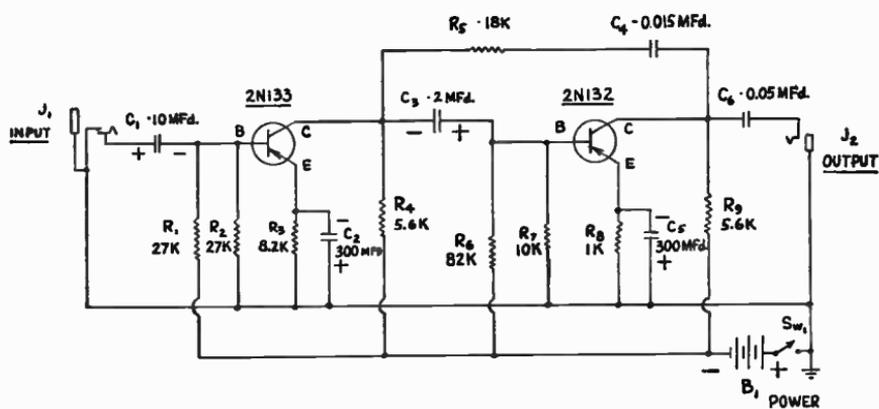
Fig. 7-21.—Circuit of a transistorized Hi Fi Preamplifier
