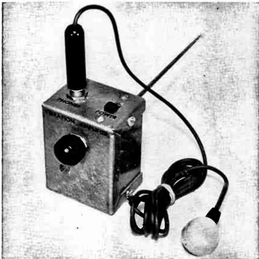
*Fig. 7-6.—Exterior view of the electronic "Stethoscope"*
