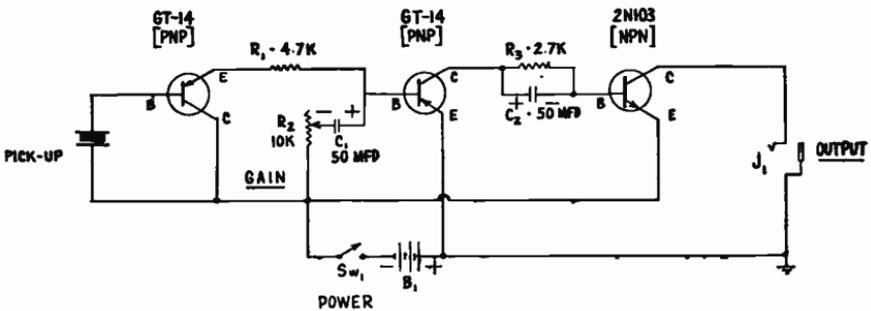
Fig. 7-5.—A transistorized electronic "Stethoscope".
