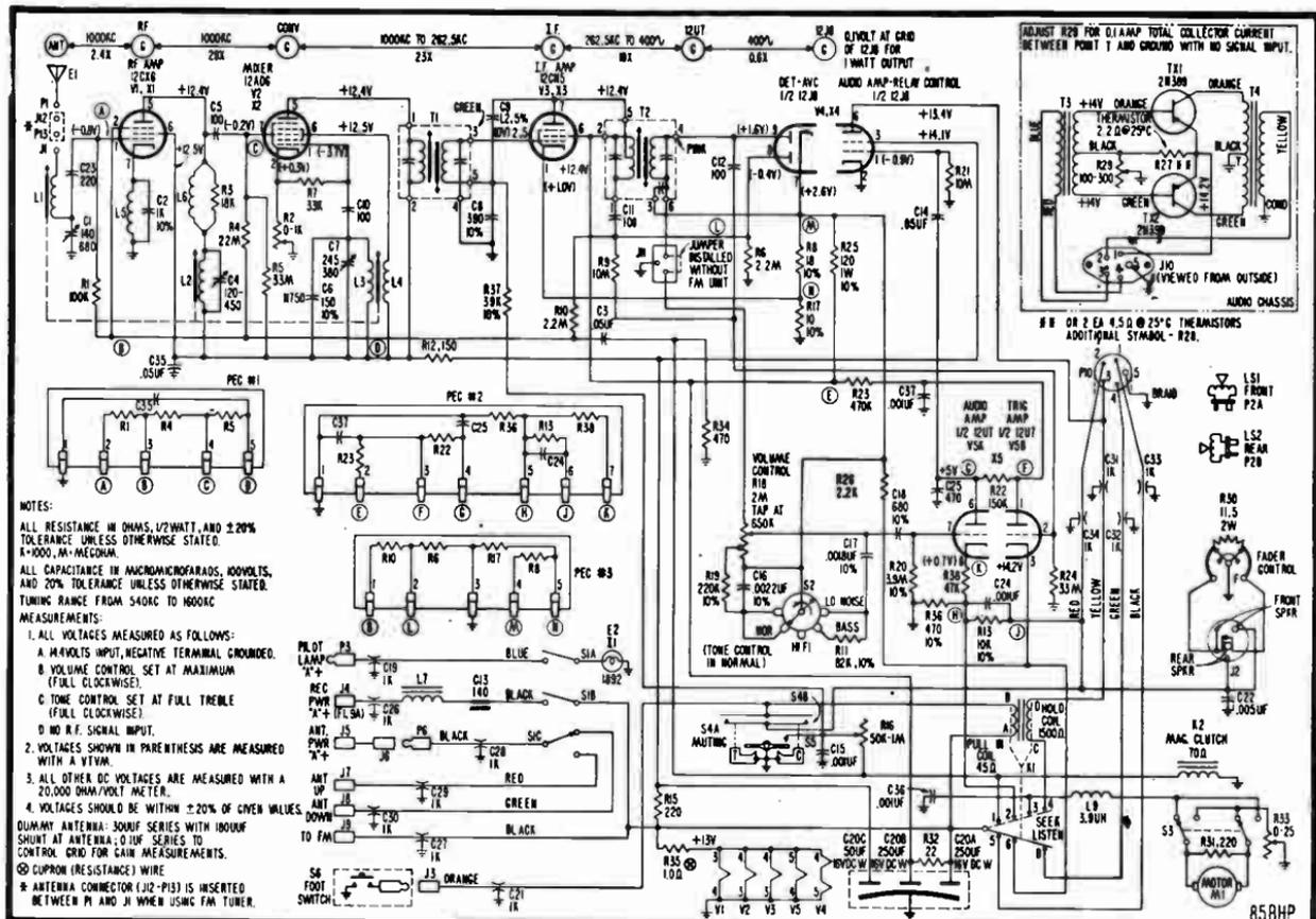
Fig. 14-11.—Circuit diagram of BENDIX'S Model R858HP car radio. This set was designed for installation in 1958 Lincoln cars and is equipped with a transistORIZED push-pull power amplifier. As in other hybrid receivers, vacuum tubes are used in the R.F. and I.F. stages.
