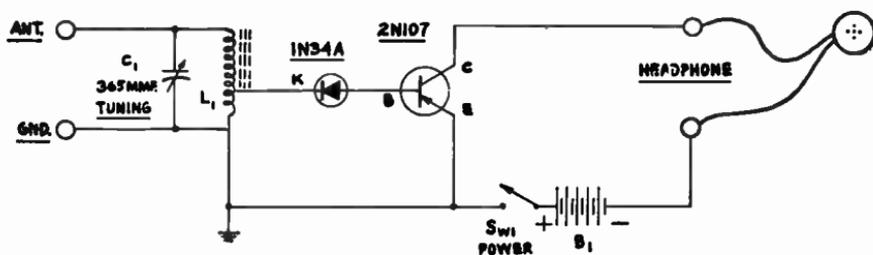
Fig. 8-1.—Simple transistorized Receiver using a diode detector.
