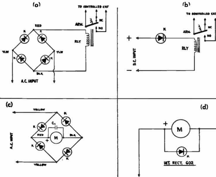
Fig. 10-27.—Semiconductor diode Relay and Meter applications: (a) Sensitive A.C. Relay; (b) Polarized Relay; (c) A.C. Meter; (d) Meter Protection Circuit.
