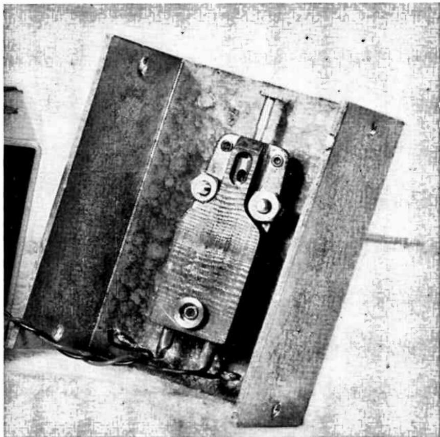
Fig. 7-7.—Detail of crystal cartridge mounting.
