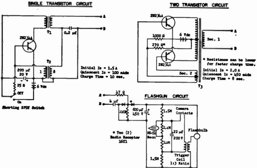
Fig. 14-25.—Schematic diagrams of typical transistorized photoflash circuits. Basically, the transistor serves in a D.C. to D.C. CONVERTER, charging a high-voltage capacitor from a low-voltage source.
