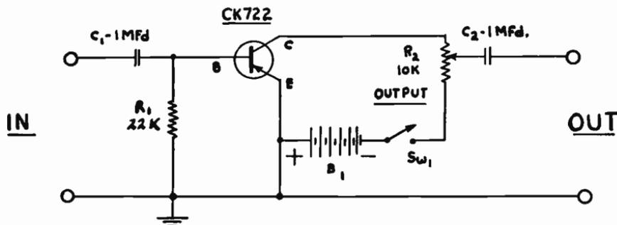
Fig. 9-16.—Schematic of a simple, but useful, test instrument—a Sine Wave Clipper.
