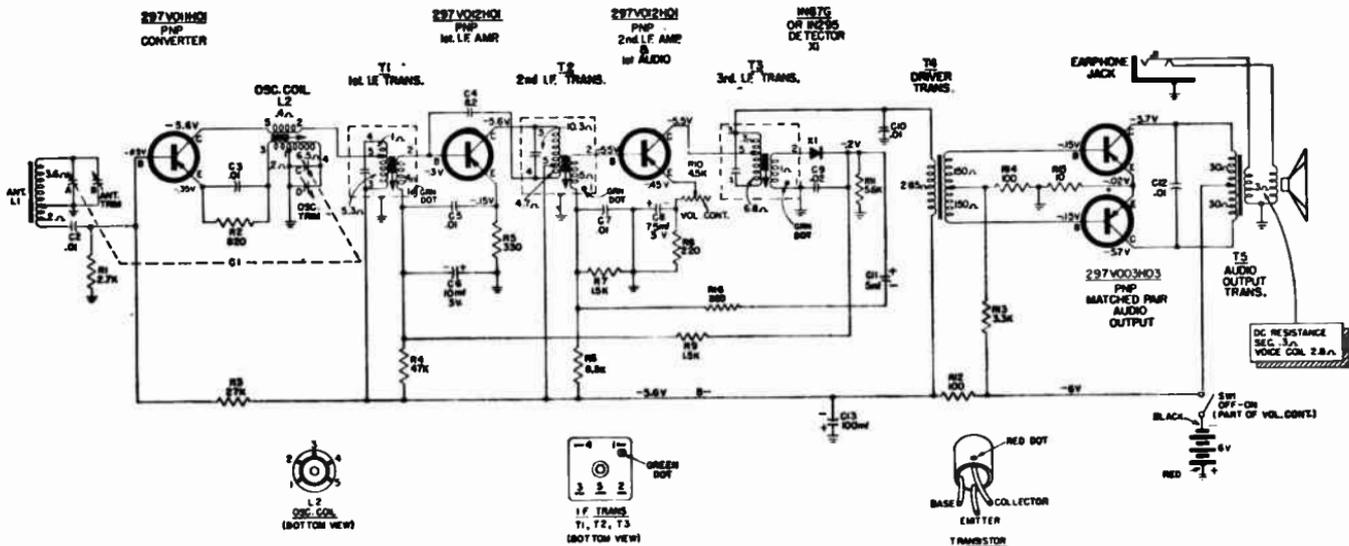
Fig. 14-14. — Circuit of WESTINGHOUSE Models H-655P5 and H-656P5 receivers. These five-transistor sets feature a push-pull output stage, and a reflexed I.F. amplifier.
