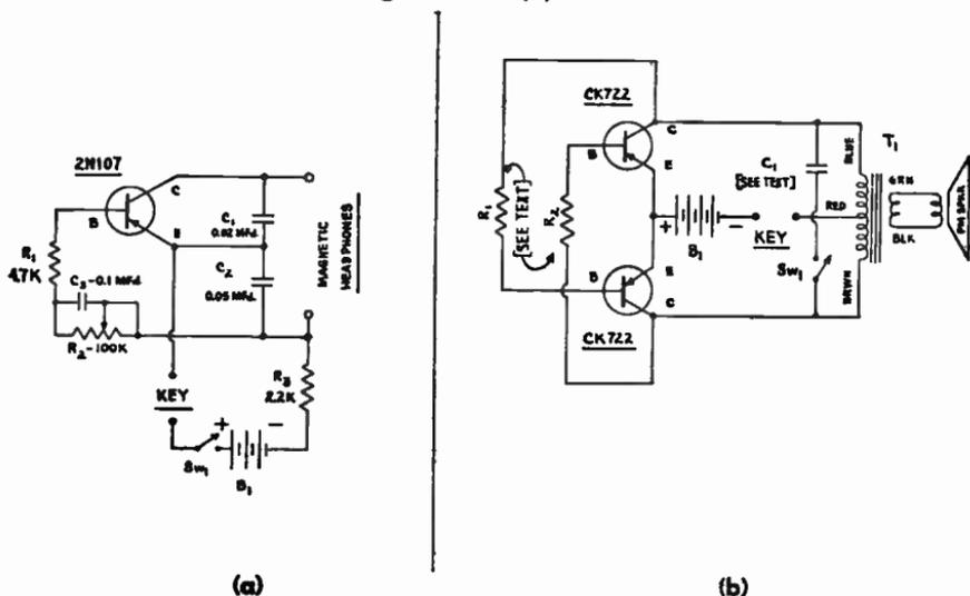
Fig. 10-12.—Diagrams for two easily built Code Practice Oscillators—(a) Headphone type; (b) Loudspeaker type.
