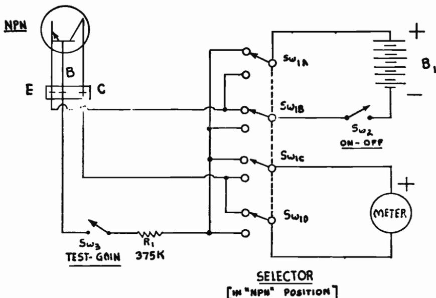
Fig. 9-18.—Circuit for a simple Transistor Checker.
