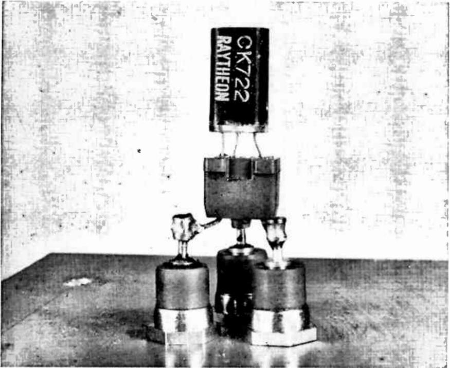
*Fig. 2-5.—Detail of transistor socket mounting.*
