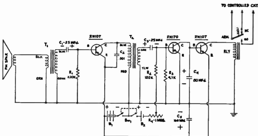
Fig. 10-11.—Circuit of a transistorized Sound Switch or voice-controlled relay.
