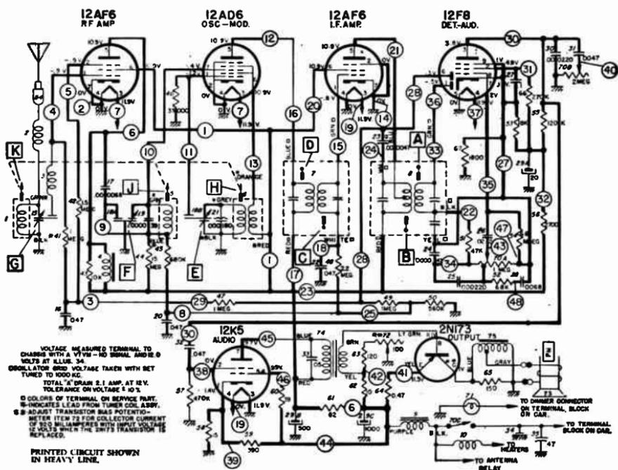
Fig. 14-9.—Wiring diagram of the PONTIAC Model 988671 automobile radio. A "hybrid" receiver using five tubes and a single transistor, this set was manufactured by DELCO.
