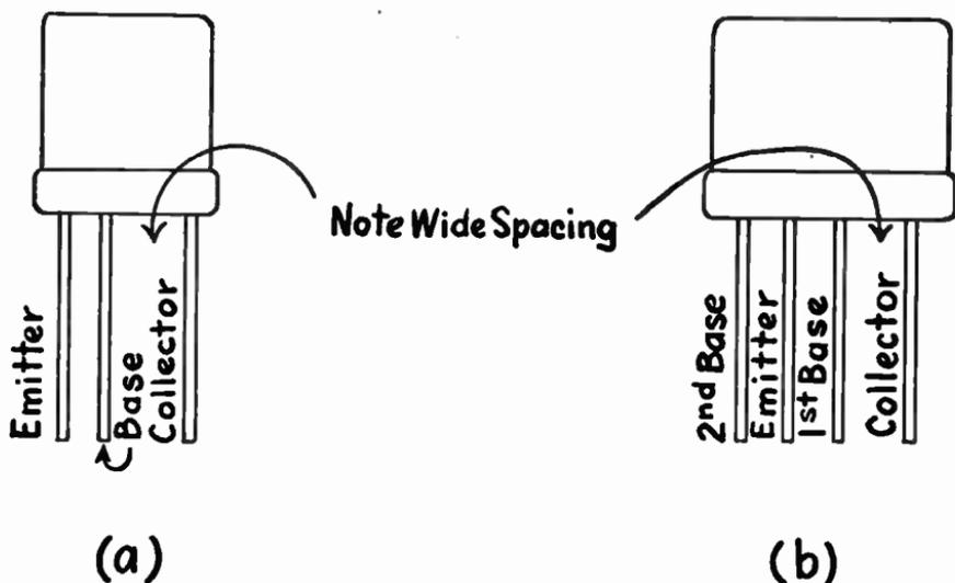
Fig. 2-7.—Pin connections for standard triode (a) and tetraode junction (b) transistors.
