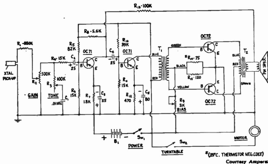
**Fig. 7-23.**—Circuit of a high quality transistorized *Phonograph Amplifier*. This unit might also be used as a *Guitar* or similar "Music" amplifier, or even as a low power P.A. system.
