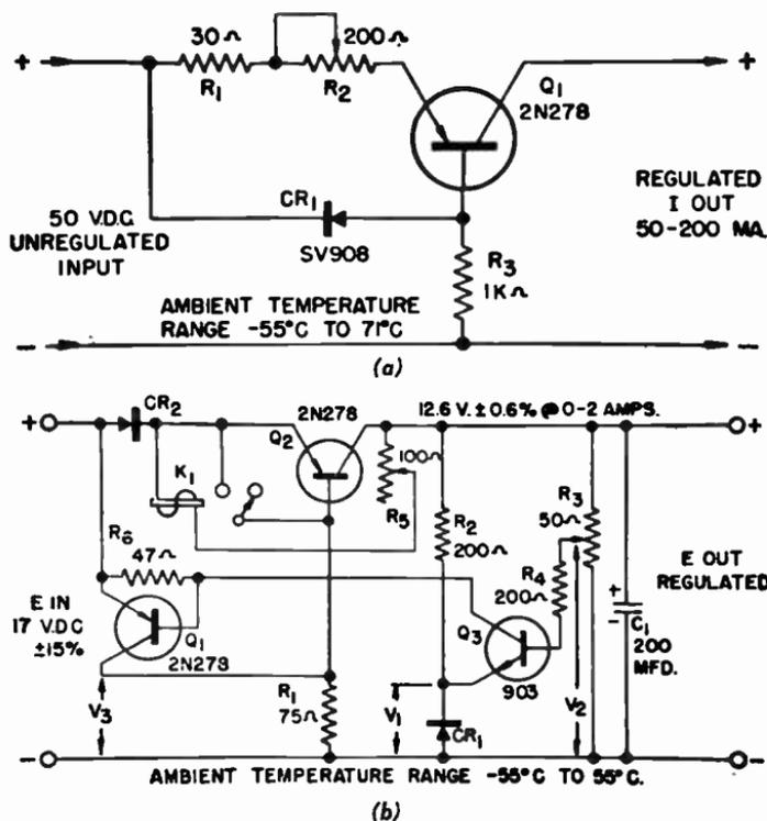
Fig. 14-24.—Typical regulator circuits — (a) Series CURRENT regulator and (b) VOLTAGE regulator. Both serve to maintain a constant output with changes in input and loading.
