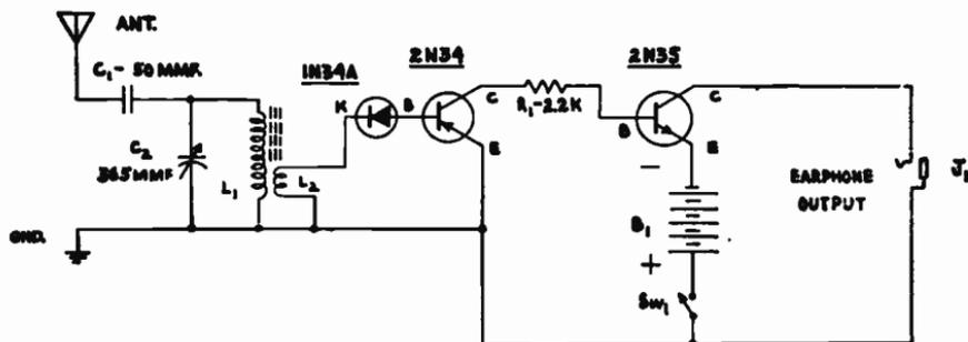
Fig. 8-5.—Schematic diagram of a Pocket Receiver using a two-stage complementary amplifier.
