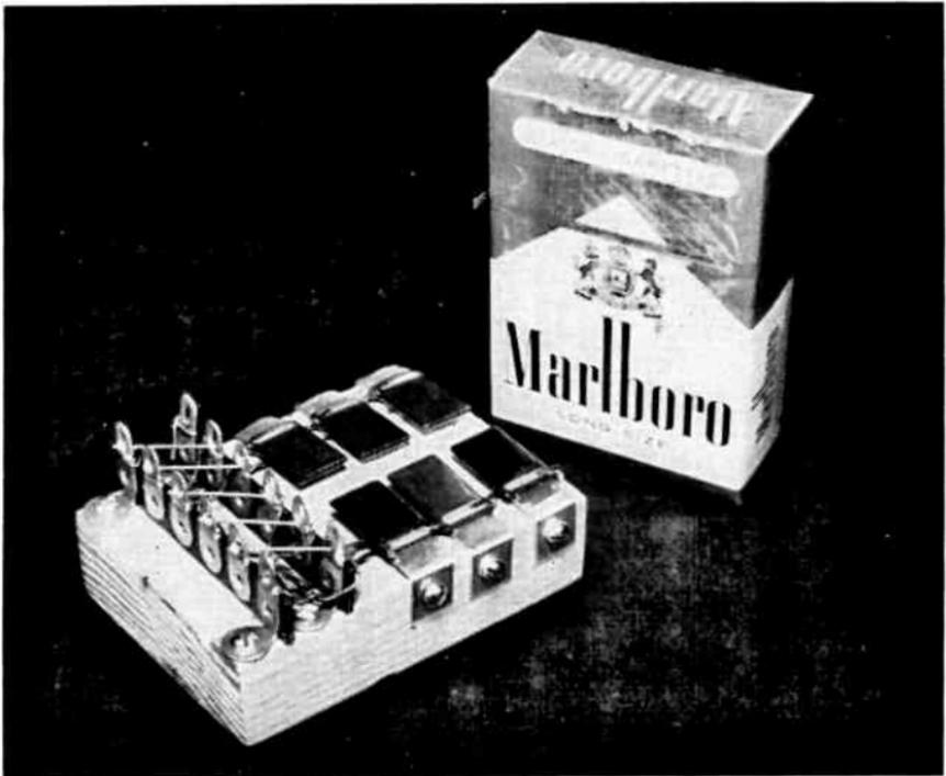
Fig. 10-29.—Easily assembled "Sun Battery" . . . will power a simple receiver, an audio amplifier, or a Code Practice Oscillator, or even a low-power transmitter in full sunlight.
