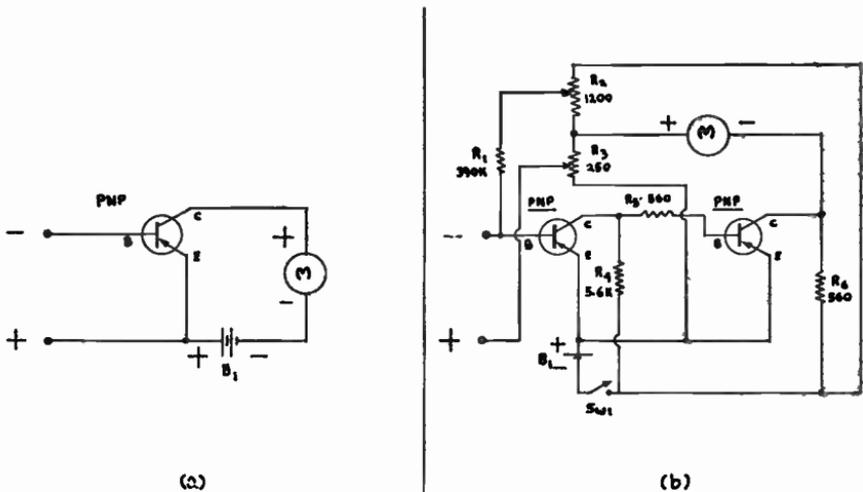
Fig. 9-21.—Circuits for two transistorized Meter Amplifiers—(a) Single Stage and (b) Cascaded Stages.
