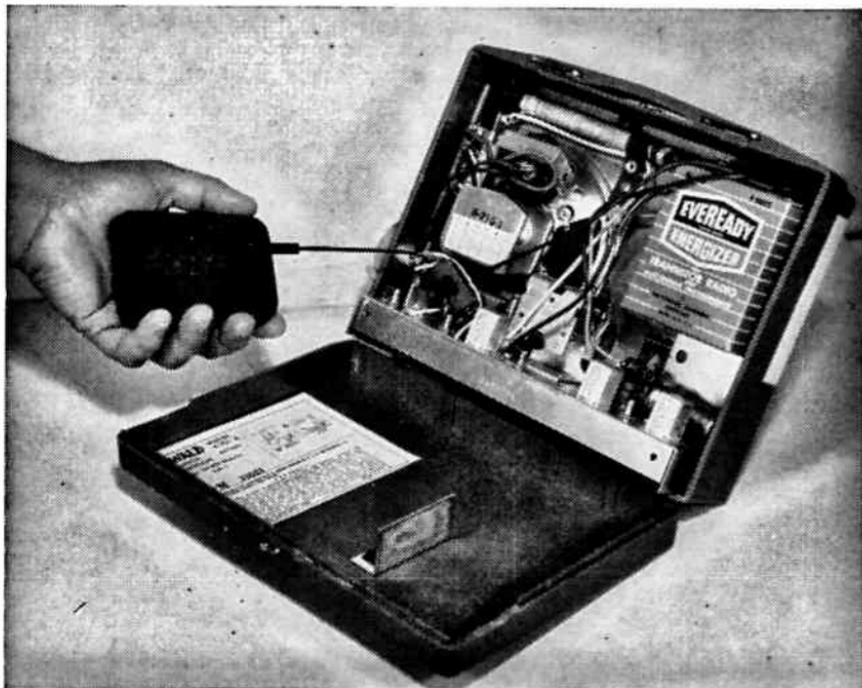
Fig. 9-9.—Using The Signal Squirrelter to service a transistorized receiver.
