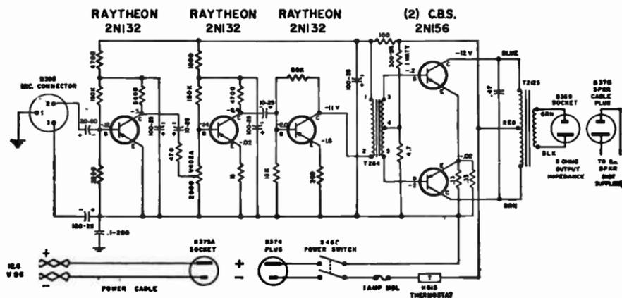
Fig. 14-5.—Circuit of the BOGEN Model BT12 transistorized P.A. Amplifier. With an output of 4 watts, this amplifier is designed for use with a moderate impedance (200 to 500 ohm) microphone.
