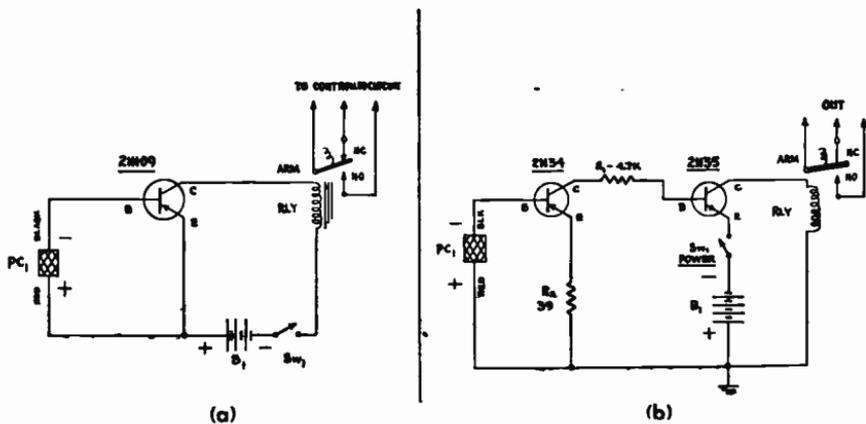
Fig. 10-6.—Two "Electric Eye" relay circuits (a) Basic circuit; (b) Sensitive version.
