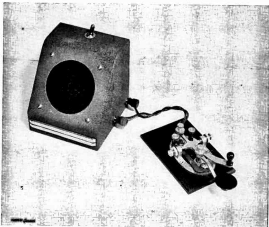
*Fig. 10-14.—Loudspeaker type Code Practice Oscillator.*
