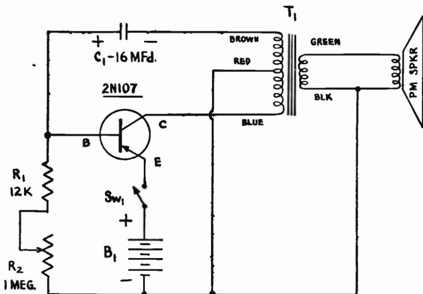
Fig. 10-16.—Schematic diagram of a transistorized *Metronome*.
