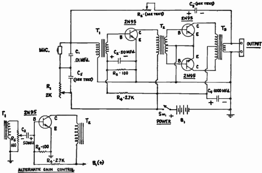
Fig. 7-19.—A transistorized P.A. System.
