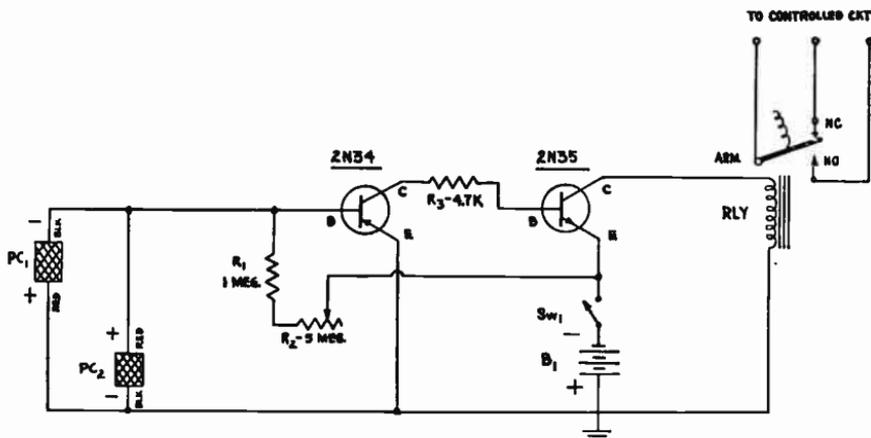
Fig. 10-7.—Schematic of a transistorized "ON-OFF" Light Control circuit.
