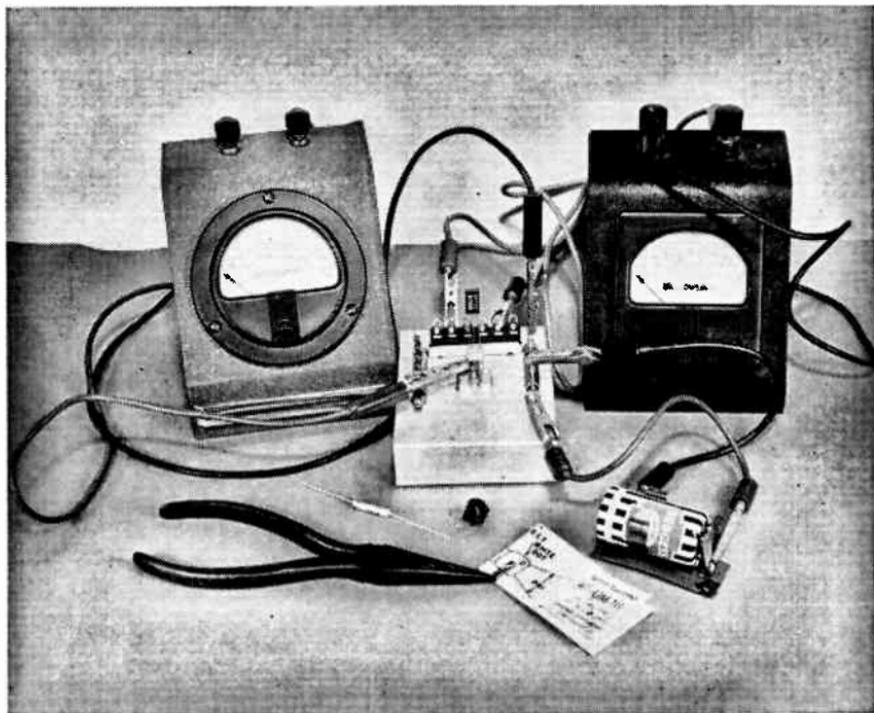
*Fig. 2-6.—A typical experimental set-up for checking a breadboarded transistor circuit.*
