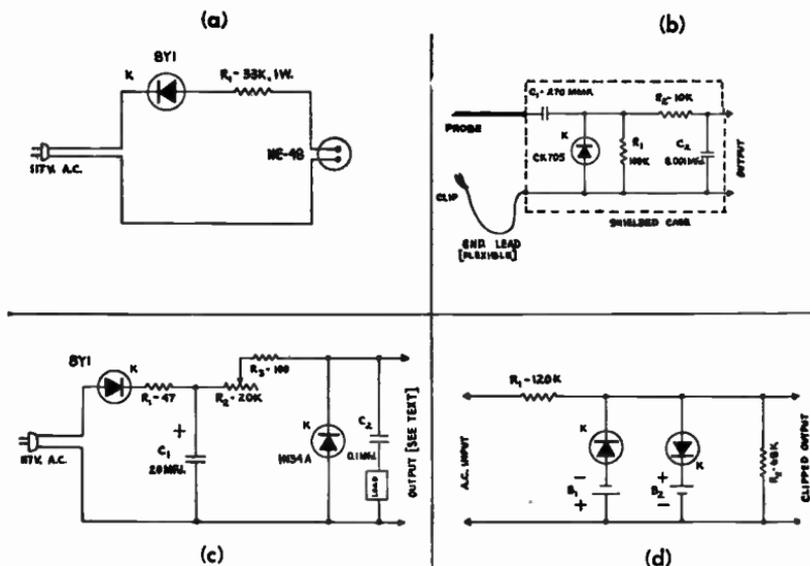
Fig. 10-24.—General semiconductor applications: (a) 60 Cycle Stroboscope; (b) Signal Tracing Probe; (c) Zener Oscillator; (d) Clipper.
