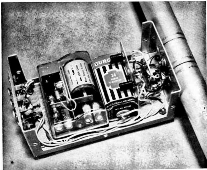
Fig. 10-9.—Interior view of the "ON-OFF" Light Controlled Relay.
