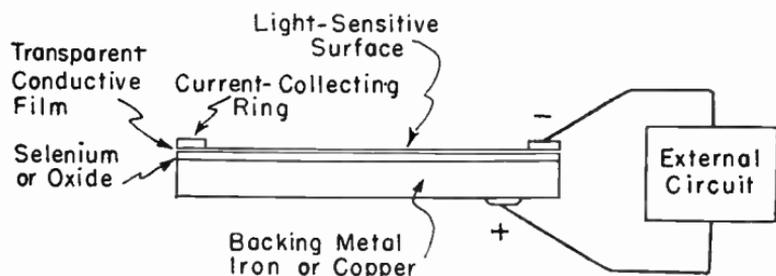
FIG. 1.—Principal Parts of Barrier Layer Photocells.
