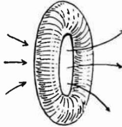
FIG. 2.—Magnetic Field of Toroid
