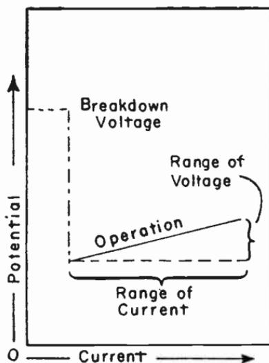
FIG. 2.—Relations between Voltage and Current During Operation of Voltage Regulator.
