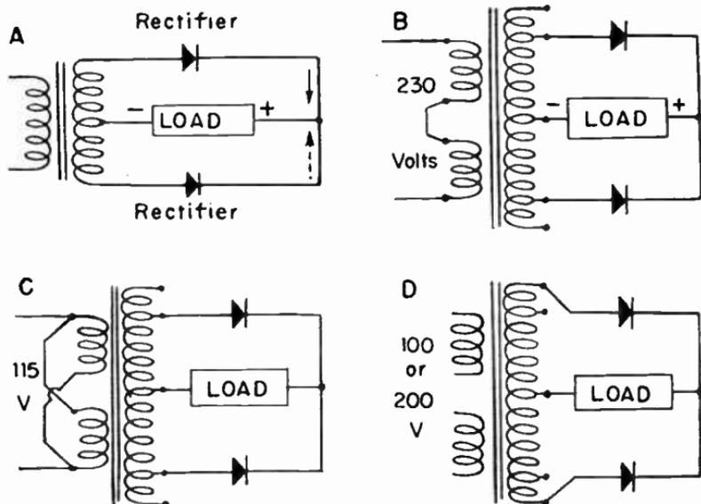
FIG. 5.—Contact Rectifiers in Full-wave Circuits.
