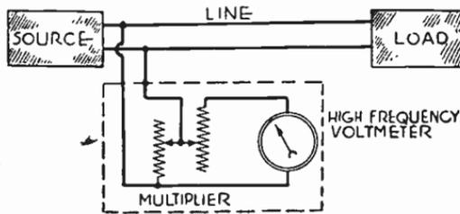
FIG. 1.—Simple Form of Volume Indicator.
