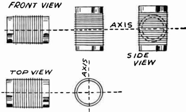
Relative Coil Positions for Minimum Coupling.
