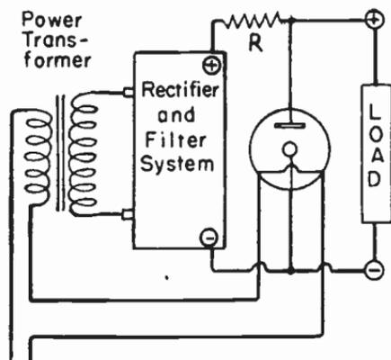
FIG. 3.—Connections Used with Single Regulator Tube.
