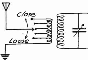
FIG. 3.—Tapped Coil for Antenna Coupling.
