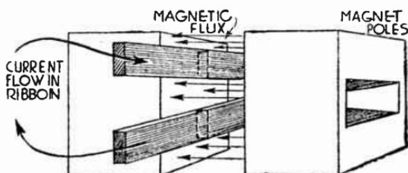
FIG. 8.—Magnetic Action in Light Valve.
