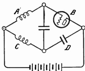
FIG. 10.—The Rice Balanced Circuit in Bridge Form.
