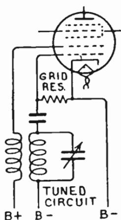
FIG. 24.—Pentagrid Oscillator Circuit.
