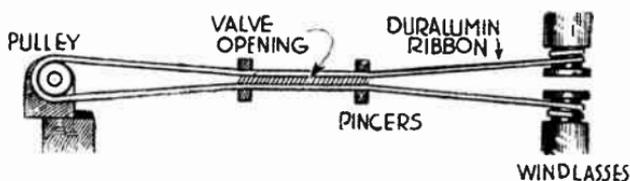
FIG. 7.—Principle of Western Electric Light Valve.
