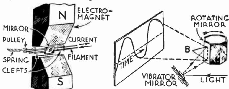
FIG. 2.—Principle of the Duddell Oscillograph.
