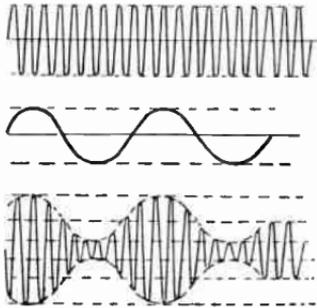
FIG. 7.—Combining the Frequencies in Modulation.
