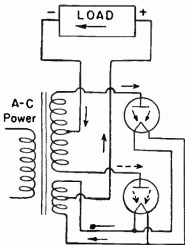
FIG. 1.—Two Filament-cathode Tubes in Full-wave Rectifier.
