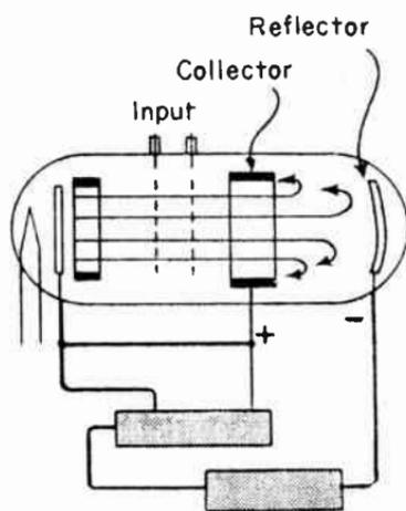
FIG. 2.—Method of Changing Velocity to Intensity Modulation.
