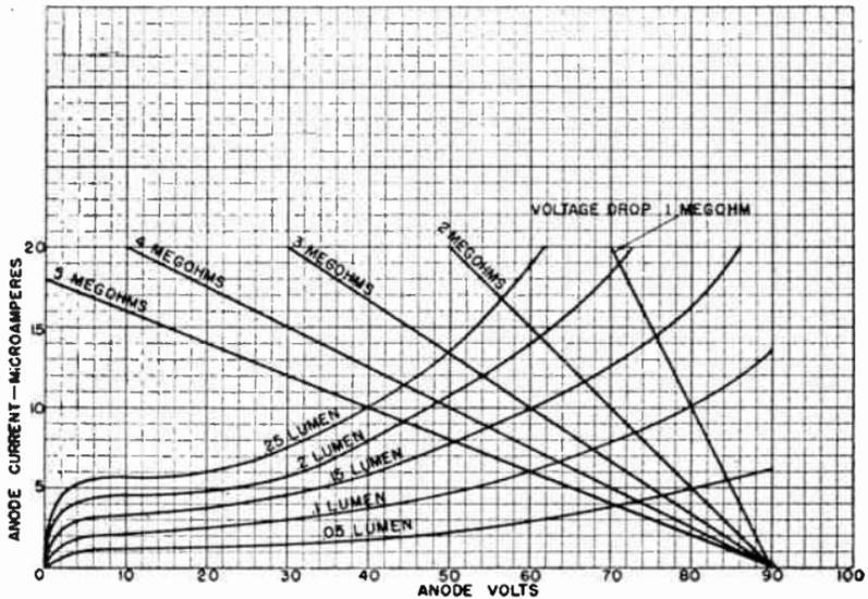
FIG. 9.—Load Lines Showing Phototube Performance.
