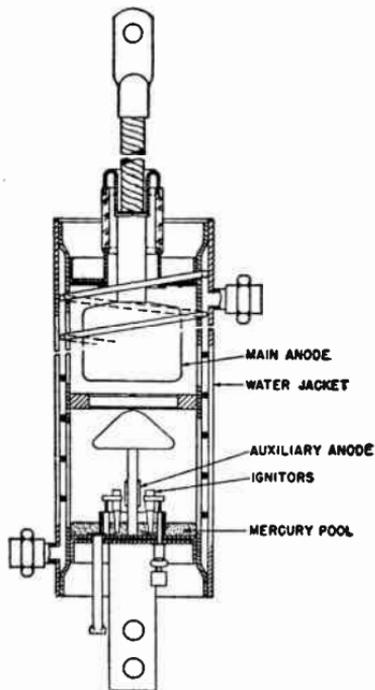
FIG. 3.—A General Electric Sealed Ignitron Having Two Ignitons and an Auxiliary Anode.
