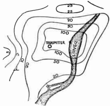
FIG. 11.—Variations in Radio Field Intensity.
