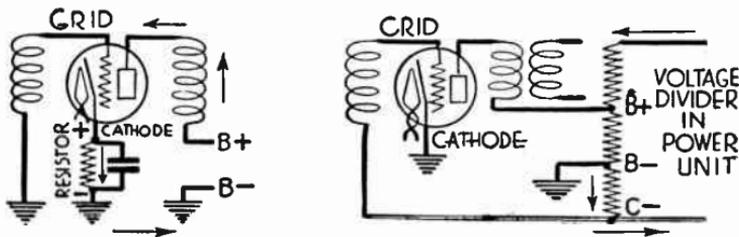
FIG. 6.—Biasing for Heater Tubes.
