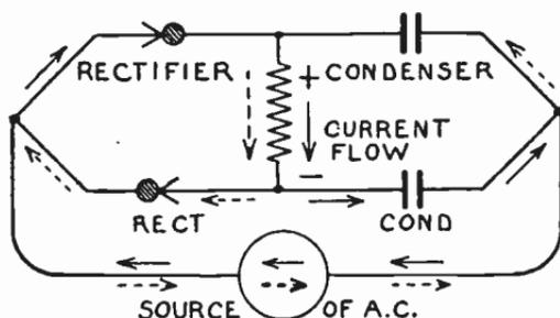
FIG. 2.—Equivalent Circuit for Voltage Doubler.
