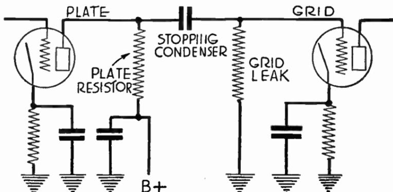
FIG. 1.—Resistance-capacity Coupled Amplifier.
