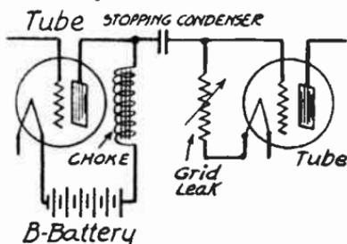
FIG. 2.—The Impedance Coupled Audio Amplifier.
