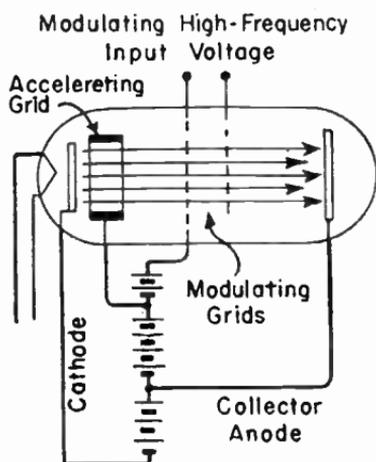
FIG. 1.—The Elements Employed for Velocity Modulation.
