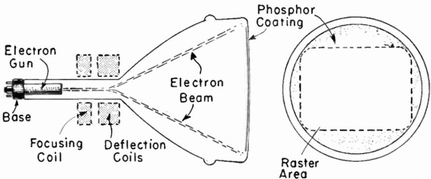
FIG. 5.—Television Picture Tube for Magnetic Deflection.
