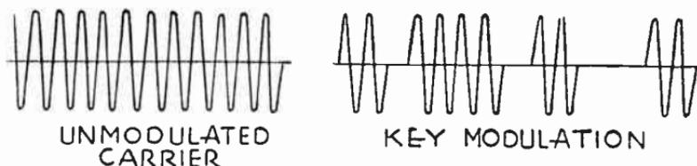
FIG. 1.—Unmodulated Carrier Wave and Key Modulation.
