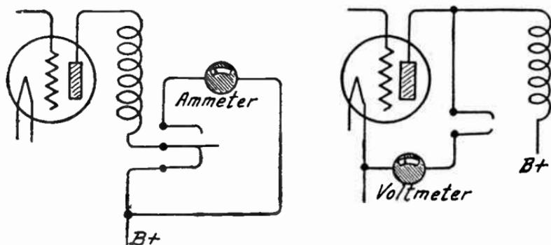
FIG. 4.—Meter Connections Made with Switches.
