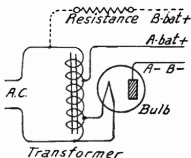
FIG. 3.—Two Voltages with Auto-transformer.
