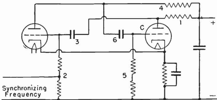
FIG. 3.—Circuit of Multivibrator Oscillator.
