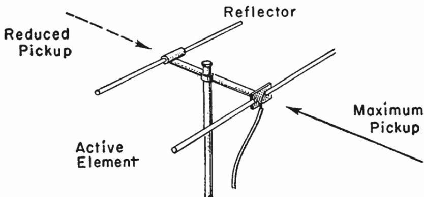
FIG. 15.—Half-wave Dipole with Reflector.
