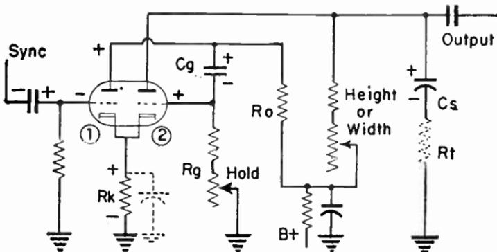
FIG. 27.—Multivibrator Oscillator for Television Sweep Circuits.
