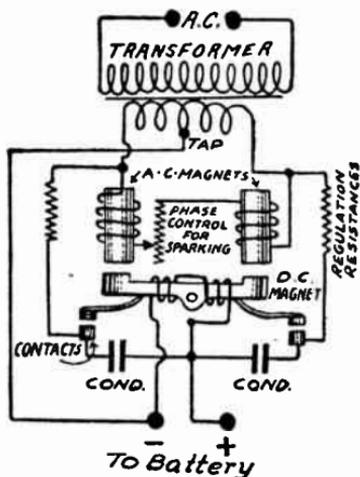
FIG. 1.—Full-wave Vibrating Rectifier.
