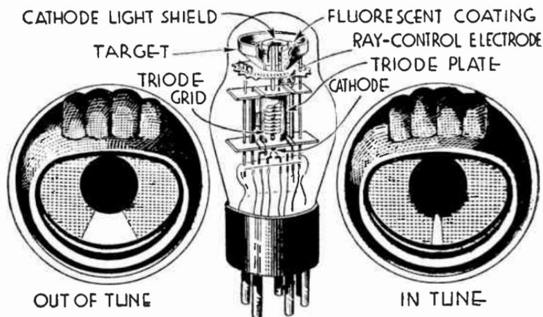
FIG. 13.—Cathode Ray Tuning Meter
