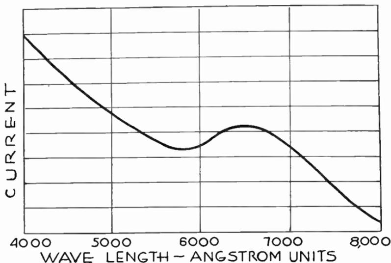
FIG. 5.—Color Sensitivity of Selenium Cell.
