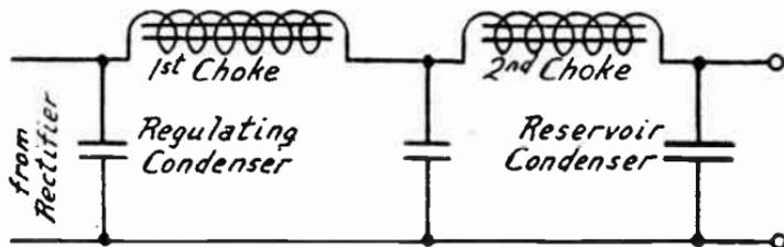
FIG. 5.—Power Unit Filter System with Three Condensers.
