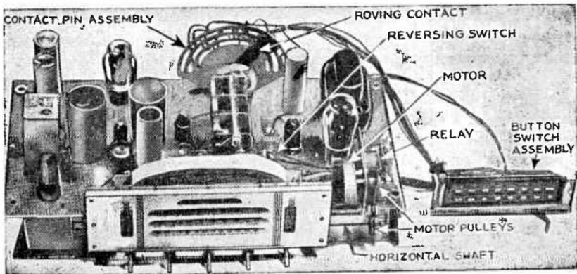
FIG. 1.—General Electric Touch Tuning Chassis.
