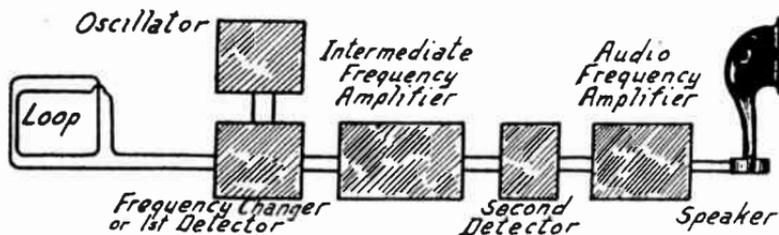
FIG. 2.—Parts Used in Early Superheterodynes.
