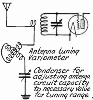
FIG. 2.—Use of Variometer for Antenna Tuning.
