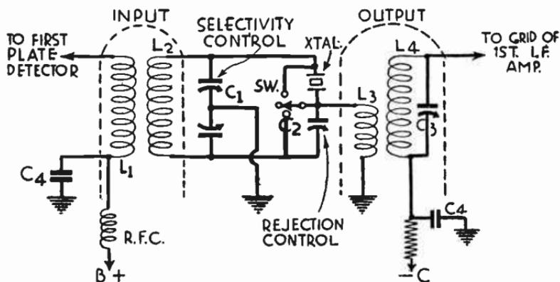
FIG. 15.—Crystal Filter Circuit
