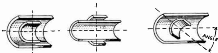
Effect of Coil Position on Coupling Coefficient.
