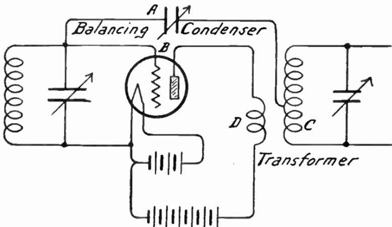
FIG. 2.—Neutrodyne Method of Balancing.
