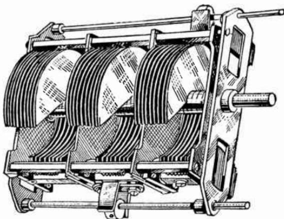
A Ganged Condenser for Tuning Three Circuits.
