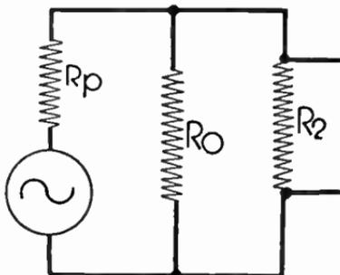
FIG. 4.—Coupling Circuit without Condenser.
