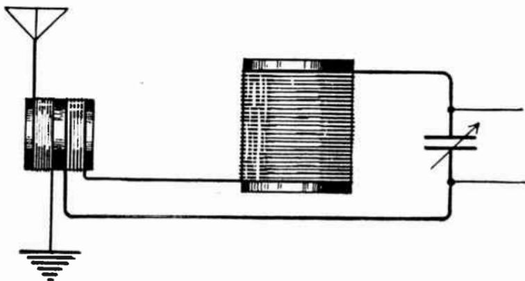
FIG. 2.—Separate Coupling Coil for Antenna Circuit.
