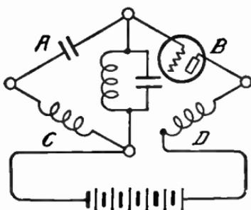
FIG. 9.—The Neutrodyne Balanced Circuit in Bridge Form.
