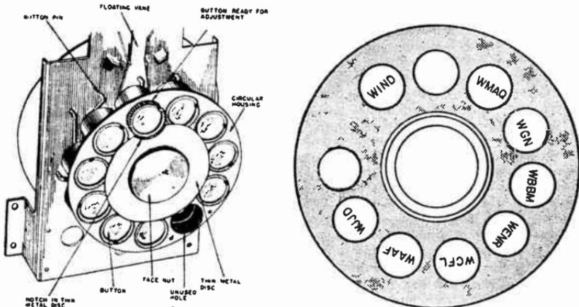
FIG. 6.—Telephone Type Tuning Dial.
