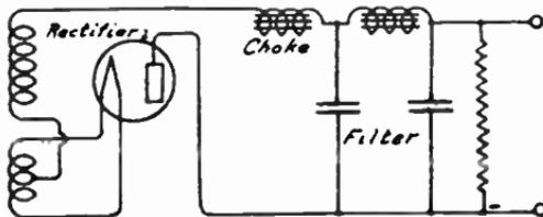
FIG. 8.—Filter with Choke Input.
