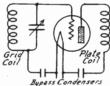
FIG. 1.—Grid and Plate Coils Entering into Regeneration.
