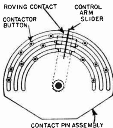
FIG. 3.—Roving Contact Pin Assembly.
