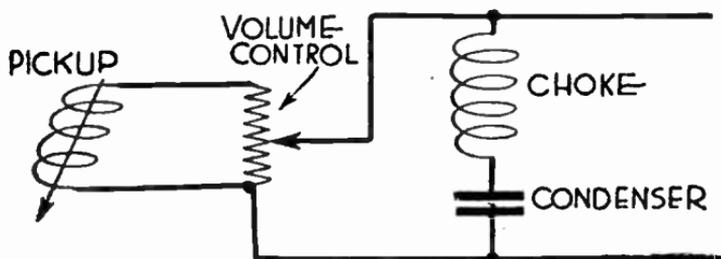
FIG. 10.—Connections for Scratch Filter.
