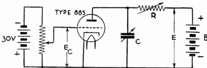
FIG. 11.—Thyatron Sweep Circuit Oscillator.
