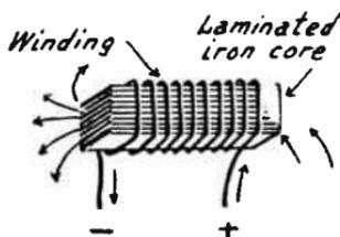
FIG. 4.—An Electromagnet with Its Field
