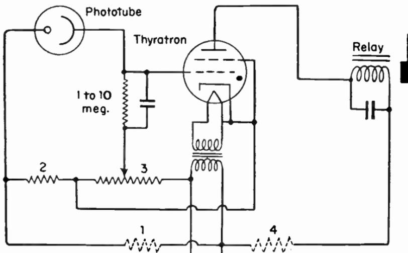
FIG. 12.—Phototube and Thyratron for Pull-in of Relay upon Increase of Light.
