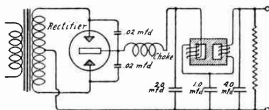
FIG. 9.—Connection of Bucking Coil Filter Choke.
