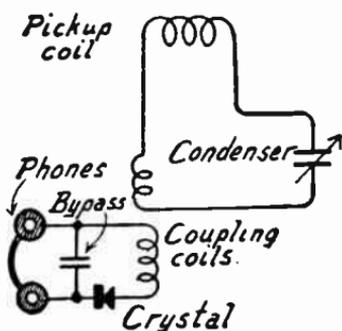
FIG. 3.—Inductively Coupled Indicator Circuit for Frequency Meter.
