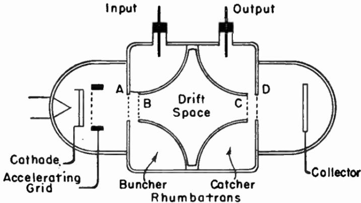
FIG. 1.—Arrangement of Elements in a Klystron.
