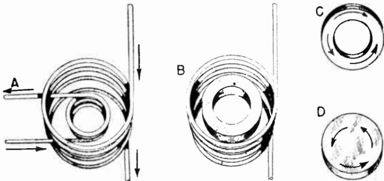
FIG. 1.—Elementary Principle of Induction Heating.
