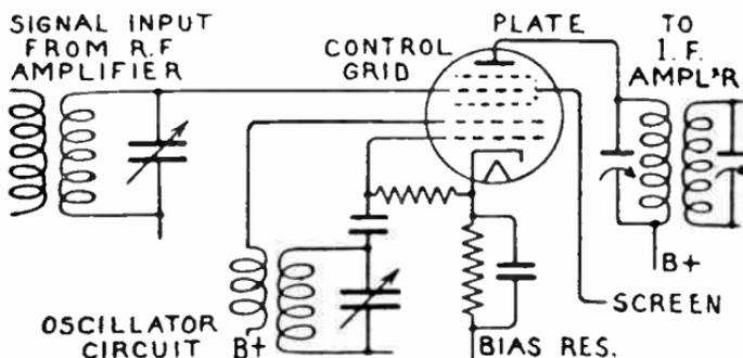
Fig. 25.—Complete Pentagrid Converter Connections.
