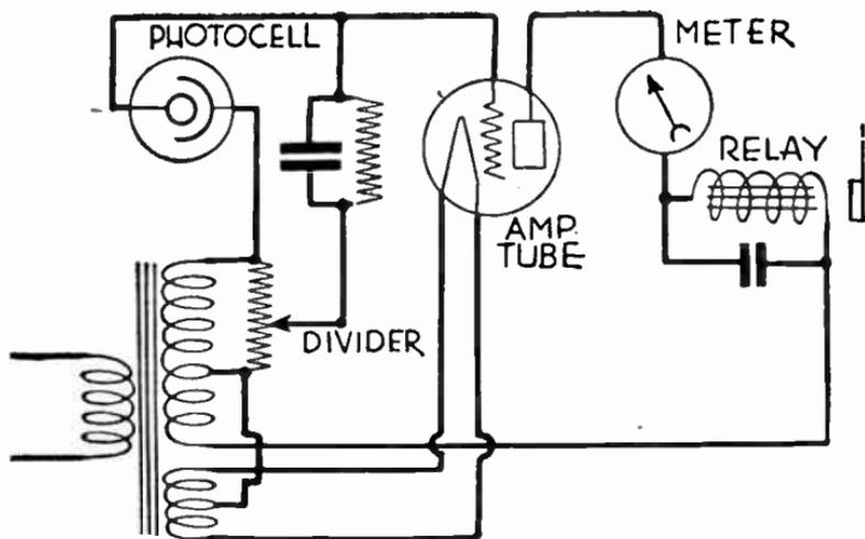
FIG. 11.—The Relay Opens upon Increase of Light.
