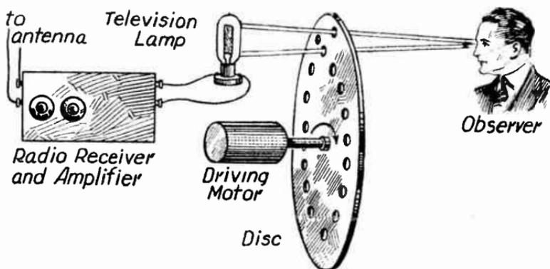
FIG. 2.—Nipkow Disc Reproduction at Television Receiver.
