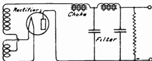
FIG. 8.—Filter with Choke Input.
