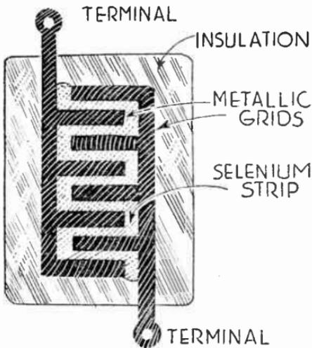
FIG. 1.—Photoconductive Element.
