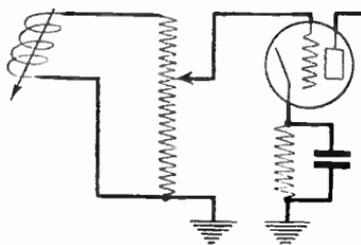
FIG. 4.—Voltage Divider for Vacuum Tube Input.
