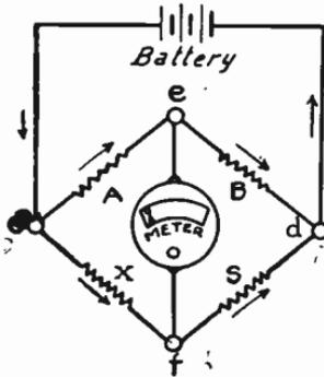
FIG. 1.—Principle of the Wheatstone Bridge.
