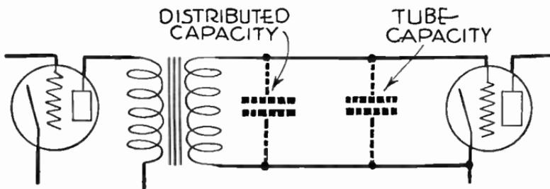
FIG. 7.—Capacities in Transformer Secondary Circuit.
