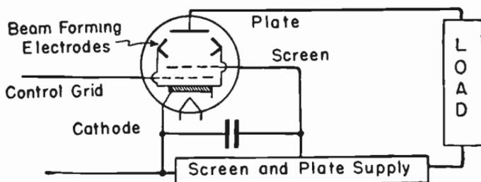
FIG. 3.—Circuit Connections to a Beam Power Tube.
