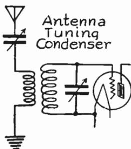
FIG. 1.—Connection of Series Condenser for Antenna Tuning
