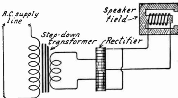
FIG. 7.—Rectifier Field Current Supply.
