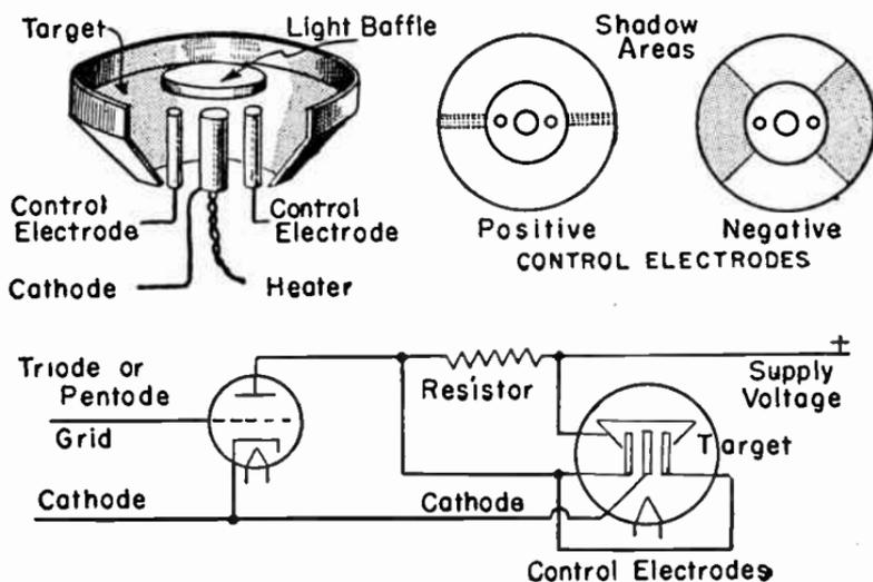
FIG. 1.—Two Ray Control Electrodes and Tube Circuit.
