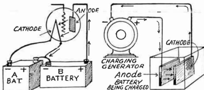
Anodes and Cathodes in Electric Circuits.
