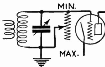
FIG. 17.—Volume Control in Grid Circuit.
