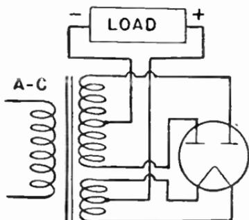
FIG. 3.—Full-wave Filament-cathode Rectifier.
