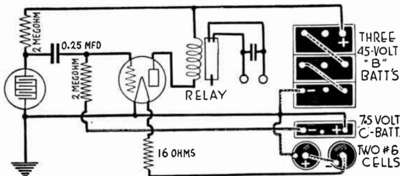
FIG. 6.—Photoconductive Cell Amplifier for Batteries.
