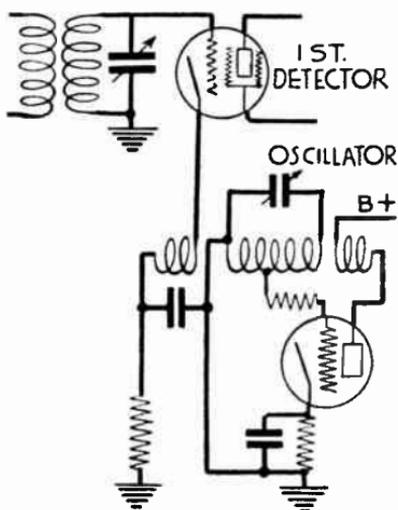
FIG. 10.—Oscillator Coupled to Detector Cathode.
