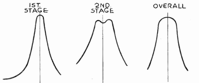
FIG. 15.—Resonance Curves for Intermediate Amplifier.
