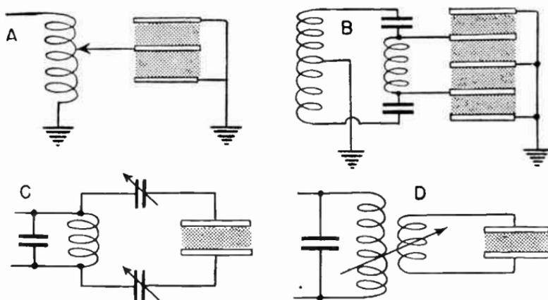
FIG. 2.—Electrode Arrangements for Electrostatic Heating.
