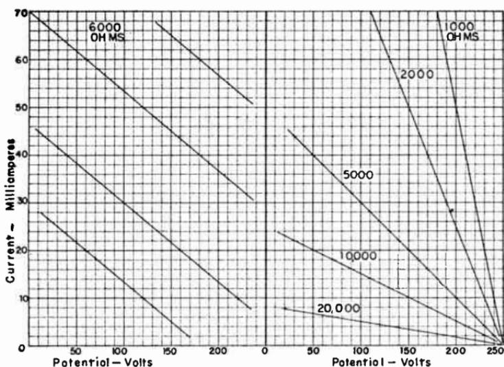
FIG. 2.—Load Lines for 6,000 Ohms Resistance.
