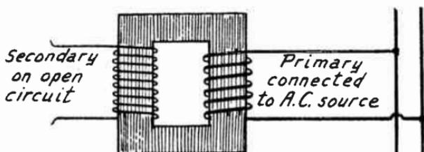
FIG. 9.—Transformer at No Load.
