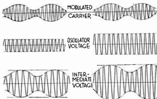
FIG. 12.—How Oscillator Voltage Increases Intermediate Voltage.
