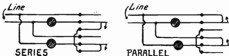
FIG. 7.—Switch for Series or Parallel Connection.
