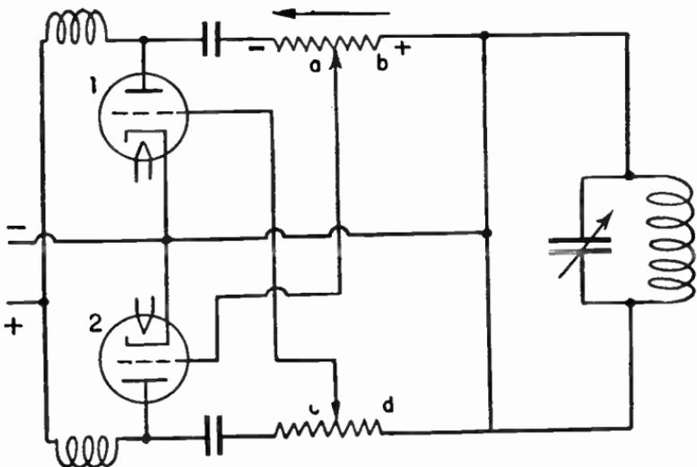
FIG. 10.—Negative Resistance Oscillator with Two Tubes.
