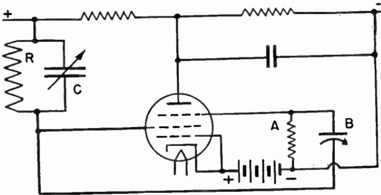
FIG. 9.—Negative Resistance Oscillator Employing Resistance-capacity Circuits.
