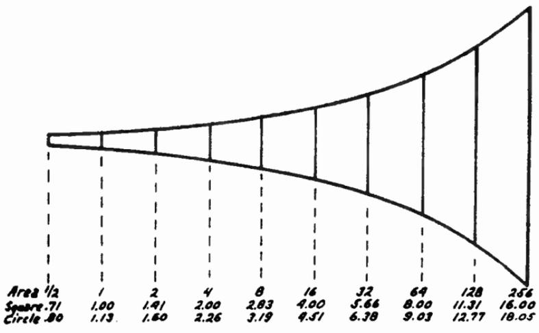
FIG. 3.—Design of Exponential Horn.
