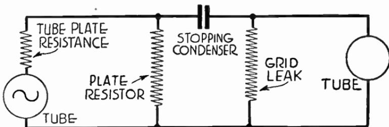
FIG. 2.—Simplified Diagram of Resistance Coupling.
