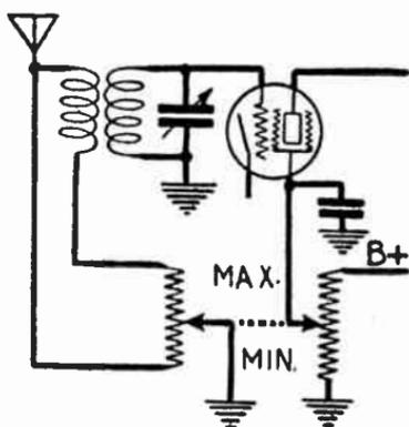
FIG. 20.—Dual Control with One Potentiometer. FIG. 21.—Twin Control for Antenna and Screen Voltage.
