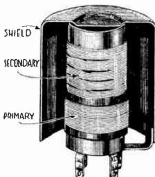
FIG. 2.—Shielded Radio Frequency Transformer.
