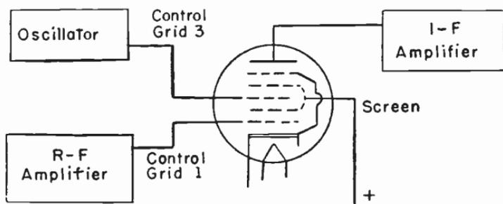
FIG. 26.—Connections for a Pentagrid Mixer.
