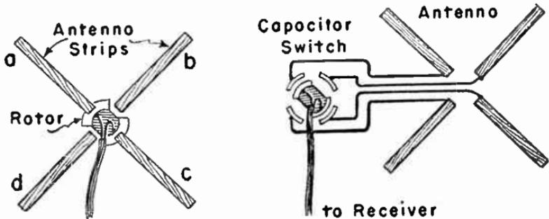
FIG. 16.—Methods for electrical rotation of built-in antennas.
