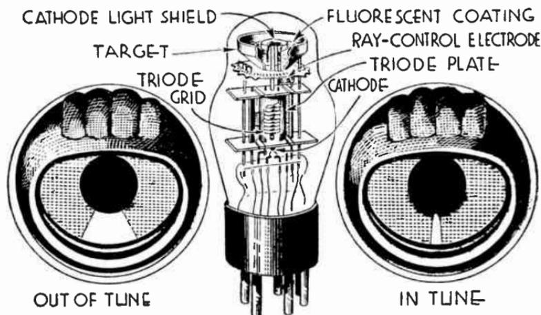
FIG. 13.—Cathode Ray Tuning Meter
