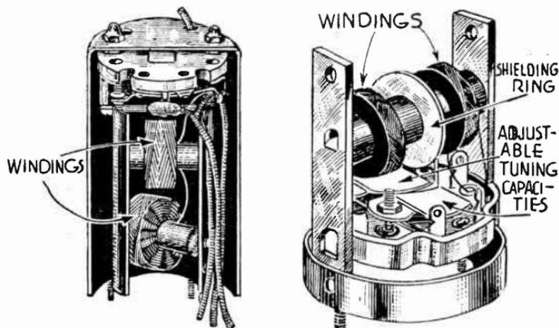
FIG. 16.—Construction of Intermediate Frequency Transformers.
