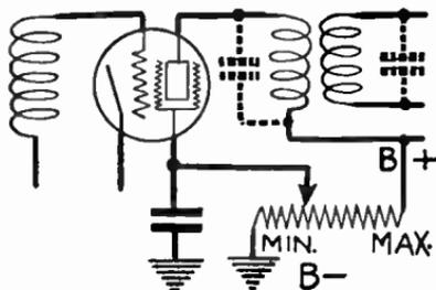
FIG. 16.—Screen Voltage Control of Volume.
