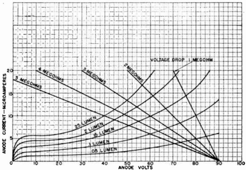
FIG. 9.—Load Lines Showing Phototube Performance.
