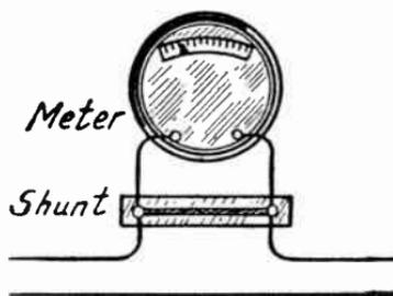
FIG. 4.—Shunt Used with Ammeter.
