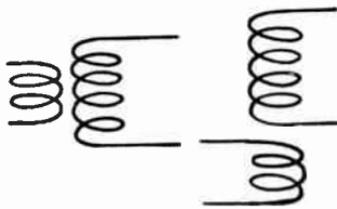
FIG. 6.—Symbols for Air Core Transformer.
