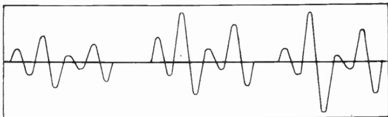
FIG. 6.—Result of Amplitude Distortion.
