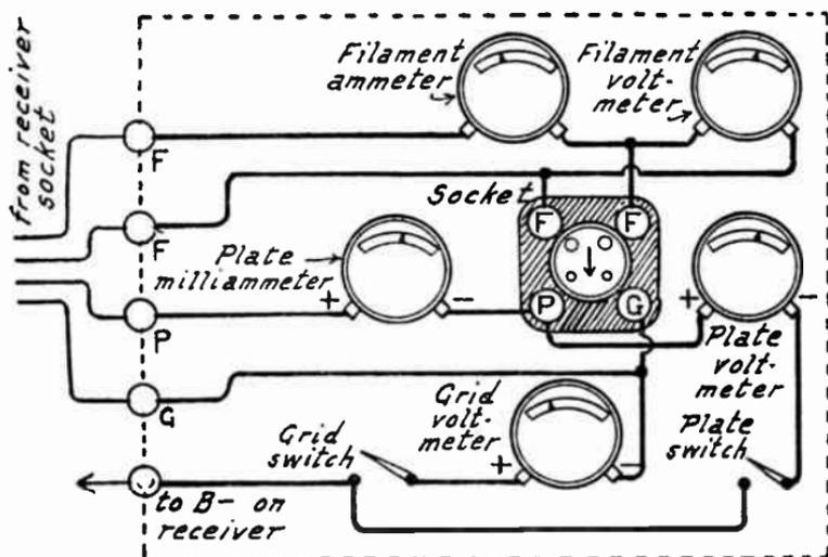
FIG. 8.—Receiver Tester with Attached Meters.
