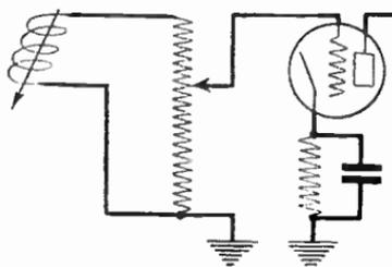
FIG. 4.—Voltage Divider for Vacuum Tube Input.
