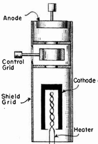
FIG. 1.—Element Arrangement in Heavy-duty Four-element Thyatron.
