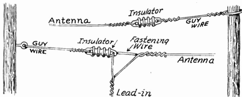
FIG. 1.—Installation of Antenna Insulators.
