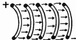
FIG. 2.—Electrostatic Field of a Coil Winding.
