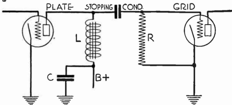
FIG. 1.—Principle of Impedance Coupling.
