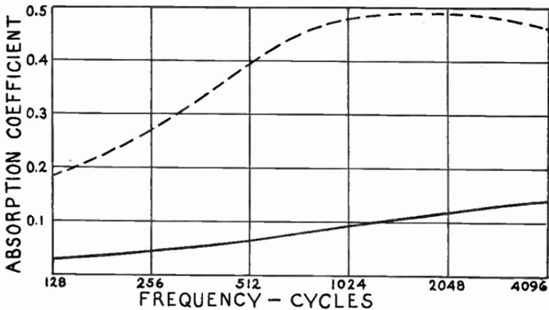
FIG. 3.—Effect of Frequency on Absorption of Sound.
