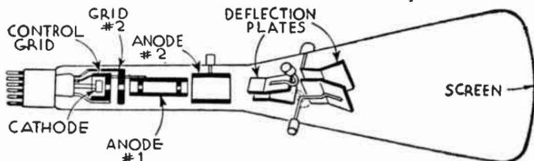
FIG. 3.—Details of Cathode-ray Tube.
