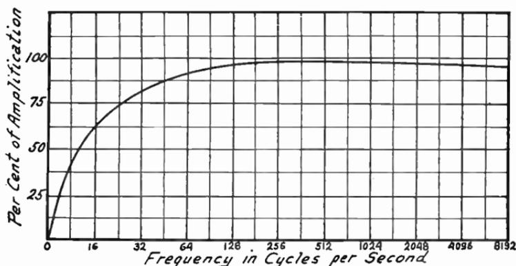
FIG. 2.—Amplification Curve for a Good Audio Transformer.
