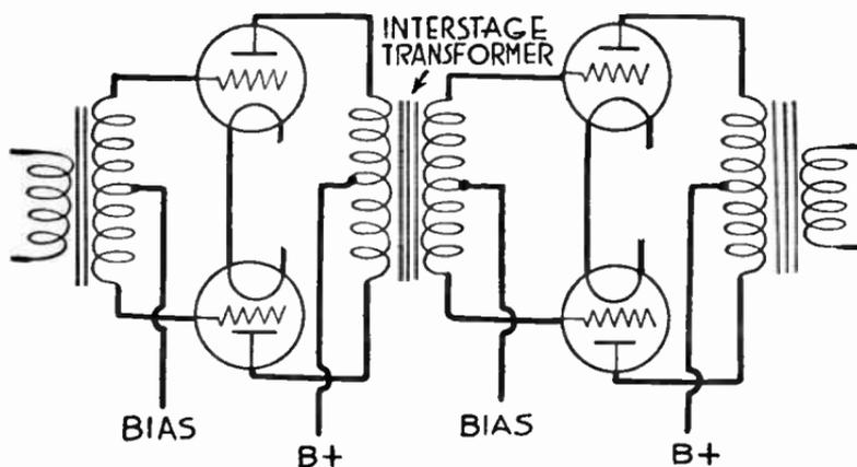
FIG. 12.—Dual Push-pull Amplification.
