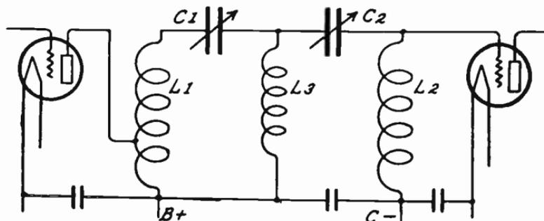
FIG. 7.—Circuit Arrangement of Vreeland Band Selector.
