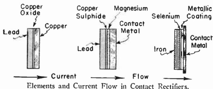
Elements and Current Flow in Contact Rectifiers.
