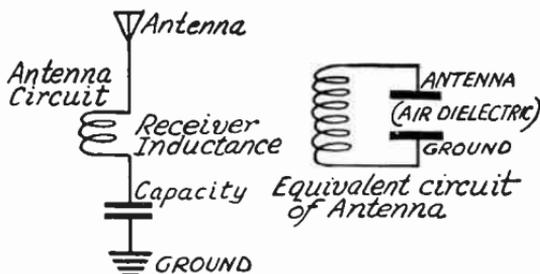
The Antenna Circuit and Its Electrical Equivalent.
