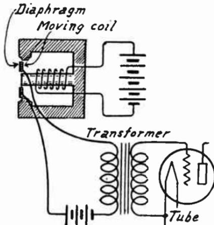
FIG. 4.—Moving Coil Microphone.
