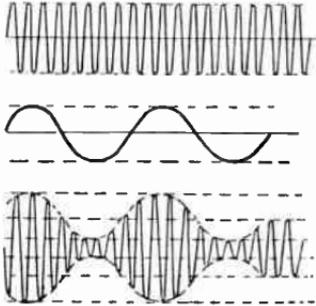
FIG. 7.—Combining the Frequencies in Modulation.
