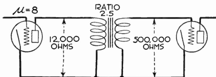
FIG. 3.—Simplified Diagram of Transformer Coupling.
