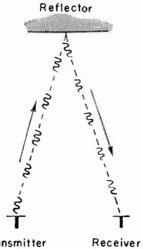
FIG. 2.—Wave Pulses between Transmitter and Receiver.
