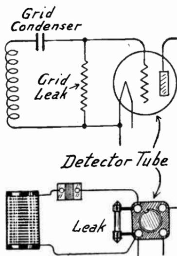
FIG. 1.—Grid Leak Connected to Detector Tube Terminals.
