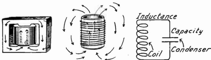
Magnetic Circuits in Iron Core
