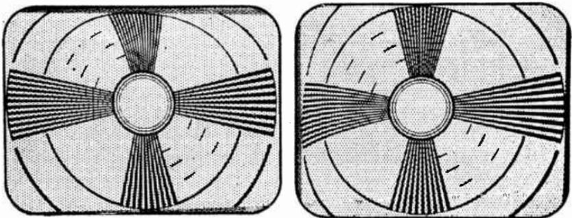
FIG. 34.—Effects of Wrong Adjustment of Linearity Controls.
