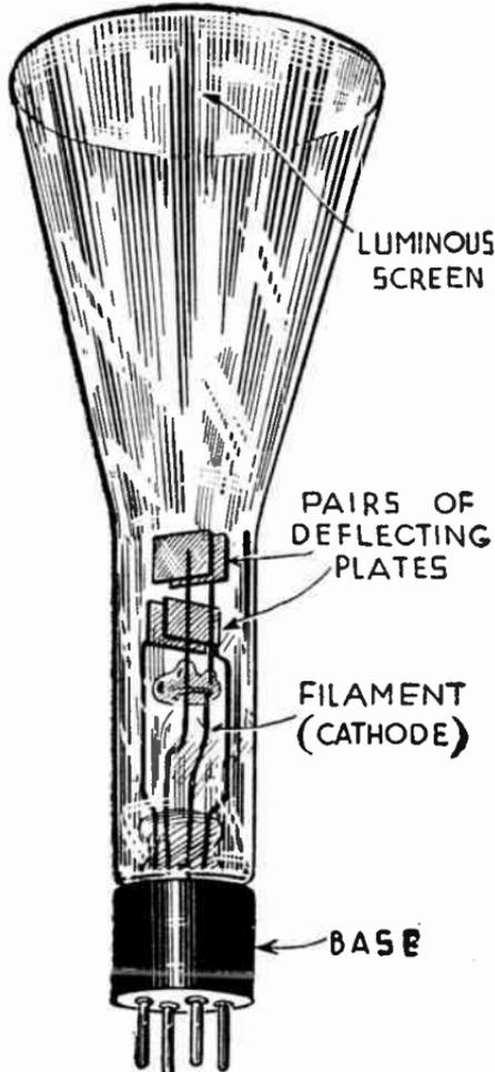
FIG. 1.—A Cathode-ray Tube.
