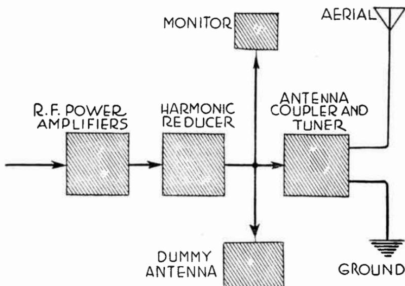
FIG. 3.—High Power Equipment Used at Transmitter.
