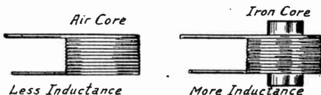
FIG. 2.—Iron Core for Increase of Self-Inductance.
