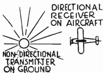
FIG. 1.—Ground Transmitter and Airplane Receiver.
