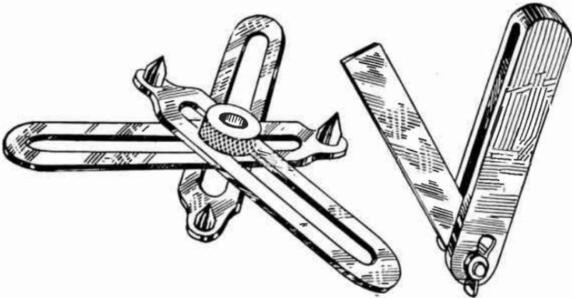
FIG. 1.—Adjustable Template and Adjustable Square.
