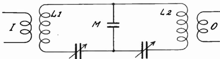
FIG. 10.—Mutual Coupling with Condenser.
