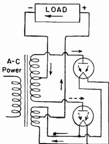
FIG. 1.—Two Filament-cathode Tubes in Full-wave Rectifier.
