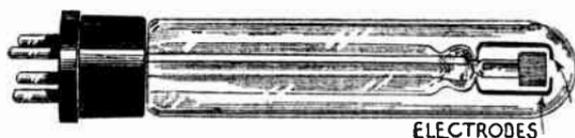
FIG. 9.—Glow Lamp for Sound Recording on Film.
