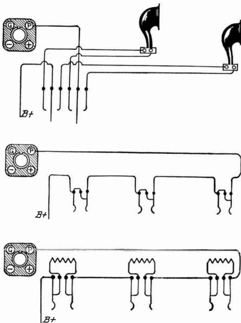
FIG. 6. - Jacks for Connection of Several Speakers.
