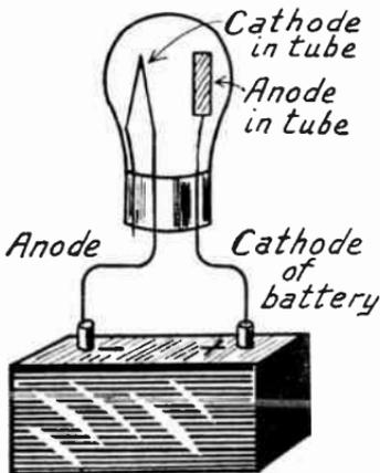
Electrodes of Tube and Battery.
