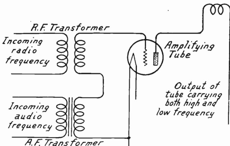
FIG. 1.—Effect of Reflexing on Amplifying Tube.
