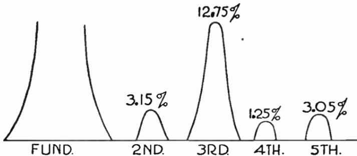
FIG. 6.—Harmonics with Push-pull Amplification.
