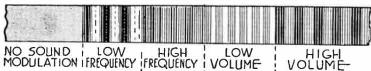
FIG. 6.—Changes in Variable Density Sound Track.
