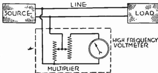
FIG. 1.—Simple Form of Volume Indicator.
