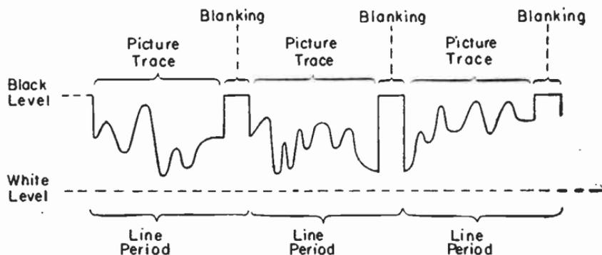
FIG. 6.—Horizontal Blanking Intervals Between Picture Signals.
