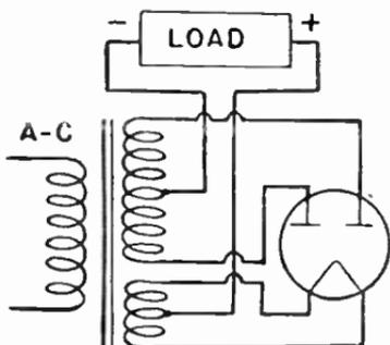
FIG. 3.—Full-wave Filament-cathode Rectifier.
