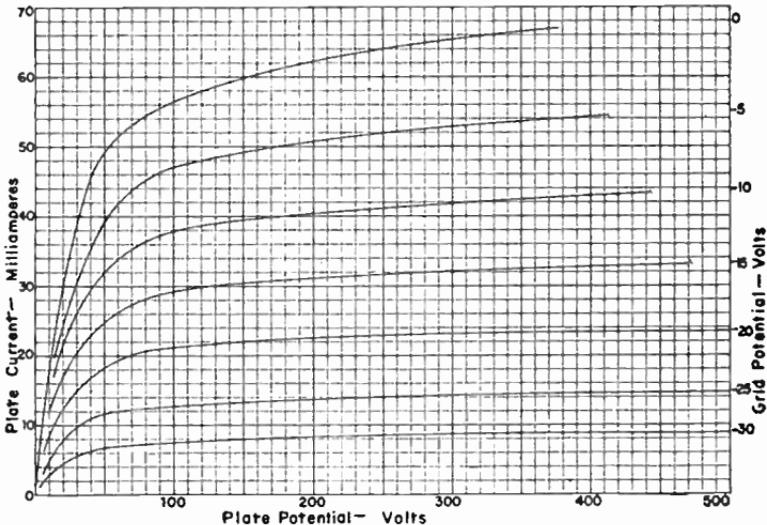
FIG. 1.—Plate Characteristics of a Power Pentode.
