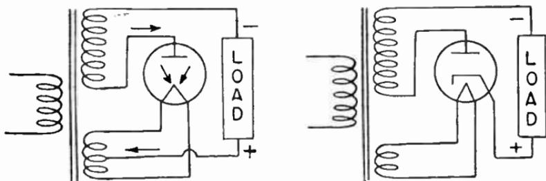
FIG. 1.—Tubes Used as Half-wave Rectifiers.
