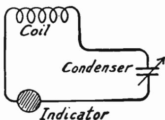
FIG. 1.—The Simplest Frequency Meter Circuit.
