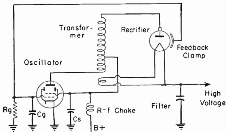
FIG. 38.—High-voltage Supply Using an R-f Oscillator.
