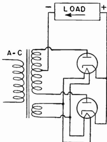
FIG. 2.—Two Heater-cathode Tubes in Full-wave Rectifier.
