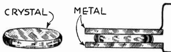
FIG. 1.—The Quartz Plate.
