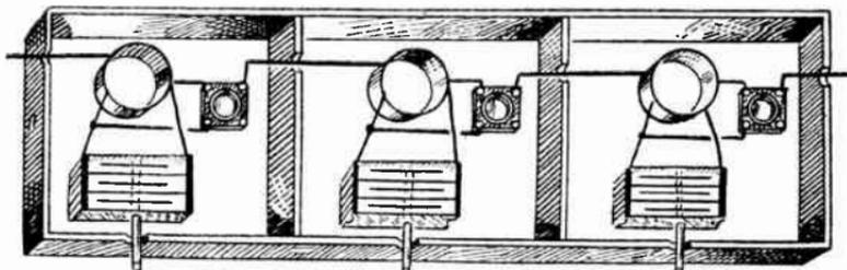
FIG. 5.—Amplifying Stages Enclosed in Individual Shields.
