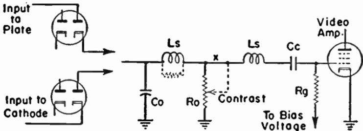
Fig. 19.—Typical Connections for Video Detectors.
