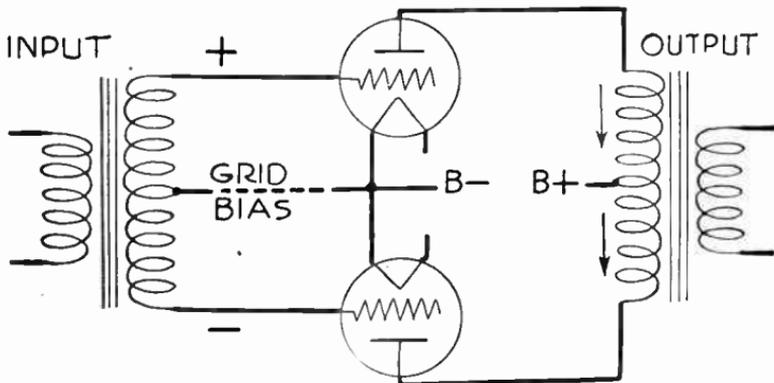
FIG. 1.—Elementary Push-pull Circuit.
