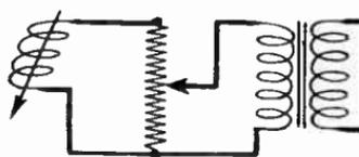
FIG. 3.—Voltage Divider or Potentiometer Control.
