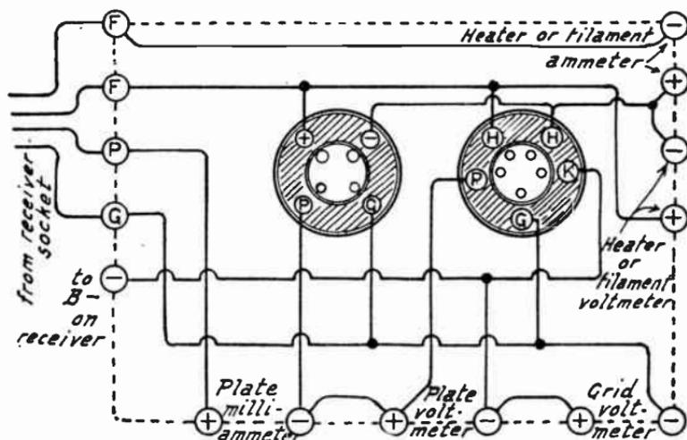
FIG. 9.—Test Board with Sockets.
