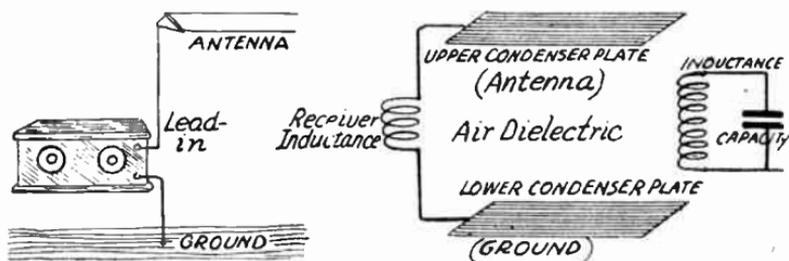
FIG. 2.—The Principle of the Capacity Antenna.
