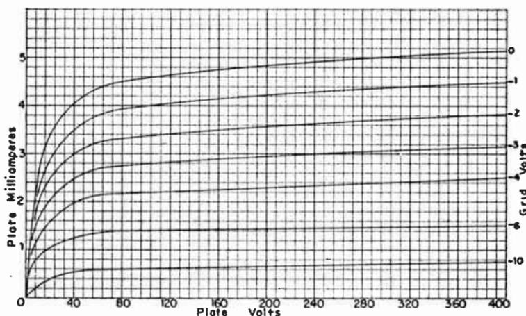
FIG. 4.—Plate Characteristics of a Voltage-amplifier Pentode.
