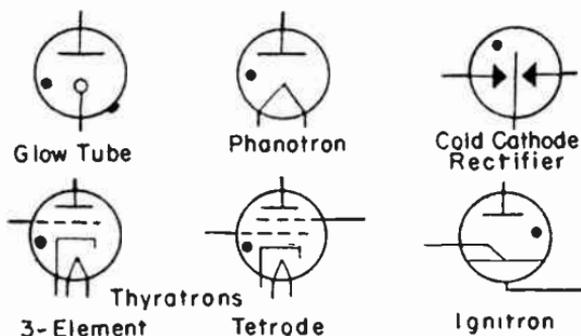
FIG. 1.—Symbols for Gas-filled Tubes.
