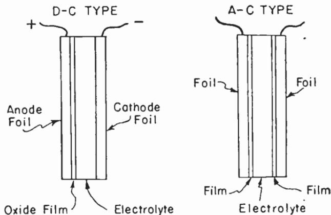
Elements Used in Electrolytic Condensers.
