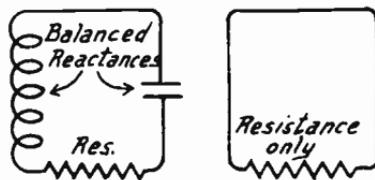
FIG. 2.—Condition of Series Resonance.
