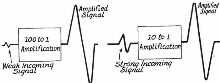
The Effect of Amplification on Signal Strength.
