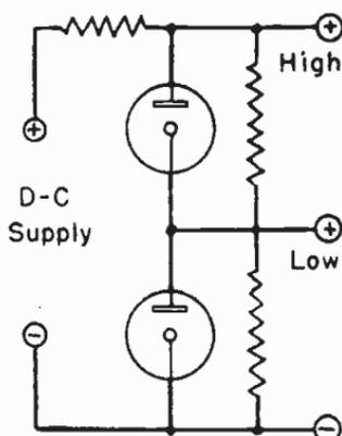
FIG. 4.—Two Tubes Regulating Two Voltages.
