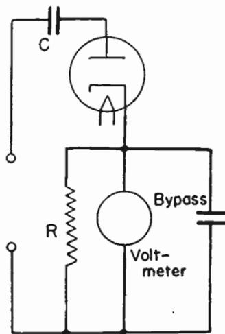
FIG. 6.—Diode Used for a VT Voltmeter.
