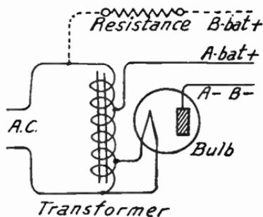
FIG. 3.—Two Voltages with Auto-transformer.
