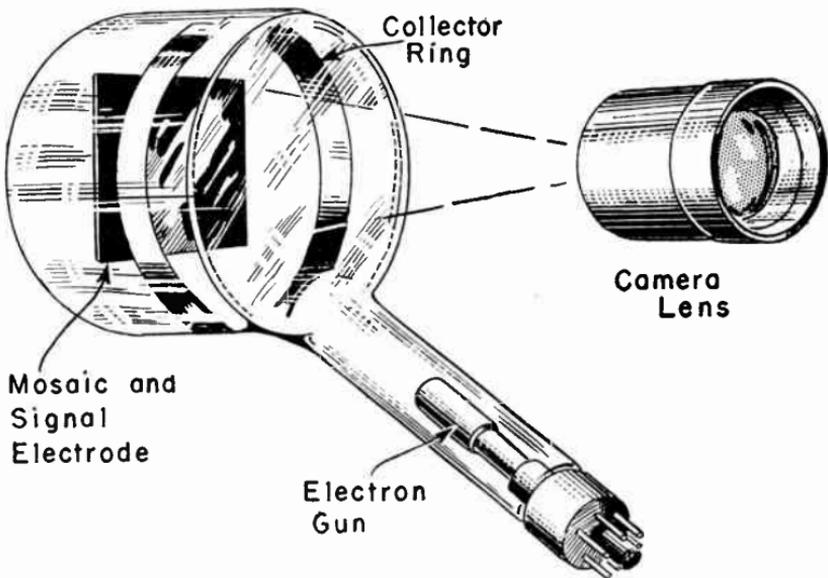
FIG. 1.—An Iconoscope Used in a Television Camera.
