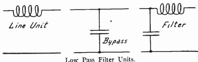
In order to turn the undesired high frequencies back to the source a condenser may be used as a bypass as shown in the center. The capacity of a condenser may be selected of such value that it offers little reactance or opposition to frequencies above a certain value, yet greatly impedes the flow of lower frequencies through it. Such a condenser is used for low pass filters.
