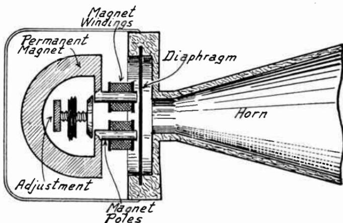
FIG. 1.—Electromagnetic Type of Loud Speaker.
