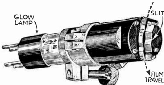
FIG. 10.—Glow Lamp Holder with Slit.
