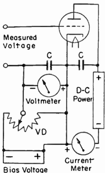
FIG. 3.—Slide Back Instrument Using Two Meters.
