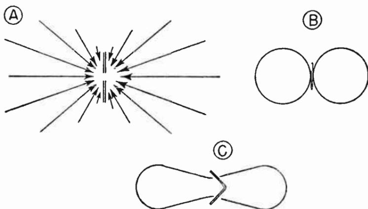
FIG. 6.—Directional patterns of a straight dipole and of an inclined V-dipole.
