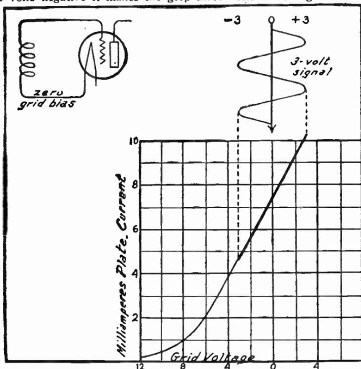
FIG. 1.—Effect of Zero Grid Bias, Distortion.
