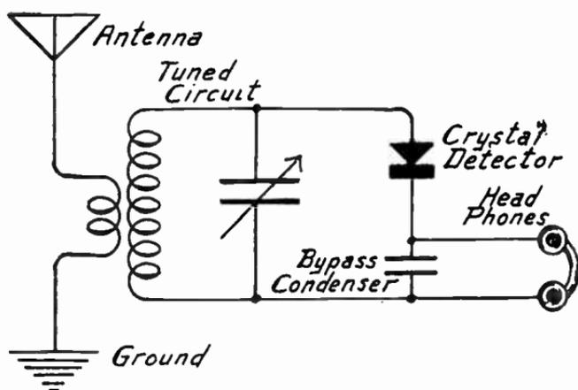
Receiver Circuit with Crystal Detector.
