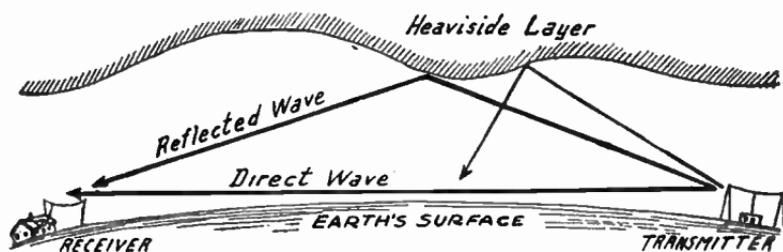
FIG. 1.—Effect of Heaviside Layer on Fading
