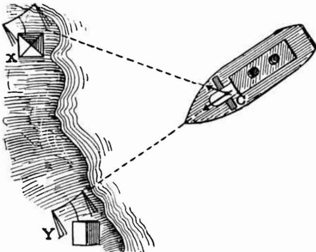
FIG. 2.—Determining Ship's Position with Radio Compass.
