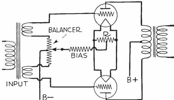
FIG. 8.—Equalizing Plate Currents in Push-pull Tubes.
