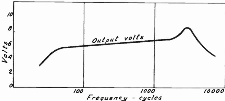
FIG. 5.—Result of Frequency Distortion in Amplifier.
