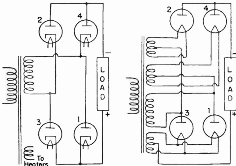
FIG. 7.—Four Tubes in Full-wave Bridge Circuit.
