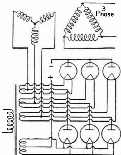
FIG. 2.—Polyphase Full-wave Rectifier.
