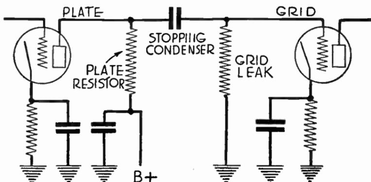
FIG. 1.—Resistance-capacity Coupled Amplifier.
