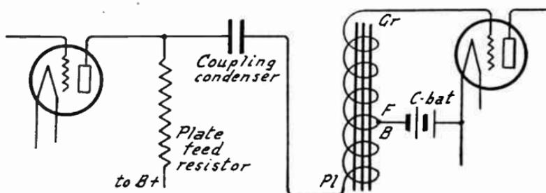
FIG. 11.—Parallel Feed with Resistor and Transformer.
