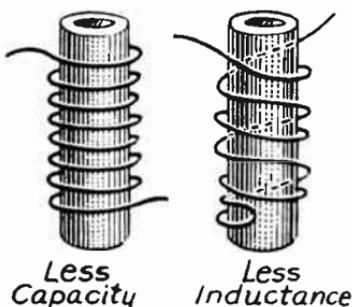
FIG. 1.—Space Winding and Non-inductive Winding of Resistors.
