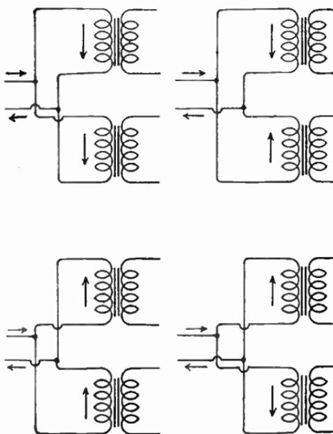
FIG. 11.—Connections of Transformers to Supply Line.
