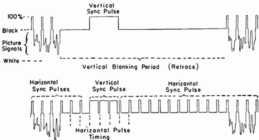
FIG. 8.—Vertical Sync Pulse During Vertical Blanking Period.
