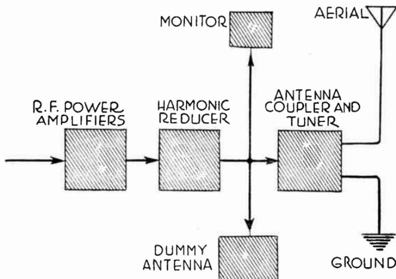
FIG. 3.—High Power Equipment Used at Transmitter.
