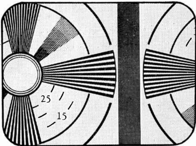
FIG. 36.—Effect of Wrong Adjustment of Phase Control.
