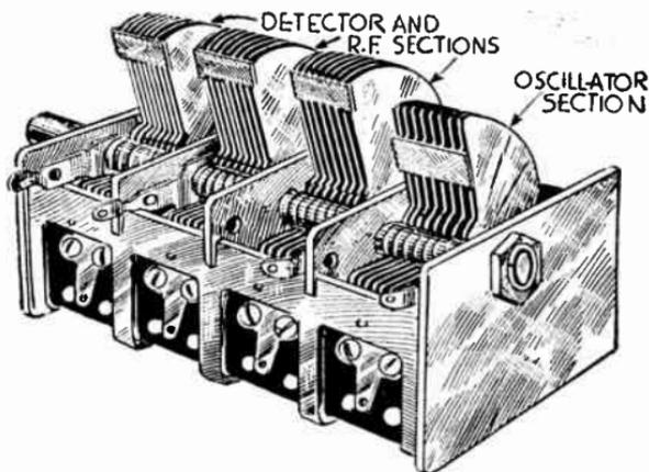
FIG. 20.—Oscillator Tuning Condenser with Special Plates.
