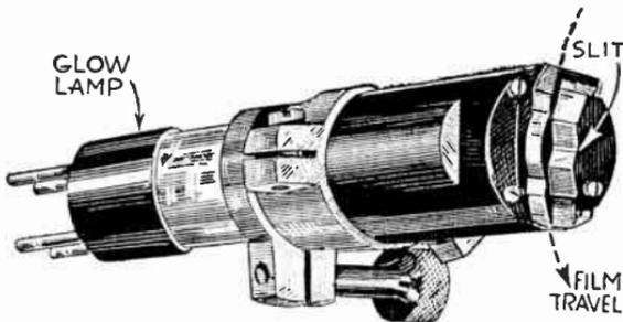
FIG. 10.—Glow Lamp Holder with Slit.
