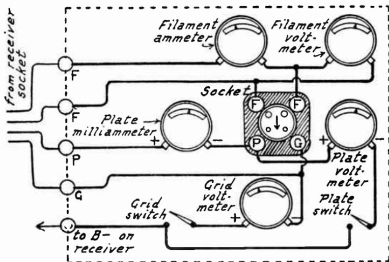
FIG. 8.—Receiver Tester with Attached Meters.
