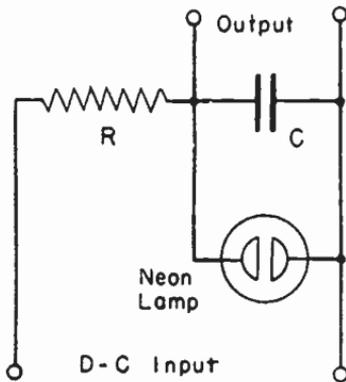
FIG. 4.—Neon Lamp in Relaxation Oscillator.
