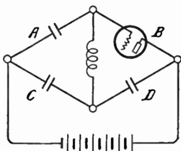
FIG. 8.—The Isofarad Balanced Circuit in Bridge Form.
