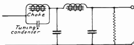
FIG. 10.—Principle of Tuned Filter.
