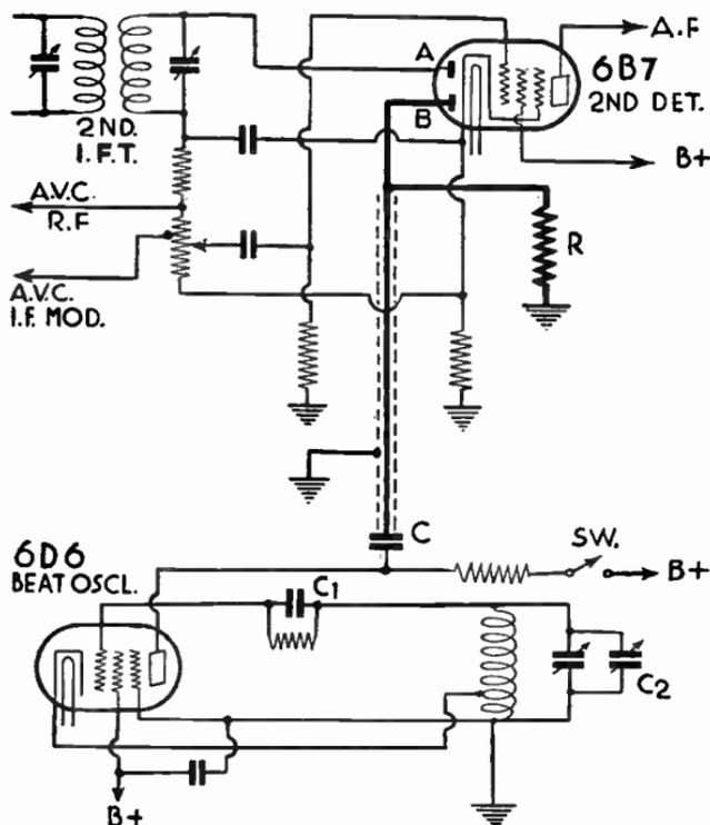
FIG. 10.—Beat Frequency Oscillator Circuit
