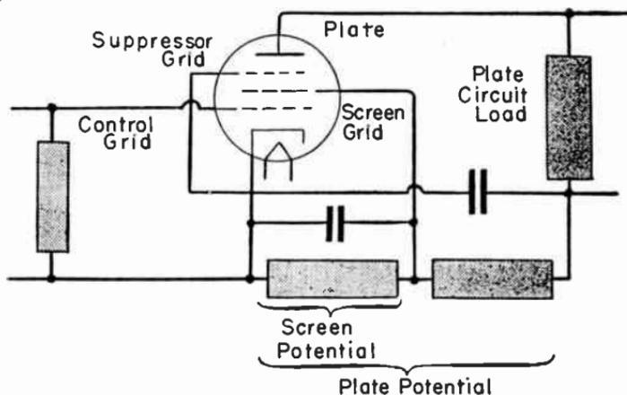
FIG. 2.—Typical Connections for Pentode Voltage Amplification.
