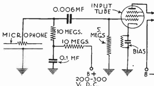
FIG. 2b.—Circuit Connection of Static Velocity Microphone.
