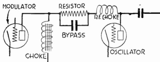
FIG. 12.—Connection of Voltage Dropping Resistor.
