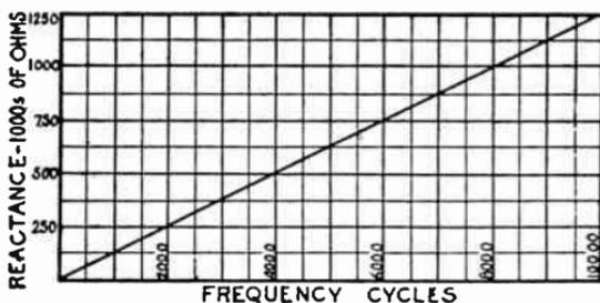
FIG. 5.—Frequency Effect on Inductive Reactance.
