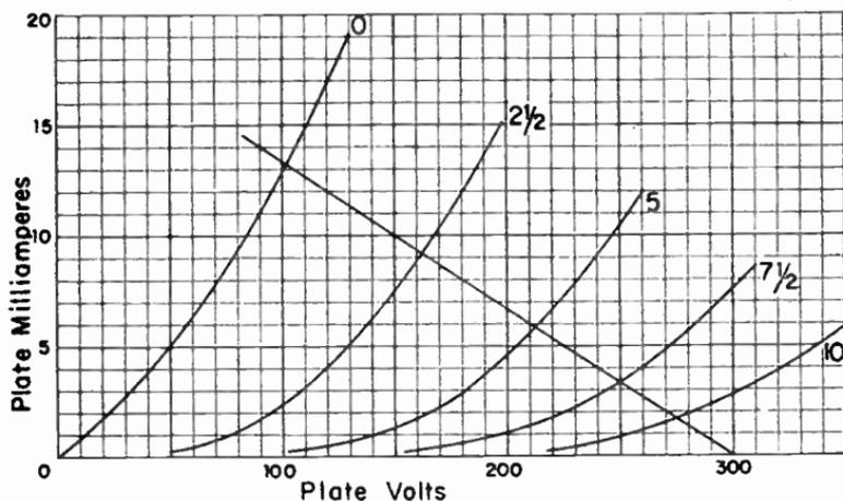
Load Line Used for Computing Voltage Amplification.
