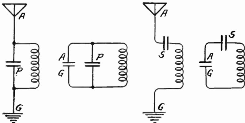
FIG. 2.—Connection of Parallel or Shunting Antenna Condenser.
