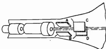
FIG. 3.—Electrostatic Deflection of the Beam.
