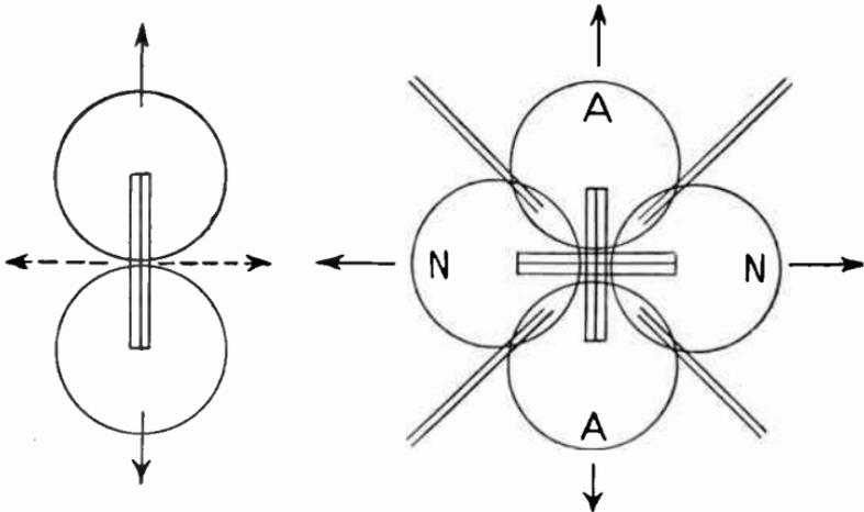
FIG. 4.—Radiation from Loop Antennas.
