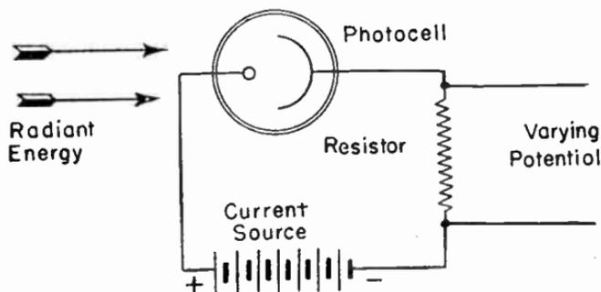
FIG. 3.—The Basic Phototube Circuit.
