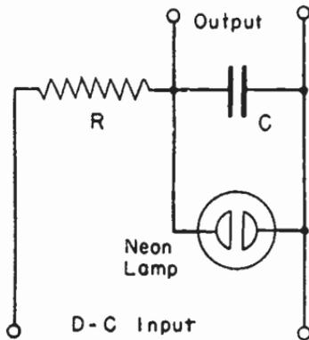
FIG. 4.—Neon Lamp in Relaxation Oscillator.
