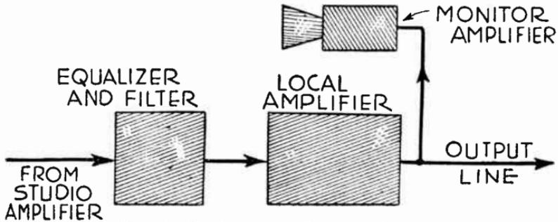
FIG. 4.—Equipment at Repeater Station.
