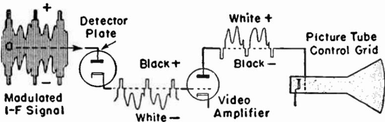
Fig. 20.—Signal Polarities with a Single Video Amplifier.
