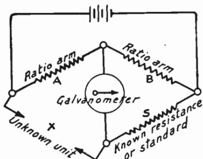
FIG. 3.—Functions of the Arms in a Bridge.
