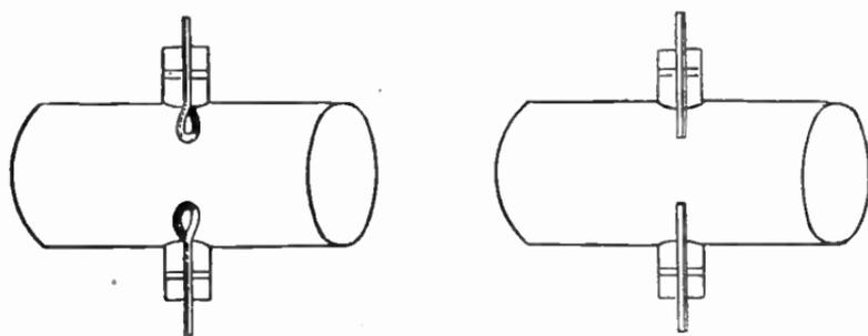
FIG. 2.—Energy Transfer Probes for Cavity Resonator.
