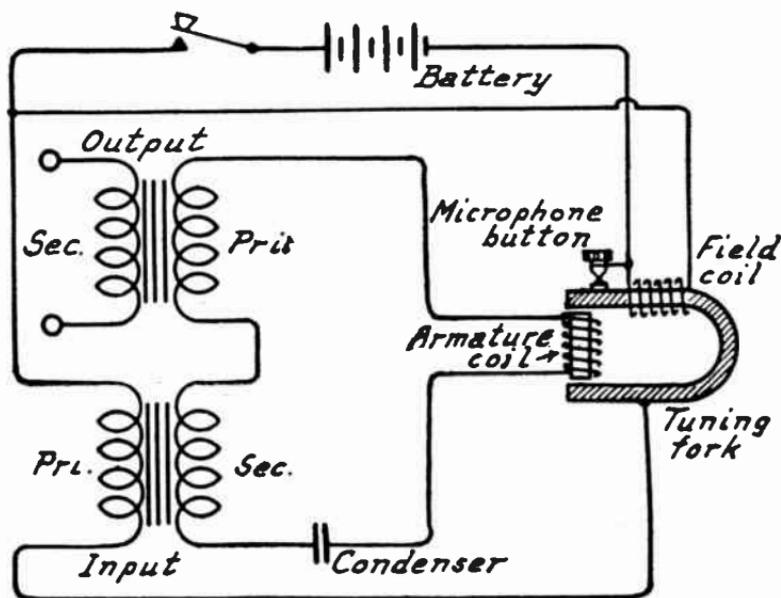
FIG. 2.—Tuning Fork Audio Oscillator.
