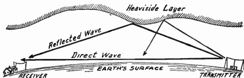
FIG. 1.—Effect of Heaviside Layer on Fading
