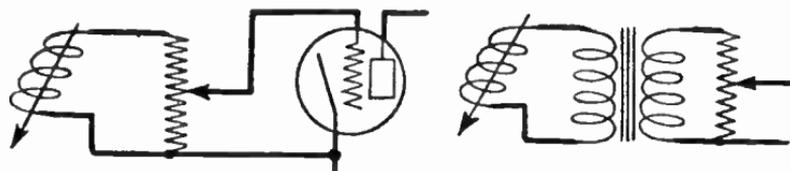
FIG. 11.—Volume Controls for Phonograph Pickups.
