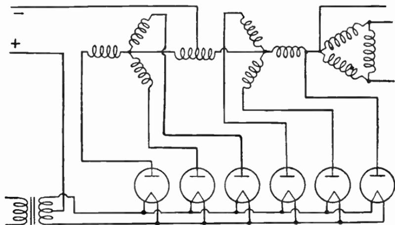
FIG. 3.—Three-phase Double-Y Parallel Rectifier.
