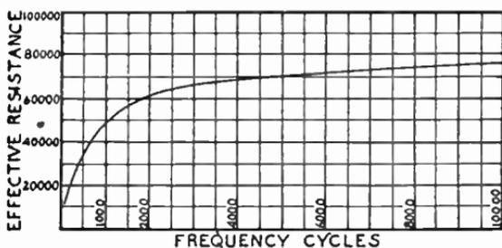
FIG. 6.—Frequency Effect on Apparent Resistance.
