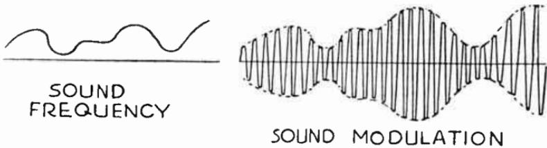
FIG. 2.—Modulation with Sound Frequency.
