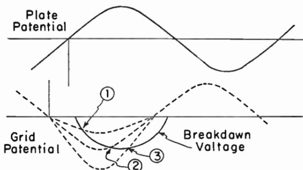
FIG. 5.—Breakdown Control by Variation of Grid Potential Amplitude, with Phase Shift of Grid Potential.
