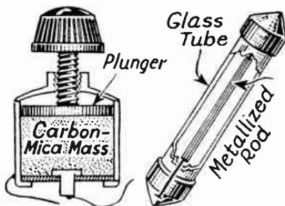
FIG. 2.—Carbon Type and Metallized Type of Resistors.
