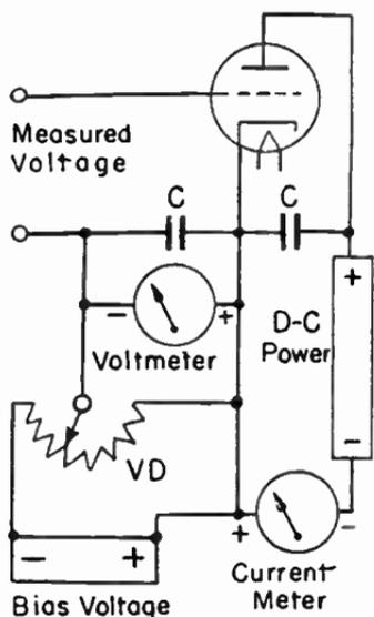
FIG. 3.—Slide Back Instrument Using Two Meters.
