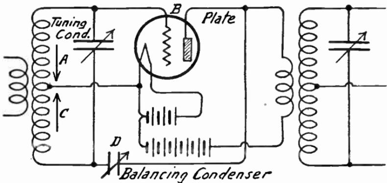
FIG. 4.—Rice Method of Balancing.
