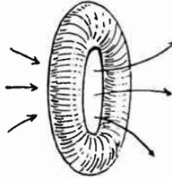
FIG. 2.—Magnetic Field of Toroid
