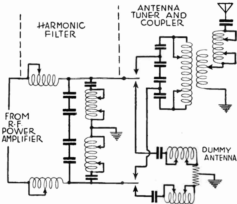
FIG. 10.—Antenna System and Harmonic Filter.
