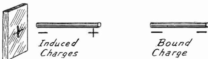
Charges Produced by Electrostatic Induction.
