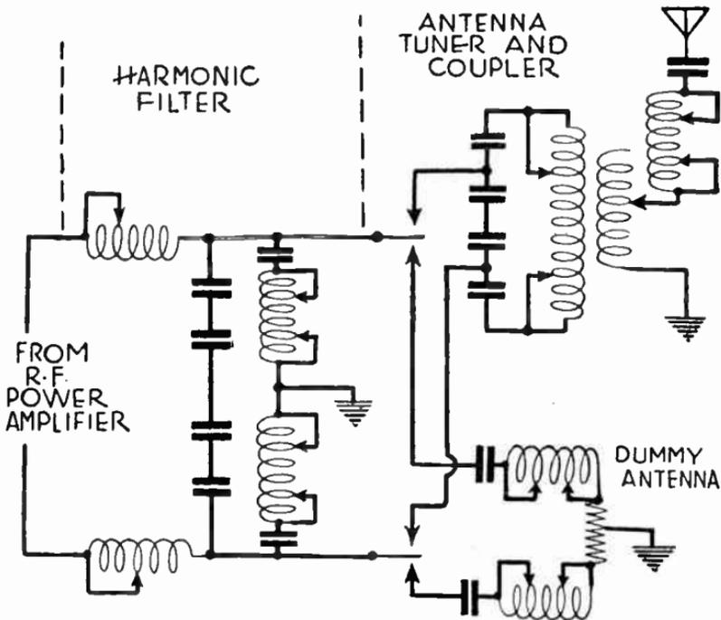
FIG. 10.—Antenna System and Harmonic Filter.
