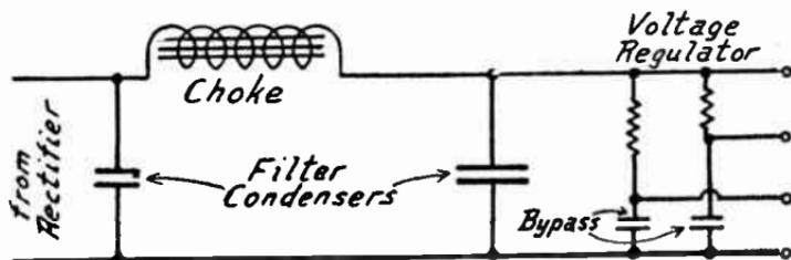
FIG. 6.—Power Unit Filter System with Single Choke.
