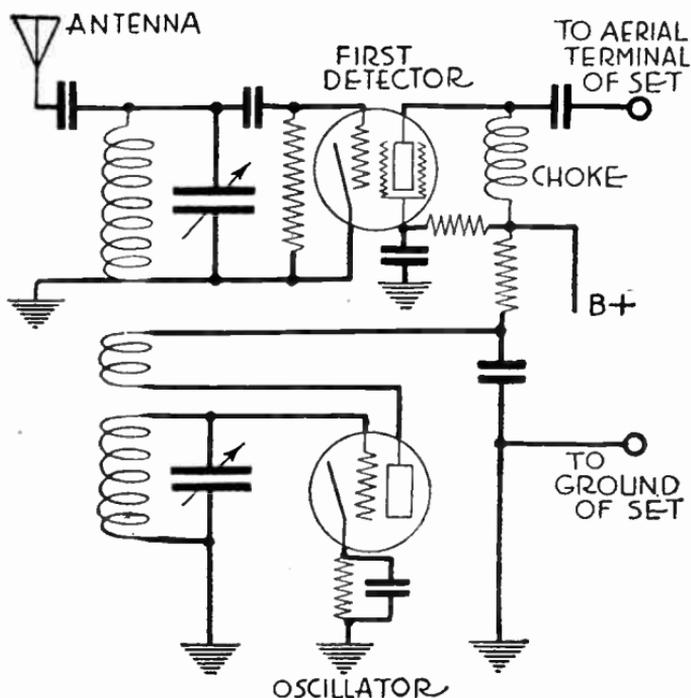
FIG. 6.—Superheterodyne Converter for Short Wave Reception
