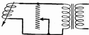
FIG. 2.—Rheostat for Volume Control.
