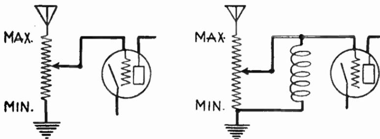
FIG. 14.—Volume Controls for Untuned Antenna Circuits.
