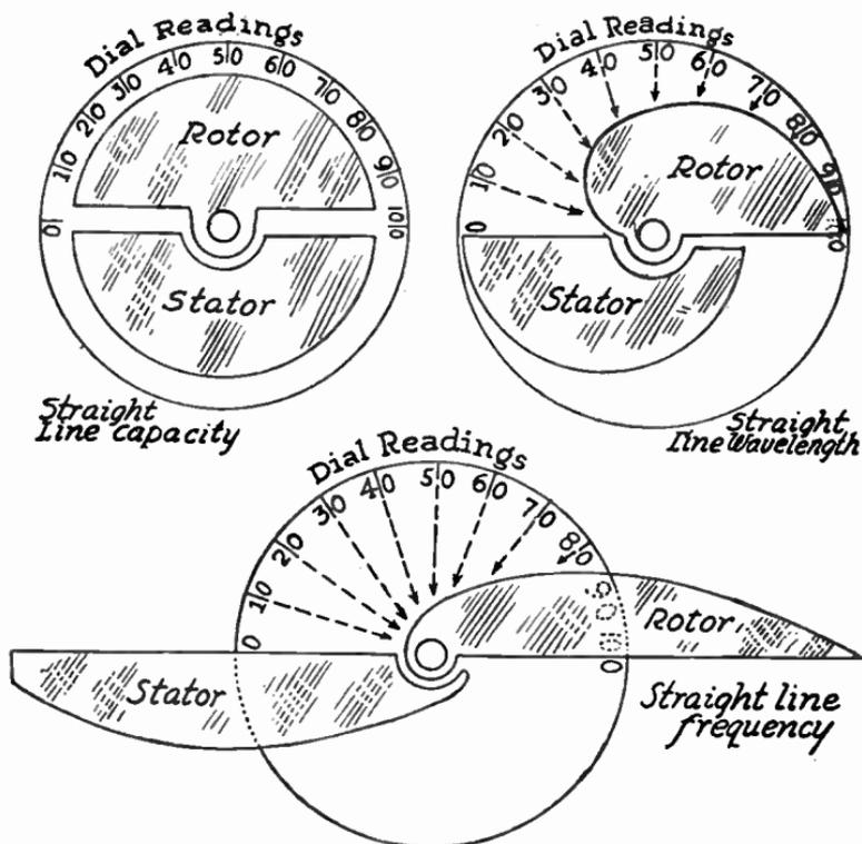
FIG. 5.—Basic Forms of Condenser Rotor Plates.
