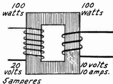
FIG. 8.—A Step-Down Transformer.
