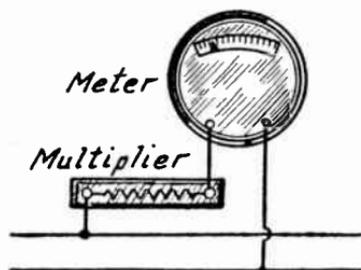
FIG. 3.—Multiplier Used with Voltmeter.
