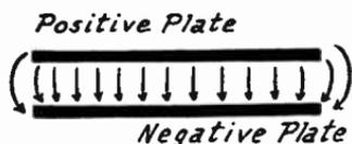
FIG. 1.—Electrostatic Field between Condenser Plates.
