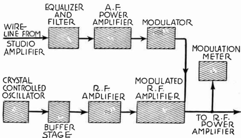
FIG. 2.—Low Power Equipment for Amplifying.
