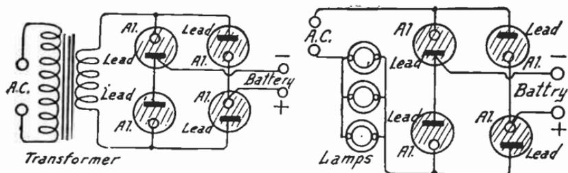
FIG. 8.—Electrolytic Rectifiers in Full-wave Bridge Circuit.
