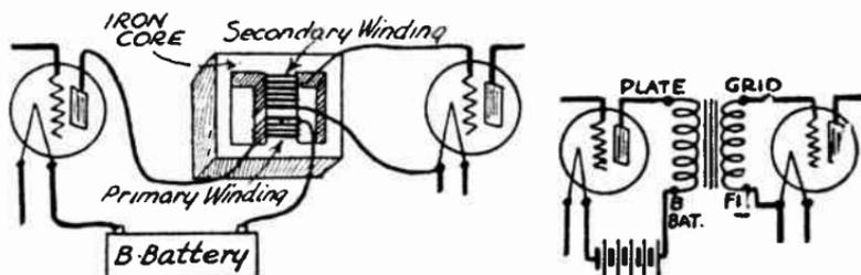
FIG. 1.—Transformer Coupling for Audio Frequency Amplifier.
