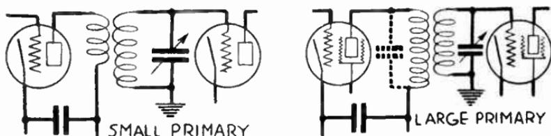
FIG. 3.—Primaries of High and Low Frequency.
