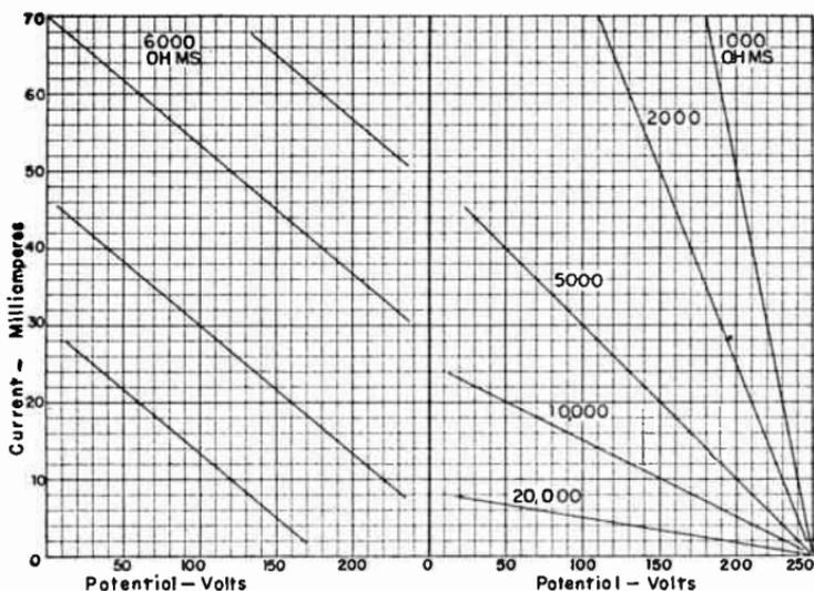
FIG. 2.—Load Lines for 6,000 Ohms Resistance.
