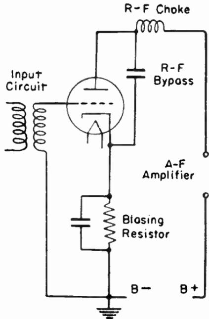
FIG. 3.—Typical Circuit for a Plate Current Detector.
