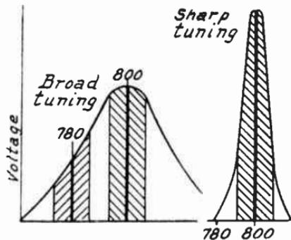
FIG. 2.—Response of Resonant Circuits.
