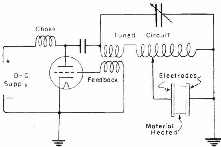
FIG. 1.—Simplified Circuit for Electrostatic Heating.
