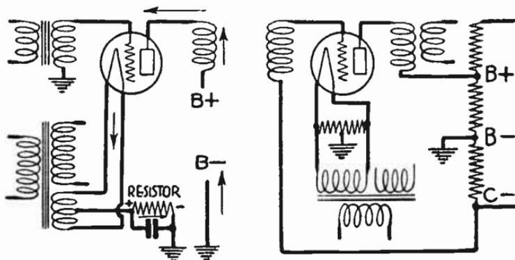
FIG. 7.—Biasing for Filament Tubes.
