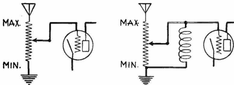
FIG. 14.—Volume Controls for Untuned Antenna Circuits.
