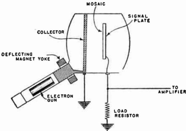
FIG. 4.—Circuit for Signal Current in the Iconoscope.
