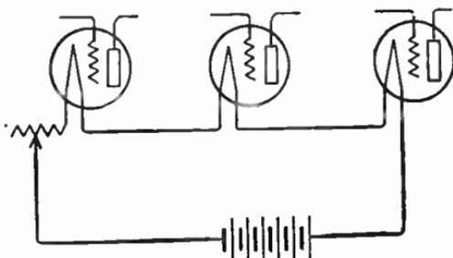
FIG. 1.—A Series Circuit.
