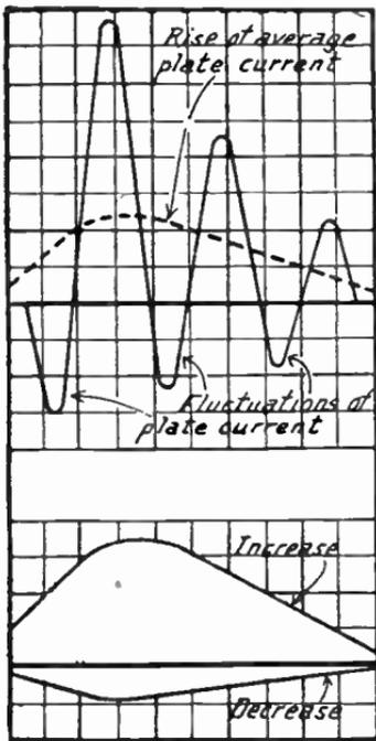
FIG. 2.—Current Change During Plate Current Detection.
