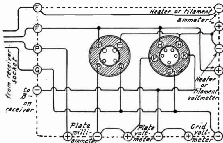
FIG. 9.—Test Board with Sockets.
