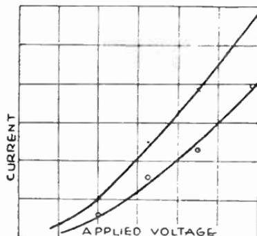
Fig. 4.—Current-voltage Curve of Selenium Cell.
