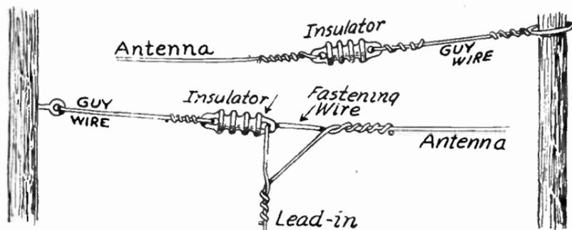
FIG. 1.—Installation of Antenna Insulators.
