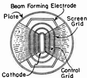
FIG. 1.—Element Arrangement in Beam Power Tube.
