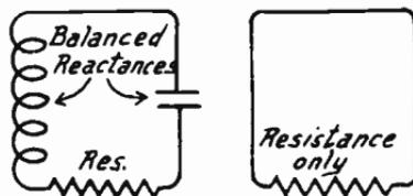
FIG. 2.—Condition of Series Resonance.
