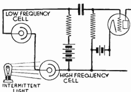
FIG. 15.—Phototube Amplification of Carrier Frequency.
