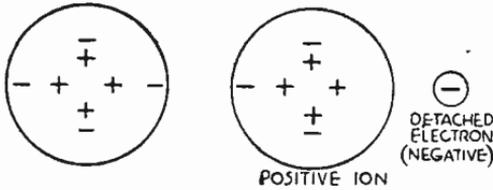
FIG. 1.—Neutral Atom and Positive Ion.
