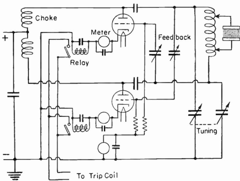
FIG. 3.—Typical Circuit for Electrostatic Heating.
