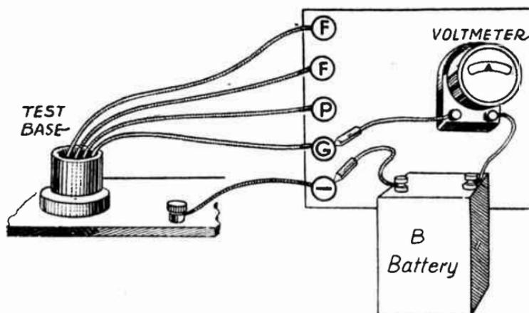
FIG. 10.—Circuit Tests on Receiver.
