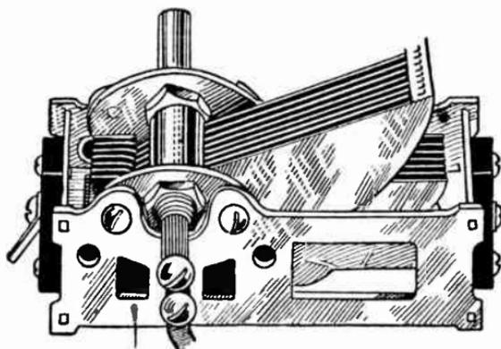
FIG. 6.—Modified Straight Line Frequency Condenser.
