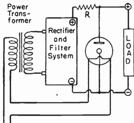
FIG. 3.—Connections Used with Single Regulator Tube.
