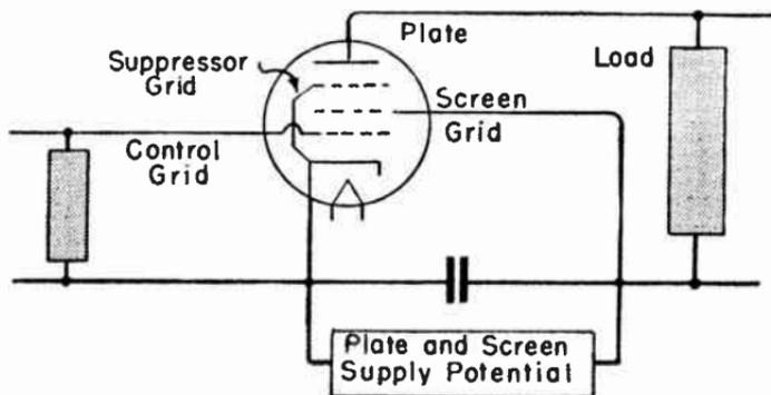
FIG. 3.—Typical Connections for Pentode Power Amplifier.
