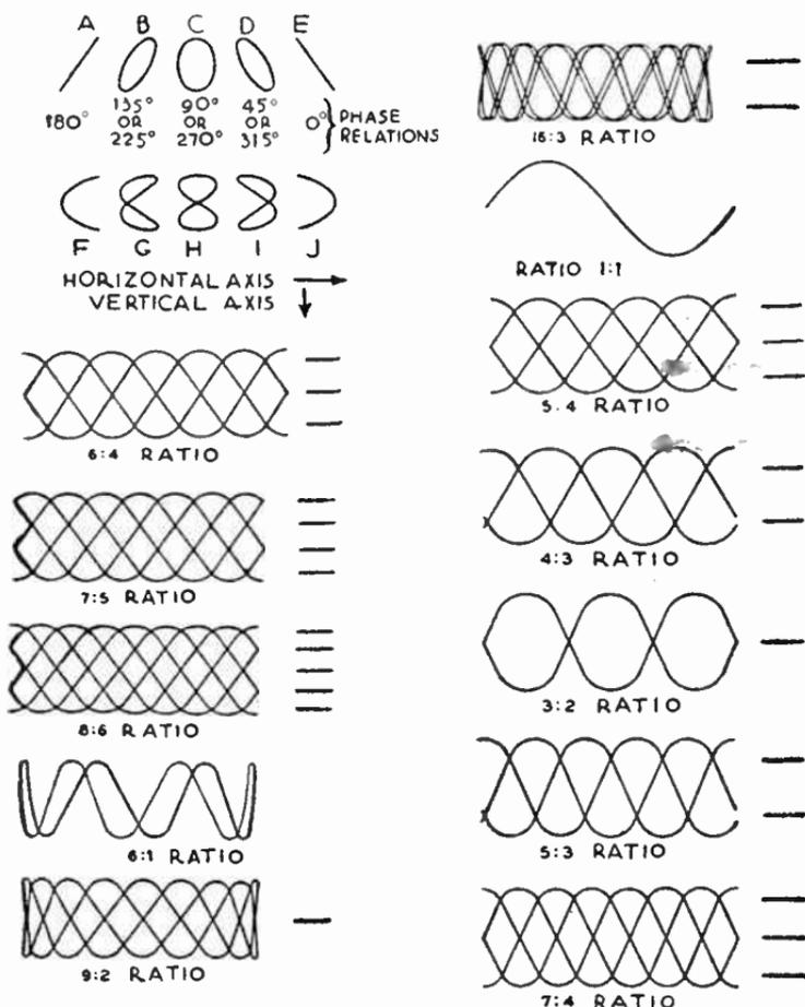
FIG. 13.—Lissajous Figures Caused by a Frequency Difference between Voltages Applied to Vertical and Horizontal Deflecting Plates of Cathode Ray Oscilloscope.
