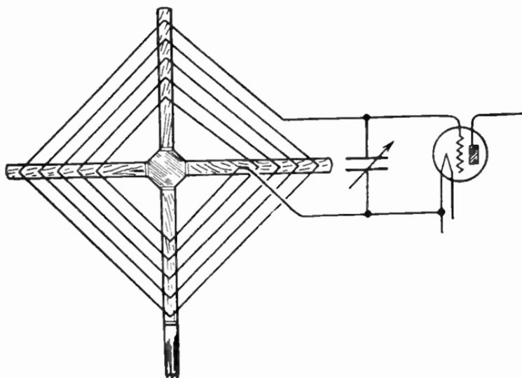
Connections from Spiral Loop to Receiver.
