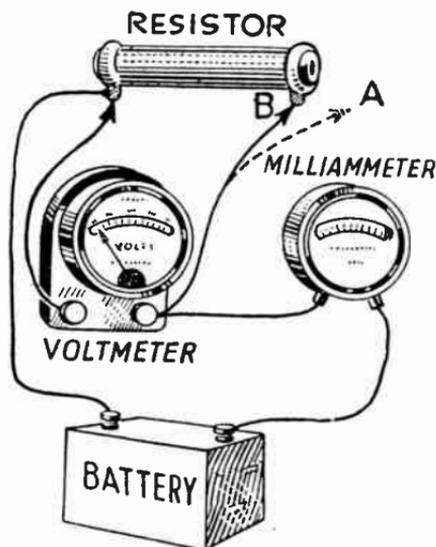
FIG. 18.—Measuring the Resistance of a Resistor.
