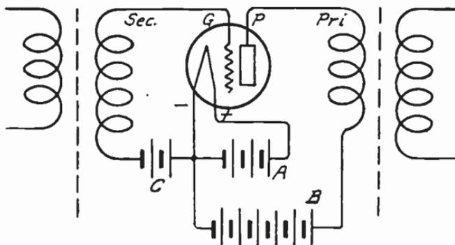
FIG. 6.—Circuits of Amplifying Stage.
