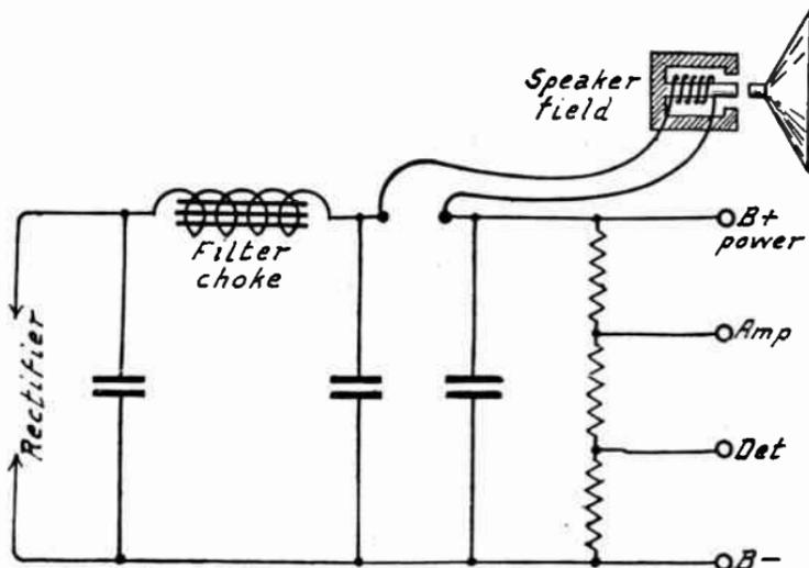
FIG. 6.—Speaker Field Used As a Filter Choke.
