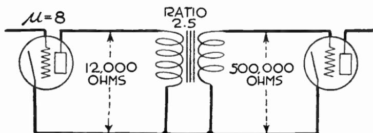
FIG. 3.—Simplified Diagram of Transformer Coupling.
