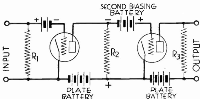
FIG. 2.—Two-Stage Direct Current Amplifier.
