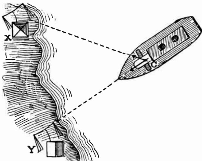
FIG. 2.—Determining Ship's Position with Radio Compass.
