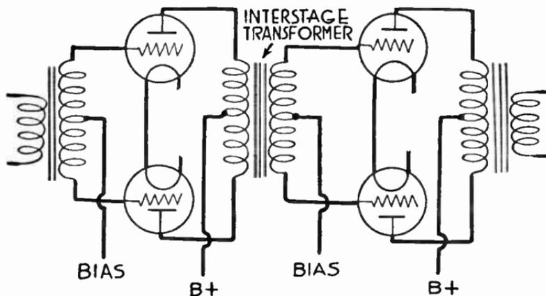
FIG. 12.—Dual Push-pull Amplification.
