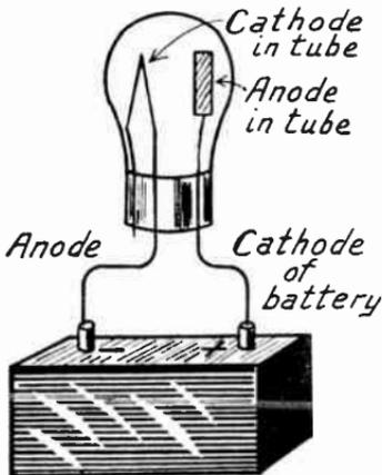
Electrodes of Tube and Battery.
