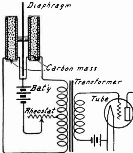
FIG. 2.—Double-button Carbon Microphone.
