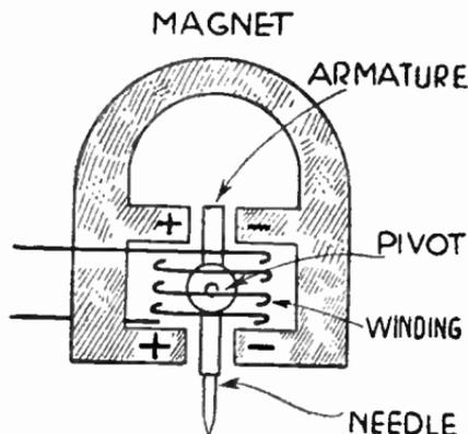
FIG. 7.—Balanced Armature Type of Electromagnetic Pickup.
