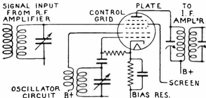
Fig. 25.—Complete Pentagrid Converter Connections.
