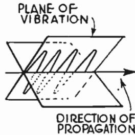
FIG. 4.—Plane Polarized Light.
