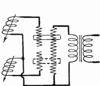
FIG. 9.—Simplified T-section Fader.
