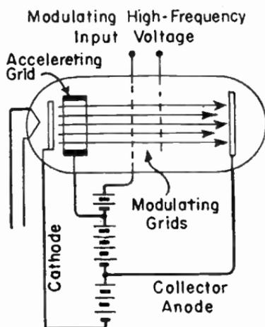
FIG. 1.—The Elements Employed for Velocity Modulation.
