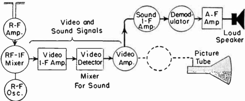
FIG. 23.—Path of Signal in Intercarrier Sound System.
