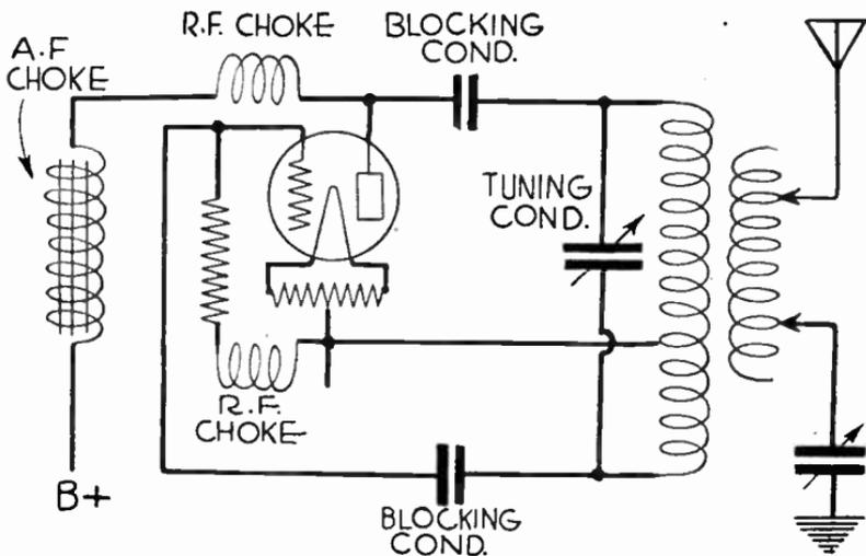
FIG. 3.—Oscillator Coupled to Transmitting Antenna.
