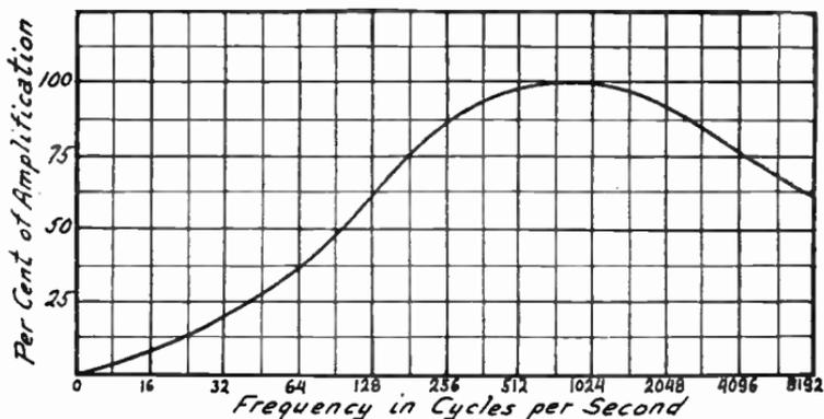
FIG. 3.—Amplification Curve of a Poor Audio Transformer.
