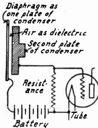
FIG. 3.—Condenser Microphone.
