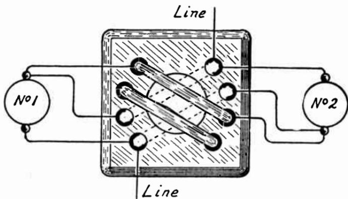
FIG. 1.—Special Form of Series-Parallel Switch.
