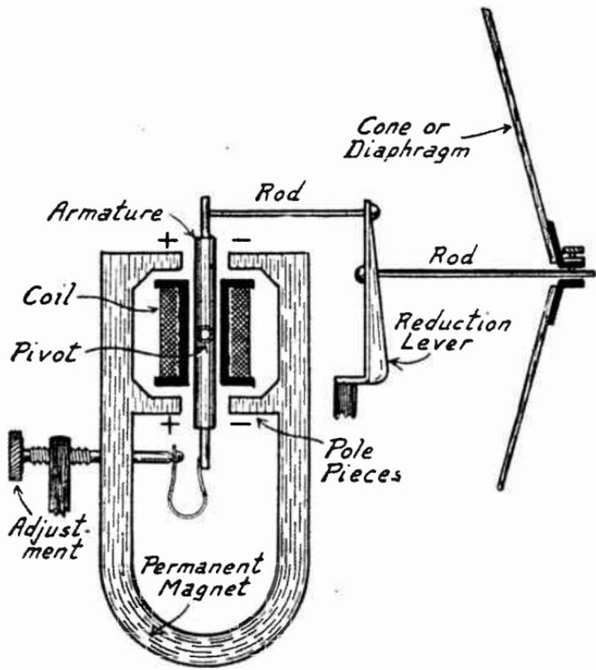
FIG. 2.—Balanced Armature Type of Loud Speaker.
