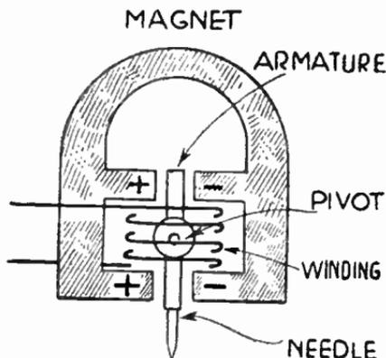
FIG. 7.—Balanced Armature Type of Electromagnetic Pickup.
