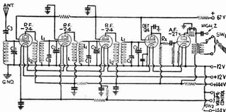
FIG. 15.—Circuits of Typical Airplane Receiver.
