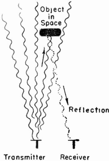
FIG. 1.—Reflection of Radar Waves.
