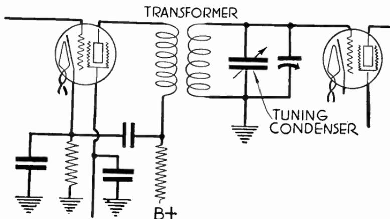
FIG. 1.—Transformer Coupling for Radio Frequencies.
