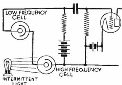
FIG. 15.—Phototube Amplification of Carrier Frequency.
