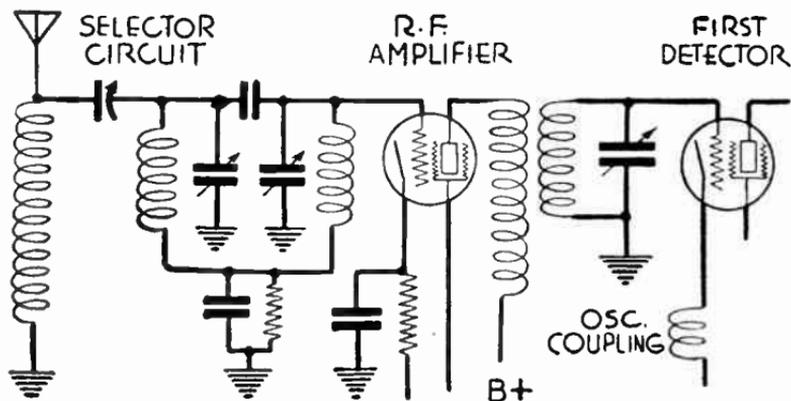
FIG. 13.—Band Selector Type of Pre-amplifier for Superheterodyne.
