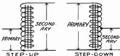
FIG. 1.—Principle of the Auto-Transformer.
