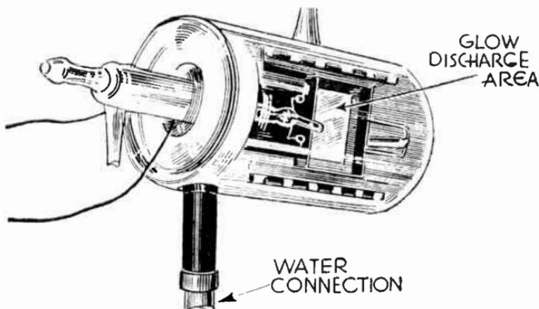
FIG. 7.—High Power Glow Lamp for Television.
