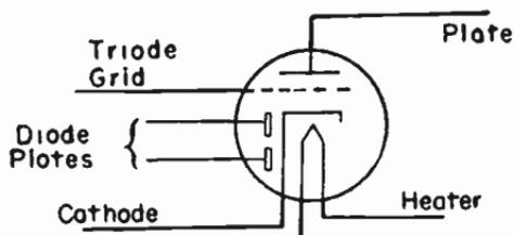
FIG. 1.—Elements of Double-diode Triode.
