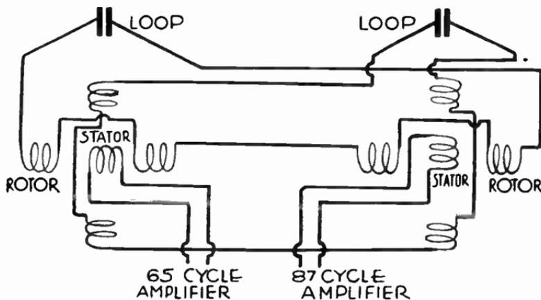
FIG. 11.—Circuit for Beacon Loops.
