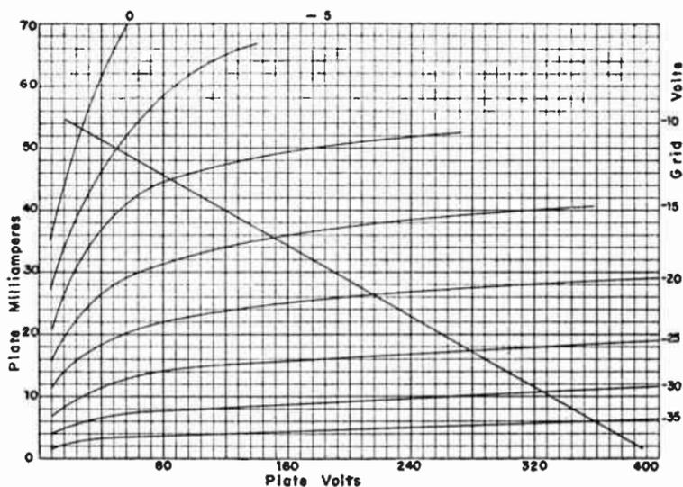
FIG. 5.—Plate Characteristics of a Power-amplifier Pentode.
