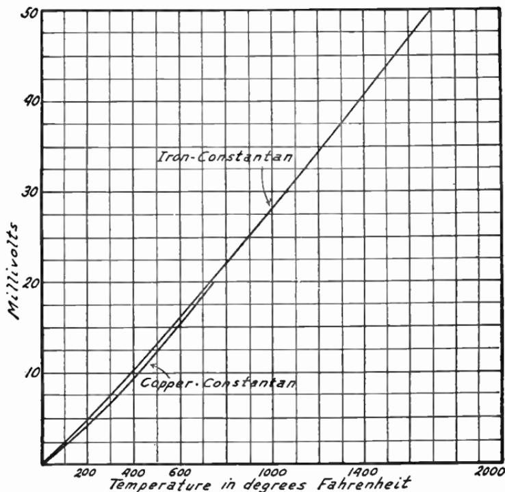
FIG. 2.—Voltage Developed by Thermocouples.
