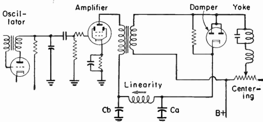
FIG. 28.—Sweep Circuits for Magnetic Deflection.
