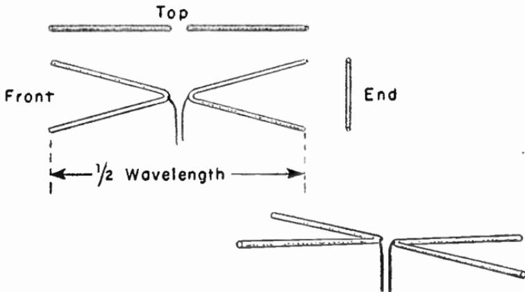
FIG. 4.—V-type or X-type antennas with conductors in a vertical plane (left) and in a horizontal plane (right).
