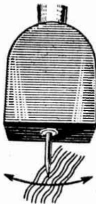
FIG. 6.—Sidewise Motion of Needle Point.
