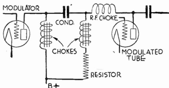
FIG. 13.—Separate Chokes for Modulator and Oscillator.
