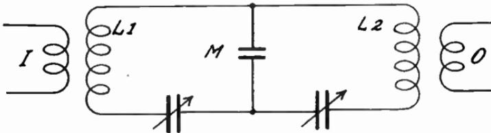
FIG. 10.—Mutual Coupling with Condenser.
