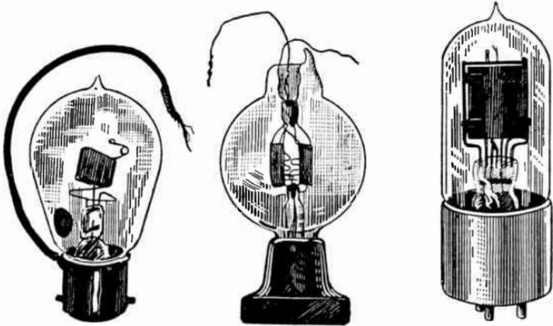
FIG. 1.—Early Experimental Types of Vacuum Tubes
