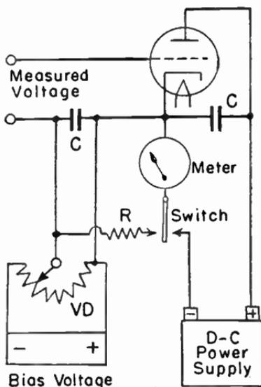
FIG. 4.—Slide Back Instrument Using a Single Meter.
