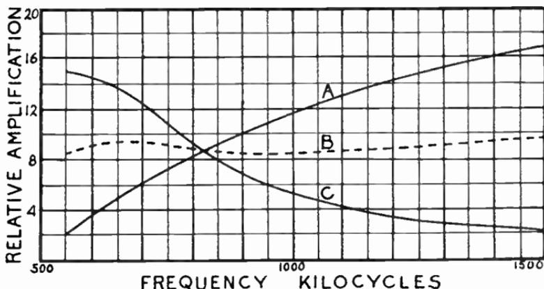
FIG. 4.—Effect of Primary Frequency on Amplification.
