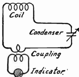
FIG. 2.—Frequency Meter with Coupled Indicator Circuit.
