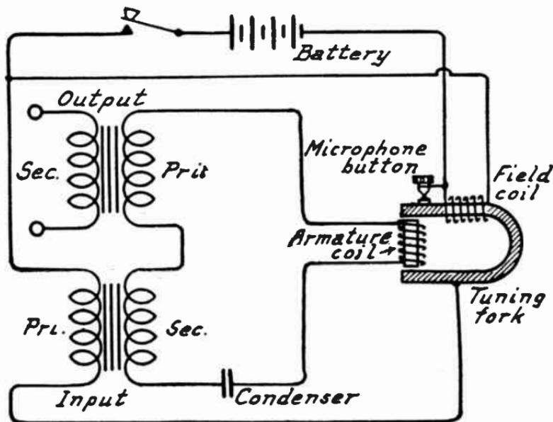
FIG. 2.—Tuning Fork Audio Oscillator.
