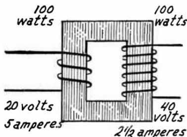
FIG. 7.—A Step-Up Transformer.
