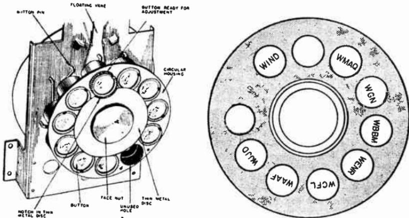
FIG. 6.—Telephone Type Tuning Dial.
