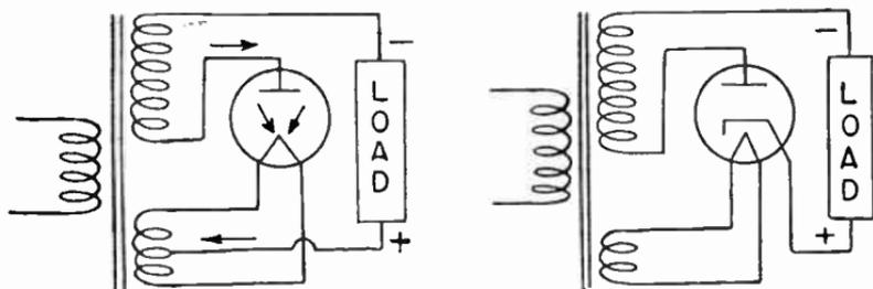
FIG. 1.—Tubes Used as Half-wave Rectifiers.
