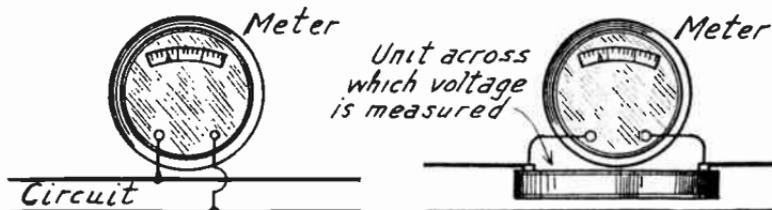
FIG. 2.—Voltmeter Connected Across a Circuit.
