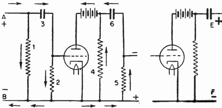
FIG. 2.—Operating Principle of the Multivibrator.
