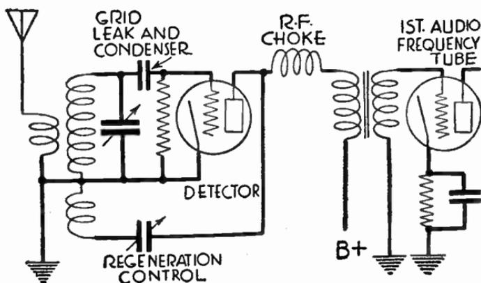
FIG. 4.—Regenerative Detector for Short Wave Reception
