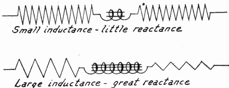
FIG. 6.—Effect of Filter Inductances on Alternating Currents.
