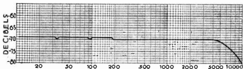
FIG. 3.—Response Curve of Velocity Microphone.
