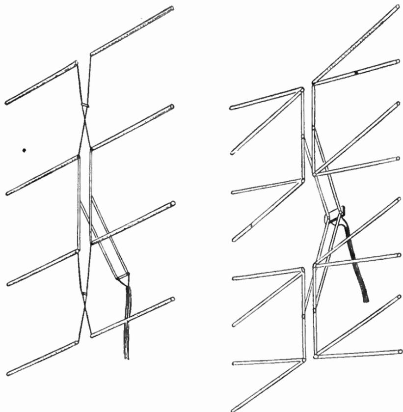
FIG. 13.—Connections for stacked antennas with four bays.
