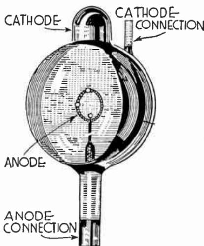
FIG. 1.—Phototube with Wall Type of Cathode.
