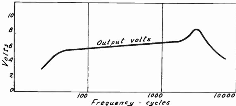
FIG. 5.—Result of Frequency Distortion in Amplifier.
