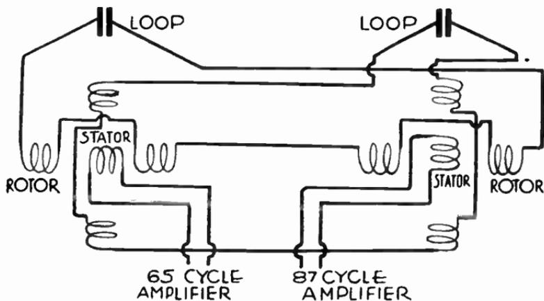
FIG. 11.—Circuit for Beacon Loops.
