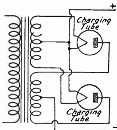
FIG. 3.—Charging Tubes Used as Filament Supply Rectifier.
