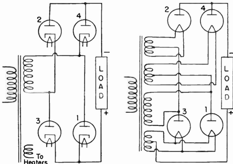
FIG. 7.—Four Tubes in Full-wave Bridge Circuit.
