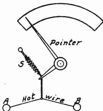
FIG. 7.—Hot Wire Meter Movement.
