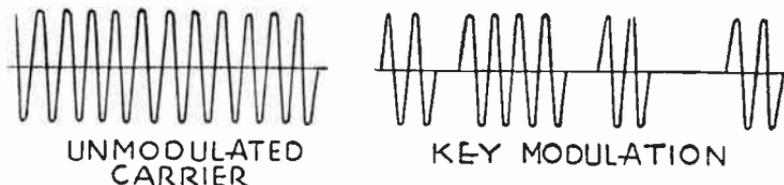
FIG. 1.—Unmodulated Carrier Wave and Key Modulation.
