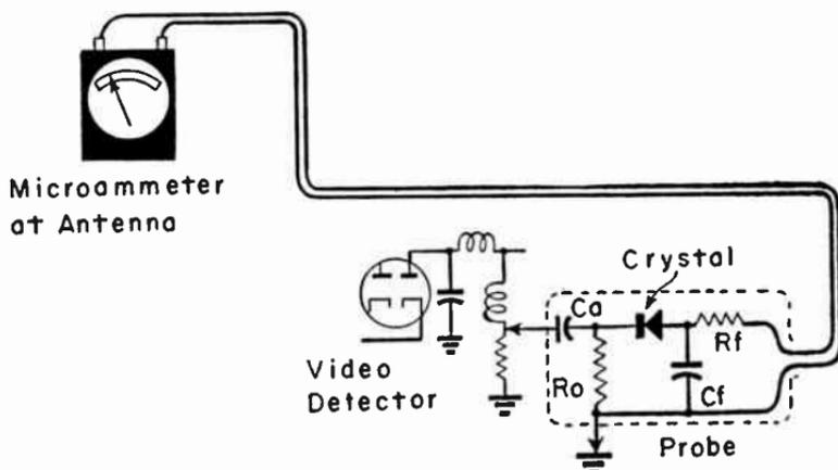
FIG. 14.—Connections for a meter used to indicate signal strengths during orientation of an antenna.
