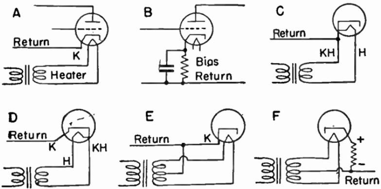
FIG. 2.—Returns for Heater-cathode Type Tubes.
