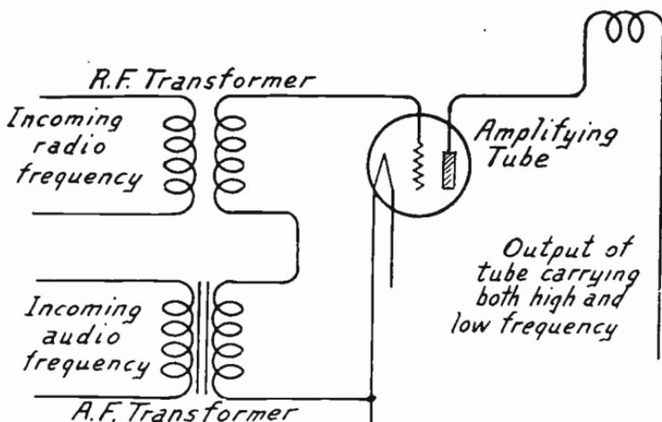
FIG. 1.—Effect of Reflexing on Amplifying Tube.
