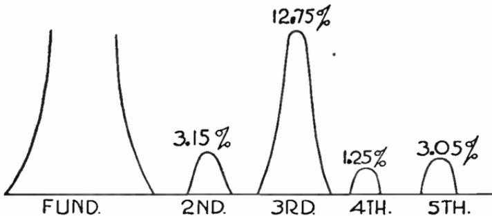
FIG. 6.—Harmonics with Push-pull Amplification.
