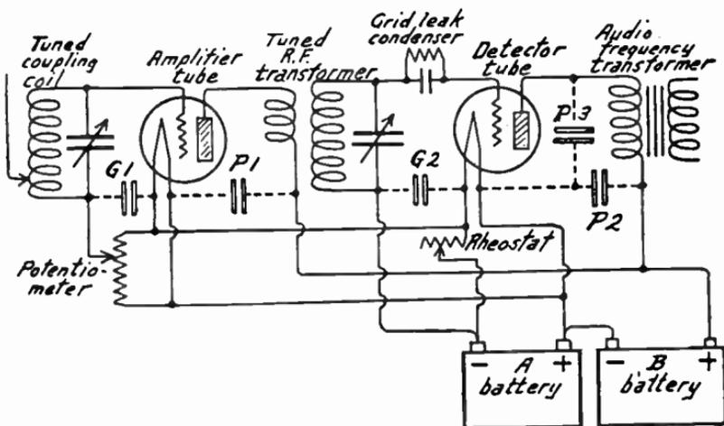
FIG. 2.—Bypass Condensers in a Receiver.
