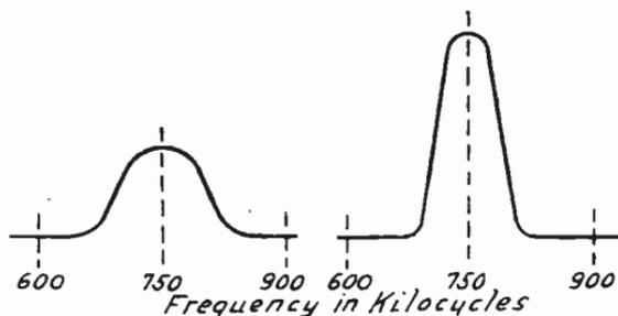
FIG. 3.—Effect of Regeneration on Signal.
