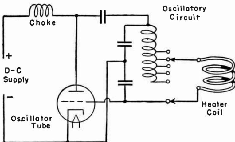
FIG. 2.—Simplified Circuit for Induction Heating.
