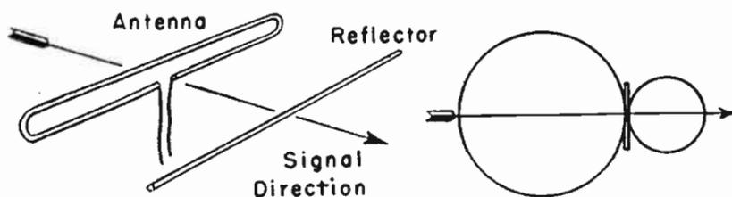
FIG. 9.—A reflector and the resulting directional pattern.
