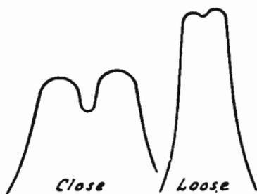
FIG. 5.—Peaks Secured with Changes in Coupling.
