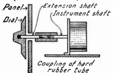
Extension Shaft for Avoiding Body Capacity Effect.
