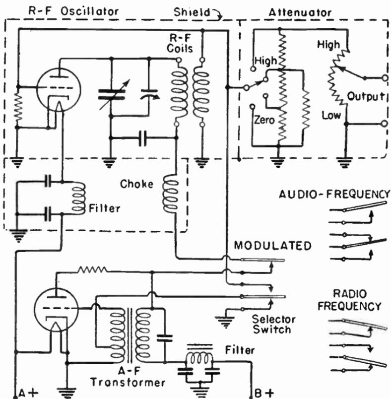
Modulated Oscillator or Signal Generator.
