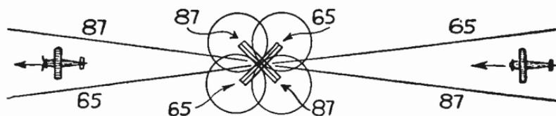
FIG. 7.—Reversal of Signals as Beacon Is Passed.
