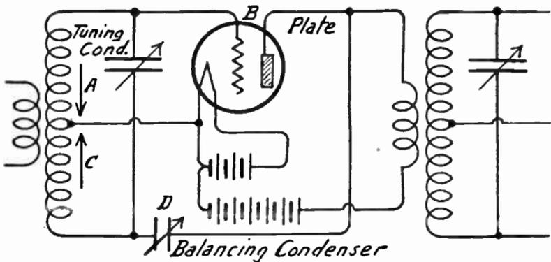
FIG. 4.—Rice Method of Balancing.
