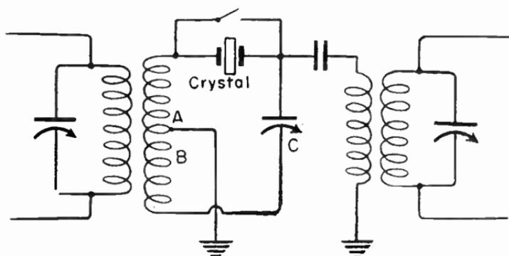
FIG. 27.—Crystal Used in Intermediate-frequency Amplifier.
