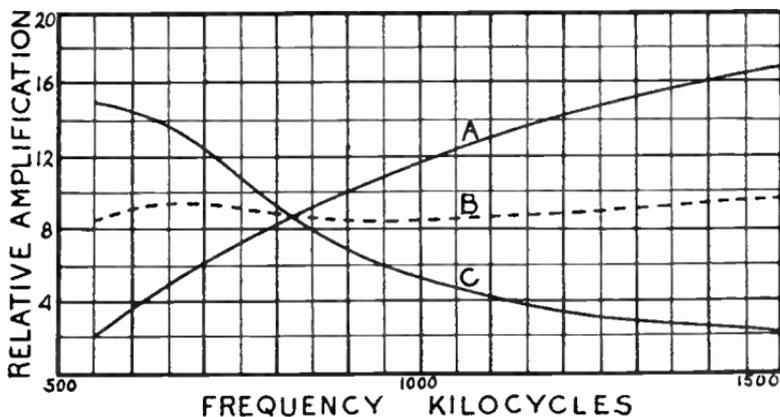
FIG. 4.—Effect of Primary Frequency on Amplification.
