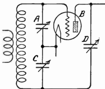
FIG. 7.—The Isofarad Method of Balancing.
