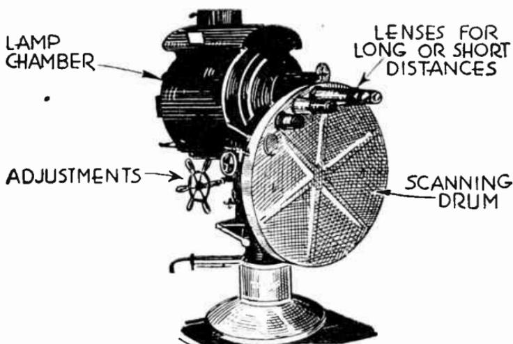
FIG. 6.—Television Scanner Employing an Arc Lamp.
