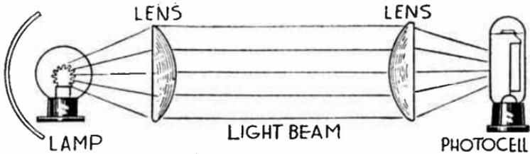
FIG. 8.—Reflector and Lenses Prevent Excessive Spread of Light.
