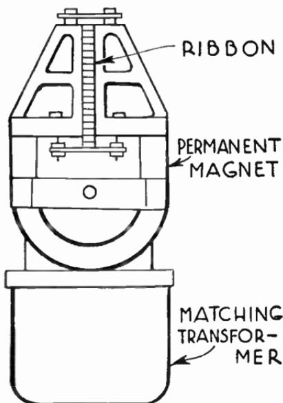
FIG. 1.—Constructional Details of Velocity Microphone.
