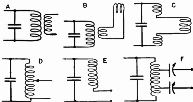
FIG. 11.—Output Connections for Taking Power from the Plate Circuits of Oscillators.
