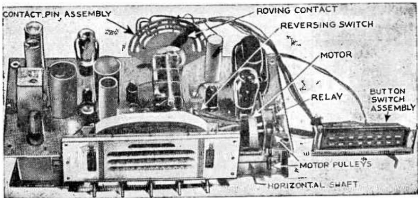
FIG. 1.—General Electric Touch Tuning Chassis.
