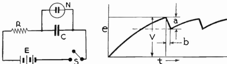
FIG. 10.—Relaxation Oscillator Showing Resulting Saw-tooth Wave Shape.
