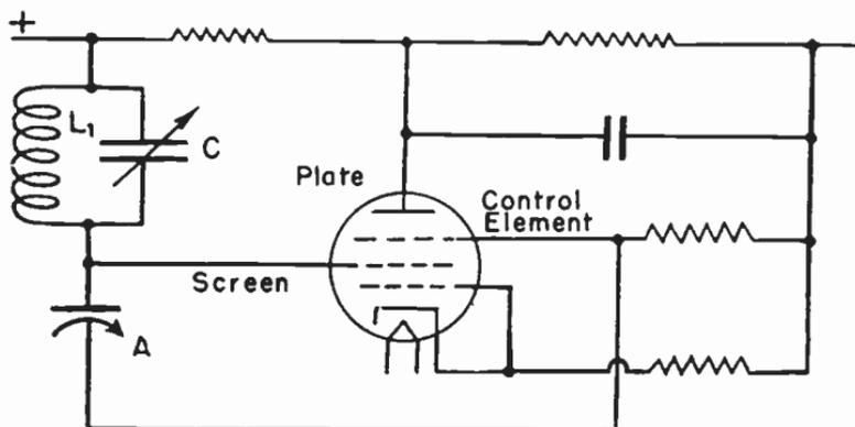
FIG. 8.—Negative Transconductance Oscillator.
