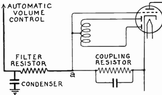
FIG. 3.—Double-diode in Automatic Volume Control.
