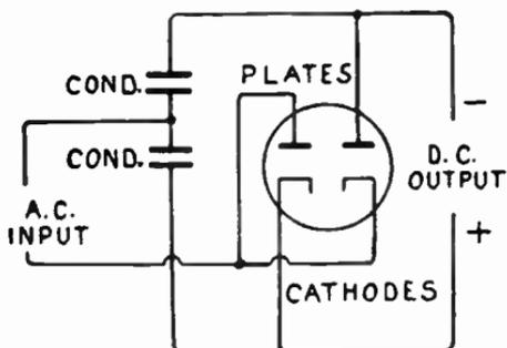
FIG. 1.—Voltage Doubler Connections.
