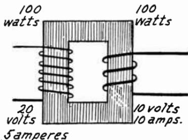
FIG. 8.—A Step-Down Transformer.
