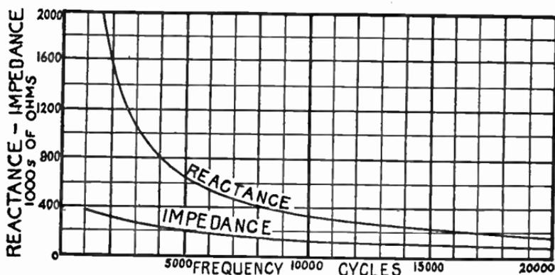
FIG. 8.—Effect of Frequency on Reactance and Impedance.
