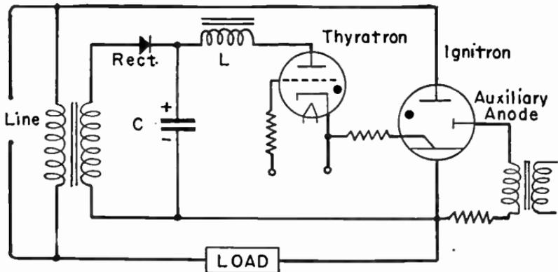
FIG. 4.—Ignitron Control Circuit with Auxiliary Anode Connections.
