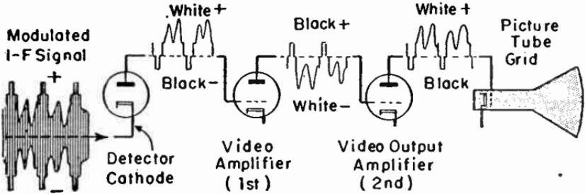
FIG. 21.—Signal Polarities with Two Video Amplifiers.
