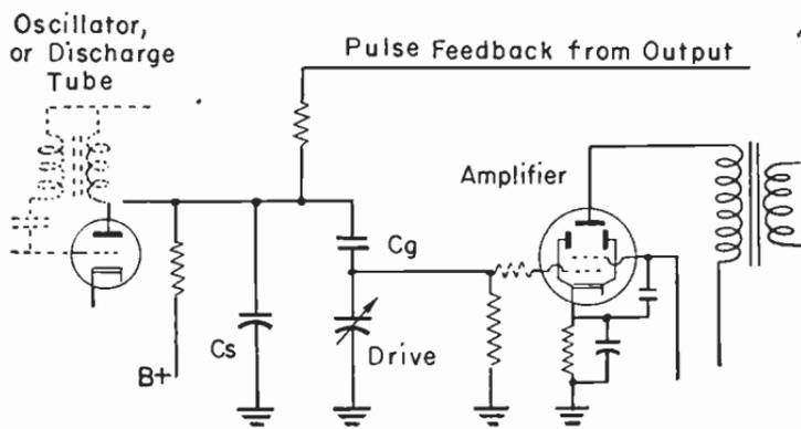
FIG. 32.—A Drive Control in the Amplifier Grid Circuit.
