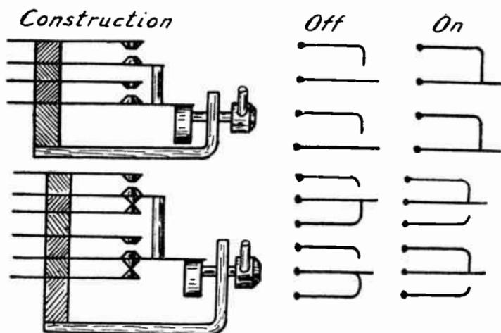
FIG. 2.—Operation of a Jack Switch.
