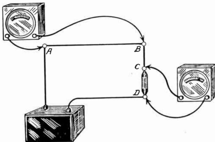
FIG. 1.—Principle of Testing for Open Circuits.
