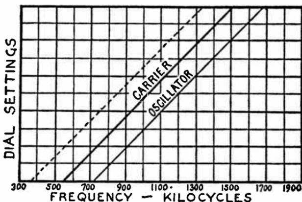
FIG. 5.—Relation of Oscillator and Carrier Frequencies.
