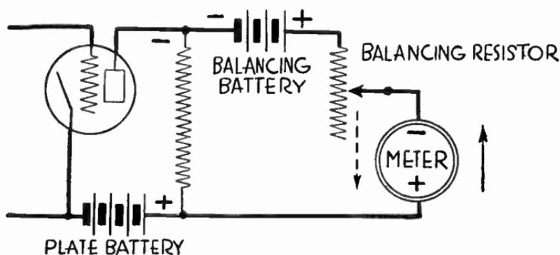
FIG. 3.—Balancing the Plate Resistor Voltage.
