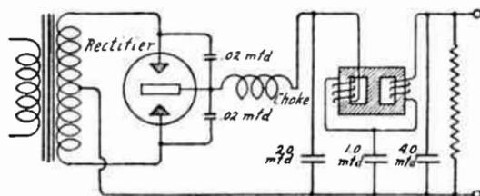
FIG. 9.—Connection of Bucking Coil Filter Choke.
