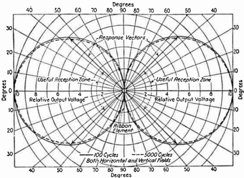
FIG. 4.—Polar Response Curve of Velocity Microphone.
