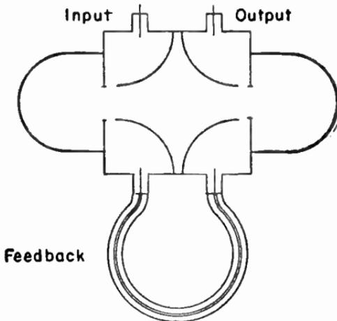
FIG. 2.—Feedback for Klystron Used as an Oscillator.
