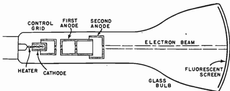
FIG. 1.—Principal Parts of a Cathode-ray Tube.
