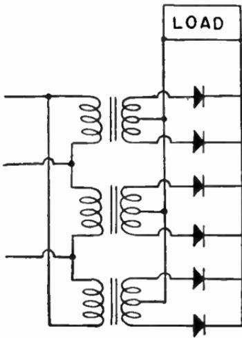
FIG. 4.—Six Elements with Center-tapped Transformer.
