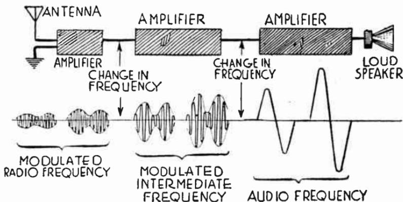
FIG. 1.—The Three Frequencies Used in Superheterodyne Reception.
