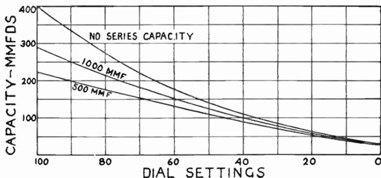
FIG. 22.—How Series Capacities Affect the Tuning.
