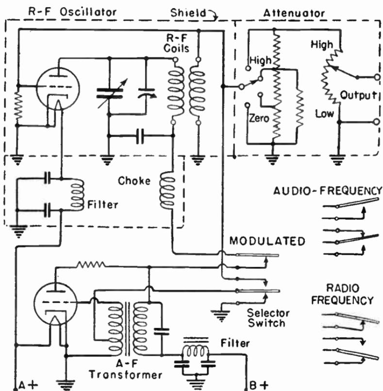
Modulated Oscillator or Signal Generator.
