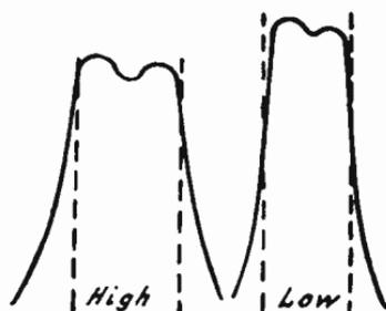
FIG. 6.—Effect of Frequency on Resonance Peaks.
