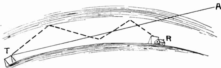
FIG. 3.—Reflection of Radiated Waves.
