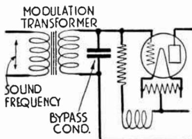
FIG. 4.—Grid Circuit Modulation.
