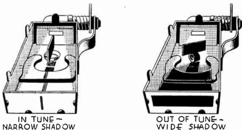
FIG. 12.—Iron Vane Tuning Meter
