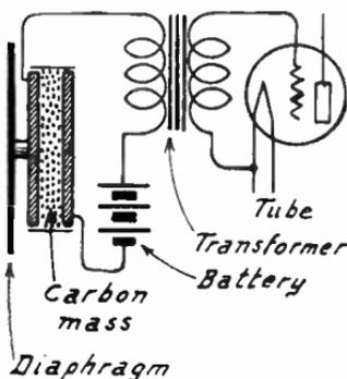
FIG. 1.—Simple Type of Microphone.
