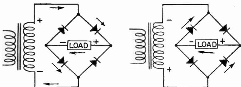
FIG. 6.—Bridge Type Full-wave Rectifier.
