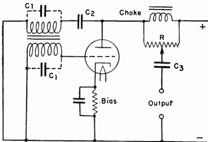
FIG. 1.—Feedback Type of Audio-frequency Oscillator.
