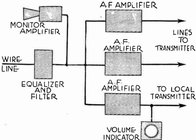
FIG. 5.—Bridging System Used in Chain Broadcasting.
