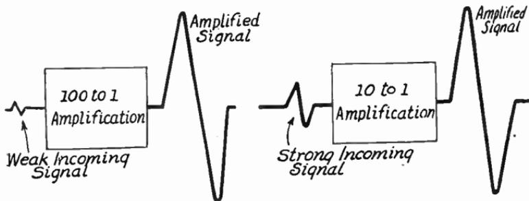
The Effect of Amplification on Signal Strength.
