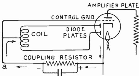
FIG. 2.—Double-diode Triode as Detector and Amplifier.
