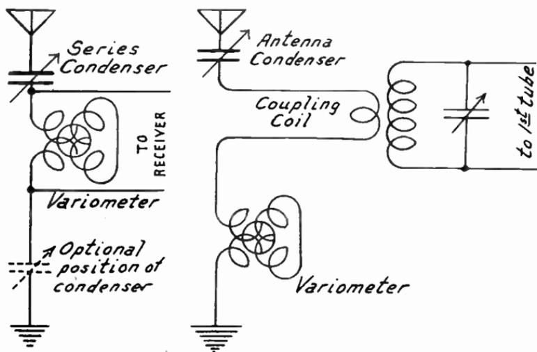
FIG. 4.—Variometer and Series Condenser for Antenna.
