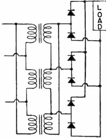
FIG. 5.—Six Elements in a Bridge Circuit.
