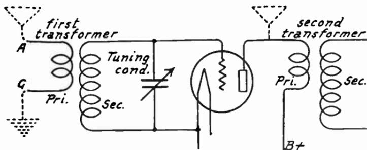
FIG. 1.—Antenna Connections for Testing Radio Stages.
