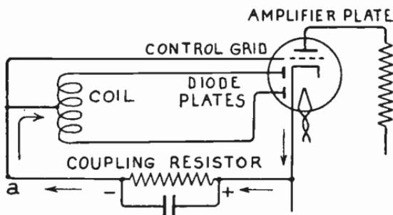
FIG. 2.—Double-diode Triode as Detector and Amplifier.
