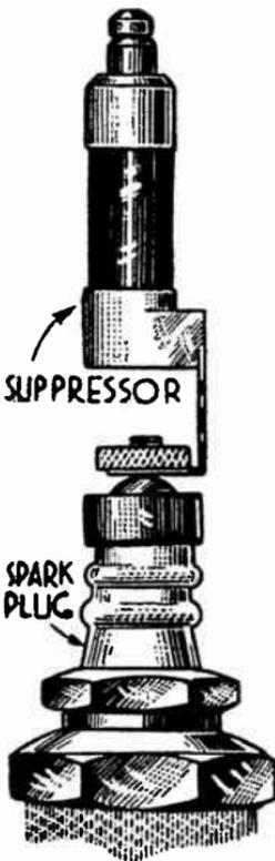
FIG. 10.—Spark Plug Auto Radio Suppressor.
