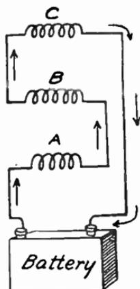
FIG. 1.—A Series Circuit.
