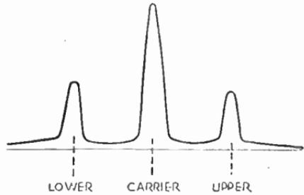
FIG. 8.—Side Frequencies and Carrier Frequency.
