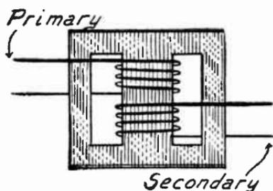
FIG. 3.—Shell Type Transformer.
