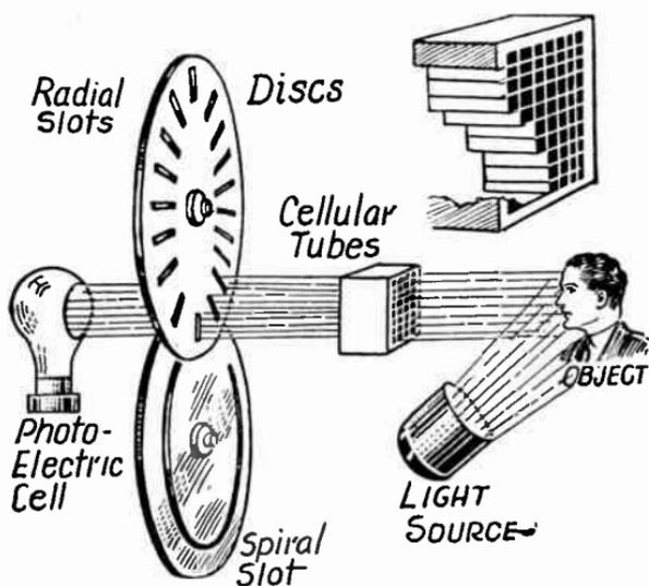
FIG. 3.—Action of Baird Discs in Television.
