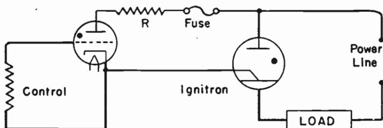
FIG. 2.—Thyratron Used for Control of an Ignitron.
