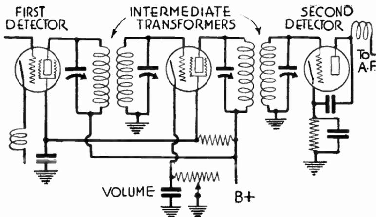
FIG. 14.—Typical Intermediate Frequency Amplifier.
