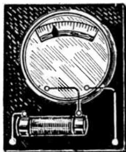
FIG. 5.—Milliammeter Used as Voltmeter.
