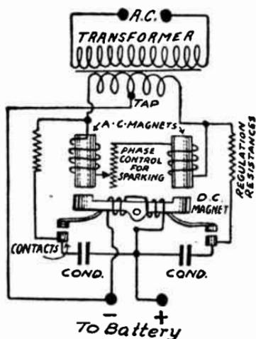
FIG. 1.—Full-wave Vibrating Rectifier.
