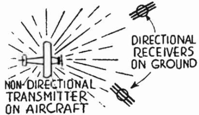
FIG. 2.—Airplane Transmitter and Ground Receivers.
