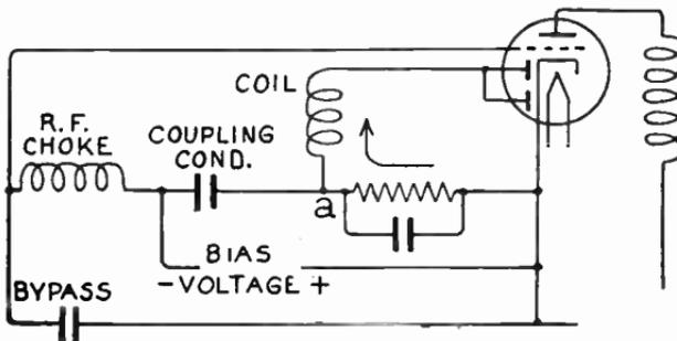
FIG. 4.—Double-diode Half-wave Detector.
