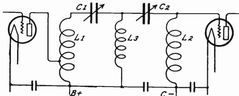
FIG. 7.—Circuit Arrangement of Vreeland Band Selector.
