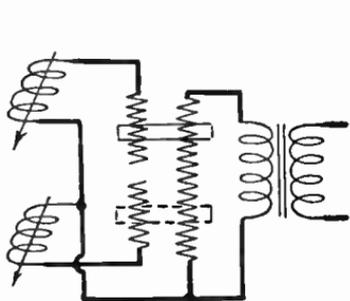
FIG. 9.—Simplified T-section Fader.
