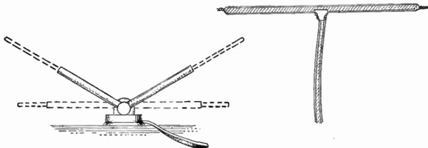
FIG. 15.—Two types of indoor antennas.
