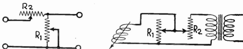
FIG. 5.—L-section Attenuators.
