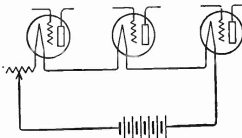
FIG. 2.—Tube Filaments in Series Circuit.
