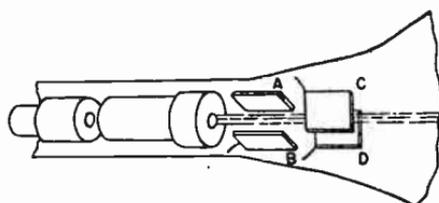
FIG. 3.—Electrostatic Deflection of the Beam.
