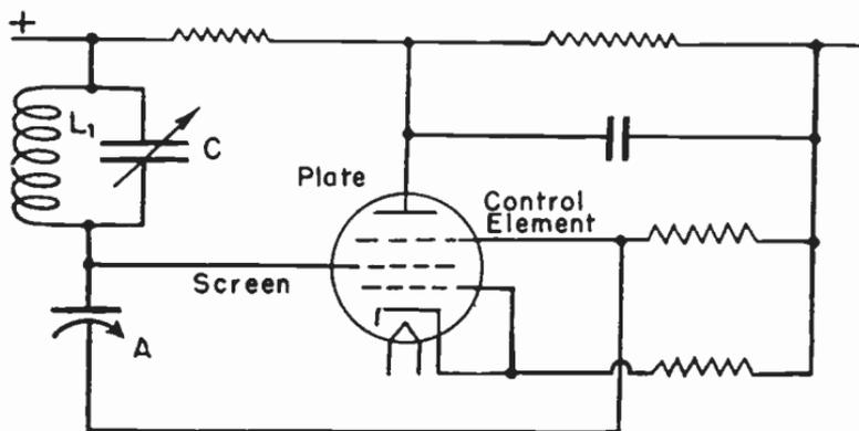
FIG. 8.—Negative Transconductance Oscillator.
