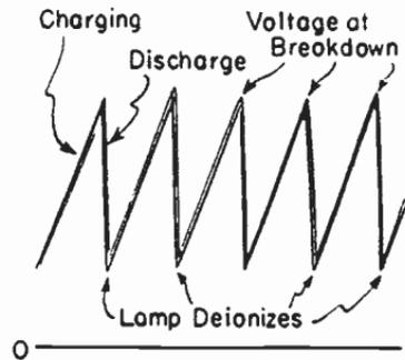
FIG. 5.—Output Wave Form of Neon Oscillator.
