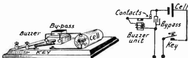
Construction and Circuit of Buzzer Exciter.
