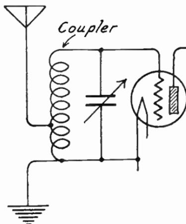
FIG. 4.—Auto-Transformer Antenna Coupling.
