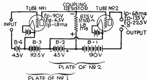
Fig. 1.—Simple Form of Direct Coupled Amplifier.
