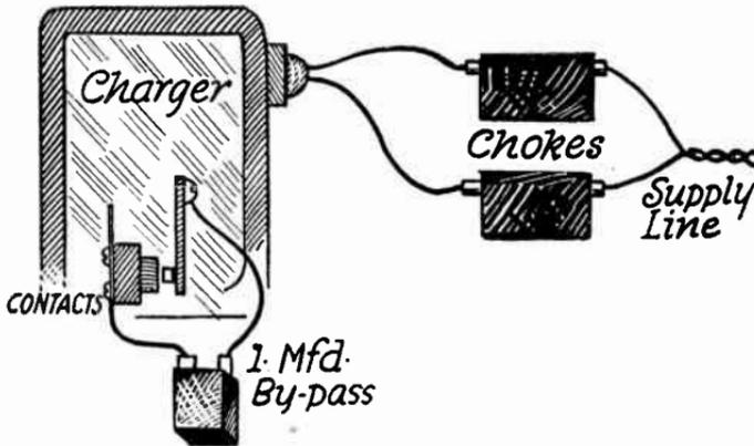
FIG. 5.—Handling Interference of Vibrators and Flashers.
