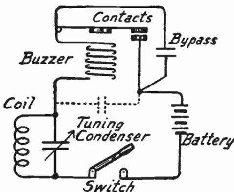
Oscillator Circuit Excited by Buzzer.
