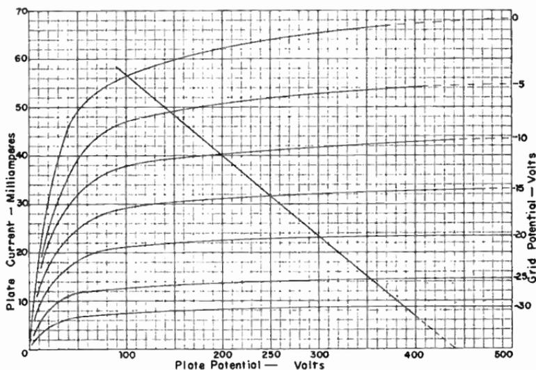
FIG. 4.—A 6,000-ohm Load Line on the Plate Characteristics.
