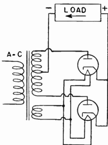
FIG. 2.—Two Heater-cathode Tubes in Full-wave Rectifier.
