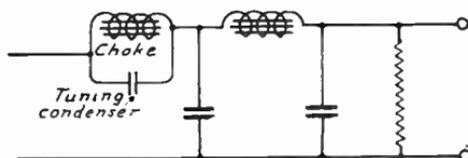
FIG. 10.—Principle of Tuned Filter.
