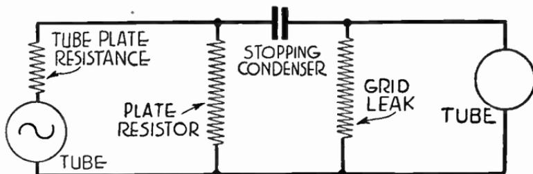
FIG. 2.—Simplified Diagram of Resistance Coupling.
