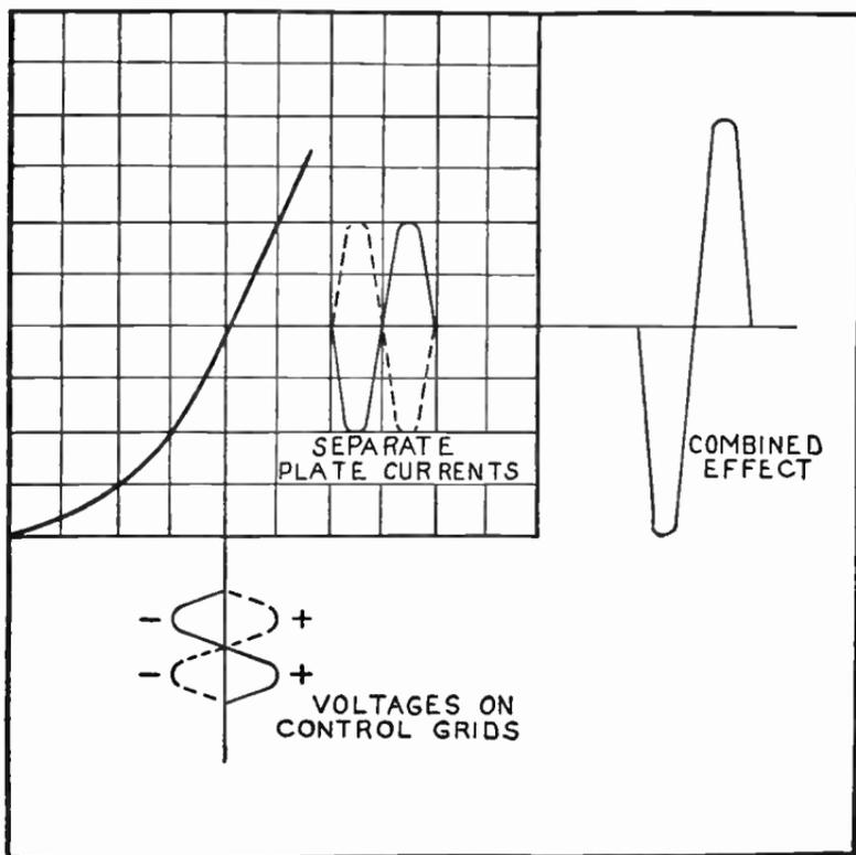
FIG. 2.—Combining Plate Currents in Push-pull Amplifier.
