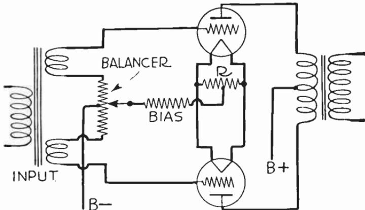
FIG. 8.—Equalizing Plate Currents in Push-pull Tubes.
