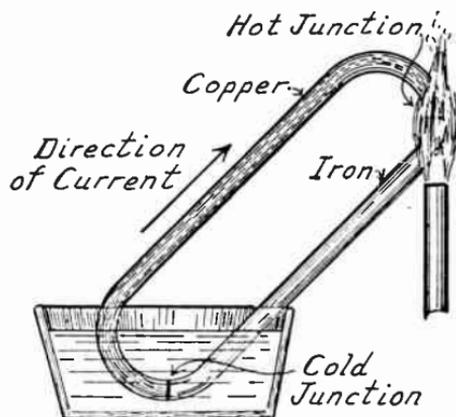
FIG. 1.—Principle of the Thermocouple.
