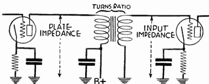
FIG. 2.—Circuit for Transformer Coupling.
