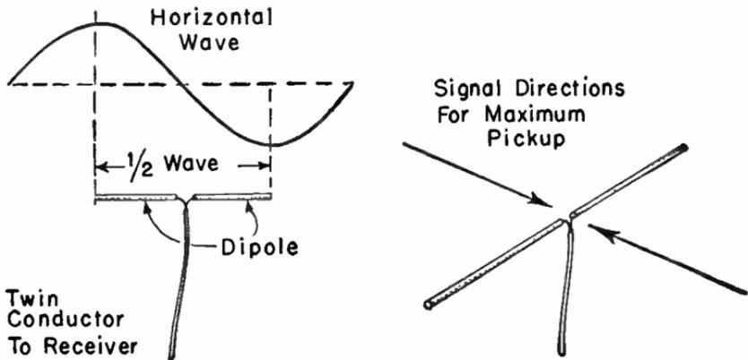
FIG. 14.—Half-wave Dipole Antenna.
