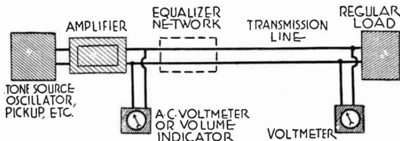
FIG. 5.—Making Measurements for Line Equalizing.
