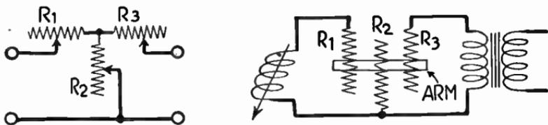
FIG. 6.—T-section Attenuators.
