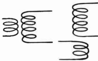
FIG. 6.—Symbols for Air Core Transformer.
