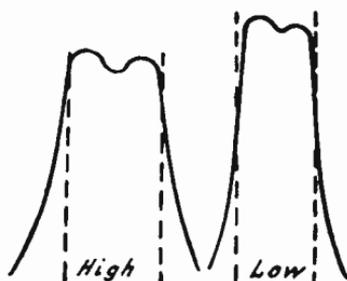
FIG. 6.—Effect of Frequency on Resonance Peaks.
