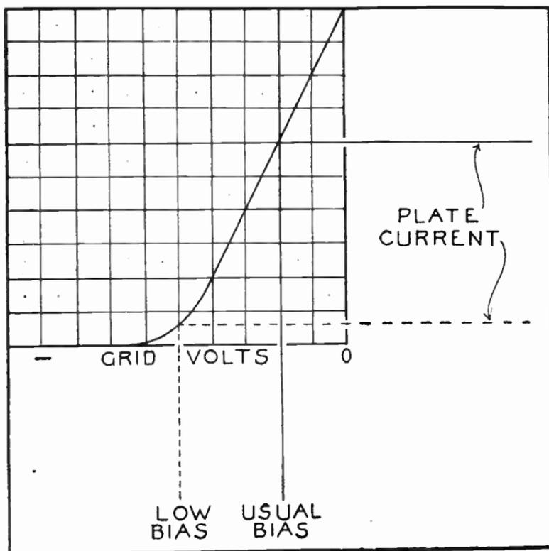
FIG. 5.—Biasing Points on Characteristic Curve.
