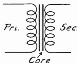
FIG. 4.—Symbol for Iron Core Transformer.
