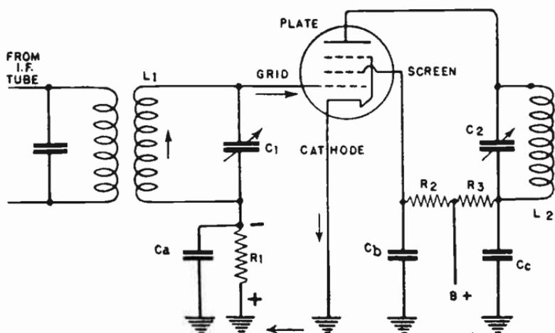
FIG. 3.—Connections for a Typical Limiter.
