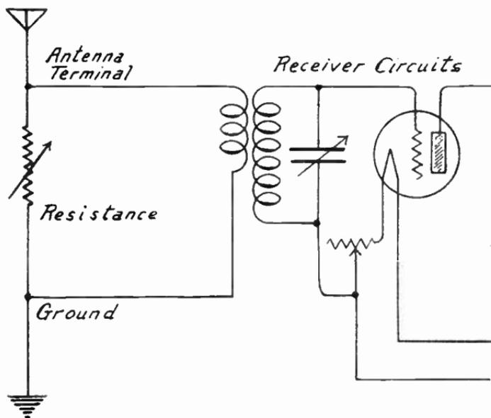
FIG. 1.—Using Resistance to Reduce Effect of Interference.
