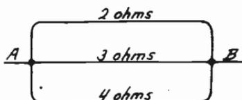
FIG. 4.—Parallel Circuits with Unequal Resistances.
