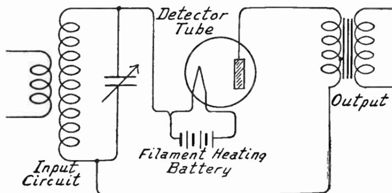
Elementary Principle of Diode Detector.
