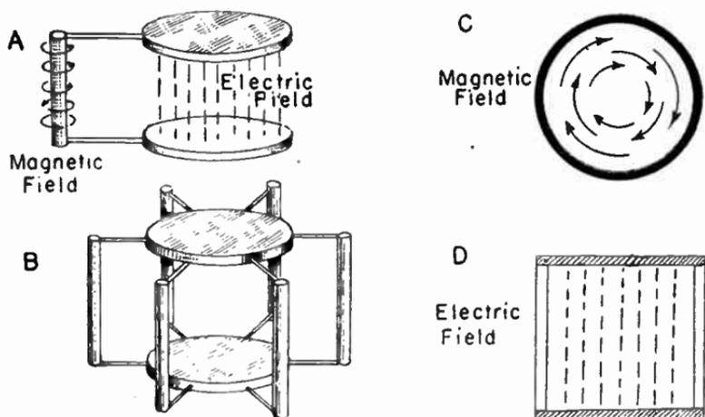
FIG. 1.—Principle of the Cavity Resonator.
