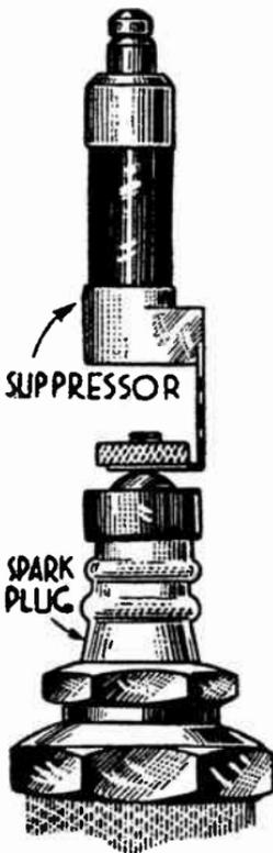
FIG. 10.—Spark Plug Auto Radio Suppressor.
