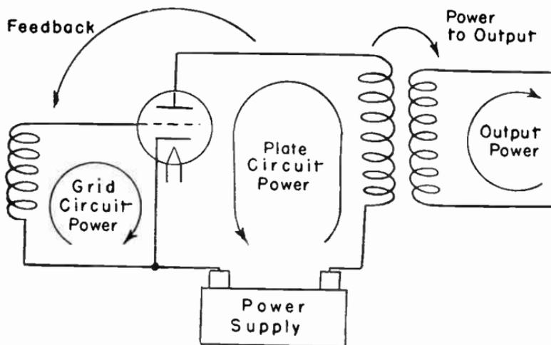
FIG. 1.—Principle of the Feedback Oscillator.
