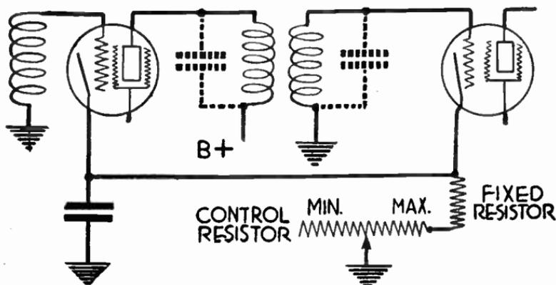
FIG. 15.—Volume Control by Variation of Cathode Resistor.
