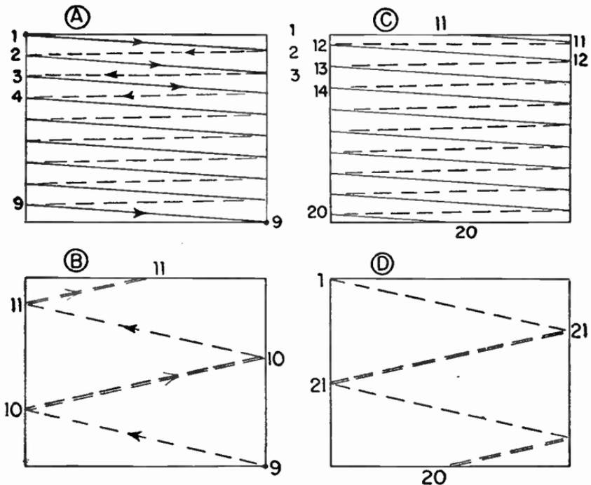
FIG. 3.—Travel of Electron Beam for Interlaced Scanning.
