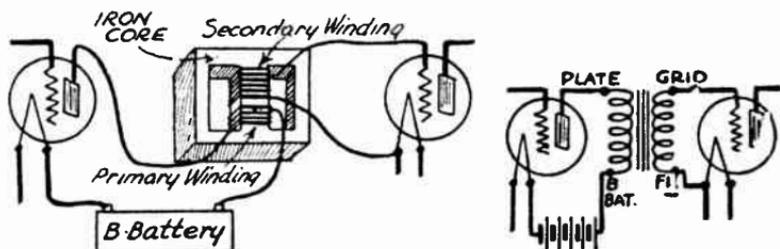
FIG. 1.—Transformer Coupling for Audio Frequency Amplifier.
