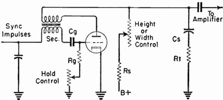
FIG. 26.—Blocking Oscillator Used in Sweep Circuits.
