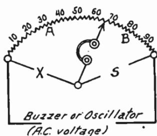
FIG. 4.—Principle of the Slide Wire Bridge.
