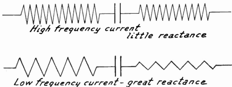
FIG. 5.—Effect of Filter Condensers on High and Low Frequencies.
