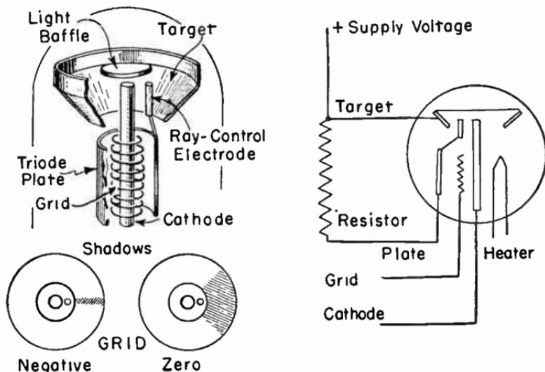
FIG. 2.—Tube and Circuit for Single Control Electrode.
