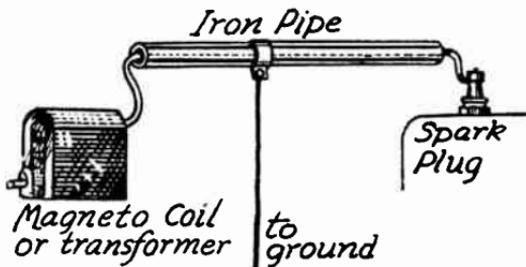
FIG. 6.—Shielding of Ignition Circuits to Prevent Interference.
