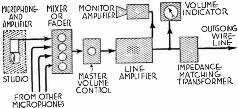
FIG. 1.—Speech Input Equipment for Broadcasting.
