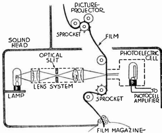
FIG. 12.—Principal Parts of a Sound Head.
