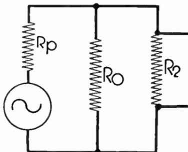
FIG. 4.—Coupling Circuit without Condenser.
