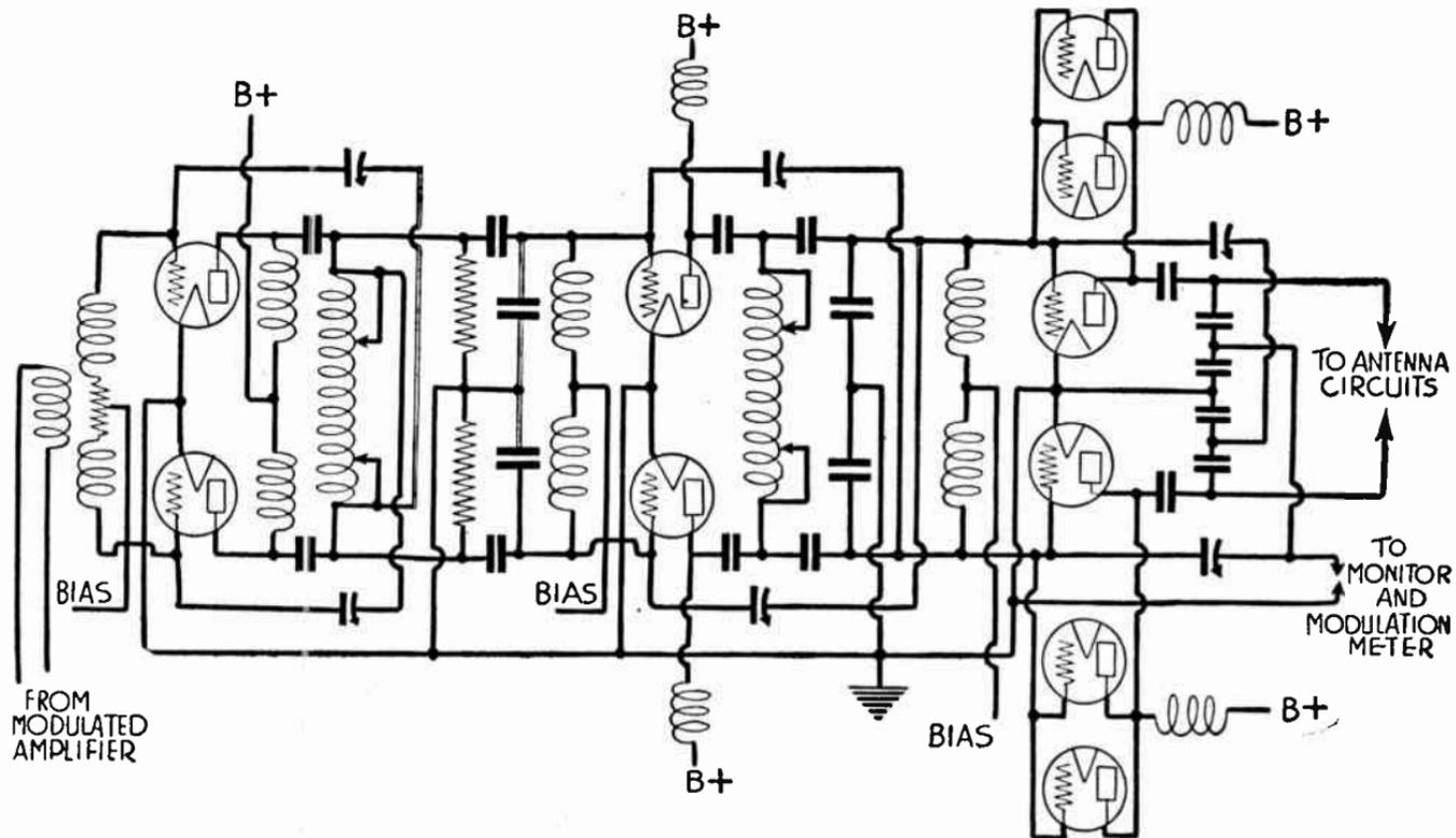
FIG. 9.—Power Amplifier Used at Transmitter.
