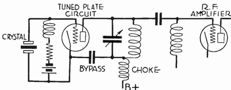
FIG. 3.—Circuit of Crystal Controlled Oscillator.
