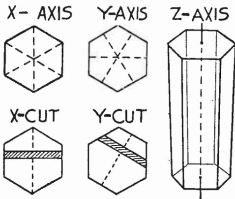
FIG. 2.—Methods of Cutting Quartz Plates.
