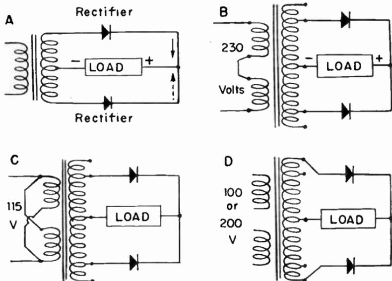
FIG. 5.—Contact Rectifiers in Full-wave Circuits.
