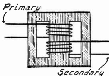
FIG. 3.—Shell Type Transformer.
