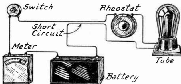
FIG. 2.—Testing for Short Circuit with Voltmeter.
