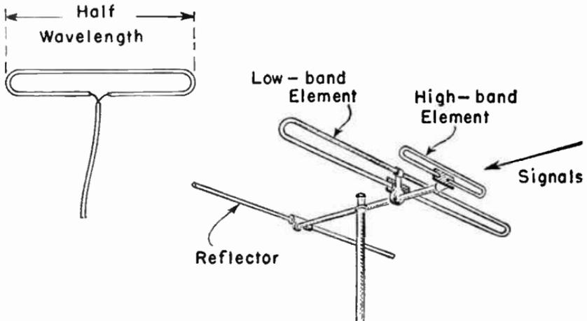
FIG. 16.—Folded Dipole Antenna.
