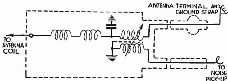
FIG. 11.—“Magic Eliminode” Used on Galvin Motorola Automobile Radio Receivers.
