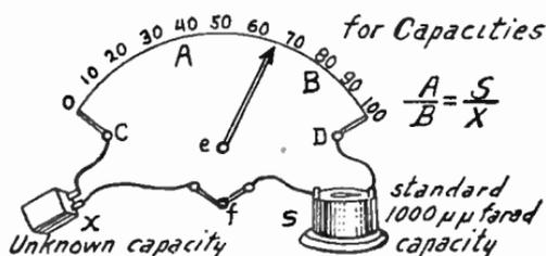
FIG. 8.—Capacity Measurement with Bridge.
