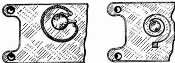
Pigtail Connections for Rotor Shafts.
