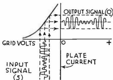
FIG. 1-A.—Class A Operating Characteristics.
