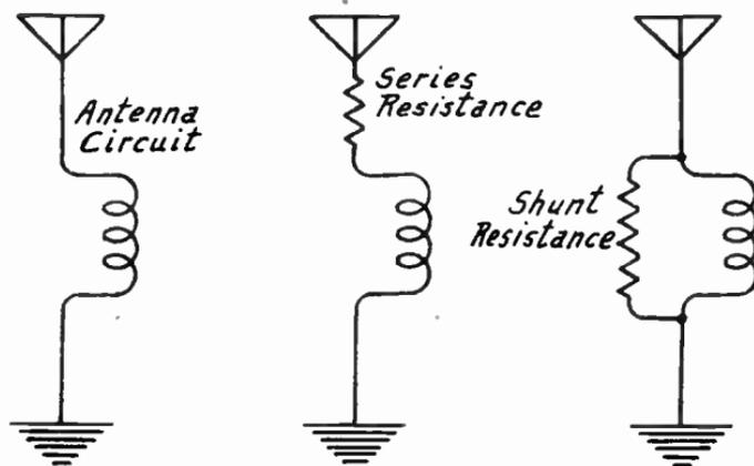
FIG. 2.—Equivalent Resistances in Antenna Circuit.
