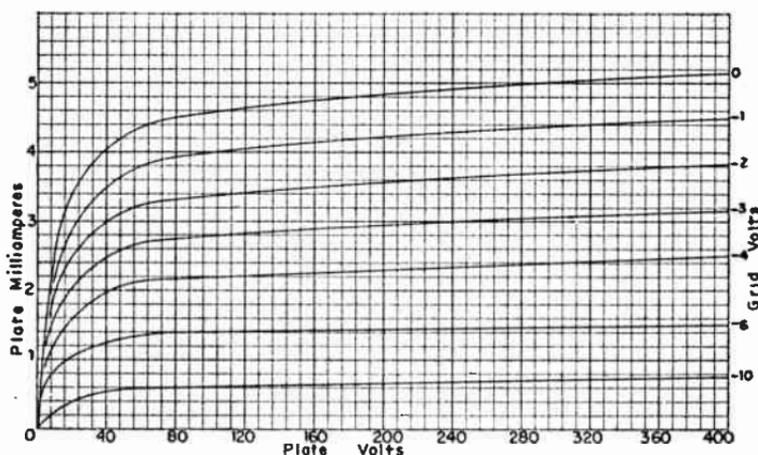
FIG. 4.—Plate Characteristics of a Voltage-amplifier Pentode.
