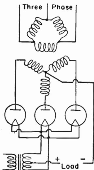
FIG. 1.—Polyphase Half-wave Rectifier.
