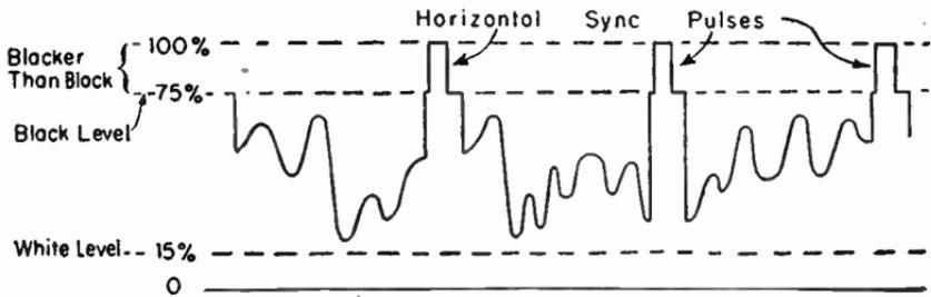
FIG. 7.—Horizontal Sync Pulses During Blanking Intervals.
