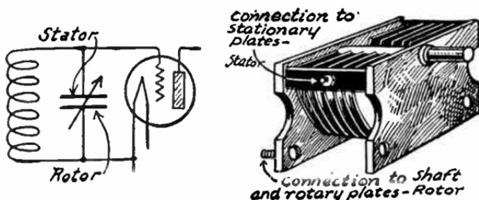
FIG. 4.—Connections to Rotor and Stator of Condenser.
