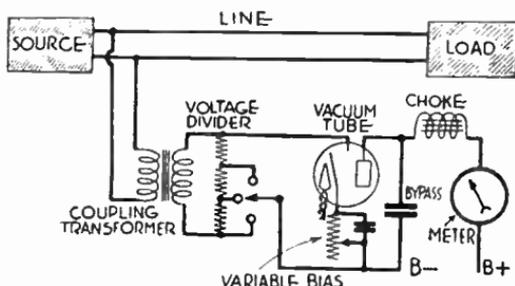
FIG. 2.—Vacuum Tube Type of Volume Indicator.
