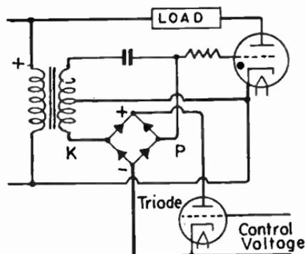
FIG. 10.—Phase-shift Control by Means of a Vacuum Triode Connected to a Bridge Rectifier.
