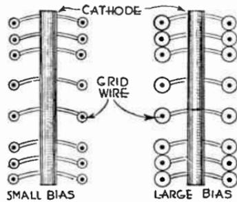
FIG. 2.—Control Grid Spacing in Variable-mu Tube.
