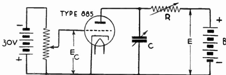
FIG. 11.—Thyatron Sweep Circuit Oscillator.
