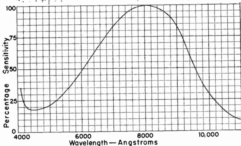
FIG. 4.—Wavelength Sensitivity of One Type of Phototube.
