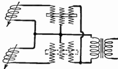
FIG. 8.—T-section Type of Fader.
