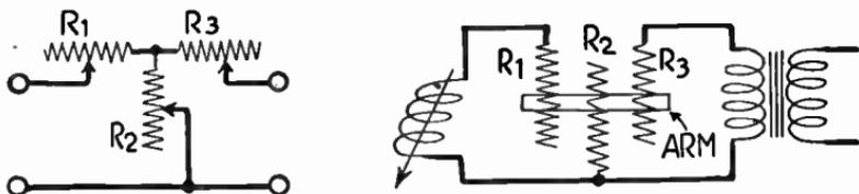
FIG. 6.—T-section Attenuators.
