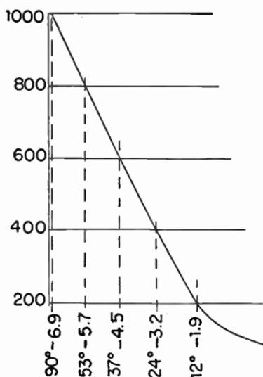
FIG. 7.—Average Grid and Anode Potentials for Breakdown.
