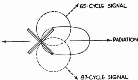
FIG. 10.—Radiation from Visual Beacon Transmitter.
