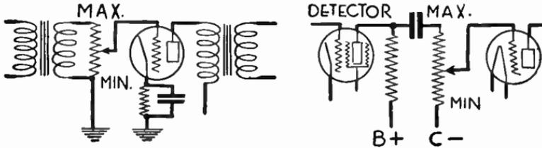
FIG. 18.—Volume Control in Audio Frequency Stages.
