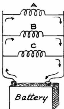
FIG. 1.—Parallel Circuits.
