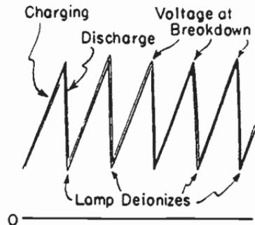
FIG. 5.—Output Wave Form of Neon Oscillator.
