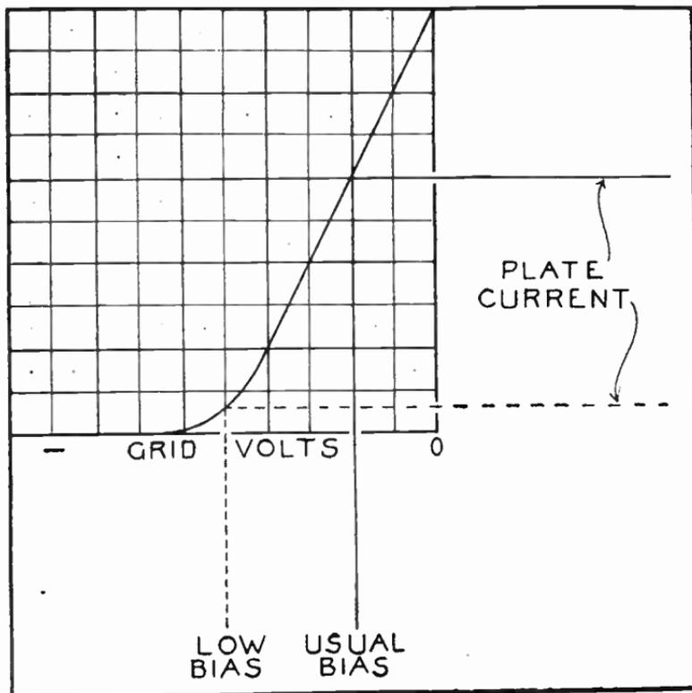
FIG. 5.—Biasing Points on Characteristic Curve.
