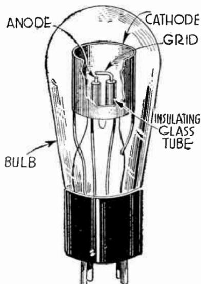
FIG. 1.—Construction of One Style of Grid-glow Tube.
