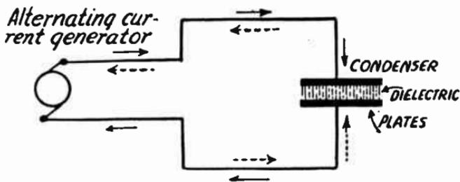
FIG. 6.—Flow of Alternating Current Through a Condenser.
