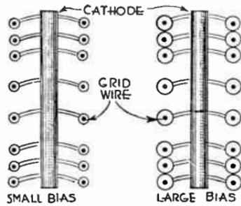
FIG. 2.—Control Grid Spacing in Variable-mu Tube.
