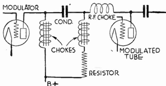
FIG. 13.—Separate Chokes for Modulator and Oscillator.
