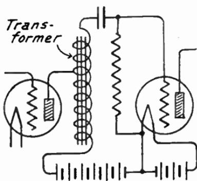
FIG. 3.—Auto-Transformer Interstage Coupling.
