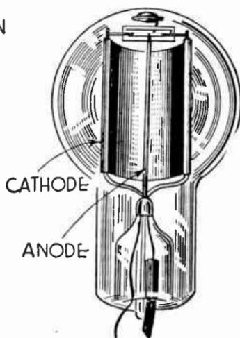
FIG. 2.—Phototube with Inserted Cathode.
