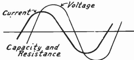
FIG. 2.—Current Leading Voltage.
