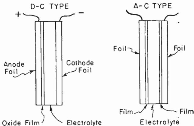
Elements Used in Electrolytic Condensers.
