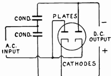
FIG. 1.—Voltage Doubler Connections.
