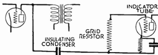
FIG. 3.—Indicator Connection Through Condenser.
