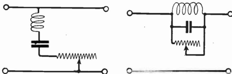
FIG. 6.—Filters for Reduction of Resonance Peaks.
