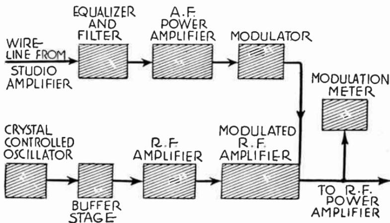
FIG. 2.—Low Power Equipment for Amplifying.
