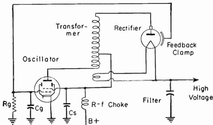
FIG. 38.—High-voltage Supply Using an R-f Oscillator.
