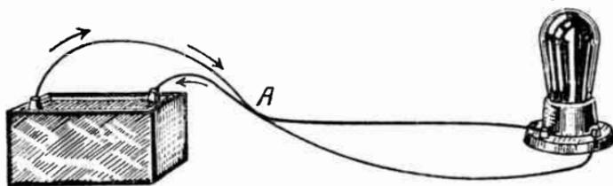
FIG. 1.—Short Circuit in Filament Lines.
