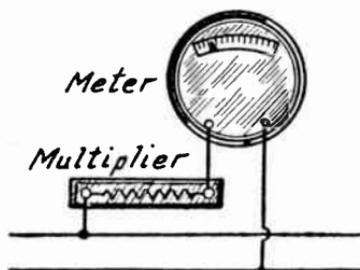
FIG. 3.—Multiplier Used with Voltmeter.
