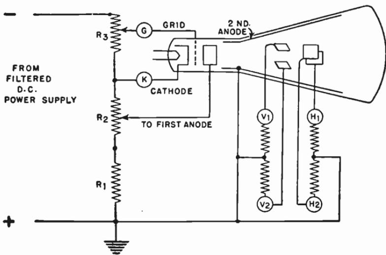
FIG. 4.—Control Circuits for Cathode-ray Tube.
