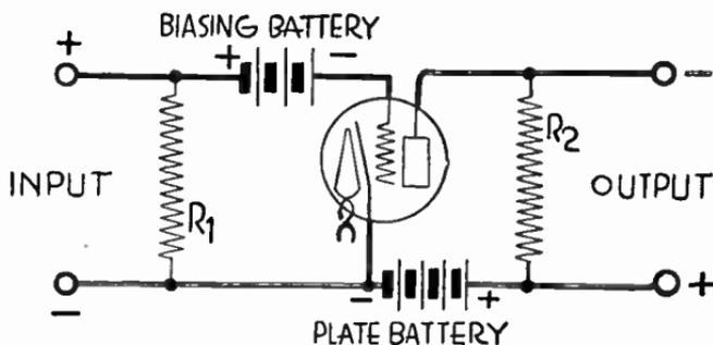
FIG. 1.—Simple Form of Direct Current Amplifier.
