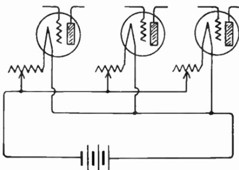
FIG. 2.—Tube Filaments in Parallel Circuit.
