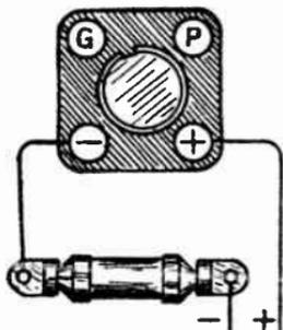
FIG. 1.—Filament Resistor.
