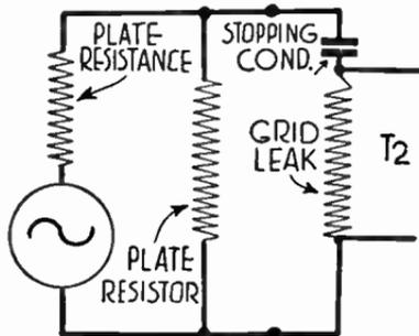
FIG. 3.—Condenser and Grid Leak in Series.
