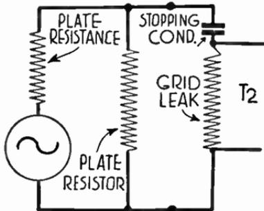
FIG. 3.—Condenser and Grid Leak in Series.
