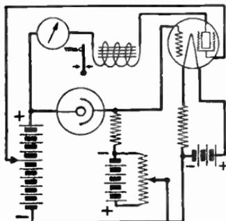
FIG. 14.—Screen Grid Amplifier for Phototube.
