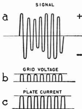
FIG. 4.—How the Limiter Affects a Strong Signal.
