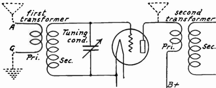
FIG. 1.—Antenna Connections for Testing Radio Stages.
