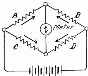
FIG. 5.—Balancing Principle of the Wheatstone Bridge.
