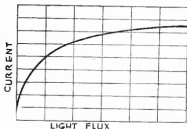
Fig. 3.—Current-illumination Characteristic of Photoconductive Cell.
