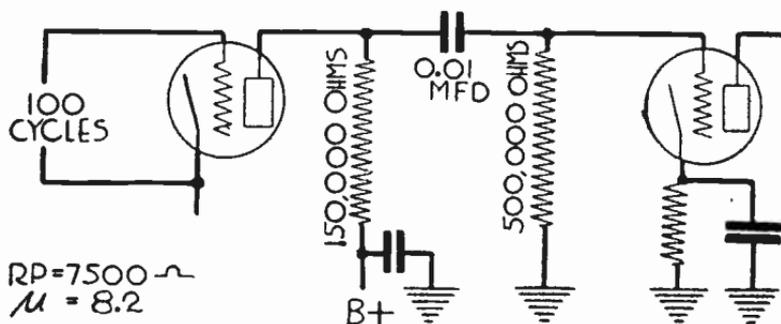
FIG. 5.—Typical Values for Resistance Coupling.
