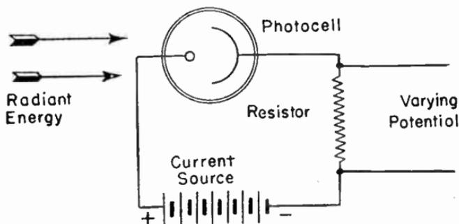
FIG. 3.—The Basic Phototube Circuit.
