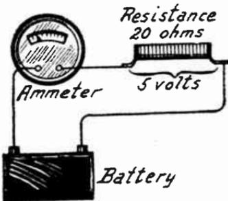
FIG. 2.—Determining Voltage Drop with Ohm's Law.
