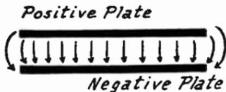
FIG. 1.—Electrostatic Field between Condenser Plates.
