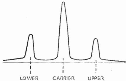
FIG. 8.—Side Frequencies and Carrier Frequency.
