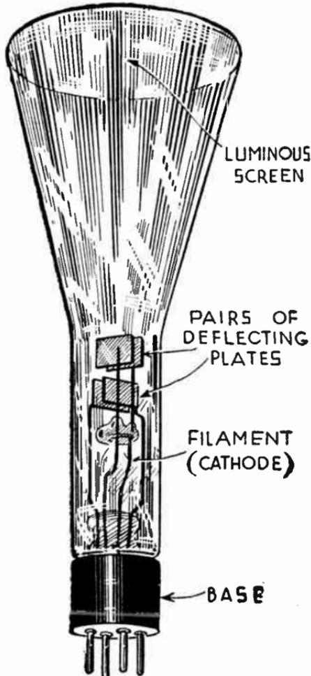
FIG. 1.—A Cathode-ray Tube.
