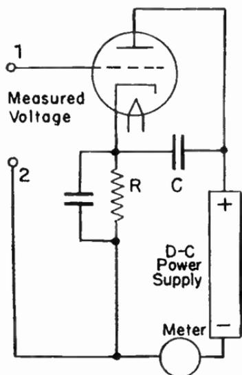
FIG. 1.—Plate Current Detector Used as VT Voltmeter.
