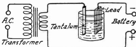
Tantalum Electrolytic Rectifier for Battery Charging.
