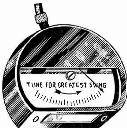
FIG. 11.—Reversed Scale Meter Tuning Indicator
