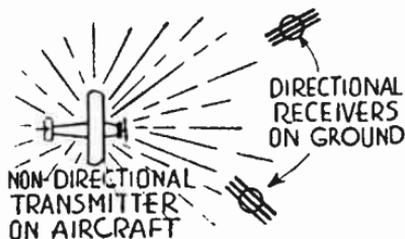
FIG. 2.—Airplane Transmitter and Ground Receivers.
