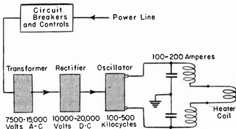
FIG. 5.—Principal Parts of an Induction Heating System.
