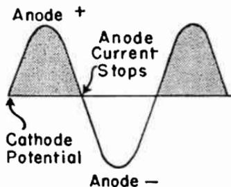
FIG. 5.—Anode Current Flows Only During Positive Half-cycles.
