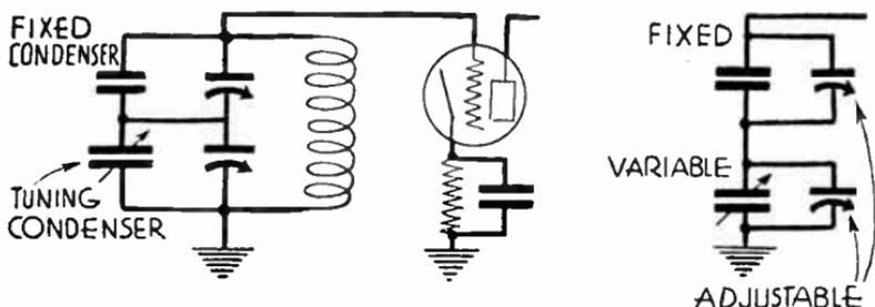
FIG. 21.—Arrangement of Capacities for Oscillator Tuning
