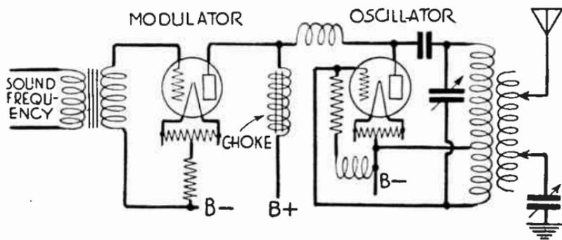
FIG. 6.—Connection of Modulator to Oscillator.
