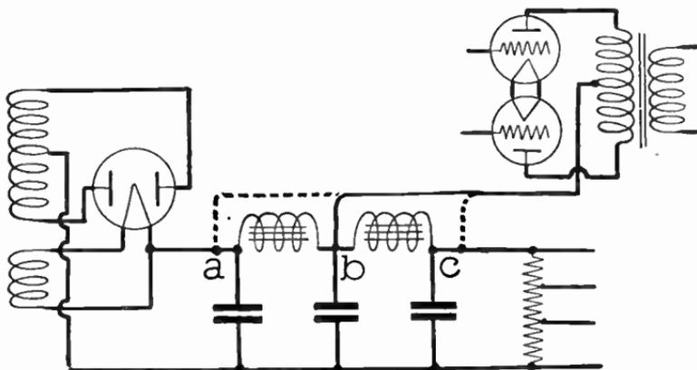
FIG. 7.—Connections of Plate Circuit to Filter.
