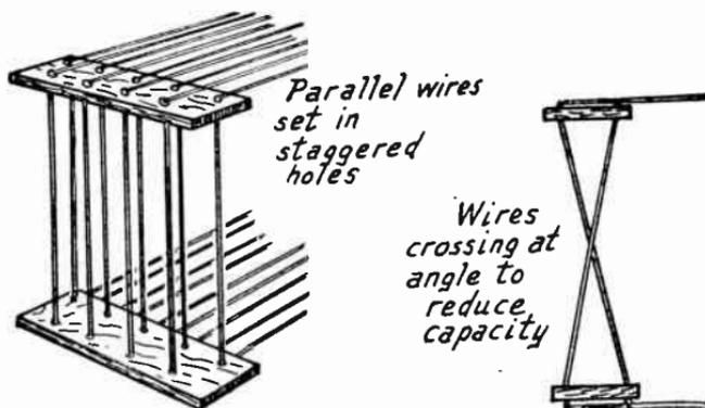
Arrangement of Wire on Loop Framework.
