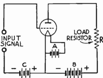
B.—Circuit Connections for Class A Operation.
